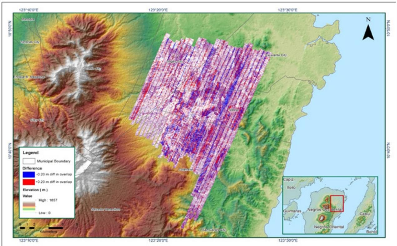
Figure A-8.14 Elevation difference between flight lines
