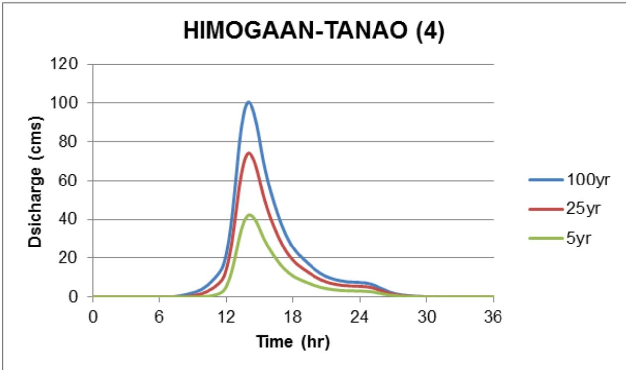
Figure 67. Himogaan and Tanao river (4) generated discharge using 5-, 25-, and 100-year Iloilo and Mactan stations' rainfall intensity-duration-frequency (RIDF) in HEC-HMS
