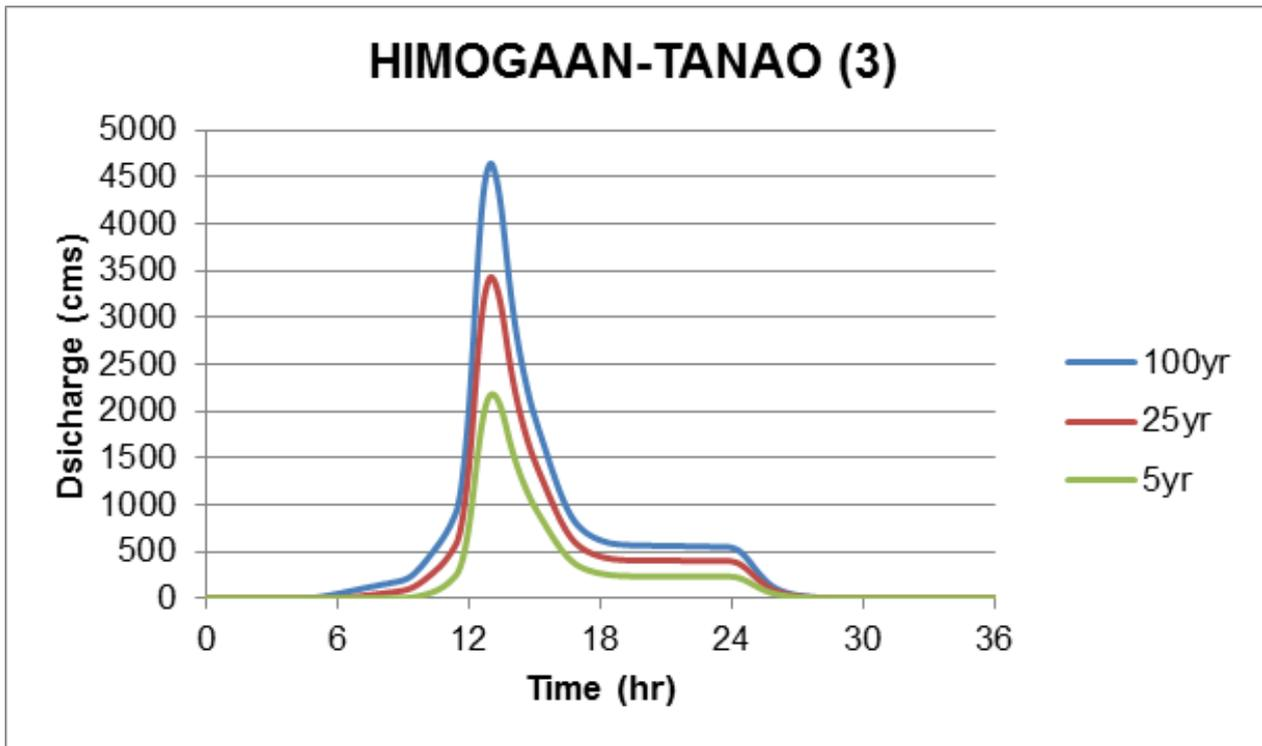
Figure 66. Himogaan and Tanao river (3) generated discharge using 5-, 25-, and 100-year Iloilo and Mactan stations' rainfall intensity-duration-frequency (RIDF) in HEC-HMS
