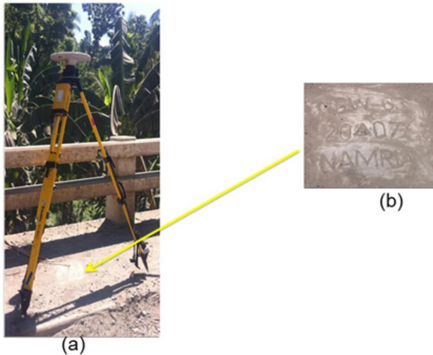
Figure 7. GPS set-up over NGW-63 at the NE end of the sidewalk of Daan-Lunsod Bridge at Brgy. Lemery, Calatrava, Negros Occidental (a) and NAMRIA reference point NGW-63 (b) as recovered by the field team.
