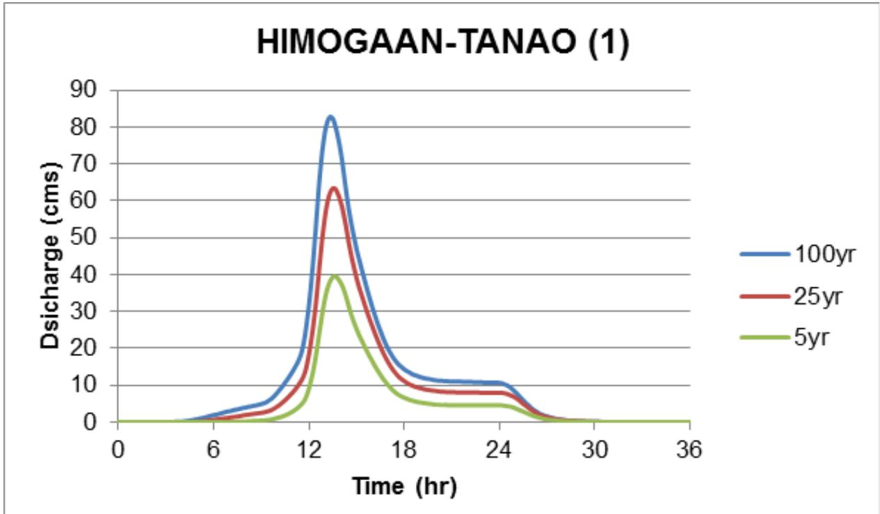
Figure 64. Himogaan and Tanao river (1) generated discharge using 5-, 25-, and 100-year Iloilo and Mactan stations' rainfall intensity-duration-frequency (RIDF) in HEC-HMS
