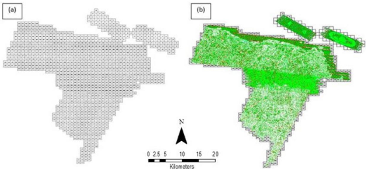
Figure 19. The coverage of the Tanao Floodplain Survey (a) the tile system (b) depicts the classification results in TerraScan.
