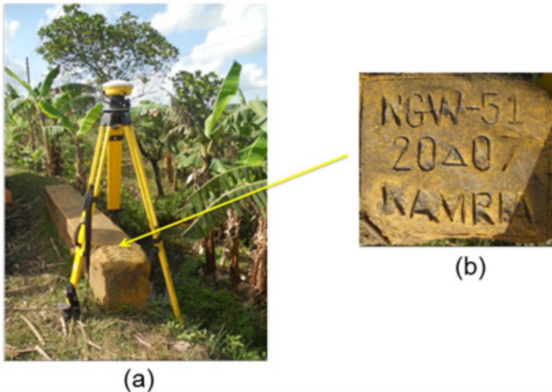
Figure 5. GPS set-up over NGW-51 at the NW tip of a yellow headwall found at the SW of Escalante-Bacolod national road at Brgy. Had Fe, Escalante, Negros Occidental (a) and NAMRIA reference point NGW-51 (b) as recovered by the field team.
