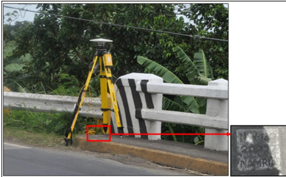
Figure 36. The GNSS (Trimble® SPS 852) receiver occupation, at NW-130 in Troso Bridge, Brgy. Daga, Cadiz City, Negros Occidental
