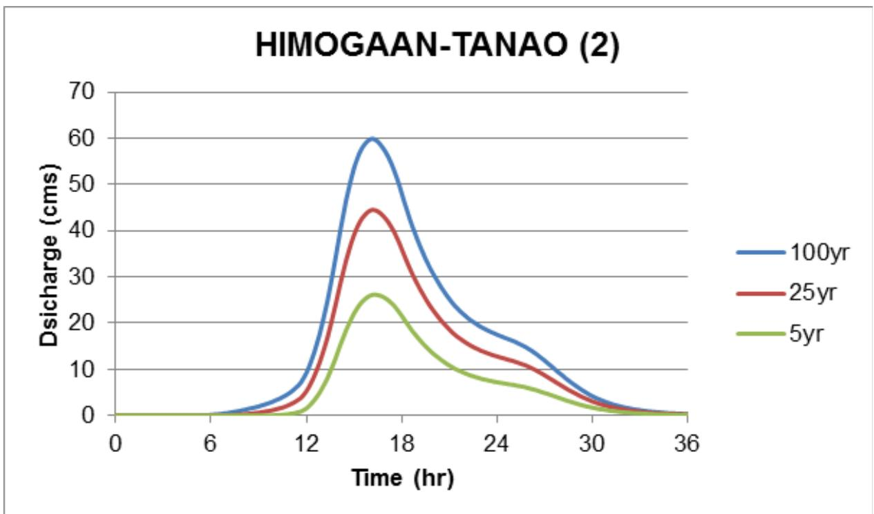
Figure 65. Himogaan and Tanao river (2) generated discharge using 5-, 25-, and 100-year Iloilo and Mactan stations' rainfall intensity-duration-frequency (RIDF) in HEC-HMS
