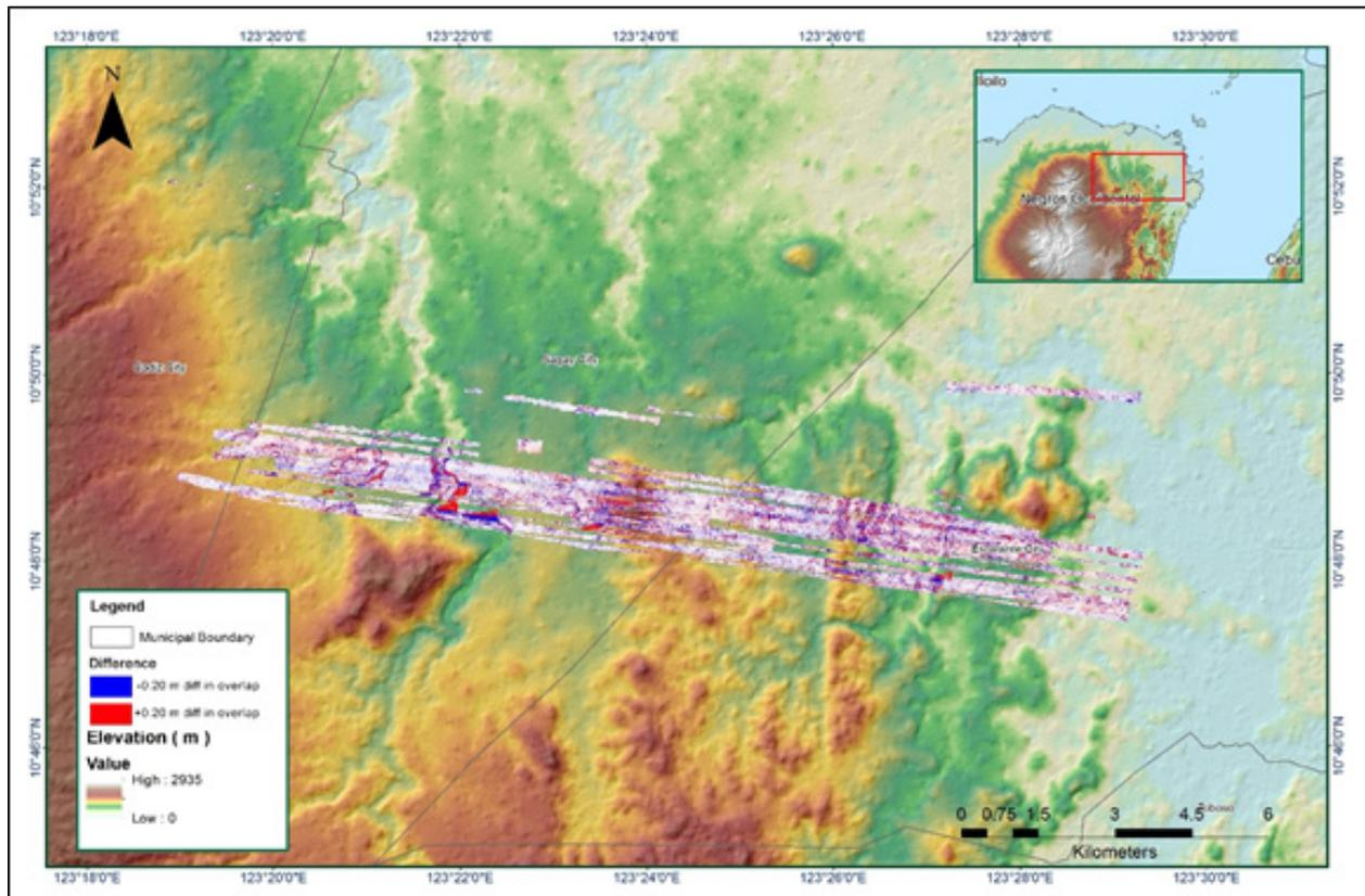
Figure A-8.28 Elevation difference between flight lines
