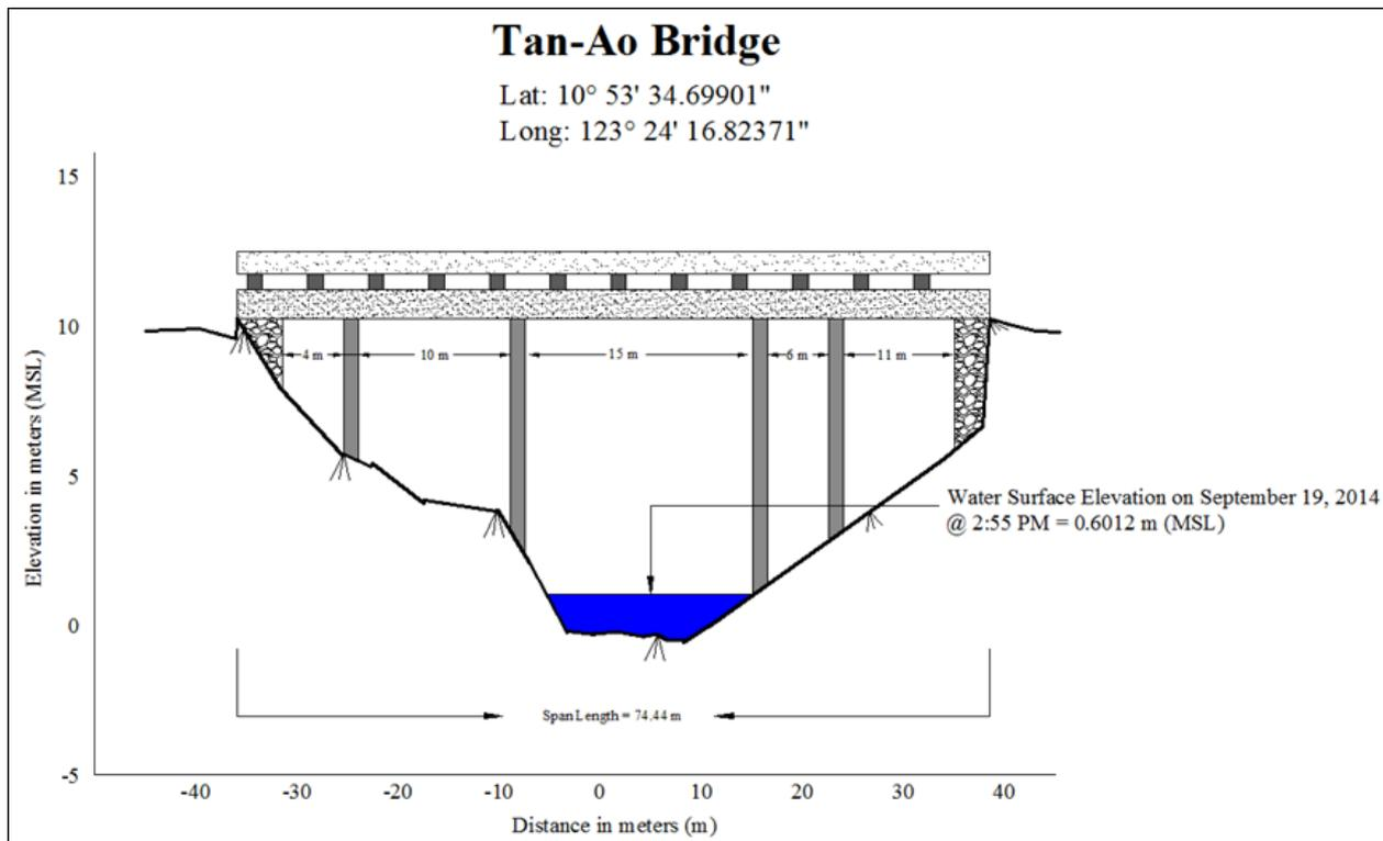
Figure 38. The Tan-ao Bridge cross-section survey drawn to scale
