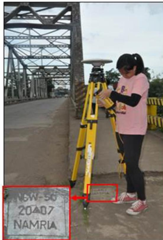
Figure 34. The GNSS base receiver setup, Trimble® SPS 852, at NGW-50 in Himoga-An Bridge, Brgy. Paraiso, Sagay City, Negros Occidental
