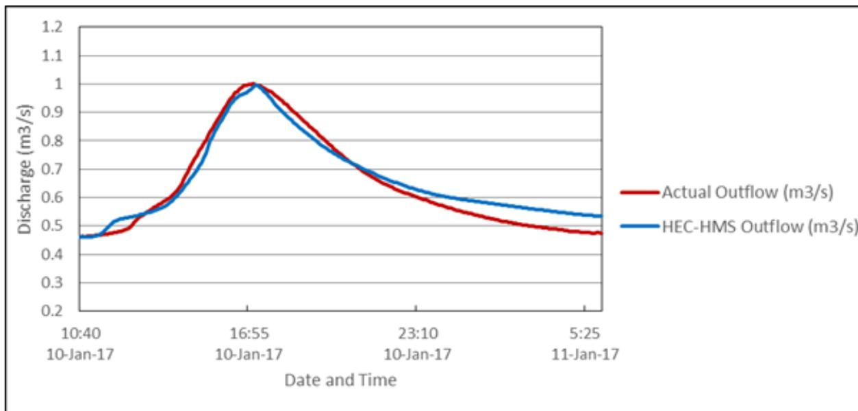
Figure 62. Outflow Hydrograph of Tanao produced by the HEC-HMS model compared with observed outflow
