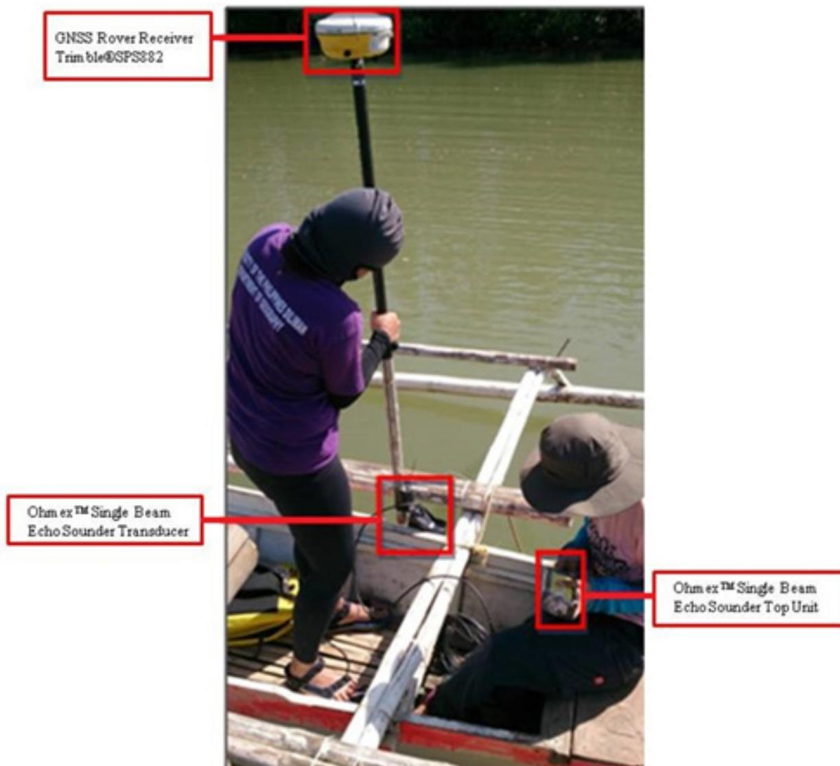
Figure 44. Set up of Ohmex™ Single Beam Echo Sounder integrated with a roving GNSS receiver on a motor boat for the bathymetric survey in Brgy. Old Sagay, Sagay City, Negros Occidental
