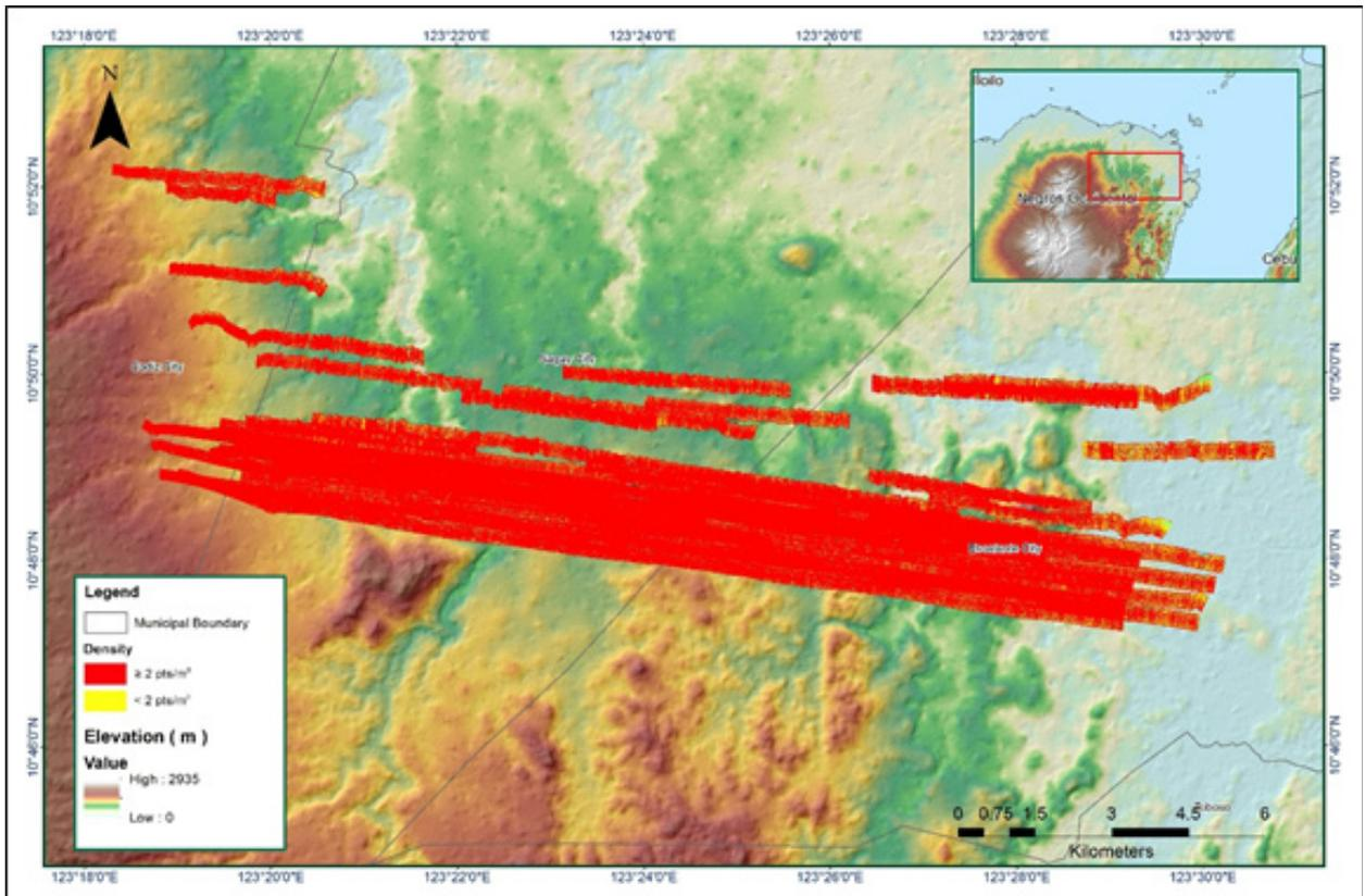
Figure A-27 Density map of merged LiDAR data
