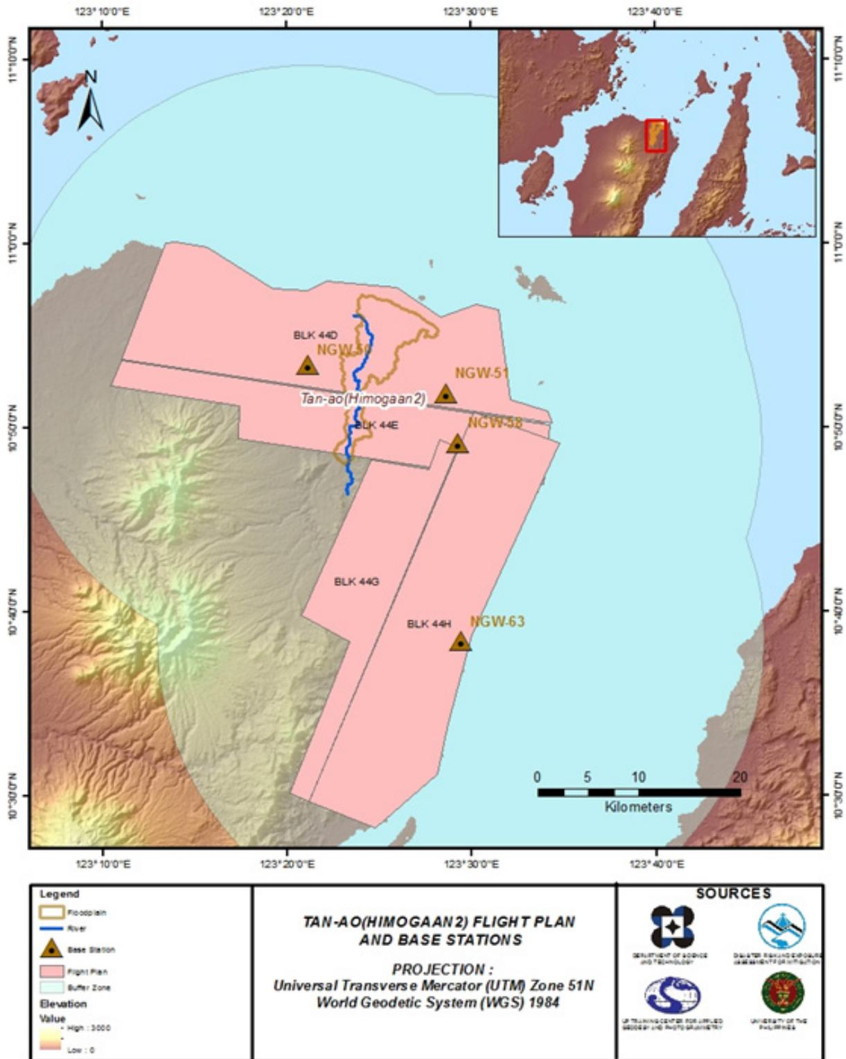
Figure 3. Flight Plan and base stations used for the Tanao Floodplain survey using Pegasus sensor.
