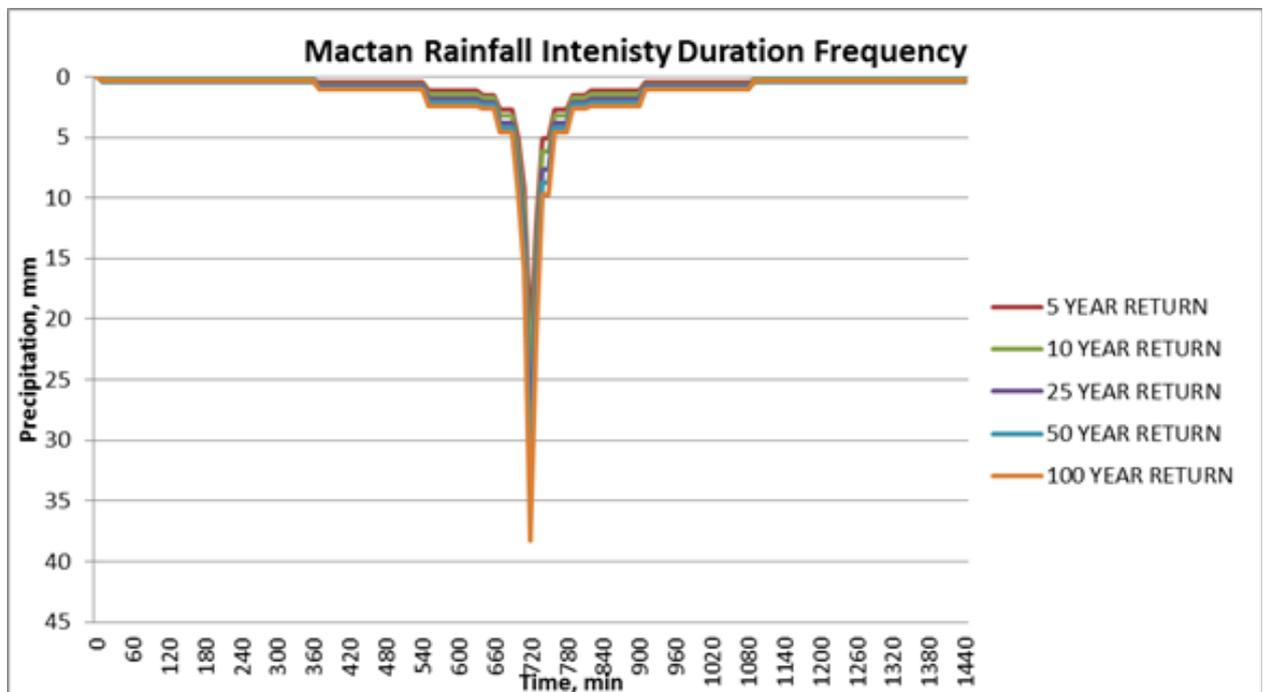
Figure 52. Synthetic storm generated for a 24-hour period rainfall for various return periods
