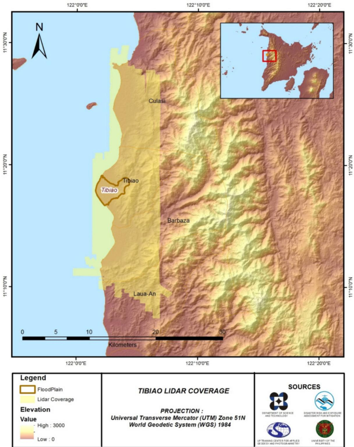
Figure 5. Actual LiDAR survey coverage of the Tibiao Floodplain.
