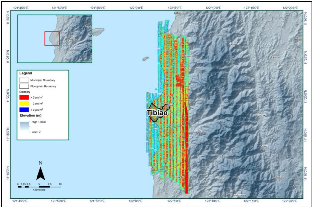
Figure 12. Pulse density map of merged LiDAR data for Tibiao Floodplain.
