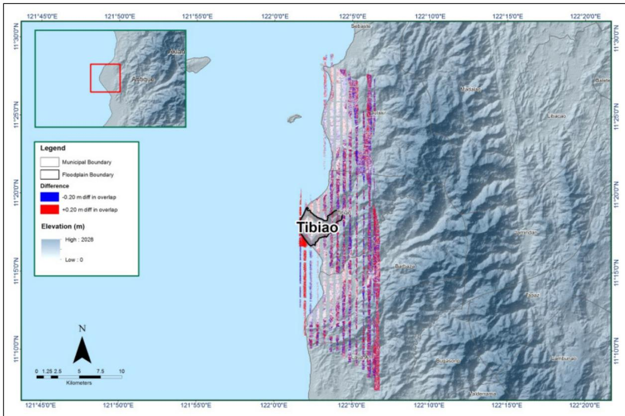
Figure 13. Elevation Difference Map between flight lines for Tibiao Floodplain Survey.
