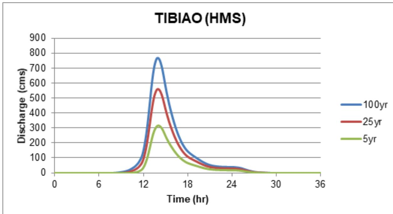
Figure 59. Tibiao river (1) generated discharge using 5-, 25-, and 100-year Iloilo and Mactan stations’ rainfall intensity-duration-frequency (RIDF) in HEC-HMS
