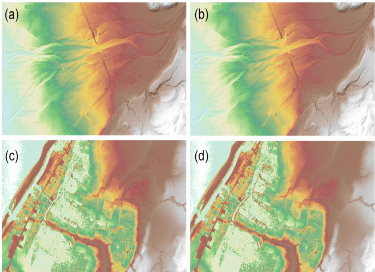
Figure 20. Portions in the DTM of Tibiao Floodplain – bridges before (a) and after (b) manual editing; paddy fields before (c) and after (d) data retrieval
