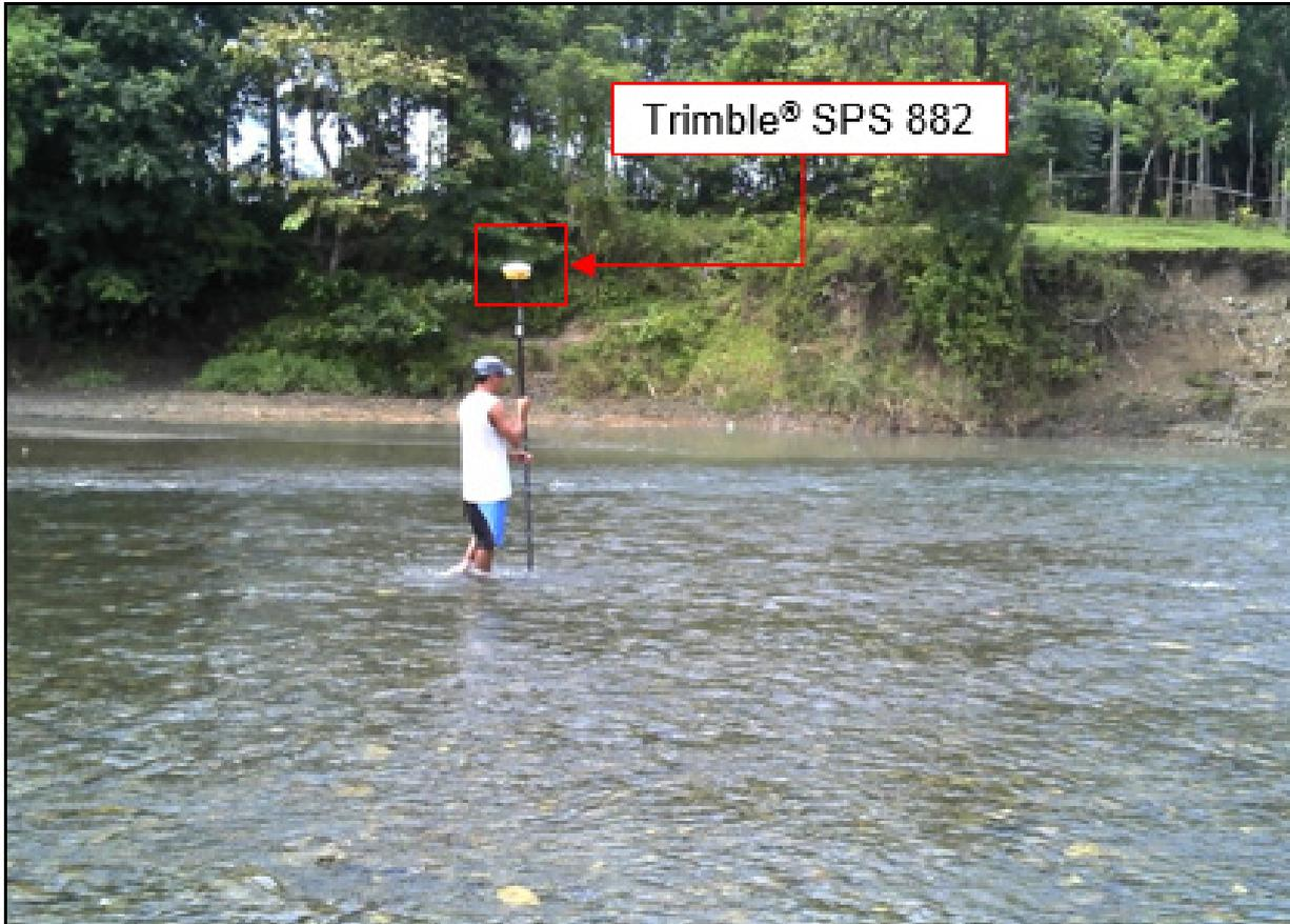
Figure 39. Manual bathymetric survey along Tibiao River
