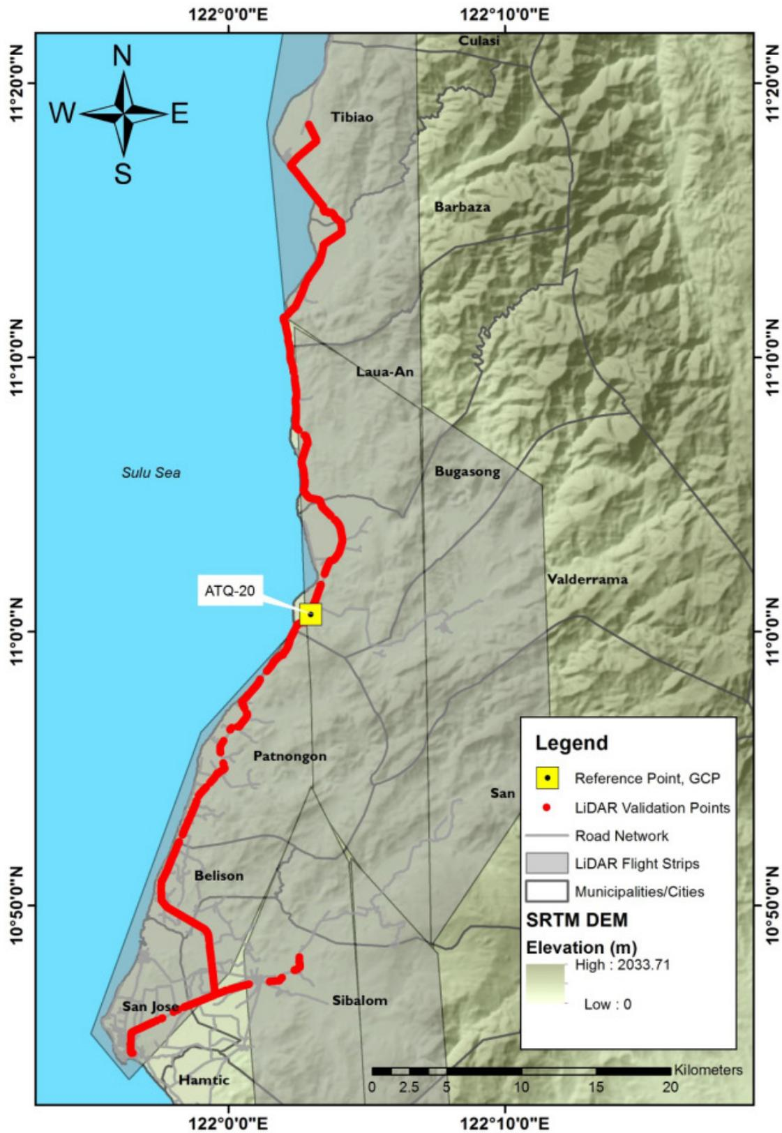
Figure 38. Validation point acquisition survey of Tibiao River basin
