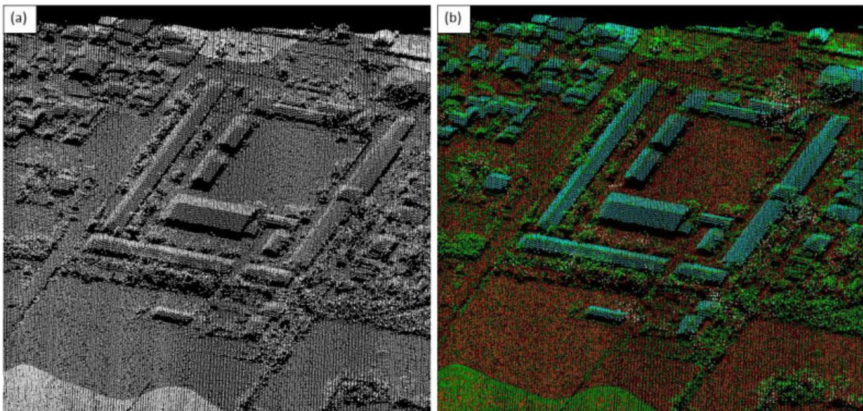
Figure 16. Point cloud before (a) and after (b) classification
