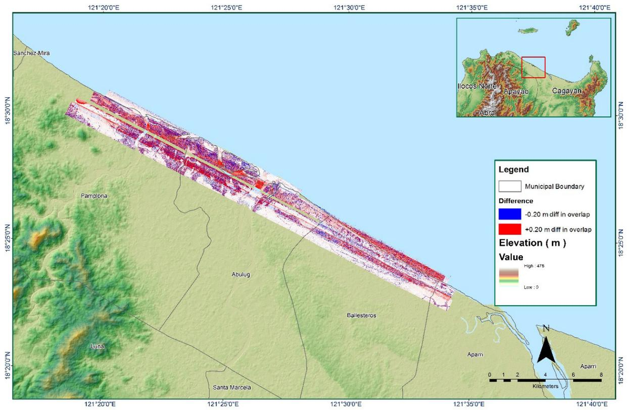
Figure A-8.49. Elevation difference between flight lines
