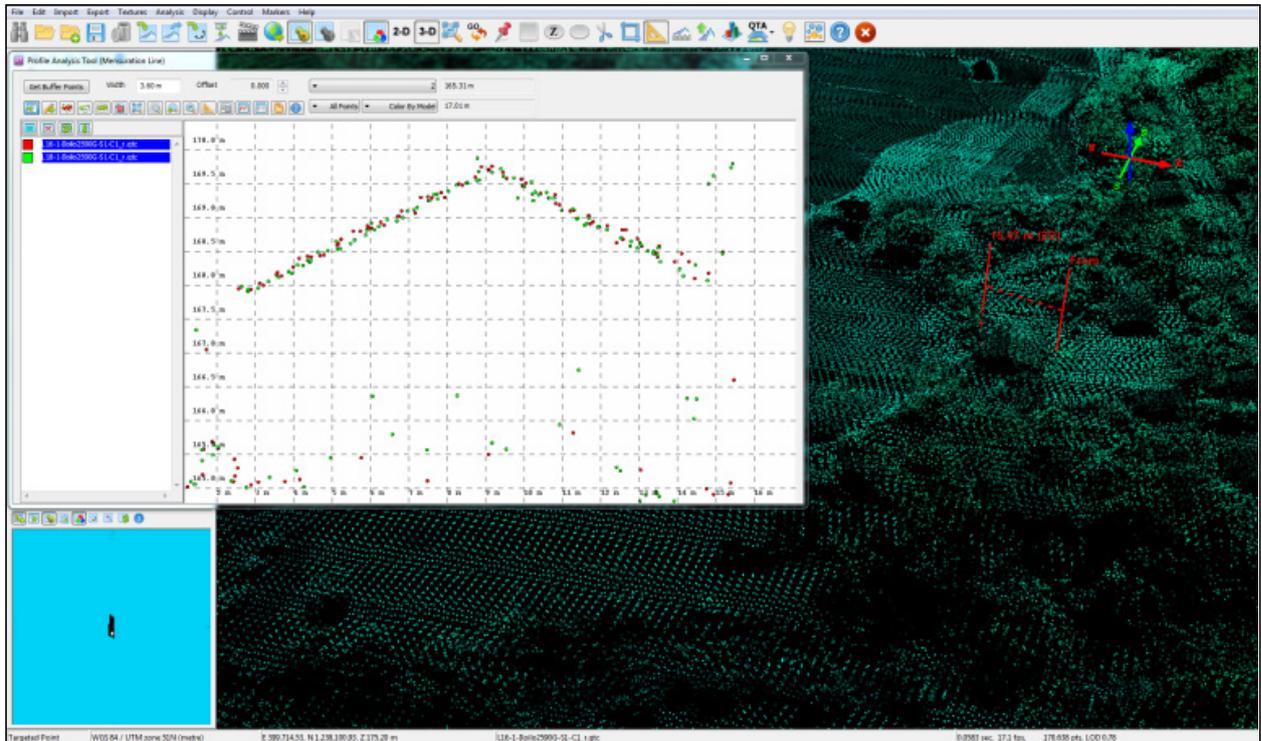
Figure 14. Quality checking for a Tibiao flight 2590G using the Profile Tool of QT Modeler
