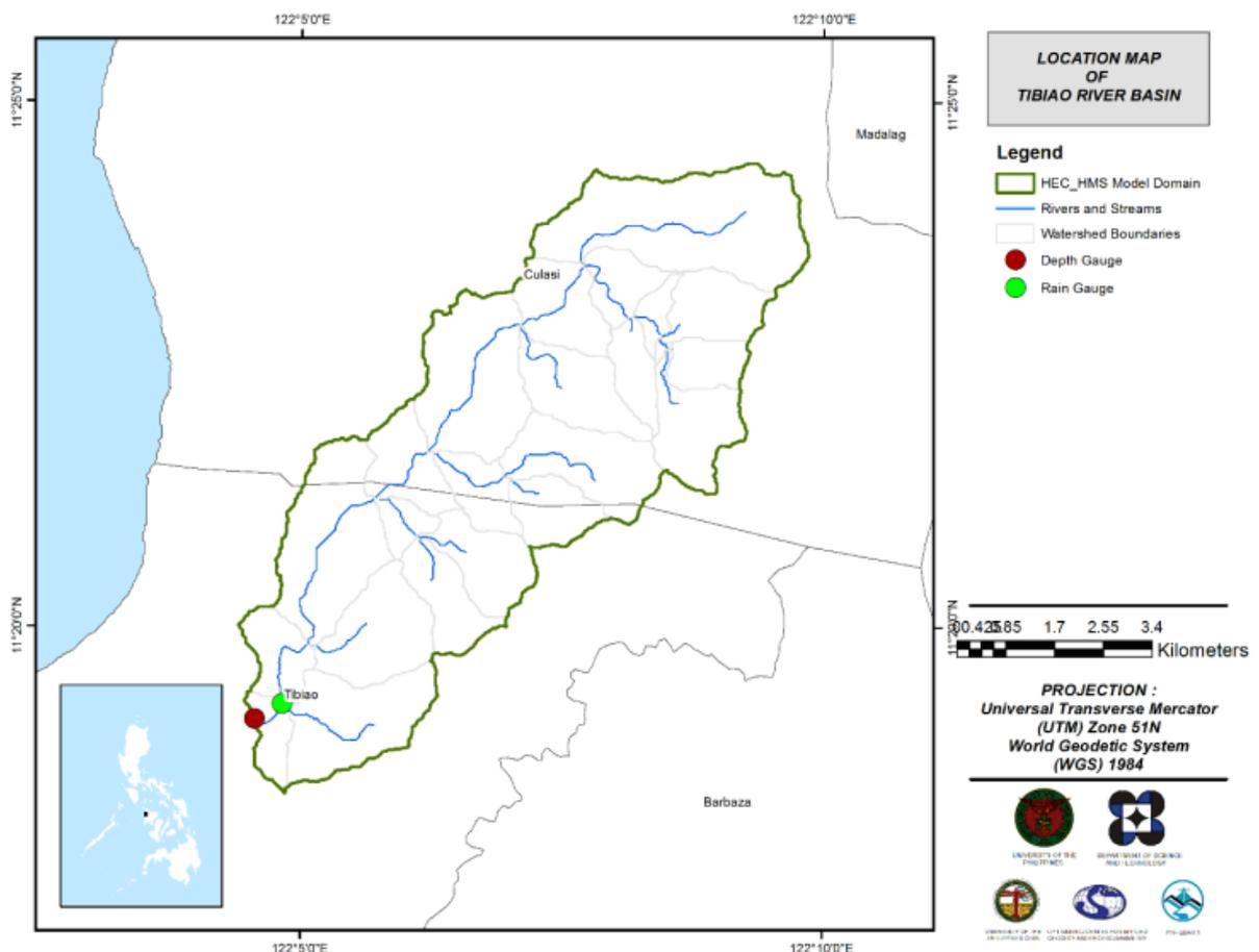
Figure 42. Location map of the Tibiao HEC-HMS model used for calibration.
