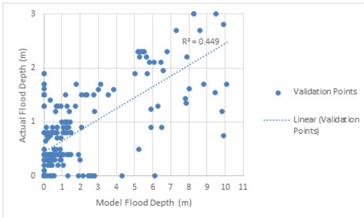
Figure 71. Flood map depth vs. actual flood depth
