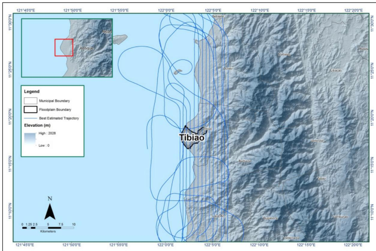
Figure 9. Best estimated trajectory of the LiDAR missions conducted over the Tibiao Floodplain.
