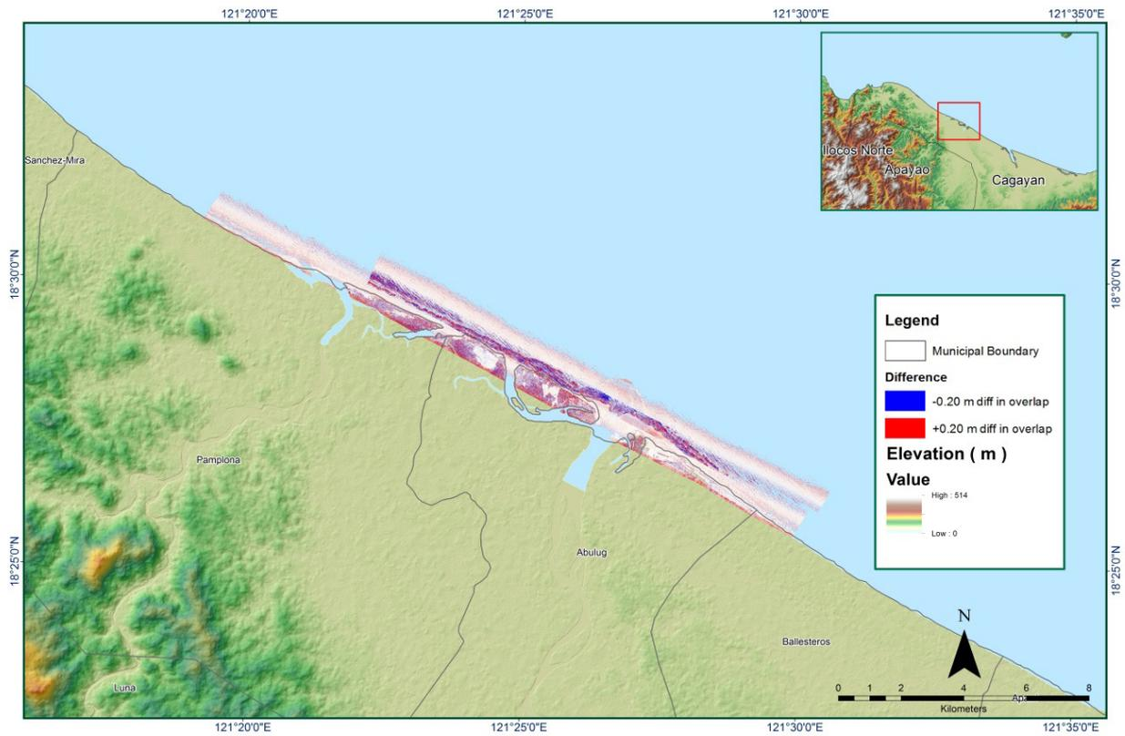
Figure A-8.63. Elevation difference between flight lines
