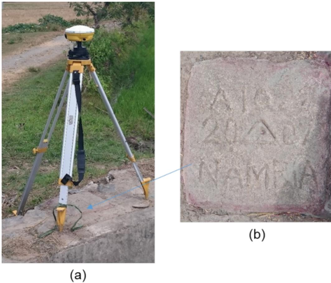
Figure 4. GPS set-up over ATQ-22 on an irrigation canal in Barangay Concepcion, Belison, Province of Antique (a) and NAMRIA reference point ATQ-22 (b) as recovered by the field team
