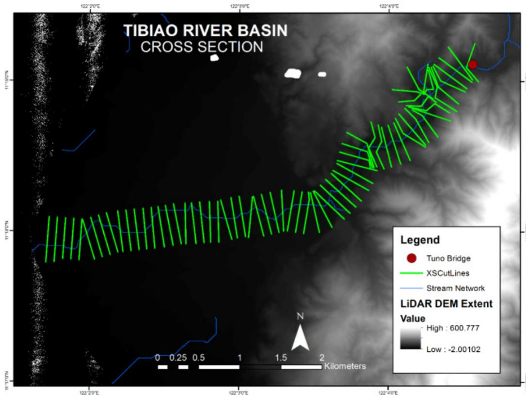
Figure 53. River cross-section of Tibiao River generated through Arcmap HEC GeoRAS tool
