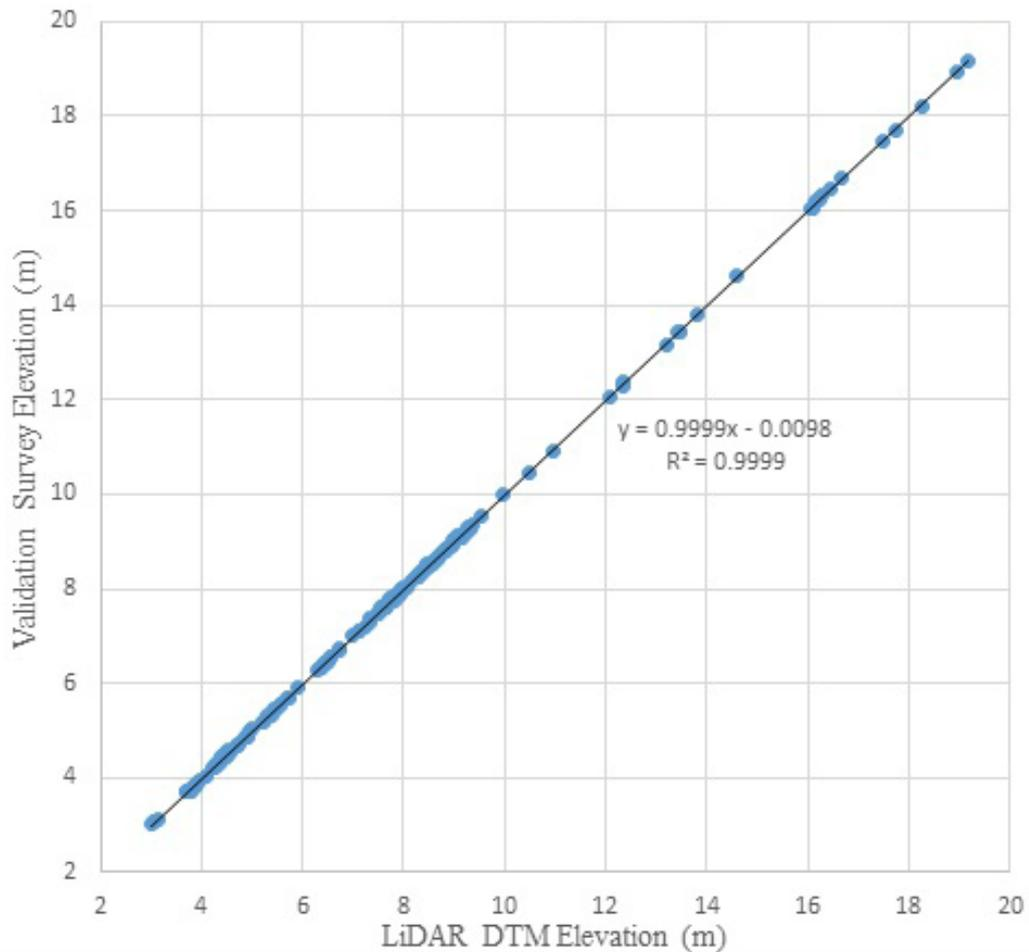
Figure 24. Correlation plot between validation survey points and LiDAR data.
