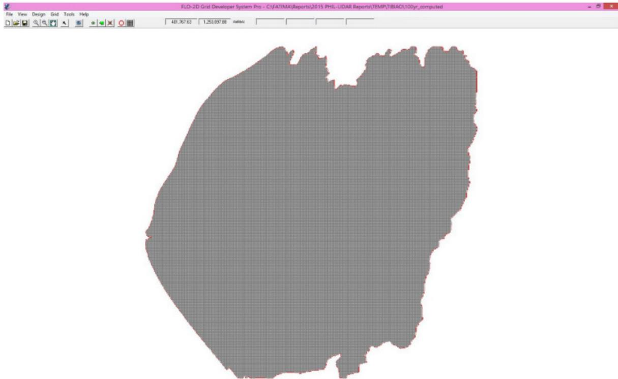
Figure 54. Screenshot of river sub-catchment with the computational area to be modeled in FLO-2D Grid Developer System Pro (FLO-2D GDS Pro)
