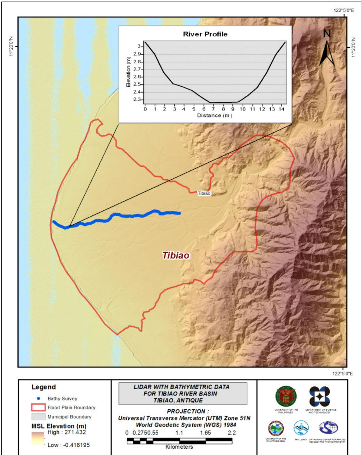
Figure 25. Map of Tibiao Floodplain with bathymetric survey points shown in blue.
