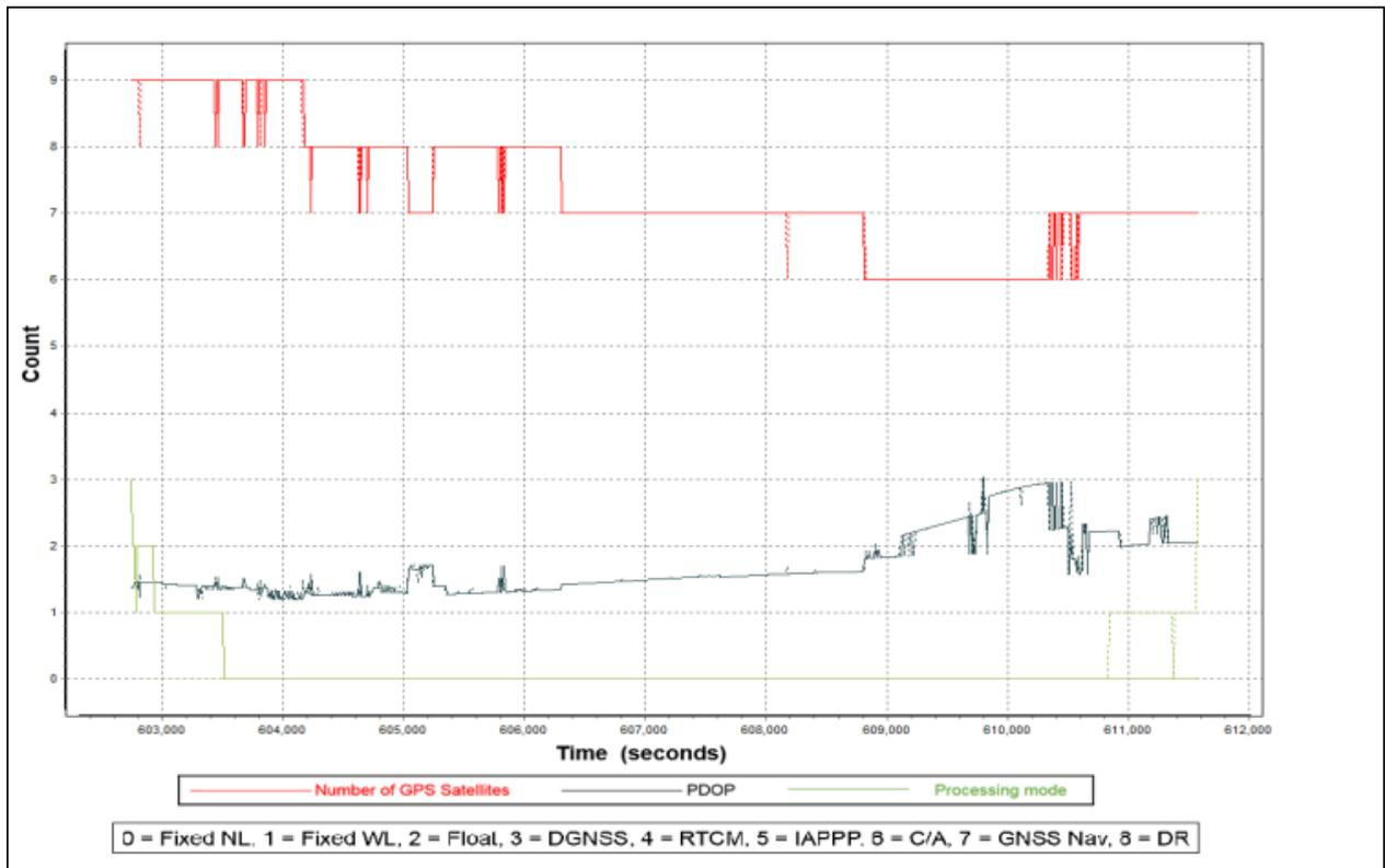
Figure 8. Solution Status Parameters of Tibiao Flight 2590G
