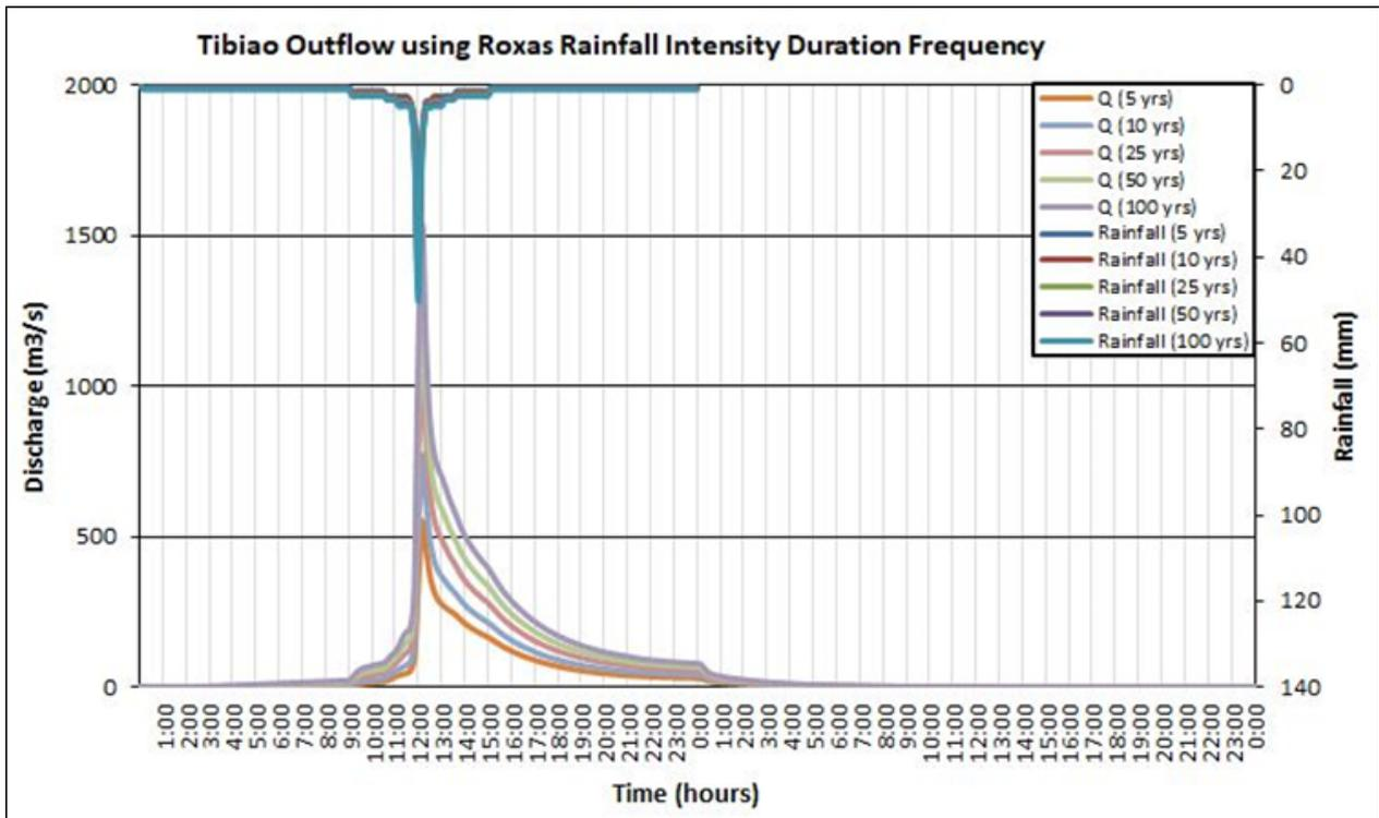
Figure 58. The Outflow hydrograph at Tibiao Station generated using Iloilo RIDF simulated in HEC-HMS
