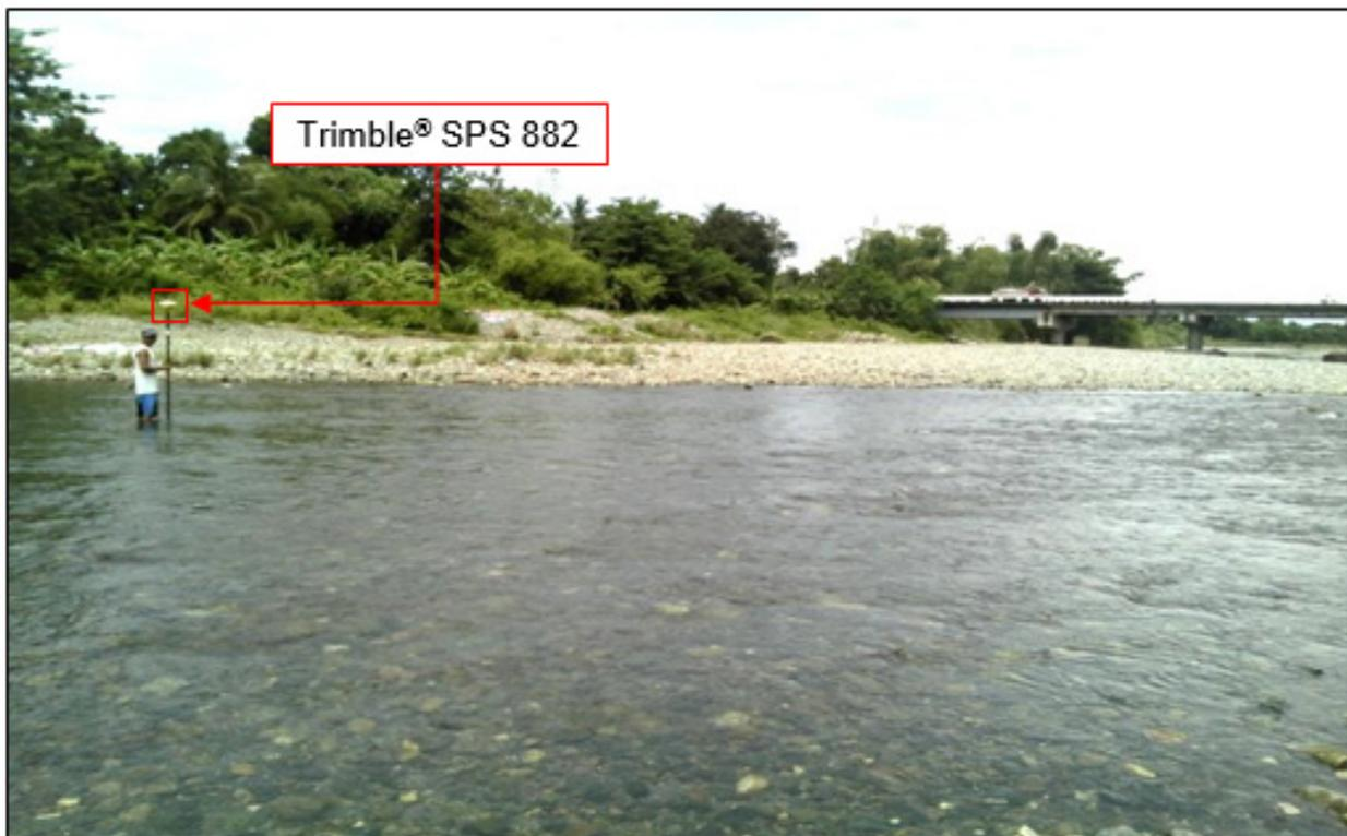
Figure 33. Cross-section survey across Tibiao River about 254 m downstream of Tibiao Bridge in Tibiao, Antique
