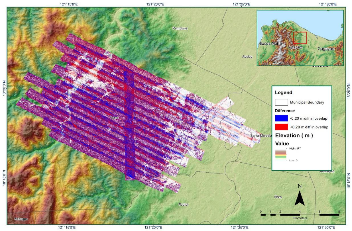
Figure A-8.7. Elevation difference between flight lines
