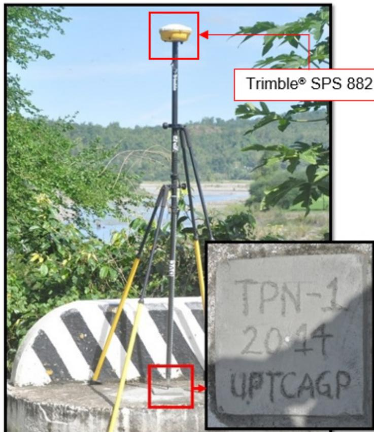
Figure 32. UP-TCAGP established control point, TPN-1, with Trimble® SPS 882 on Tipuluan Bridge in Brgy. Pasong, Municipality of Sibalom, Antique
