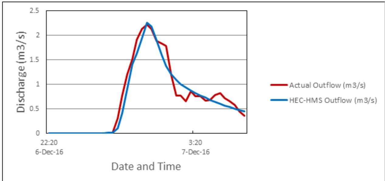
Figure 57. Outflow hydrograph of Tibiao produced by the HEC-HMS model compared with observed outflow
