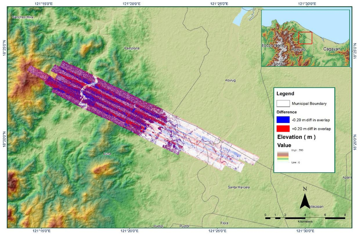
Figure A-8.28. Elevation difference between flight lines
