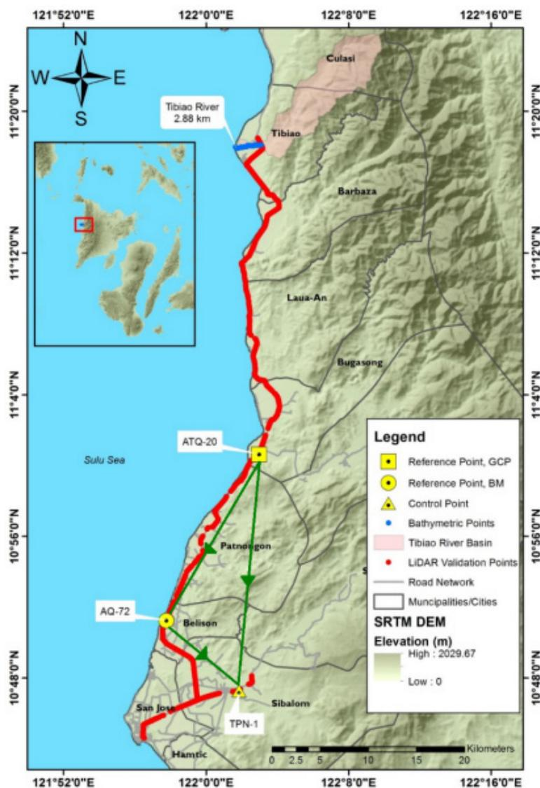
Figure 28. Extent of the bathymetric survey (in blue line) in Tibiao River and the LiDAR data validation survey (in red).
