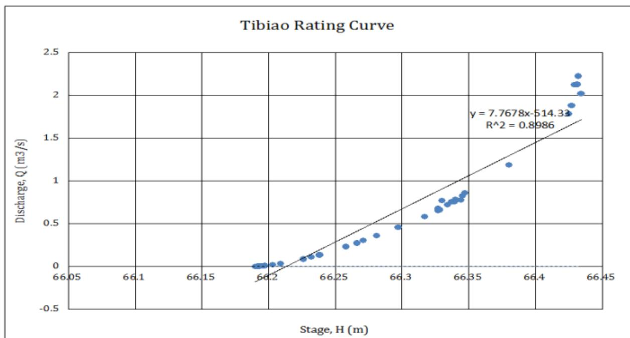
Figure 44. Rating curve at Tuno footbridge, Tibiao, Antique
