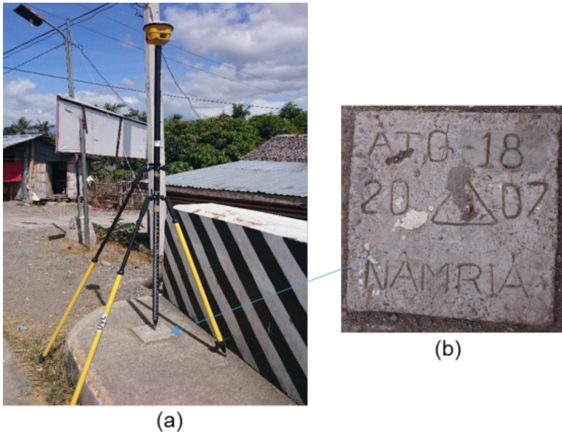
Figure 3. GPS set-up over ATQ-18 in Binangbang Bridge of Barangay Cubay, Barbaza, Province of Antique (a) and NAMRIA reference point ATQ-18 (b) as recovered by the field team
