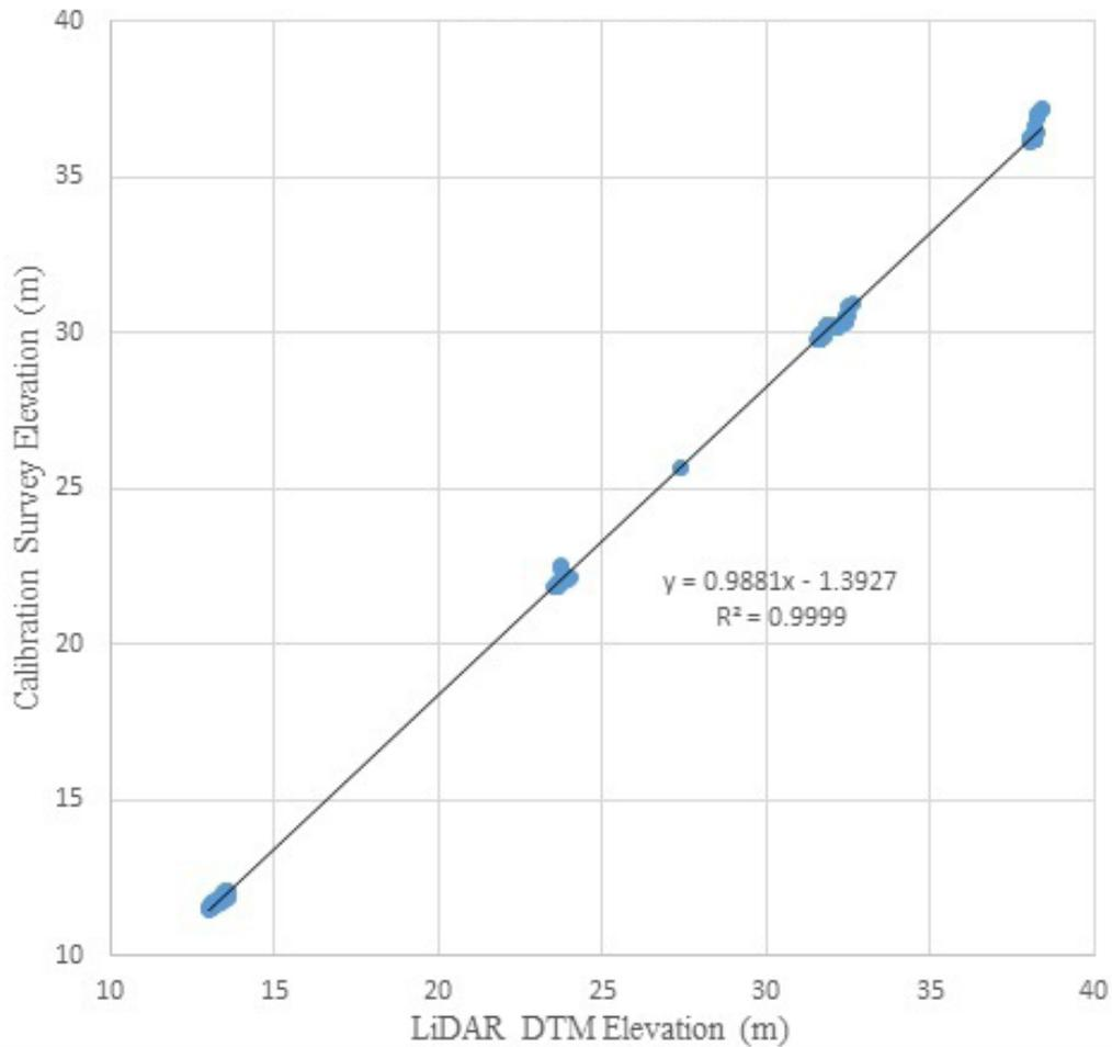
Figure 23. Correlation plot between calibration survey points and LiDAR data.
