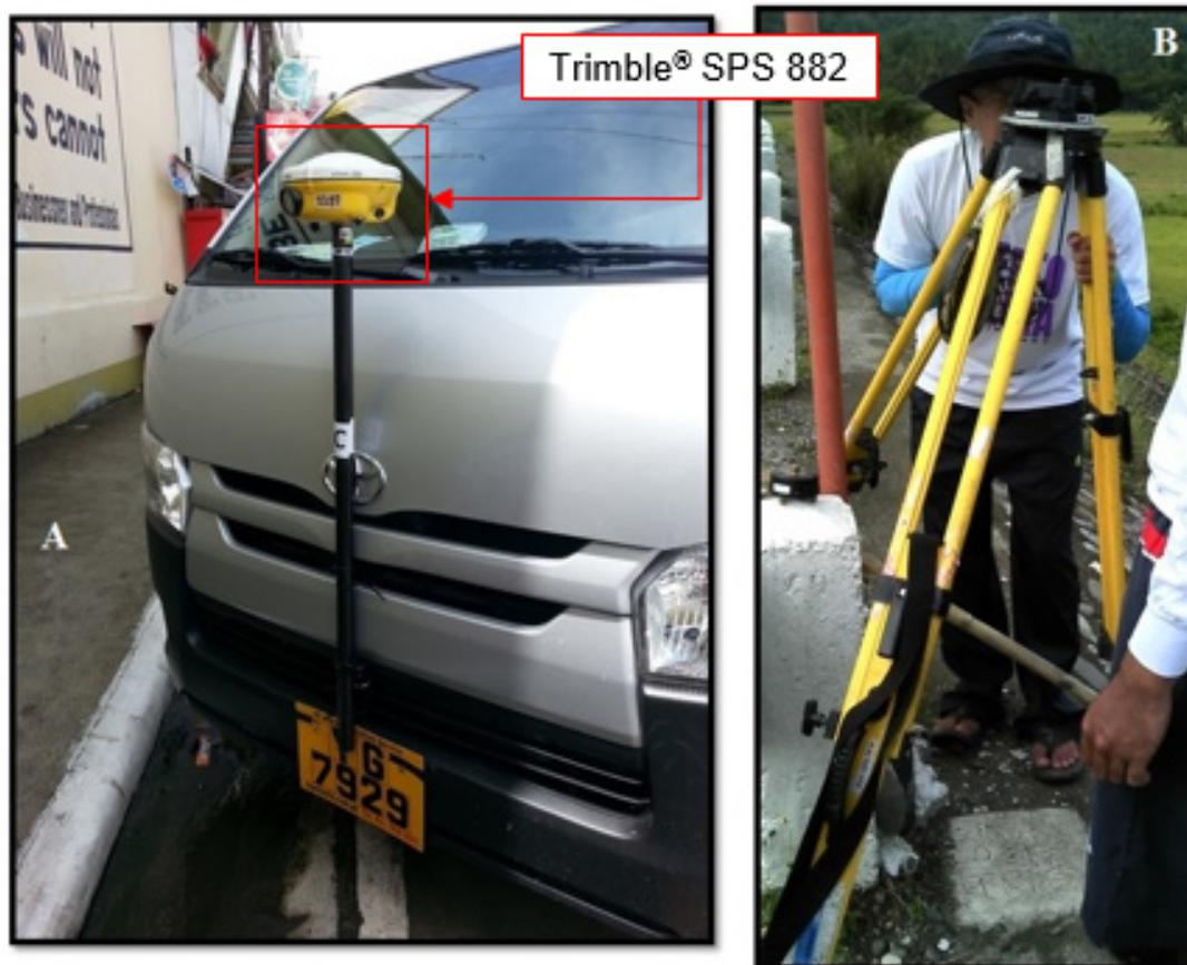
Figure 37 A) Setup of Trimble® SPS 882 in a van and (B) occupation of GNSS base station at ATQ-20
