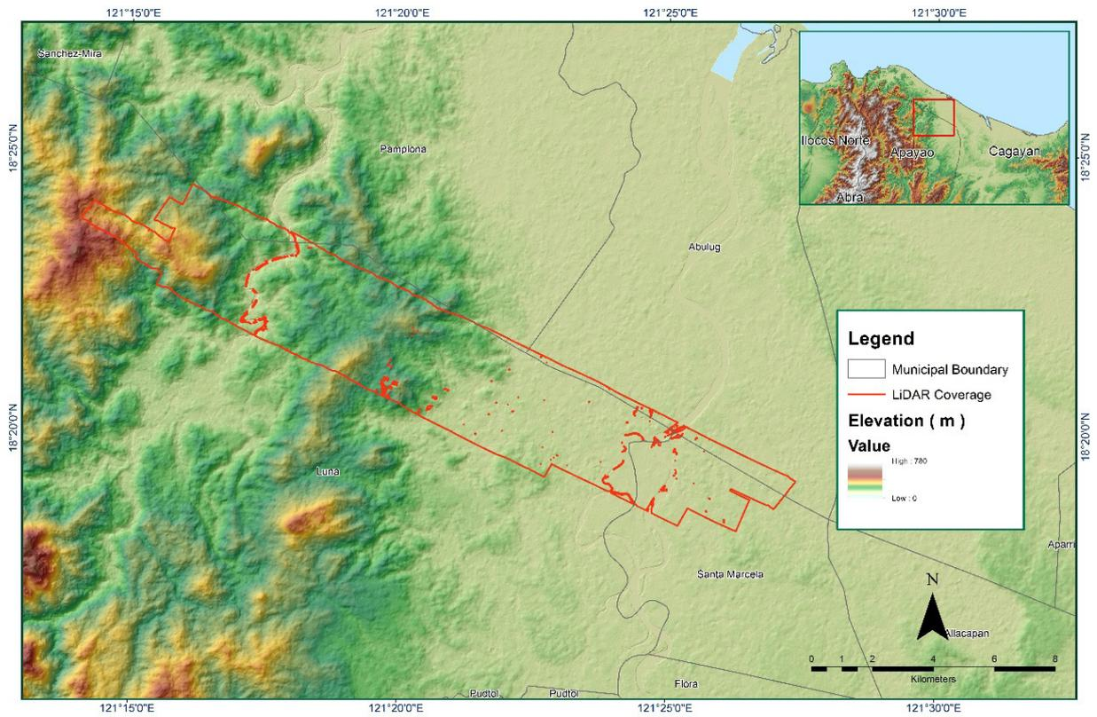
Figure A-8.25. Coverage of LiDAR data
