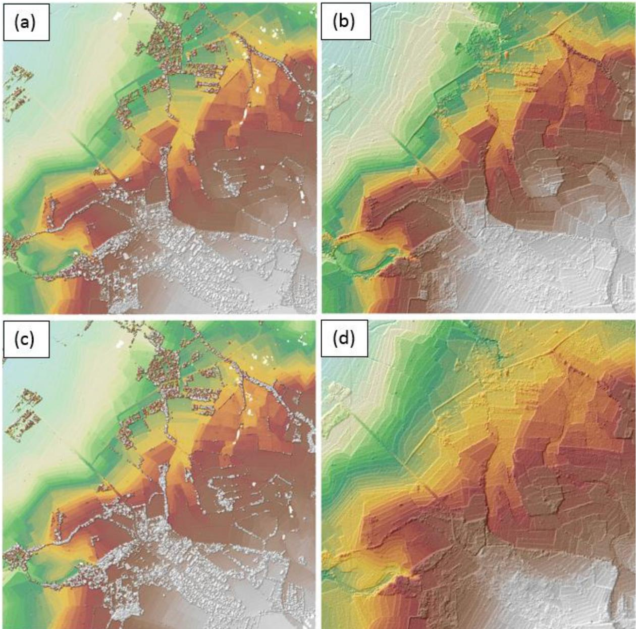
Figure 17. The production of last return DSM (a) and DTM (b), first return DSM (c) and secondary DTM (d) in some portion of Tibiao Floodplain.
