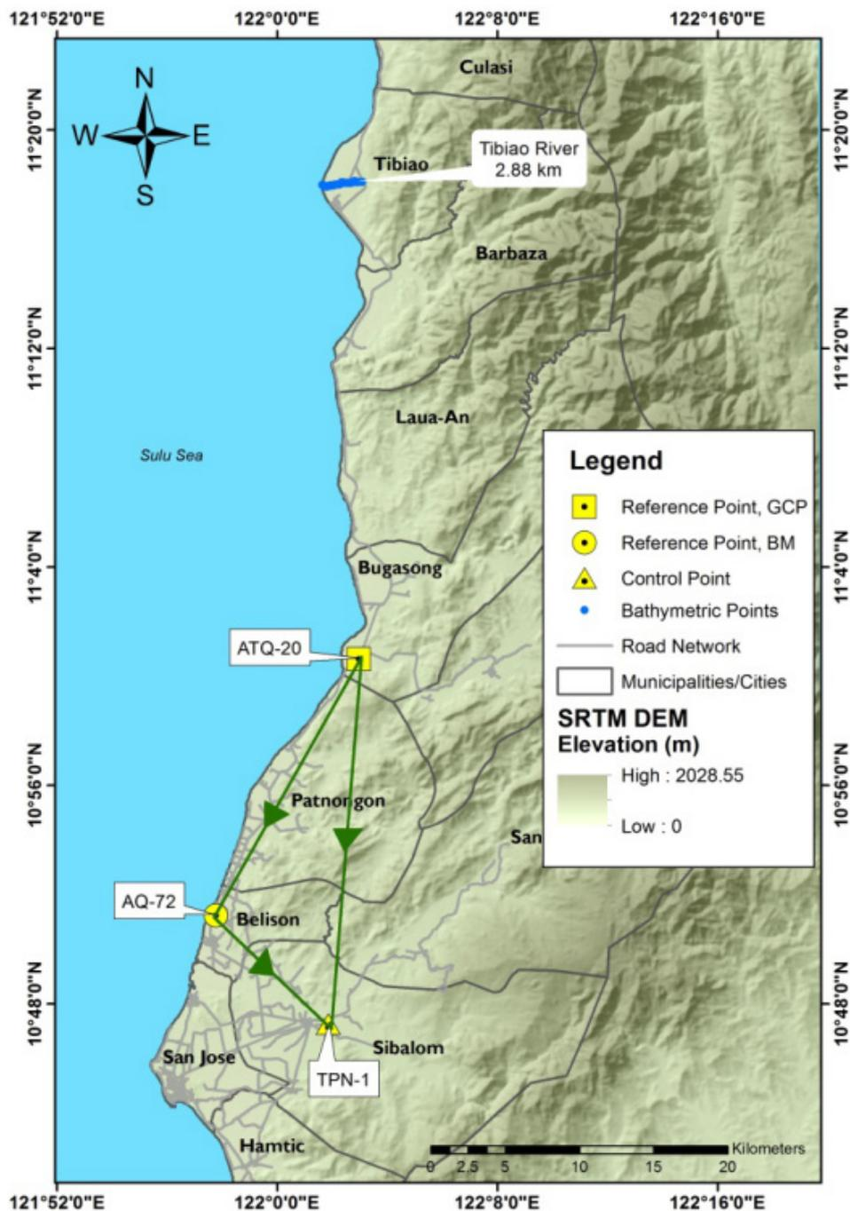
Figure 29. The GNSS Network established in the Tibiao River Survey.
