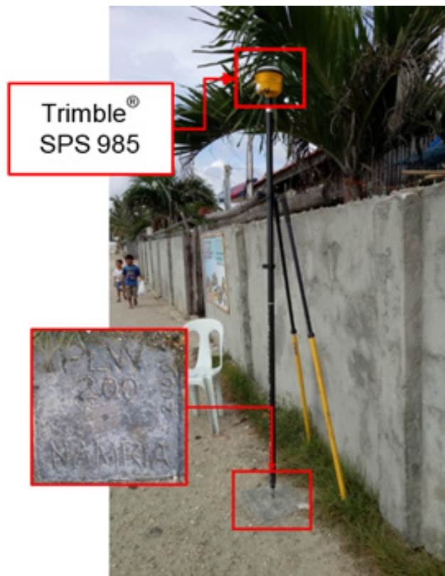
Figure 29. GNSS receiver setup, Trimble® SPS 985 at PLW-200, located along the shoreline in Brgy. 1 Poblacion, Municipality of Roxas, Palawan.
