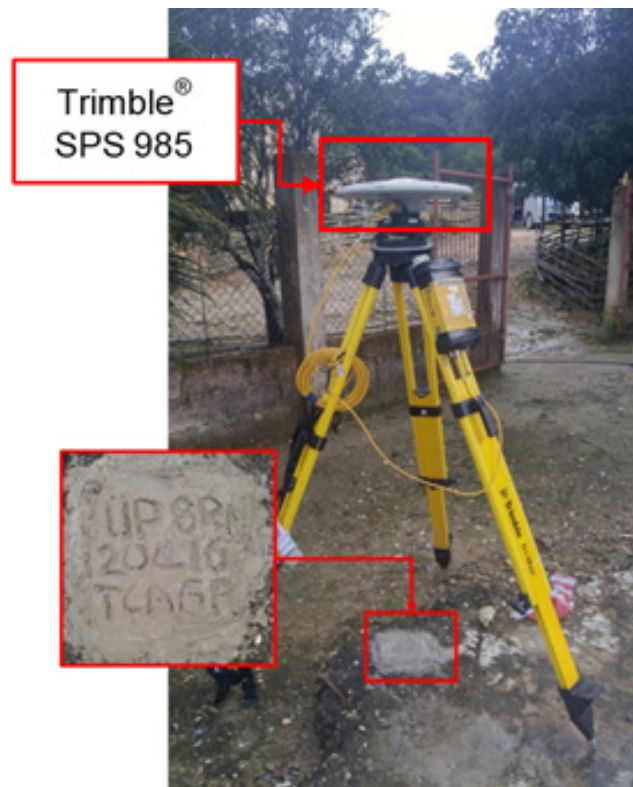
Figure 30. GNSS receiver setup, Trimble® SPS 852, at UP-BRN, located near Port Barton in Brgy. Port Barton, Municipality of San Vicente, Palawan.
