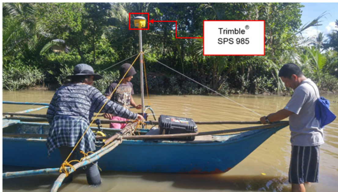
Figure 43. Set up of the bathymetric survey at Abongan River using Ohmex™ single beam echo sounder.
