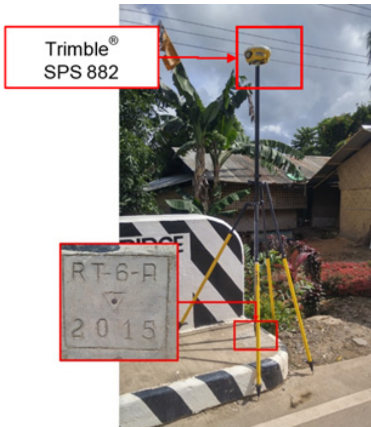
Figure 32. GNSS receiver setup, Trimble® SPS 882, at RT-6-A, located at the approach of Abongan Bridge in Brgy. Abongan, Municipality of Taytay, Palawan.
