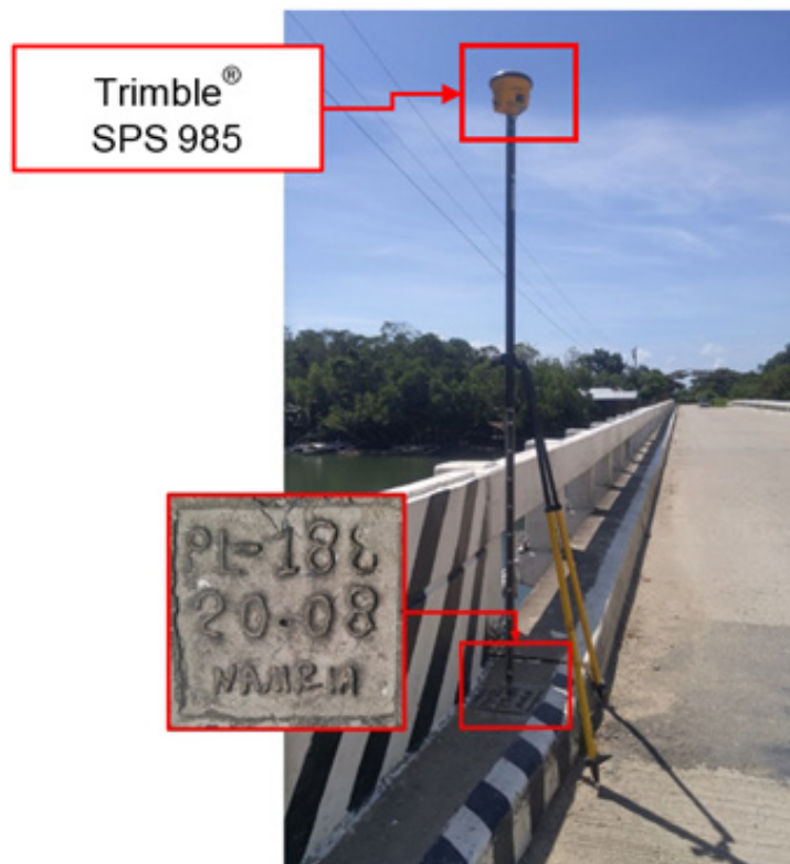
Figure 33. GNSS receiver setup, Trimble® SPS 985, at PL-188, located at the approach of Langan Bridge in Brgy. Langan, Puerto Prinsesa City, Palawan
