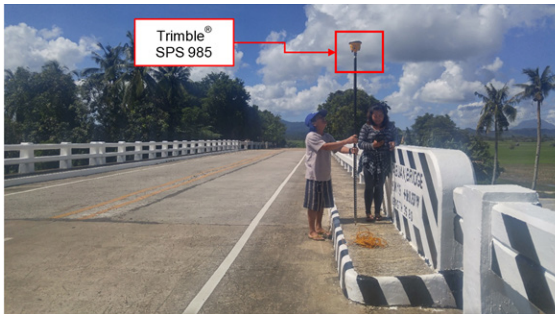
Figure 36. Bridge As-Built Survey using PPK Technique.
