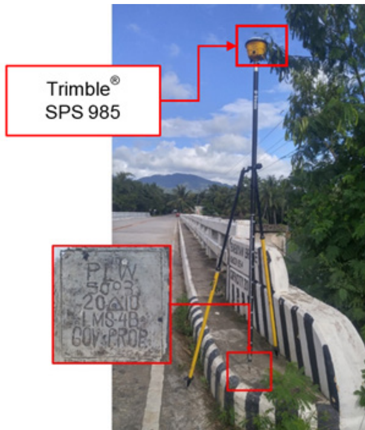
Figure 31. GNSS receiver setup, Trimble® SPS 985 at PLW-5093, located at the approach of Itabiak Bridge in Brgy. New Agutaya, Municipality of San Vicente, Palawan.
