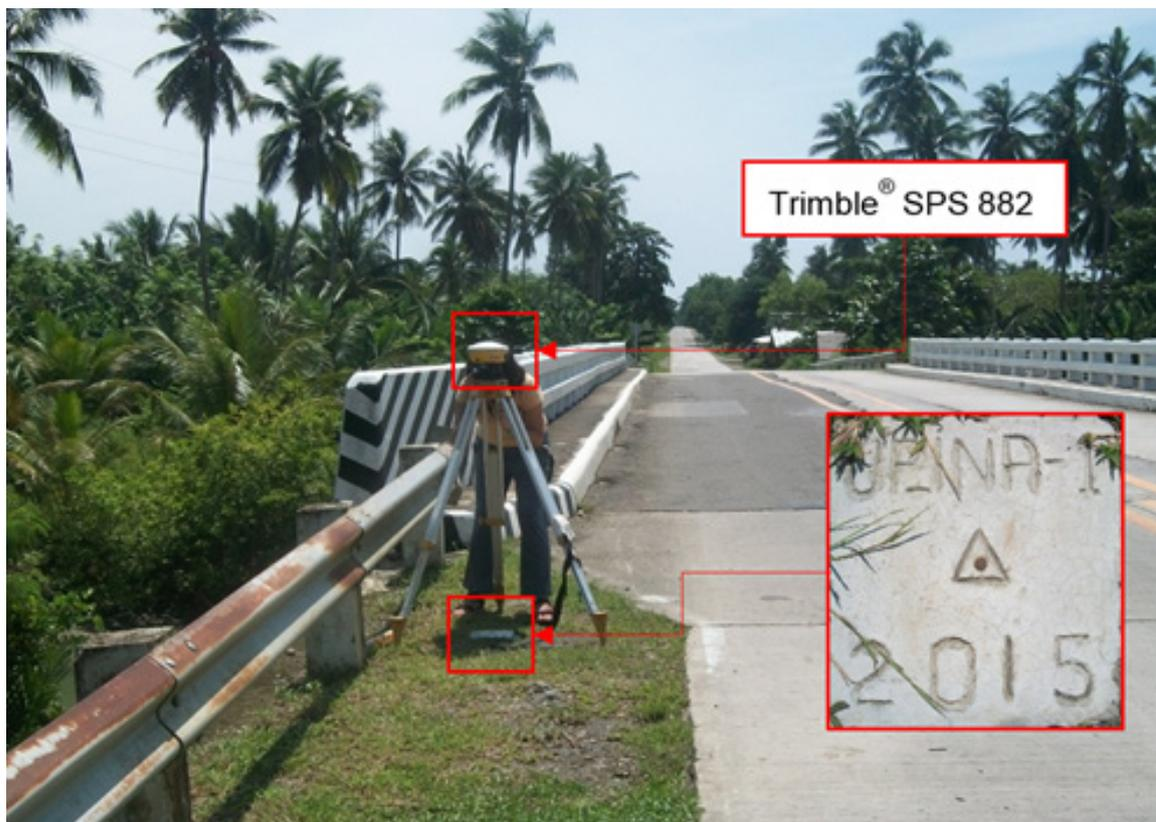
Figure 38. GNSS receiver set-up, Trimble® SPS 882, at UP\_INA-1, located beside the approach of Inagauan Bridge in Brgy. Inagauan Sub-Colony, Puerto Princesa City, Palawan.
