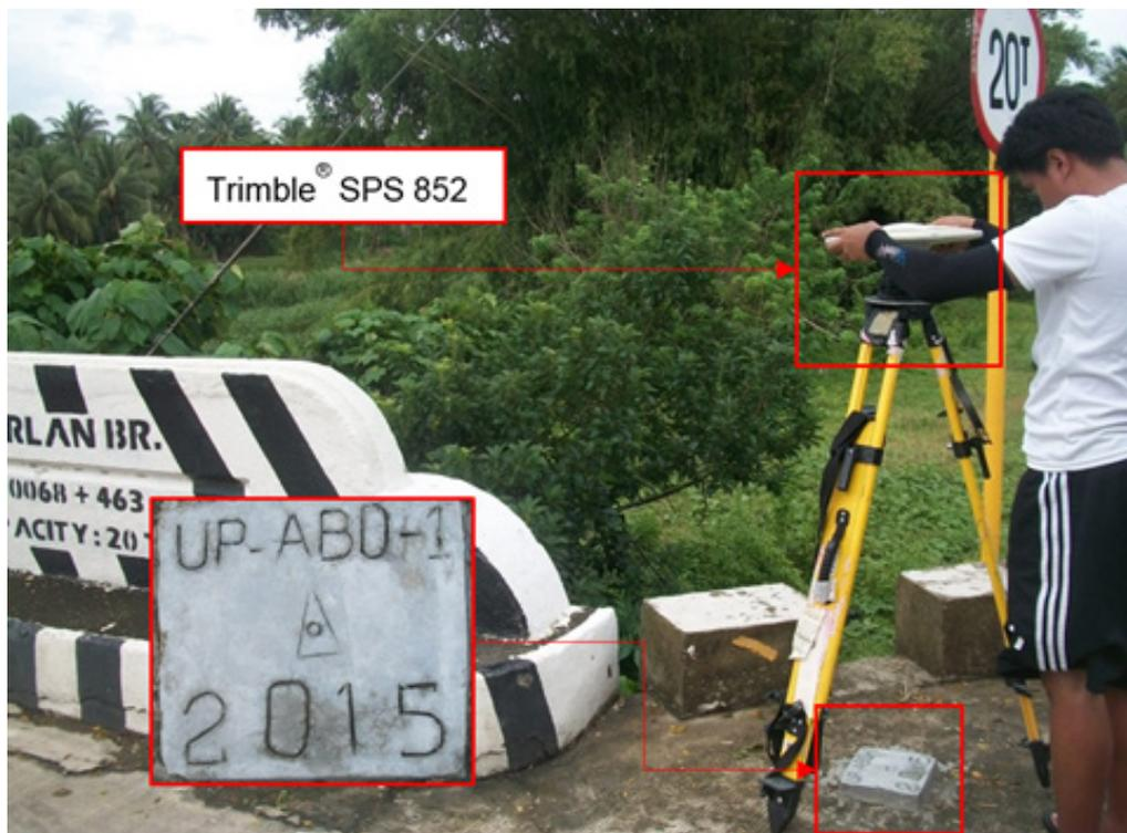
Figure 37. GNSS receiver set-up, Trimble® SPS 852, at UP\_ABO-1, an established control point, beside the approach of Aborlan Bridge in Brgy. Gogognan, Aborlan, Palawan.
