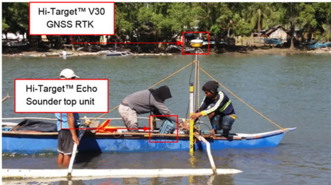
Figure 48. Bathymetric survey of ABSD at Aborlan River using Hi-Target™ Echo Sounder.
