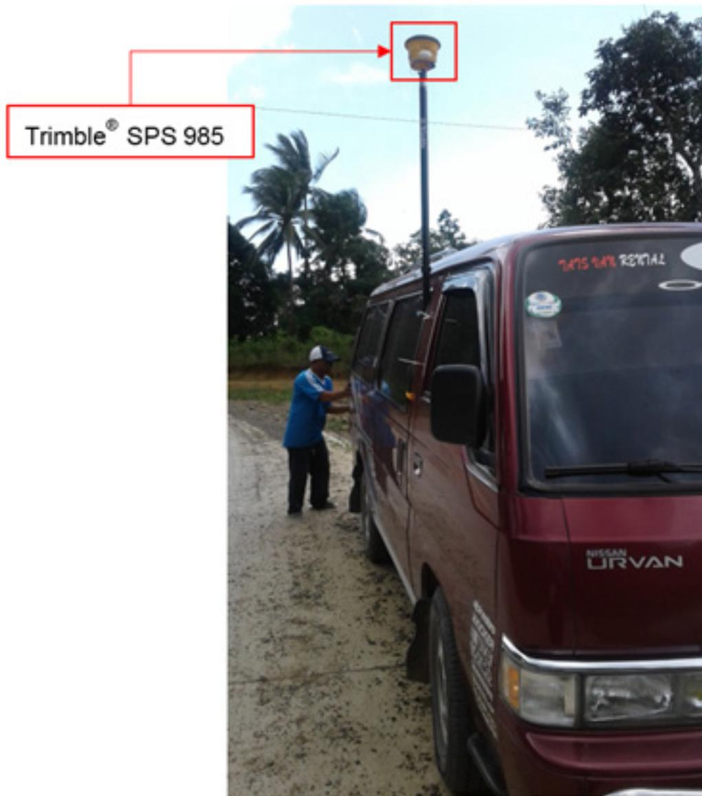
Figure 45. Validation points acquisition survey set-up for Aborlan River.
