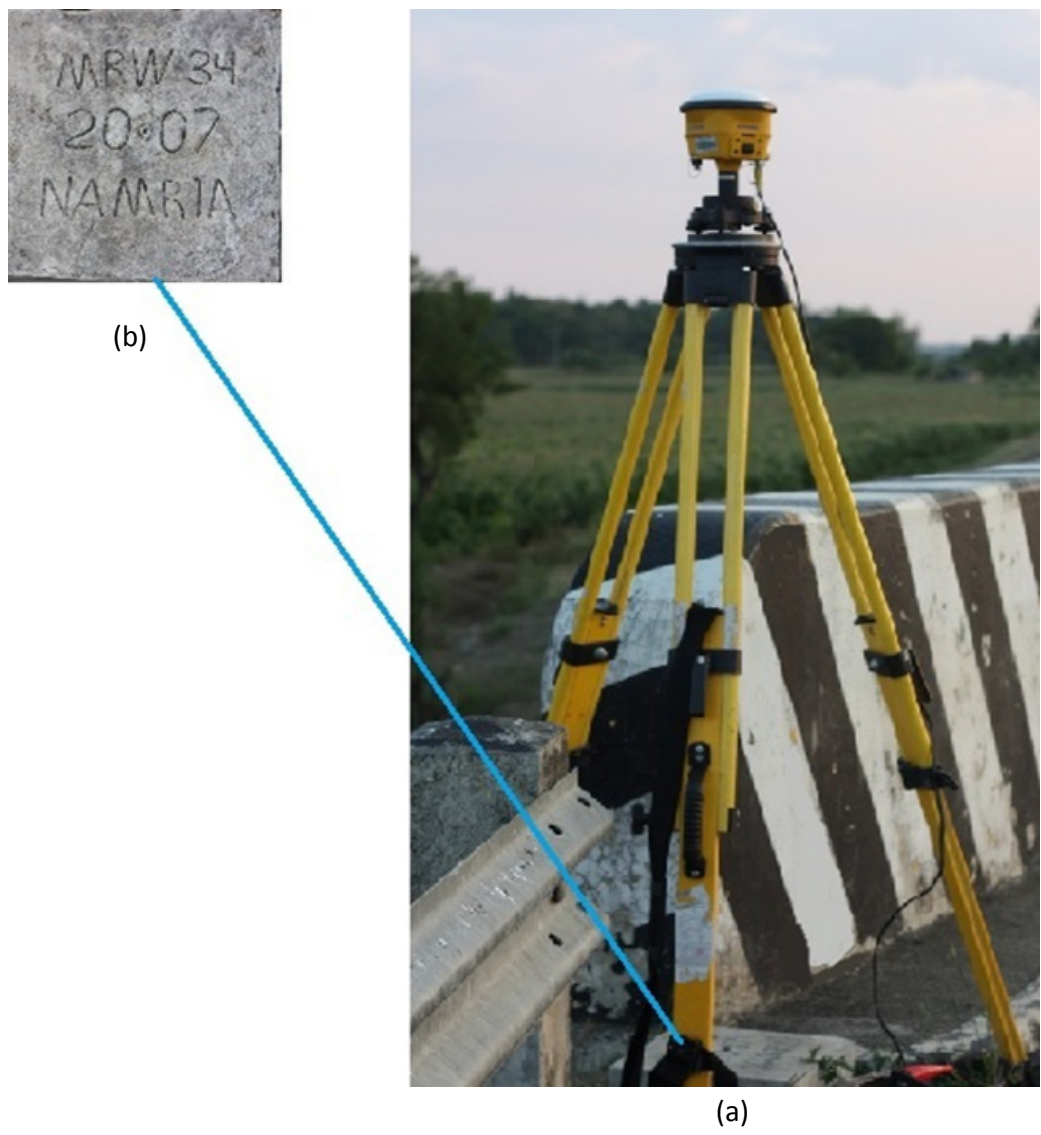
Figure 5. GPS set-up over MRW-34 as recovered in Balibago Bridge in Brgy. Armado, municipality of Abra de Ilog, Occidental Mindoro (a) and NAMRIA reference point MRW-34 (b) as recovered by the field team.
