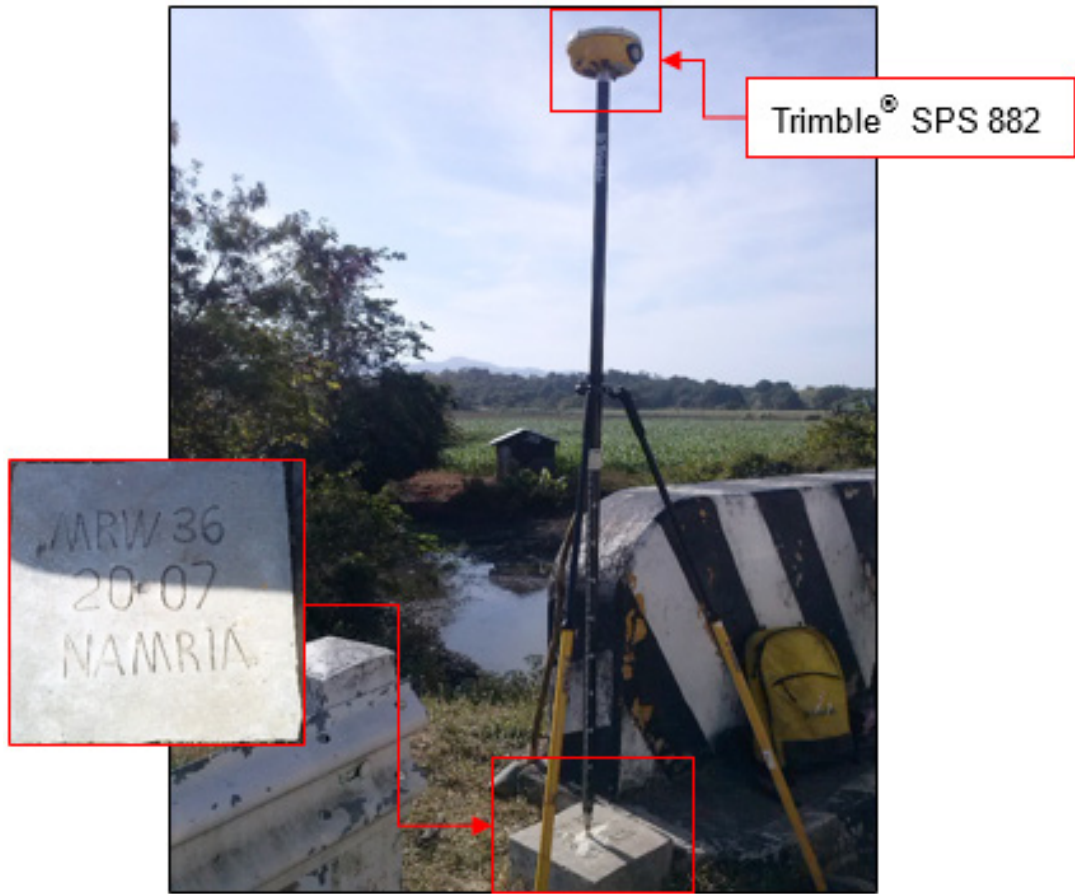
Figure 34. GNSS receiver set up, Trimble® SPS 882, at MRW-36, located beside the approach of Baclaran Bridge in Brgy. Armado, Abra de Ilog, Occidental Mindoro
