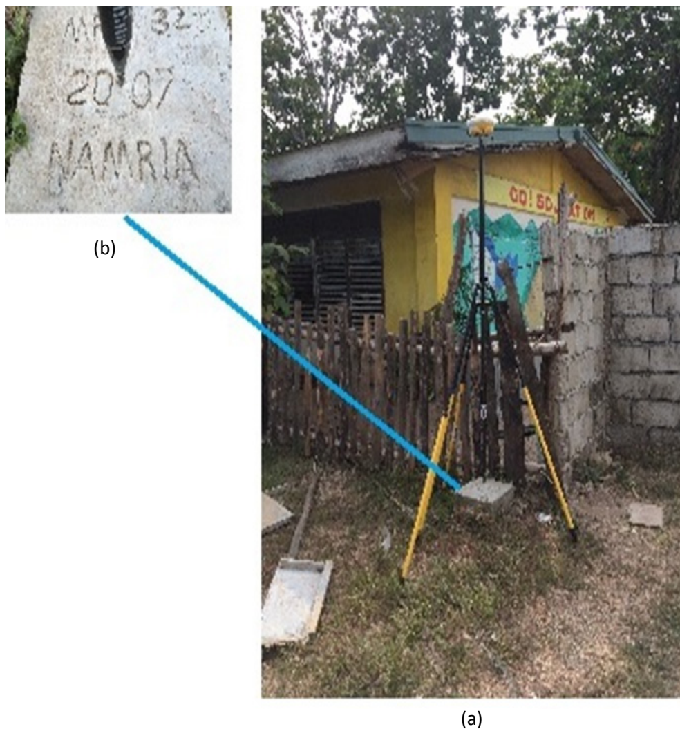
Figure 6. GPS set-up over MRW-32 as recovered in the corner of a day care center in Brgy. Fatima, municipality of Mamburao, Occidental Mindoro (a) and NAMRIA reference point MRW-32 (b) as recovered by the field team.
