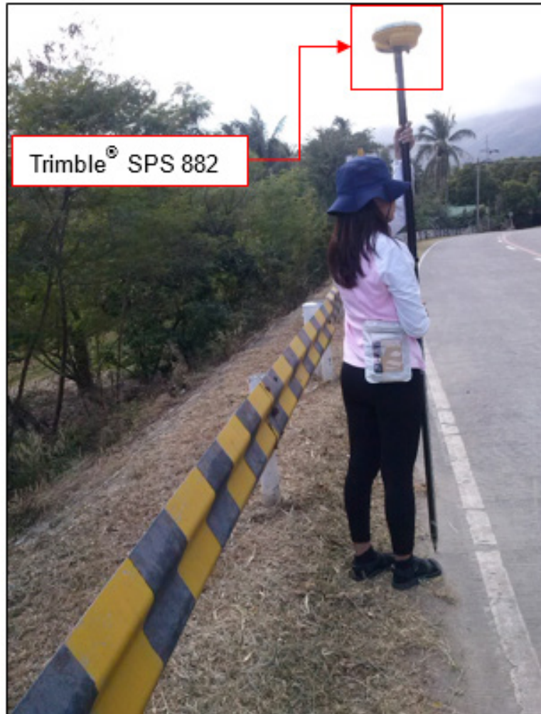
Figure 40. Gathering of random cross-section points along Lumang Bayan Bridge
