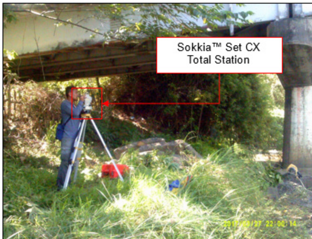
Figure 39. Cross-section survey of Lumang Bayan Bridge
