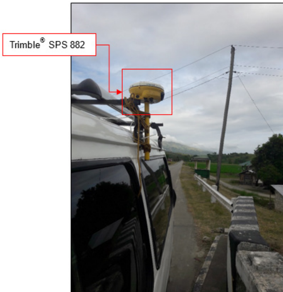
Figure 46. Validation points acquisition survey set-up for Abra de Ilog River
