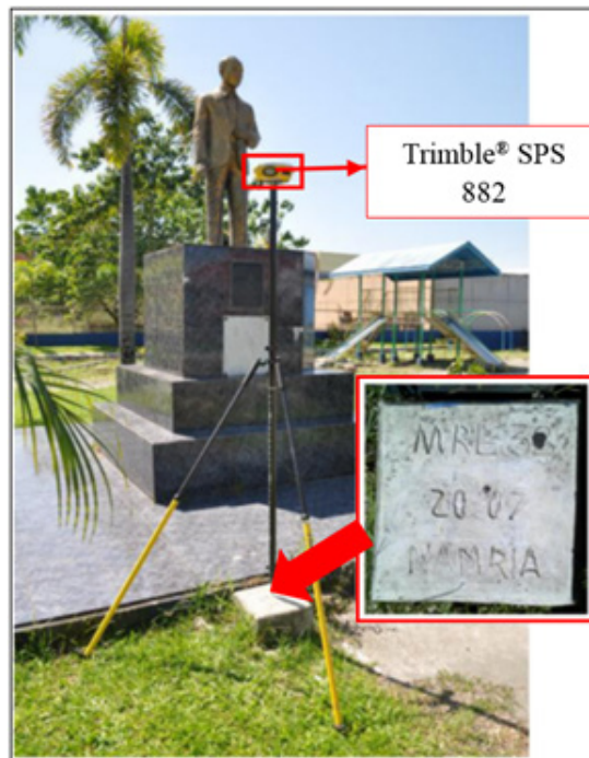
Figure 31. GPS set-up of Trimble® SPS 882 at MRE-32, located at the Municipal Park of Victoria, in Brgy. Poblacion I, Oriental Mindoro
