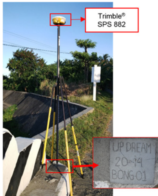
Figure 34. GNSS set-up of Trimble® SPS 882 on BONG-01 in Brgy. San Isidro, Municipality of Bongabong, Oriental Mindoro
