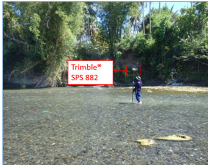
Figure 49. Manual bathymetric survey in Agsalin River
