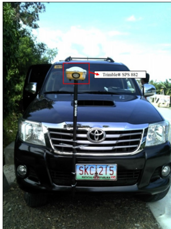
Figure 47. Validation points acquisition survey set-up
