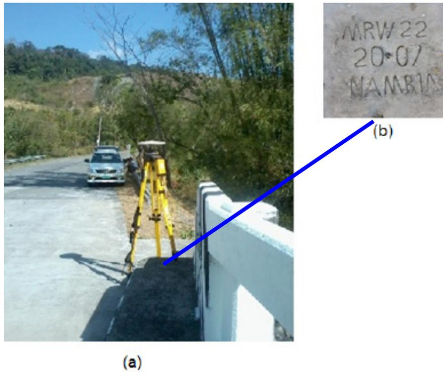
Figure 4. GPS set-up over MRW-22 in Lumintao Bridge in Brgy. Tanyag, municipality of Calintaan, Occidental Mindoro (a) and NAMRIA reference point MRW-22 (b) as recovered by the field team.
