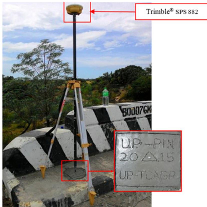
Figure 38. The GNSS receiver occupation, Trimble® SPS 882, at UP-PIN Pinamanaán Bridge approach in Brgy. Mapaya, Municipality of San Jose, Occidental Mindoro
