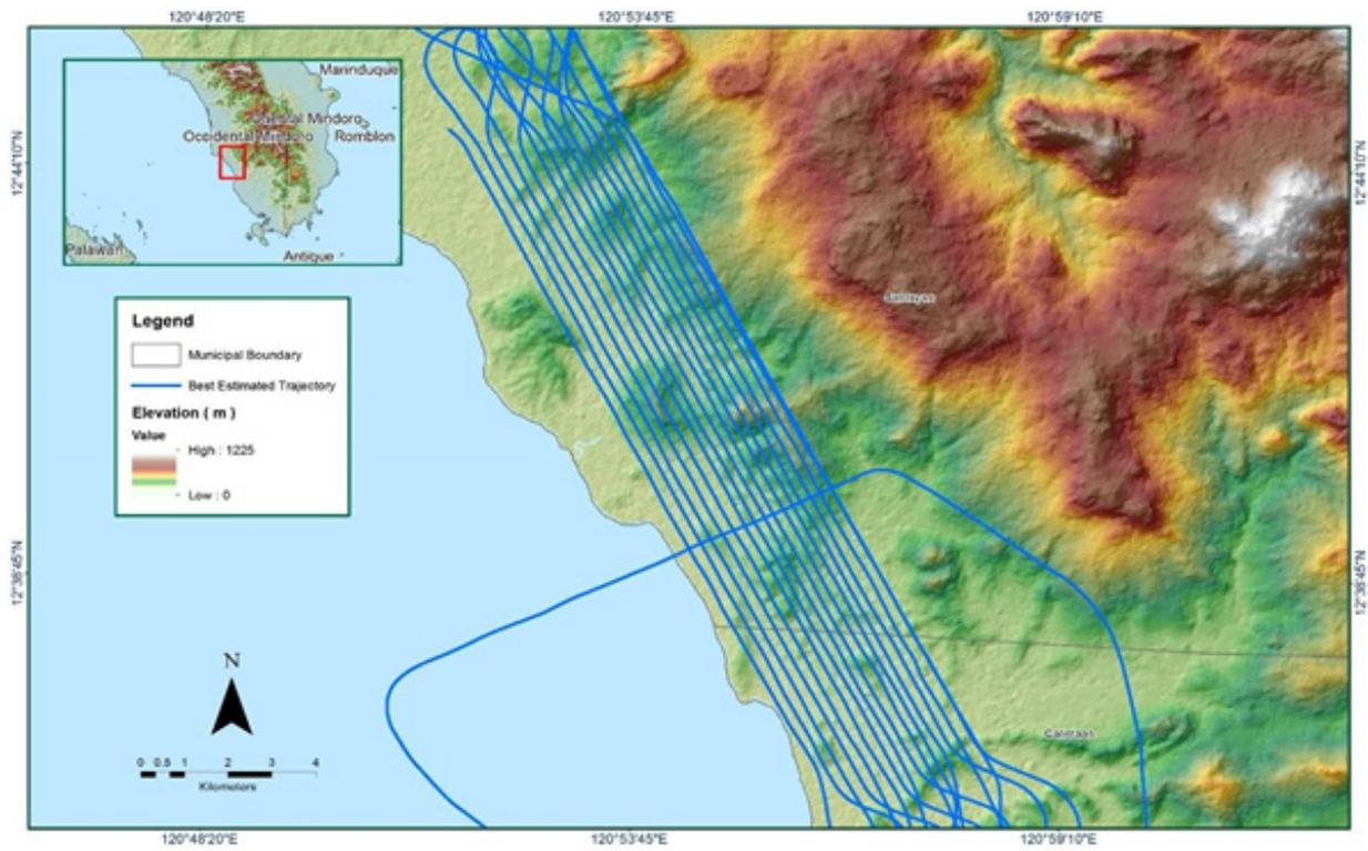
Figure A-8.10. Best estimated trajectory of LiDAR missions conducted over the Anahawin Floodplain.
