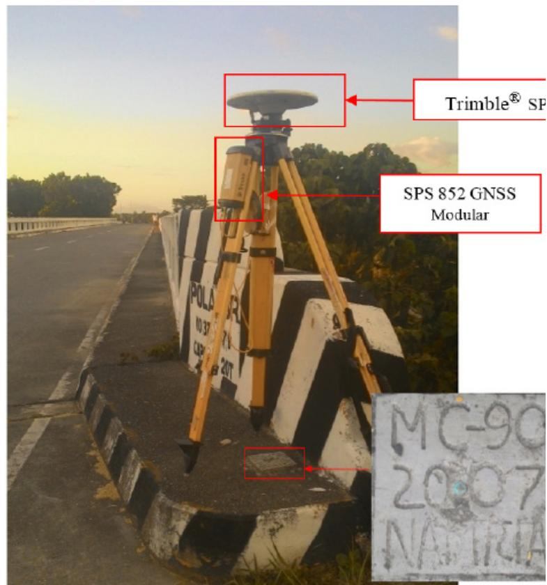
Figure 36. The GNSS (Trimble® SPS 852) base occupation at MC-90, used as marker, located at the Pola Bridge approach in Brgy. Barahan, Municipality of Santa Cruz, Occidental Mindoro
