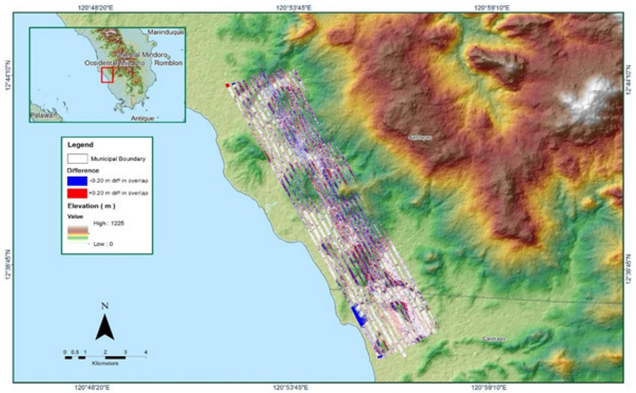
Figure A-8.14. Elevation difference between flight lines
