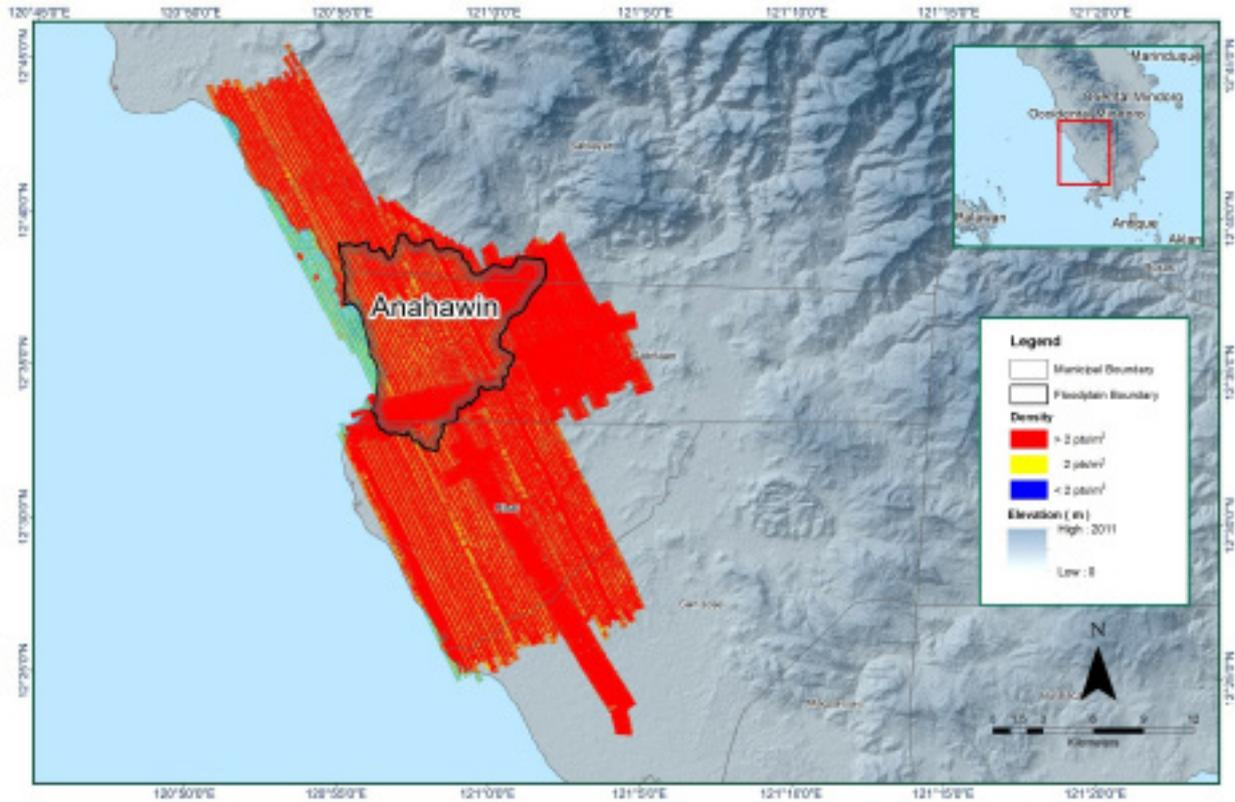
Figure 16. Pulse density map of the merged LiDAR data for the Anahawin Floodplain Survey.
