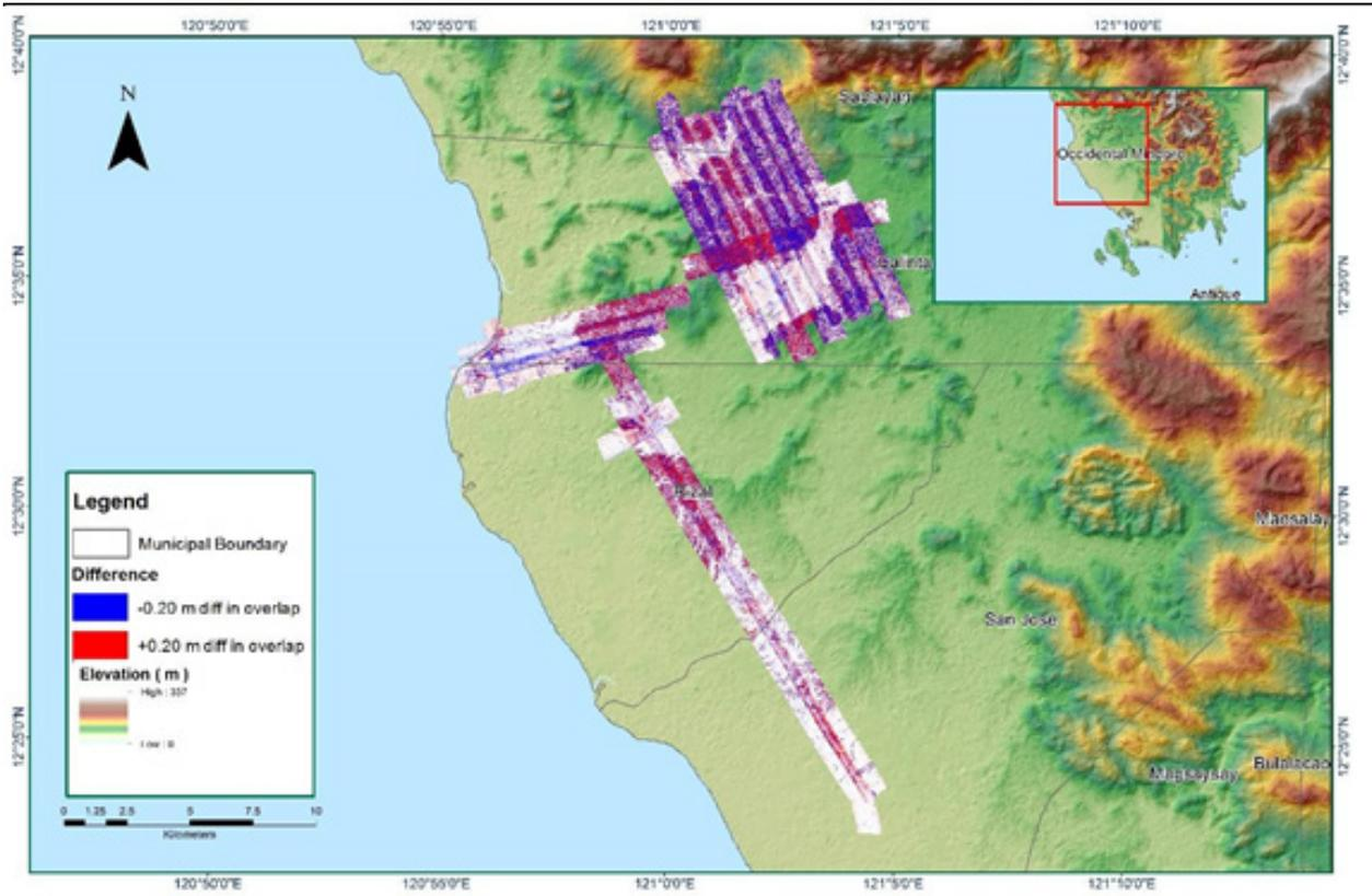
Figure A-8.42. Elevation difference between flight lines
