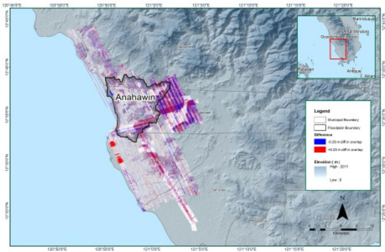
Figure 17. Map of elevation difference Map between flight lines for the Anahawin Floodplain Survey.
