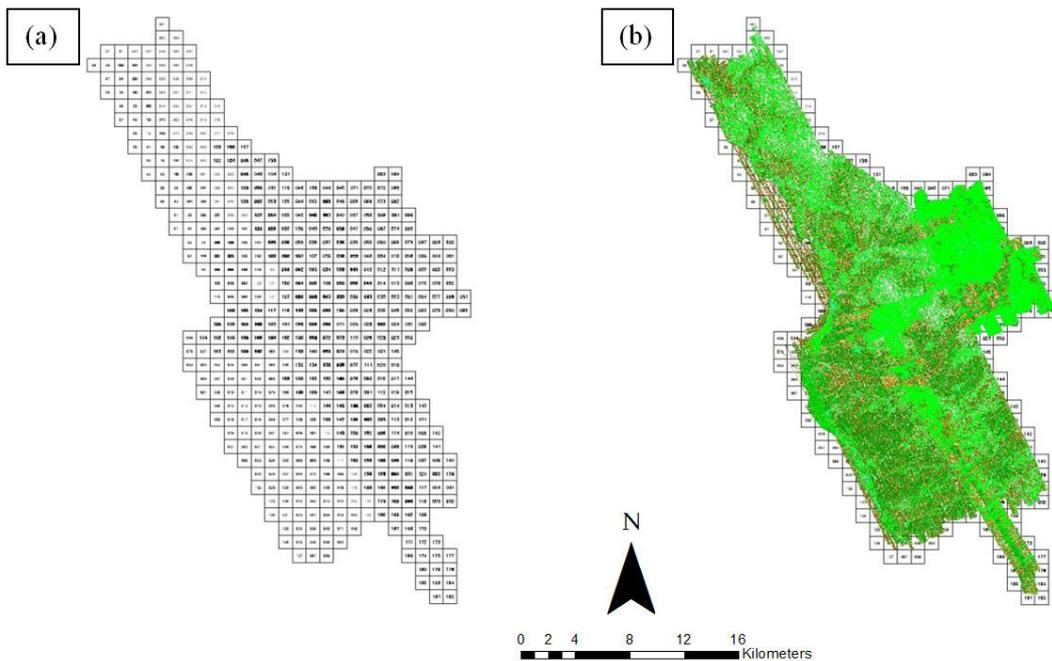
Figure 19. The coverage of the Anahawin Floodplain Survey(a) the tile system (b) depicts the classification results in TerraScan.
