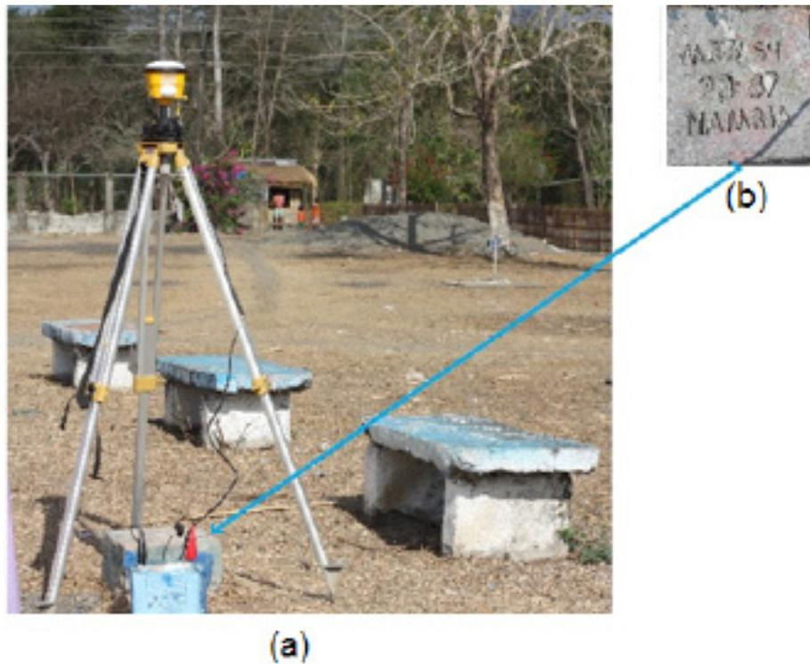
Figure 6. NAMRIA reference point MRW-54 (a) as recovered by the field team and GPS set-up over MRW-54 as recovered in near basketball open court in Brgy. Malisbong, municipality of Sablayan, Occidental Mindoro (b).
