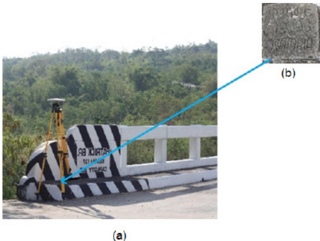
Figure 3. NAMRIA reference point MRW-6 (a) as recovered by the field team and GPS set-up over MRW-6 as recovered in Patrick Bridge in Brgy. Yabang, municipality of Sablayan, Occidental Mindoro (b).
