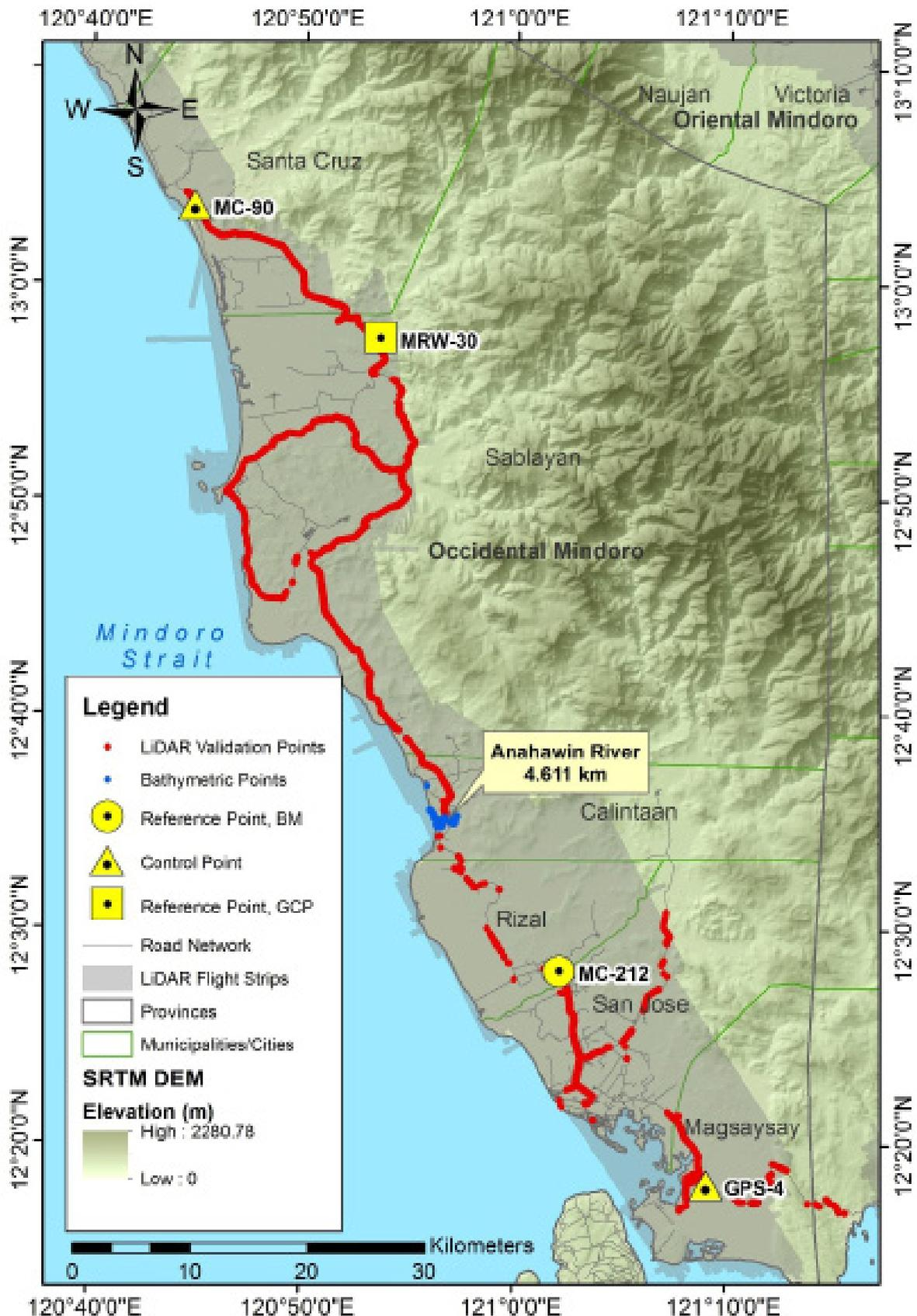
Figure 46. The extent of the LiDAR ground validation survey for Anahawin River Basin
