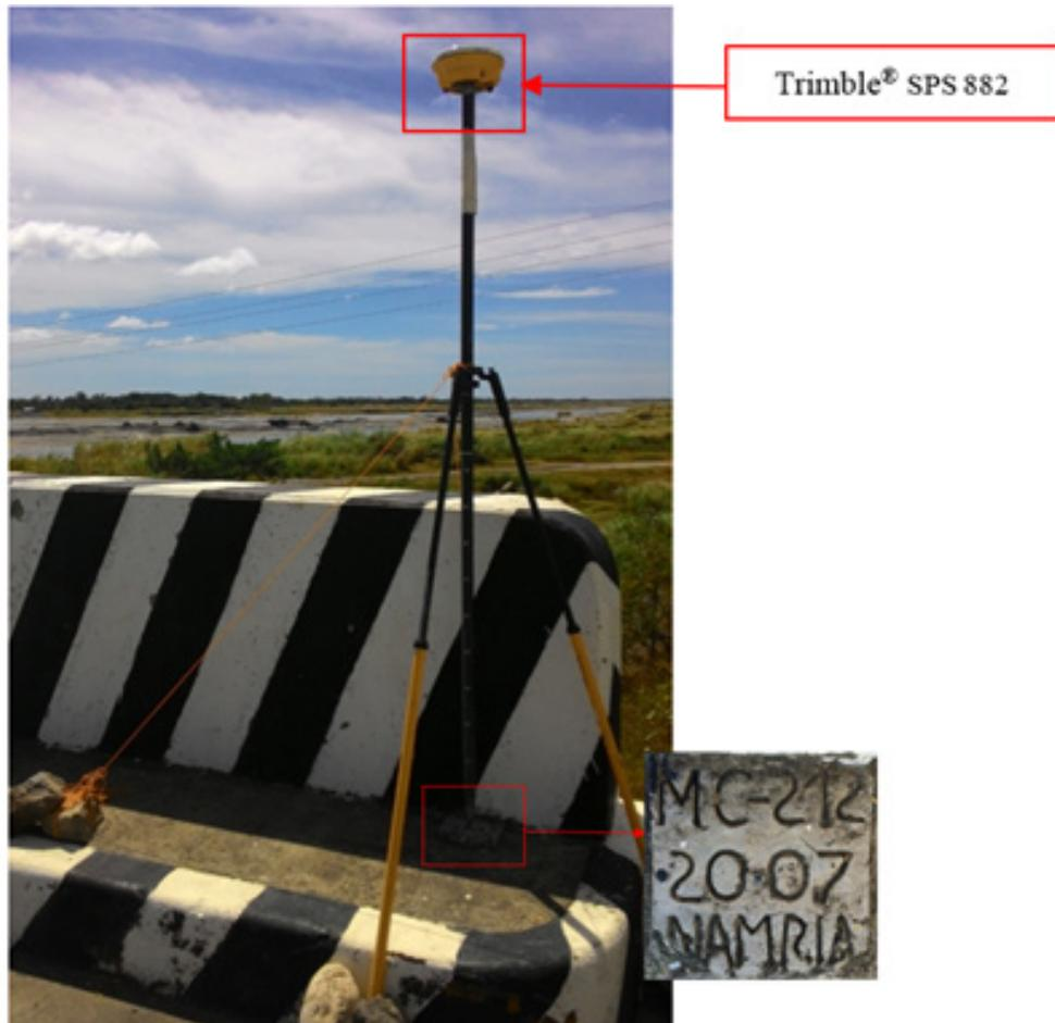
Figure 35. The GNSS (Trimble® SPS 852) base occupation at MC-212, located at the approach of Busuanga Bridge in Brgy. Sto Niño, Municipality of Rizal, Occidental Mindoro
