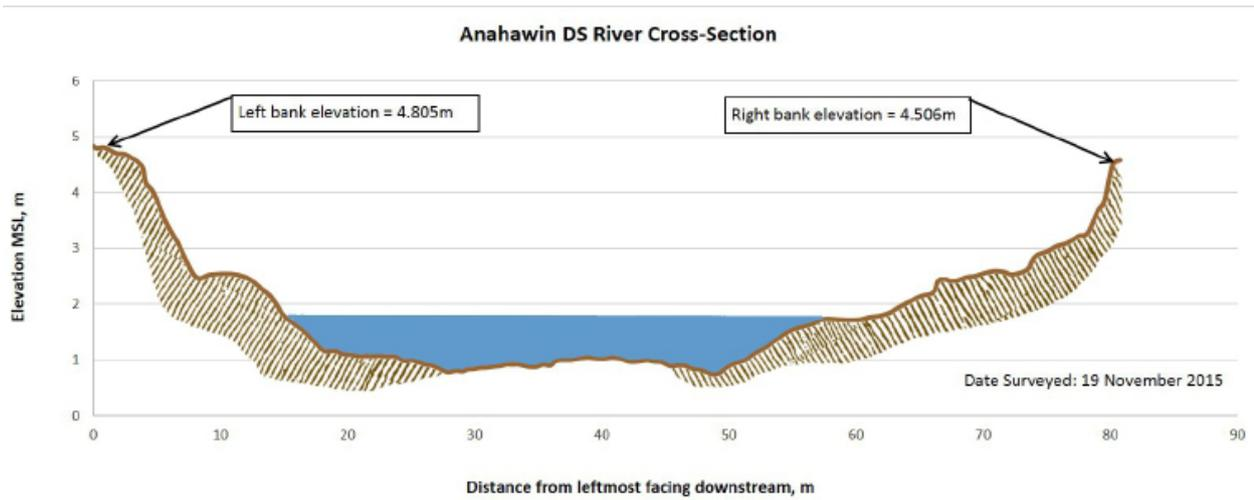
Figure 51. The cross-section plot of the Anahawin Bridge
