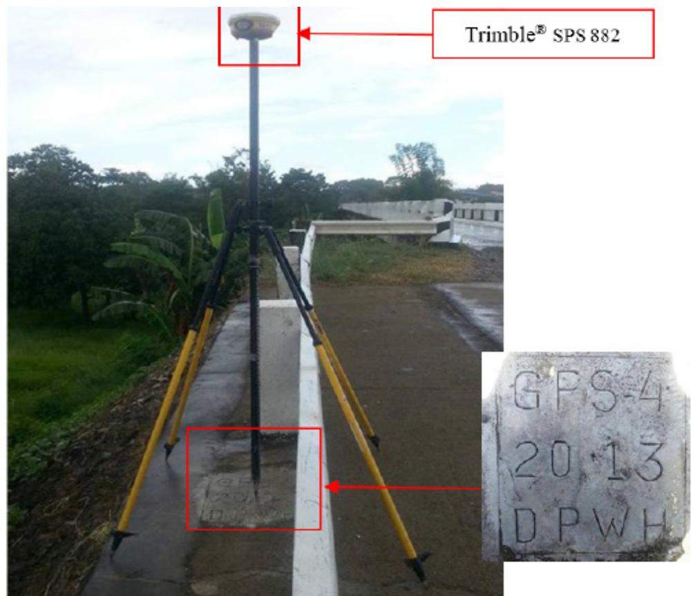
Figure 37. The GNSS (Trimble® SPS 882) base occupation , at GPS-4 on right side of the road abutment after Caguray Bridge going to Bulalacao in Brgy. Poblacion, Municipality of Magsaysay, Occidental Mindoro
