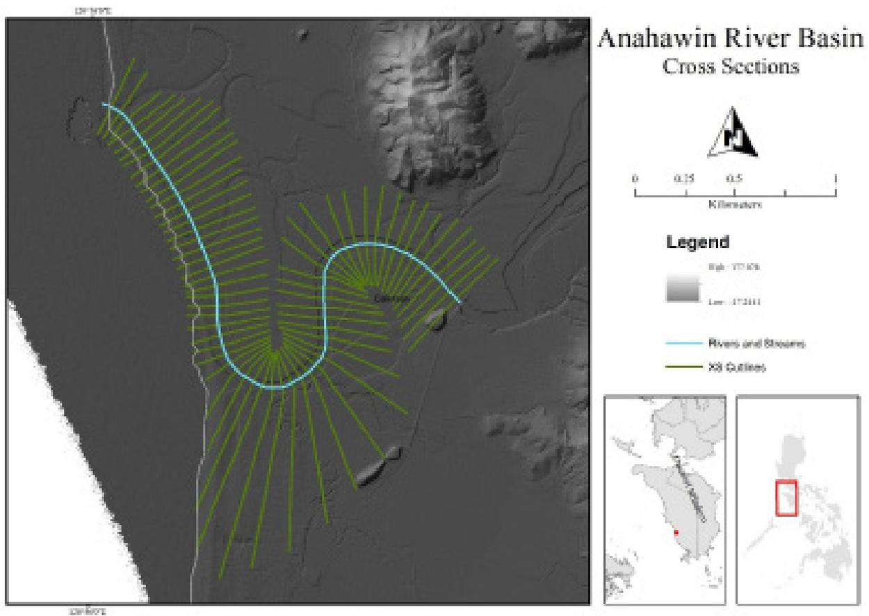
Figure 61. River cross-section of the Anahawin River through the ArcMap HEC GeoRAS tool
