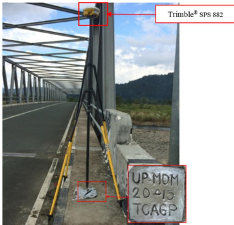
Figure 39. The GNSS receiver occupation, Trimble® SPS 882, at UP-MOM, Mompong Bridge approached in Brgy. Lumang Bato, Municipality of Sablayan, Occidental Mindoro
