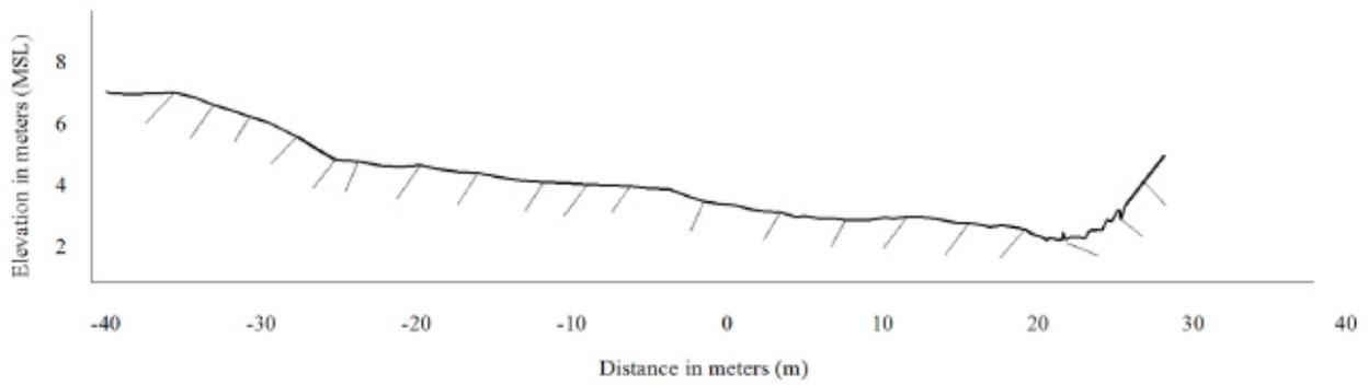
Figure 43. The upstream side of the Anahawin Bridge cross-section survey drawn to scale
