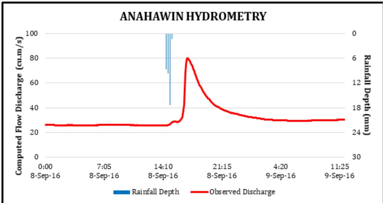
Figure 53. Rainfall and outflow data of the Anahawin River Basin, which was used for modeling.
