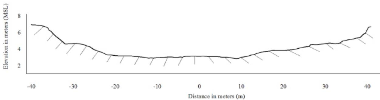
Figure 44. The downstream side of the Anahawin Bridge cross-section survey drawn to scale
