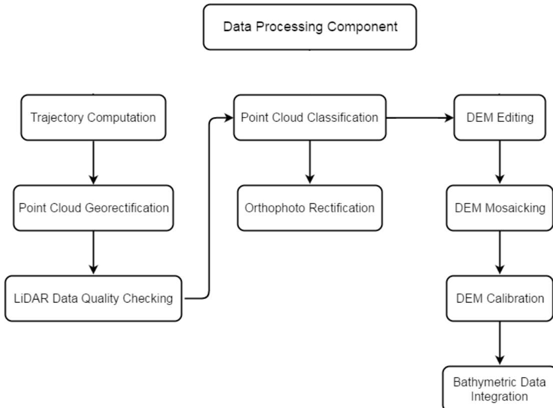
Figure 10. Schematic diagram for Data Pre-processing
