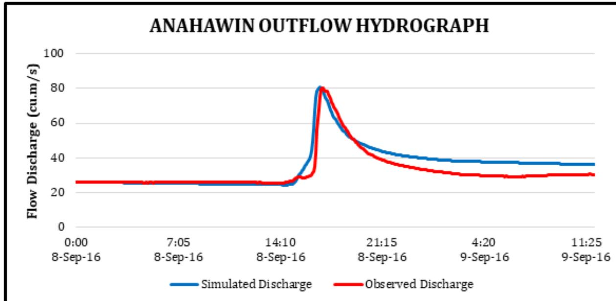
Figure 63. Outflow Hydrograph of Anahawin produced by the HEC-HMS model compared with observed outflow
