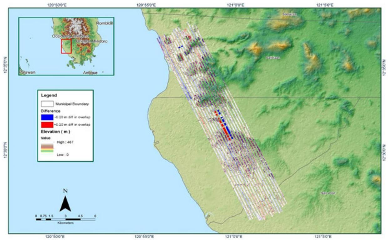
Figure A-8.35. Elevation difference between flight lines
