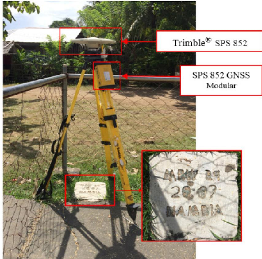
Figure 32. The GNSS base receiver setup, Trimble® SPS 852, at MRW-24, located in front of Iriron Elementary School in Brgy. Iriron, Municipality of Calintaan, Occidental Mindoro.
