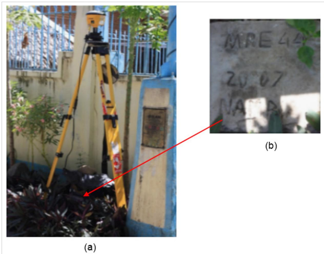
Figure 3. GPS set-up over MRE-44 just outside the compound of the barangay hall of Happy Valley, municipality of Roxas, Oriental Mindoro (a) and NAMRIA reference point MRE-44 (b) as recovered by the field team.
