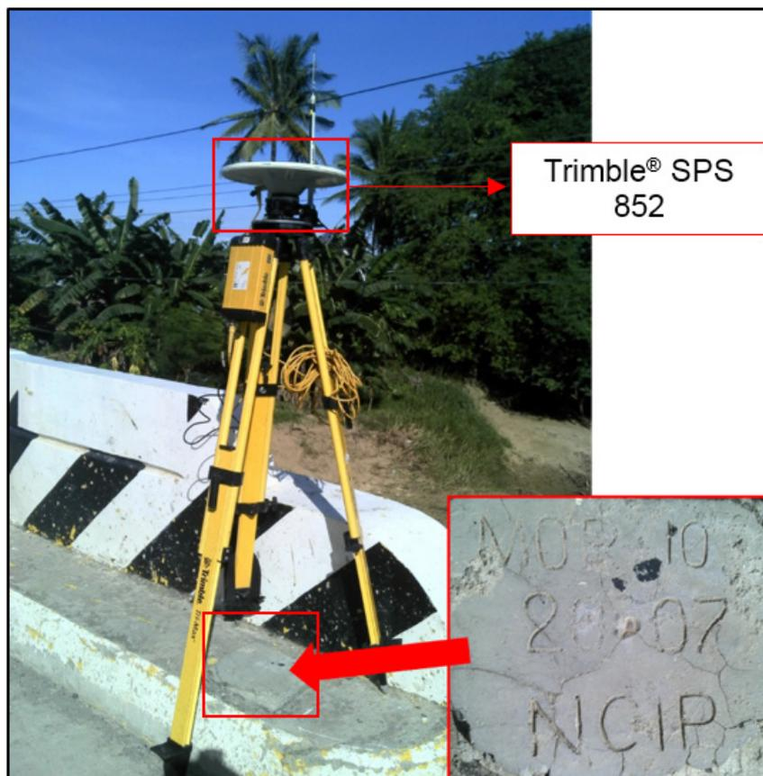
Figure 32. GPS setup of Trimble® SPS 852 at MOR-10, located in the approach of the Cawacat Bridge, in Bry. Campasaan, Municipality of Bulalacao, Oriental Mindoro
