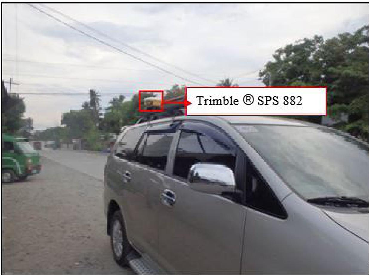
Figure 42. Trimble® SPS 882 setup for validation points acquisition survey for Baroc River
