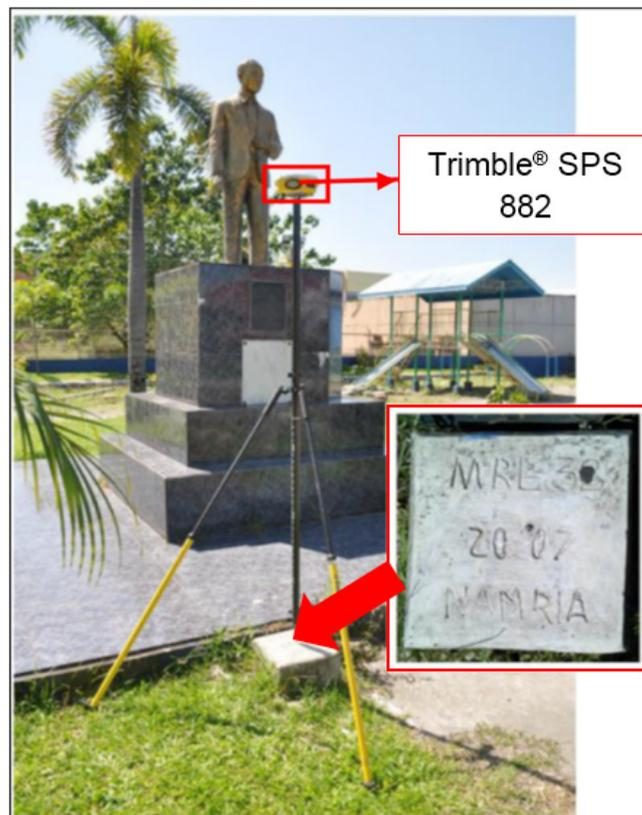
Figure 28. GPS setup of Trimble® SPS 882 at MRE-32, located at the Municipal Park of Victoria, in Brgy. Poblacion 1, Oriental Mindoro
