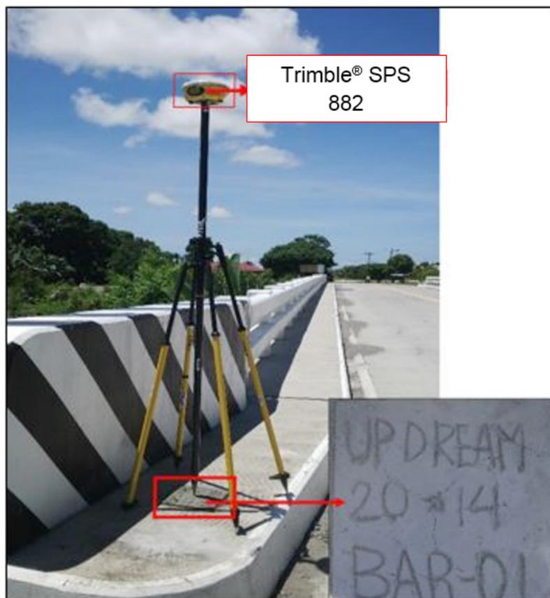
Figure 30. GPS setup of Trimble® SPS 882 at BAR-1, an established control point located in Baroc Bridge, Brgy. San Isidro, Mansalay, Oriental Mindoro
