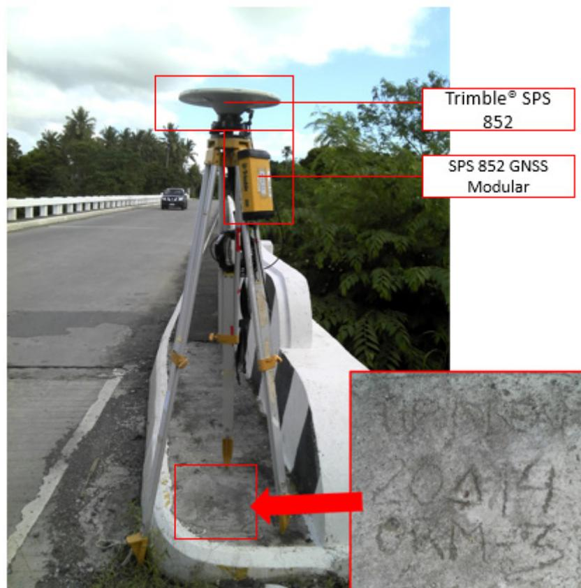
Figure 34. Trimble® SPS 985 setup at ORM-3 located at the approach of Balete Bridge, Brgy. Balete, Municipality of Gloria, Oriental Mindoro
