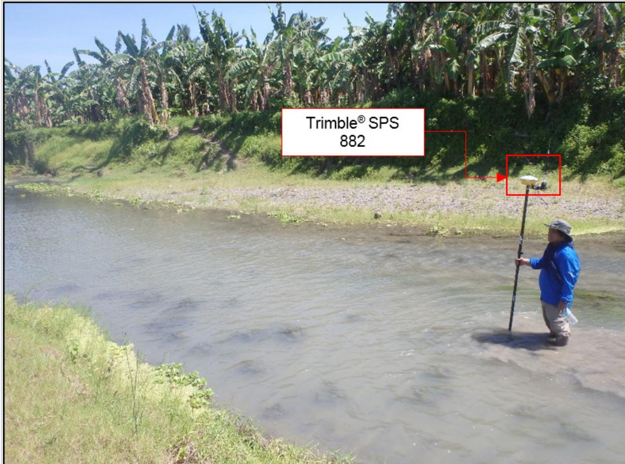
Figure 44. Trimble® SPS 882 setup for validation points acquisition survey for Baroc River
