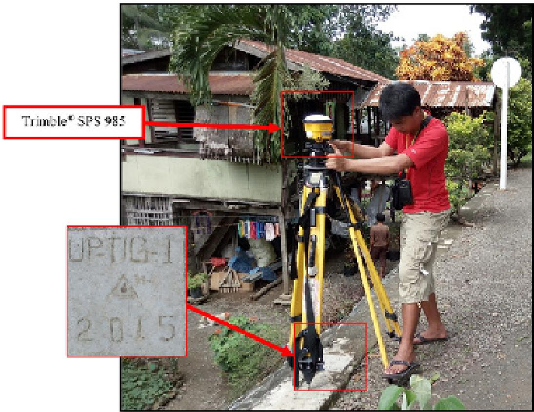
Figure 30. Figure 30. GNSS receiver set up, Trimble® SPS 985, at UP\_TIG-1, located at the approach of Tigaplan Bridge in Brgy. Tigaplan, Brookes Point, Province of Palawan.
