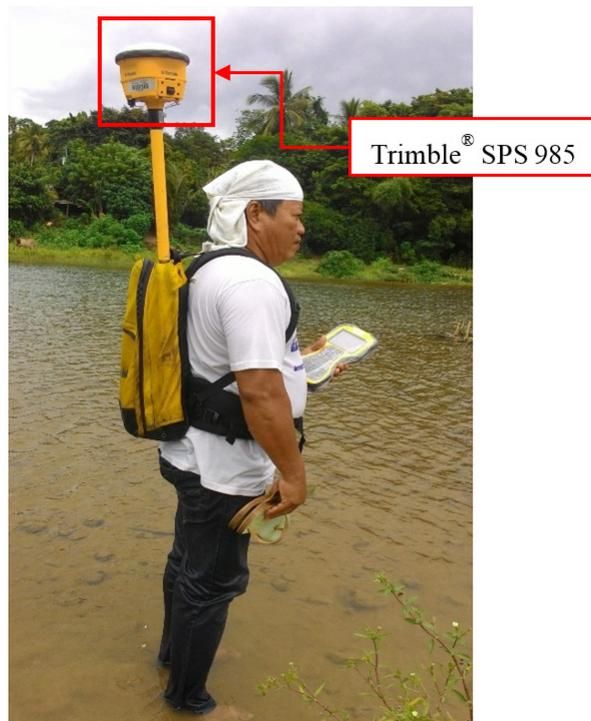
Figure 39. Bathymetric survey using Trimble® SPS 985 in GNSS PPK survey technique in the Boac River
