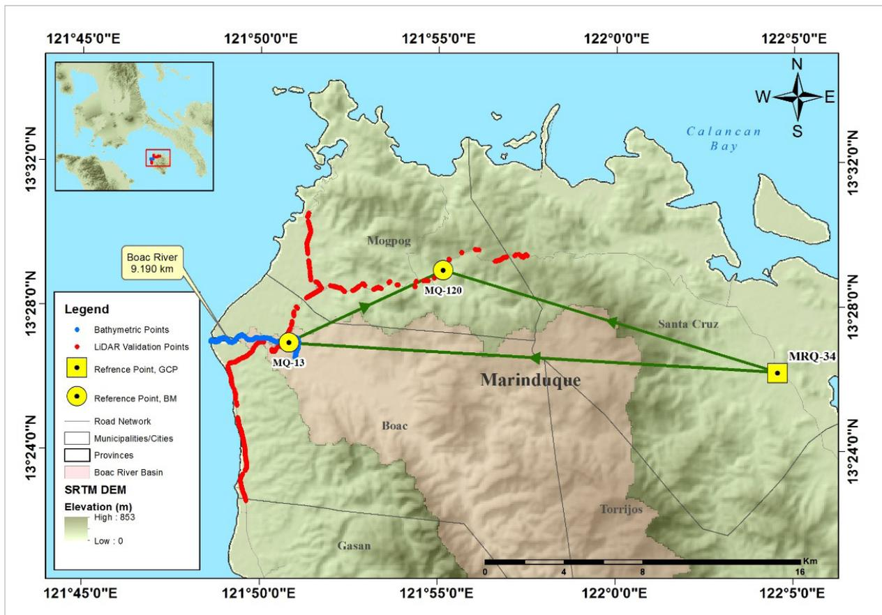
Figure 25. Extent of the bathymetric survey (in blue line) in the Boac River and the LiDAR data validation survey (in red).
