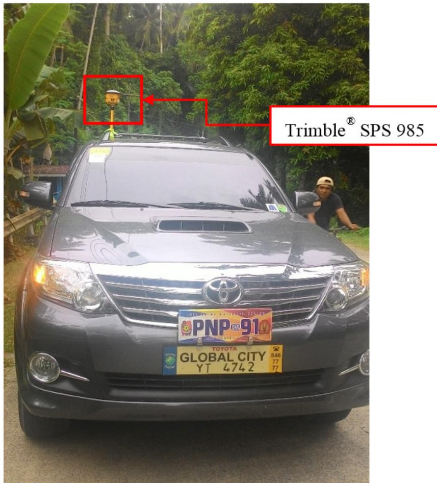
Figure 36. Validation points acquisition survey set-up along the Boac River Basin
