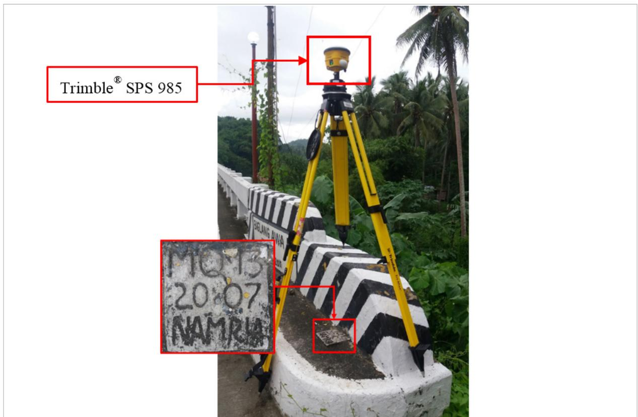
Figure 28. GNSS receiver set-up, Trimble® SPS 985 at MQ-13, located at the approach of the Biglang Awa Bridge in Barangay Mataas na Bayan, Boac, Marinduque
