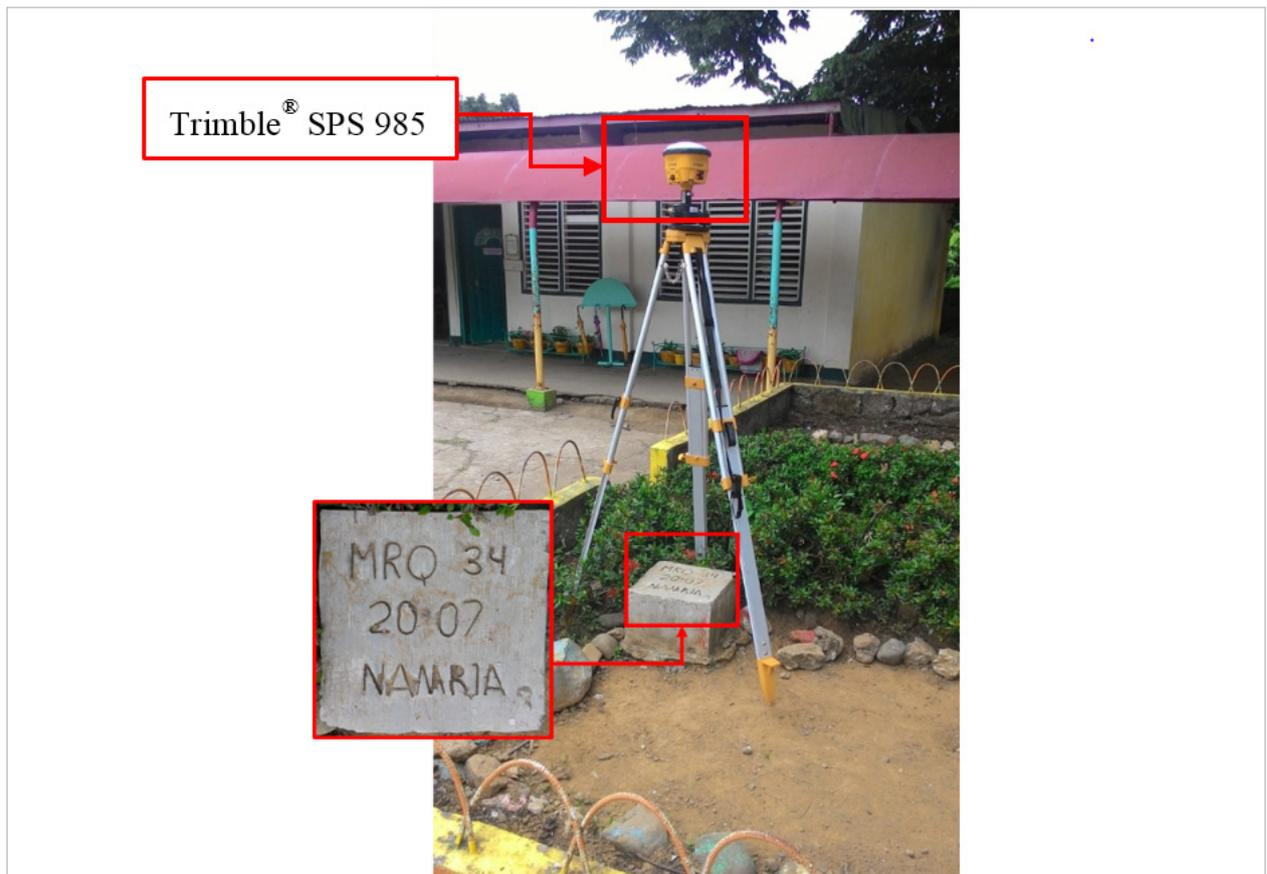
Figure 27. GNSS base set-up, Trimble® SPS 985 at MRQ-34, located near the Rizal statue inside Makapuyat Elementary School in Barangay Napo, Sta. Cruz, Marinduque
