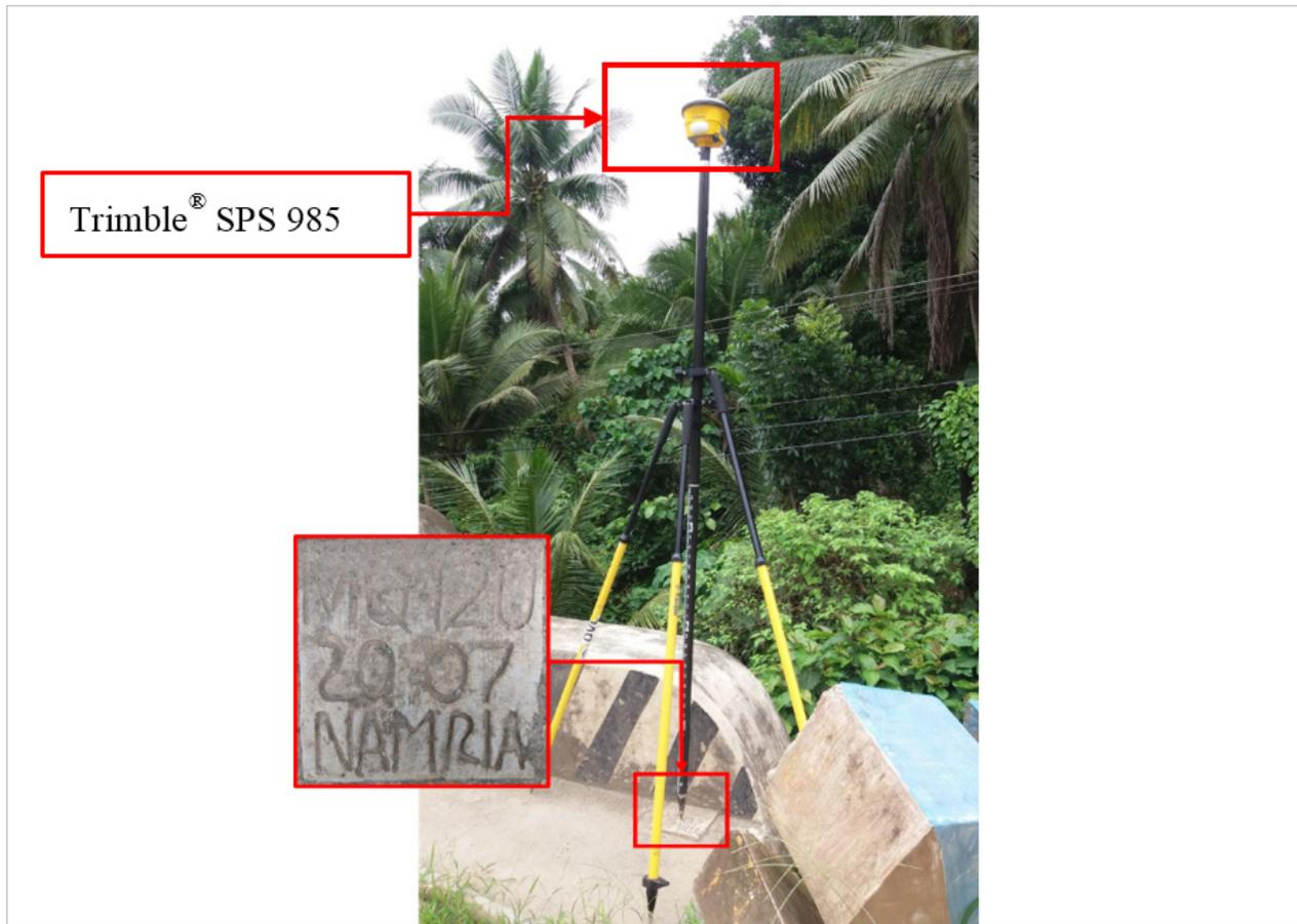
Figure 29. GNSS receiver set-up, Trimble® SPS 985 at MQ-120, located at the approach of the Mangamnan Bridge in Barangay Butansapa, Mogpong, Marinduque
