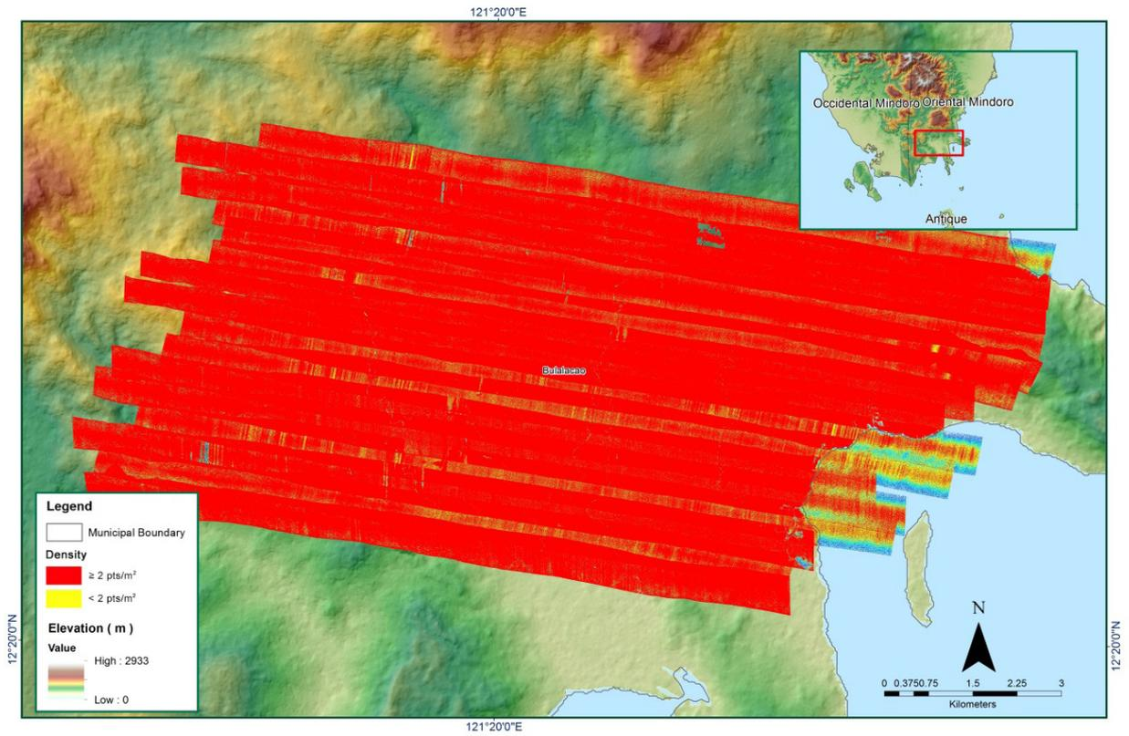
Figure A-8.27. Density of merged LiDAR data
