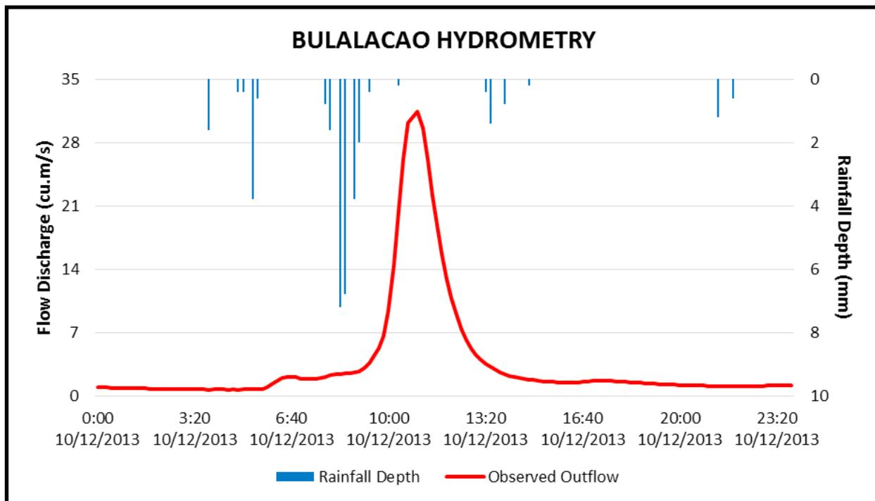
Figure 51. Rainfall and outflow data at Bulalacao River Basin used for modeling
