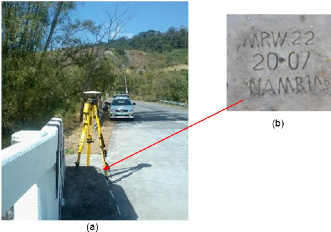
Figure 3. GPS set-up over MRW-22 as recovered in Lumintao Bridge in Brgy. Tanyag, municipality of Calintaan, Occidental Mindoro (a) and NAMRIA reference point MRW-22 (b) as recovered by the field team.
