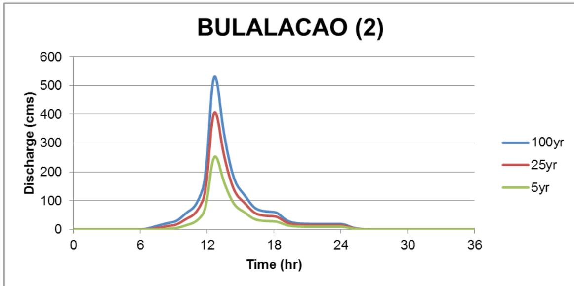
Figure 64. Bulalacao river (2) generated discharge using 5-, 25-, and 100-year Romblon rainfall intensity-duration-frequency (RIDF) in HEC-HMS
