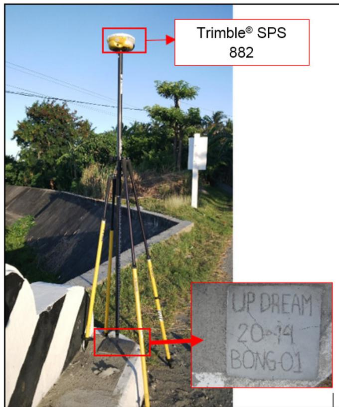
Figure 31. GNSS setup of Trimble® SPS 882 on BONG-01 in Brgy. San Isidro, Municipality of Bongabong, Oriental Mindoro
