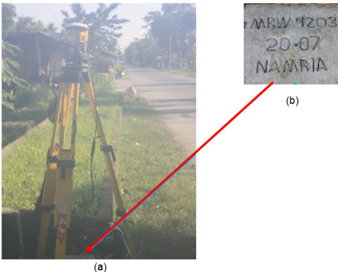
Figure 4. GPS set-up over MRW-4203 as recovered front of the barangay hall of Brgy. Mapaya, municipality of San Jose, Occidental Mindoro (a) and NAMRIA reference point MRW-4203 (b) as recovered by the field team.
