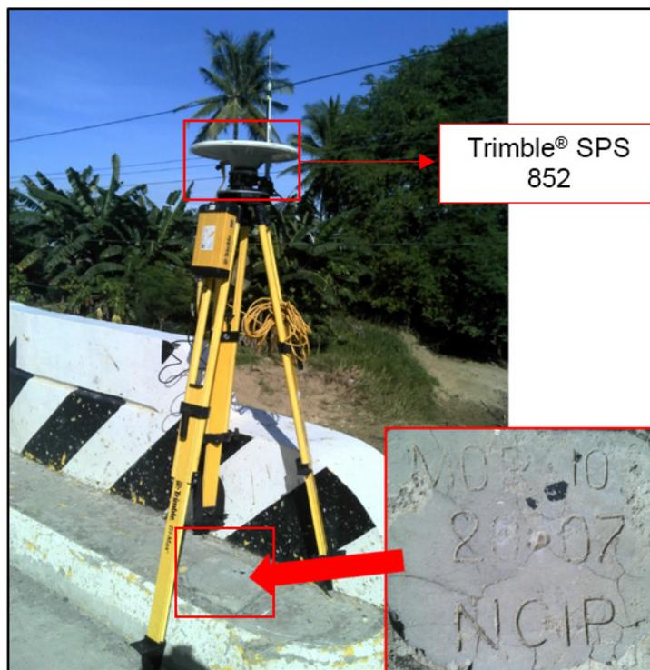
Figure 32. GPS setup of Trimble® SPS 852 at MOR-10, located in the approach of the Cawacat Bridge, in Bry. Campasaan, Municipality of Bulalacao, Oriental Mindoro
