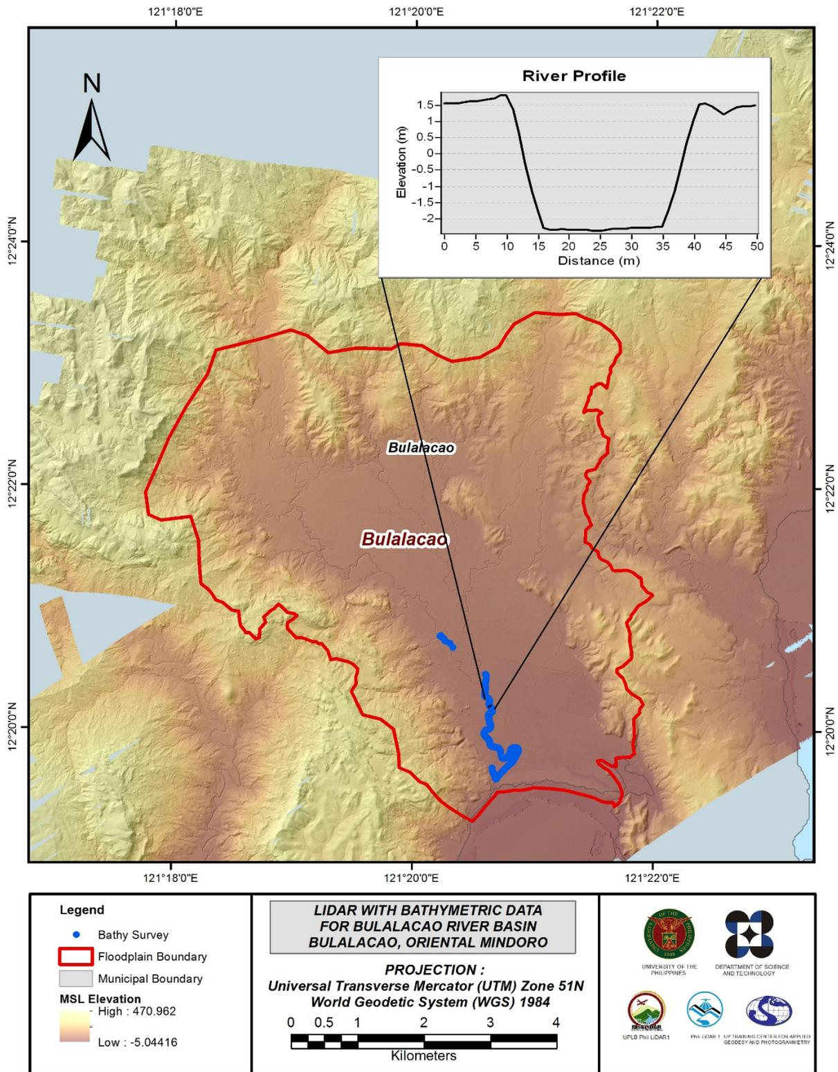
Figure 25. Map of Bulalacao Floodplain with bathymetric survey points shown in blue.
