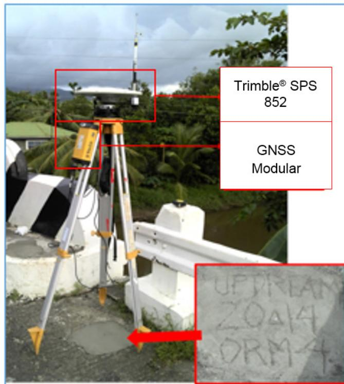
Figure 35. GNSS receiver Trimble® SPS 852 setup at ORM-4, located at the right side of the approach of Pola Bridge in Barangay Casiligan, Municipality of Pola, Oriental Mindoro
