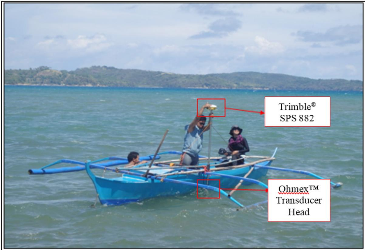
Figure 45. Bathymetric survey conducted in Bulalacao River using Trimble SPS 882 and Ohmex Transducer Head
