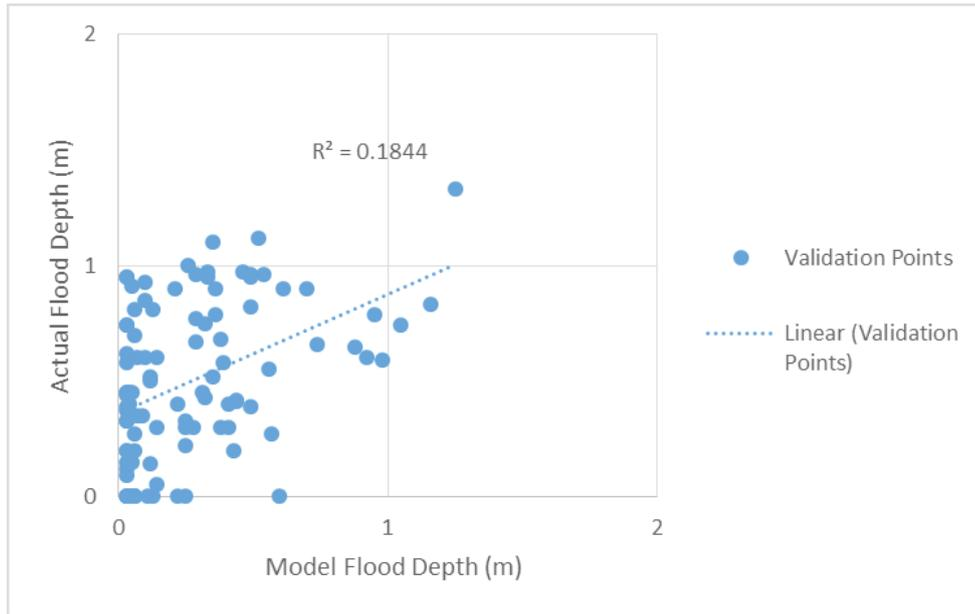
Figure 76. Flood map depth vs. actual flood depth
