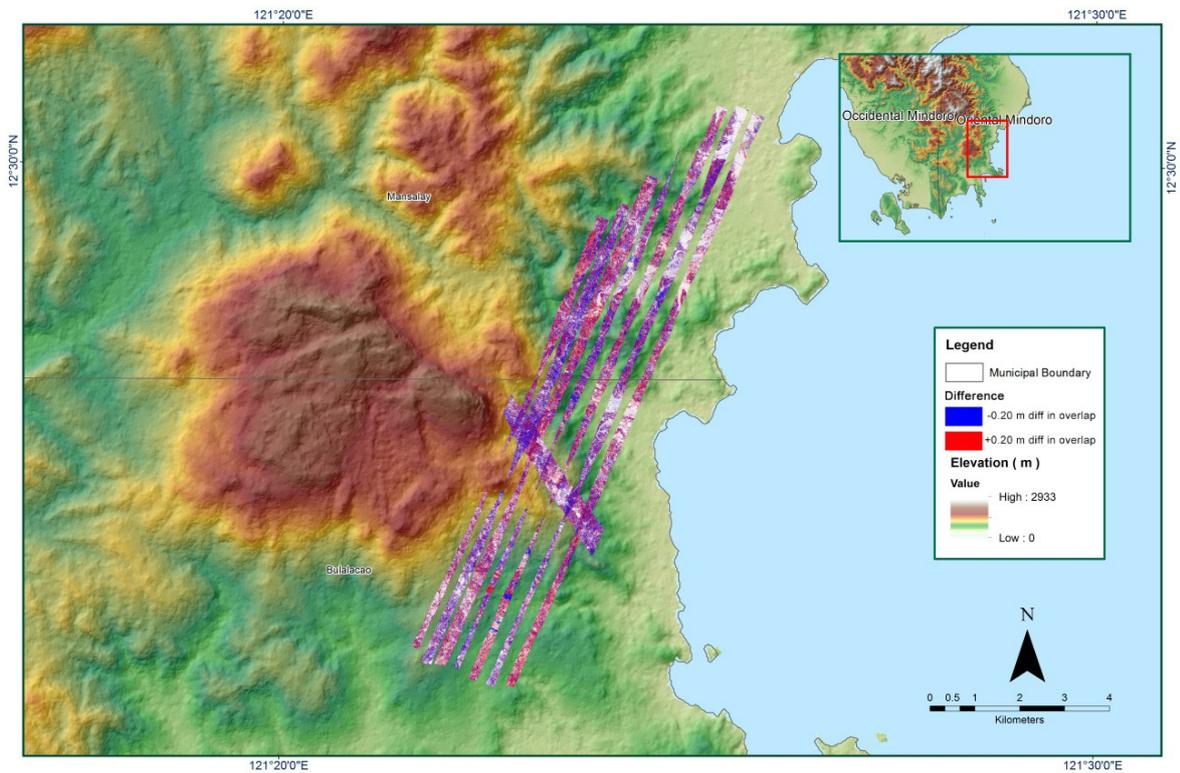
Figure A-8.21. Elevation difference between flight lines
