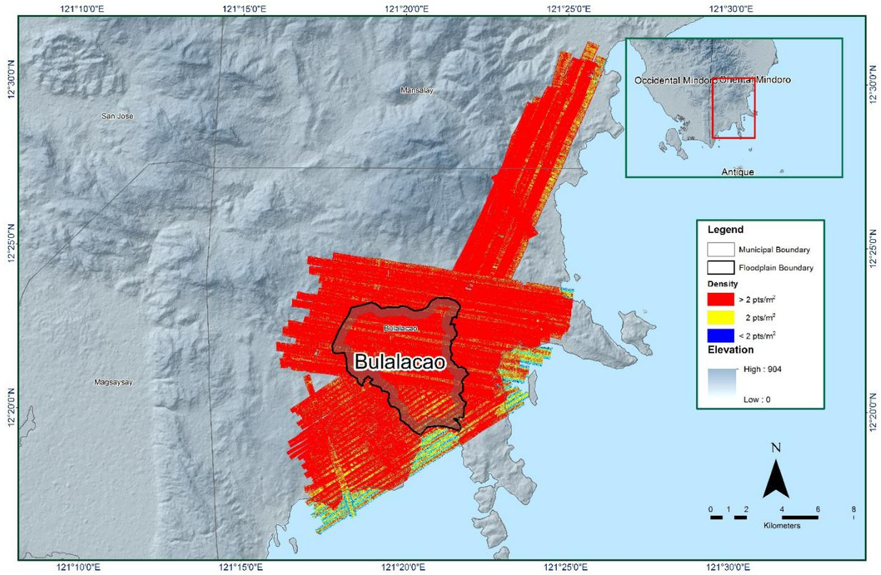
Figure 12. Pulse density map of merged LiDAR data for Bulalacao Floodplain.
