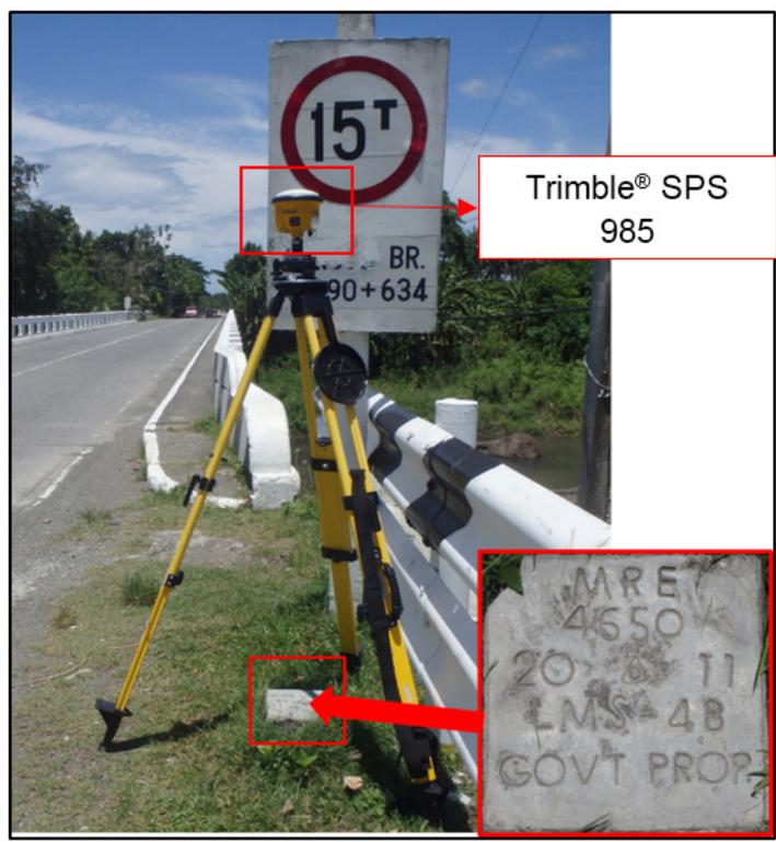
Figure 29. The GPS setup of Trimble® SPS 985 at MRE-4650, an LMS control point located at the approach of Bansud Bridge, in Brgy. Pagasa, Municipality of Bansud, Oriental Mindoro
