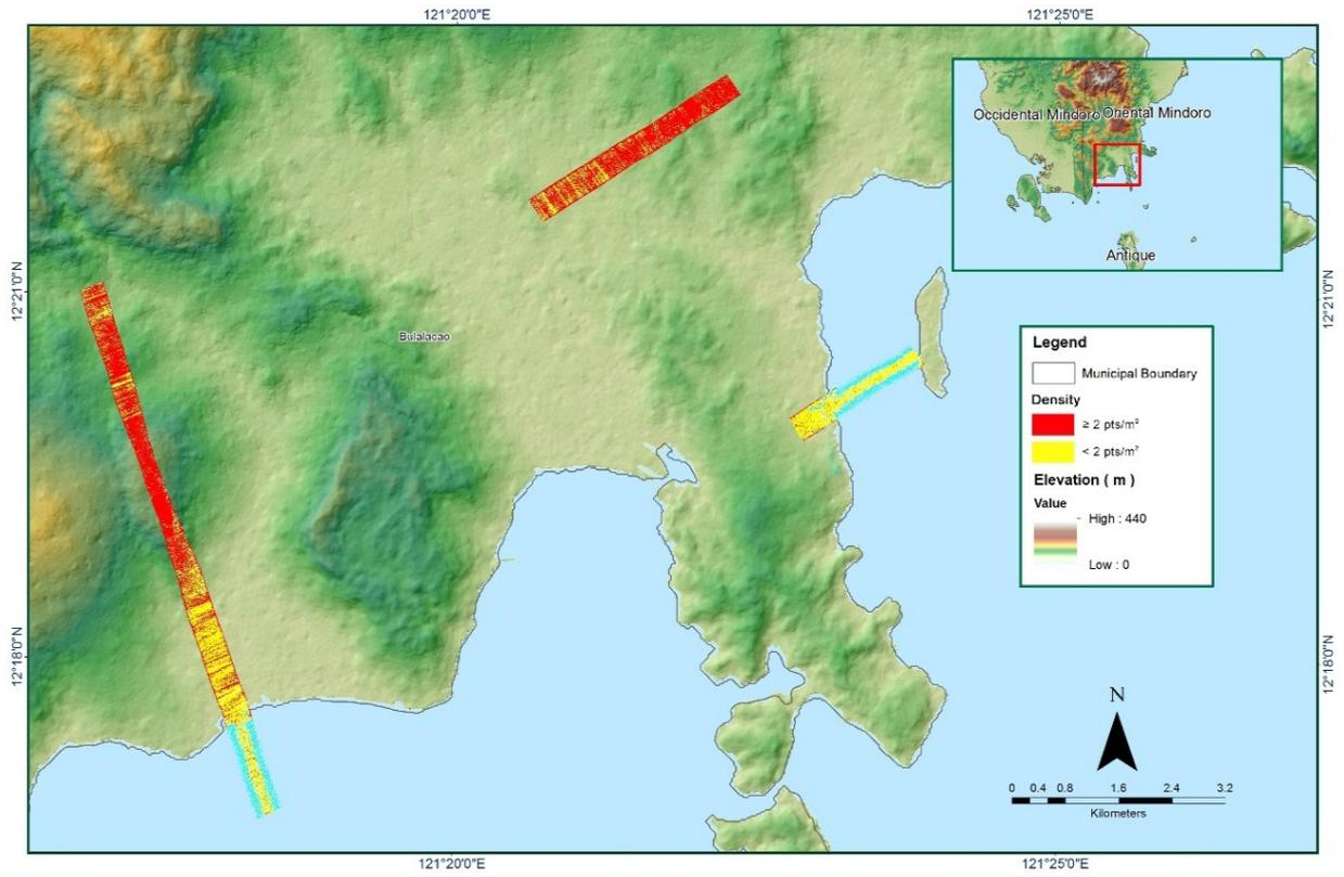
Figure A-8.13. Density of merged LiDAR data
