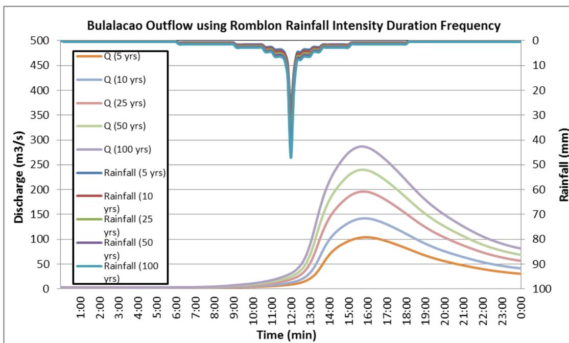
Figure 62. Outflow hydrograph at Bulalacao Station generated using Romblon RIDF simulated in HEC-HMS
