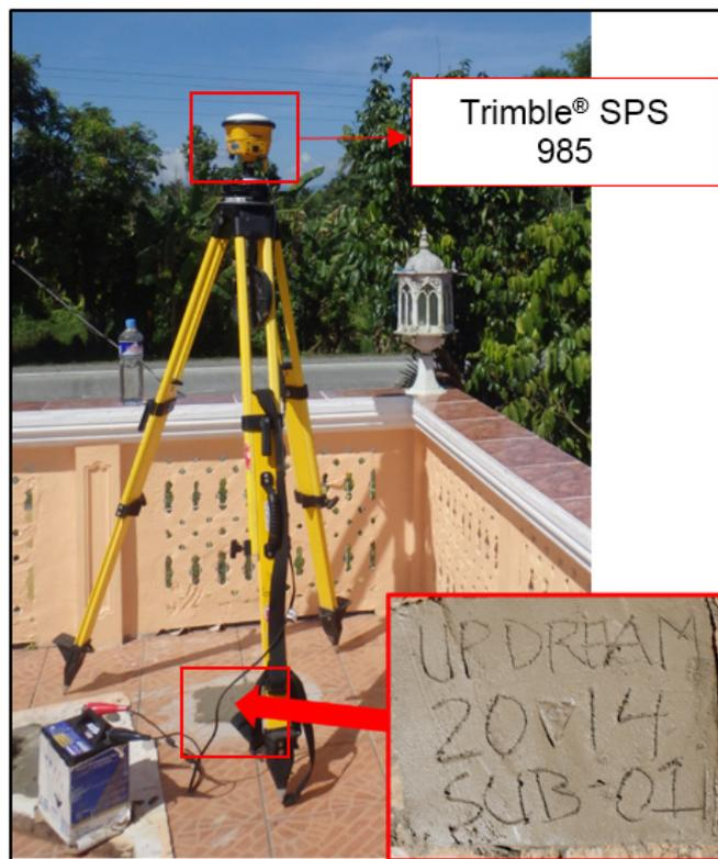
Figure 36. GPS setup of Trimble® SPS 985 at SUB-1, an established control point located at Maramot Residence in Brgy. Subaan, Municipality of Socorro, Oriental Mindoro
