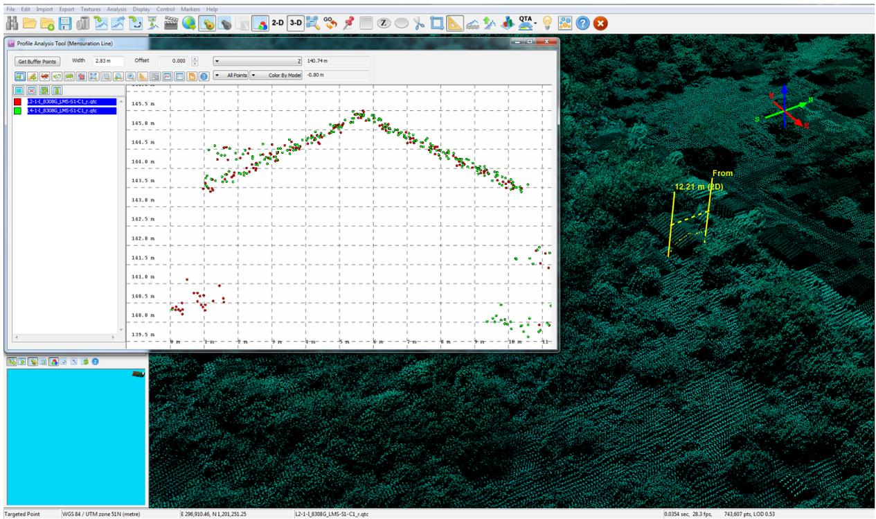
Figure 14. Quality checking for Bulalacao flight 8308G using the Profile Tool of QT Modeler.
