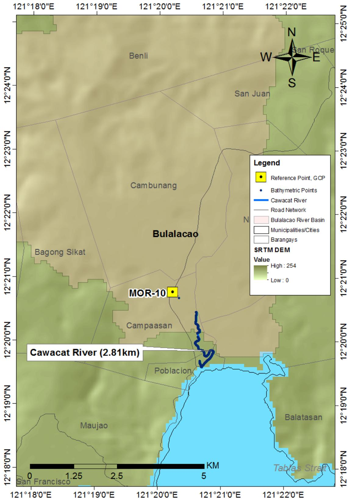
Figure 46. Bathymetric survey of Bulalacao River
