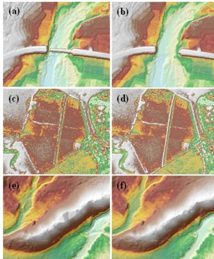
Figure 20. Portions in the DTM of Bulalacao floodplain – a bridge before (a) and after (b) manual editing; a paddy field before (c) and after (d) data retrieval; a highland before (e) and after (f) manual editing.
