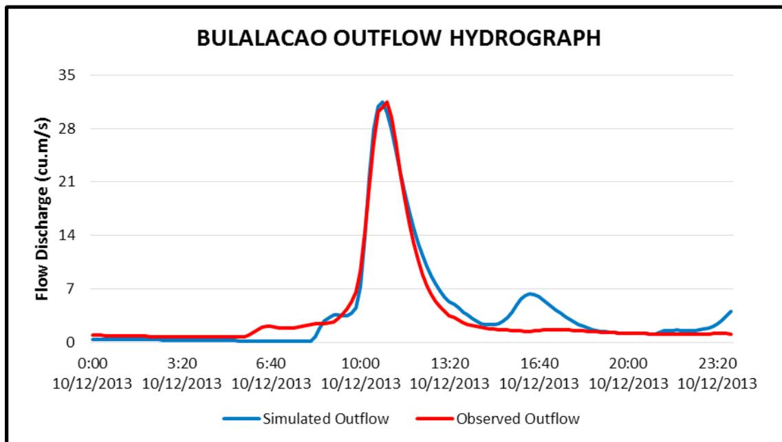
Figure 61. Outflow Hydrograph of Bulalacao produced by the HEC-HMS model compared with observed outflow.
