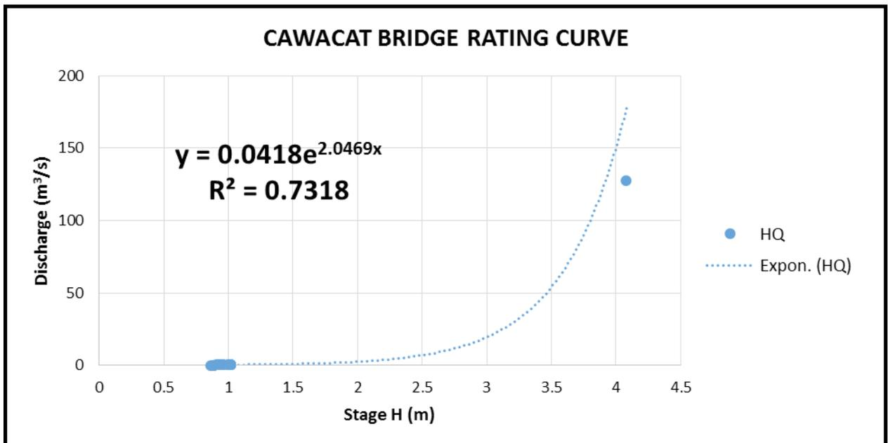
Figure 50. Rating curve at Cawacat Bridge, Bulalacao, Oriental Mindoro
