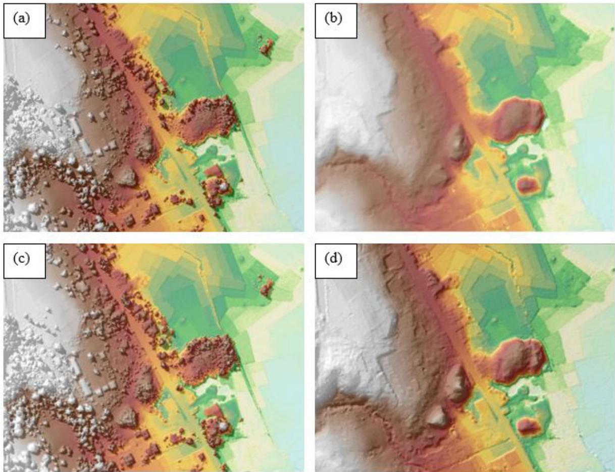
Figure 17. The production of last return DSM (a) and DTM (b), first return DSM (c) and secondary DTM (d) in some portion of Bulalacao floodplain.
