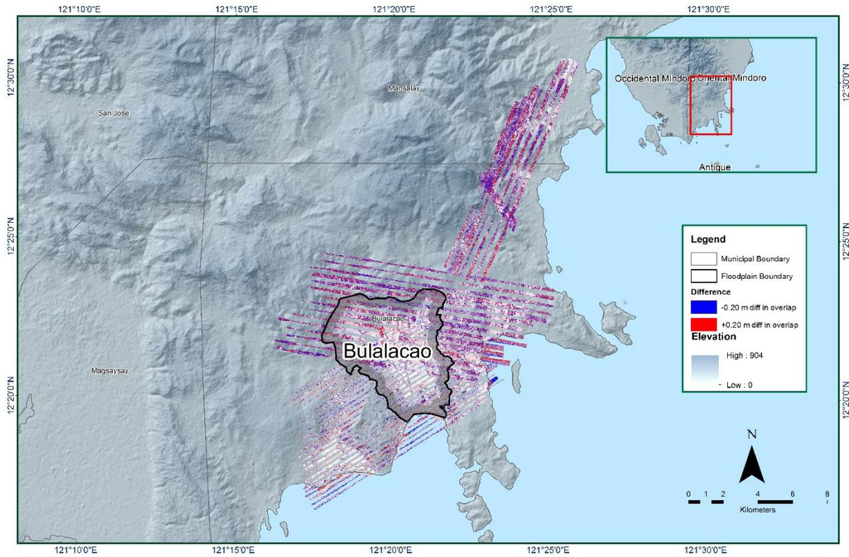
Figure 13. Elevation difference map between flight lines for Bulalacao Floodplain.
