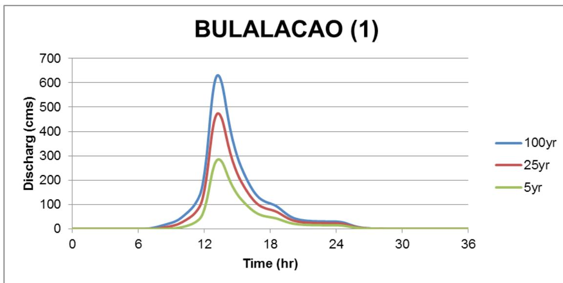
Figure 63. Bulalacao river (1) generated discharge using 5-, 25-, and 100-year Romblon rainfall intensity-duration-frequency (RIDF) in HEC-HMS
