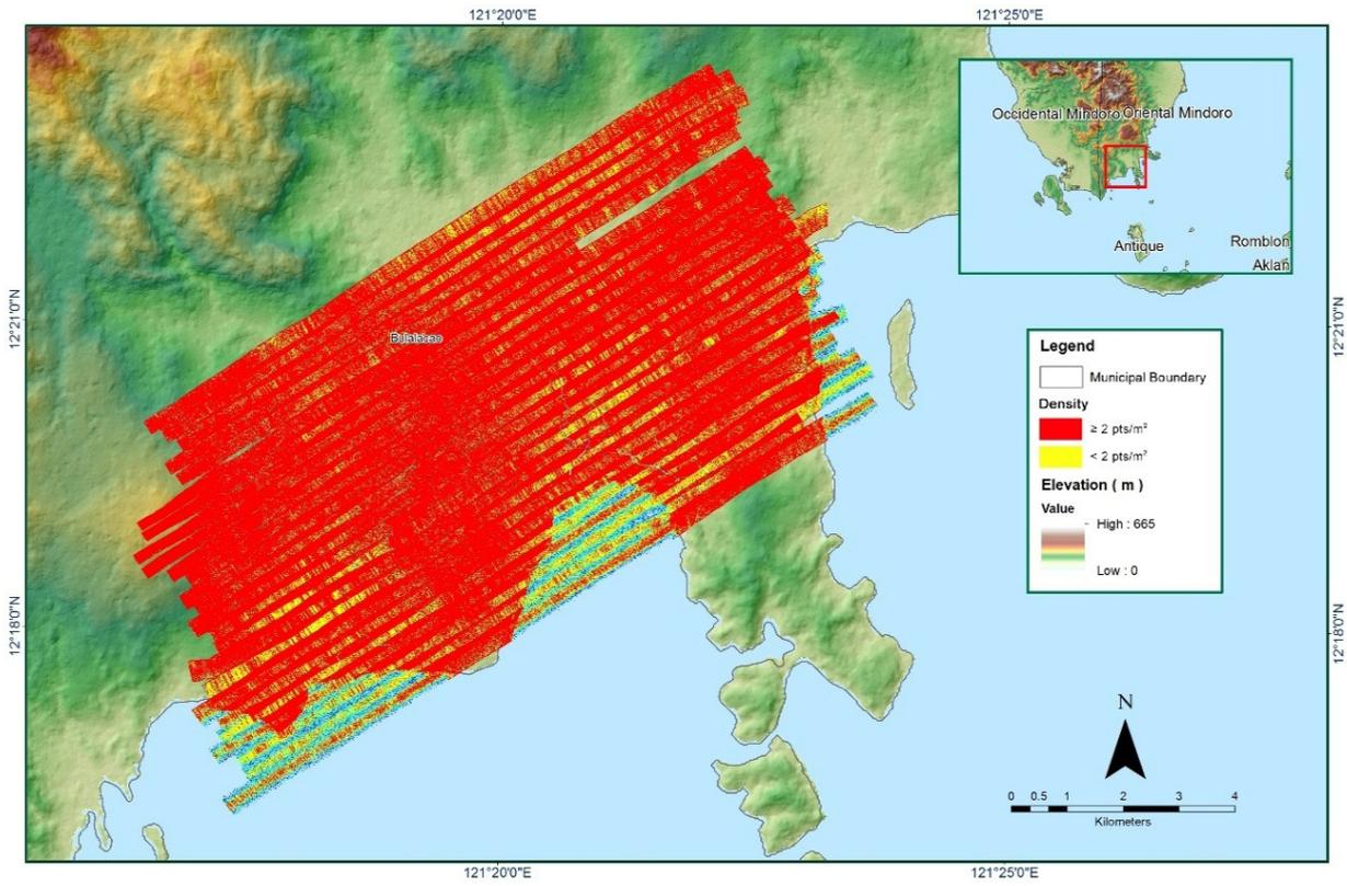
Figure A-8.6 Density of merged LiDAR data
