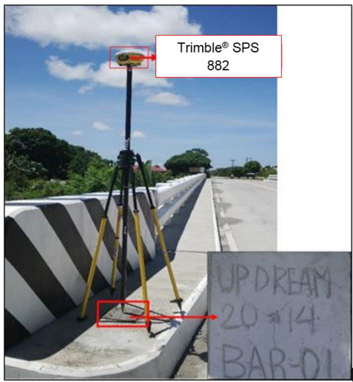
Figure 30. GNSS setup of Trimble® SPS 882 on BONG-01 in Brgy. San Isidro, Municipality of Bongabong, Oriental Mindoro
