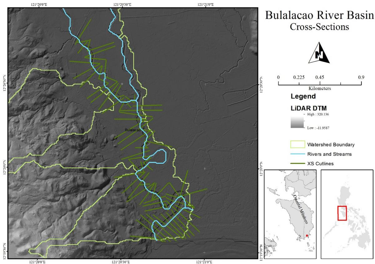
Figure 59. River cross-section of Bulalacao River generated through Arcmap HEC GeoRAS tool
