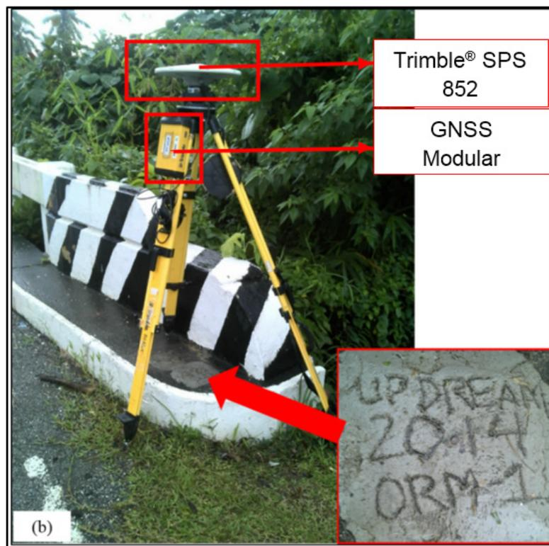
Figure 33. GPS setup of Trimble® SPS 852 at ORM-1, located on Subaan Bridge, Brgy. Subaan, Municipality of Socorro, Oriental Mindoro
