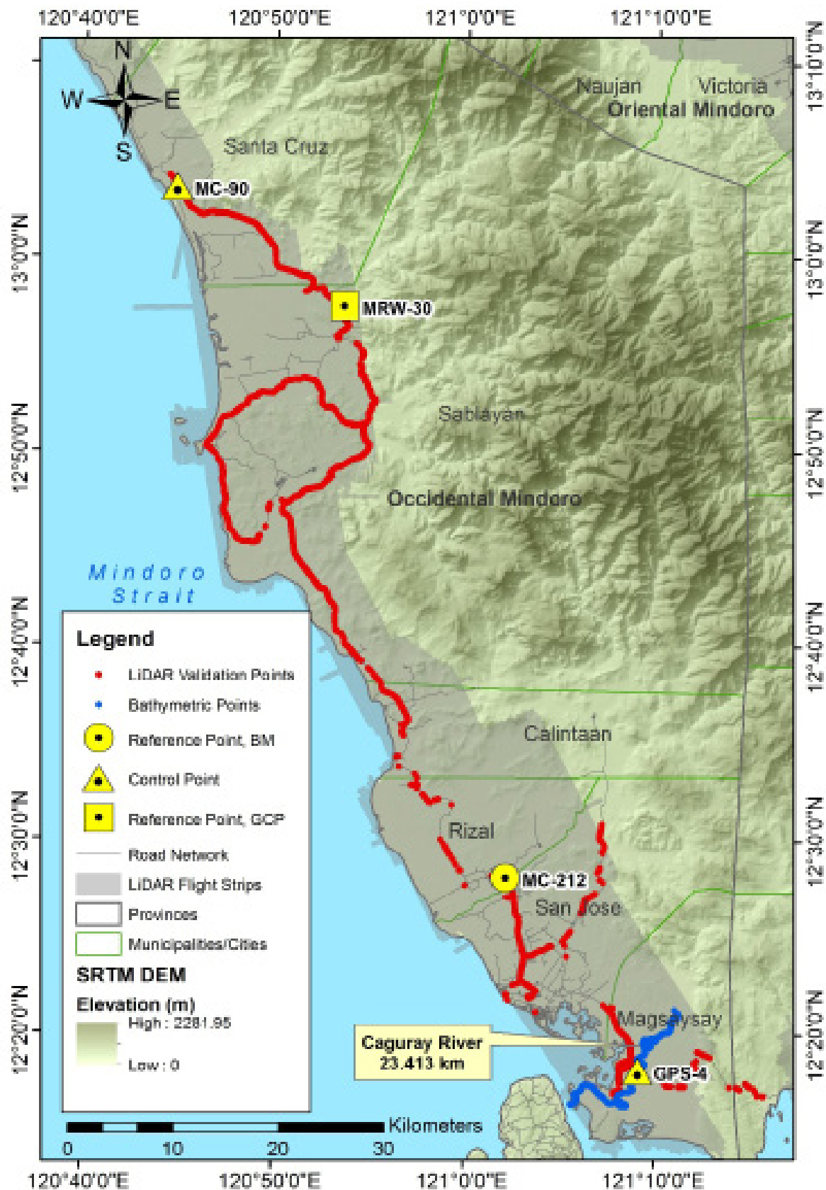
Figure 44. Validation point acquisition survey of Caguray River Basin
