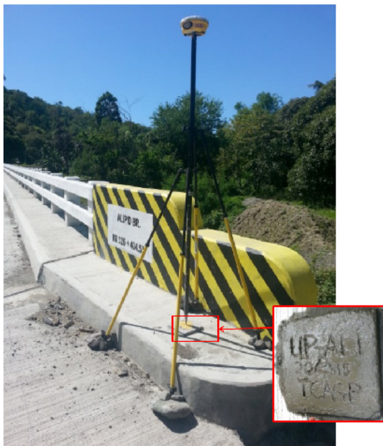
Figure 37. GNSS receiver set up, Trimble® SPS 882, at UP-ALI, Alipid Bridge approach in Brgy. Sto. Niño, Municipality of Sablayan, Occidental Mindoro
