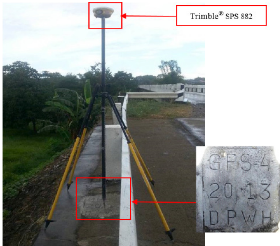
Figure 34. GNSS receiver, Trimble® SPS 882, at GPS-4 on right side of the road abutment after Caguray Bridge going to Bulalacao in Brgy. Poblacion, Municipality of Magsaysay, Occidental Mindoro
