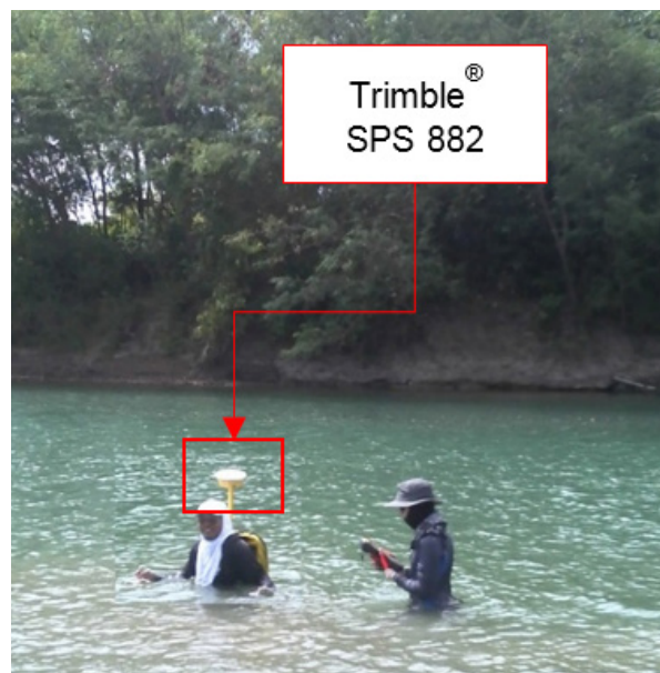
Figure 46. Manual bathymetric survey in Caguray River
