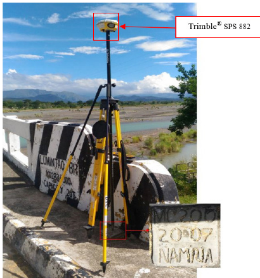
Figure 31. GNSS base receiver, Trimble® SPS 882, setup at UP-ILA in Ilaya Bridge, Brgy. Ilaya, Dapitan City
