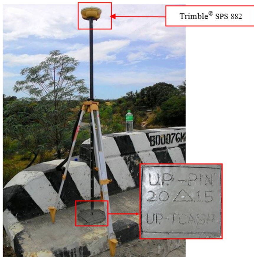
Figure 35. GNSS base receiver set-up, Trimble® SPS 882, at UP-PIN Pinamanaan Bridge approach in Brgy. Mapaya, Municipality of San Jose, Occidental Mindoro
