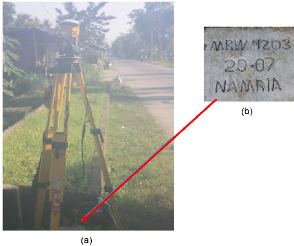
Figure 5. GPS set-up over MRW-4203 as recovered front of the barangay hall of Brgy. Mapaya, municipality of San Jose, Occidental Mindoro (a) and NAMRIA reference point MRW-4203 (b) as recovered by the field team.
