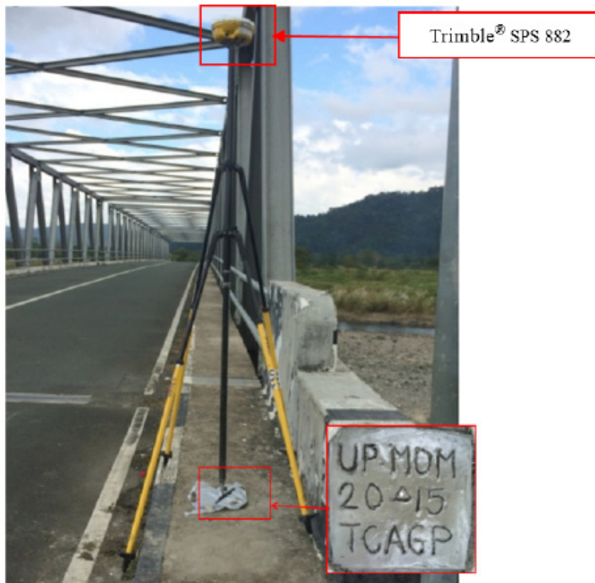
Figure 36. GNSS receiver set-up, Trimble® SPS 882, at UP-MOM, Mompong Bridge approached in Brgy. Lumang Bato, Municipality of Sablayan, Occidental Mindoro
