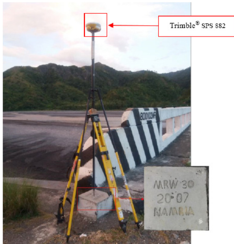
Figure 30. GNSS receiver setup, Trimble® SPS 882, at MRW-30 Amnay Bridge approach in Sitio Kabangkalan, Brgy. Pinagturilan, Municipality of Santa Cruz, Occidental Mindoro
