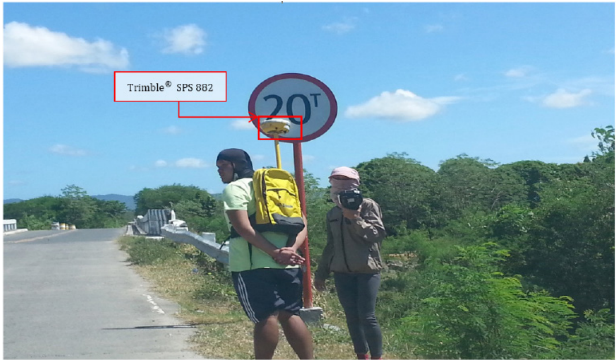
Figure 38. As-built survey at Caguray Bridge, Brgy. Poblacion, Municipality of Magsaysay
