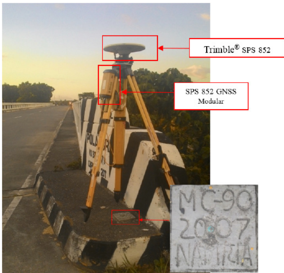
Figure 33. GNSS base, Trimble® SPS 852, at MC-90, used as marker, located at the Pola Bridge approach in Brgy. Barahan, Municipality of Santa Cruz, Occidental Mindoro
