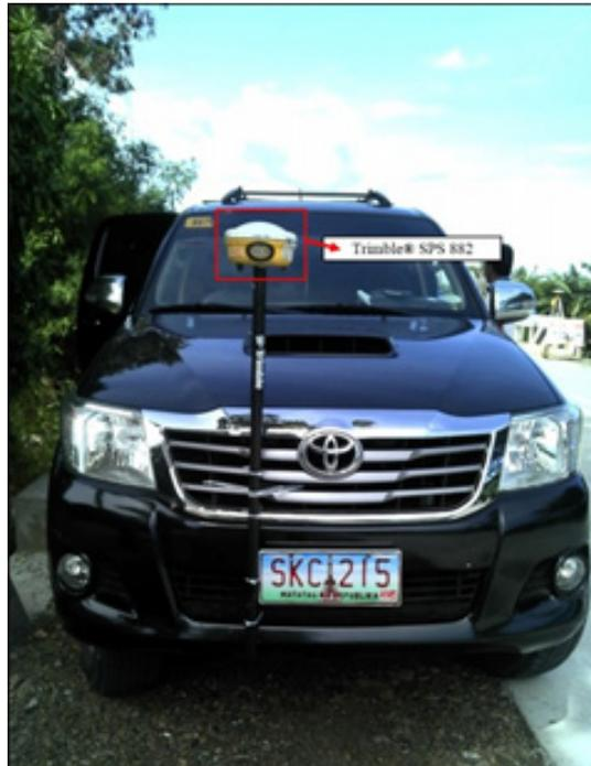
Figure 39. Validation points acquisition survey setup by the survey team: A Trimble® SPS 882 is mounted in a 2 m pole and attached in front of the vehicle
