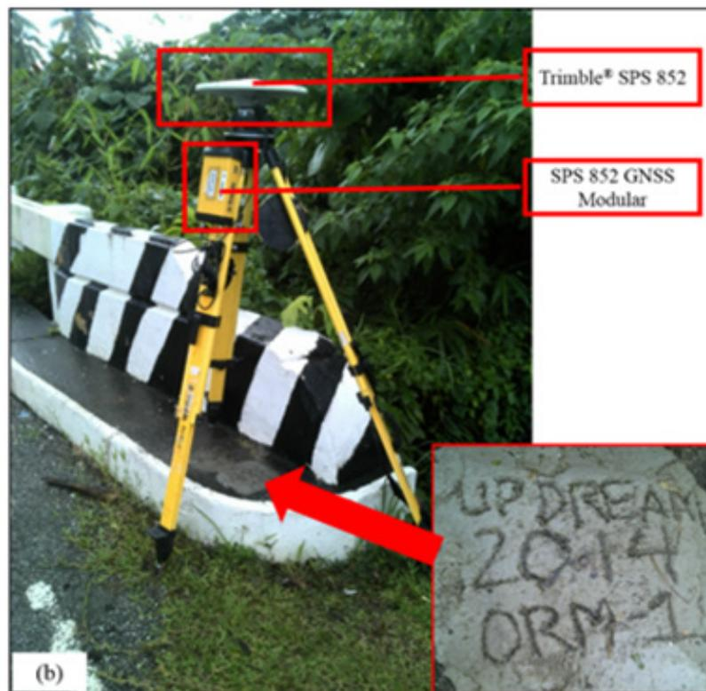
Figure 31. GNSS receiver Trimble® SPS 852 setup at ORM-1, located at Subaan Bridge in Barangay Subaan, Municipality of Socorro, Oriental Mindoro
