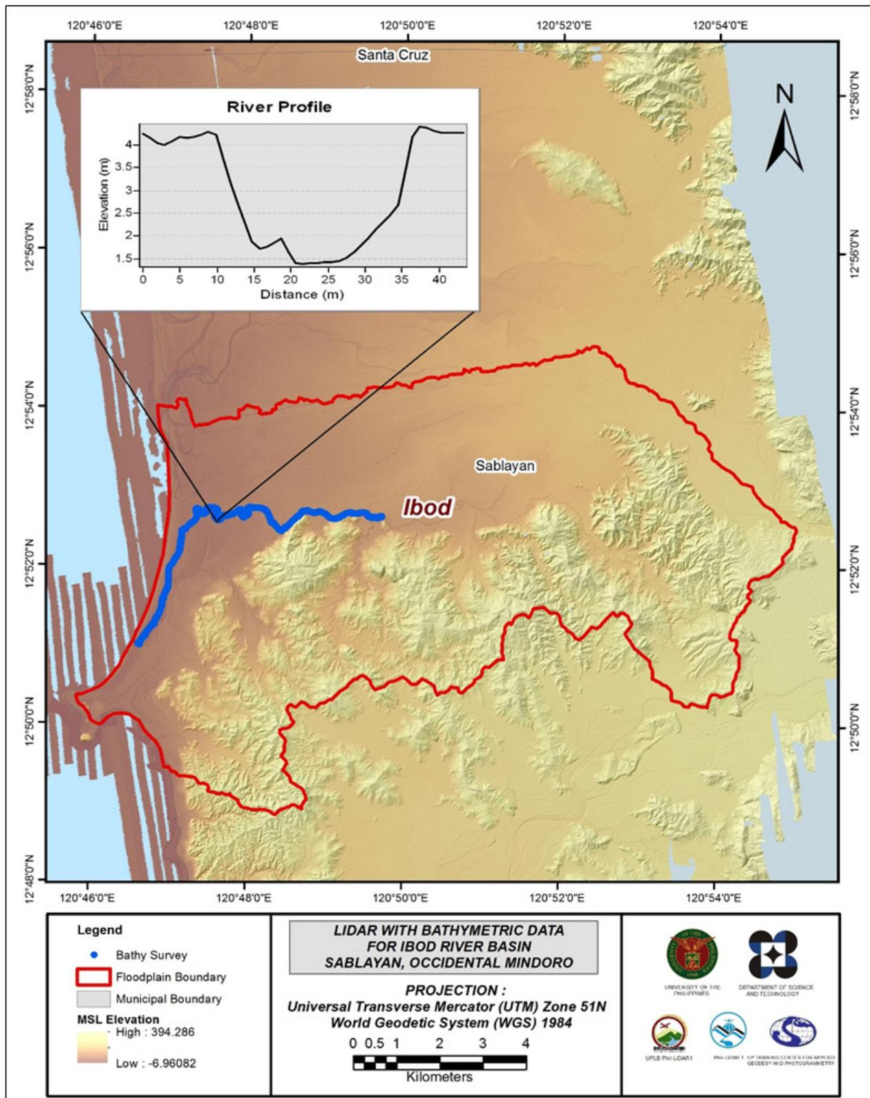
Figure 28. Map of Ibod Floodplain with bathymetric survey points shown in blue.
