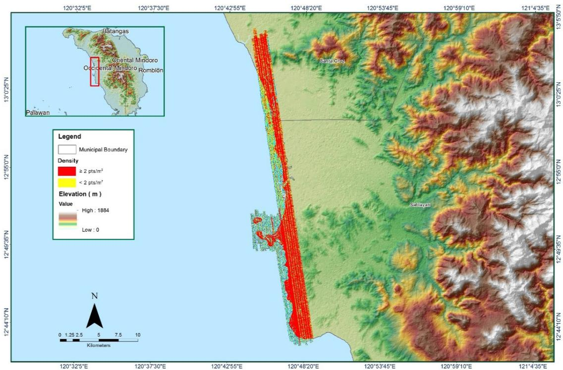
Figure A-8.6 Density of merged LiDAR data
