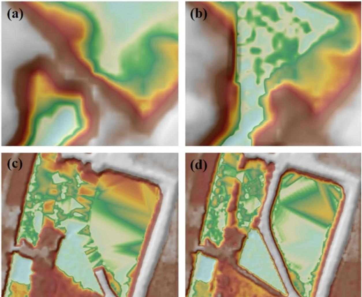
Figure 23. Portions in the DTM of Ibod Floodplain – a land bridge before (a) and after (b) data interpolation and a flattened area before (a) and after (b) data retrieval.
