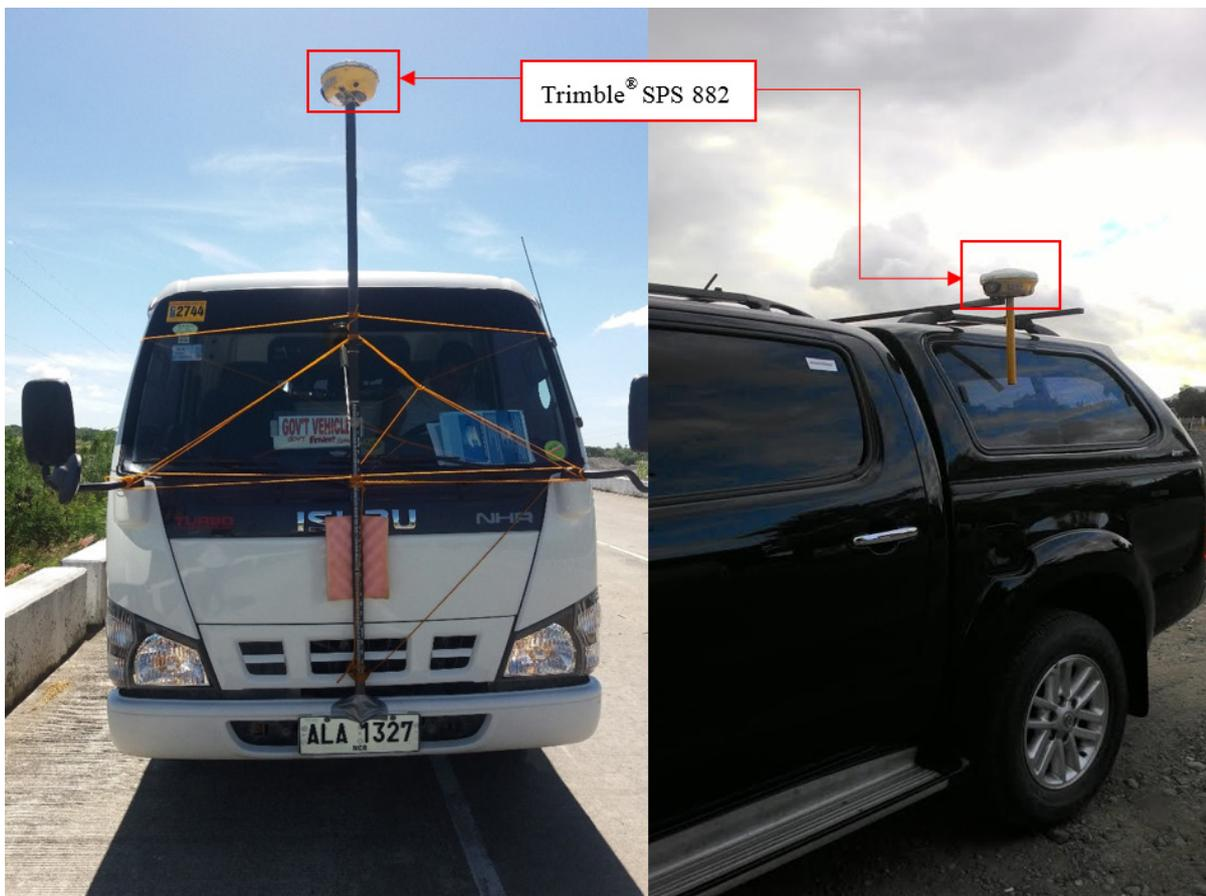
Figure 45. Validation points acquisition survey set-up for Ibod River
