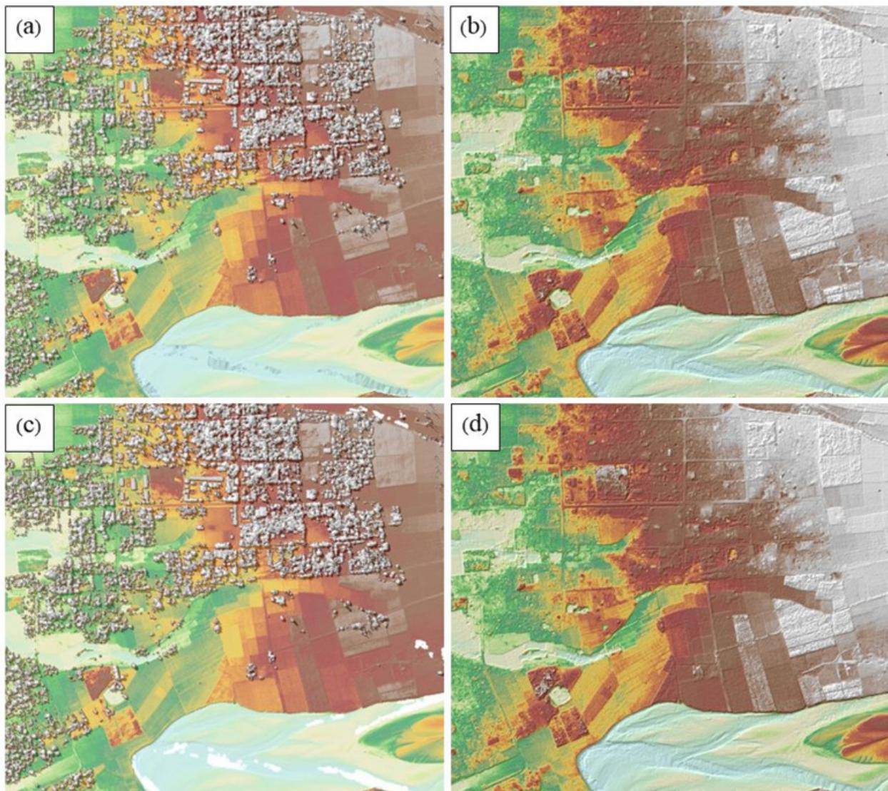
Figure 20. The production of last return DSM (a) and DTM (b), first return DSM (c) and secondary DTM (d) in some portion of Ibod floodplain.
