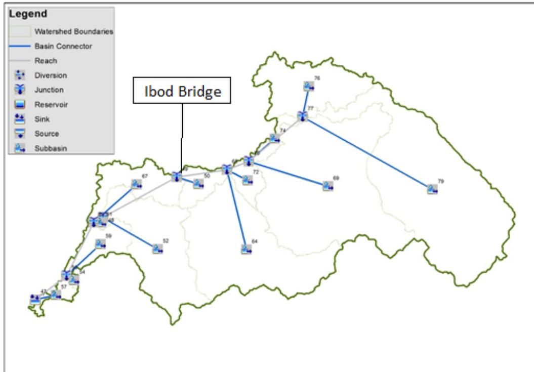
Figure 60. HEC-HMS generated Ibod River Basin Model.
