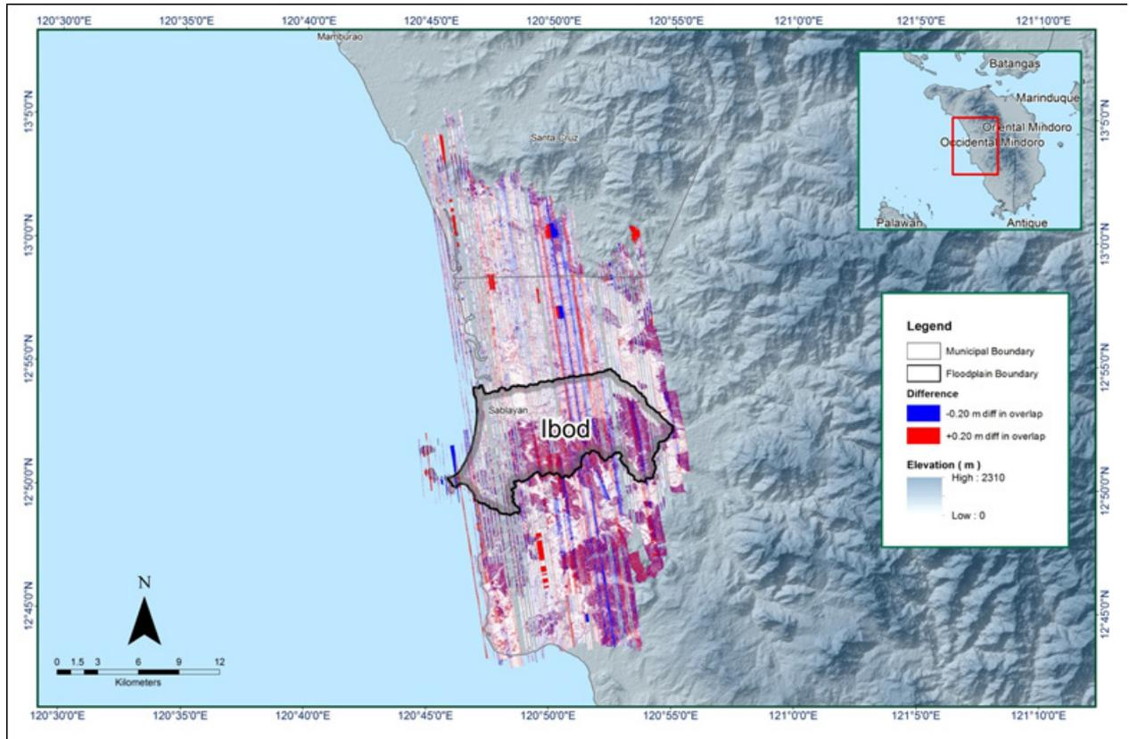
Figure 16. Elevation difference map between flight lines for Baroc Floodplain.
