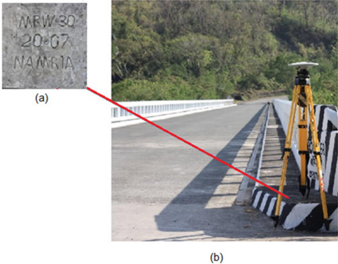
Figure 4. NAMRIA reference point MRW-30 (a) as recovered by the field team and GPS set-up over MRW-30 in Amnay Bridge in Brgy. Pinagturilan, municipality of Sta. Cruz, Occidental Mindoro (b).
