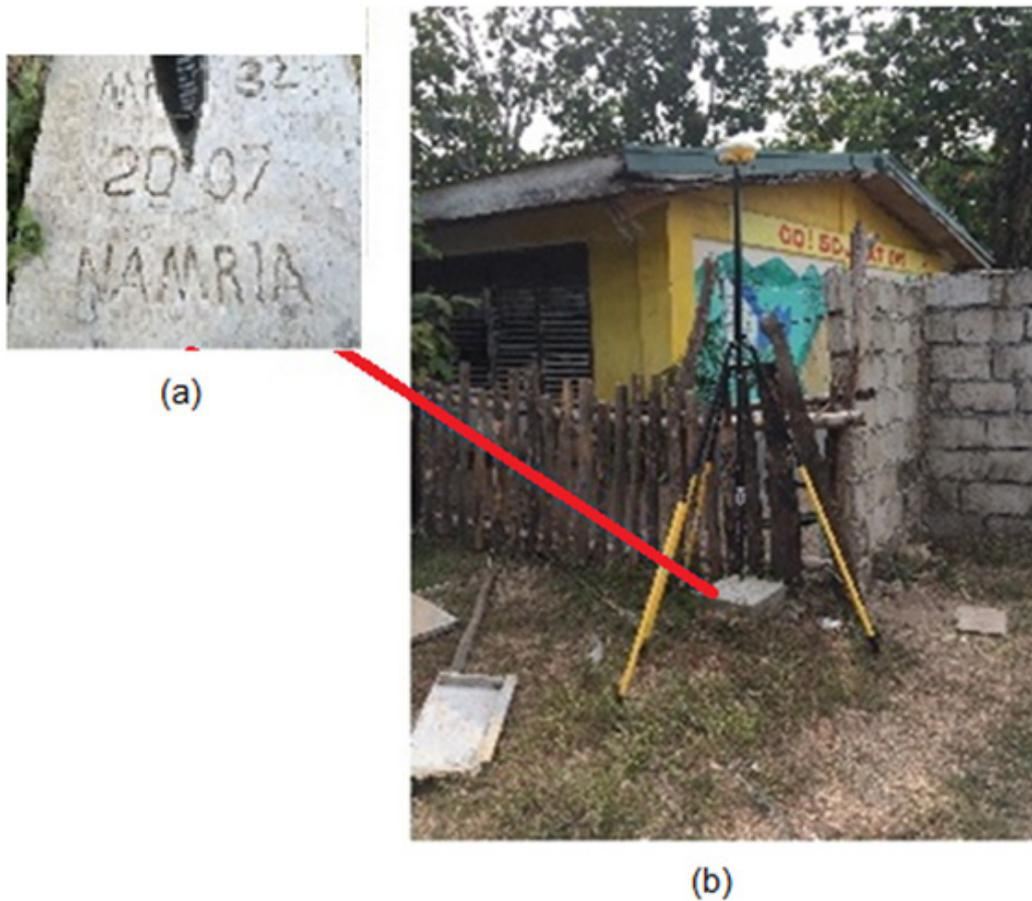
Figure 5. NAMRIA reference point MRW-32 (a) as recovered by the field team and GPS set-up over MRW-32 in the corner of a day care center in Brgy. Fatima, municipality of Mamburao, Occidental Mindoro (b).
