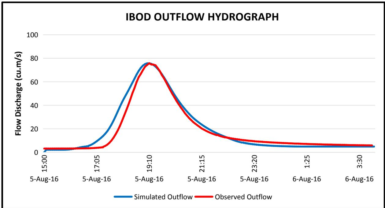
Figure 63. Outflow Hydrograph of Ibod produced by the HEC-HMS model compared with observed outflow.
