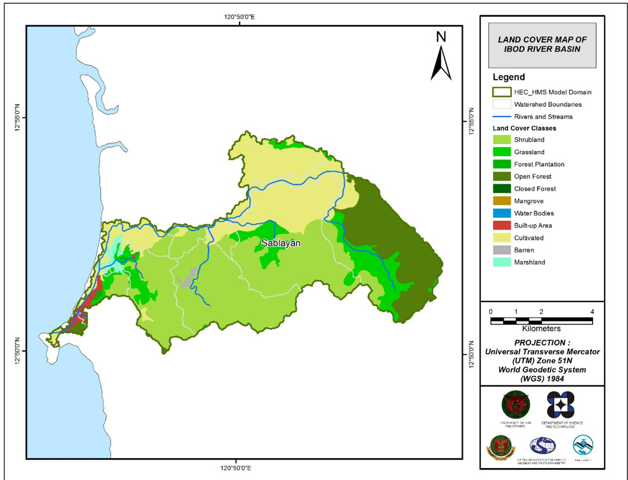
Figure 57. Land cover map of Ibod River Basin used for the estimation of the CN and watershed lag parameters of the rainfall-runoff model. (Source: NAMRIA)
