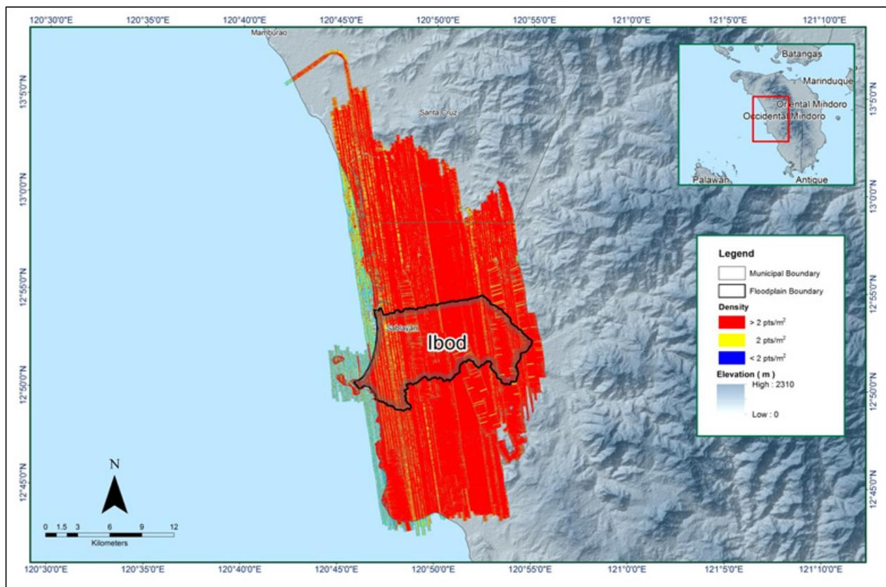
Figure 15. Pulse density map of merged LiDAR data for Ibod Floodplain.
