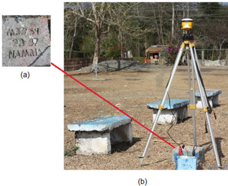
Figure 7. NAMRIA reference point MRW-54 (a) as recovered by the field team and GPS set-up over MRW-54 as recovered in near basketball open court in Brgy. Malisbong, municipality of Sablayan, Occidental Mindoro (b).
