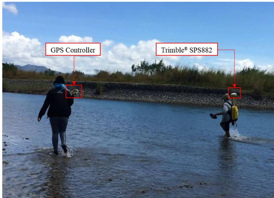
Figure 47. Bathymetry set-up and execution for Ibod River
