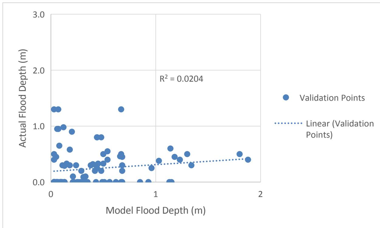
Figure 79. Flood map depth vs. actual flood depth
