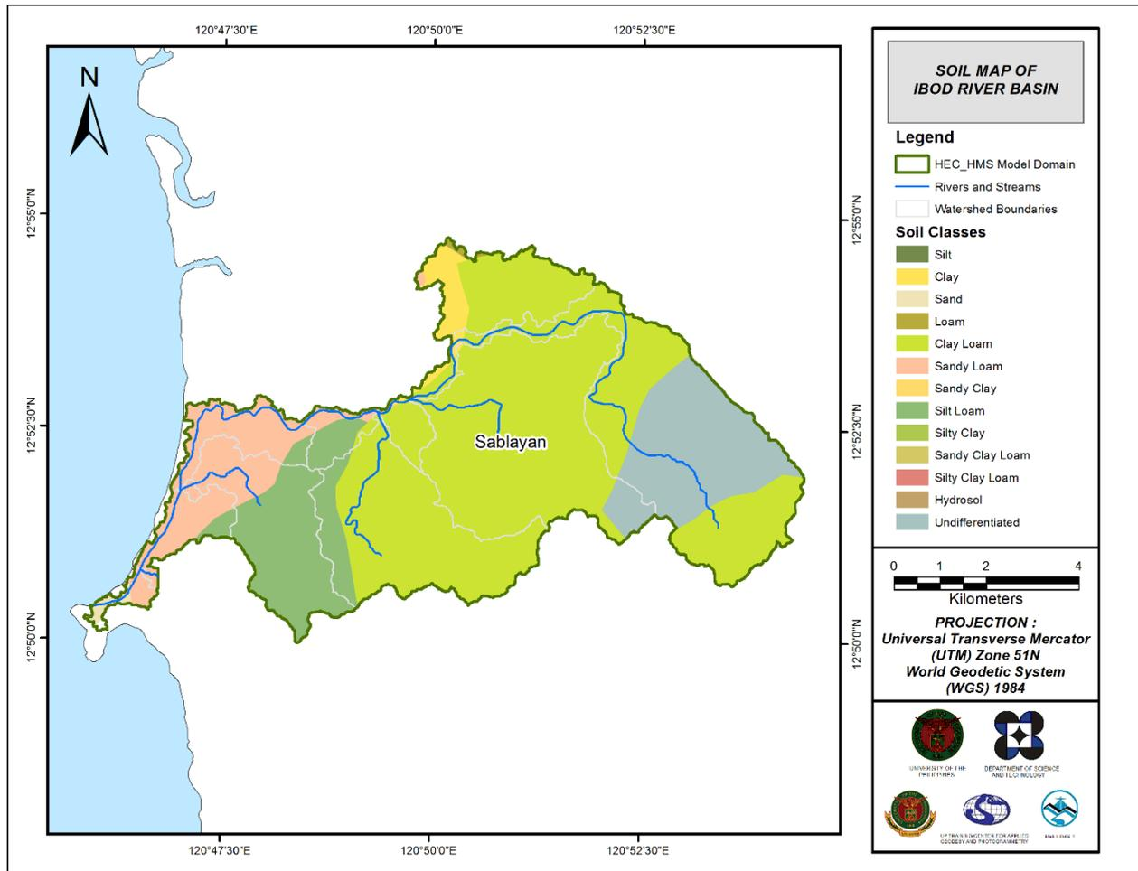
Figure 56. Soil map of Ibod River Basin used for the estimation of the CN parameter. (Source: DA)
