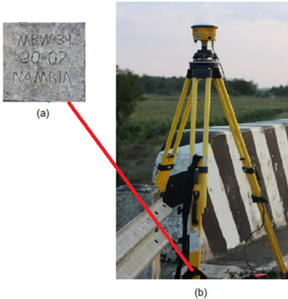
Figure 6. NAMRIA reference point MRW-34 (a) as recovered by the field team and GPS set-up over MRW-34 in Balibago Bridge in Brgy. Armado, municipality of Abra de Ilog, Occidental Mindoro (b).
