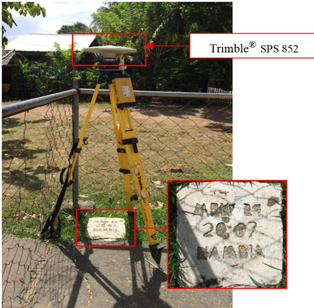
Figure 31. GNSS receiver set-up, Trimble® SPS 852, at MRW-24 in front of Iriron Elementary School in Brgy. Iriron, Municipality of Calintaan, Occidental Mindoro
