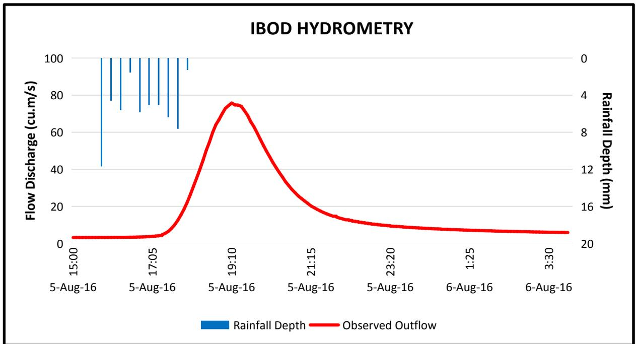
Figure 53. Rainfall and outflow data at Ibod River Basin used for modeling
