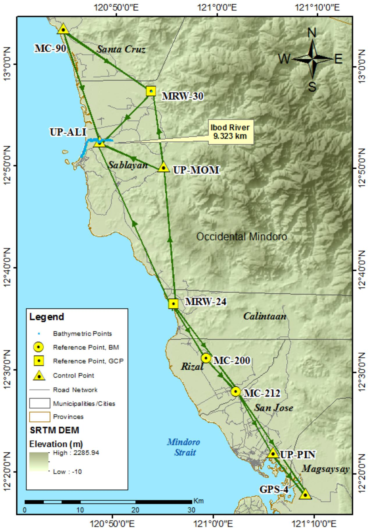
Figure 30. GNSS Network covering Ibod River
