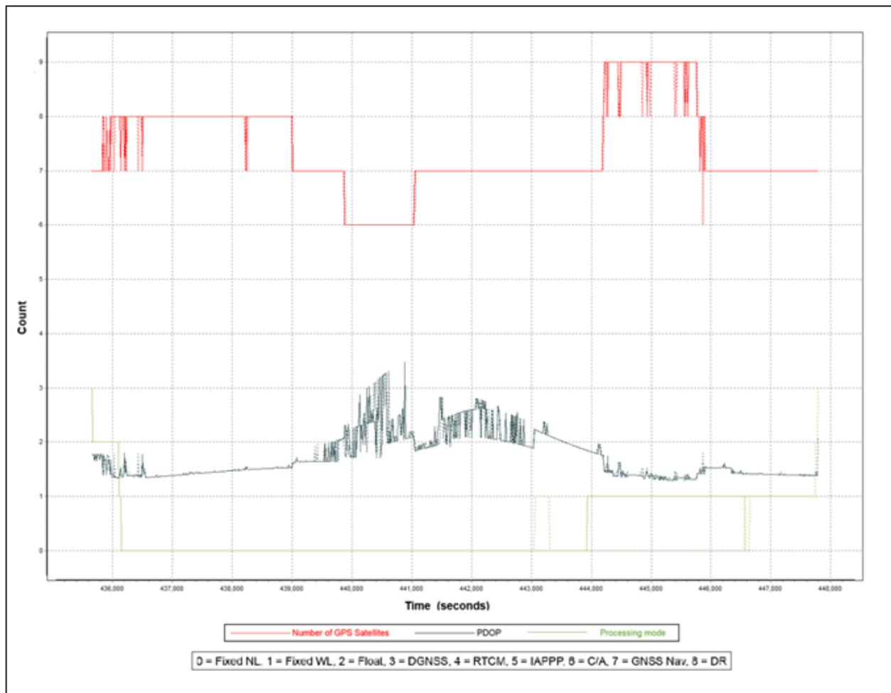
Figure 11. Solution Status Parameters of Ibod Flight 1128A.
