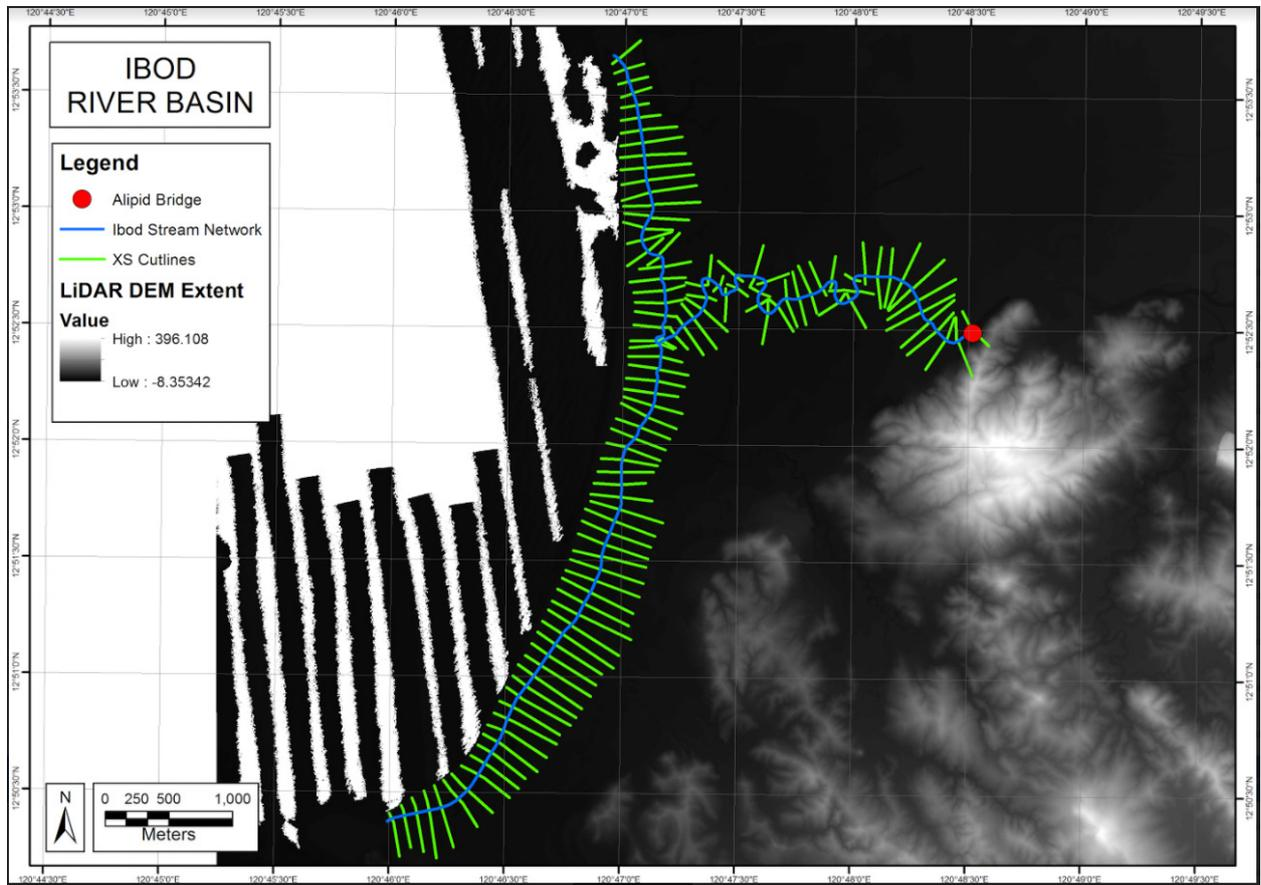
Figure 61. River cross-section of Ibod River generated through Arcmap HEC GeoRAS tool
