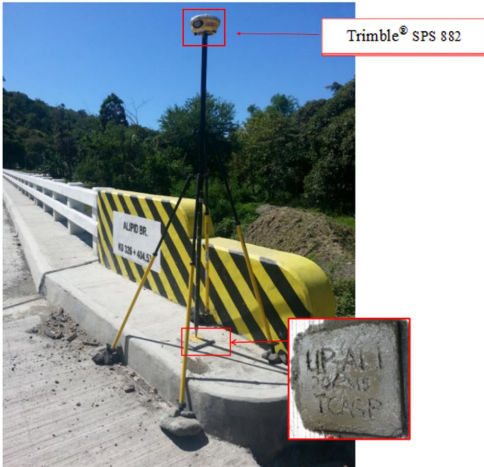
Figure 39. GNSS receiver set up, Trimble® SPS 882, at UP-ALI, Alpid Bridge approach in Brgy. Sto. Niño, Municipality of Sablayan, Occidental Mindoro
