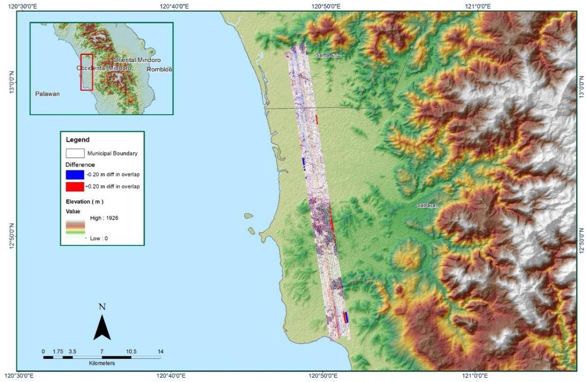
Figure A-8.21. Elevation difference between flight lines
