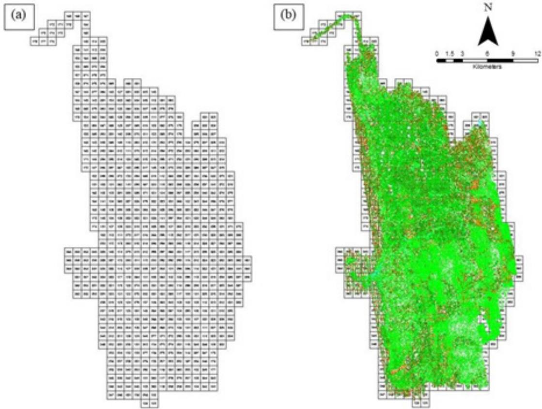
Figure 18. Tiles for Ibod Floodplain (a) and classification results (b) in TerraScan.
