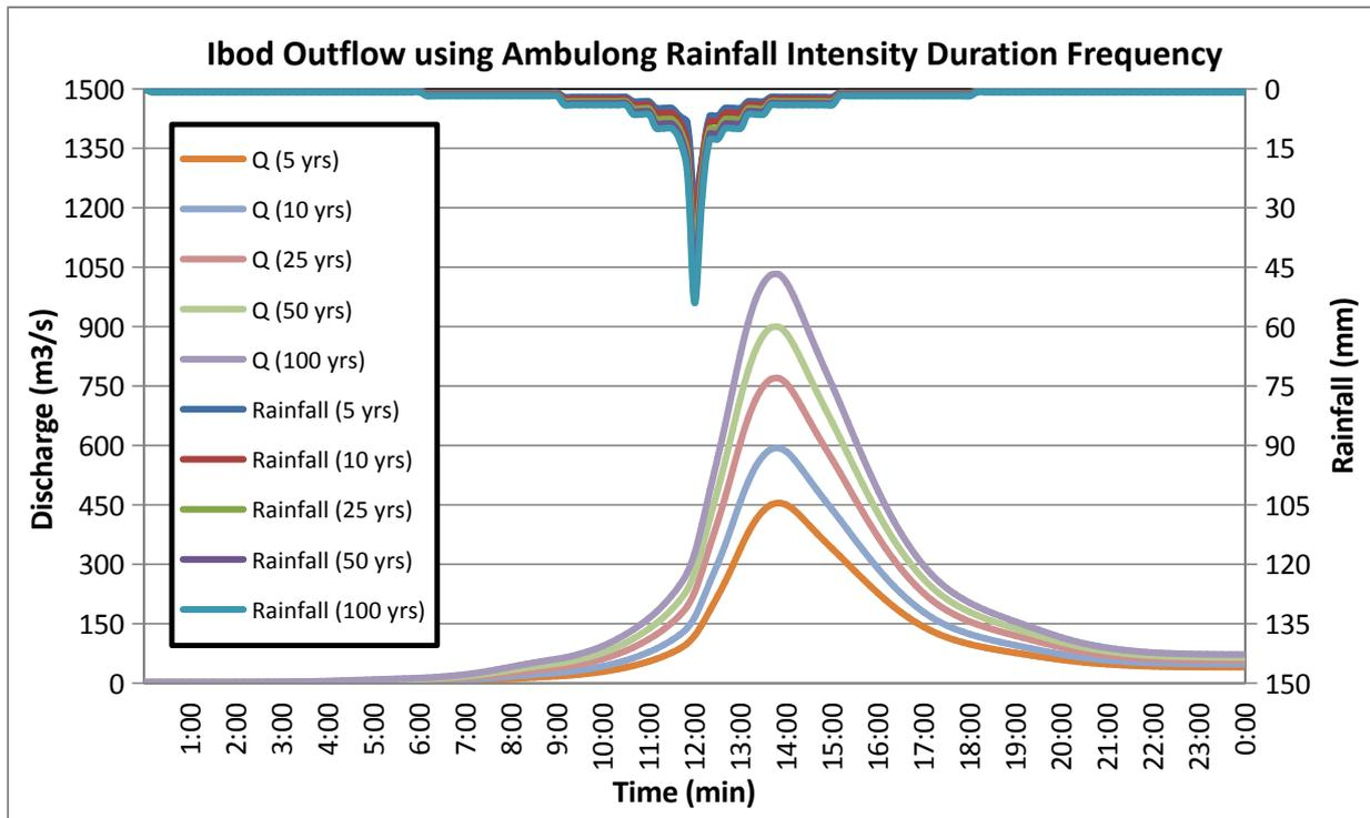
Figure 64. Outflow hydrograph at Ibod Station generated using Ambulong RIDF simulated in HEC-HMS
