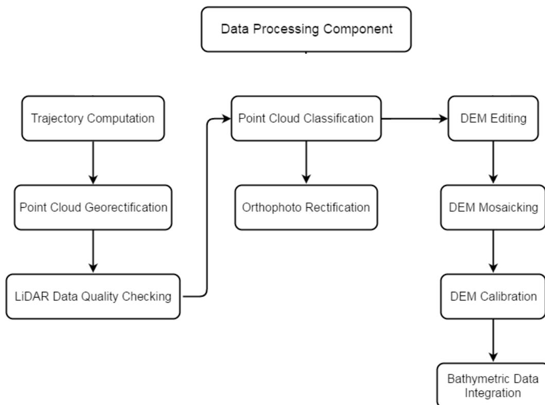
Figure 9. Schematic Diagram for Data Pre-Processing Component
