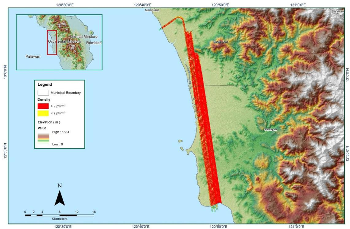
Figure A-8.13. Density of merged LiDAR data
