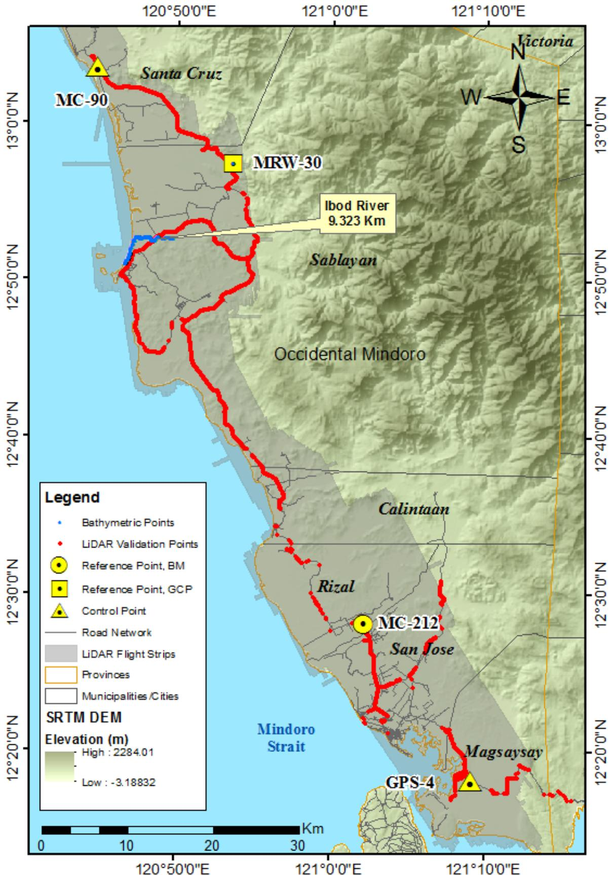
Figure 46. Validation point acquisition survey of Ibod River Basin
