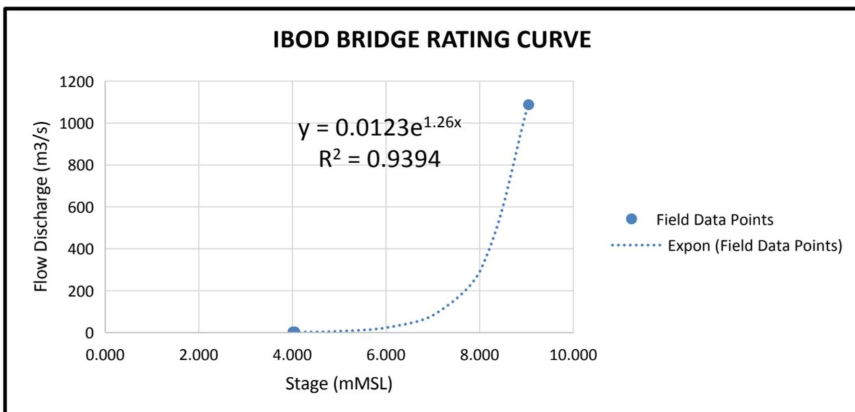
Figure 52. Rating curve at Ibod Bridge, Occidental Mindoro
