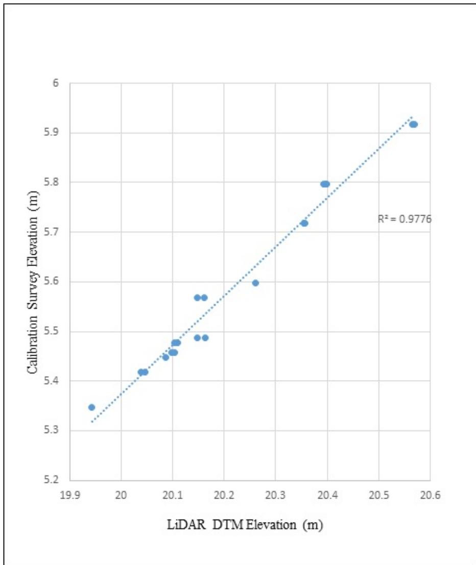
Figure 22 Correlation plot between calibration survey points and LiDAR data.
