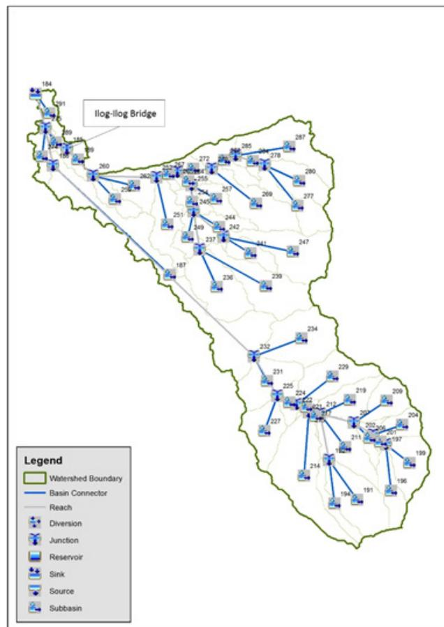
Figure 56 The Ilog-Ilog river basin model generated using HEC-HMS.
