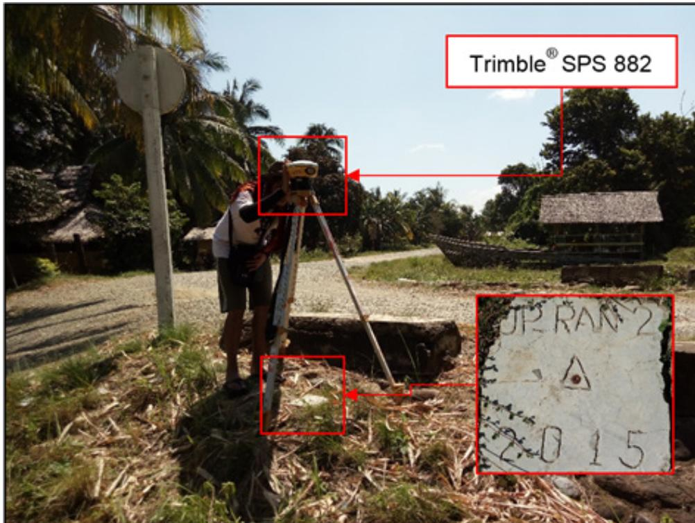
Figure 30. GNSS receiver set-up, Trimble® SPS 882, at UP\_RAN-2, located on a riprap near Ransang Bridge in Brgy. Ransang, Rizal, Province of Palawan.
