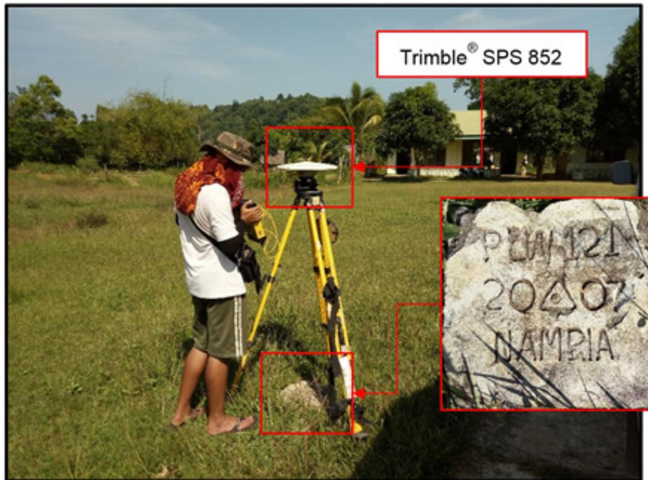
Figure 27. GNSS base set-up, Trimble® SPS 852, at PLW-121, located along the basketball court inside Cabcungan Elementary School in Brgy. Ransang, Rizal, Province of Palawan.
