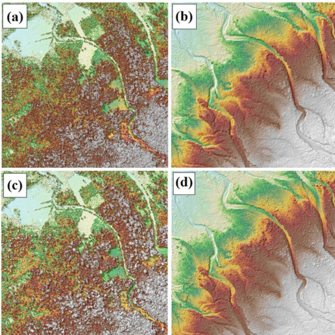
Figure 16 The production of last return DSM (a) and DTM (b), first return DSM (c) and secondary DTM (d) in some portion of Ilog-Ilog Floodplain.
