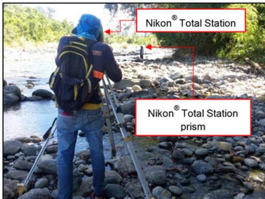
Figure 41. Manual bathymetric survey of ABSD along Ilog-Ilog River using a Nikon® Total Station.
