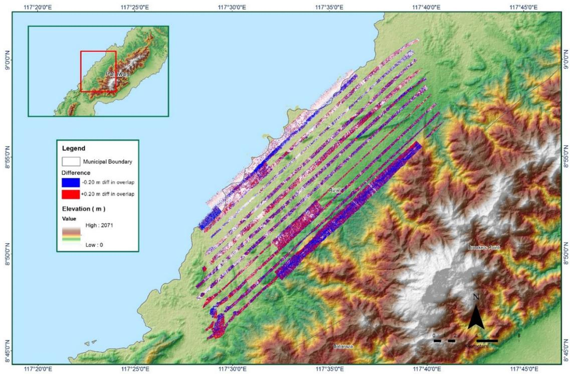
Figure A-8.21 Elevation difference between flight lines
