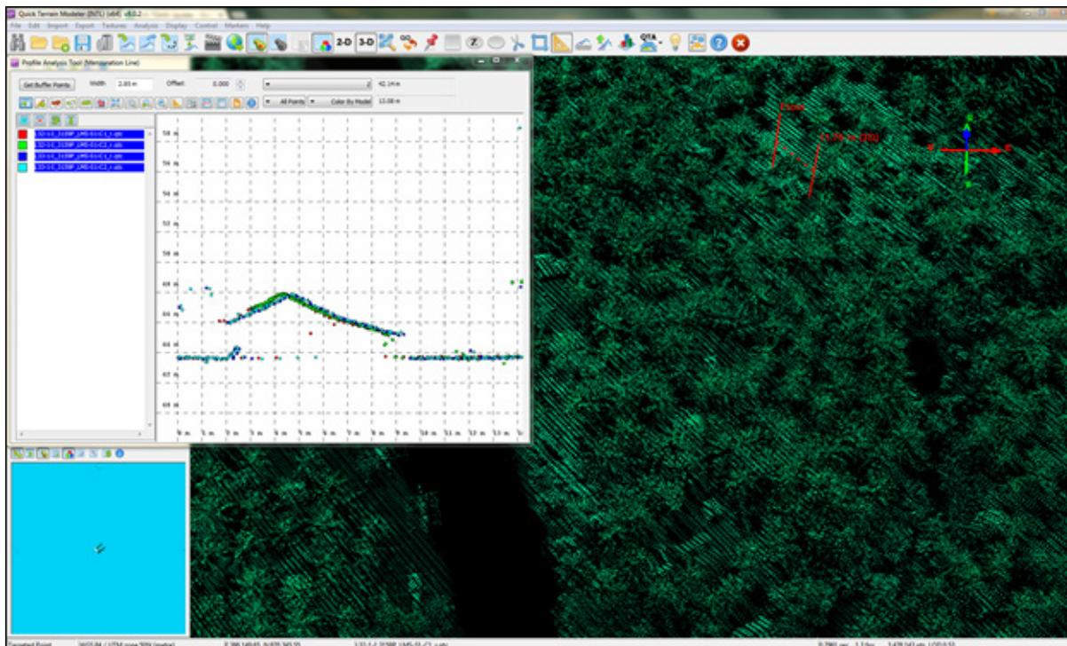
Figure 13 Quality checking for an Ilog-Ilog flight 3159P using the Profile Tool of QT Modeler.
