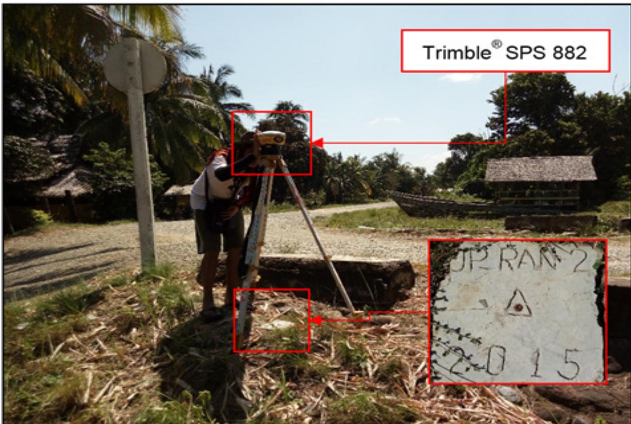
Figure 29. GNSS receiver set-up, Trimble® SPS 882, at UP\_ILO-1, located at the side of the railings near Ilog-Ilog Bridge in Brgy. Campong Ulay, Rizal, Province of Palawan.
