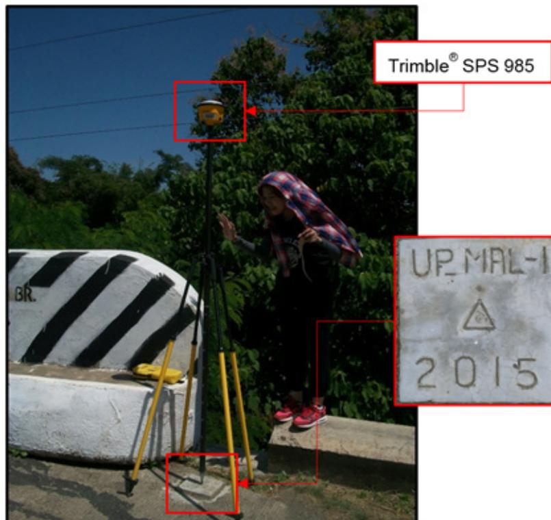
Figure 28 GNSS receiver set-up, Trimble® SPS 985, at UP\_MAL-1, located beside the approach of Malambunga Bridge in Brgy. Punta Baja, Rizal, Province of Palawan.
