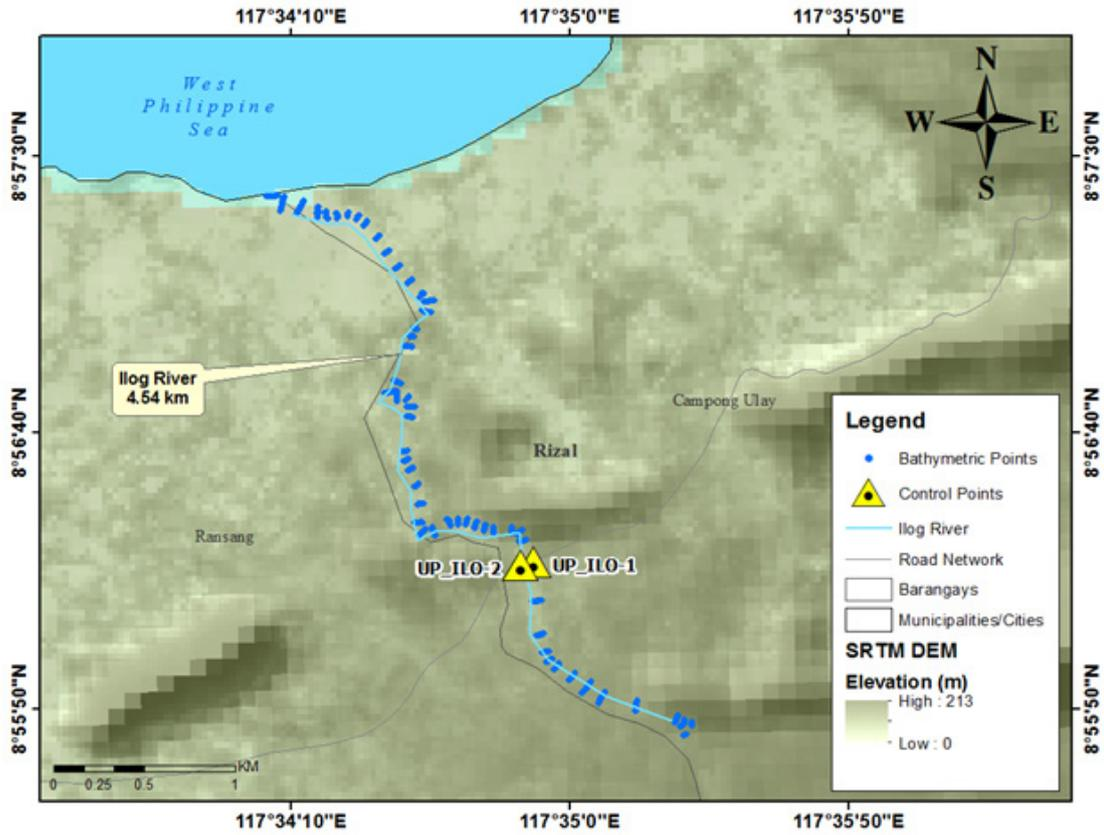
Figure 43. Bathymetric survey of Ilog-Ilog River.
