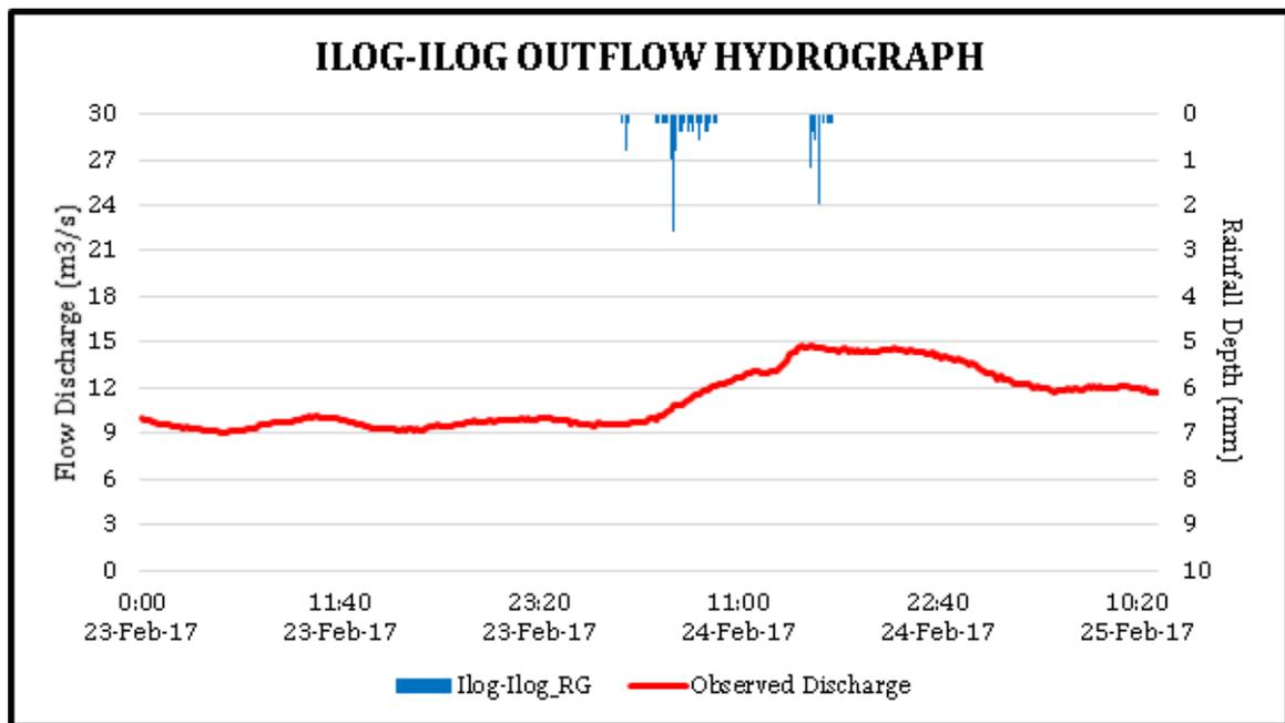
Figure 49. Rainfall and outflow data at Ilog-Ilog used for modeling.
