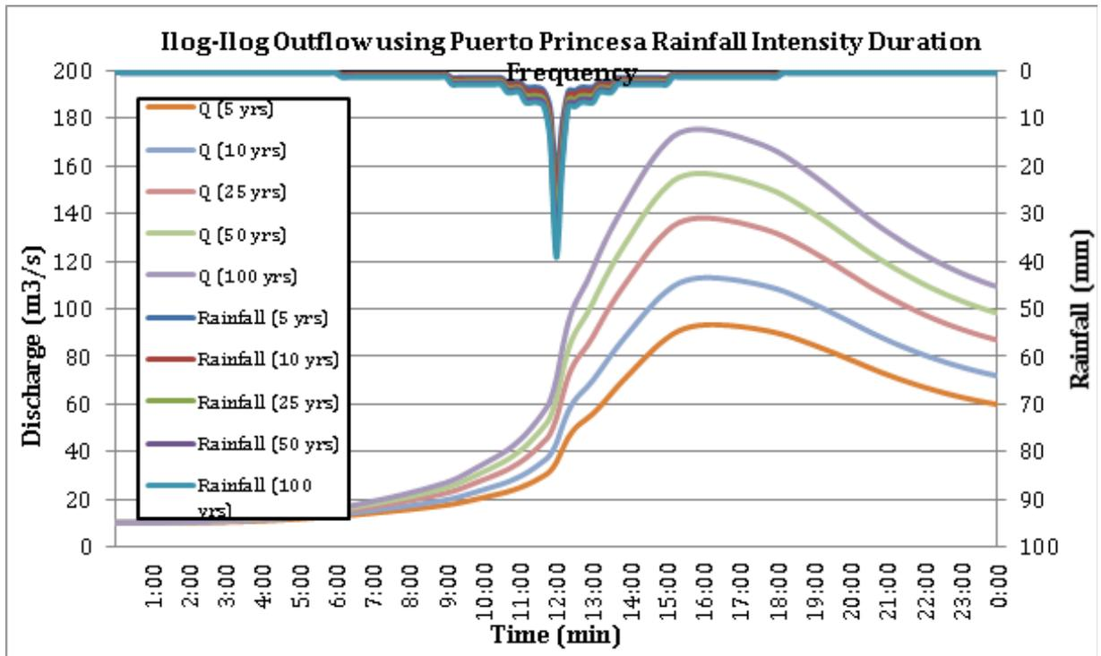
Figure 60 Outflow hydrograph at Ilog-Ilog Station generated using Puerto Princesa RIDF simulated in HEC-HMS.
