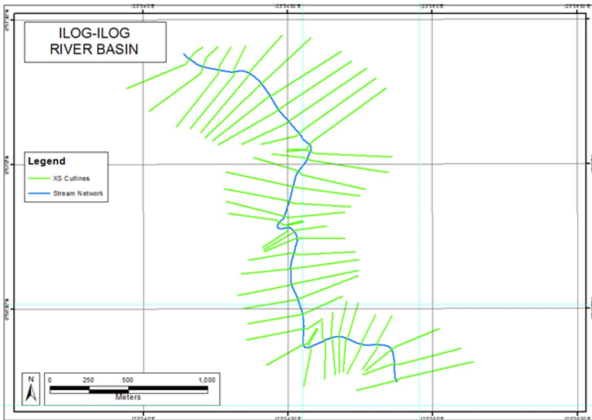
Figure 57 River cross-section of Ilog-Ilog River generated through Arcmap HEC GeoRAS tool.
