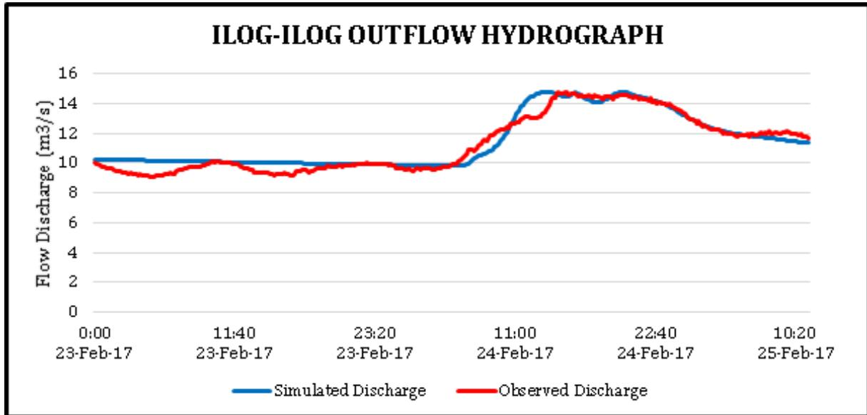
Figure 59 Outflow Hydrograph of Ilog-Ilog produced by the HEC-HMS model compared with observed outflow.
