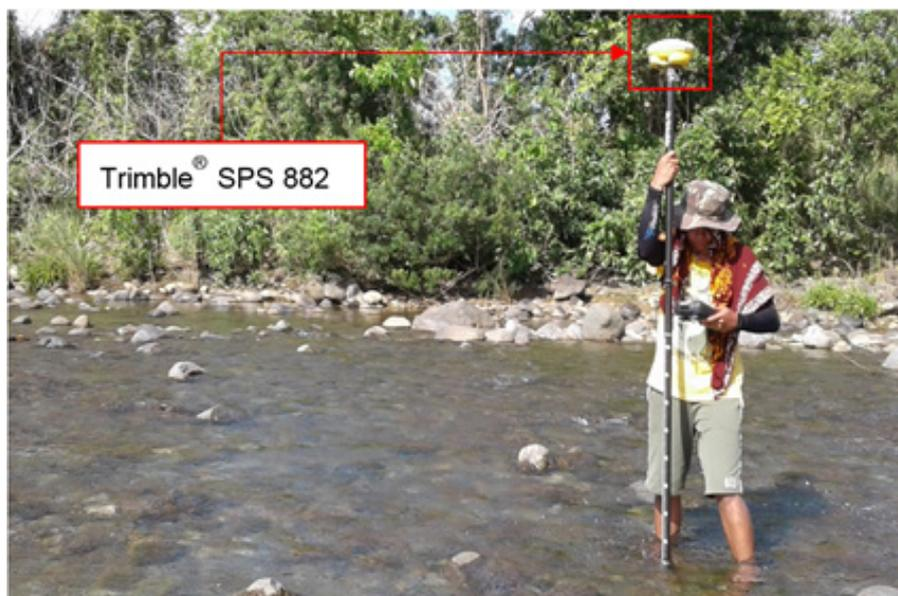
Figure 42. Gathering of bathymetric checking points along Ilog-Ilog River.
