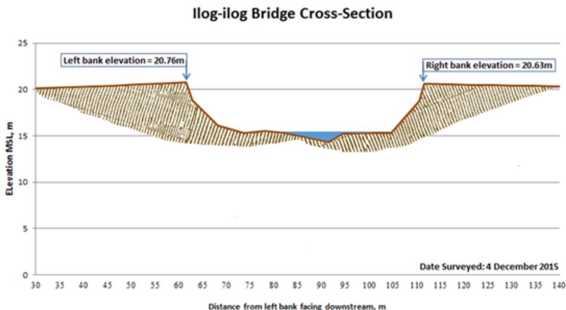
Figure 47. Cross Section Plot of Ilog-Ilog Bridge.
