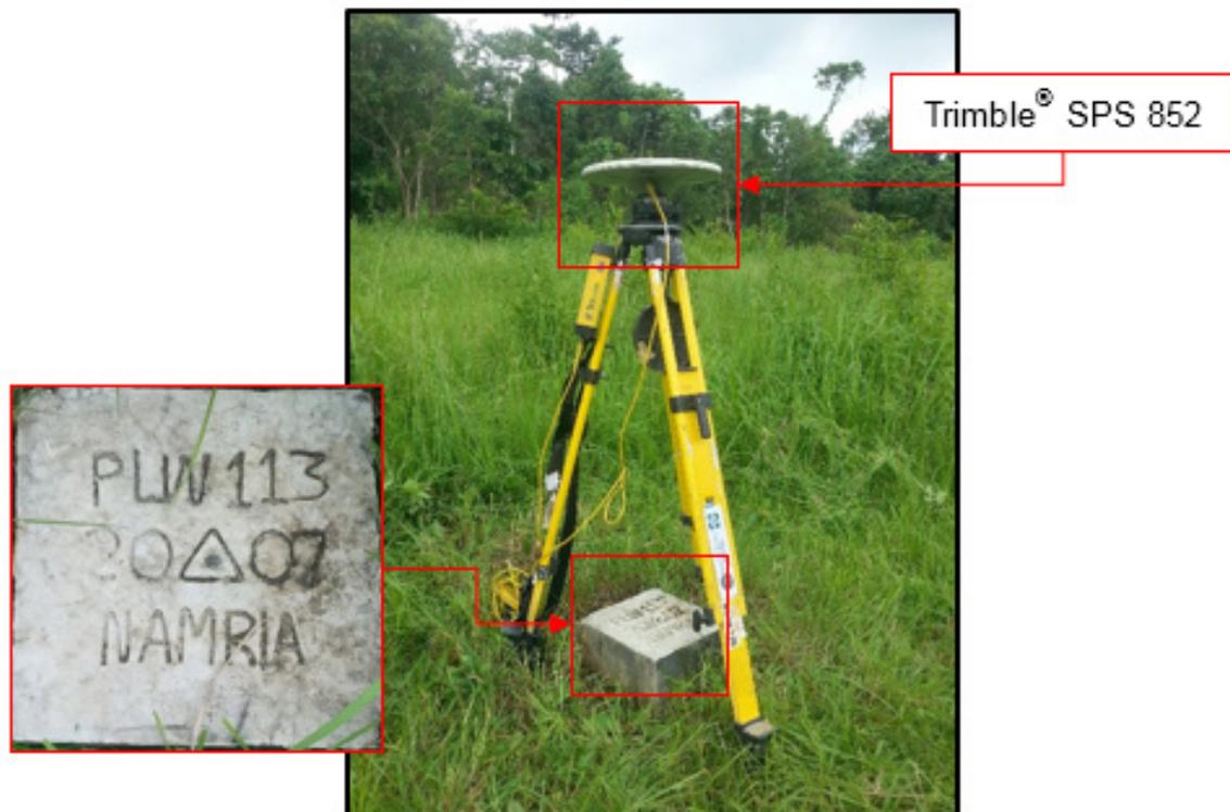
Figure 30. GNSS base set up, Trimble® SPS 852, at PLW-113, located southwest of the Aborlan Water System in Brgy. Dumagueña, Narra, Province of Palawan
