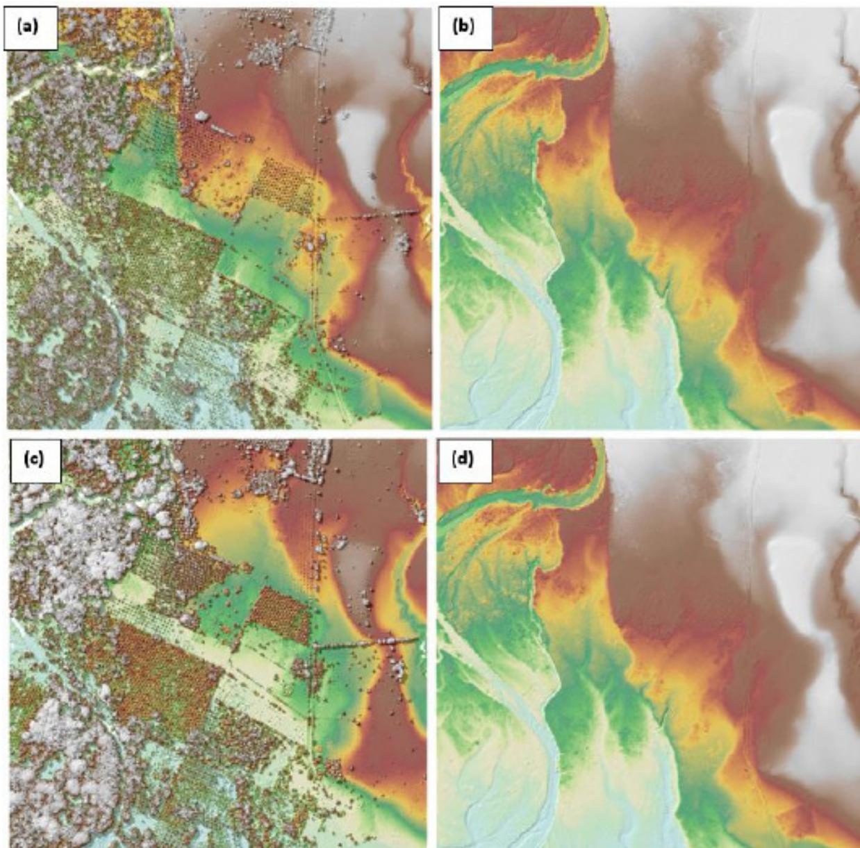
Figure 17. The production of last return DSM (a) and DTM (b), first return DSM (c) and secondary DTM (d) in some portion of Inagaun Floodplain.
