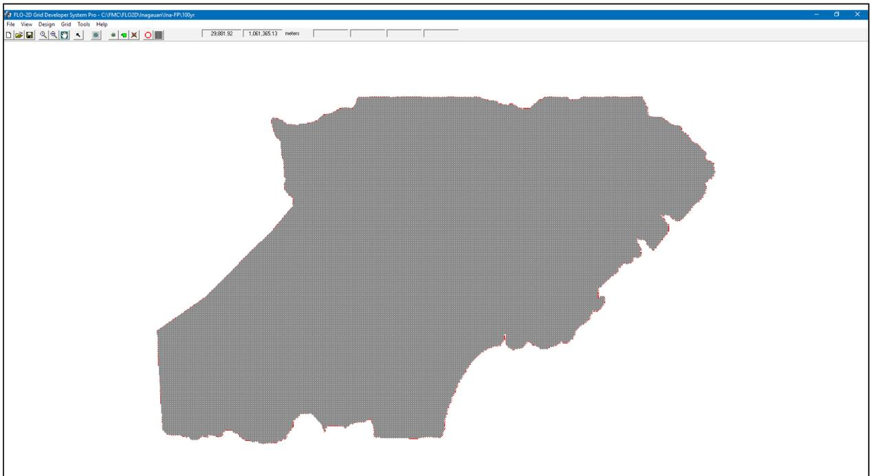
Figure 57. Screenshot of subcatchment with the computational area to be modeled in FLO-2D GDS Pro
