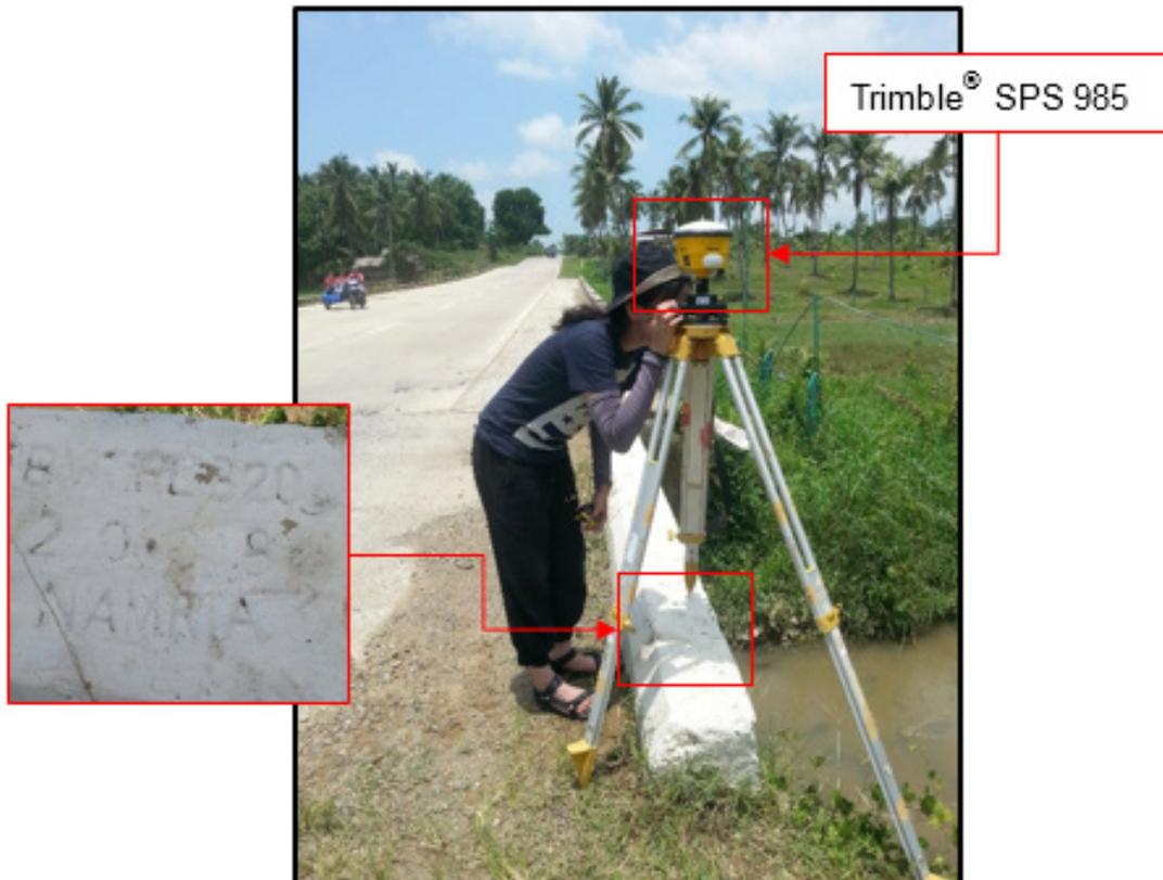
Figure 31. GNSS receiver set up, Trimble® SPS 985, at PL-320, located on top of a culvert headwall along the National Road in Brgy. Ramon Magsaysay, Aborlan, Province of Palawan
