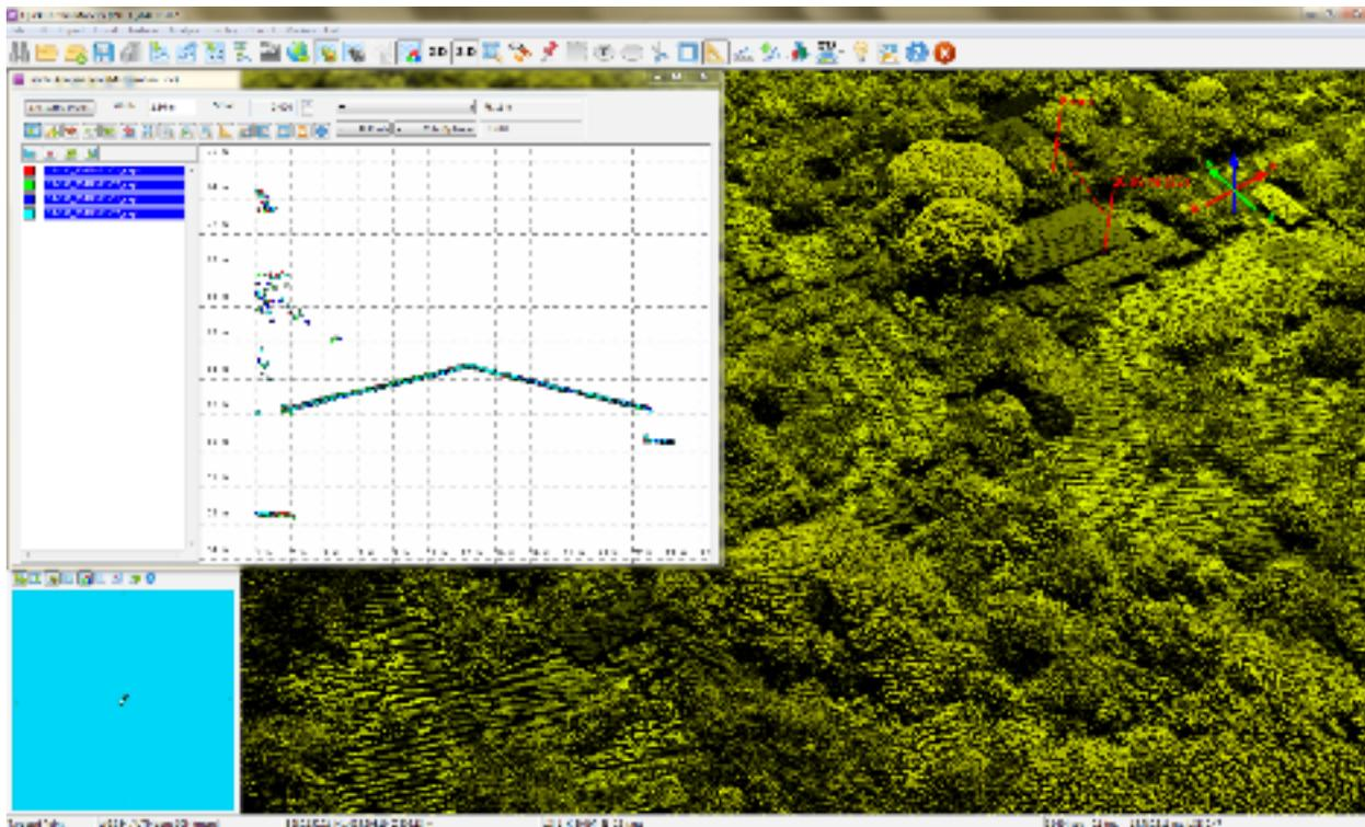
Figure 14. Quality checking for Inagauan flight 3061P using the Profile Tool of QT Modeler.
