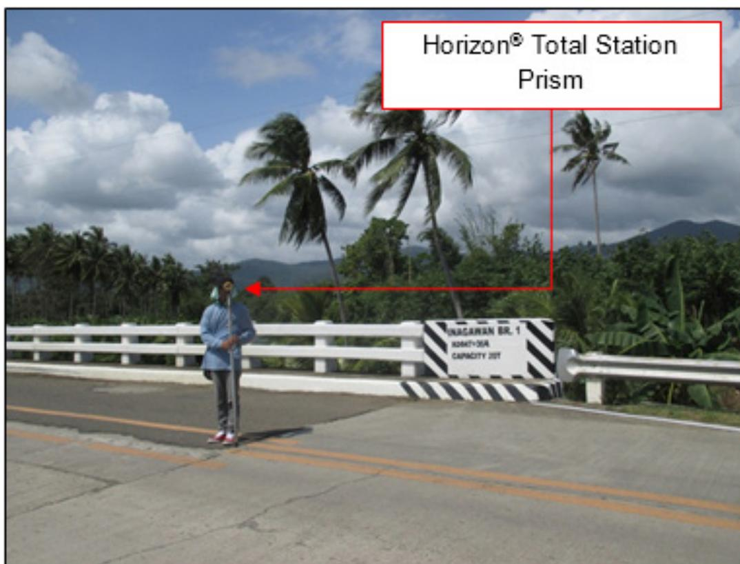
Figure 37. As-built survey of Inagauan Bridge
