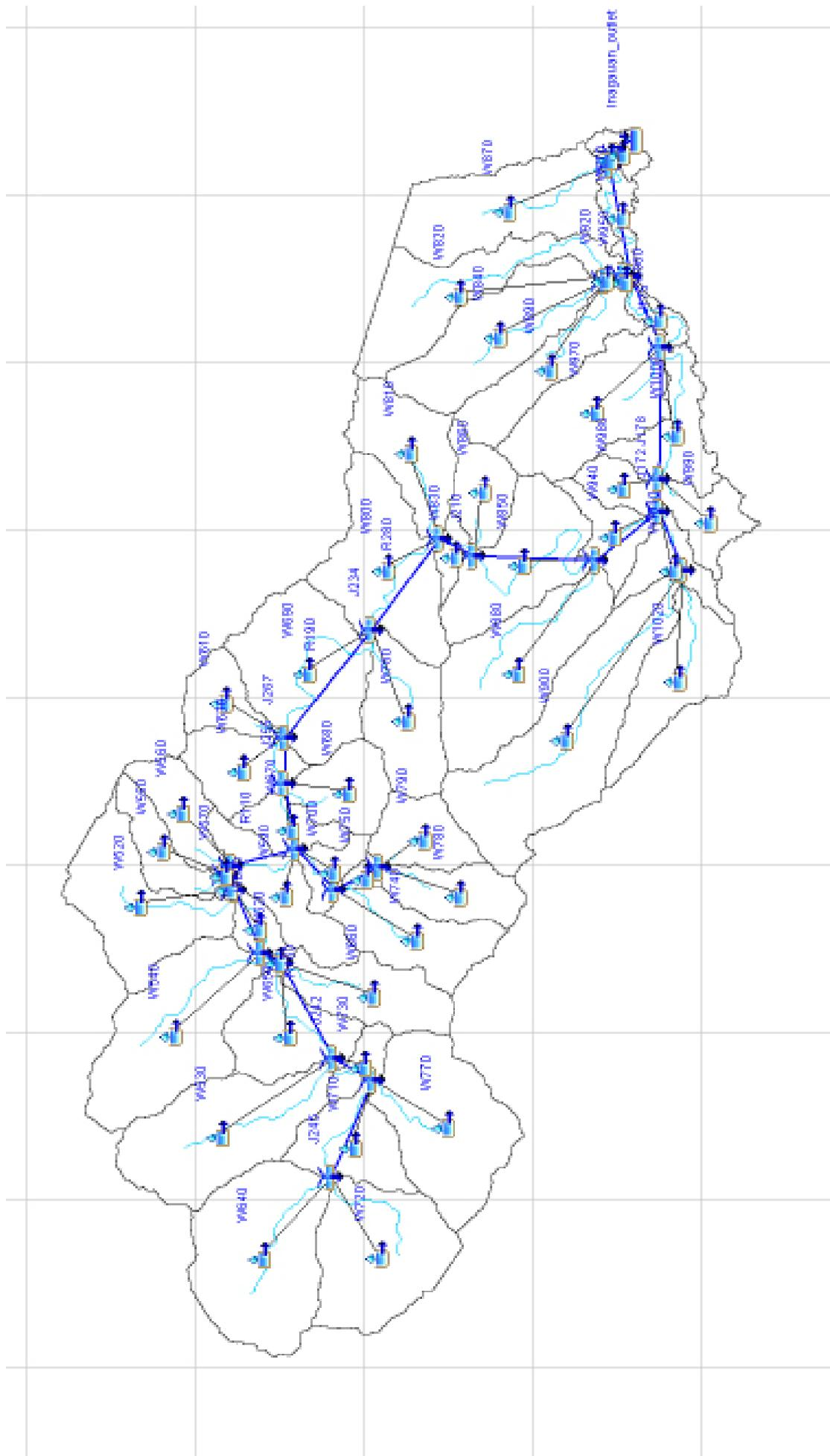
Figure 55. HEC-HMS generated Inagauan River Basin Model.
