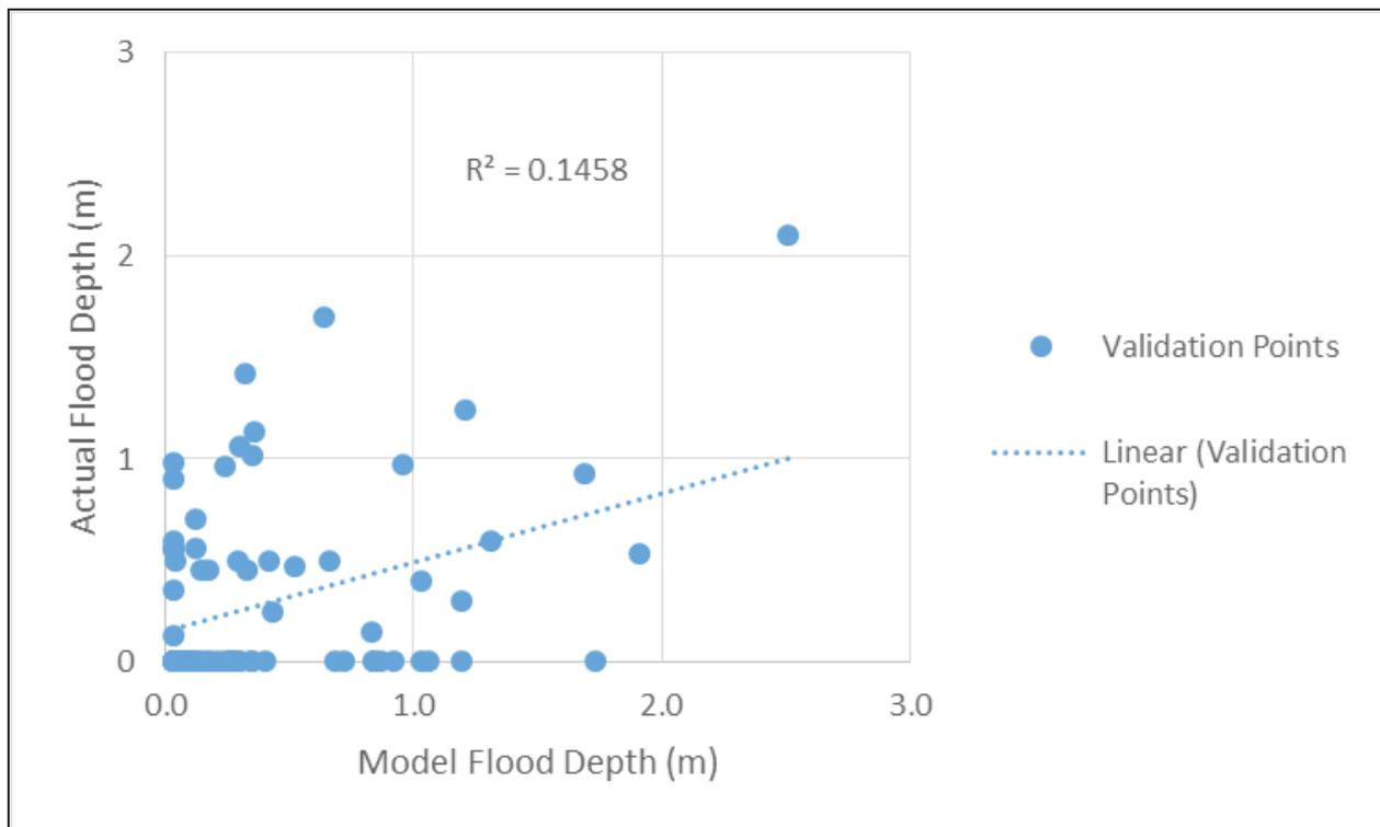
Figure 69. Flood map depth vs. actual flood depth
