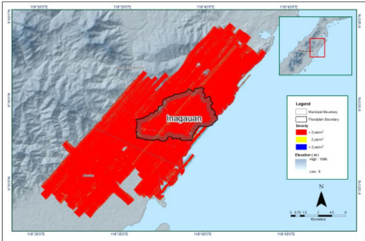
Figure 12. Pulse density map of merged LiDAR data for Inagauan Floodplain.
