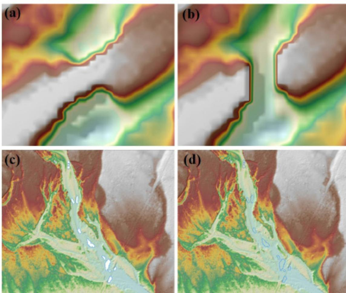
Figure 20. Figure 20. Portions in the DTM of Inagauan Floodplain – a bridge before (a) and after (b) manual data editing and a part of the river with no data before (c) and after (d) filling data gaps.
