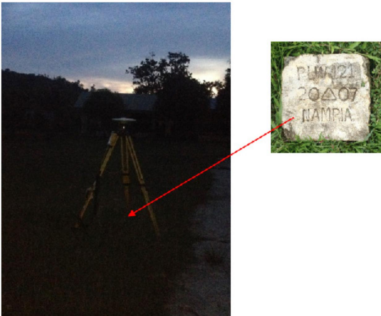
Figure 3. GPS set-up over PLW-121as recovered within the vicinity of Cabkungan Elementary School in Brgy. Campong Ulay, Rizal, Palawan (a) and NAMRIA reference point PLW-121(b) as recovered by the field team.
