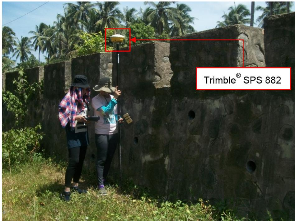
Figure 36. Gathering of random cross-section points along the approach of Iraan Bridge
