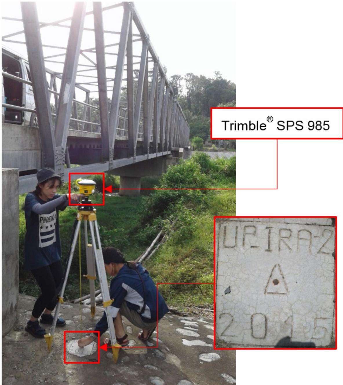
Figure 32. GNSS receiver set-up, Trimble® SPS 985, at UP IRA-2, located on the side of Iraan Bridge in Brgy. Iraan, Rizal, Province of Palawan
