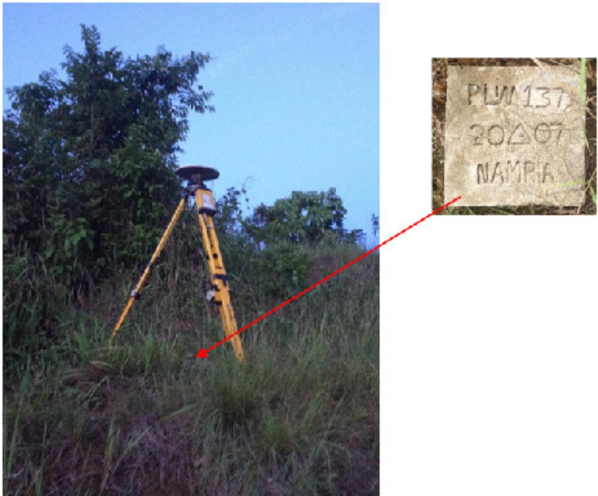
Figure 4. GPS set-up over PLW-137as recovered at the top of the ridge along national highway in Brgy. Ipilan, Quezon, Palawan (a) and NAMRIA reference point PLW-137(b) as recovered by the field team.
