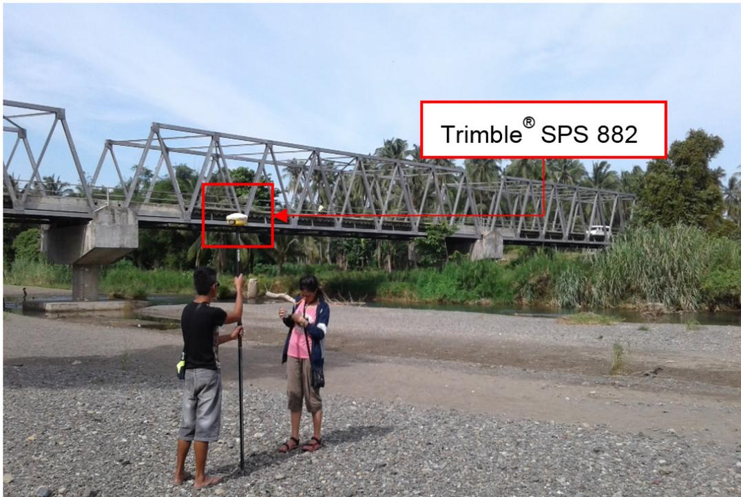
Figure 45. Gathering of bathymetric checking points along Iraan River
