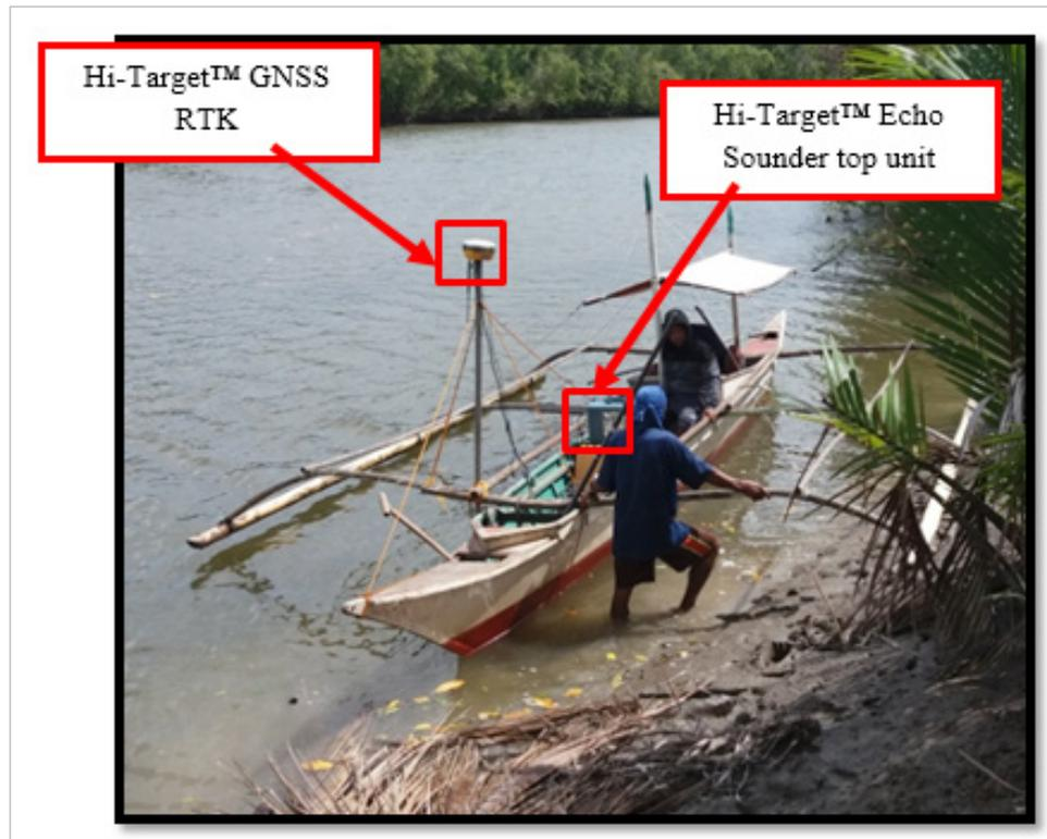
Figure 41. Bathymetric survey of ABSD at Iwahig Brookes River using Hi-Target™ Echo Sounder (upstream)
