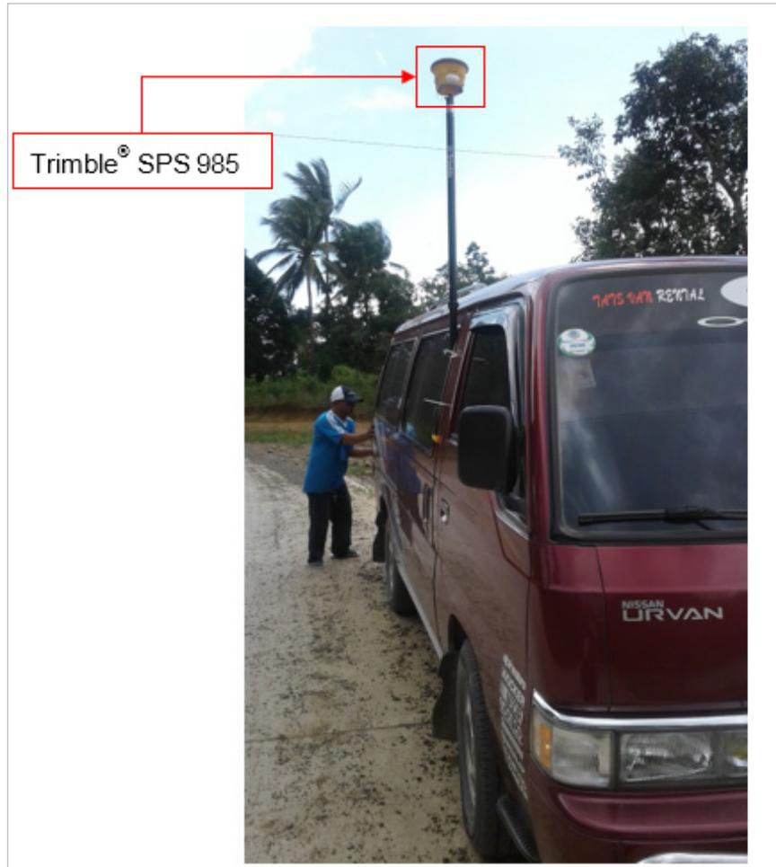
Figure 39. Validation points acquisition survey set-up for Iwahig Brookes River
