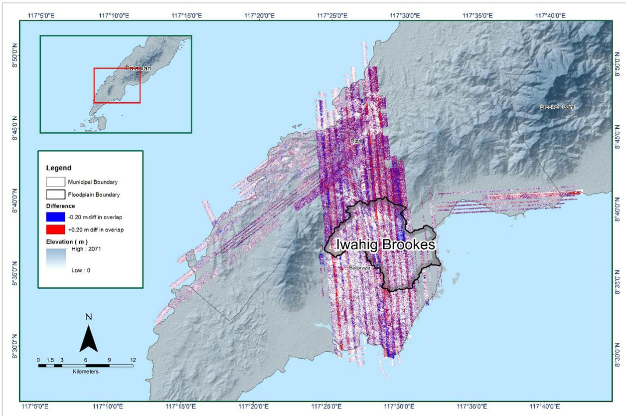
Figure 15. Elevation difference map between flight lines for Iwahig Brookes Floodplain.
