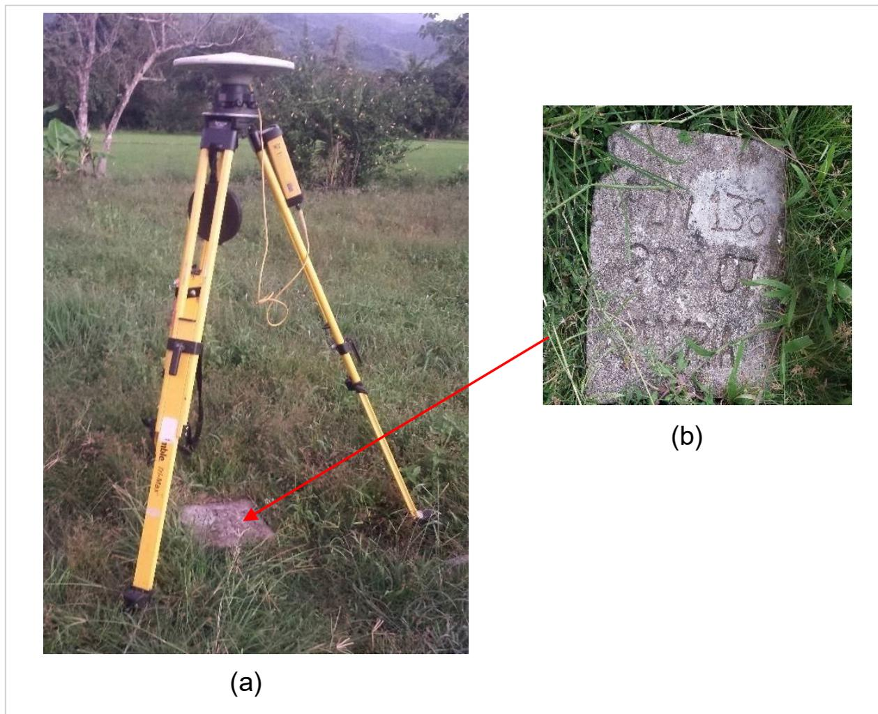
Figure 5. GPS set-up over PLW-136 as recovered in Malis Elementary School, Brooke’s Point, Palawan (a) and NAMRIA reference point PLW-136 (b) as recovered by the field team.
