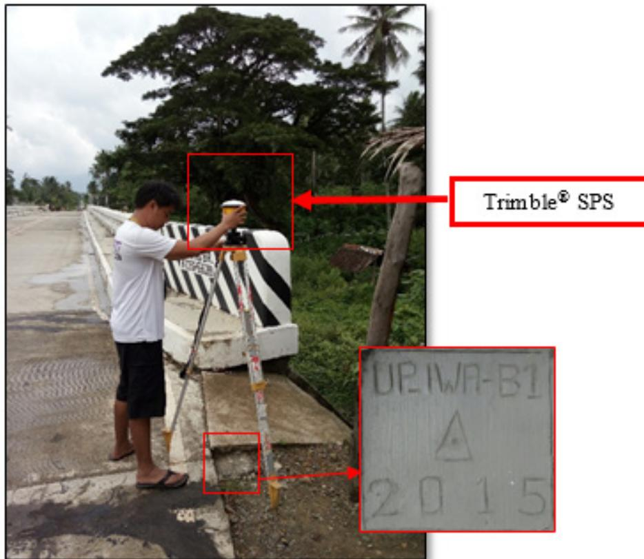
Figure 30. GNSS receiver set up, Trimble® SPS 985, at UP\_IWA-1, located at the approach of Iwahig Bridge in Brgy. Iwahig, Bataraza, Province of Palawan
