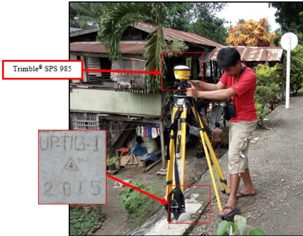
Figure 32. GNSS receiver set up, Trimble® SPS 985, at UP\_PAN-1, located on the approach of Tigaplan Bridge in Brgy. Barong-Barong, Brooke's Point, Province of Palawan
