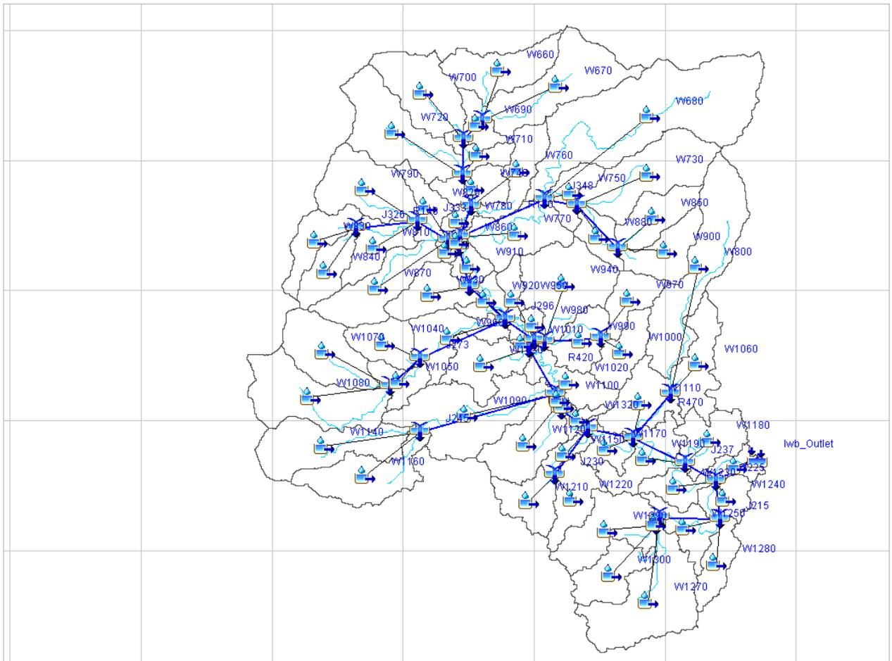
Figure 50. HEC-HMS generated Iwahig Brookes River Basin Model.
