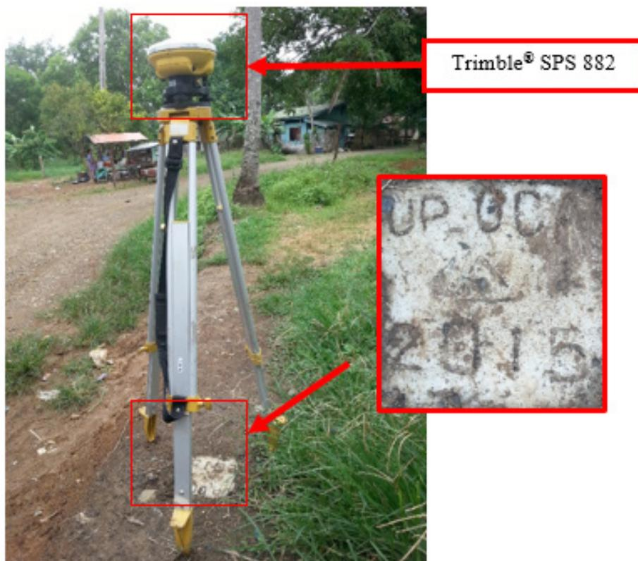
Figure 31. GNSS base set up, Trimble® SPS 882, at UP\_OCA-0, located about 23 m from Elementary School near Ocayan River in Brgy. Rio Tuba, Bataraza, Province of Palawan
