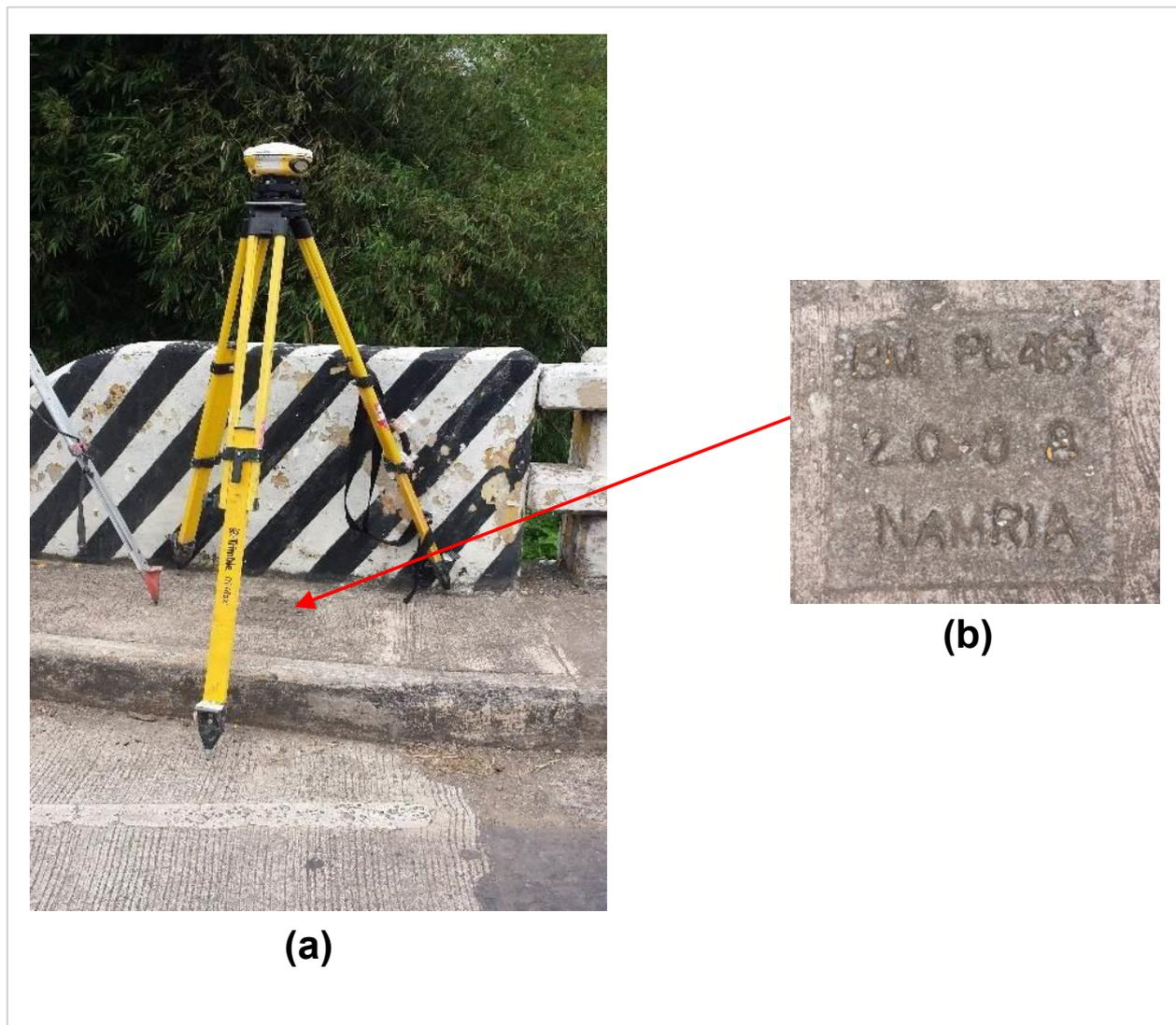
Figure 3. GPS set-up over PL-467 recovered on Inogbong Bridge, Bataraza Palawan (a) and NAMRIA reference point PL-467 (b) as recovered by the field team.
