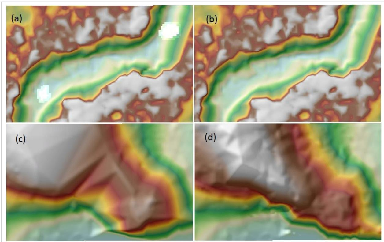
Figure 22. Portions in the DTM of Iwahig Brookes Floodplain – a data gap (a) and after (b) manual editing; and a deformed feature before (c) and after (d) object retrieval.
