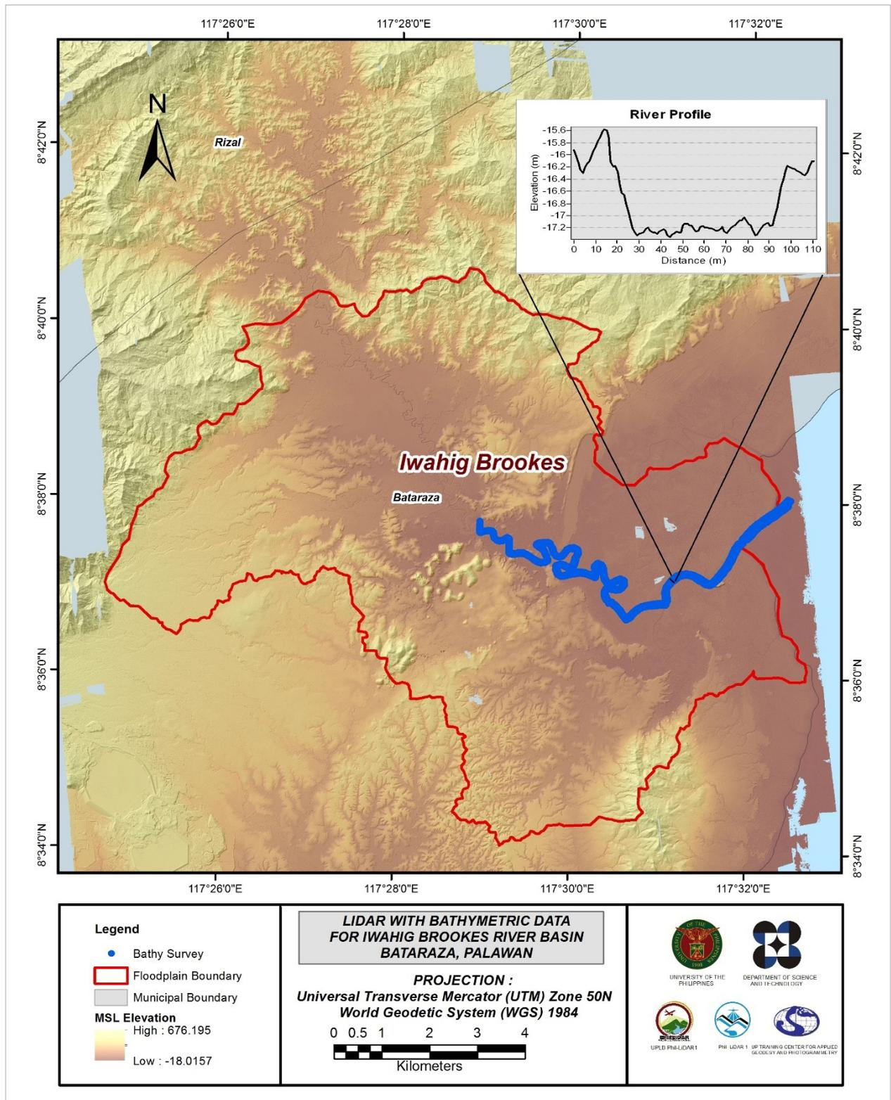
Figure 27. Map of Iwahig Brookes Floodplain with bathymetric survey points shown in blue.
