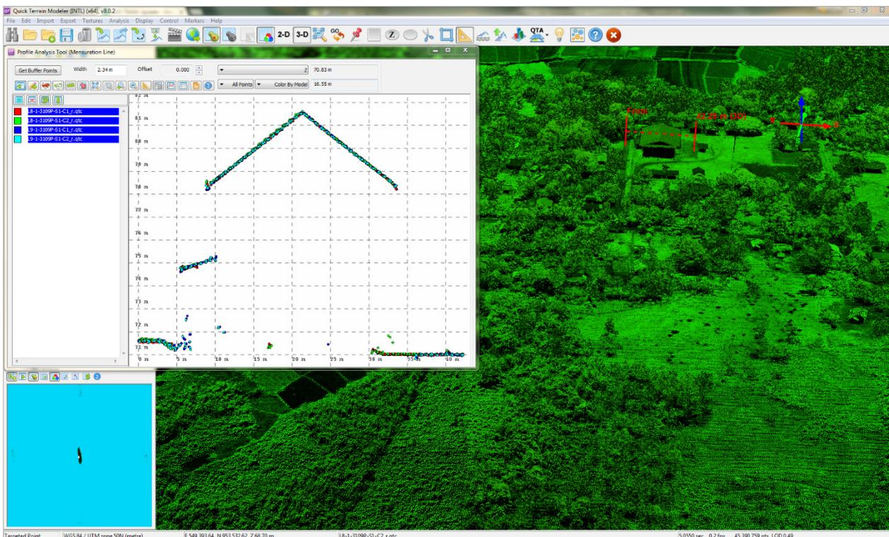
Figure 16. Quality checking for Iwahig Brookes flight 3109P using the Profile Tool of QT Modeler.
