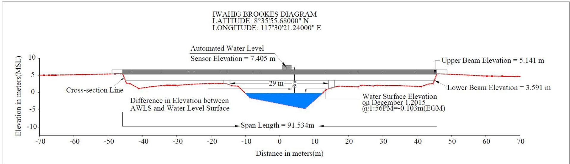
Figure 36. Iwahig Brookes Bridge cross-section diagram
