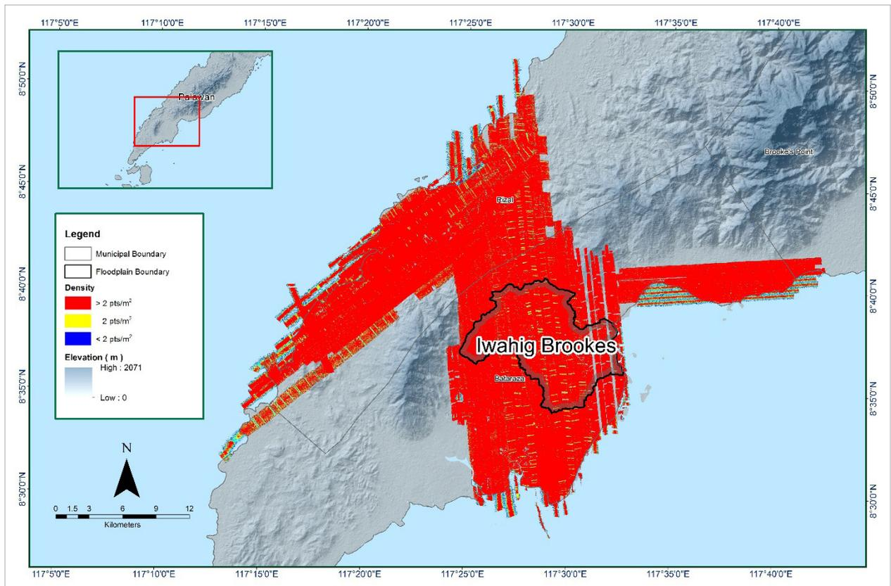
Figure 14. Pulse density map of merged LiDAR data for Iwahig Brookes Floodplain.
