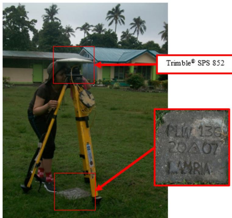
Figure 29. GNSS receiver set up, Trimble® SPS 882, at PLW-136, located at the Malis Elementary School compound, Brgy. Malis, Brooke's Point, Province of Palawan
