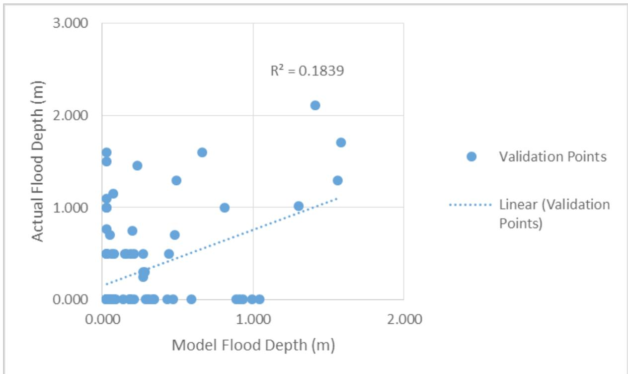
Figure 67. Flood map depth vs. actual flood depth
