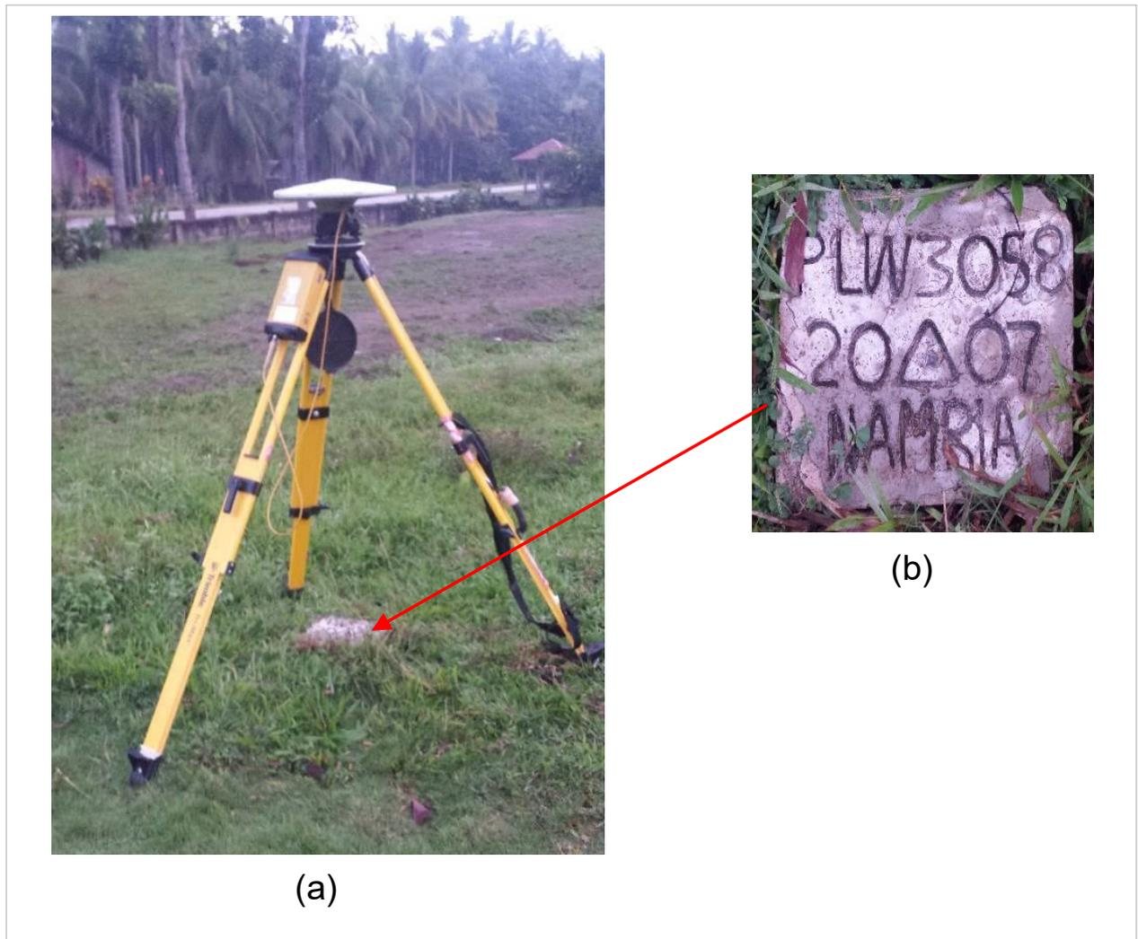
Figure 6. GPS set-up over PLW-3058 as recovered on the ground inside Caranasan Elementary School, Espanola, Palawan (a) and NAMRIA reference point PLW-3058 (b) as recovered by the field team.
