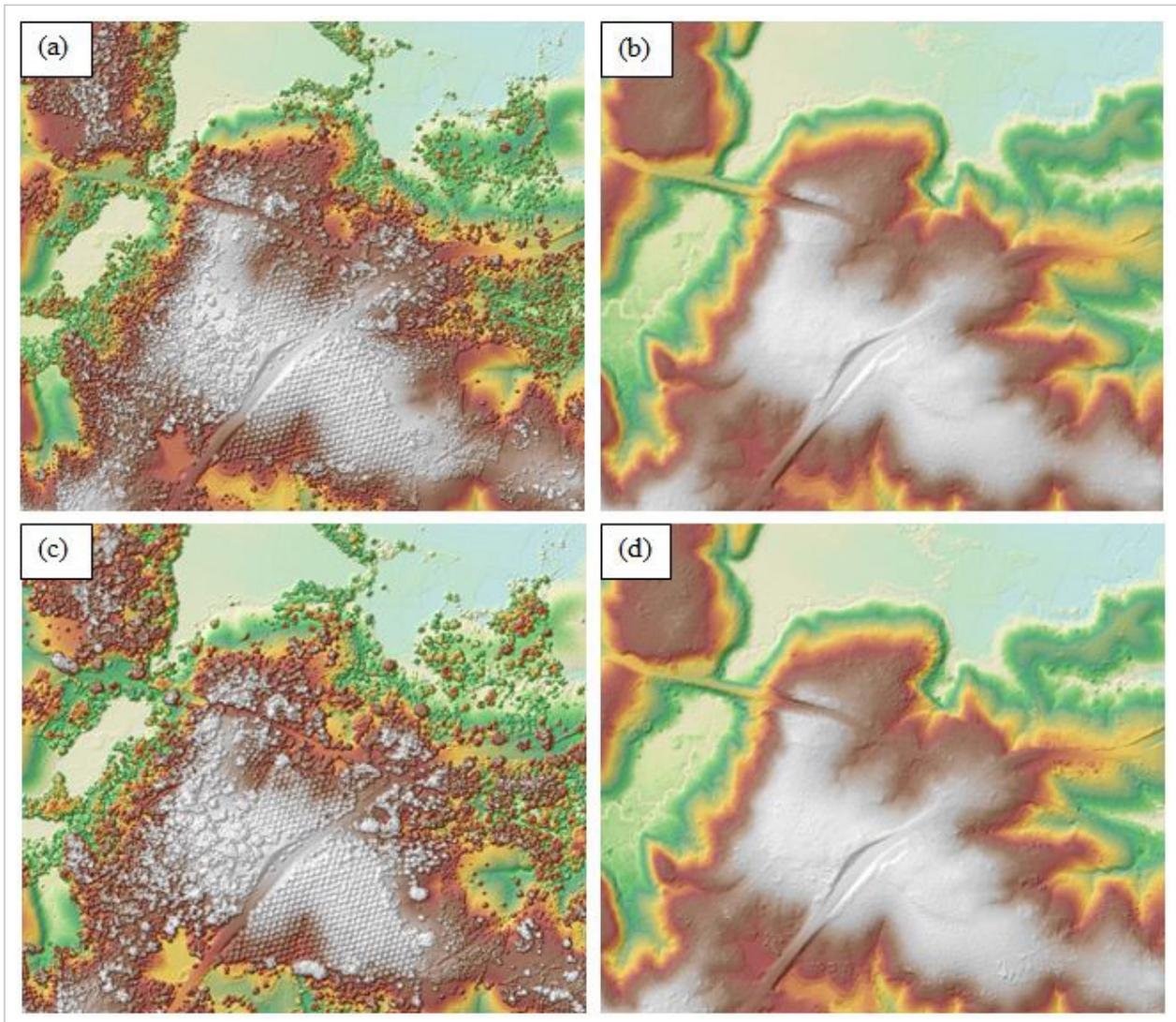
Figure 19. The production of last return DSM (a) and DTM (b), first return DSM (c) and secondary DTM (d) in some portion of Iwahig Brookes Floodplain.
