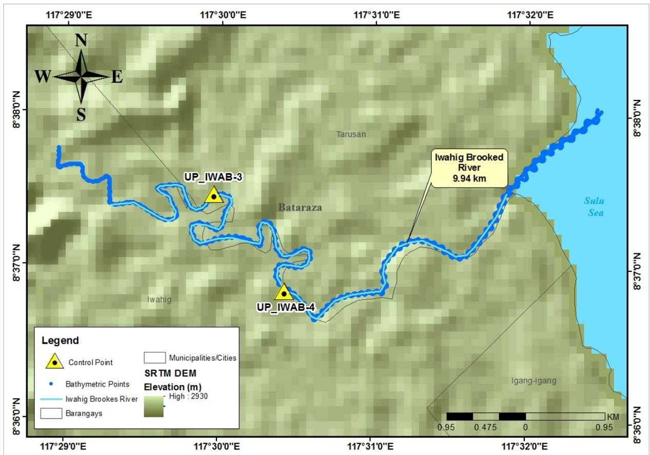
Figure 42. Bathymetric survey of Iwahig Brookes River
