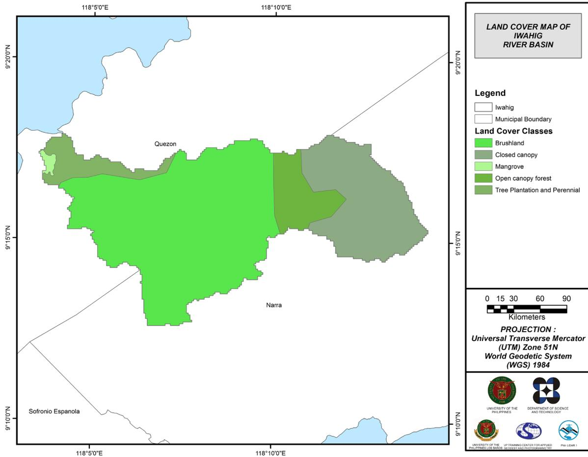
Figure 53. Land cover map of Iwahig River Basin used for the estimation of the CN and watershed lag parameters of the rainfall-runoff model. (Source: NAMRIA)
