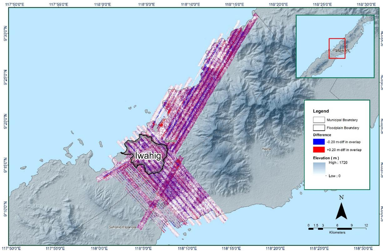
Figure 17. Elevation difference map between flight lines for Iwahig Floodplain.
