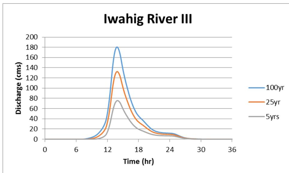
Figure 61. Iwahig river (3) generated discharge using interpolated 5-, 25-, and 100-year rainfall intensity-duration-frequency (RIDF) in HEC-HMS
