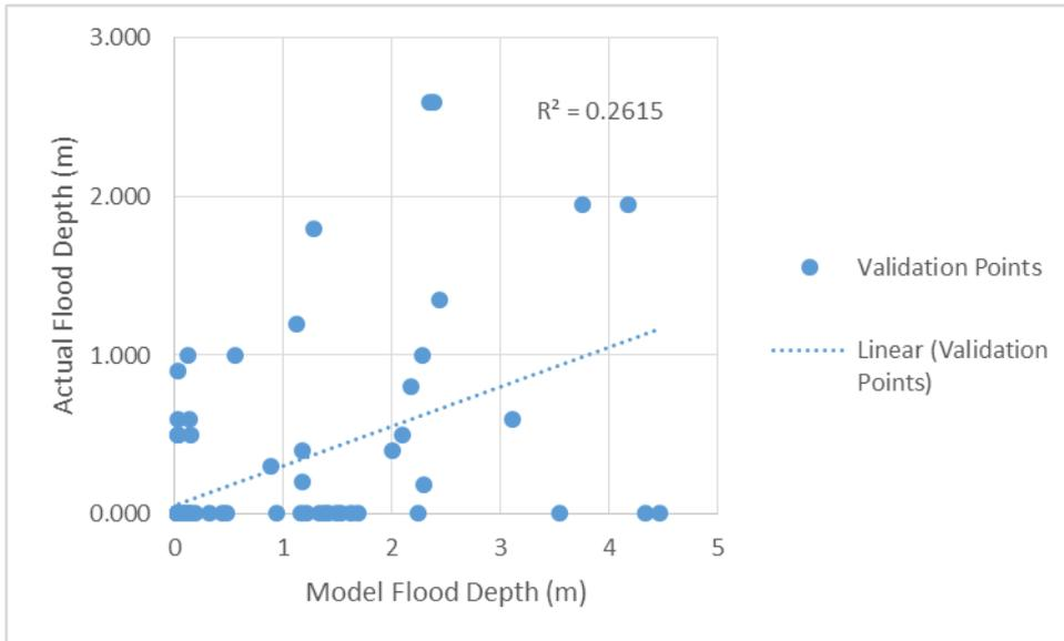
Figure 77. Flood map depth vs. actual flood depth
