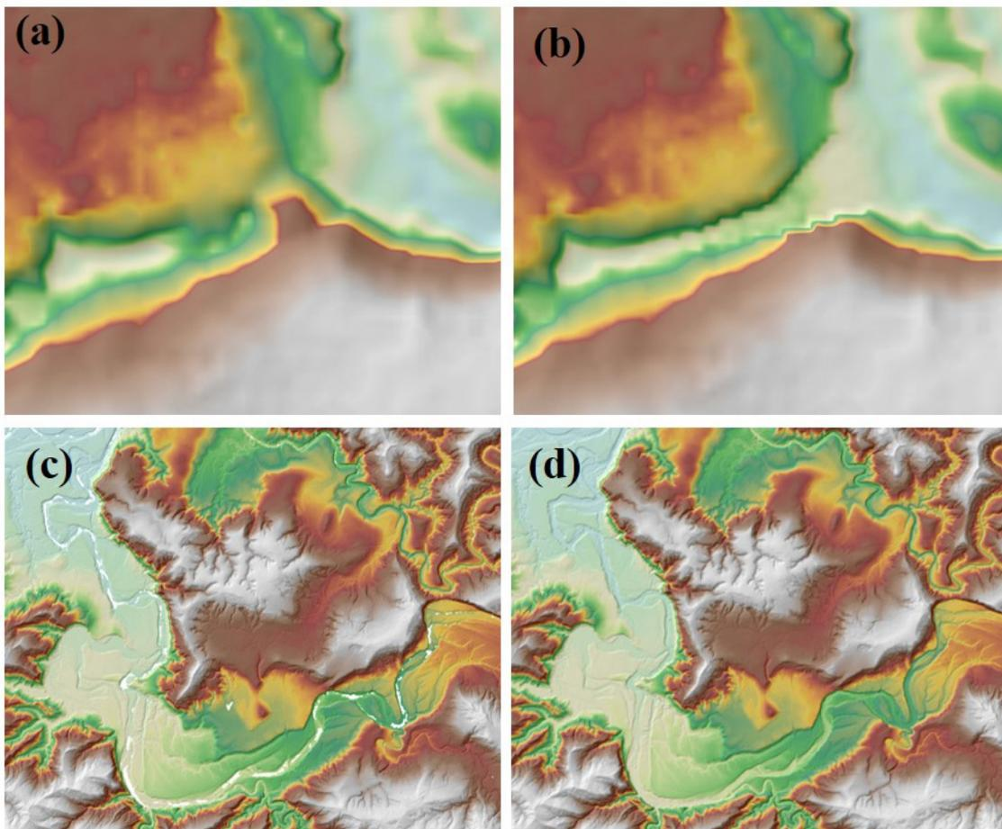
Figure 24. Portions in the DTM of Iwahig Floodplain – a land bridge before (a) and after (b) interpolation process and part of the river with data gap before (c) and after (d) filling data gap
