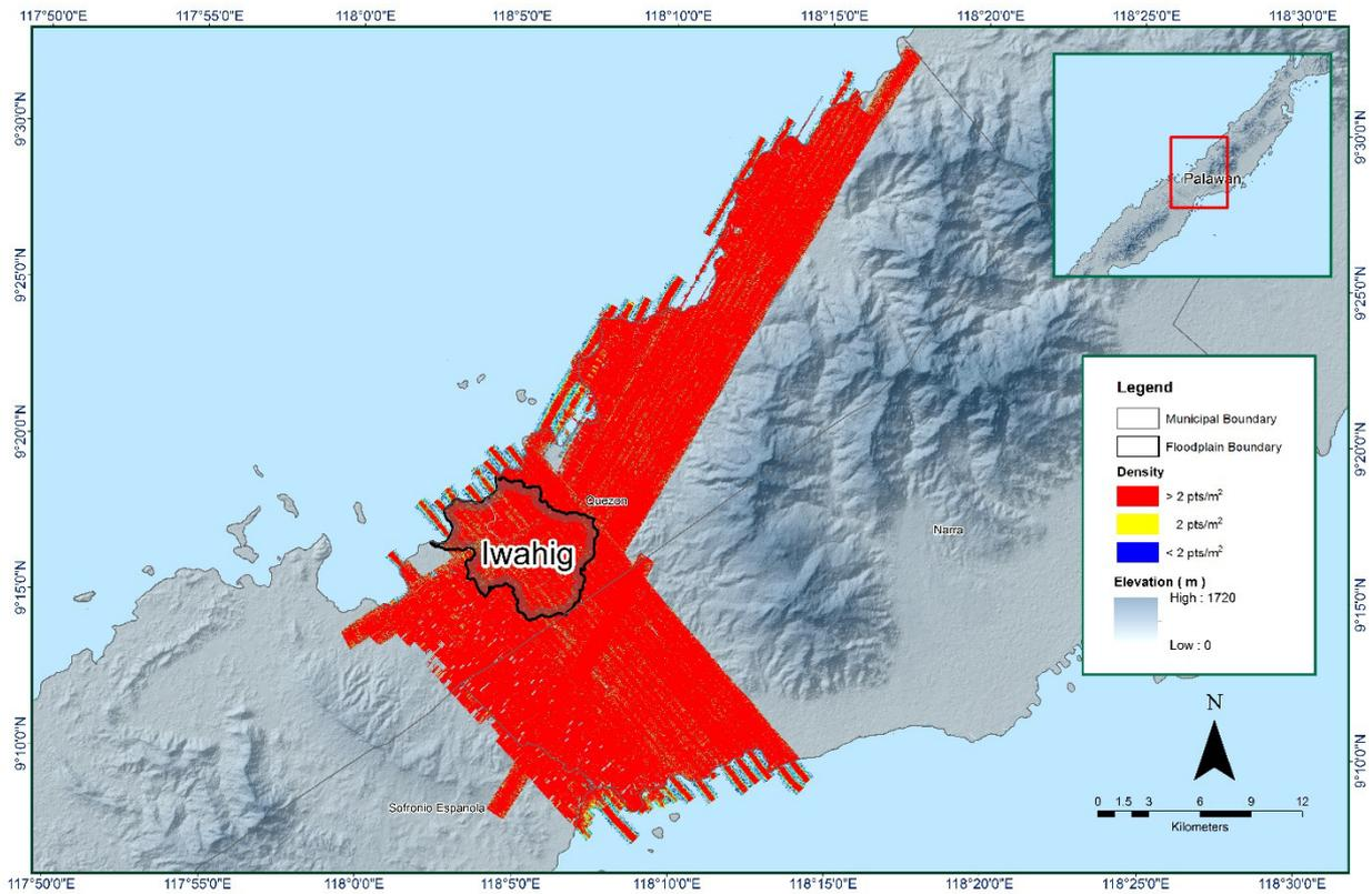
Figure 16. Pulse density map of merged LiDAR data for Iwahig Floodplain.
