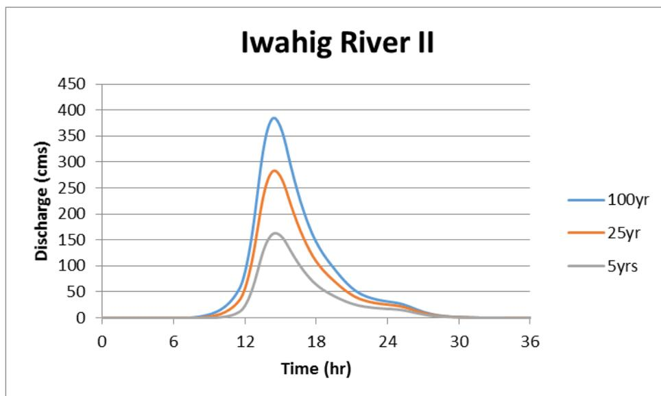
Figure 60. Iwahig river (2) generated discharge using interpolated 5-, 25-, and 100-year rainfall intensity-duration-frequency (RIDF) in HEC-HMS
