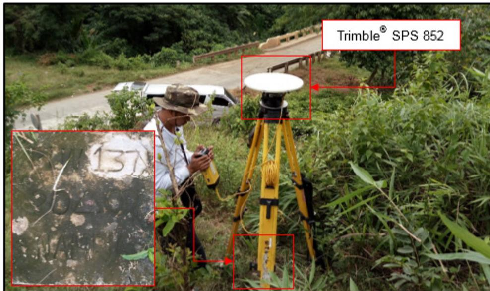
Figure 33. GNSS base set up, Trimble® SPS 852, at PLW-137, located at the top of a ridge along the National Highway in Brgy. Ipilan, Narra, Province of Palawan
