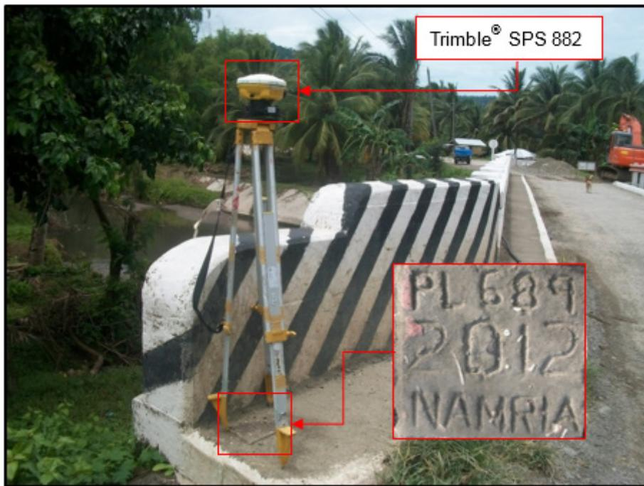
Figure 32. GNSS receiver set up, Trimble® SPS 882, at PL-689, located at the approach of Malatgao Bridge in Brgy. Sowangan, Quezon, Province of Palawan
