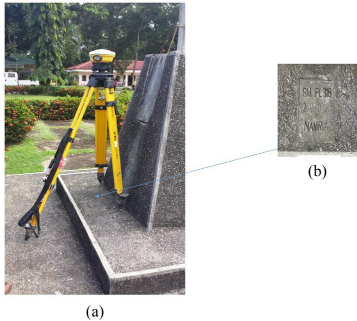
Figure 6. GPS set-up over PL-318 on the flagpole in front of Aborlan Municipal Hall, Palawan (a) and NAMRIA reference point PL-318 (b) as recovered by the field team.
