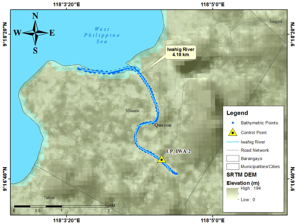
Figure 47. Bathymetric survey of Iwahig River
