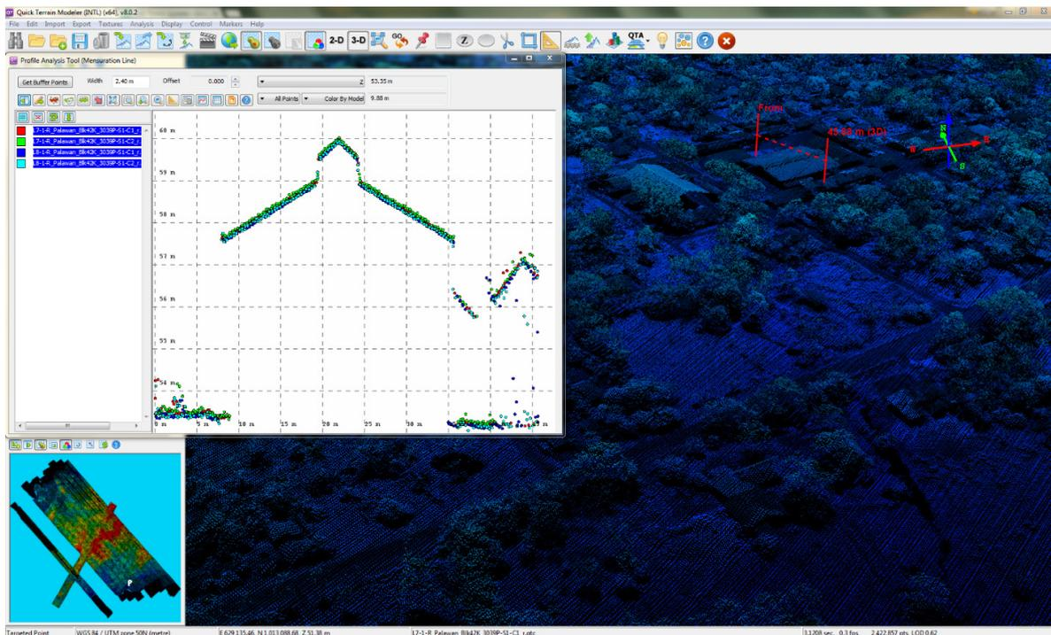
Figure 18. Quality checking for Iwahig flight 3039P using the Profile Tool of QT Modeler.
