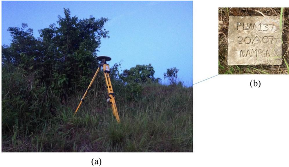
Figure 4. GPS set-up over PLW-137 at the ridge near kilometer post 133 at Brgy. Ipilan, Municipality of Narra along Narra-Aboabo (Sofronio Espanola) – Quezon highway (a) and NAMRIA reference point PLW-137 (b) as recovered by the field team.
