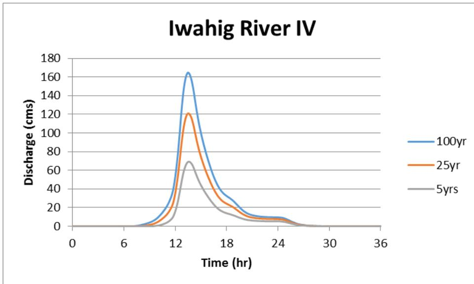
Figure 62. Iwahig river (4) generated discharge using interpolated 5-, 25-, and 100-year rainfall intensity-duration-frequency (RIDF) in HEC-HMS
