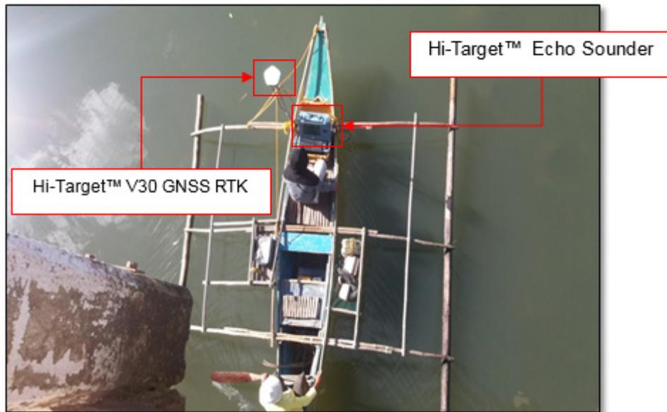
Figure 45. Bathymetric survey of ABSD at Iwahig River using Hi-Target™ Echo Sounder (upstream)
