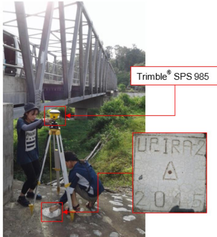
Figure 36. GNSS receiver set up, Trimble® SPS 985, at UP\_IRA-2, located on the side of Iraan Bridge in Brgy. Iraan, Rizal, Province of Palawan
