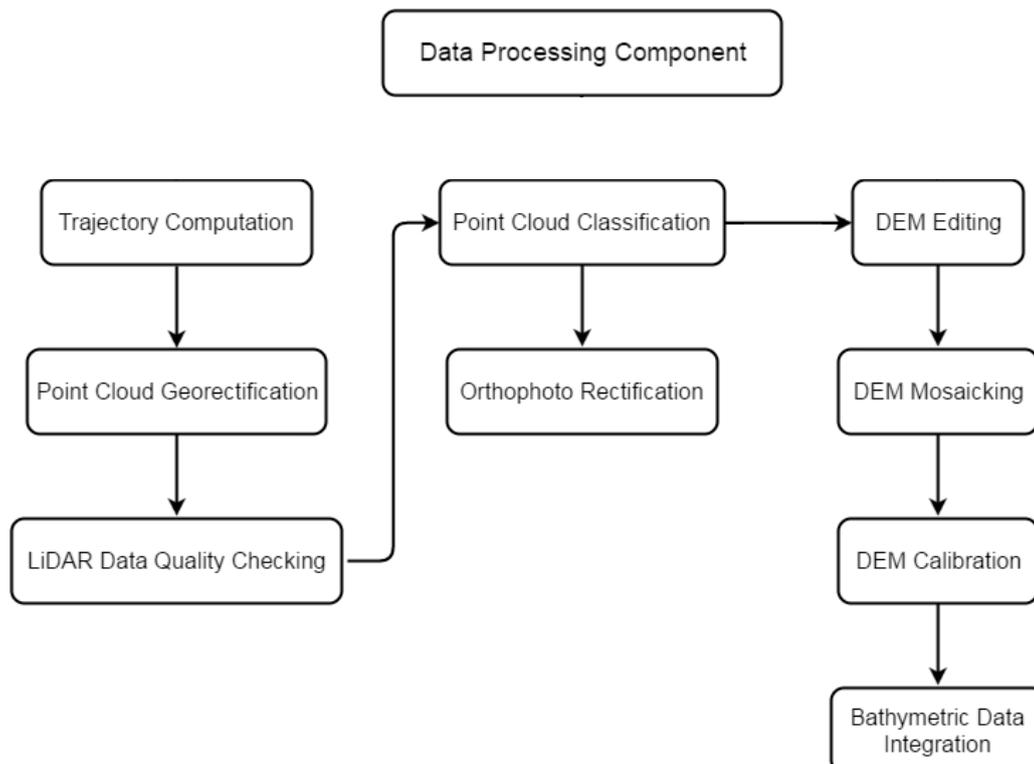
Figure 10. Schematic Diagram for Data Pre-Processing Component
