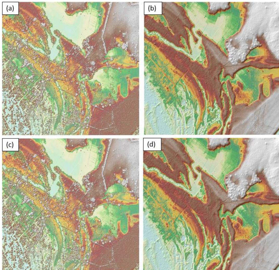
Figure 21. The production of last return DSM (a) and DTM (b), first return DSM (c) and secondary DTM (d) in some portion of Iwahig Floodplain.
