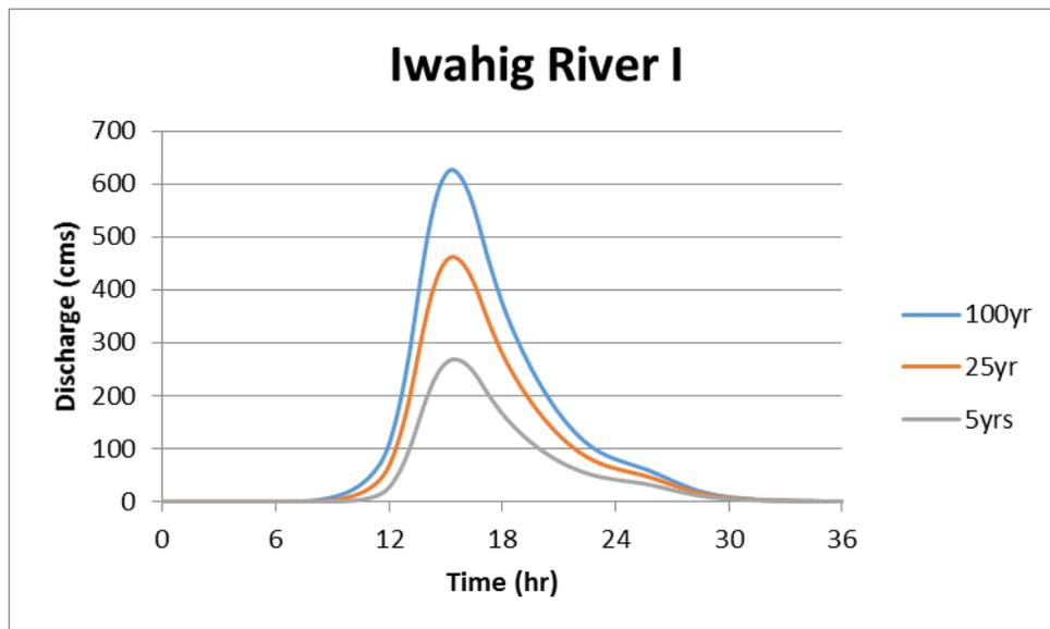
Figure 59. Iwahig river (1) generated discharge using interpolated 5-, 25-, and 100-year rainfall intensity-duration-frequency (RIDF) in HEC-HMS
