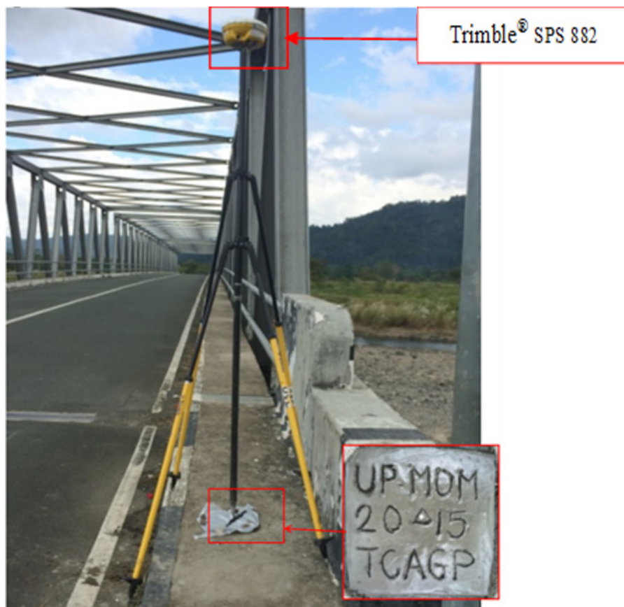
Figure 39. GNSS receiver set-up, Trimble® SPS 882, at UP-MOM, Mompong Bridge approached in Brgy. Lumang Bato, Municipality of Sablayan, Occidental Mindoro
