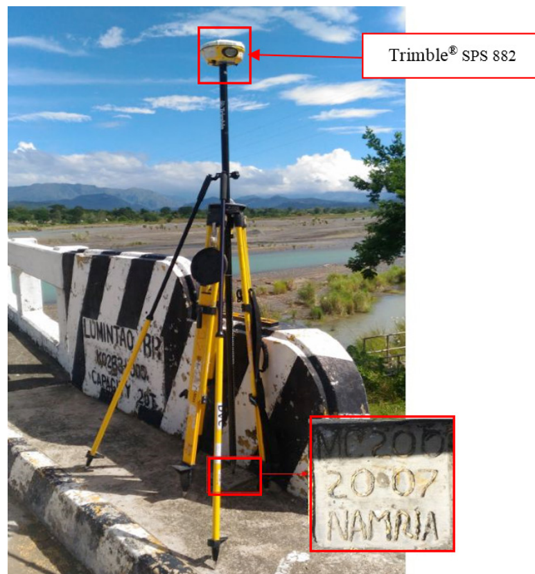
Figure 34. GNSS receiver set-up, Trimble® SPS 882, at MC-200, Lumintao Bridge approach in Brgy. Magsikap, Municipality of Rizal, Occidental Mindoro
