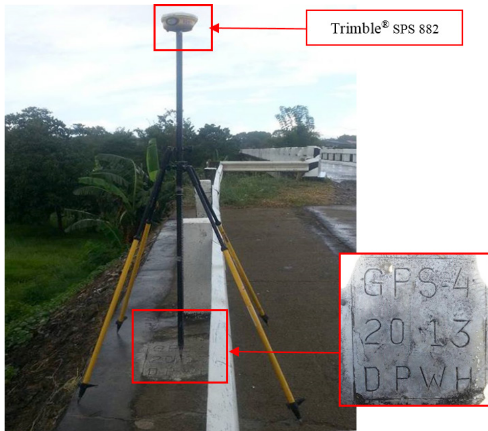
Figure 37. GNSS receiver, Trimble® SPS 882, at GPS-4 on right side of the road abutment after Caguray Bridge going to Bulalacao in Brgy. Poblacion, Municipality of Magsaysay, Occidental Mindoro
