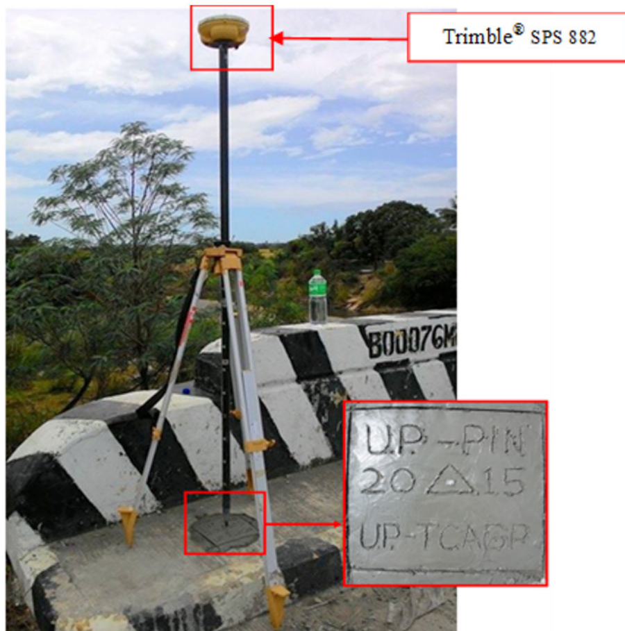
Figure 38. GNSS base receiver set-up, Trimble® SPS 882, at UP-PIN Pinamanaan Bridge approach in Brgy. Mapaya, Municipality of San Jose, Occidental Mindoro
