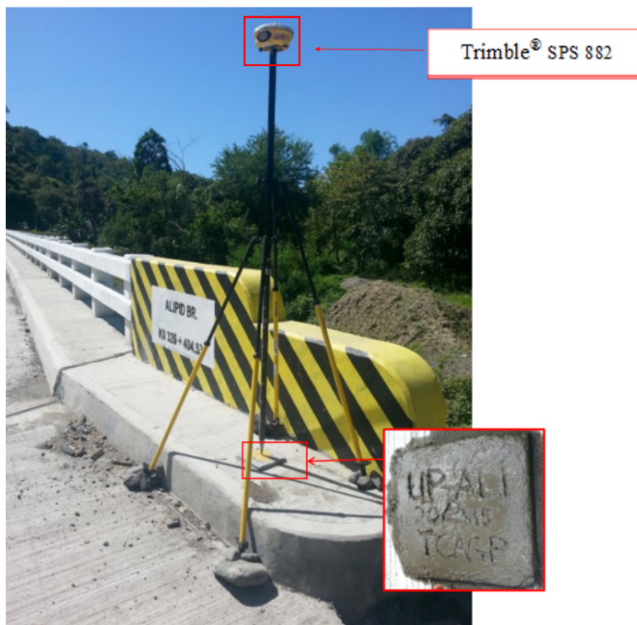
Figure 40. GNSS receiver set up, Trimble® SPS 882, at UP-ALI, Alipid Bridge approach in Brgy. Sto. Niño, Municipality of Sablayan, Occidental Mindoro
