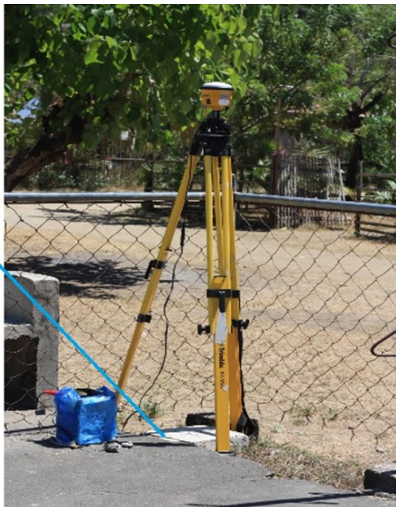
Figure 4. GPS set-up over MRW-24 in the basketball court in Brgy. Iriron, municipality of Calintaan, Occidental Mindoro (a) and NAMRIA reference point MRW-24 (b) as recovered by the field team.
