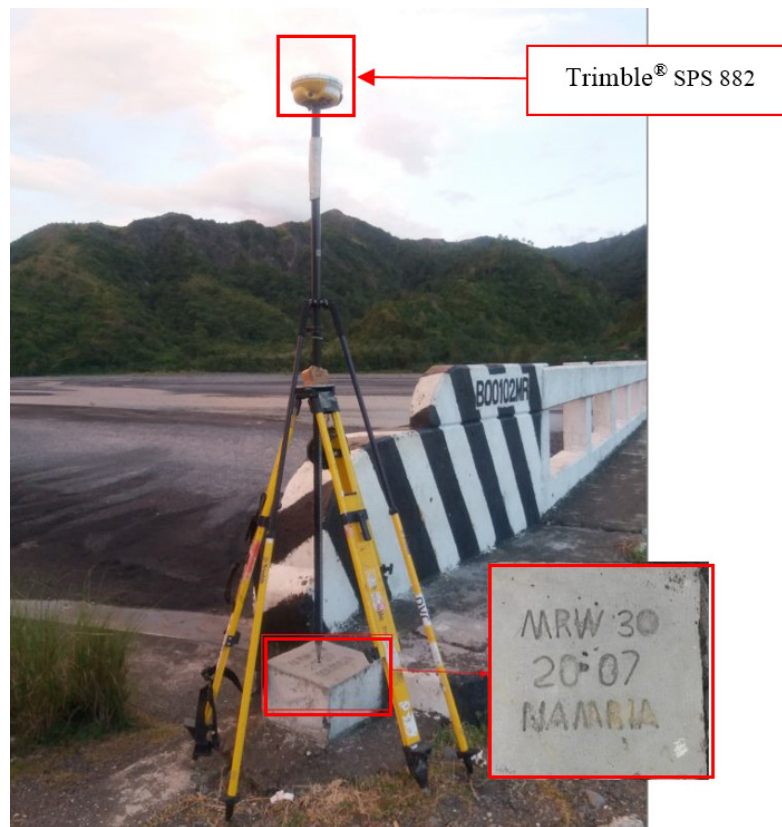
Figure 33. GNSS receiver setup, Trimble® SPS 882, at MRW-30 Amnay Bridge approach in Sitio Kabangkalan, Brgy. Pinagturilan, Municipality of Santa Cruz, Occidental Mindoro
