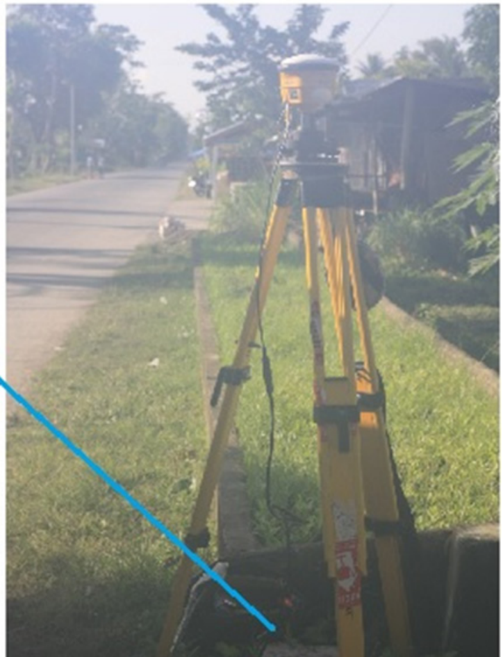
Figure 5. GPS set-up over MRW-4203 in front of the barangay hall of Brgy. Mapaya, municipality of San Jose, Occidental Mindoro (a) and NAMRIA reference point MRW-4203 (b) as recovered by the field team.
