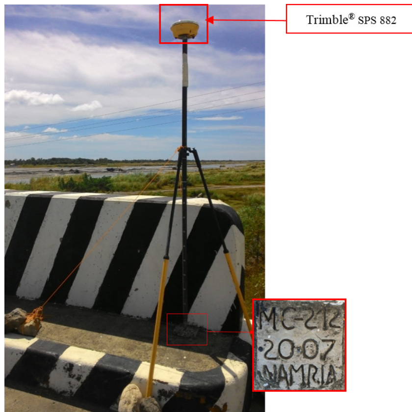
Figure 35. GNSS receiver set-up, Trimble® SPS 882, at MC-212, Busuanga Bridge approach in Bgry. Sto Niño, Municipality of Rizal, Occidental Mindoro
