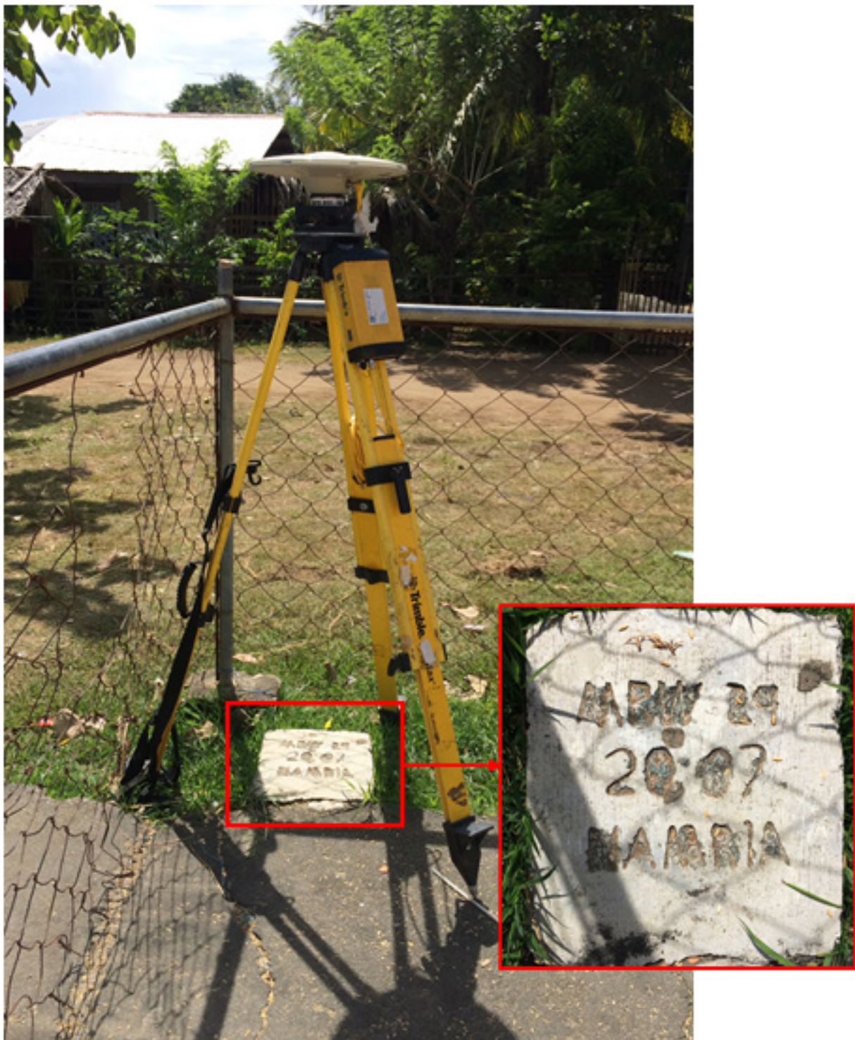
Figure 32. GNSS receiver set-up, Trimble® SPS 852, at MRW-24 in front of Iriron Elementary School in Brgy. Iriron, Municipality of Calintaan, Occidental Mindoro
