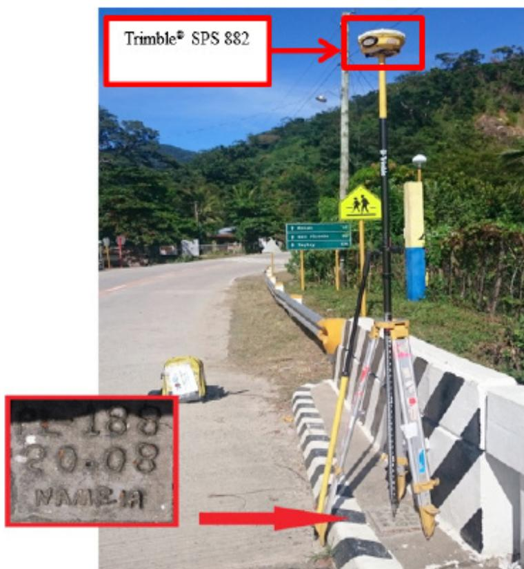
Figure 30. GNSS receiver set up, Trimble® SPS SPS 882, at PL-188 located in Langogan Bridge, Brgy. Langogan, Puerto Prinsesa, Palawan.
