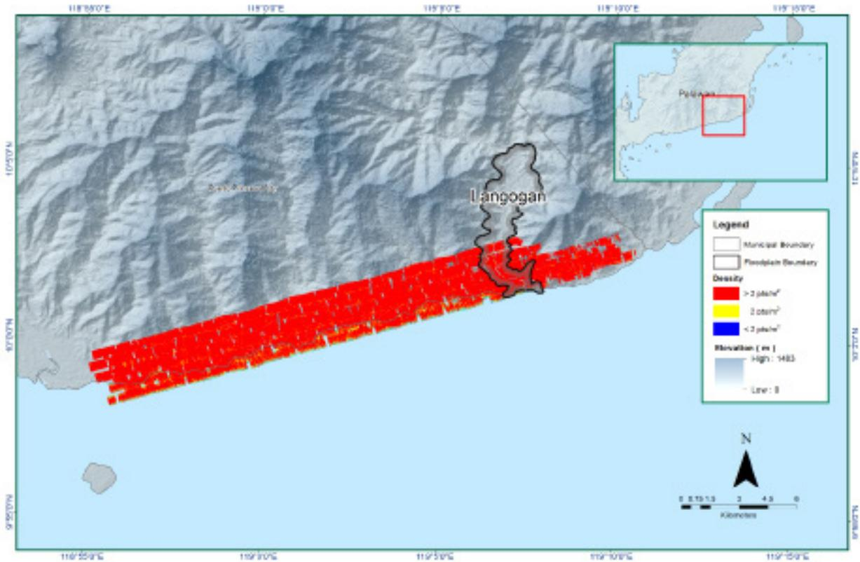
Figure 13. Pulse density map of the merged LiDAR data for Langogan floodplain.
