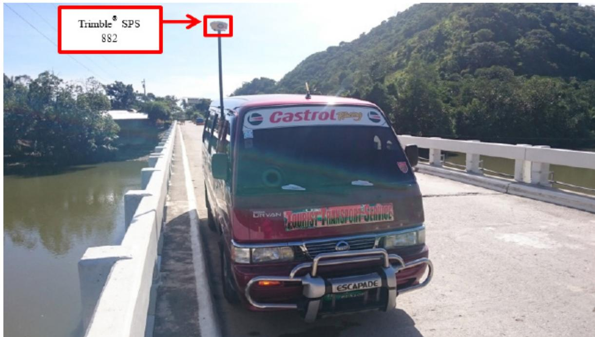
Figure 37. GNSS Receiver Trimble® SPS 882 installed on a vehicle for Ground Validation Survey.
