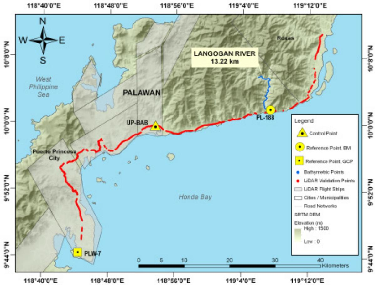
Figure 38. The extent of the LiDAR ground validation survey (in red) for Langogan River Basin
