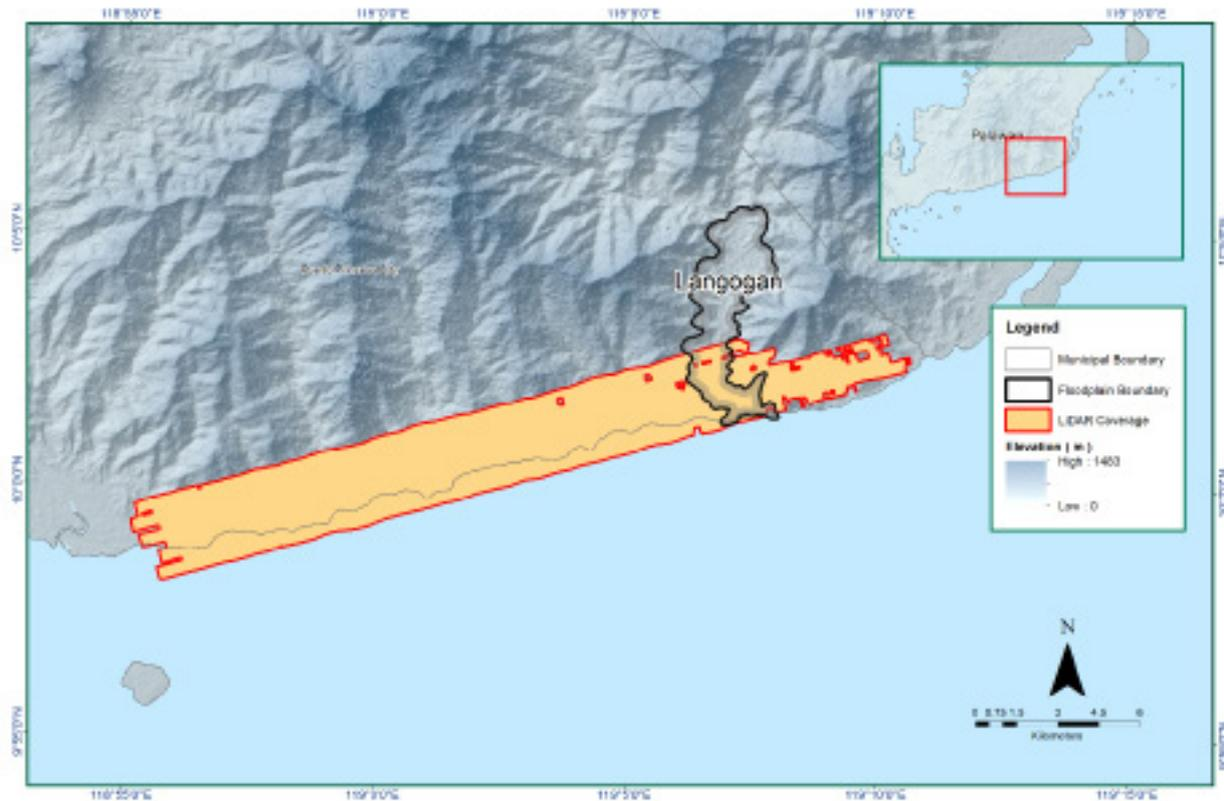
Figure 11. Boundaries of the processed LiDAR data over the Langogan Floodplain.
