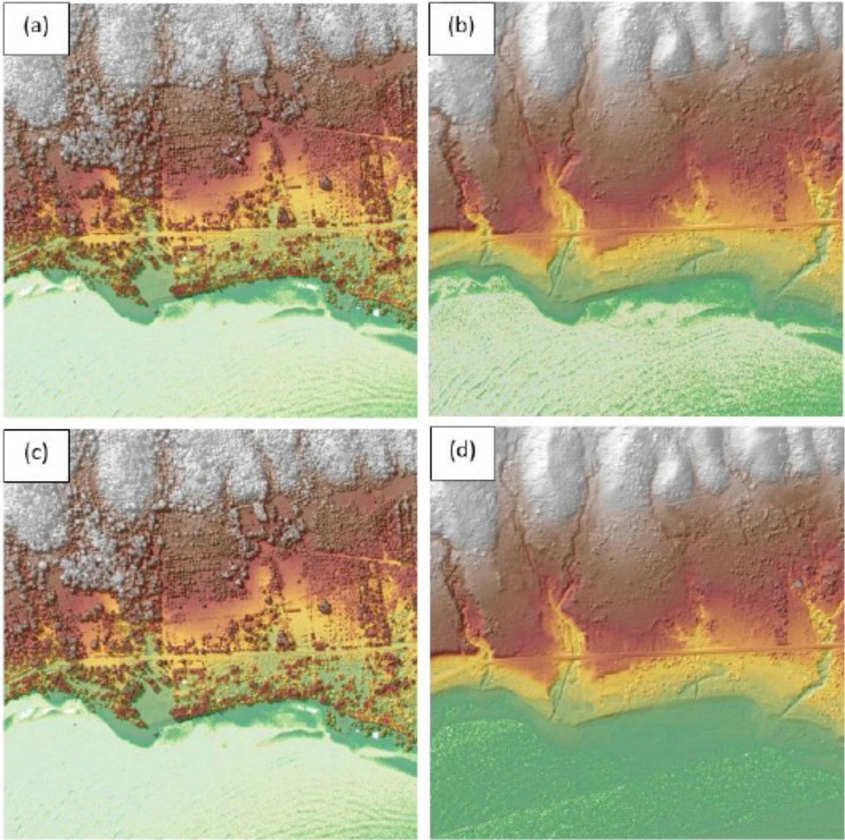
Figure 18. The production of last return DSM (a) and DTM (b), first return DSM (c) and secondary DTM (d) in some portion of Langogan floodplain.
