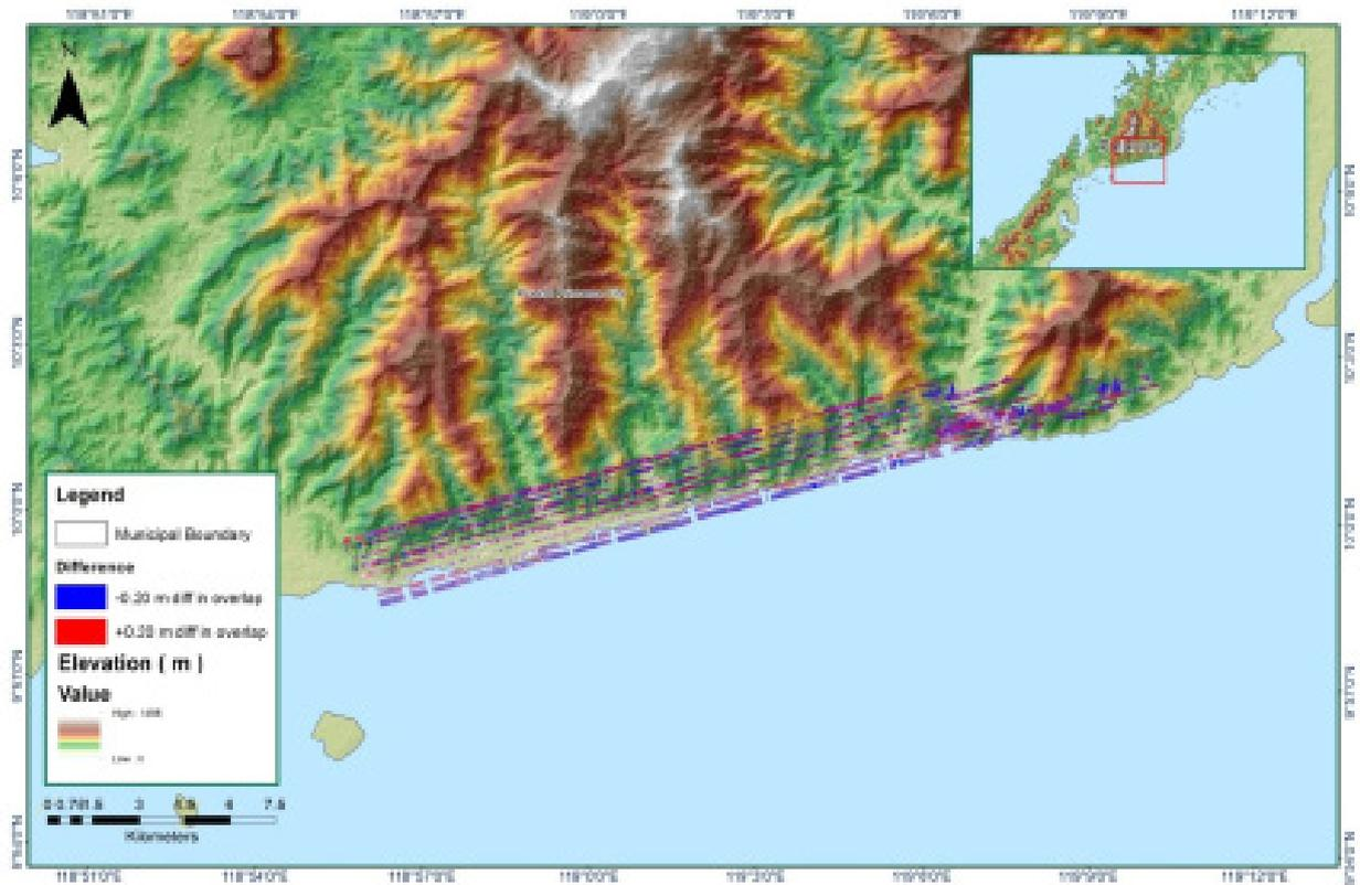
Figure A-8.7. Elevation difference between flight lines
