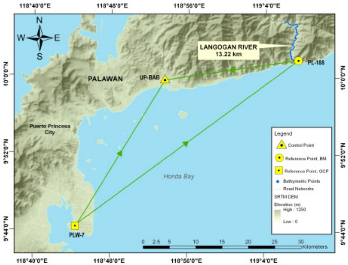
Figure 28. The GNSS Network established in the Langogan River Survey.
