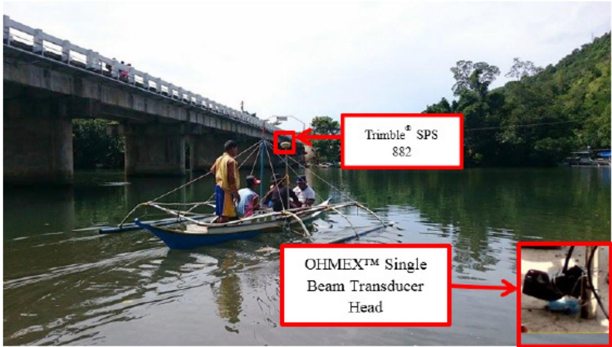
Figure 39. Set up of the bathymetric survey at Langogan River.
