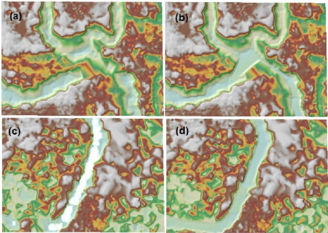
Figure 19. Portions in the DTM of the Langogan Floodplain – a portion of a waterway before (a) and after (b) manual editing; and a data gap before (c) and after (d) filling.
