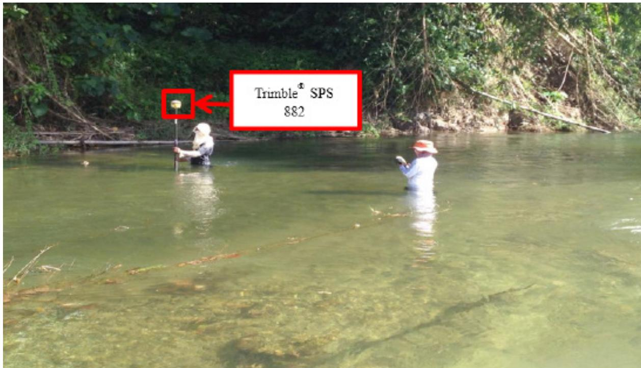
Figure 40. Setup of manual bathymetry survey for Langogan River using a Trimble® SPS 882.
