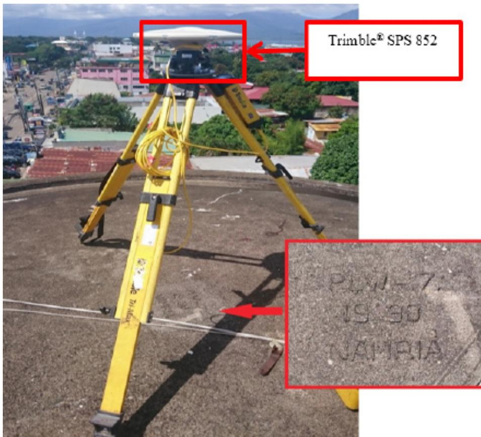
Figure 29. GNSS receiver set up, Trimble® SPS SPS 852, at PLW-7 at an old water tank inside the Water District compound, Brgy. Maningning, Puerto Prinsesa, Palawan.
