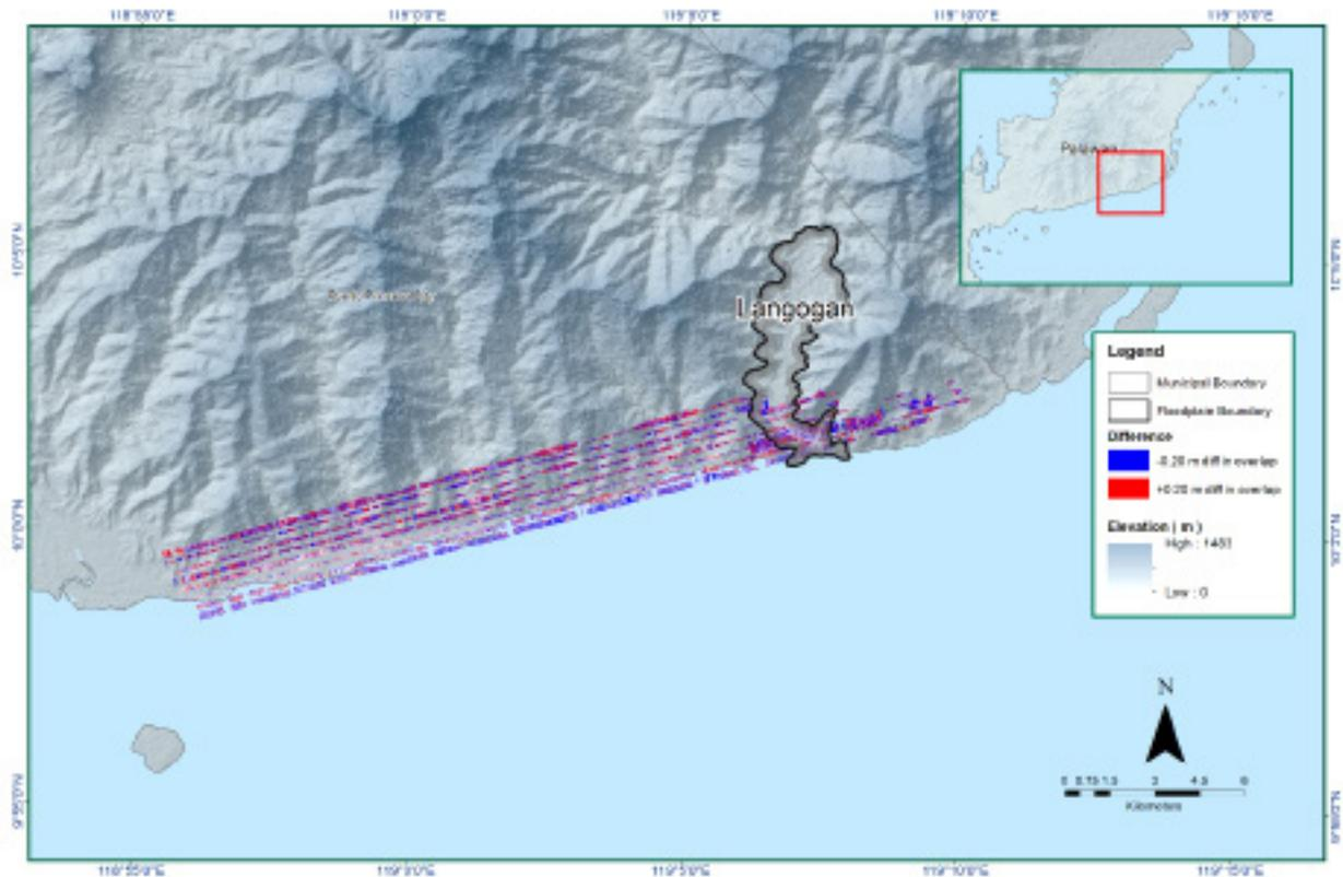
Figure 14. Elevation difference Map between flight lines for the Langogan Floodplain Survey
