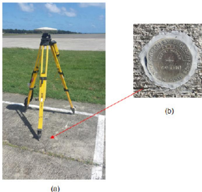
Figure 5. GPS set-up over PVP-1 (a) as recovered on the ground beside Puerto Princesa Airport Fire Station; and reference point PVP-1 (b) as recovered by the field team.
