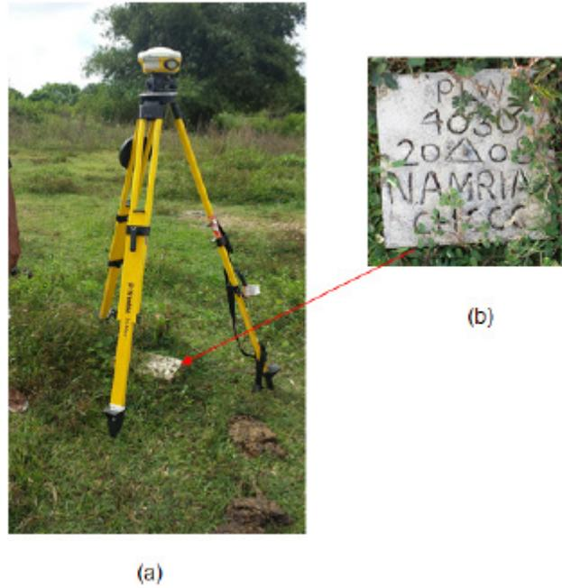
Figure 4. GPS set-up over PLW-4030 (a) as recovered on the ground beside Jolo Bridge Roxas, Palawan; and NAMRIA reference point PLW-4030 (b) as recovered by the field team.
