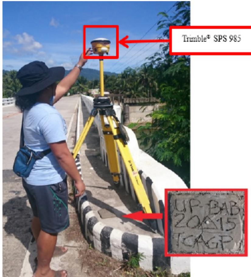
Figure 31. GNSS receiver set up, Trimble® SPS SPS 852, at UP-BAB in Babuyan Bridge, Brgy.Maoyon, Puerto Prinsesa, Palawan.
