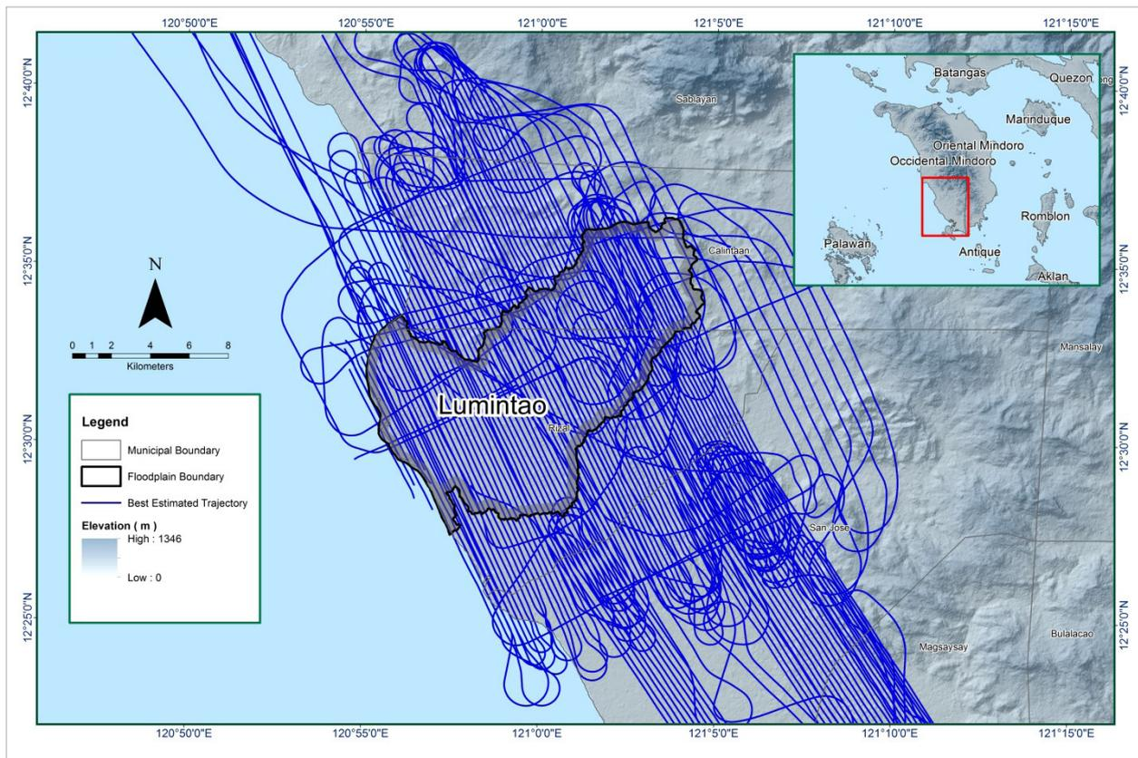
Figure 10. Best Estimated Trajectory for Lumintao floodplain.
