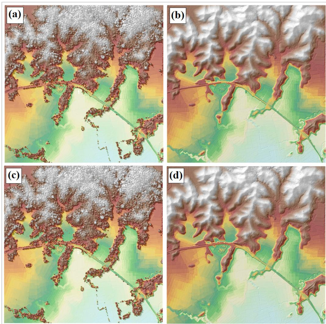
Figure 18. The production of last return DSM (a) and DTM (b), first return DSM (c) and secondary DTM (d) in some portion of Lumintao floodplain.
