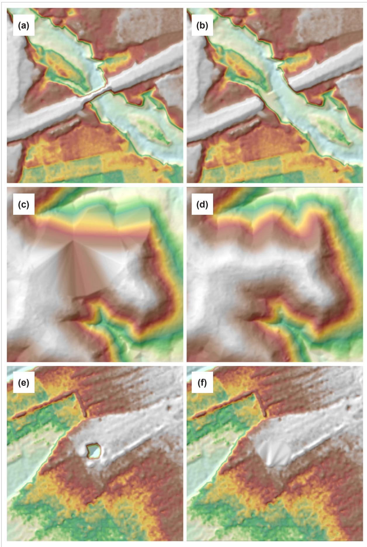
Figure 21. Portions in the DTM of Lumintao floodplain – a bridge before (a) and after (b) manual editing; a mountain before (c) and after (d) data retrieval; a pit before (e) and after (f) interpolation.
