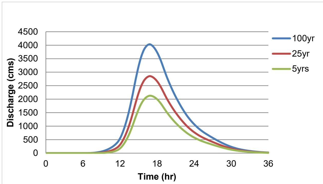
Figure 60. Lumintao river (5) generated discharge using 5-, 25-, and 100-year rainfall intensity-duration-frequency (RIDF) in HEC-HMS
