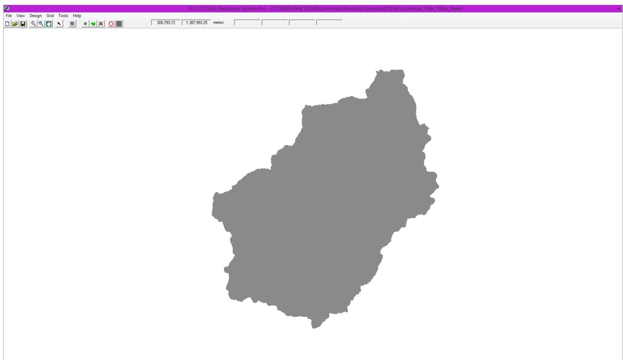
Figure 55. Screenshot of subcatchment with the computational area to be modeled in FLO-2D GDS Pro
