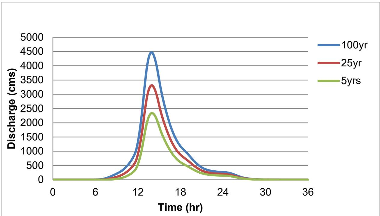
Figure 58. Lumintao river (3) generated discharge using 5-, 25-, and 100-year rainfall intensity-duration-frequency (RIDF) in HEC-HMS.
