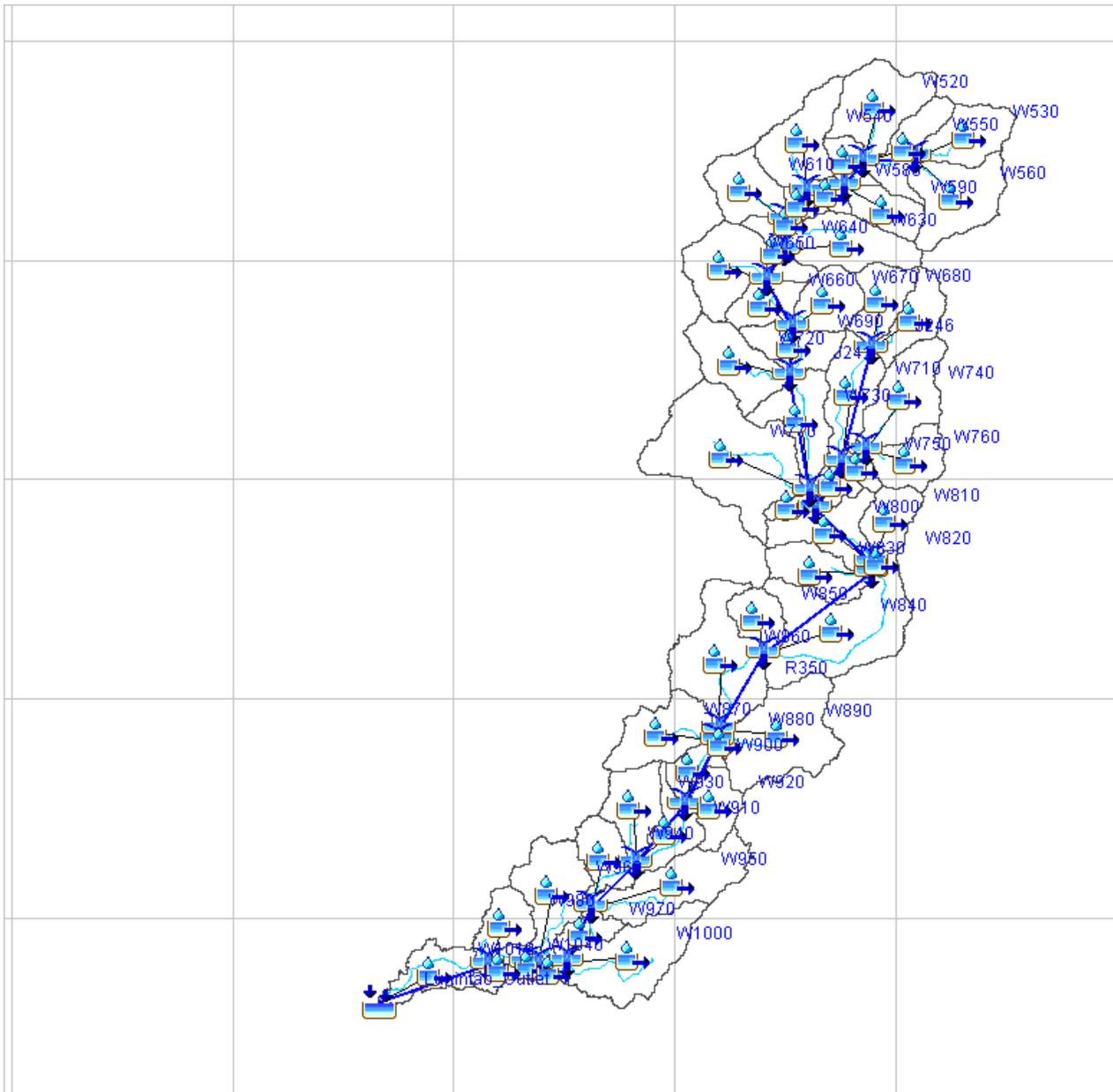
Figure 54. The Lumintao river basin model generated using HEC-HMS.
