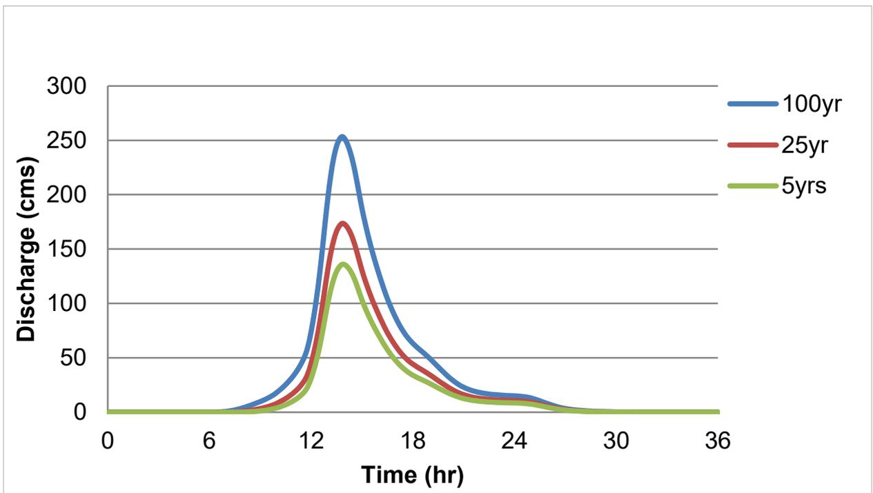
Figure 59. Lumintao river (4) generated discharge using 5-, 25-, and 100-year rainfall intensity-duration-frequency (RIDF) in HEC-HMS.
