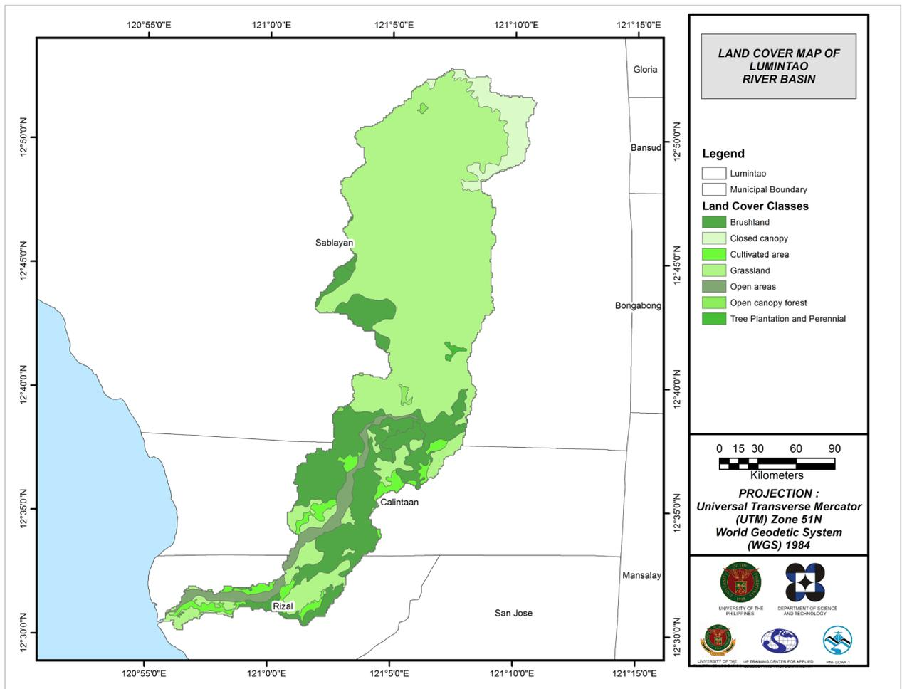
Figure 51. The land cover map of the Lumintao River Basin used for the estimation of the CN and watershed lag parameters of the rainfall-runoff model. (Source of data: Digital soil map of the Philippines published by the Bureau of Soil and Water Management – Department of Agriculture).
