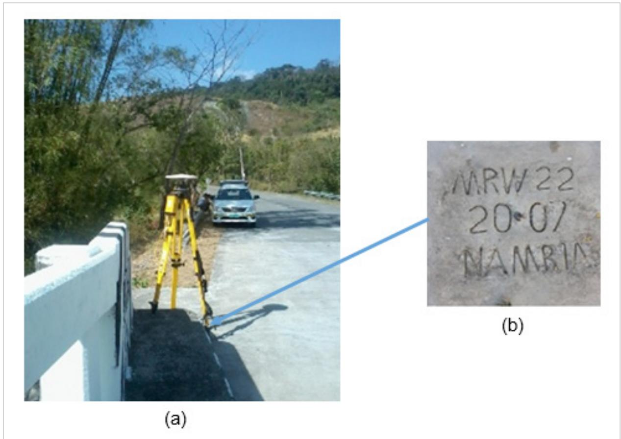
Figure 3. a) GPS set-up over MRW-22 located at Lumintao Bridge in Brgy. Tanyag, Municipality of Calintaan, Occidental Mindoro. b) NAMRIA reference point MRW-22 as recovered by the field team.
