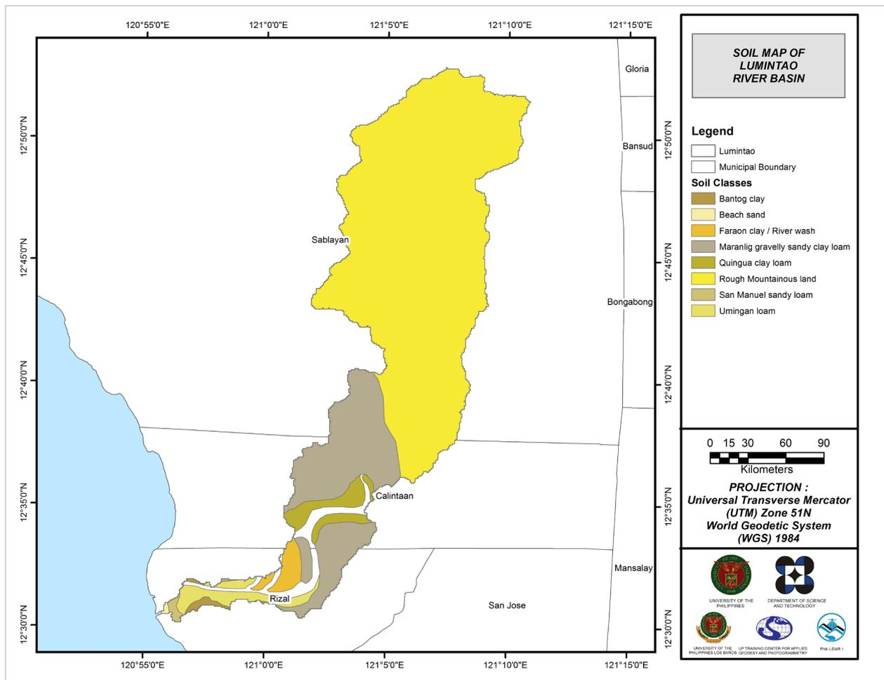
Figure 50. The soil map of the Lumintao River Basin used for the estimation of the CN parameter. (Source of data: Digital soil map of the Philippines published by the Bureau of Soil and Water Management – Department of Agriculture).
