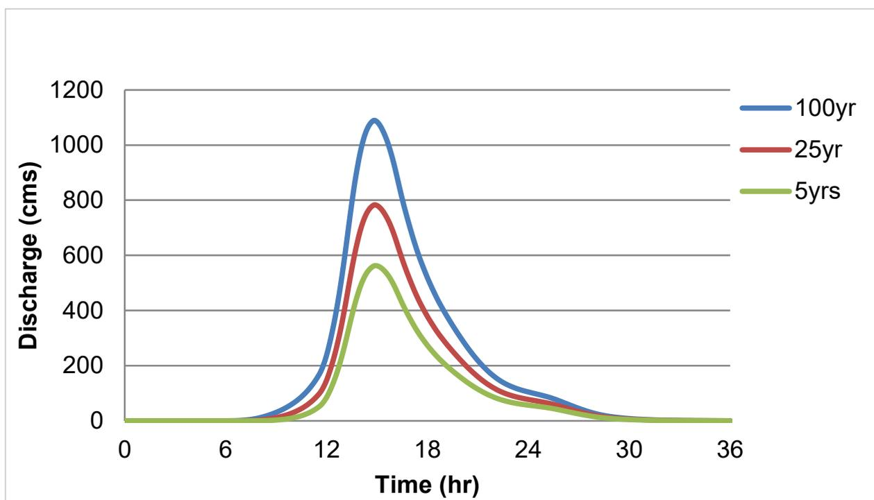
Figure 57. Lumintao river (2) generated discharge using 5-, 25-, and 100-year rainfall intensity-duration-frequency (RIDF) in HEC-HMS.
