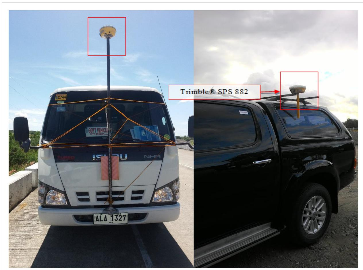
Figure 43. Validation points acquisition survey set-up.
