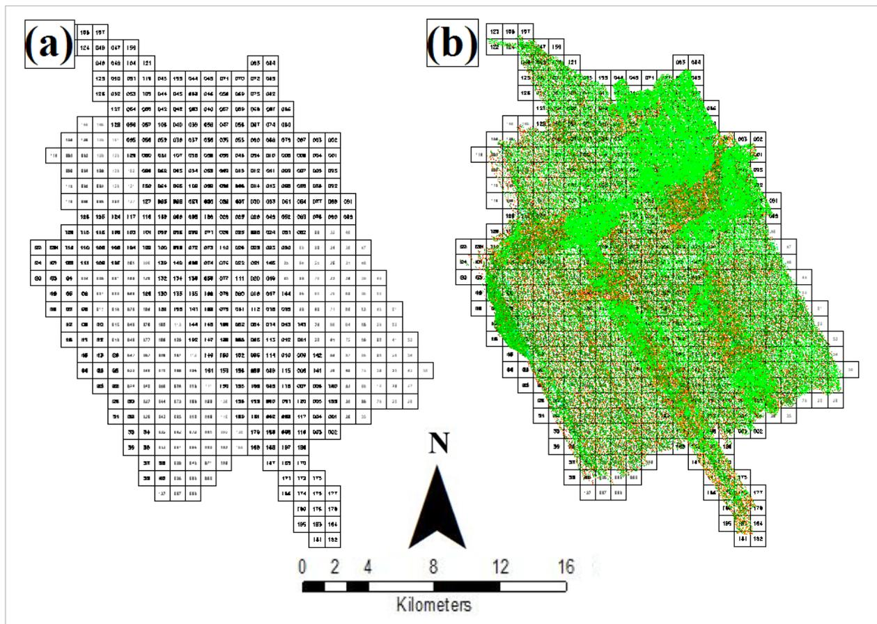
Figure 16. Tiles for Lumintao floodplain (a) and classification results (b) in TerraScan.
