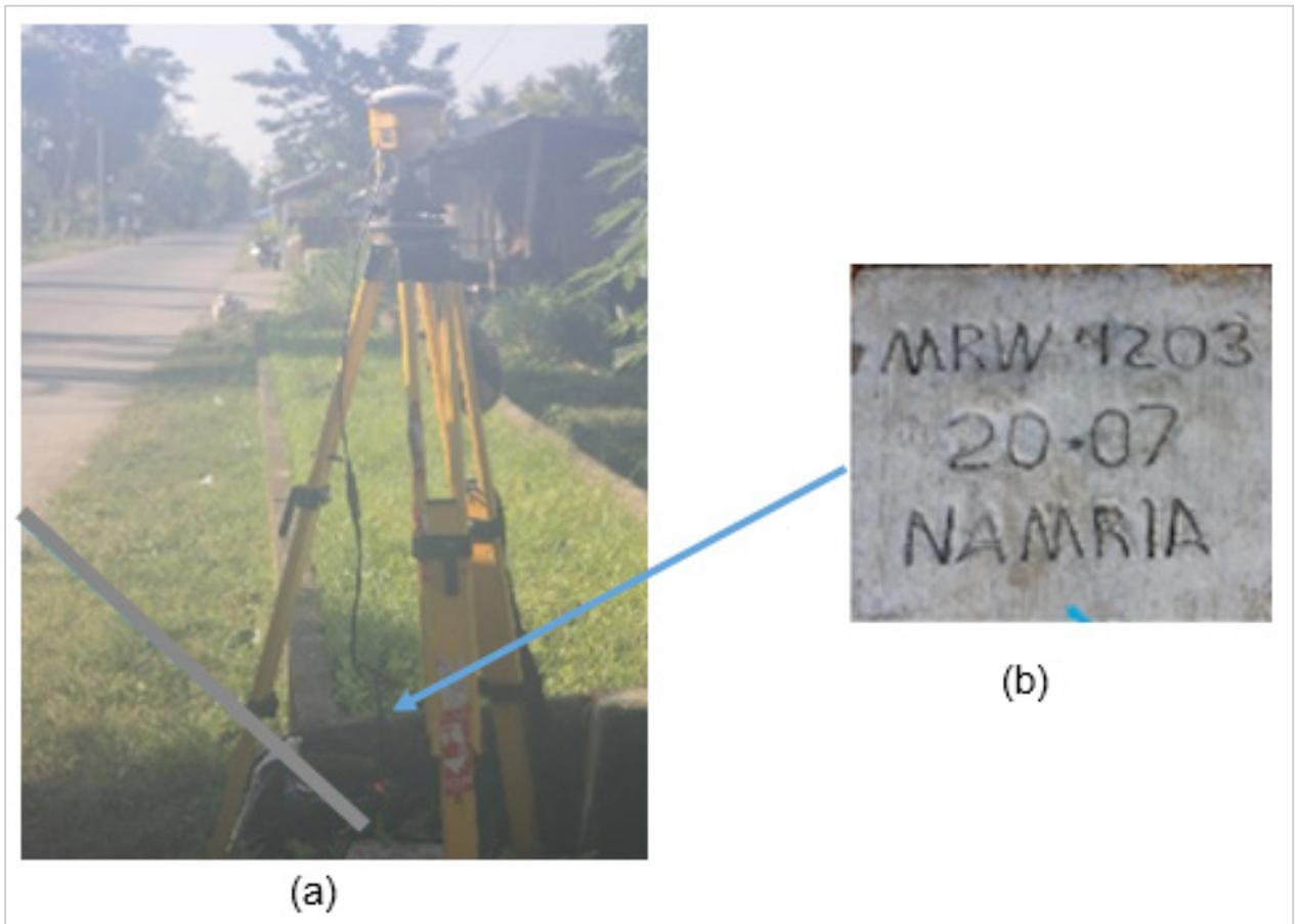
Figure 5. a) GPS set-up over MRW-4203 located in front of the barangay hall of Brgy. Mapaya, Municipality of San Jose, Occidental Mindoro b) NAMRIA reference point MRW-4203 as recovered by the field team.
