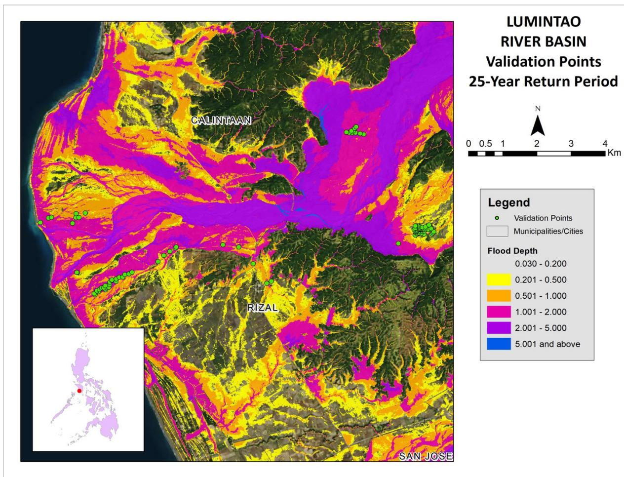
Figure 76. Validation points for 25-year Flood Depth Map of Lumintao Floodplain.
