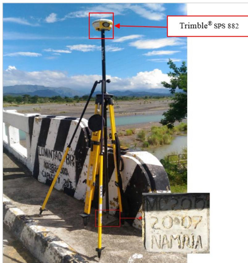
Figure 31. GNSS receiver set-up, Trimble® SPS 882, at MC-200, Lumintao Bridge approach in Brgy. Magsikap, Municipality of Rizal, Occidental Mindoro.
