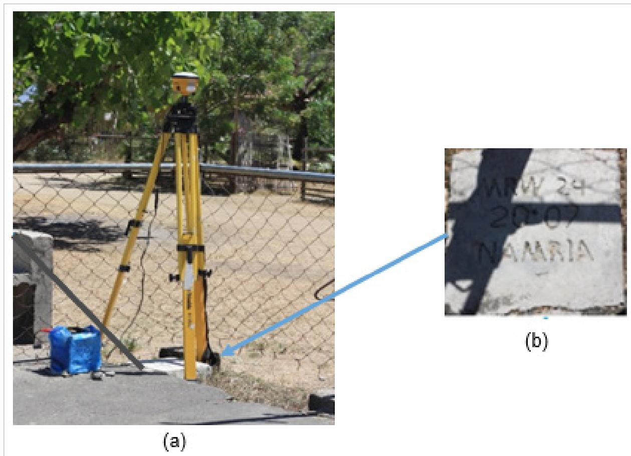
Figure 4. a) GPS set-up over MRW-24 located at the basketball court in Brgy. Iriron, Municipality of Calintaan, Occidental Mindoro b) NAMRIA reference point MRW-24 as recovered by the field team.
