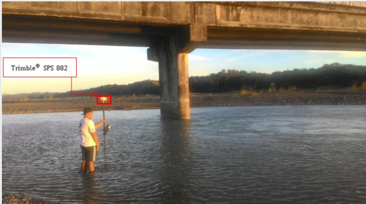
Figure 38. Bridge as-built and cross-section survey at the downstream side of Lumintao Bridge, Brgy. Magsikap, Municipality of Rizal
