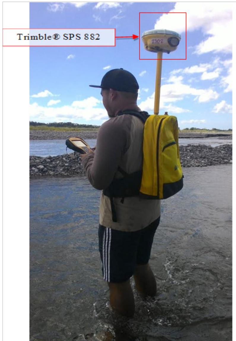
Figure 45. Manual Bathymetry along Lumintao River.
