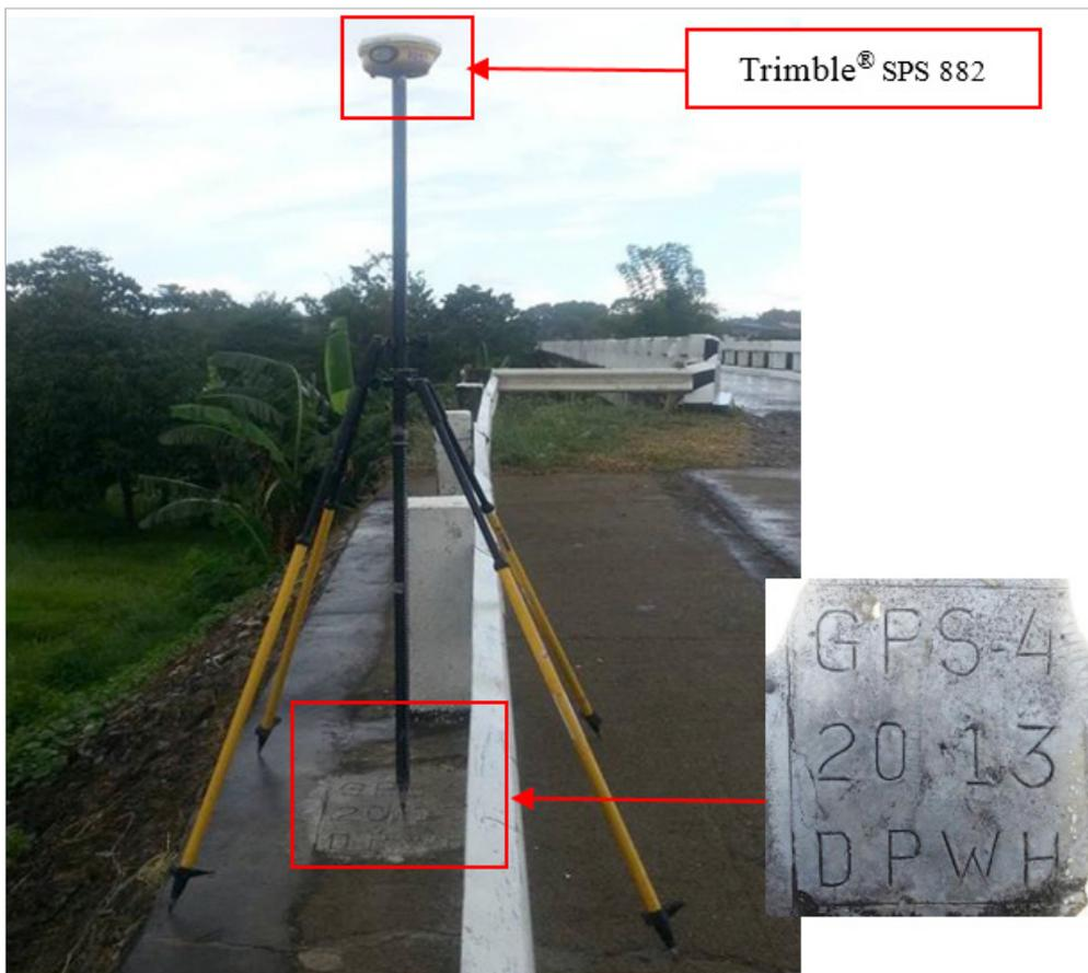
Figure 34. GNSS receiver, Trimble® SPS 882, at GPS-4 on right side of the road abutment after Caguray Bridge going to Bulalacao in Brgy. Poblacion, Municipality of Magsaysay, Occidental Mindoro.
