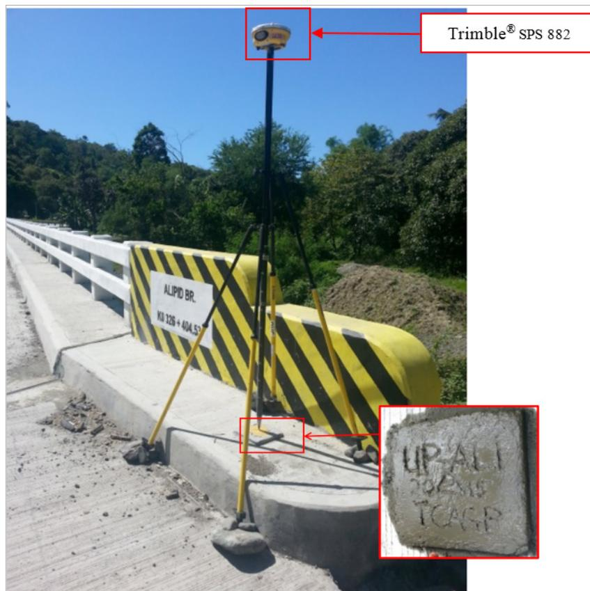
Figure 37. GNSS receiver set up, Trimble® SPS 882, at UP-ALI, Alipid Bridge approach in Brgy. Sto. Niño, Municipality of Sablayan, Occidental Mindoro
