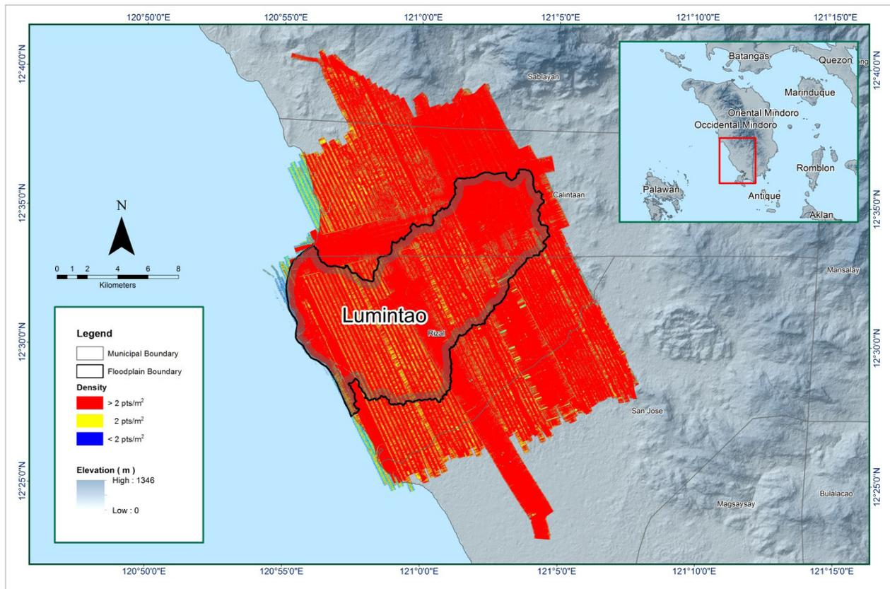
Figure 13. Pulse density map of merged LiDAR data for Lumintao Floodplain.
