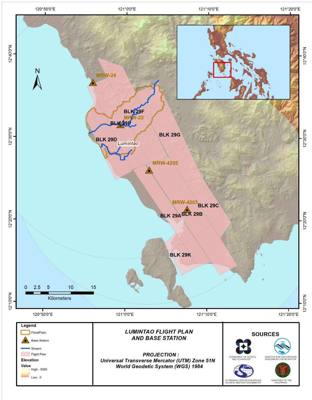
Figure 1. Flight plans used for Lumintao floodplain using Aquarius Sensor.
