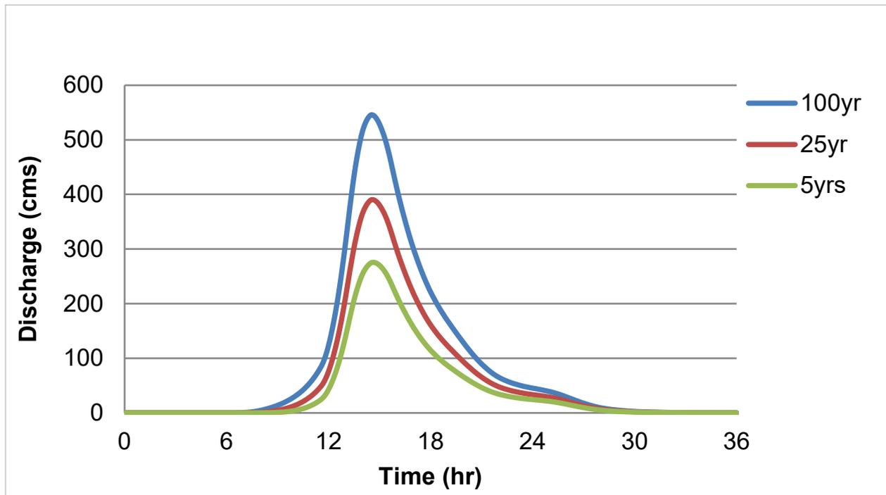
Figure 56. Lumintao river (1) generated discharge using 5-, 25-, and 100-year rainfall intensity-duration-frequency (RIDF) in HEC-HMS.
