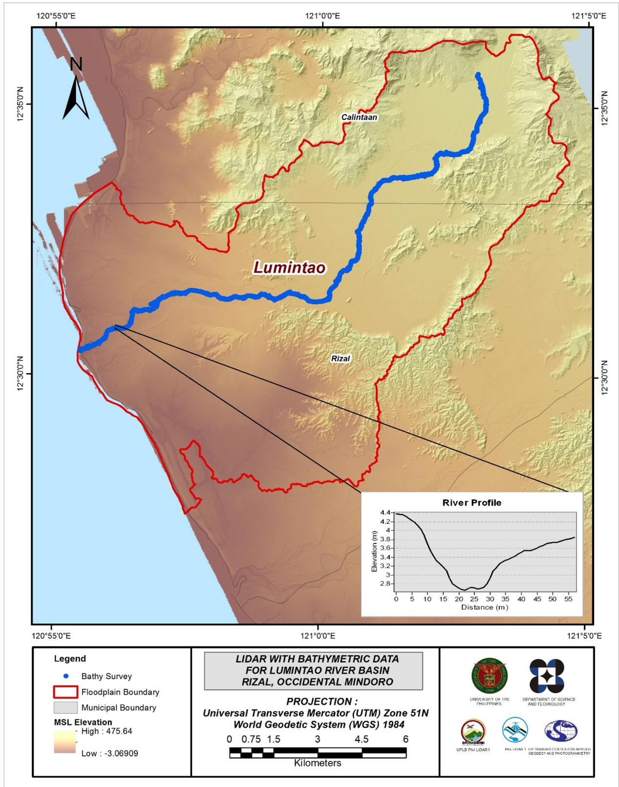
Figure 26. Map of Lumintao Flood Plain with bathymetric survey points shown in blue.
