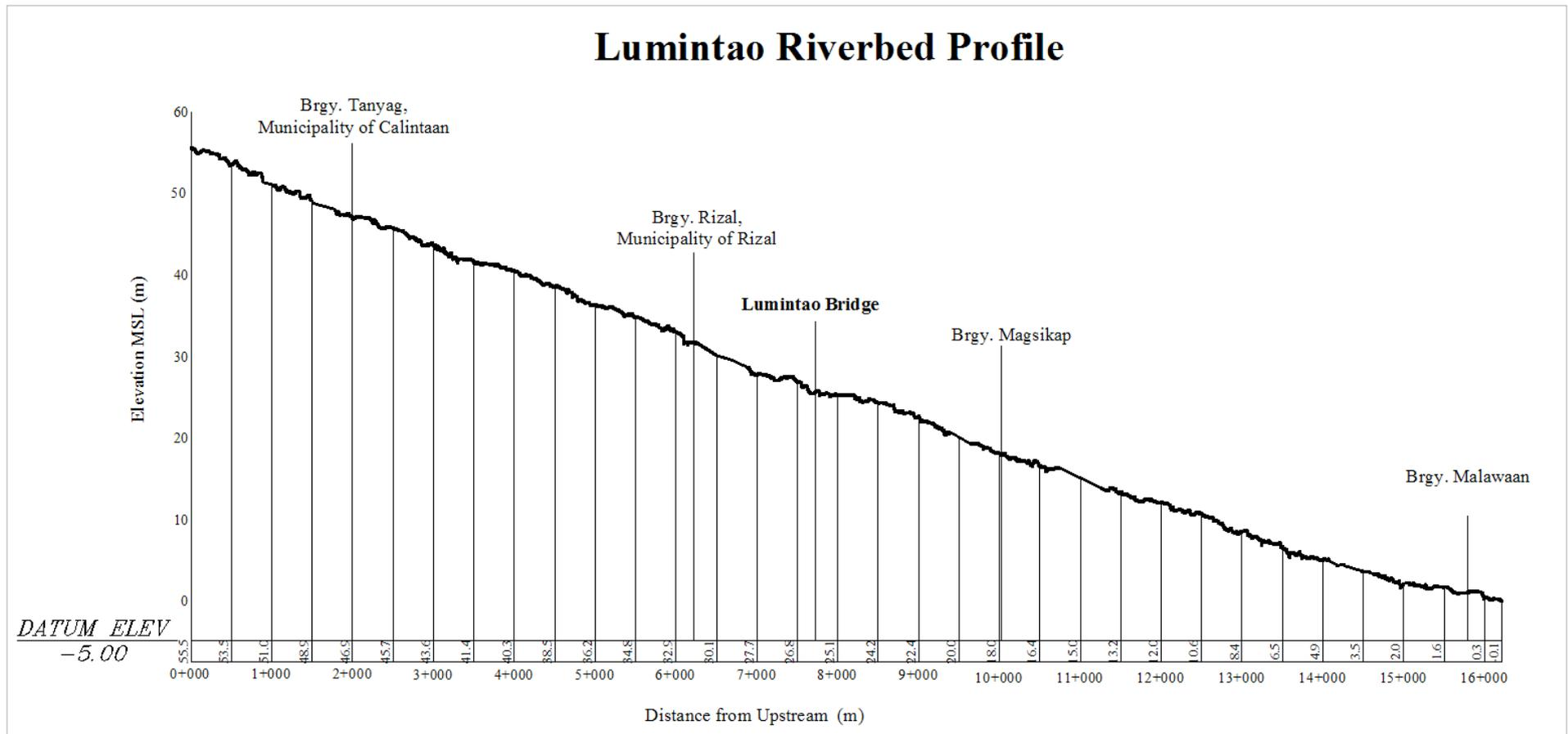
Figure 47. Riverbed profile of Lumintao River.
