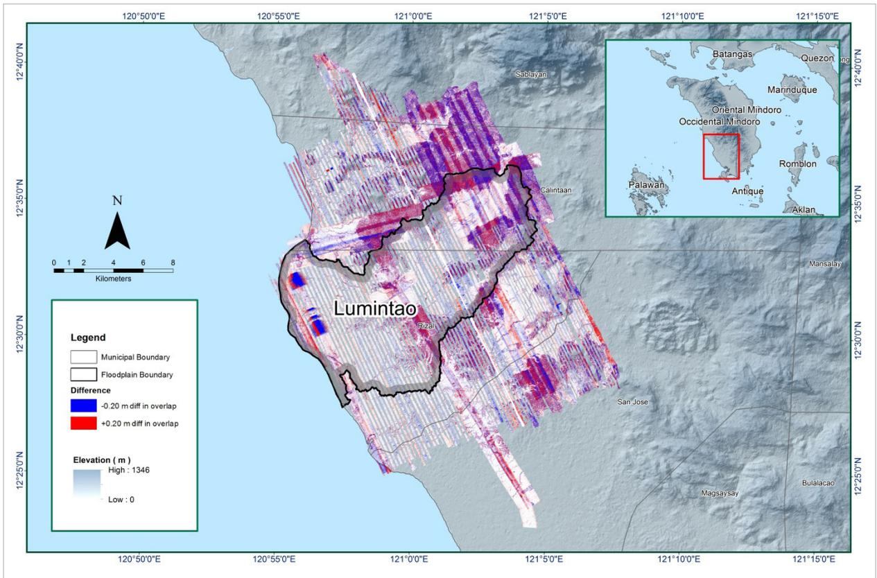
Figure 14. Elevation difference map between flight lines for Lumintao floodplain.
