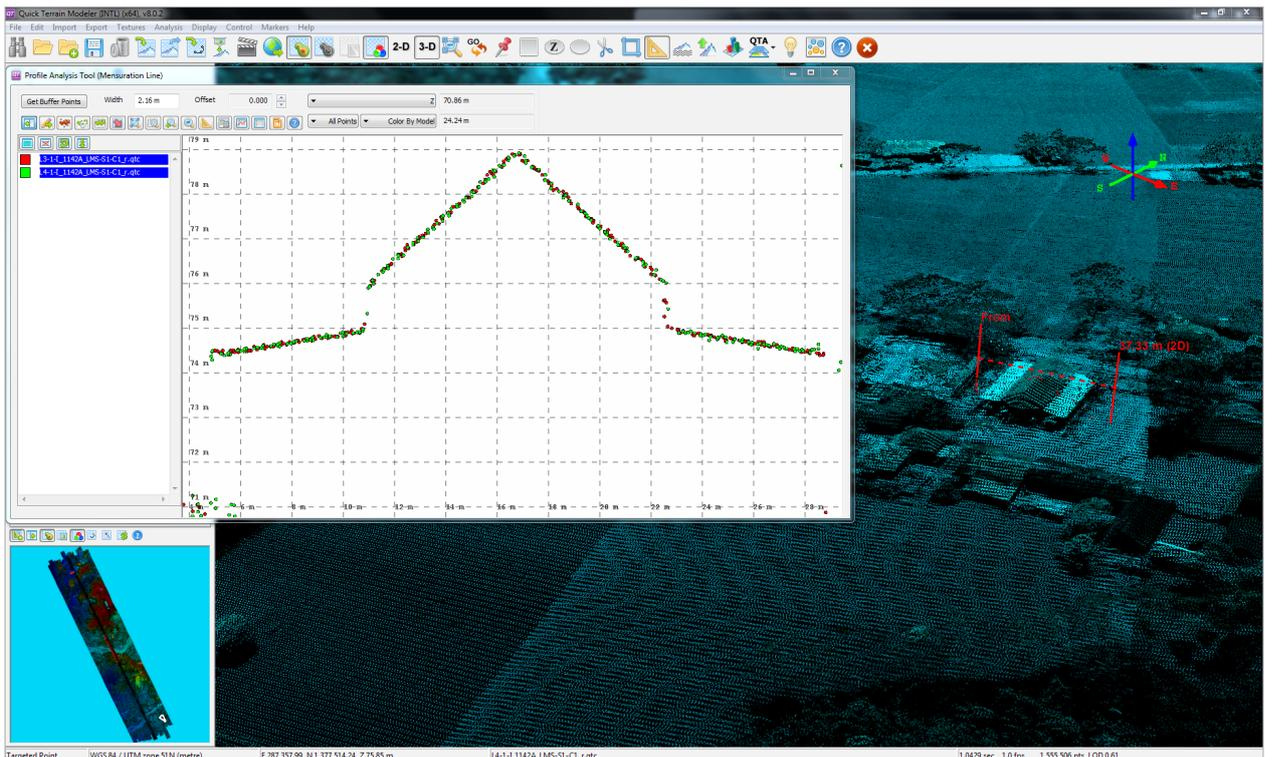
Figure 15. Quality checking for a Lumintao flight 1142AA using the Profile Tool of QT Modeler.
