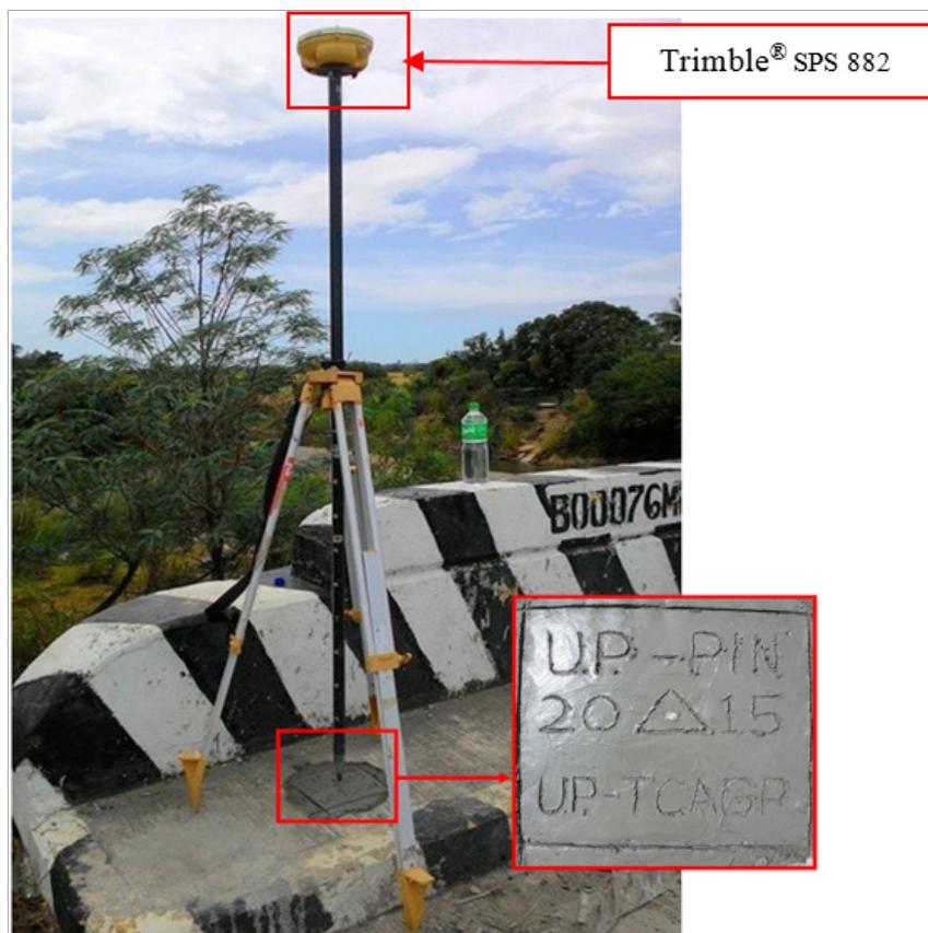
Figure 35. GNSS base receiver set-up, Trimble® SPS 882, at UP-PIN Pinamanaán Bridge approach in Brgy. Mapaya, Municipality of San Jose, Occidental Mindoro
