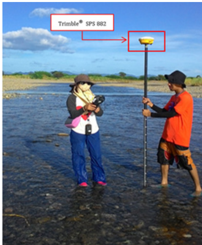
Figure 48. Manual Bathymetry along Magbando River
