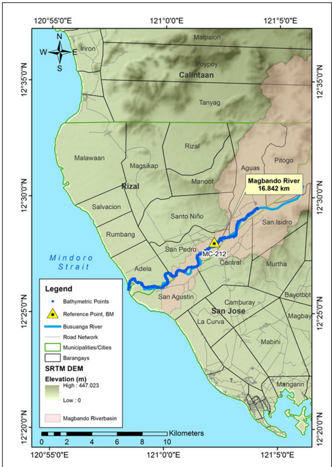
Figure 49. Bathymetric survey of Magbando River
