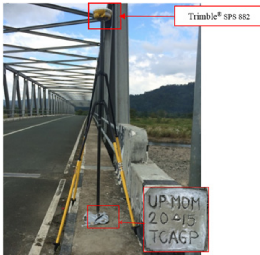
Figure 39. GNSS receiver set-up, Trimble® SPS 882, at UP-MOM, Mompong Bridge approached in Brgy. Lumang Bato, Municipality of Sablayan, Occidental Mindoro
