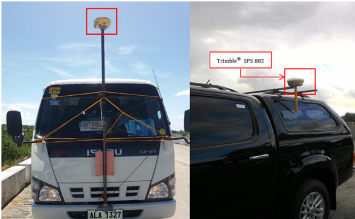
Figure 46. Trimble® SPS8 82 set-up for validation points acquisition survey for Magbando River
