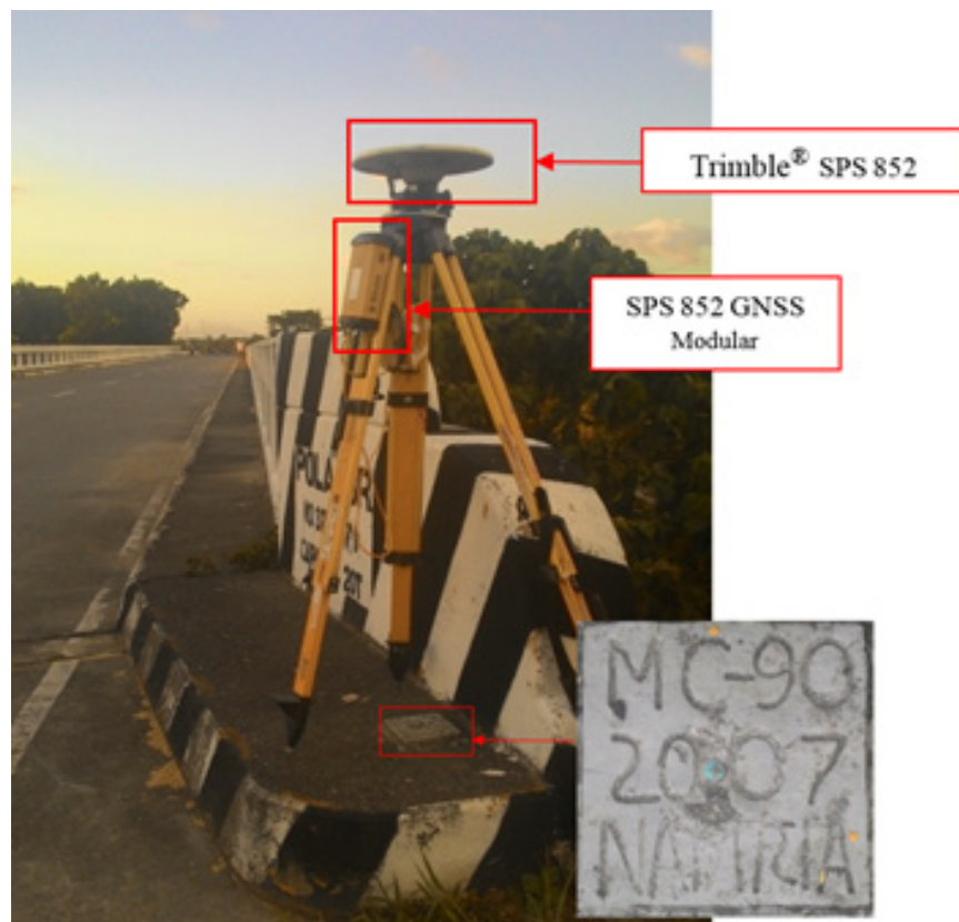
Figure 36. GNSS base, Trimble® SPS 852, at MC-90, used as marker, located at the Pola Bridge approach in Brgy. Barahan, Municipality of Santa Cruz, Occidental Mindoro
