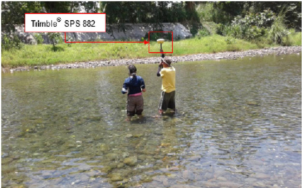
Figure 41. Gathering of bathymetric checking points along Malambunga River
