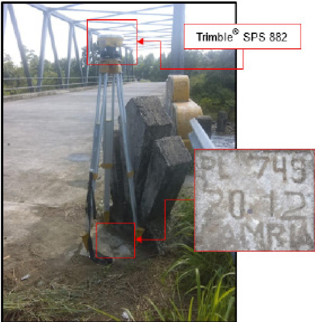
Figure 28. GNSS base set-up, Trimble® SPS 882, at PL-749, located in front of a monument near the approach of Ilog-Ilog Bridge in Brgy. Campong Ulay, Rizal, Province of Palawan
