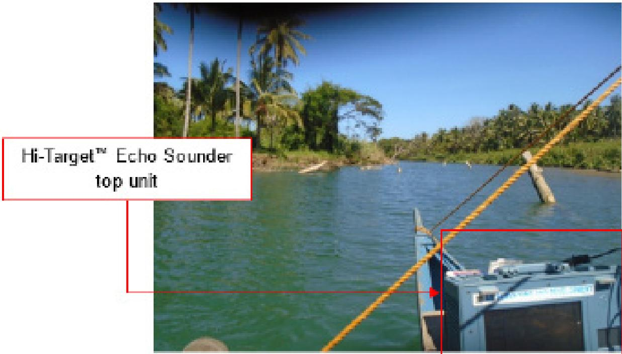
Figure 38. Bathymetric survey of ABSD at Malambunga River using a Hi-Target™ Echo Sounder
