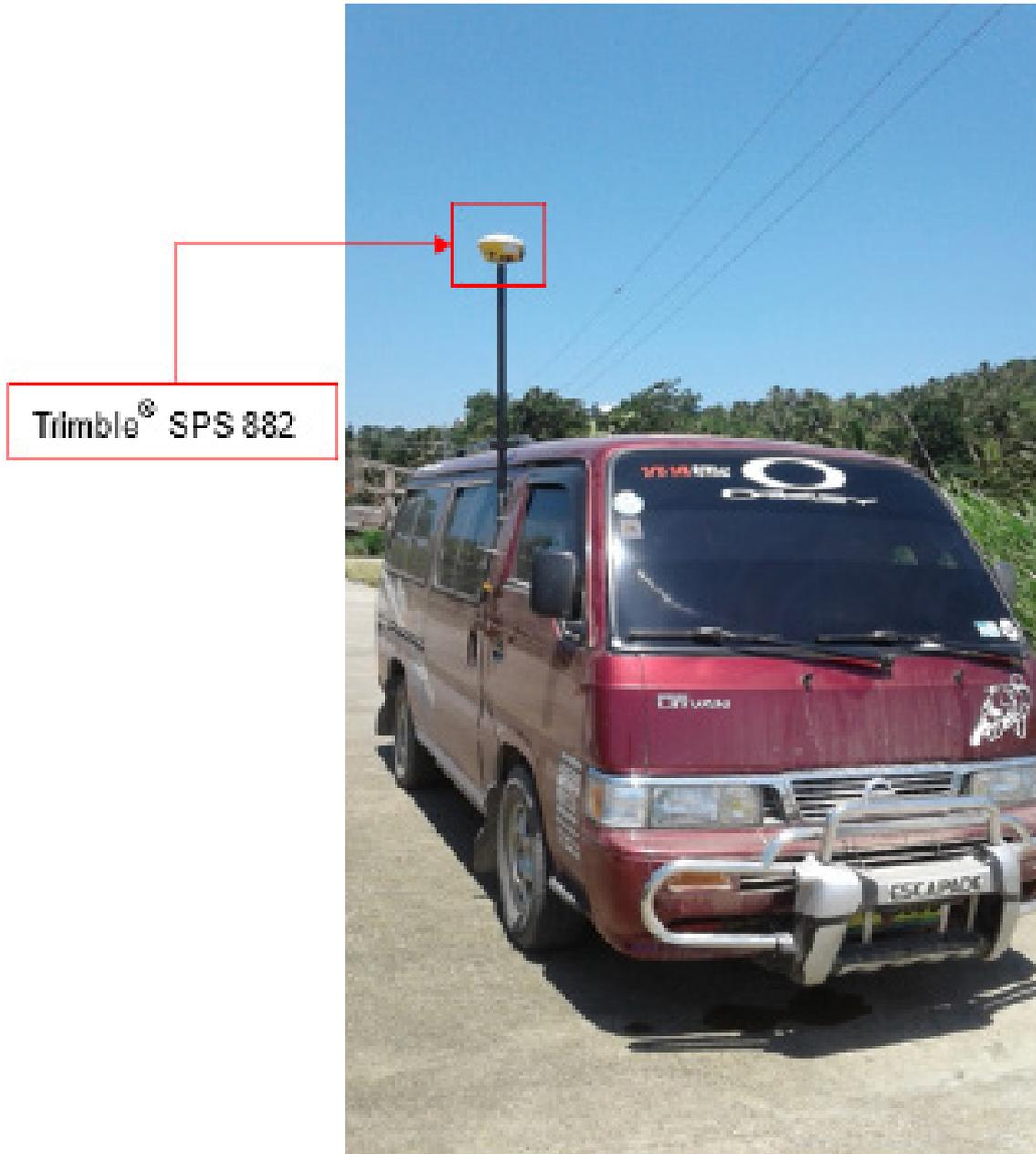
Figure 36. Validation points acquisition survey set up along Malambunga River Basin
