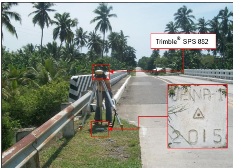
Figure 34. GNSS receiver set up, Trimble® SPS 882, at UP\_INA-1, located beside the approach of Inagauan Bridge in Brgy. Inagauan Sub-Colony, Puerto Princesa City, Palawan
