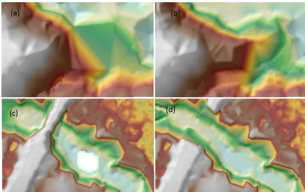
Figure 19. Portions in the DTM of Malatgao Floodplain –a flattened surface before (a) and after (b) object retrieval; and a bridge before (c) and after (d) manual editing
