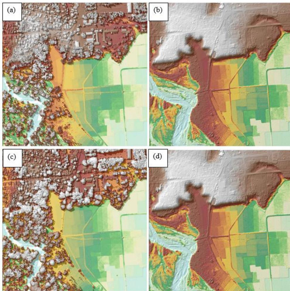
Figure 16. The production of last return DSM (a) and DTM (b), first return DSM (c) and secondary DTM (d) in some portion of Malatgao Floodplain
