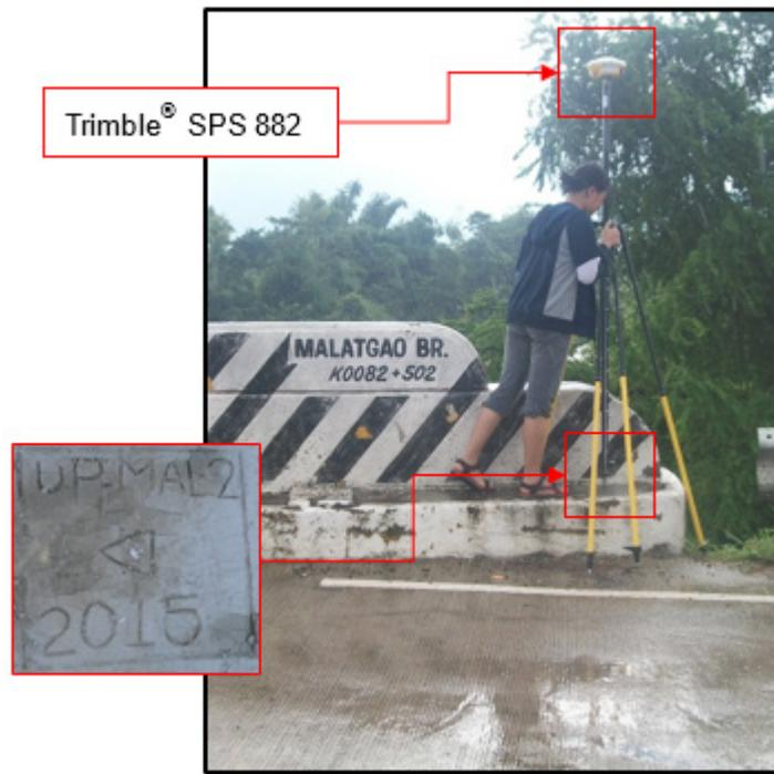
Figure 31. GNSS receiver set up, Trimble® SPS 882, at UP\_MAL-2, located at the approach of Malatgao Bridge in Brgy. Tinagong Dagat, Narra, Province of Palawan
