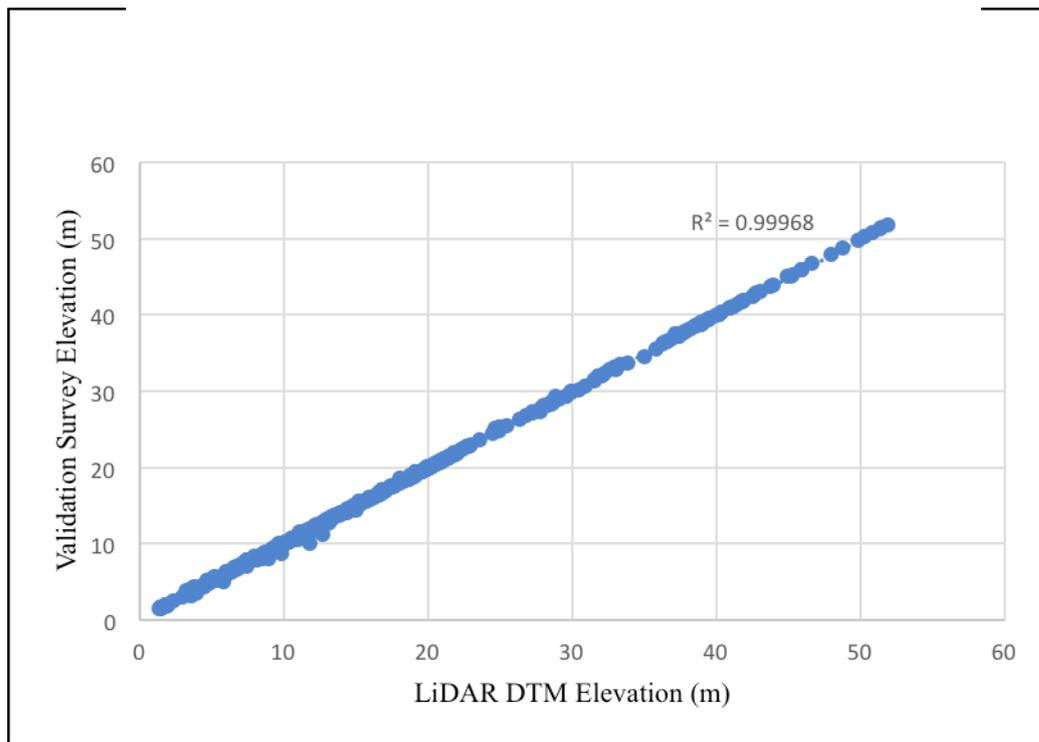
Figure 23. Correlation plot between validation survey points and LiDAR data
