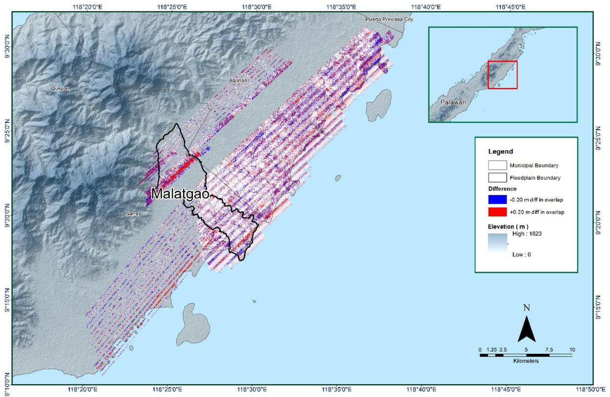
Figure 12. Elevation difference map between flight lines for Malatgao Floodplain
