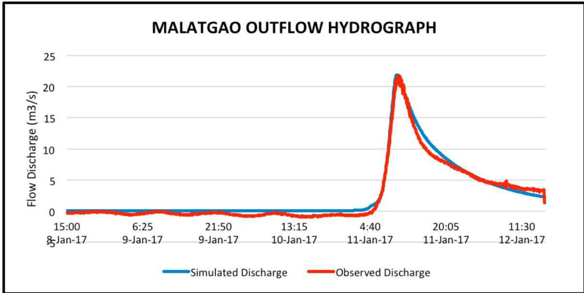
Figure 60. Outflow Hydrograph of Malatgao produced by the HEC-HMS model compared with observed outflow
