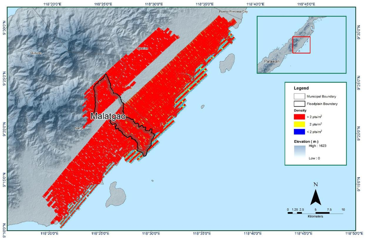
Figure 11. Density map of merged LiDAR data for Malatgao Floodplain
