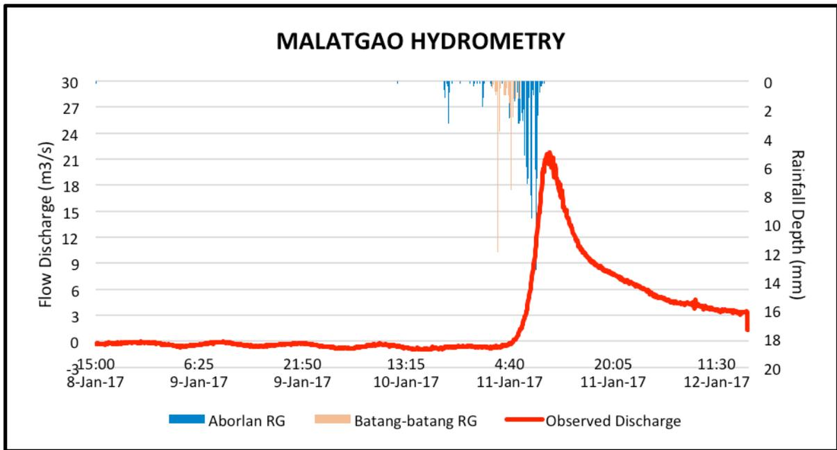
Figure 51. Rainfall and outflow data at Malatgao used for modeling
