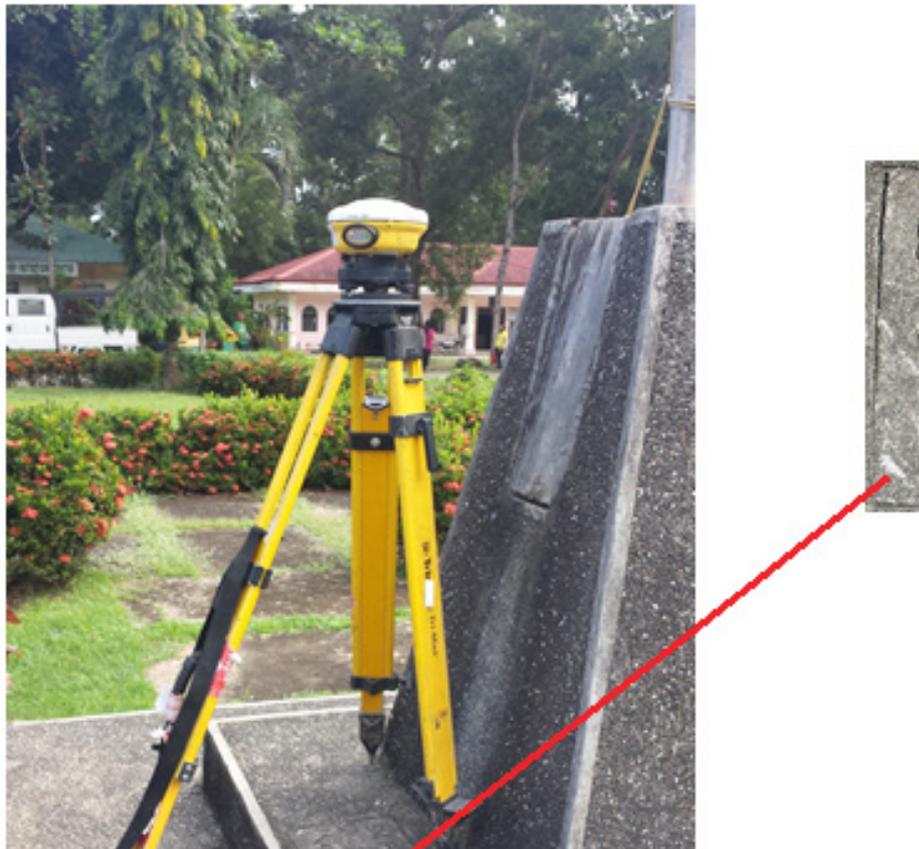
Figure 3. GPS set-up over PVP-1 located on the ground beside Puerto Princesa Airport Fire Station (a) and reference point PVP-1 (b) as recovered by the field team
