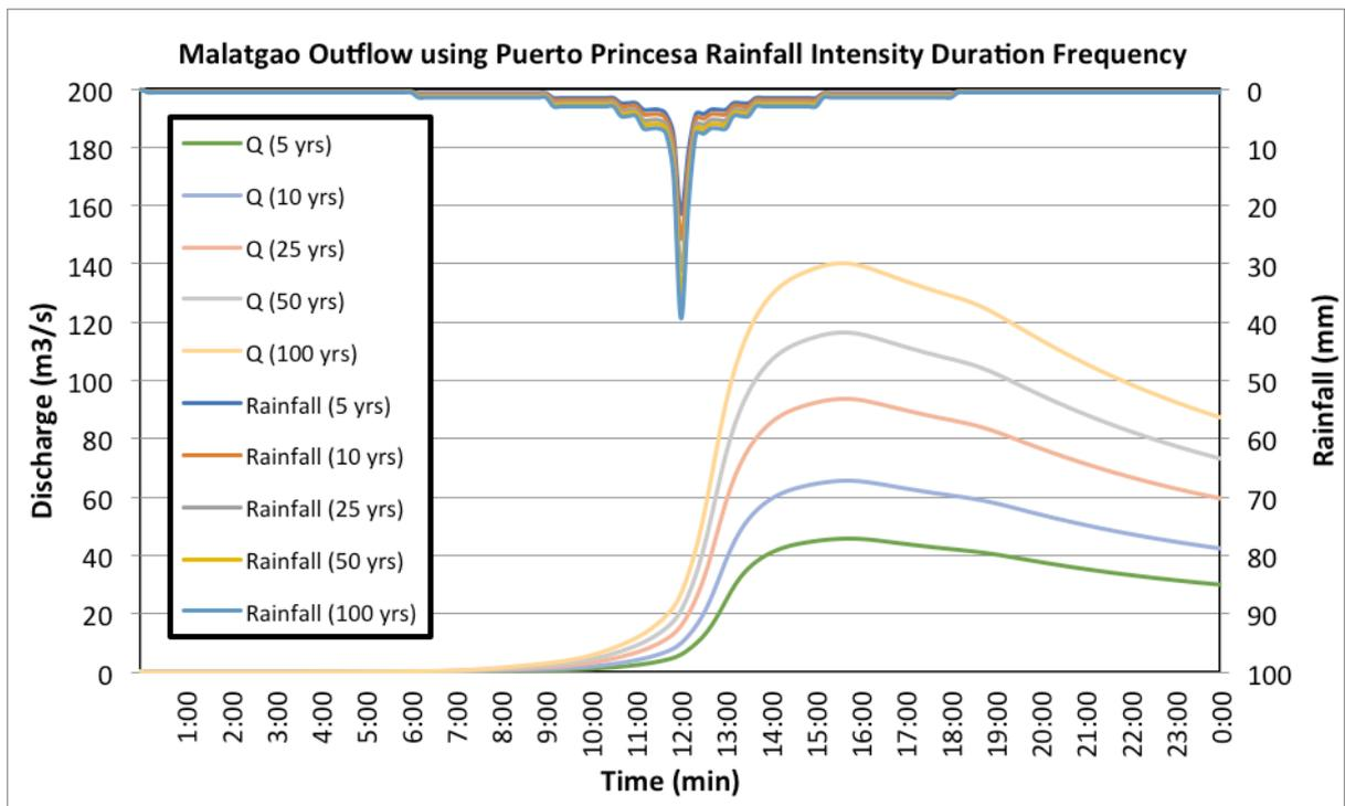
Figure 61. Outflow hydrograph at Malatgao Station generated using Puerto Princesa RIDF simulated in HEC-HMS
