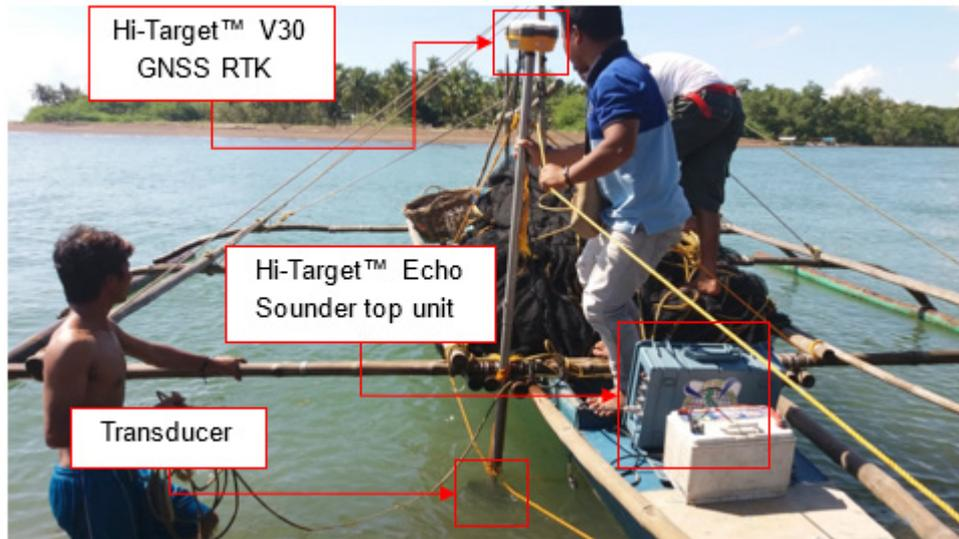
Figure 43. Bathymetric survey of ABSD at Malasgao River using Hi-Target™ Echo Sounder (downstream)
