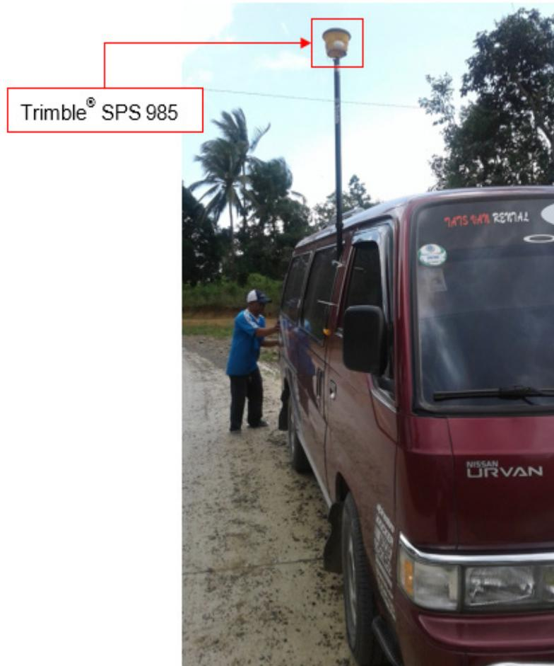
Figure 41. Validation points acquisition survey set-up for Malatgao River
