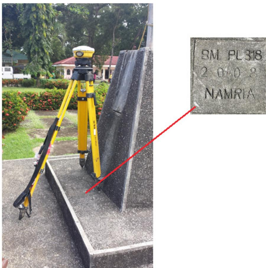
Figure 2. GPS set-up over PL-318 as recovered inside Aborlan Municipal Hall, Aborlan Palawan (a) and NAMRIA vertical control point PL-318 (b) as recovered by the field team
