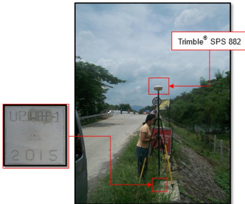
Figure 32. GNSS receiver set up, Trimble® SPS 982, at UP\_IWA-P-1, located at the approach of Iwahig Penal Bridge in Brgy. Iwahig, Puerto Princesa City, Palawan
