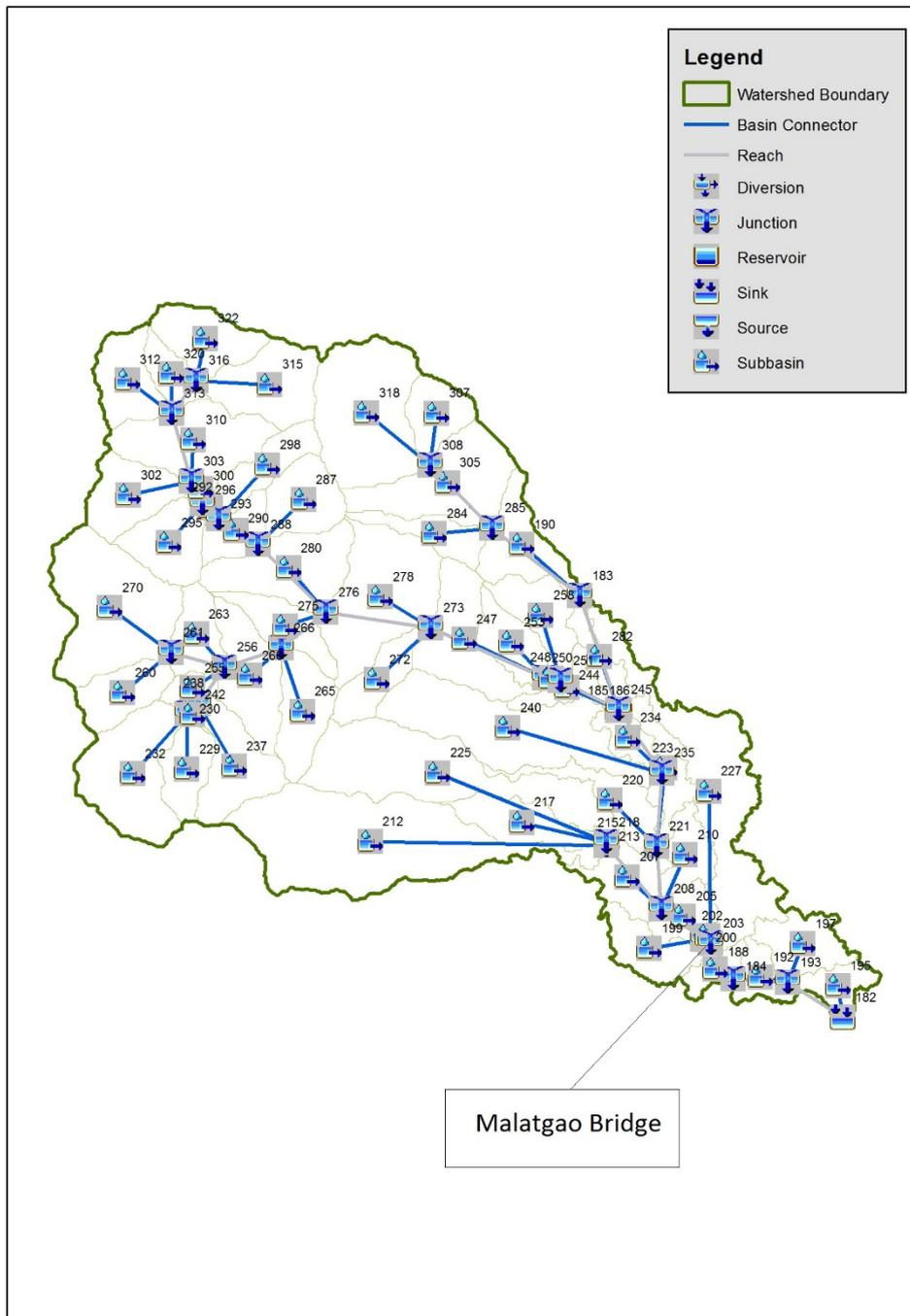
Figure 58. The Malatgao River Basin Model generated using HEC-HMS
