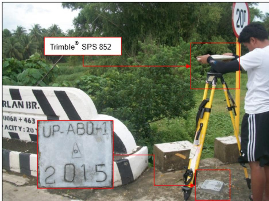
Figure 33. GNSS receiver set-up, Trimble® SPS 852, at UP\_ABO-1, an established control point, beside the approach of Aborlan Bridge in Brgy. Gogognan, Aborlan, Palawan
