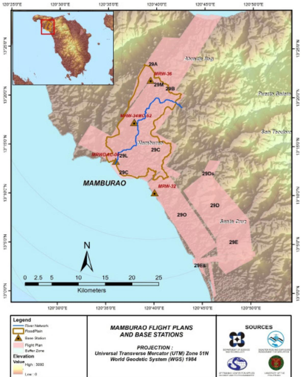
Figure 2. Flight plans and base stations used for Mamburao Floodplain survey
