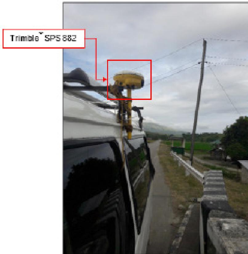
Figure 45. Validation points acquisition survey set-up for Mamburao River
