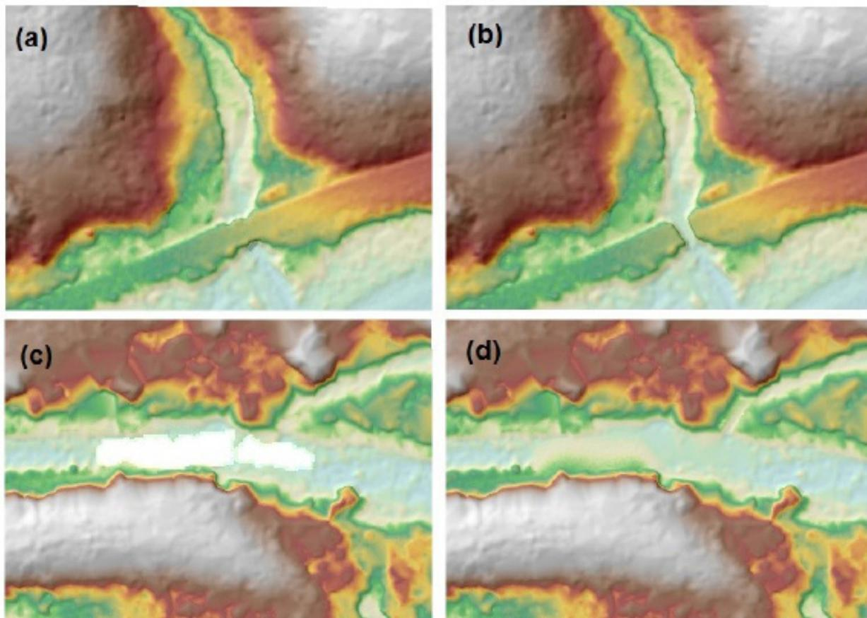
Figure 24. Portions in the DTM of Mamburao floodplain – a bridge before (a) and after (b) manual editing; and data gaps before (c) and after (d) filling.
