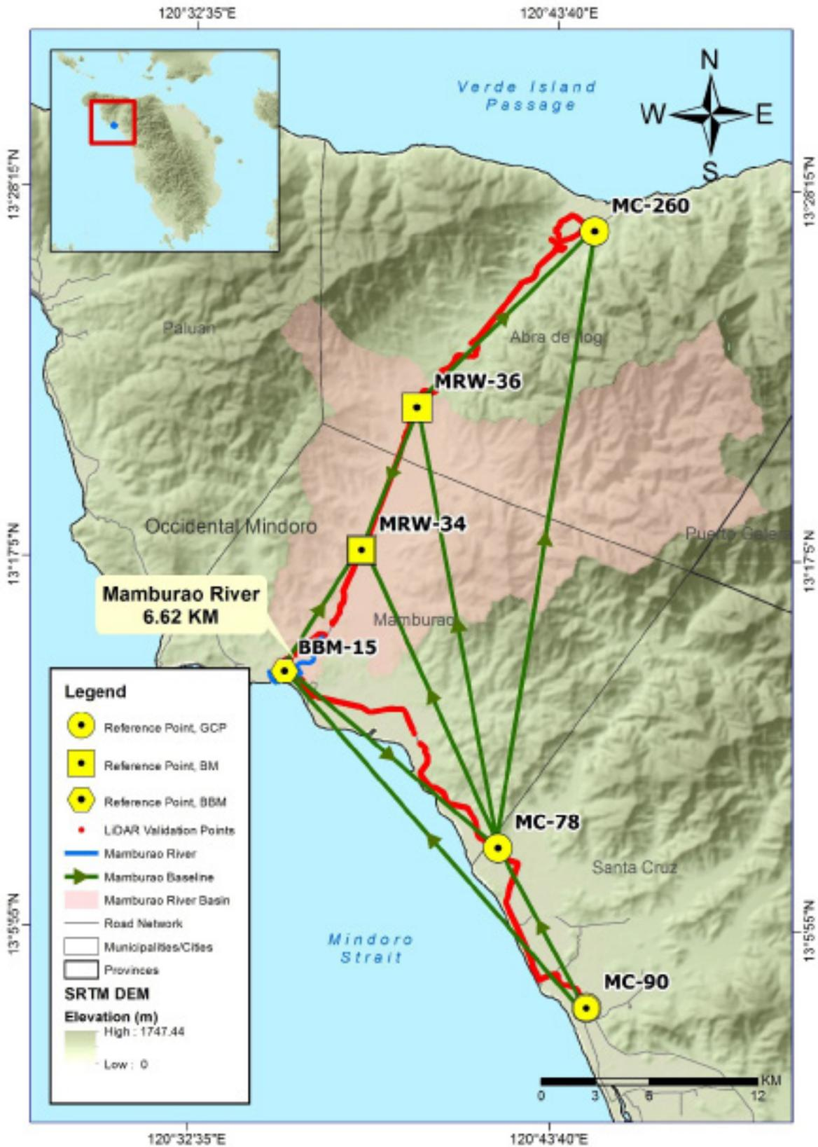
Figure 30. Extent of the bathymetric survey (blue line) in Mamburao River and the LiDAR data validation survey (red)
