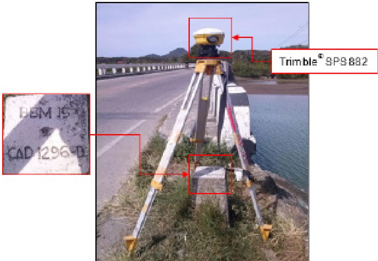
Figure 37. GNSS receiver set up, Trimble® SPS 882, at BBM-15, located beside the approach of Mamburao Bridge in Brgy. Poblacion 6, Mamburao, Occidental Mindoro
