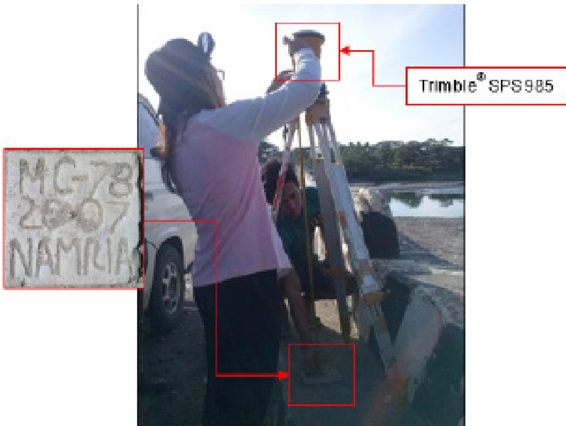
Figure 35. GNSS receiver set up, Trimble® SPS 985, at MC-78, located beside at the approach of Pagbahán Bridge in Brgy. San Vicente, Sta. Cruz, Occidental Mindoro
