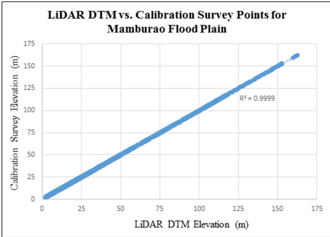
Figure 27. Correlation plot between calibration survey points and LiDAR data.
