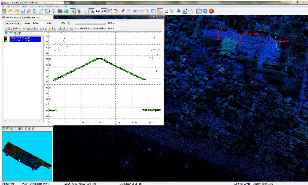
Figure 18. Quality checking for Mamburao flight 1120A using the Profile Tool of QT Modeler.
