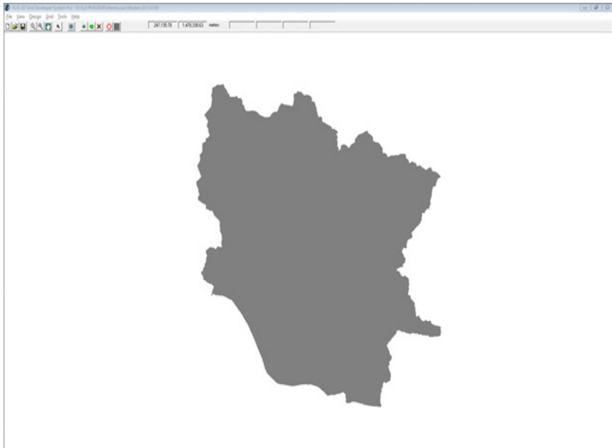
Figure 66. A screenshot of the river sub-catchment with the computational area to be modeled in FLO-2D Grid
