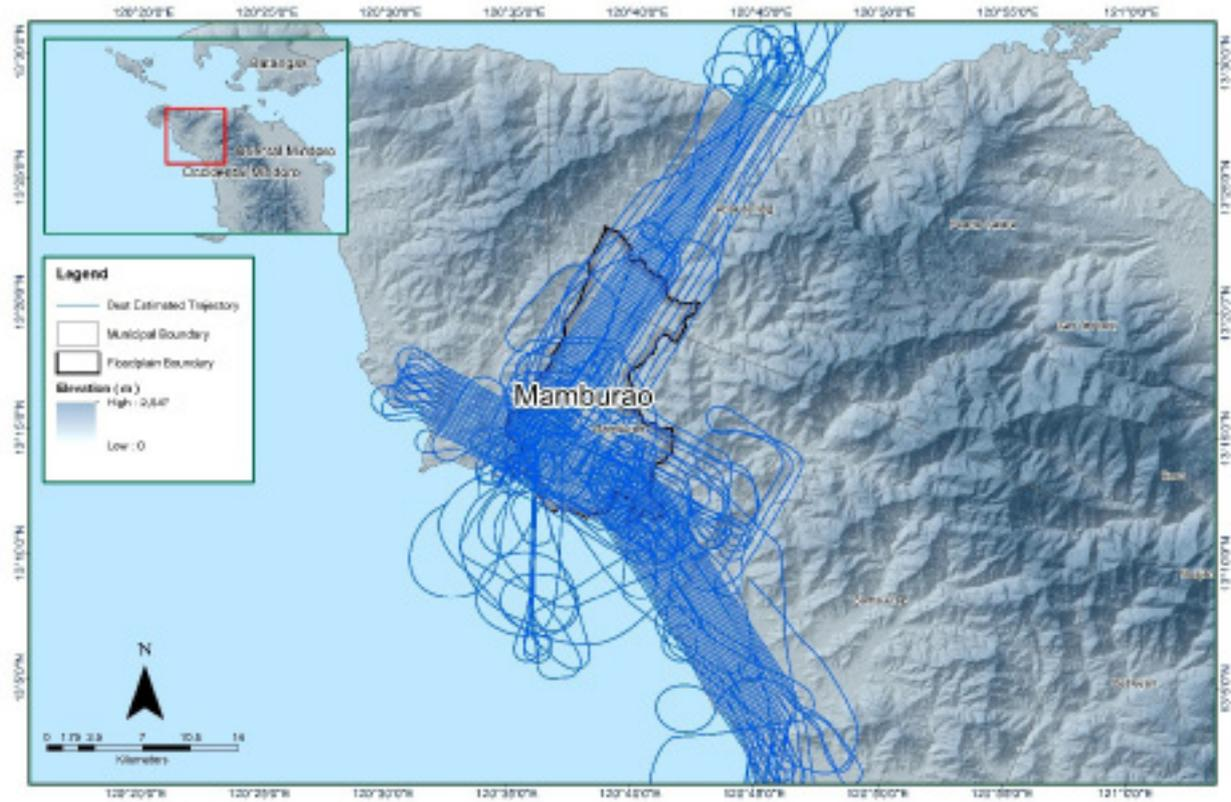
Figure 13. The best estimated trajectory of the LiDAR missions conducted over the Mamburao floodplain.
