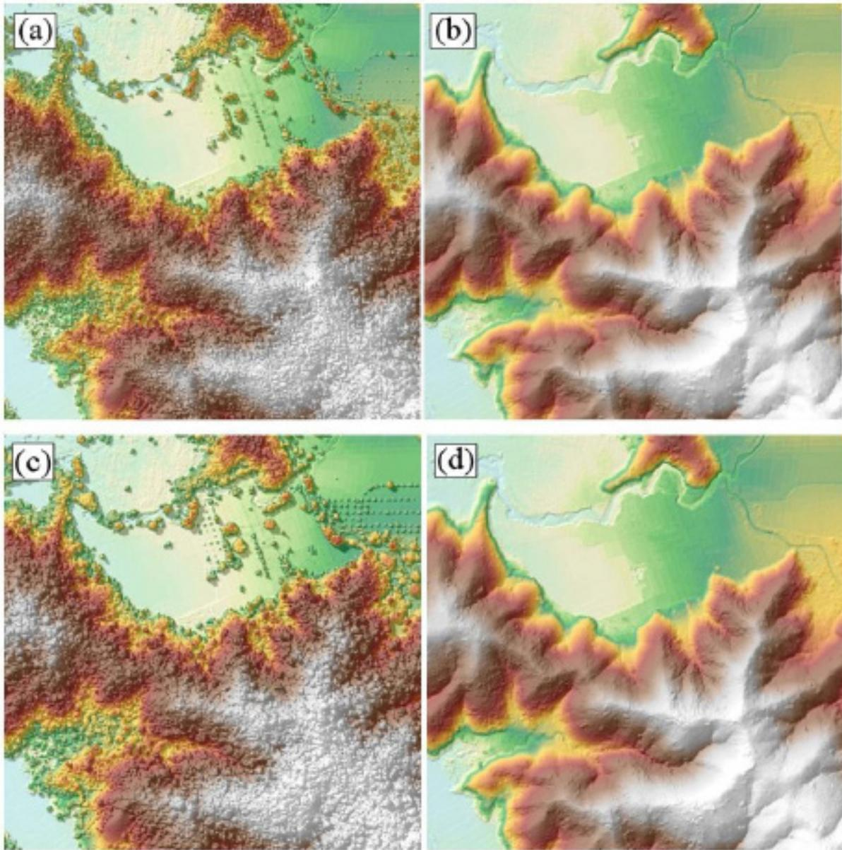
Figure 21. The production of last return DSM (a) and DTM (b), first return DSM (c) and secondary DTM (d) in some portion of Mamburao floodplain.
