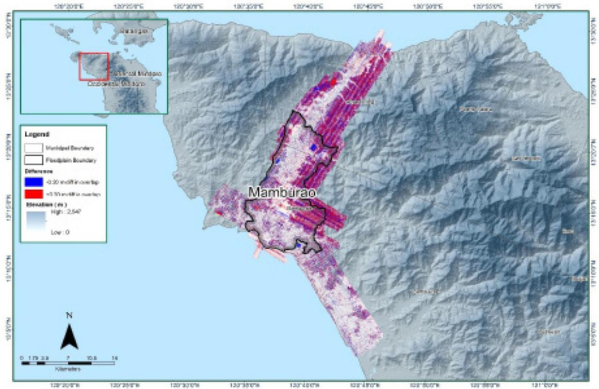
Figure 17. Elevation difference map between flight lines for Mamburao floodplain.
