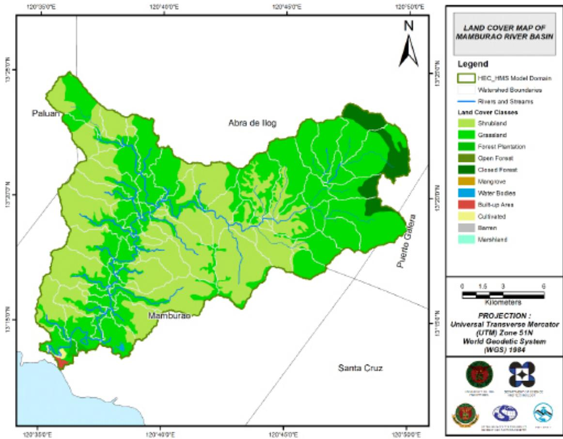
Figure 61. The land cover map of the Mamburao River Basin used for the estimation of the CN and watershed lag parameters of the rainfall-runoff model. (Source: NAMRIA)
