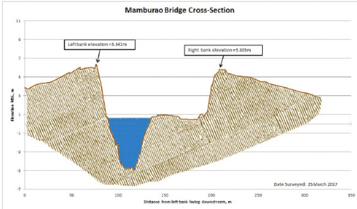
Figure 55. Cross-Section Plot of Mamburao Bridge
