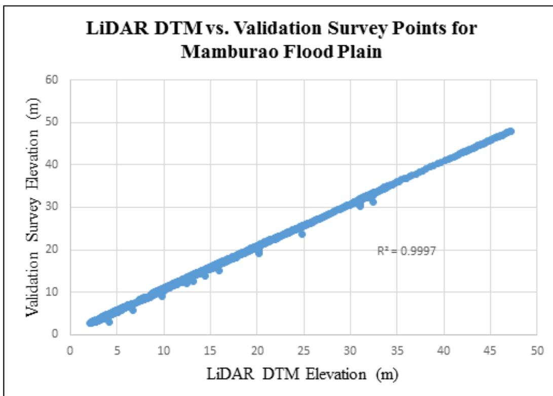
Figure 28. Correlation plot between validation survey points and LiDAR data.
