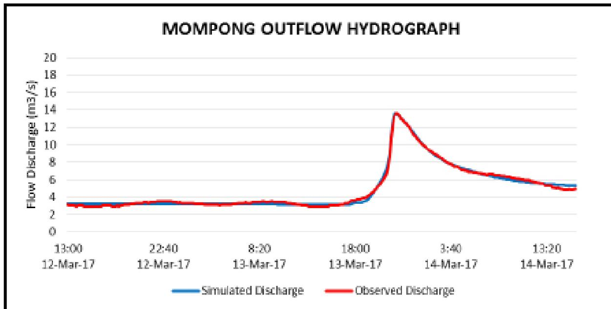
Figure 64. Outflow hydrograph of Mompong produced by the HEC-HMS model compared with observed outflow
