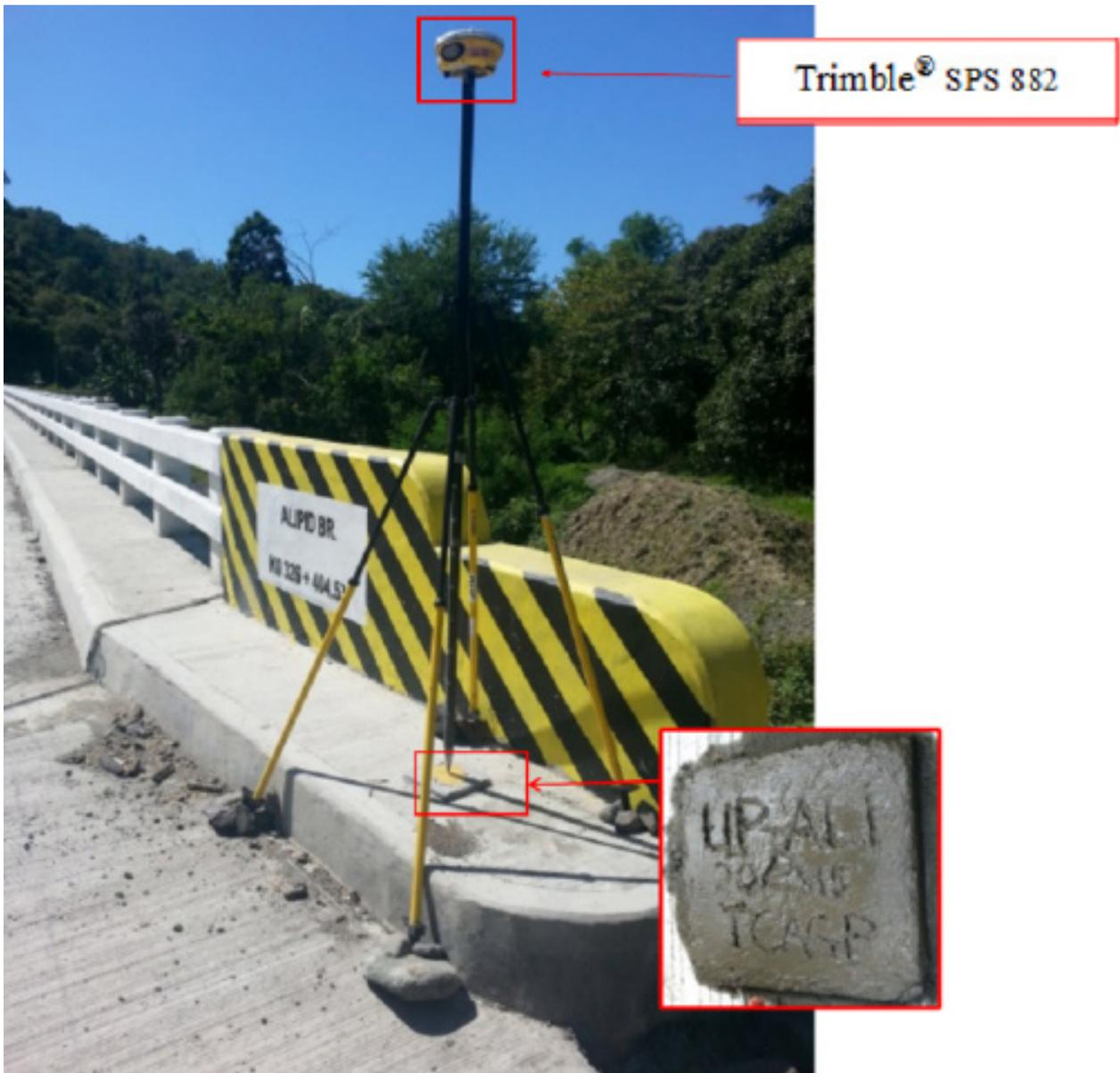
Figure 39. GNSS receiver set up, Trimble® SPS 882, at UP-ALI, Alipid Bridge approach in Brgy. Sto. Niño, Municipality of Sablayan, Occidental Mindoro
