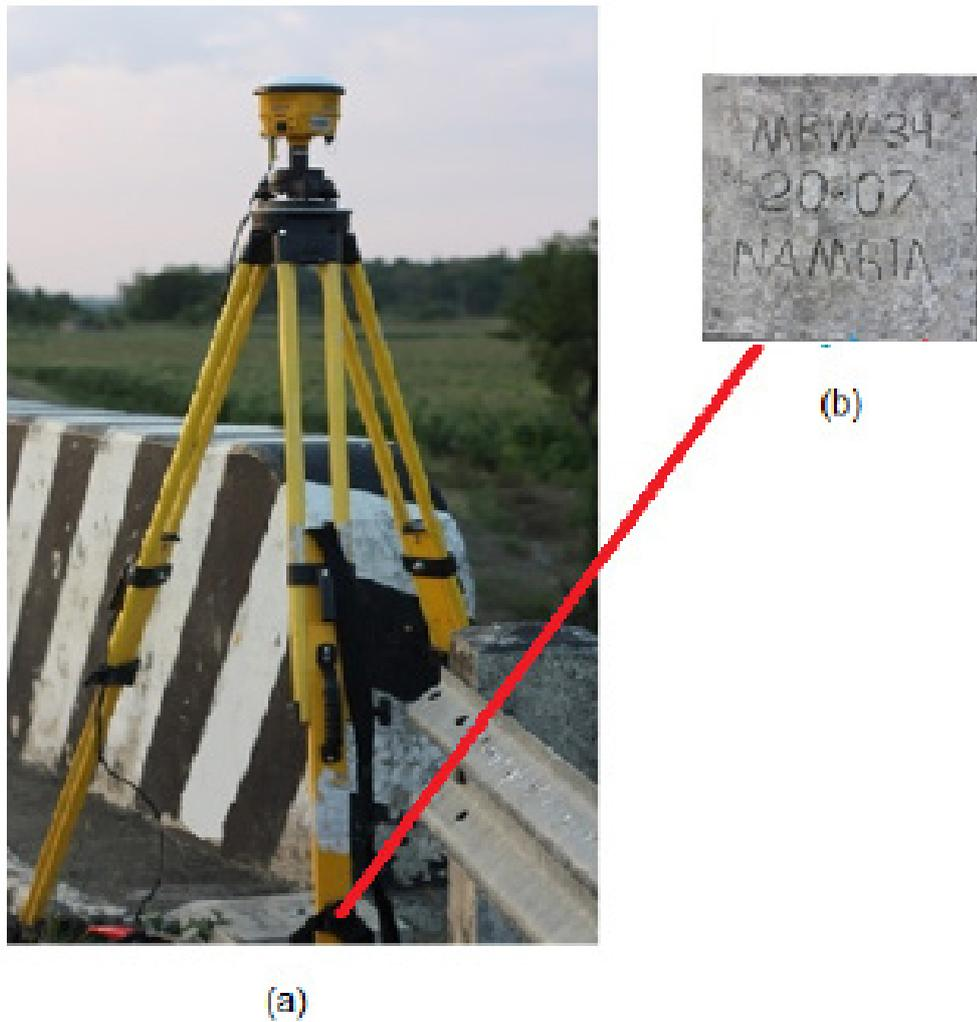
Figure 6. GPS set-up over MRW-34 in Balibago Bridge in Brgy. Armado, municipality of Abra de Ilog, Occidental Mindoro (a) and NAMRIA reference point MRW-34 (b) as recovered by the field team.
