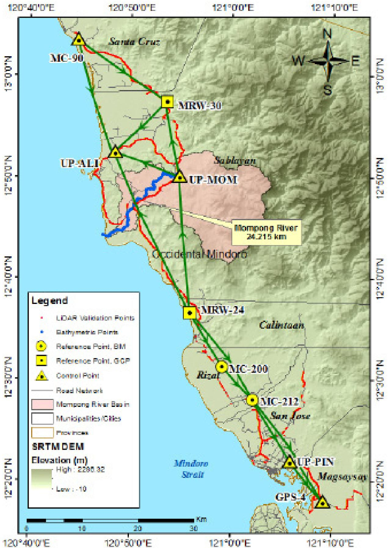
Figure 29. Extent of the bathymetric survey (in blue line) in Mompong River and the LiDAR data validation survey (in red).
