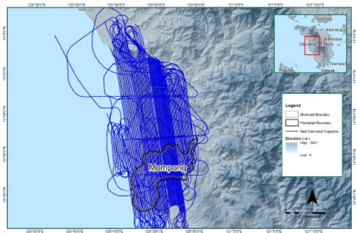
Figure 12. Best Estimated Trajectory of the LiDAR missions conducted over the Mompong Floodplain.
