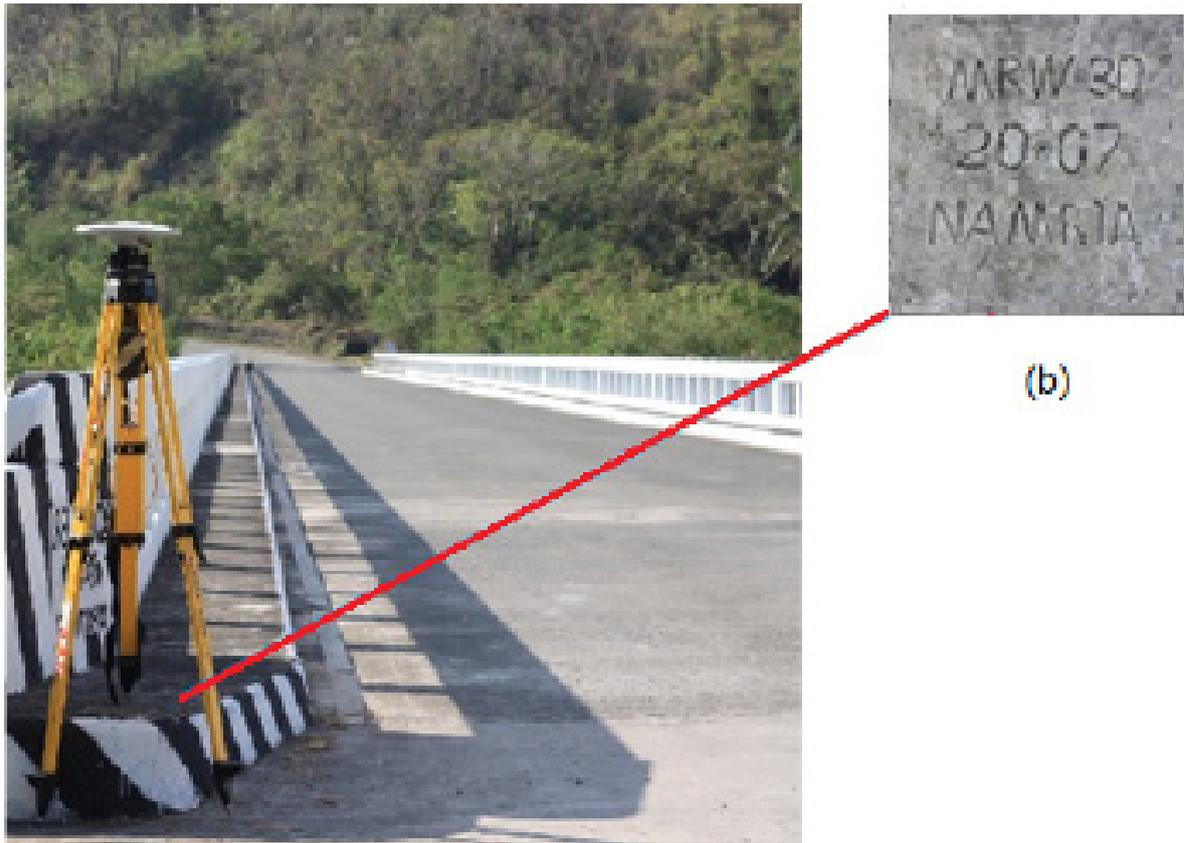
Figure 4. GPS set-up over MRW-30 at Amnay Bridge in Brgy. Pinagturilan, municipality of Sta. Cruz, Occidental Mindoro (a) and NAMRIA reference point MRW-30 (b) as recovered by the field team.
