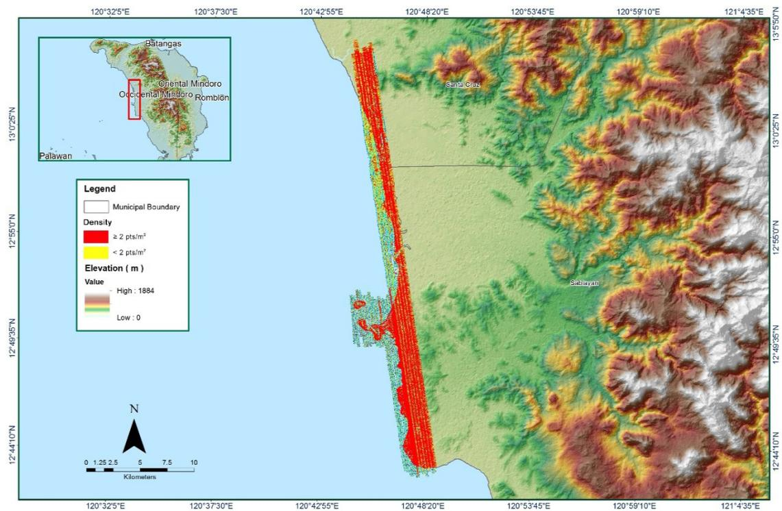
Figure A-8.6 Density of merged LiDAR data
