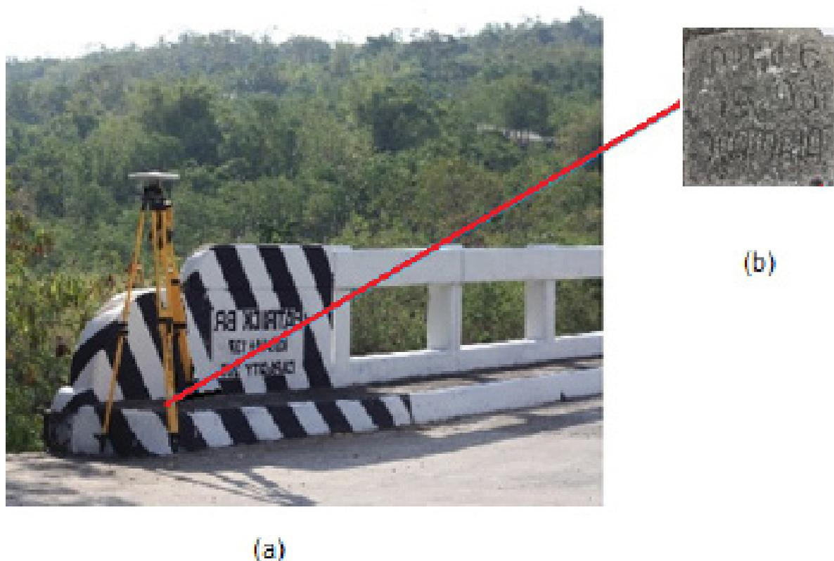
Figure 3. GPS set-up over MRW-6 at Patrick Bridge in Brgy. Yabang, municipality of Sablayan, Occidental Mindoro (a) and NAMRIA reference point MRW-6 (b) as recovered by the field team.
