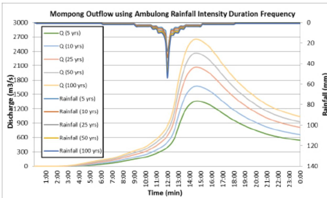
Figure 65. Outflow hydrograph at Mompong Station generated using Ambulong RIDF simulated in HEC-HMS
