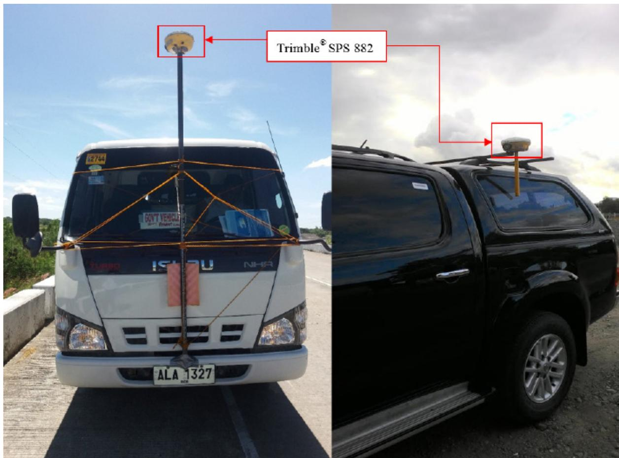
Figure 45. Validation points acquisition survey set up along Mompong River Basin
