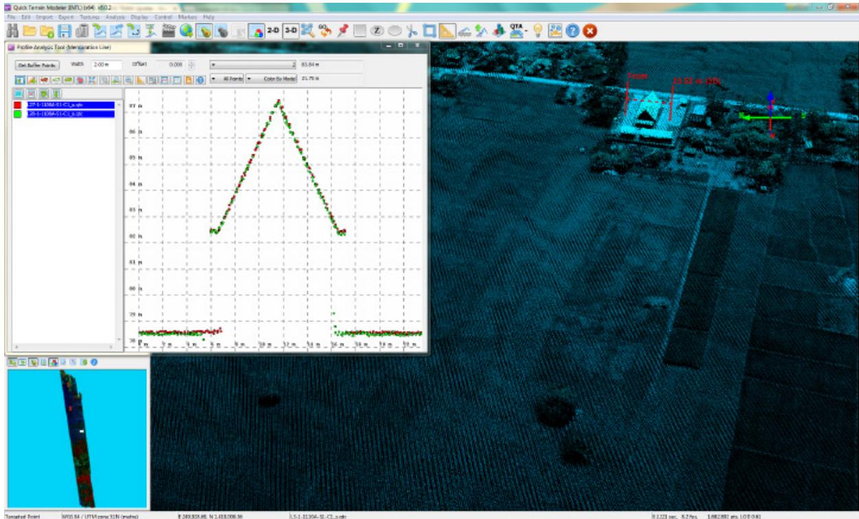
Figure 17. Quality checking for a Mompong flight 1110A using the Profile Tool of QT Modeler.
