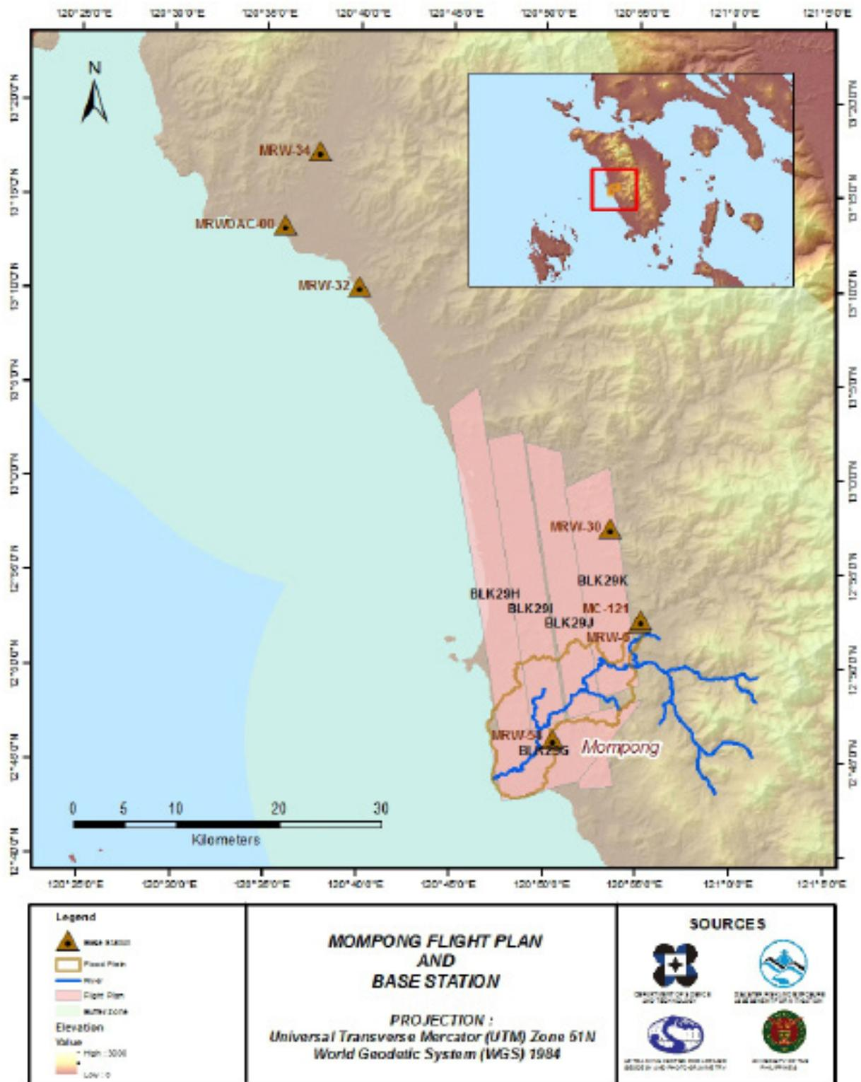
Figure 2. Flight Plan and base stations used for the Mompong Floodplain survey.
