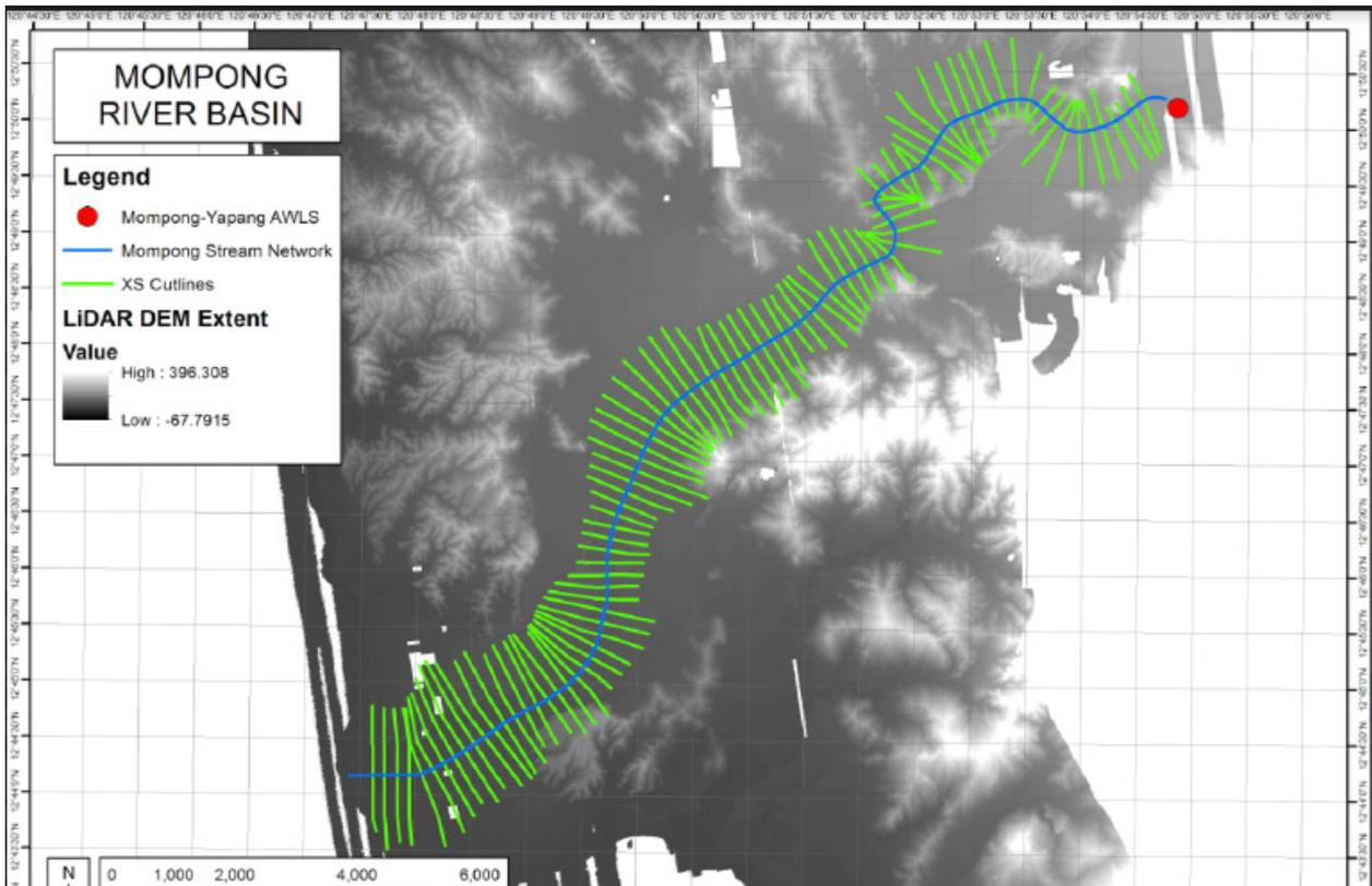
Figure 62. River cross-section of Mompong River generated through Arcmap HEC GeoRAS tool
