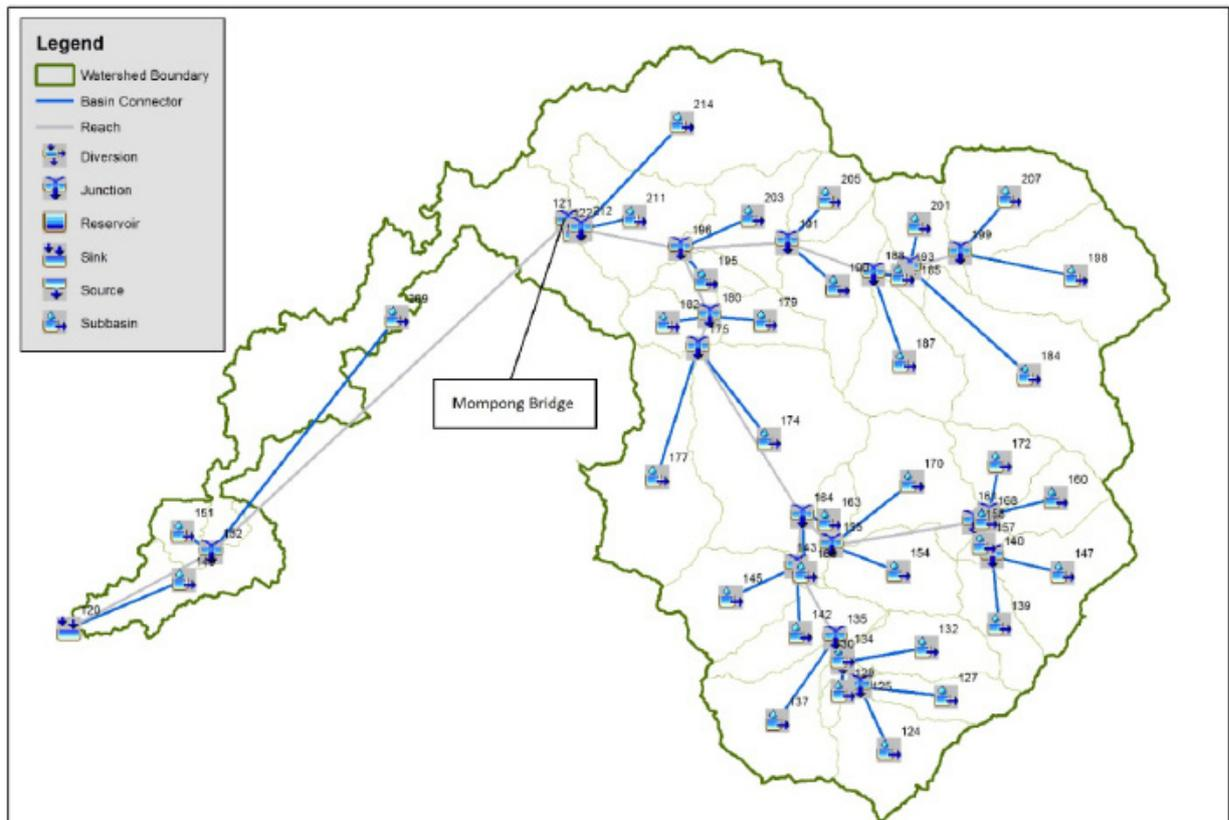
Figure 61. HEC-HMS generated Mompong River Basin Model.
