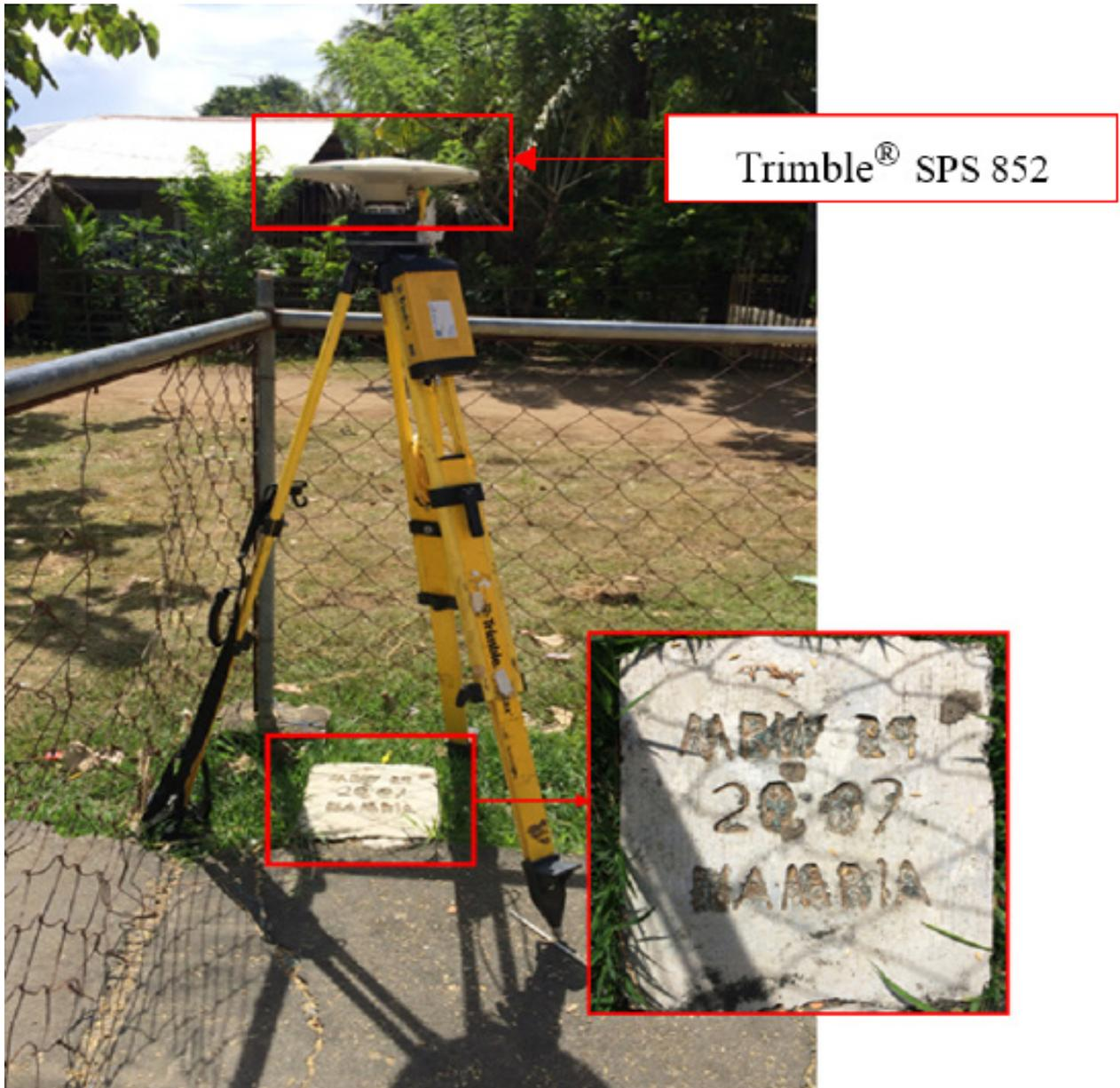
Figure 31. GNSS receiver set-up, Trimble® SPS 852, at MRW-24 in front of Iriron Elementary School in Brgy. Iriron, Municipality of Calintaan, Occidental Mindoro
