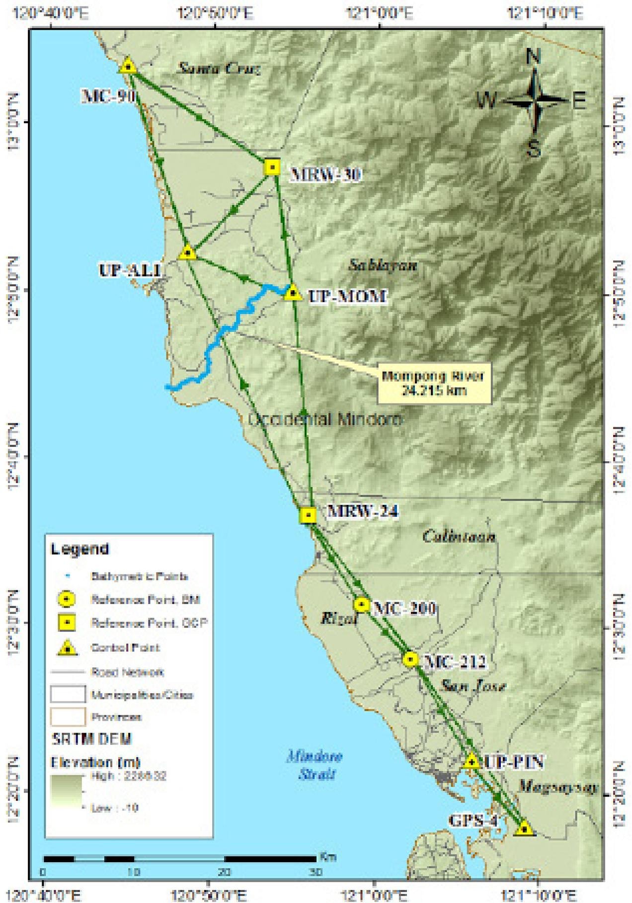
Figure 30. The GNS Network established in the Panplona River Survey.
