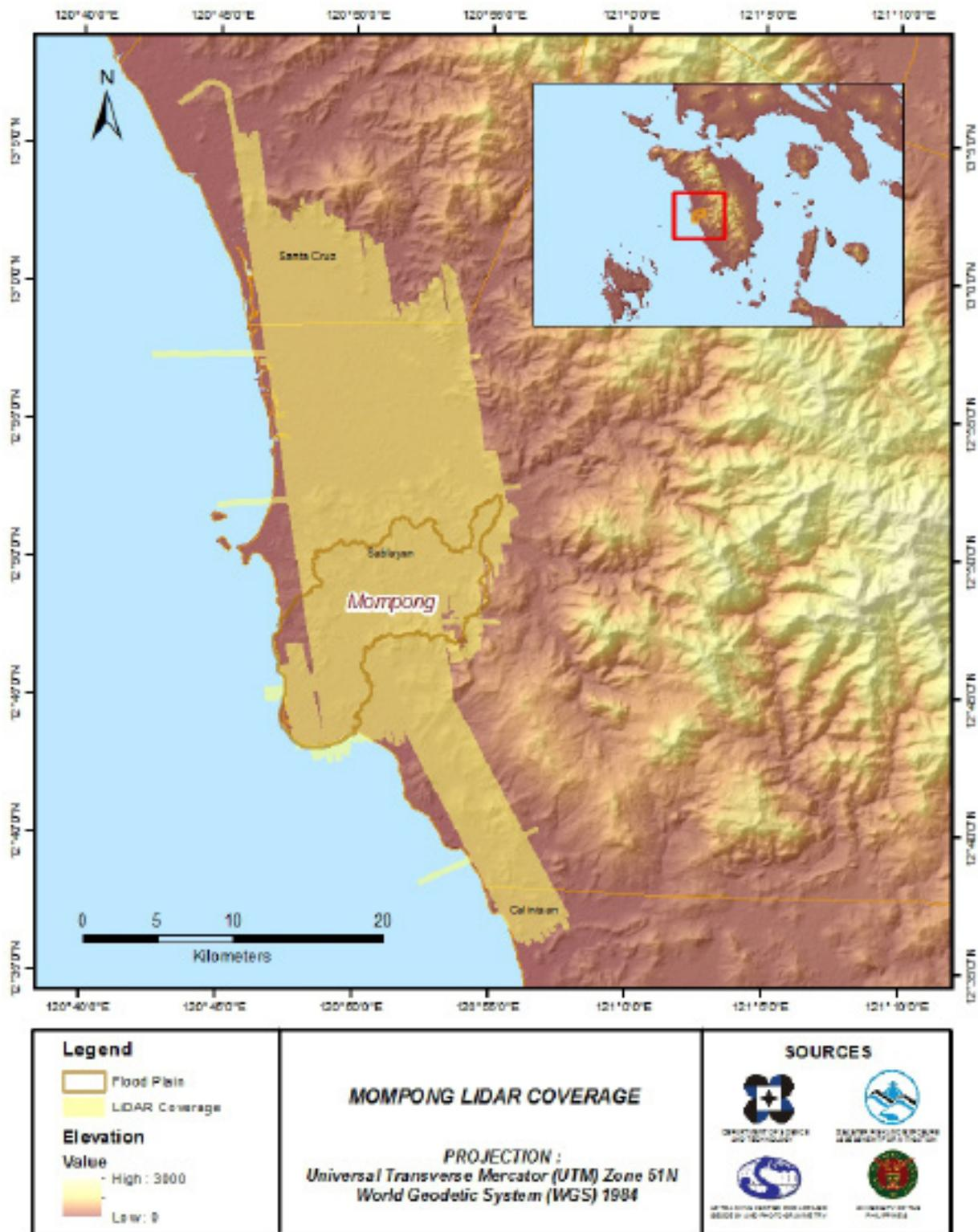
Figure 8. Actual LiDAR survey coverage of the Mompong Floodplain.
