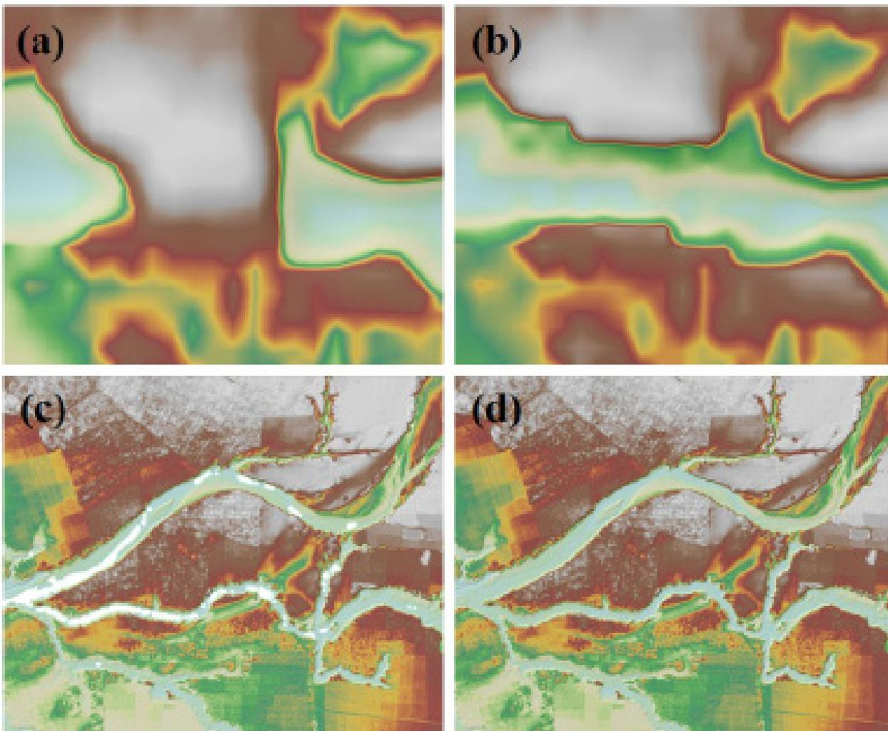
Figure 23. Portions in the DTM of Mompong Floodplain – a land bridge before (a) and after (b) interpolation process and part of the river with data gap before (c) and after (d) filling data gap.
