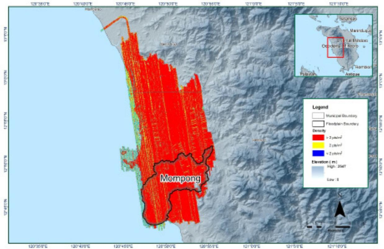
Figure 15. Pulse density map of merged LiDAR data for Mompong Floodplain.
