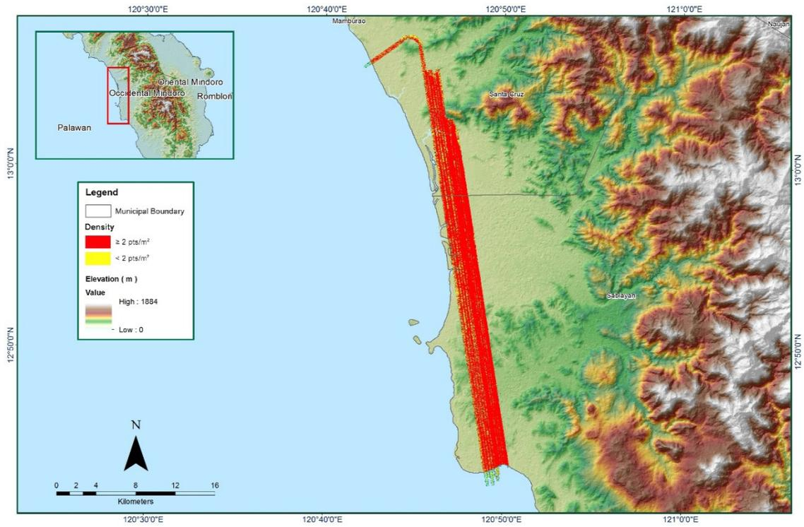
Figure A-8.13. Density of merged LiDAR data
