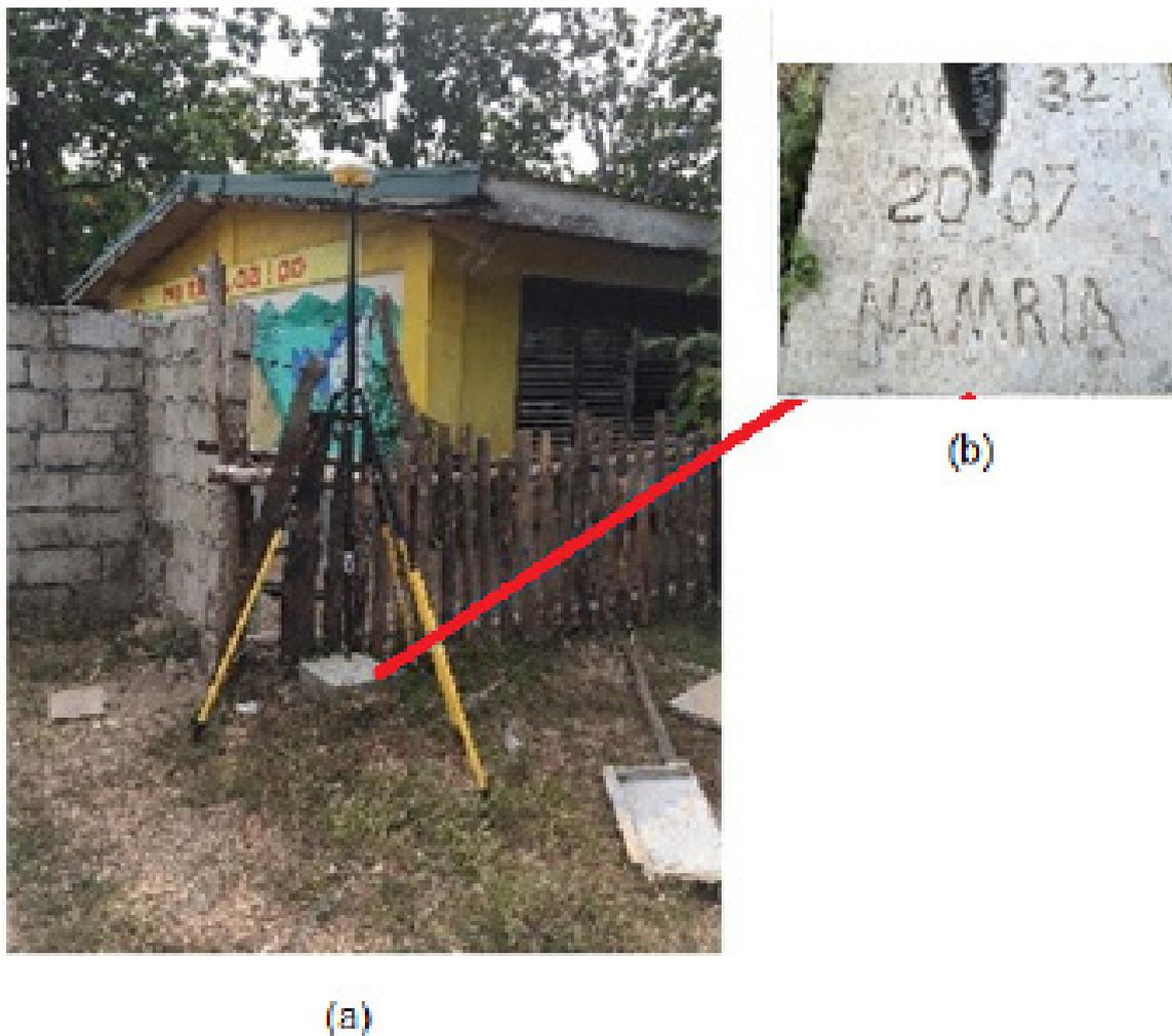
Figure 5. GPS set-up over MRW-32 at the corner of a day care center in Brgy. Fatima, municipality of Mamburao, Occidental Mindoro (a) and NAMRIA reference point MRW-32 (b) as recovered by the field team.
