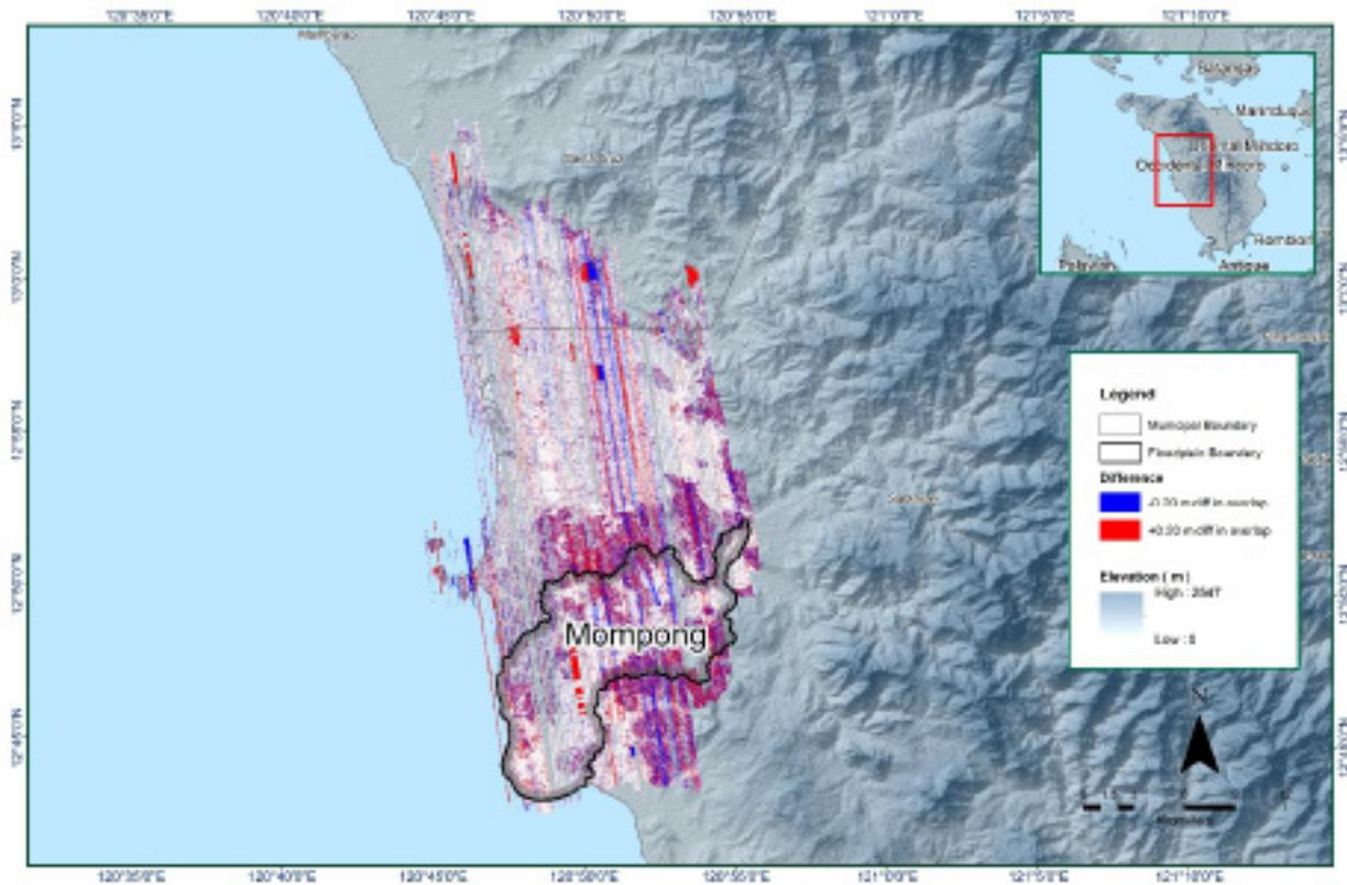
Figure 16. Elevation Difference Map between flight lines for Mompong Floodplain Survey.
