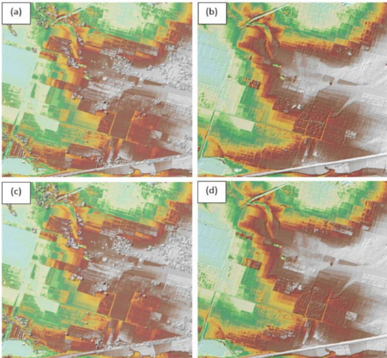
Figure 20. The production of last return DSM (a) and DTM (b), first return DSM (c) and secondary DTM (d) in some portion of Mompong Floodplain.
