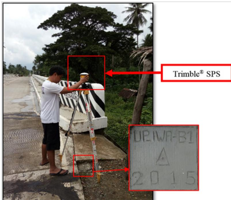
Figure 32. GNSS receiver set up, Trimble® SPS 985, at UP\_IWA-1, located at the approach of Iwahig Bridge in Brgy. Iwahig, Bataraza, Province of Palawan.
