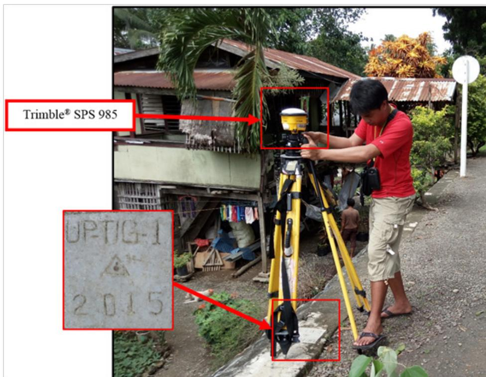
Figure 34. GNSS receiver set up, Trimble® SPS 985, at UP\_PAN-1, located on the approach of Tigaplan Bridge in Brgy. Barong-Barong, Brooke's Point, Province of Palawan.
