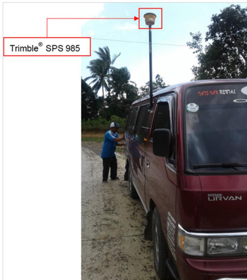
Figure 41. Validation points acquisition survey set-up for Ocayan River.
