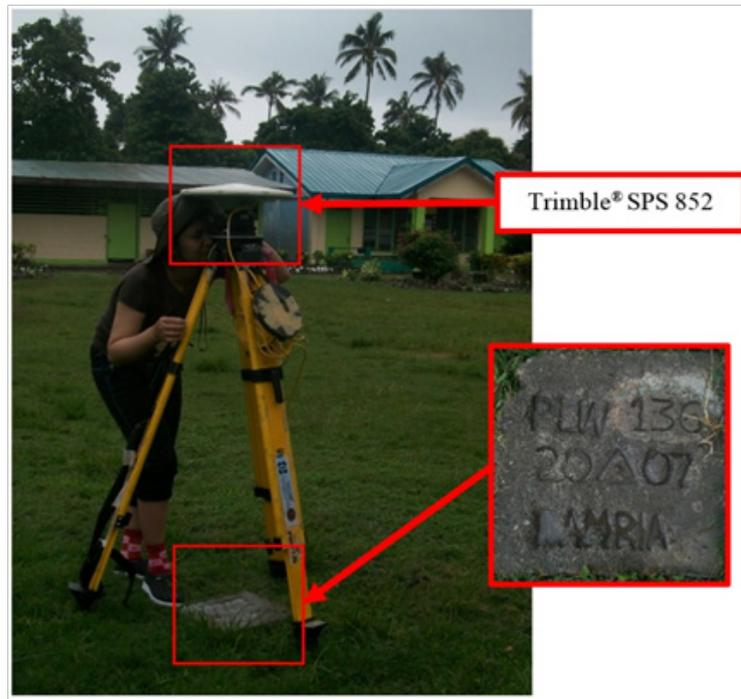
Figure 31. GNSS receiver set up, Trimble® SPS 882, at PLW-136, located at the Malis Elementary School compound, Brgy. Malis, Brooke's Point, Province of Palawan
