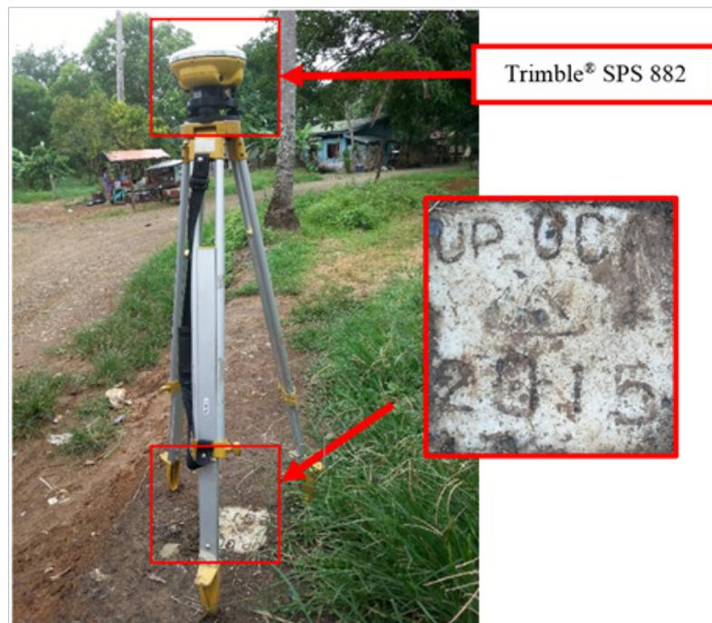
Figure 33. GNSS base set up, Trimble® SPS 882, at UP\_OCA-0, located about 23 m from Elementary School near Ocayan River in Brgy. Rio Tuba, Bataraza, Province of Palawan.
