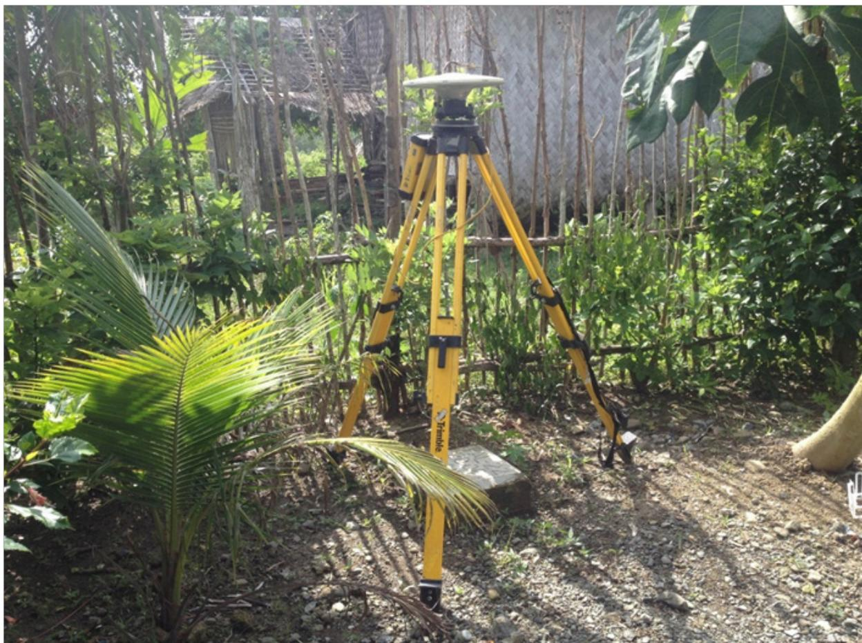
Figure 4. GPS set-up over PLW-79 (PAL-22) along the barangay road of Brgy. Sandoval near the house of Tribal Chieftain Acat in the Municipality of Bataraza.
