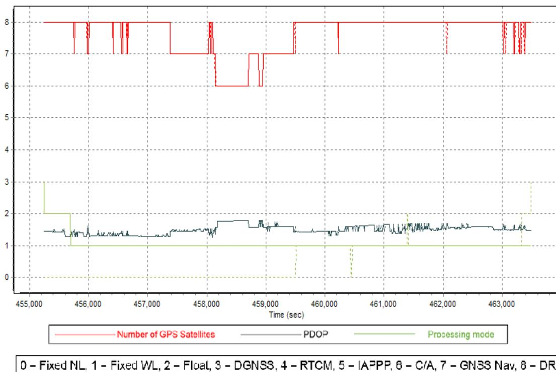
Figure 13. Solution Status Parameters of Paliwan Flight 2593P.
