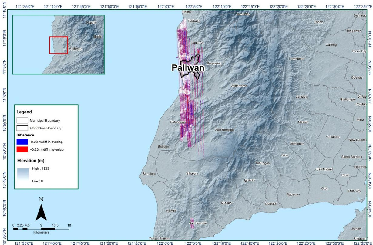
Figure 18. Elevation difference map between flight lines for Paliwan floodplain.
