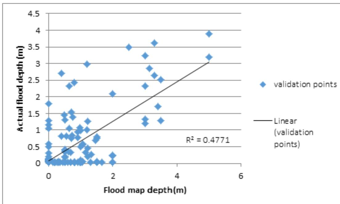
Figure 80. Flood depth map vs Actual flood depth
