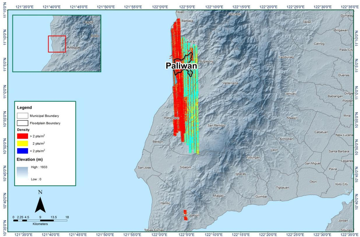
Figure 17. Density map of merged LiDAR data for Paliwan floodplain.
