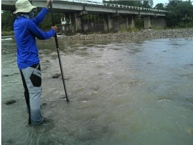
Figure 38. Cross section survey in Paliwan Bridge, Municipality of Bugasong
