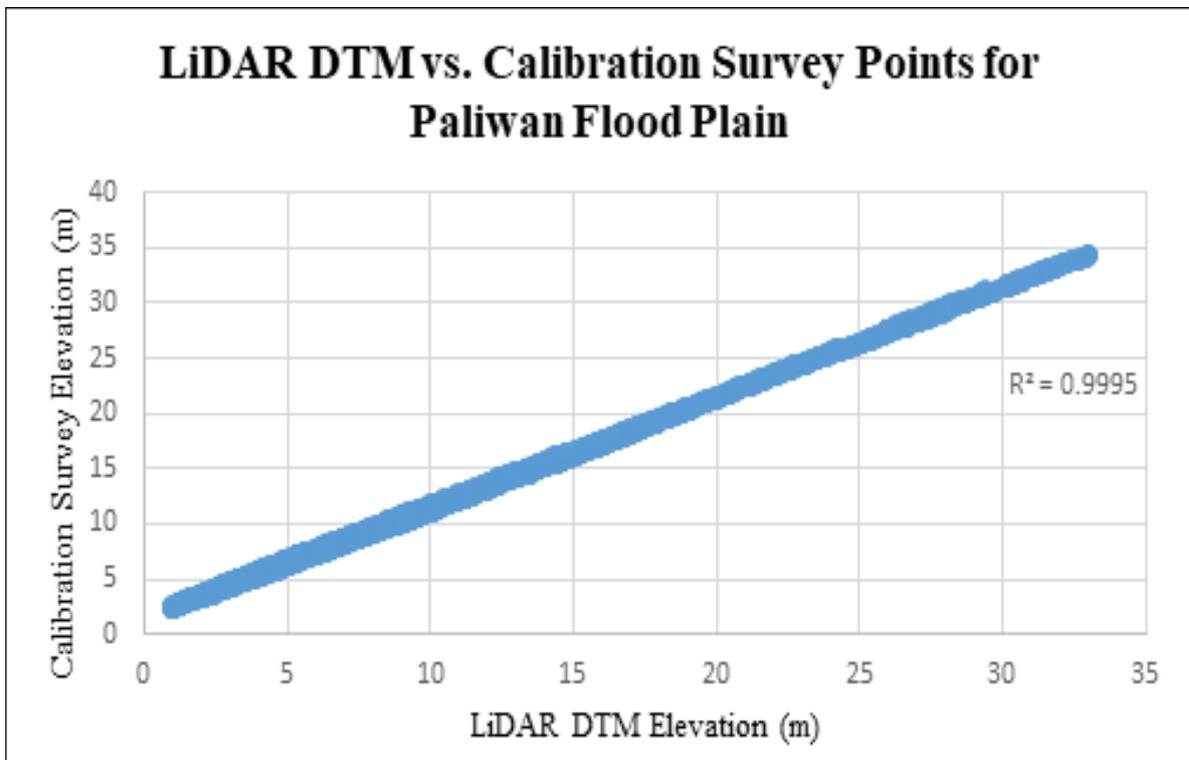
Figure 28. Correlation plot between calibration survey points and LiDAR data.
