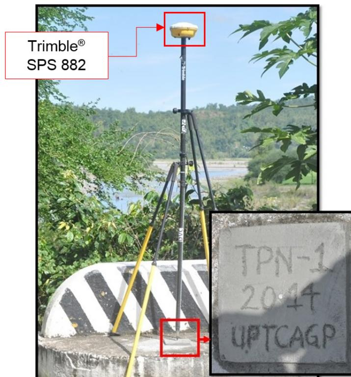
Figure 37. UP-TCAGP established control point, TPN-1, with Trimble® SPS 882 on Tipuluan Bridge in Brgy. Pasong, Municipality of Sibalom, Antique
