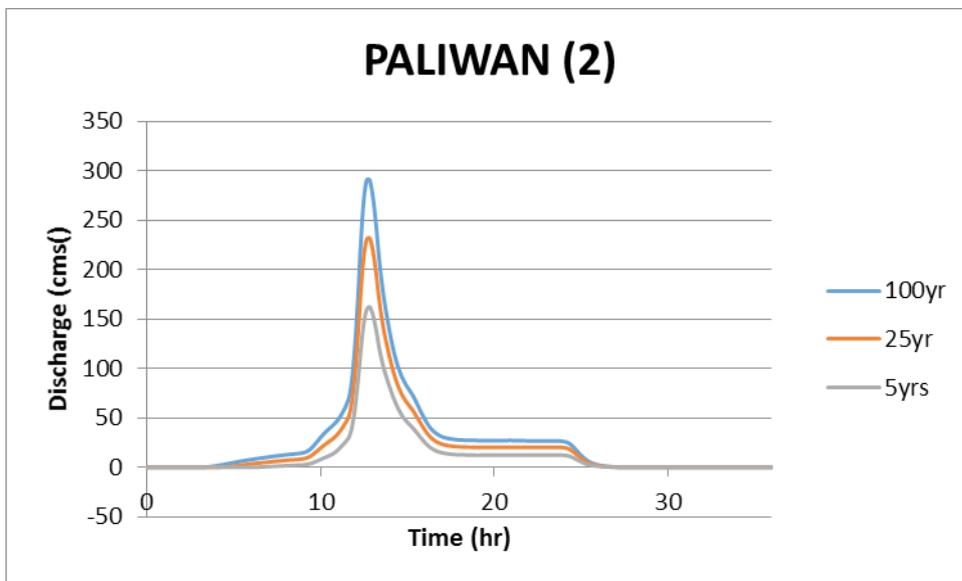
Figure 65. Paliwan river (2) generated discharge using 5-, 25-, and 100-year Iloilo rainfall intensity-duration-frequency (RIDF) in HEC-HMS
