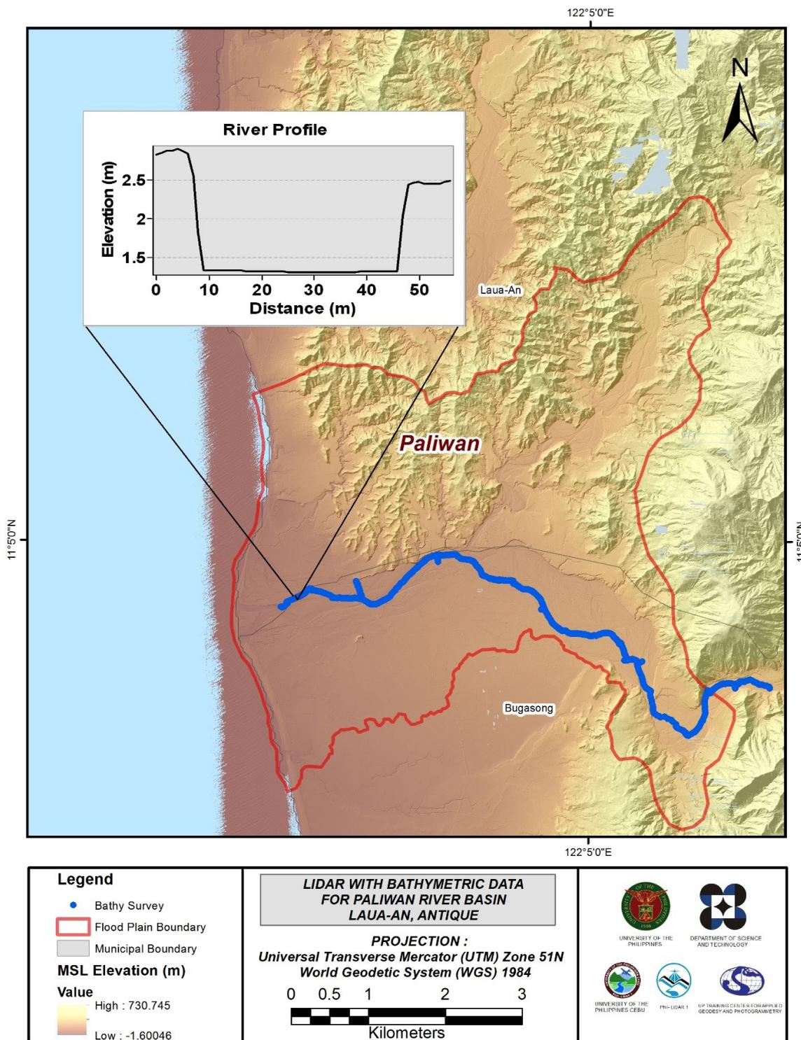
Figure 30. Map of Paliwan Flood Plain with bathymetric survey points shown in blue.
