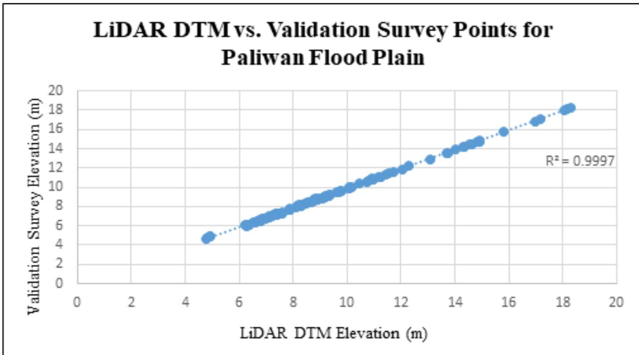
Figure 29. Correlation plot between validation survey points and LiDAR data.
