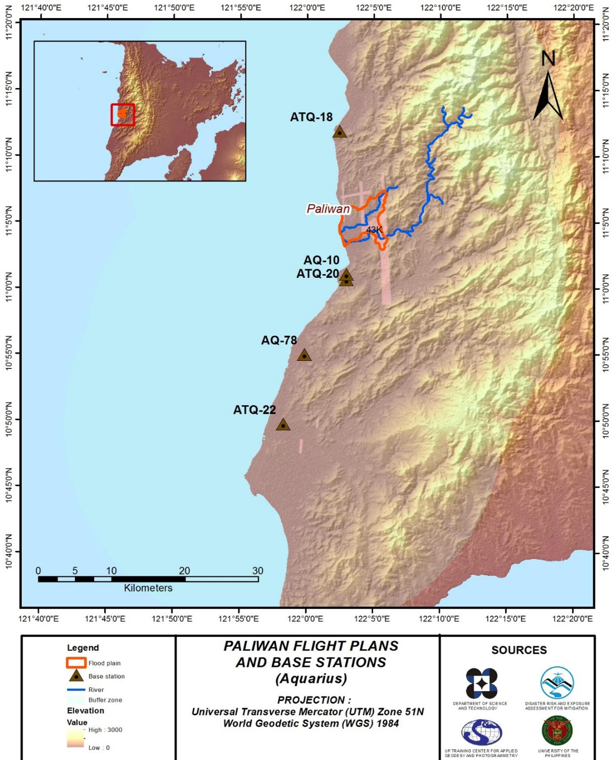
Figure 4. Flight plan and base stations using the Aquarius system to cover Paliwan Floodplain.
