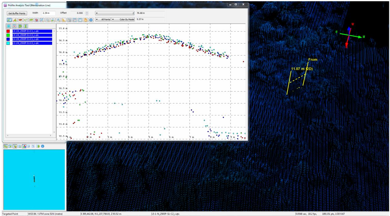
Figure 19. Quality checking for Paliwan flight 2593P using the Profile Tool of QT Modeler.
