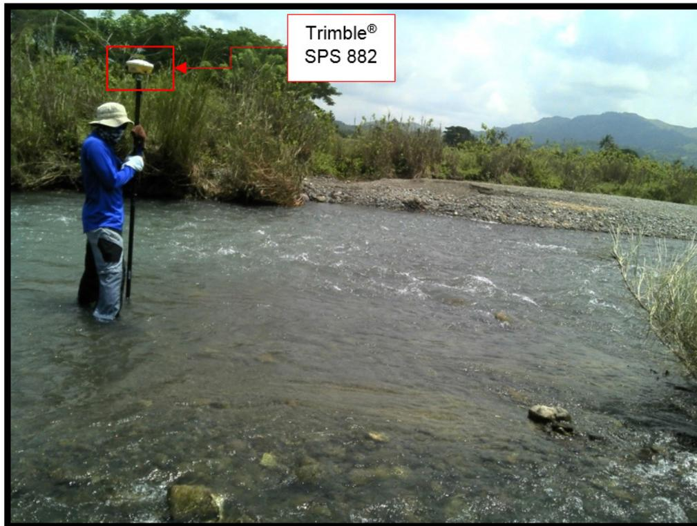
Figure 44. Bathymetric survey using a Trimble® SPS 882 in GNSS PPK in Paliwan River
