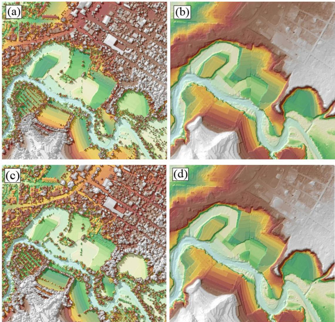
Figure 22. The production of last return DSM (a) and DTM (b), first return DSM (c) and secondary DTM (d) in some portion of Paliwan floodplain.
