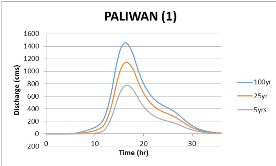
Figure 64. Paliwan river (1) generated discharge using 5-, 25-, and 100-year Iloilo rainfall intensity-duration-frequency (RIDF) in HEC-HMS
