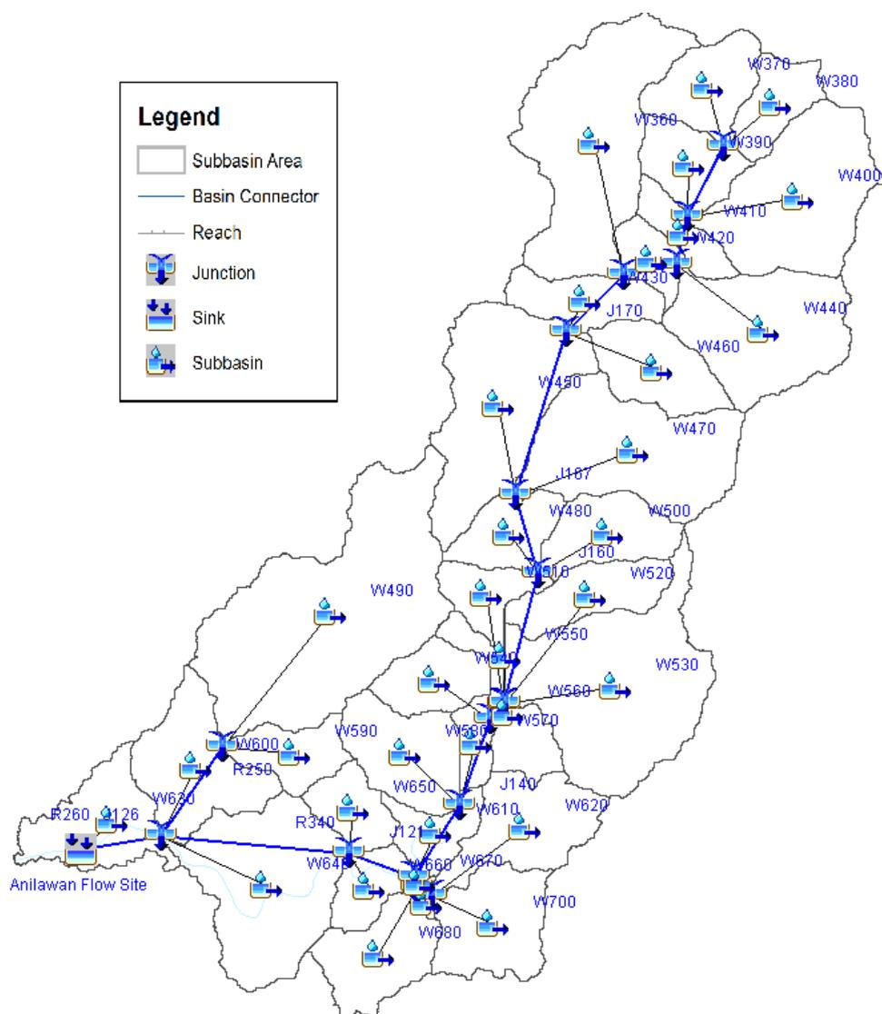
Figure 57. The Paliwan Hydrologic Model generated in HEC-HMS
