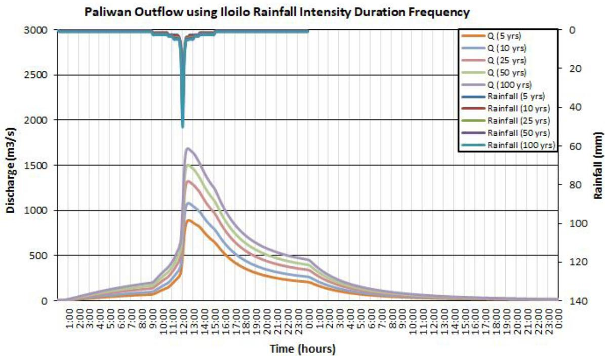
Figure 63. Outflow hydrograph at Paliwan Station generated using Iloilo RIDF simulated in HEC-HMS
