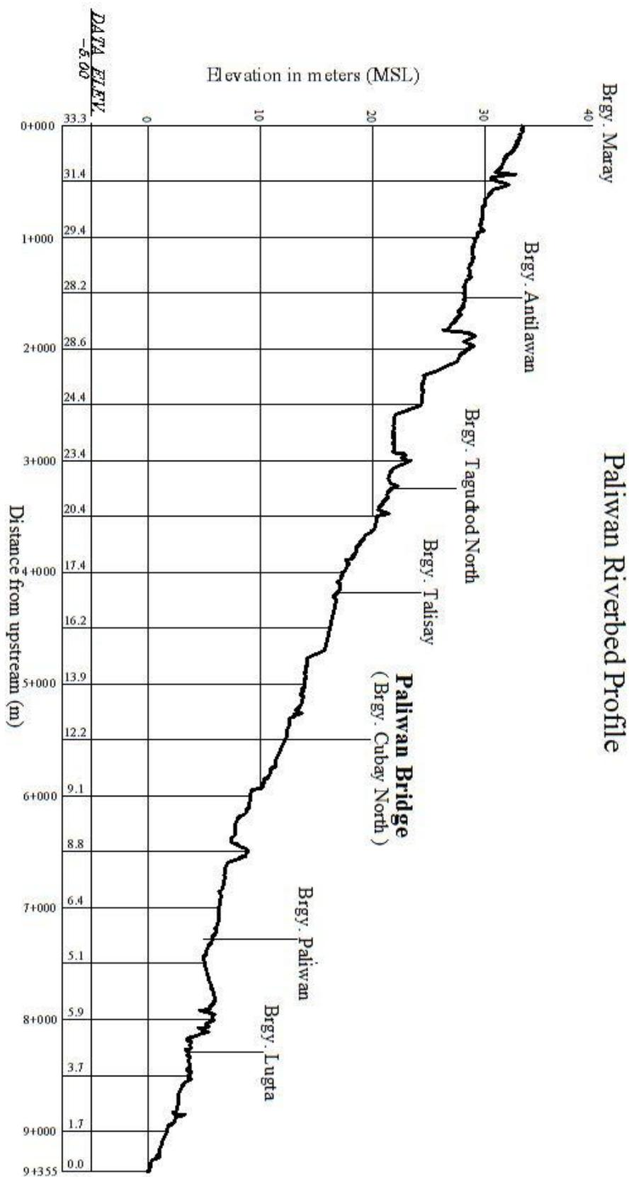
Figure 46. The Paliwan Riverbed Profile from Brgy. Maray, Municipality of Bugasong down to Brgy. Lugta, Municipality of Bugasong
