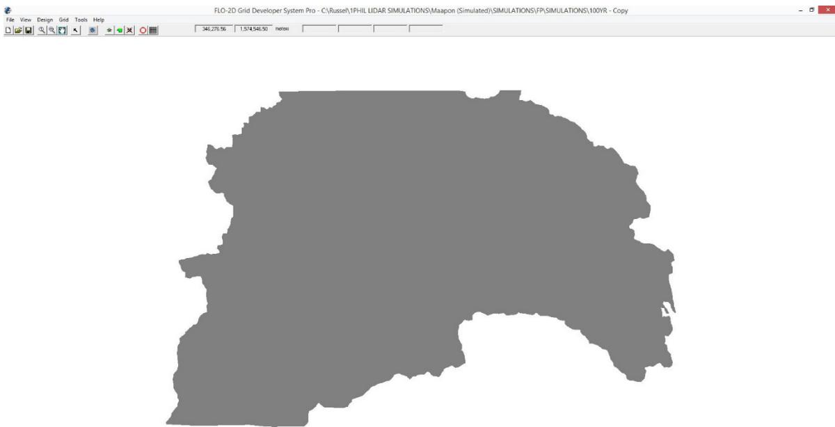
Figure 59. A screenshot of the river sub-catchment with the computational area to be modeled in FLO-2D Grid Development System Pro (FLO-@D GDS Pro)
