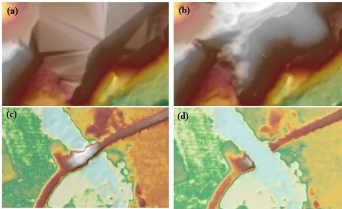
Figure 25. Portions in the DTM of Paliwan floodplain – a paddy field before (a) and after (b) data retrieval; bridge before (c) and after (d) manual editing
