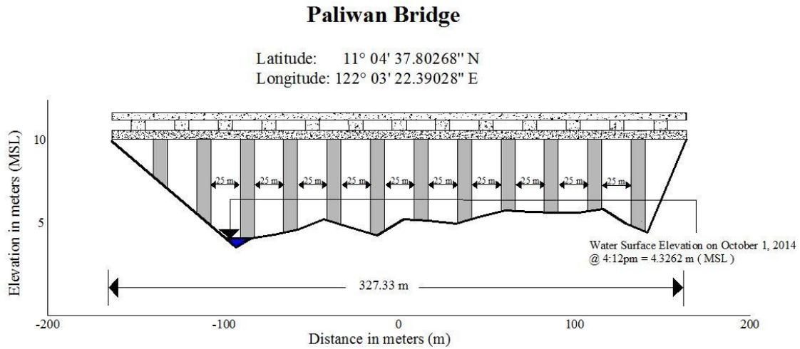
Figure 39. Paliwan Bridge cross-section survey drawn to scale
