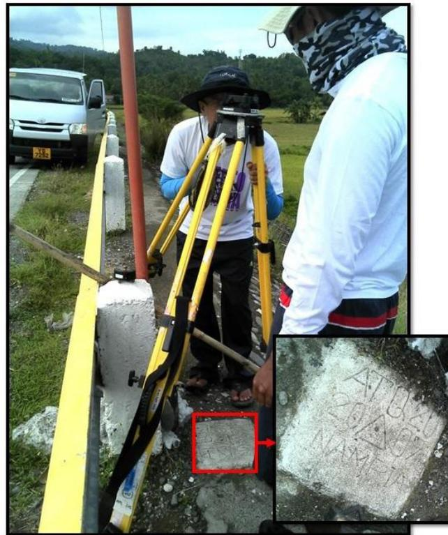
Figure 35. GNSS base receiver setup, Trimble® SPS 852 at ATQ-20 in Brgy. Zaragoza, Municipality of Bugasong, Antique
