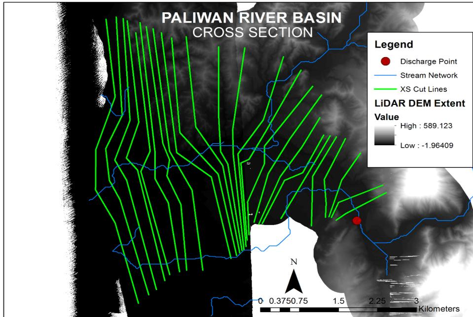
Figure 58. River cross-section of Paliwan River through Arcmap HEC GeoRAS tool
