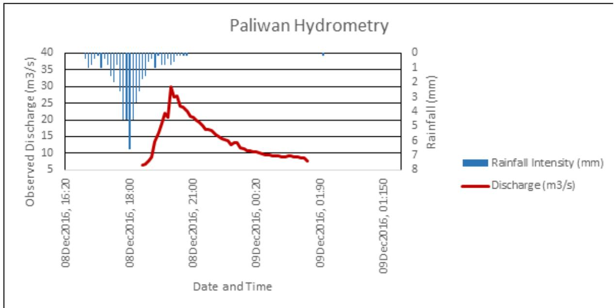
Figure 50. Rainfall and outflow data of the Paliwan River Basin, which was used for modeling
