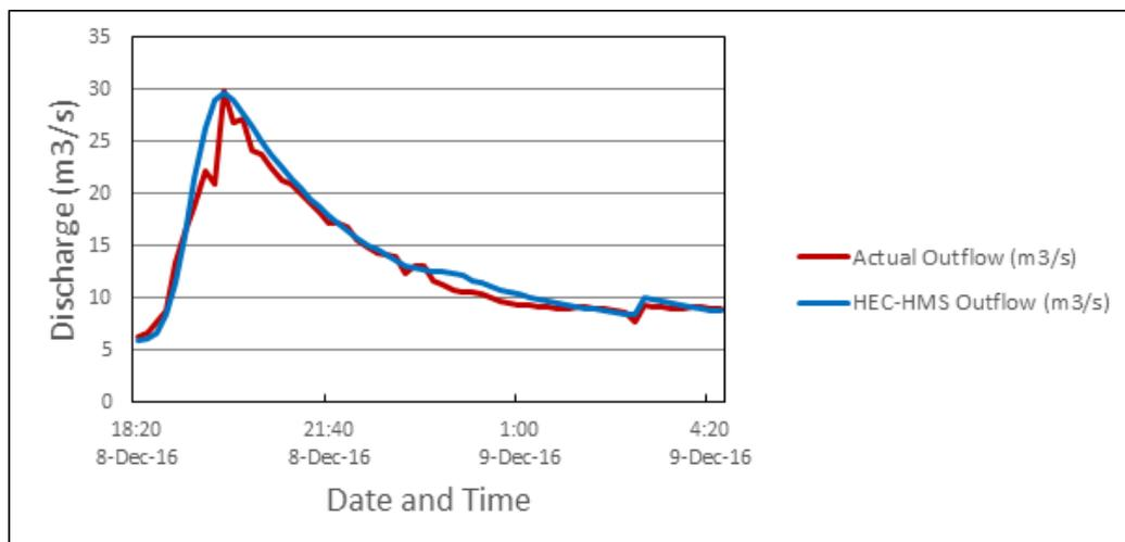
Figure 62. Outflow hydrograph of Paliwan produced by the HEC-HMS model compared with observed outflow
