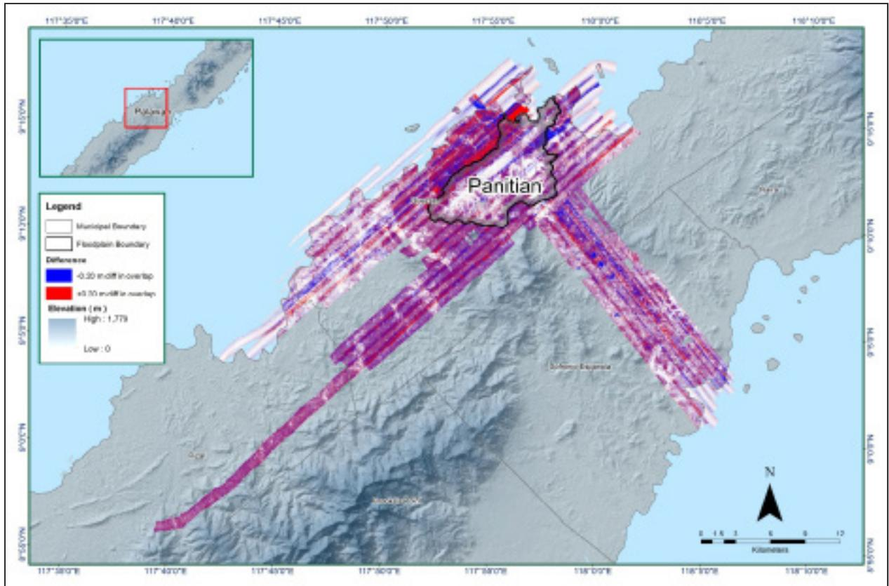
Figure 15. Elevation difference map between flight lines for Panitian Floodplain.
