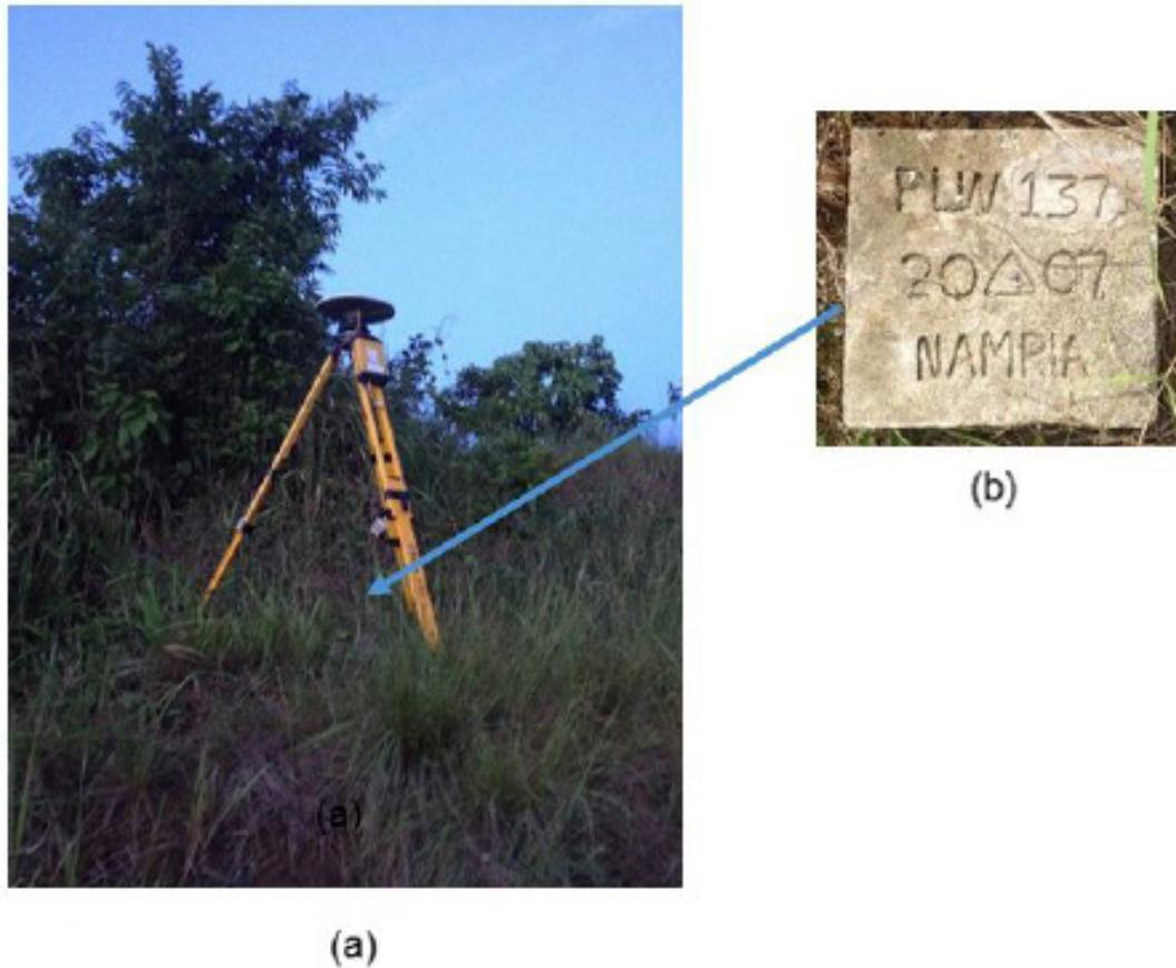
Figure 3. GPS set-up over PLW-137 as recovered at the top of the ridge along national highway in Brgy. Ipilán, Quezon, Palawan (a) and NAMRIA reference point PLW-137 (b) as recovered by the field team.
