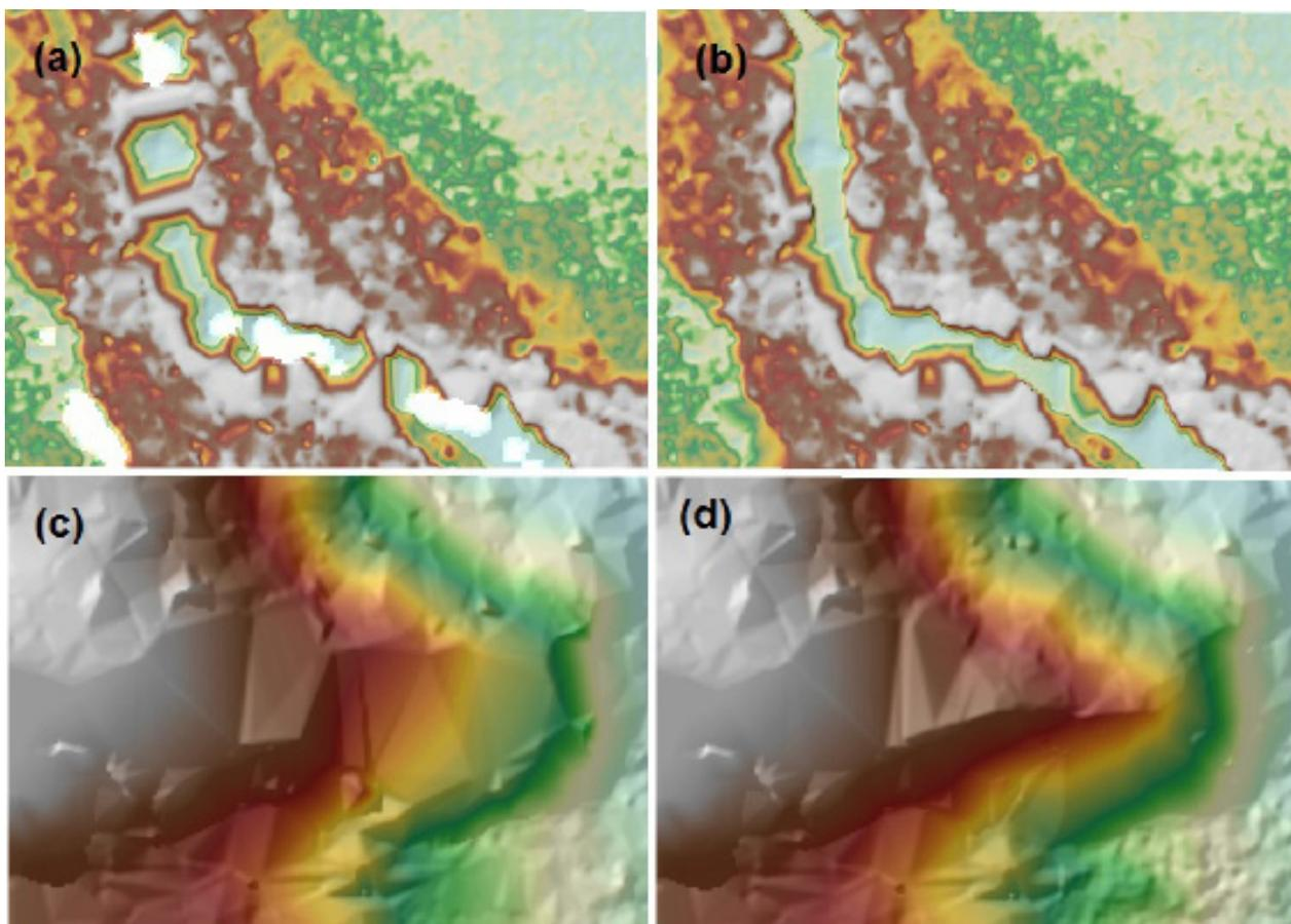
Figure 20. Portions in the DTM of Panitian Floodplain – a paddy field before (a) and after (b) data retrieval; a bridge before (c) and after manual editing (d).
