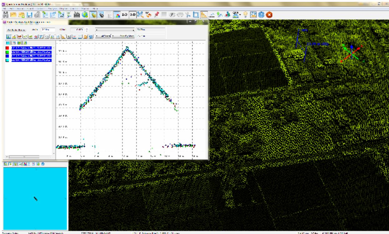
Figure 16. Quality checking for Panitian flight 3165P using the Profile Tool of QT Modeler.
