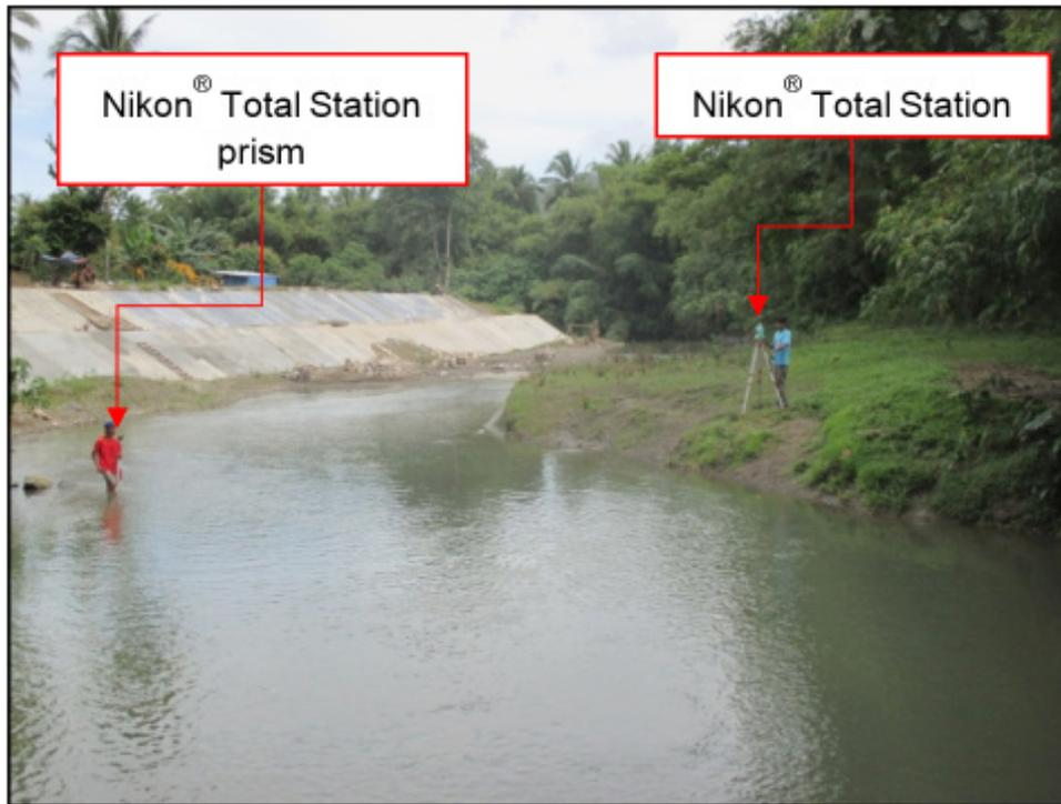
Figure 43. Manual bathymetric survey of ABSD at Panitian River using Nikon® Total Station
