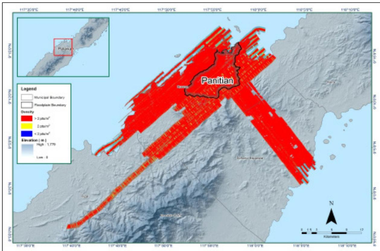
Figure 14. Pulse density map of merged LiDAR data for Panitian Floodplain.
