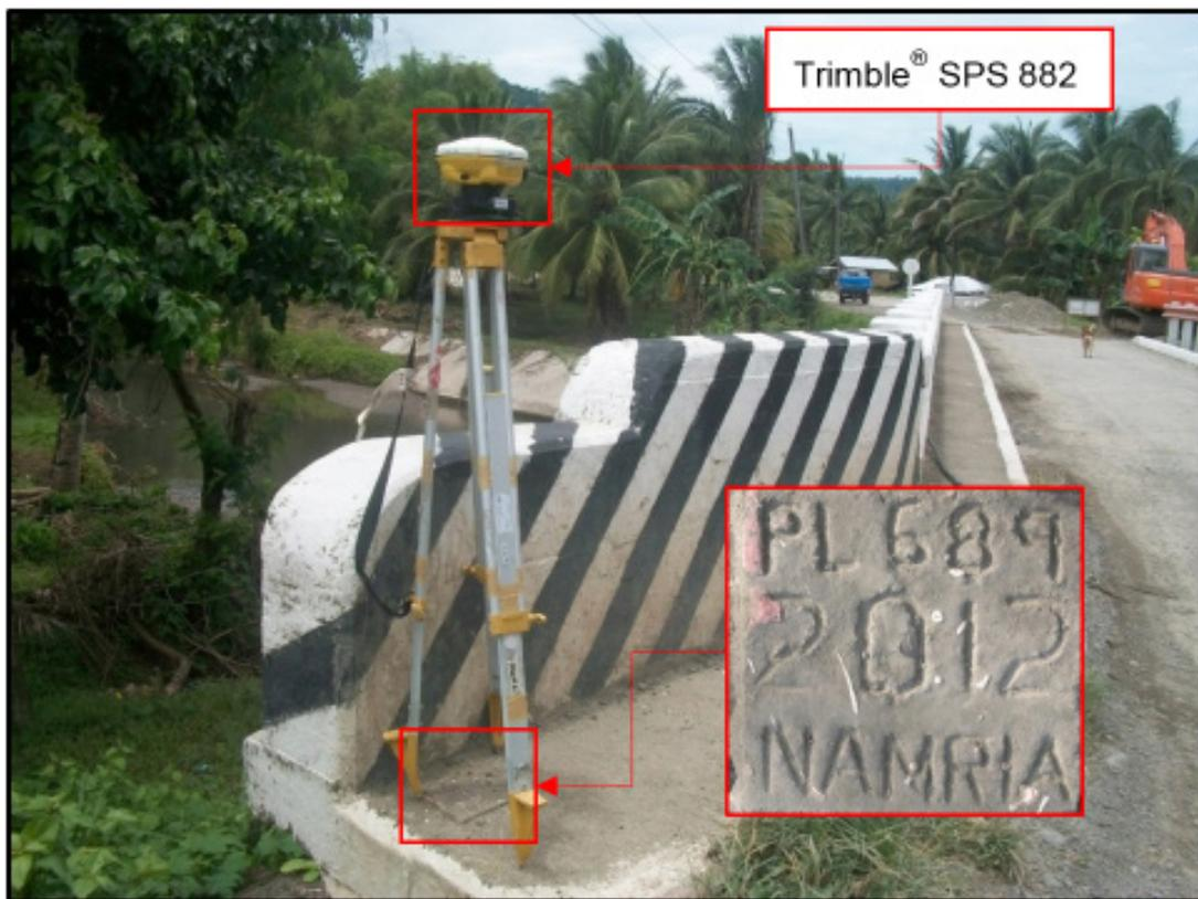
Figure 29. GNSS receiver set up, Trimble® SPS 882, at PL-689, located at the approach of Malatgao Bridge in Brgy. Sowangan, Quezon, Province of Palawan
