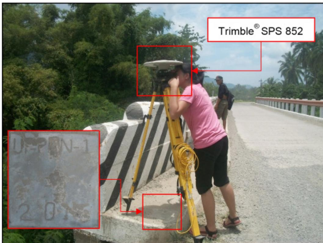
Figure 31. GNSS receiver set up, Trimble® SPS 985, at UP\_PAN-1, located on the approach of Panitian Bridge in Brgy. Malatgao, Quezon, Province of Palawan
