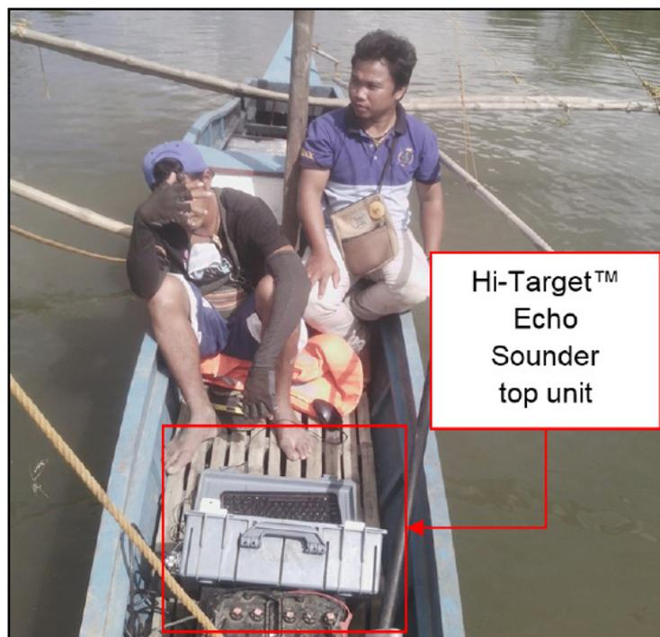
Figure 42. Bathymetric survey of ABSD at Panitian River using a Hi-Target™ Echo Sounder
