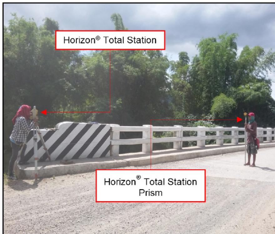
Figure 34. As-built survey of Panitian Bridge
