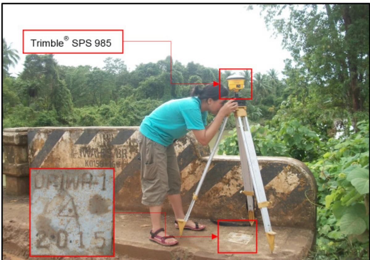
Figure 30. GNSS receiver set up, Trimble® SPS 985, at UP\_IWA-1, located at the approach of Iwahig Bridge in Brgy. Maasin, Quezon, Province of Palawan
