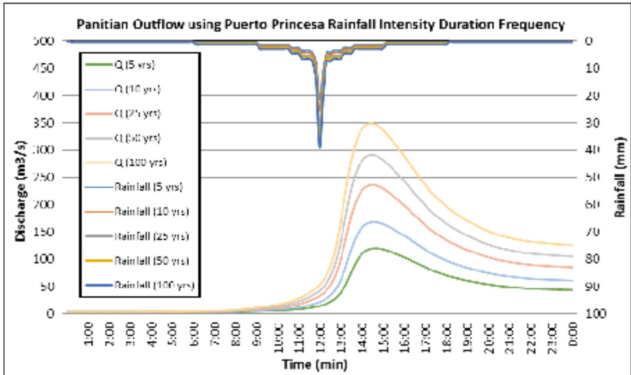
Figure 62. Outflow hydrograph at Panitian Station generated using Puerto Princesa RIDF simulated in HEC-HMS
