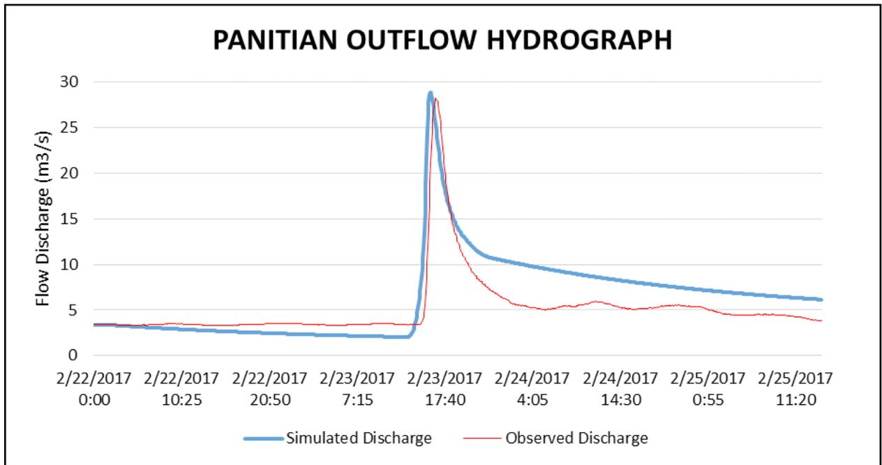
Figure 61. Outflow Hydrograph of Panitian produced by the HEC-HMS model compared with observed outflow.
