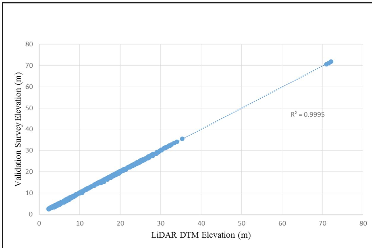
Figure 24. Correlation plot between validation survey points and LiDAR data.
