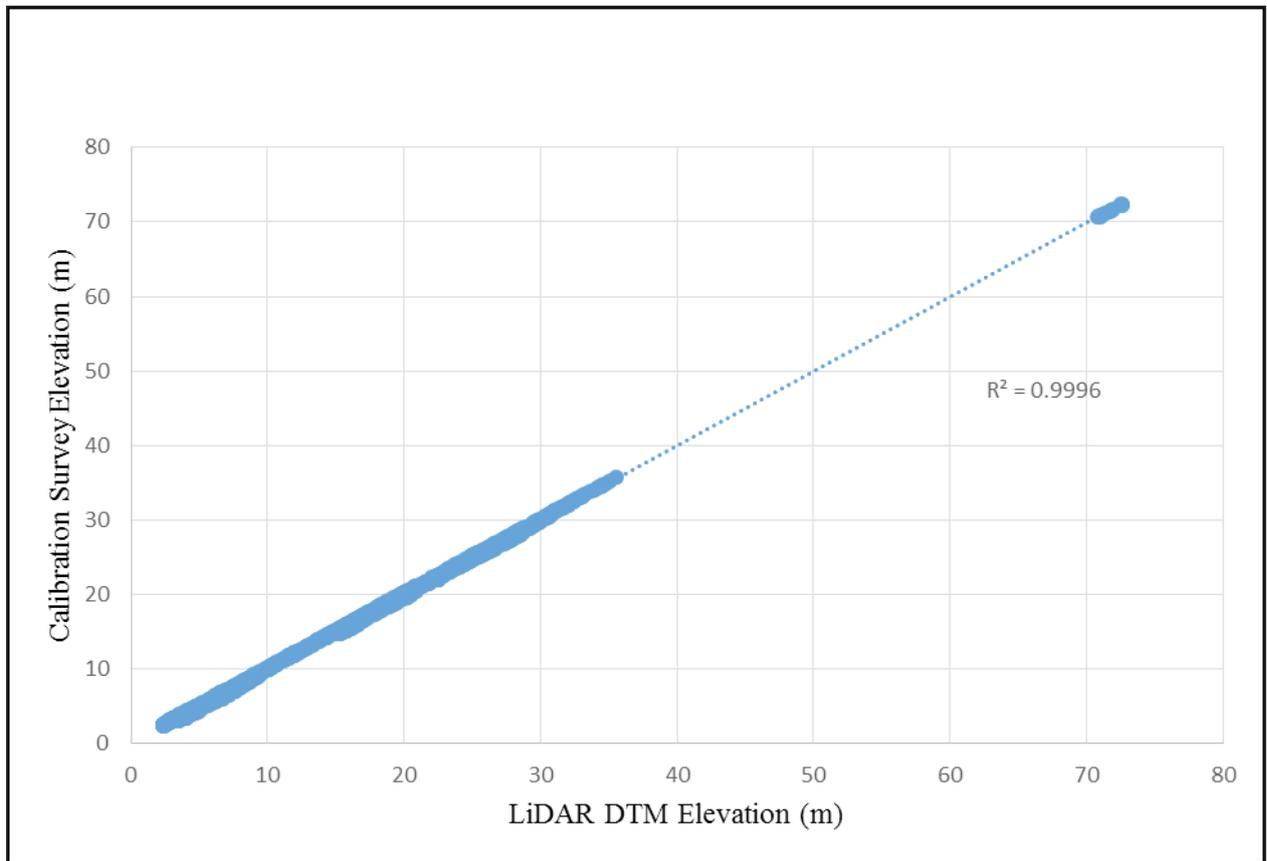
Figure 23. Correlation plot between calibration survey points and LiDAR data.
