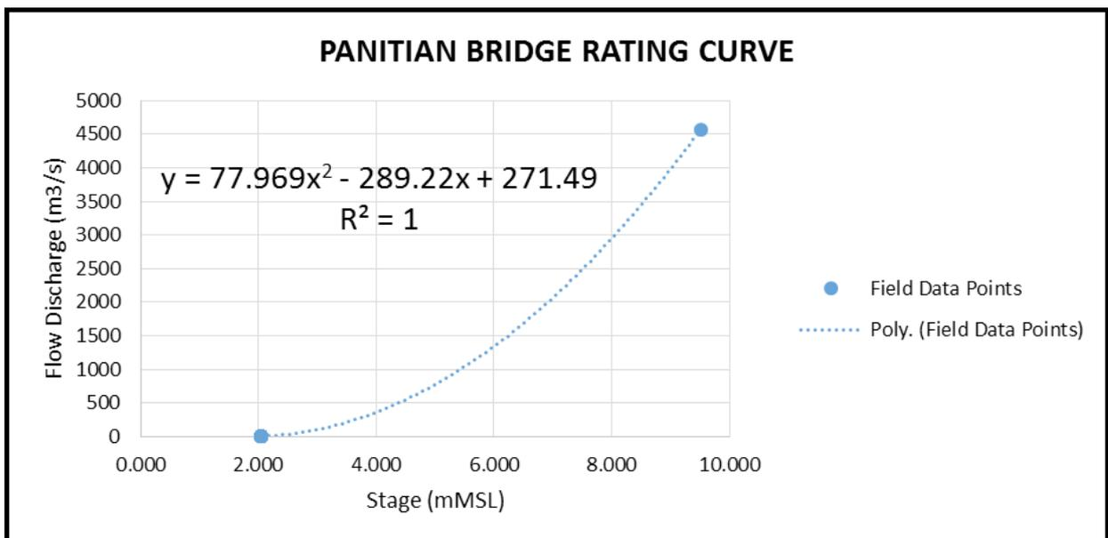
Figure 50. Rating curve at Panitian Bridge, Quezon, Palawan
