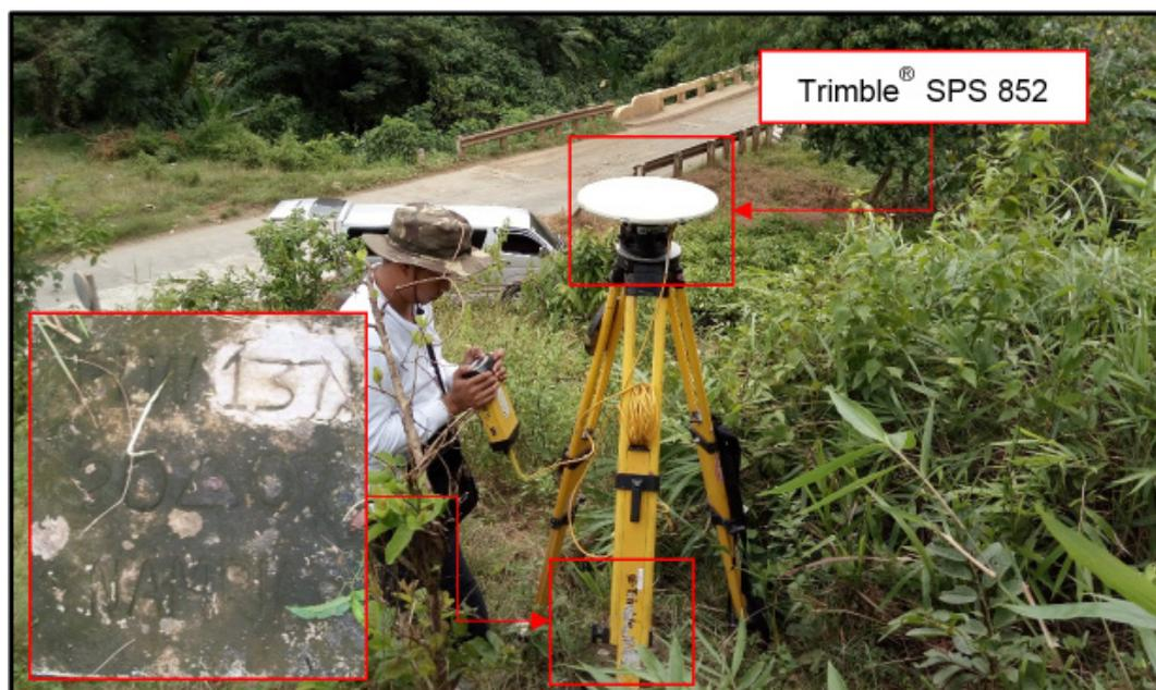
Figure 27. GNSS base set up, Trimble® SPS 852, at PLW-137, located at the top of a ridge along the National Highway in Brgy. Ipilan, Narra, Province of Palawan
