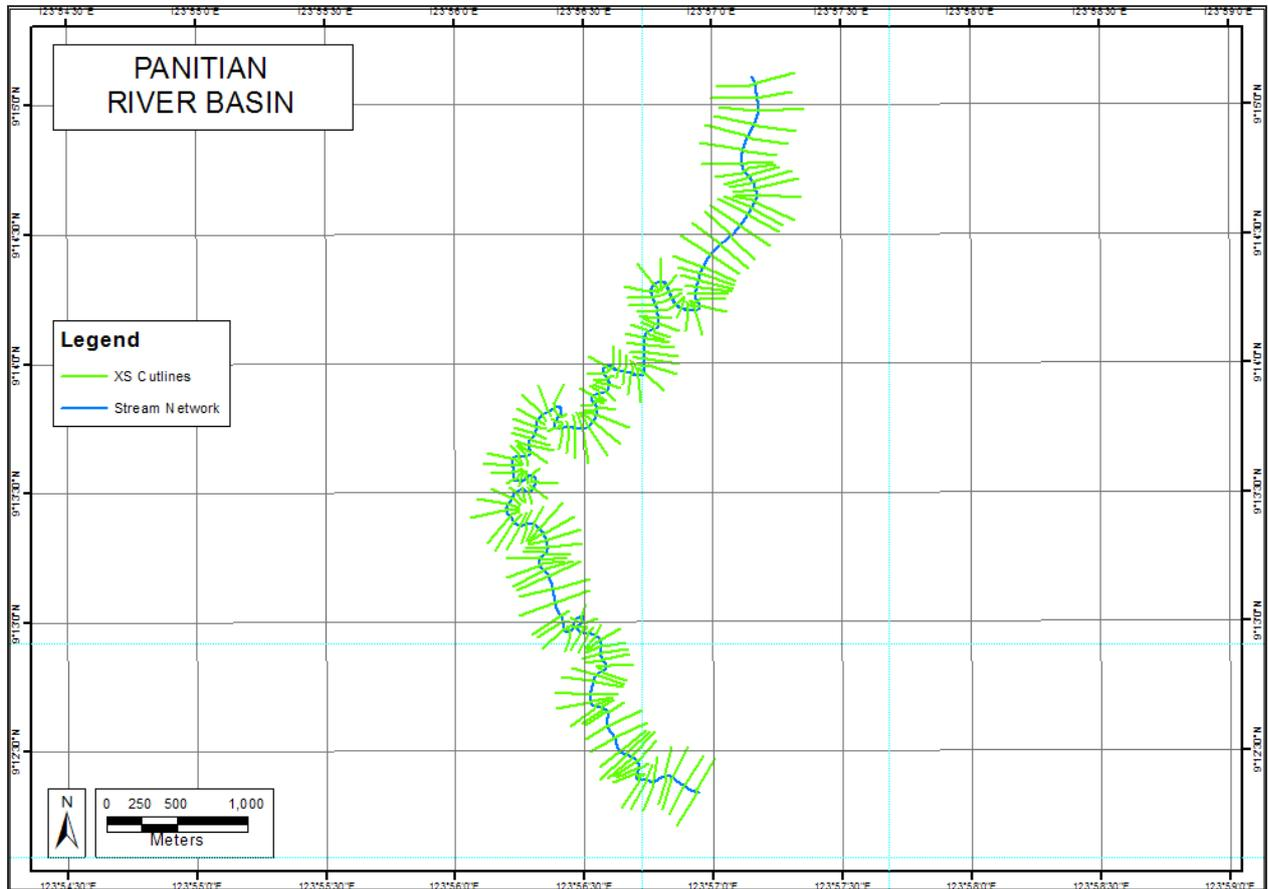
Figure 59. River cross-section of Panitian River generated through Arcmap HEC GeoRAS tool
