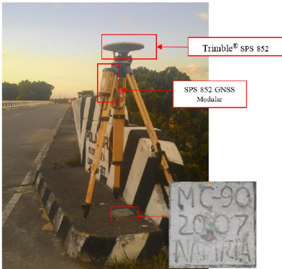
Figure 35. GNSS base, Trimble® SPS 852, at MC-90, used as marker, located at the Pola Bridge approach in Bgry. Barahan, Municipality of Santa Cruz, Occidental Mindoro
