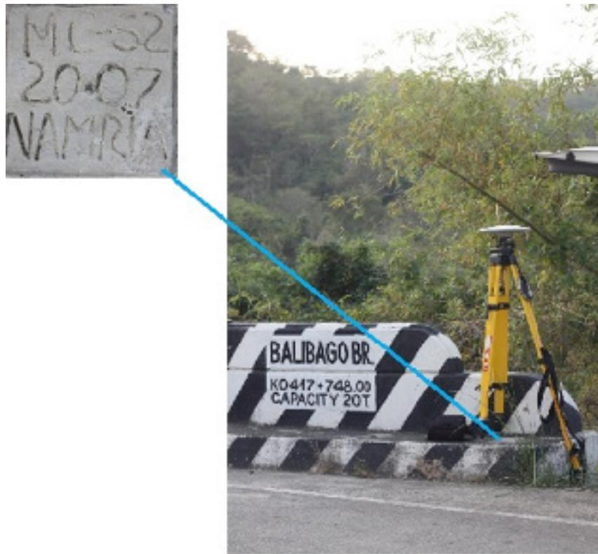
Figure 7. GPS set-up over MC-52as recovered in Balibago Bridge in Brgy. Armado, municipality of Abra de Ilog, Occidental Mindoro (a) and NAMRIA bench mark MC-52 (b) as recovered by the field team
