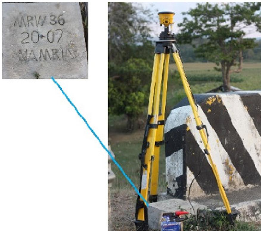
Figure 6. GPS set-up over MRW-36as recovered in Baclaran Bridge in Brgy. Cabacao, municipality of Abra de Ilog, Occidental Mindoro (a) and NAMRIA reference point MRW-36 (b) as recovered by the field team
