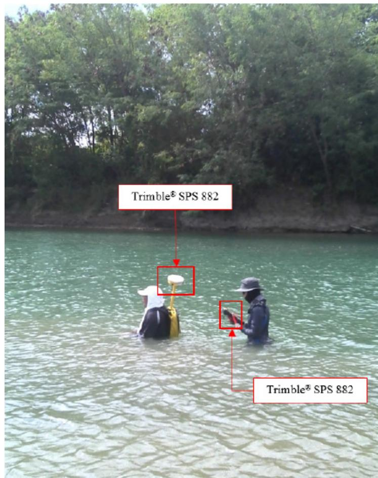
Figure 47. Manual Bathymetry set-up and execution for Pola River survey.
