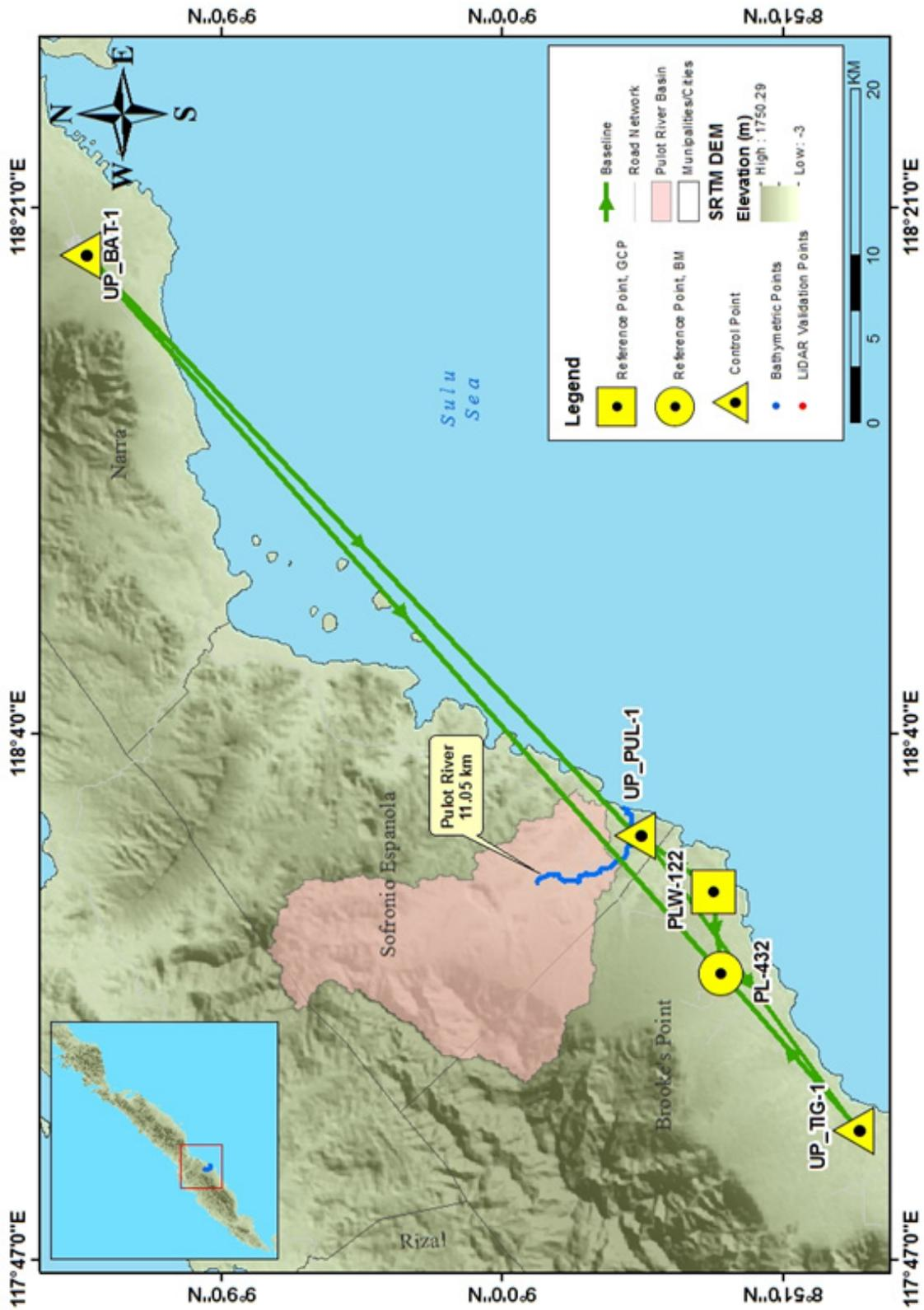
Figure 24. Extent of the bathymetric survey (in blue) in Pulot River and the LiDAR data validation (in red)
