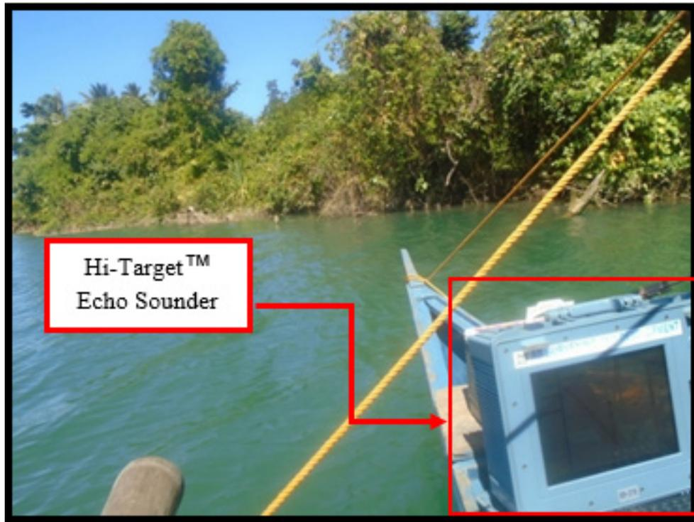
Figure 40. Bathymetric survey of ABSD at PulotRiver using Hi-Target™ EchoSounder (downstream)
