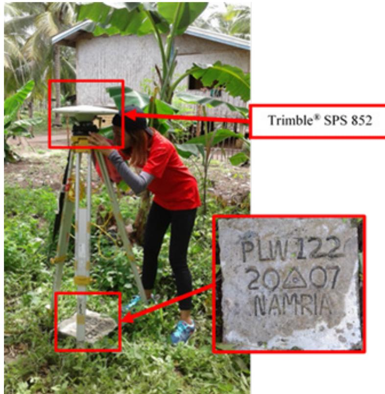
Figure 26. GNSS base set up, Trimble® SPS 852, at PLW-122, located in an open lot beside the house of Ms. Liza Jamili in Brgy. Calasaguen, Brookes Point, Province of Palawan.
