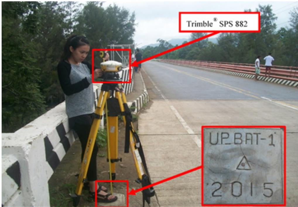
Figure 28. GNSS receiver set up, Trimble® SPS SPS 882, at UP\_BAT-1, located near the approach of Batang-batang Bridge in Brgy. PrincesaUrduja, Narra, Province of Palawan
