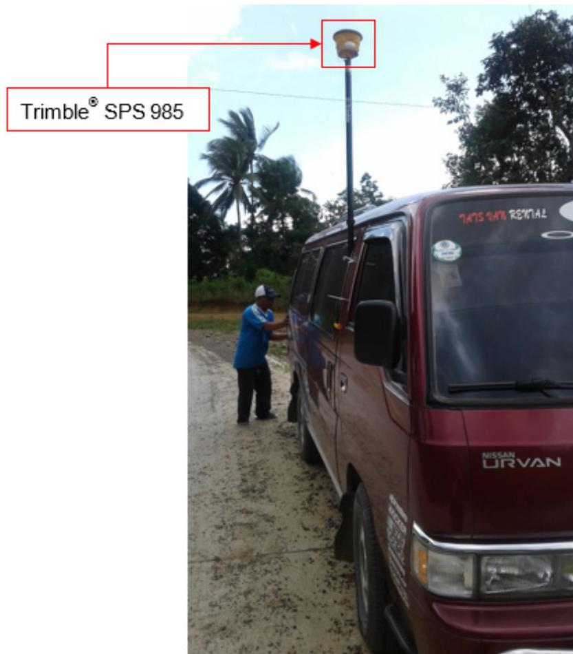
Figure 37. Validation points acquisition survey set-up for Pulot River
