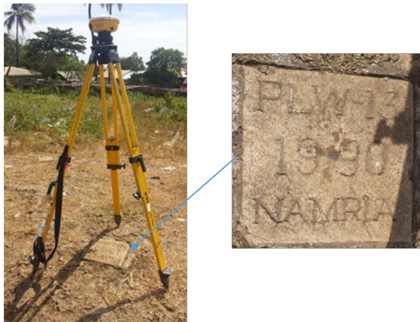
Figure 3. GPS set-up over PLW-13 at Barangay Rio Tuba, Palawan (a) and NAMRIA reference point PLW-13 (b) as recovered by the field team.
