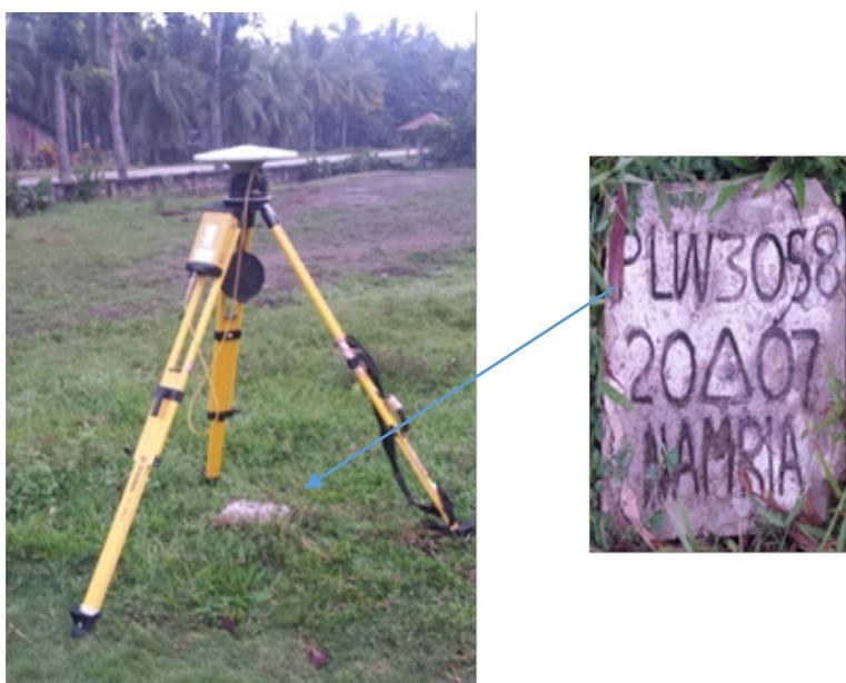
Figure 4. GPS set-up over PLW-3058 on the ground inside Caranasan Elementary School, Española, Palawan (a) and NAMRIA reference point PLW-3058 (b) as recovered by the field team.
