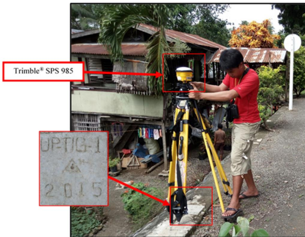
Figure 30. GNSS receiver set up, Trimble® SPS 985, at UP\_TIG-1, located at the approach of Tigaplan Bridge in Brgy. Tigaplan, Brookes Point, Province of Palawan.
