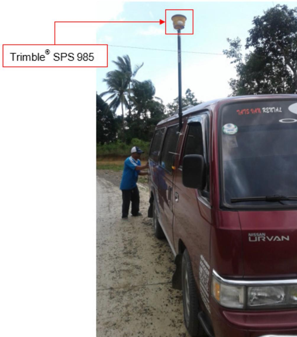
Figure 38. Validation points acquisition survey set-up for Ransang River
