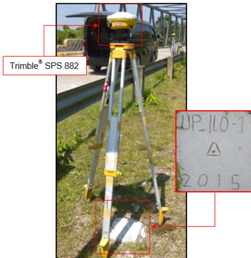
Figure 29. GNSS receiver set up, Trimble® SPS 882, at UP\_ILO-1 near the approach of Ilog-Ilog Bridge in Brgy. Campong Ulay, Rizal, Province of Palawan
