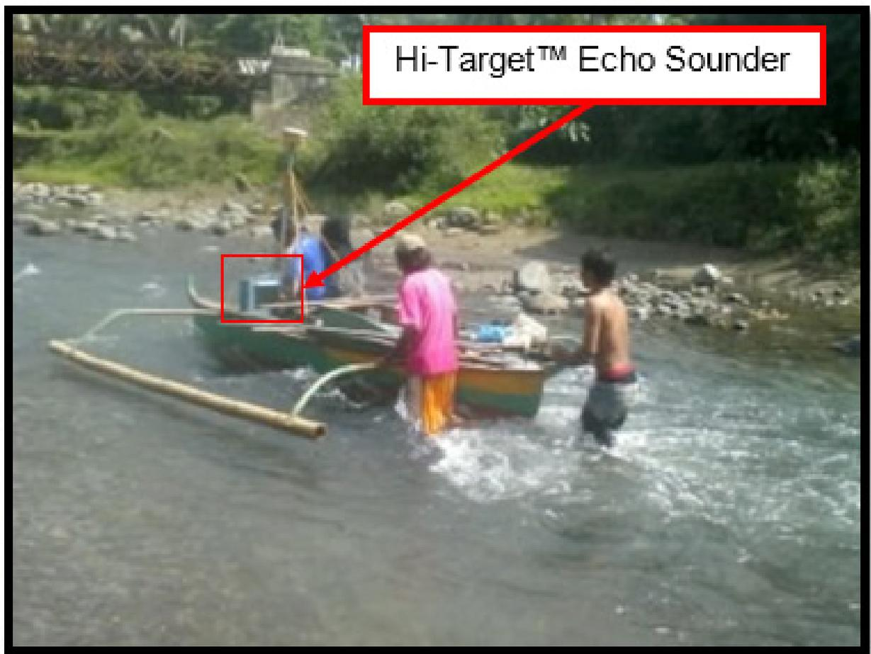
Figure 41. Bathymetric survey of ABSD at Ransang River using Hi-Target™ Echo Sounder (downstream)
