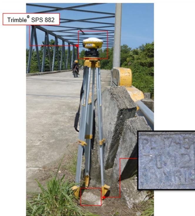
Figure 28. GNSS receiver set up, Trimble® SPS 882, at PL-749 located at the approach of Ilog-Ilog Bridge in Brgy. Campong Ulay, Rizal, Province of Palawan
