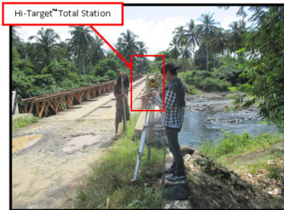
Figure 33. As-built survey of Ransang Bridge
