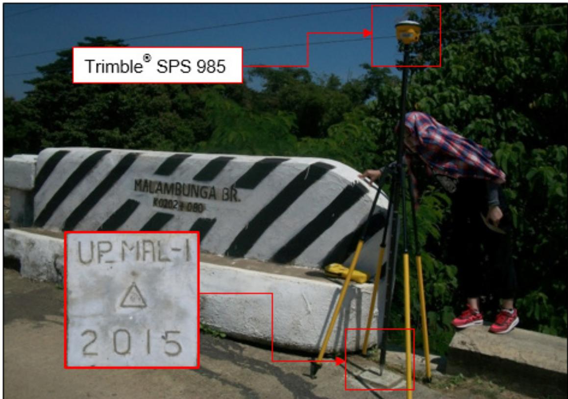
Figure 30. GNSS receiver set up, Trimble® SPS 985, at UP\_MAL-1, Malambunga Bridge in Brgy. Punta Baja, Rizal, Province of Palawan
