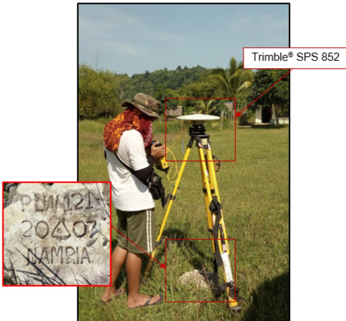
Figure 27. GNSS base set up, Trimble® SPS 852, at PLW-121, located along the edge of a basketball court inside Cabkungan Elementary School in Brgy. Ransang, Rizal, Province of Palawan
