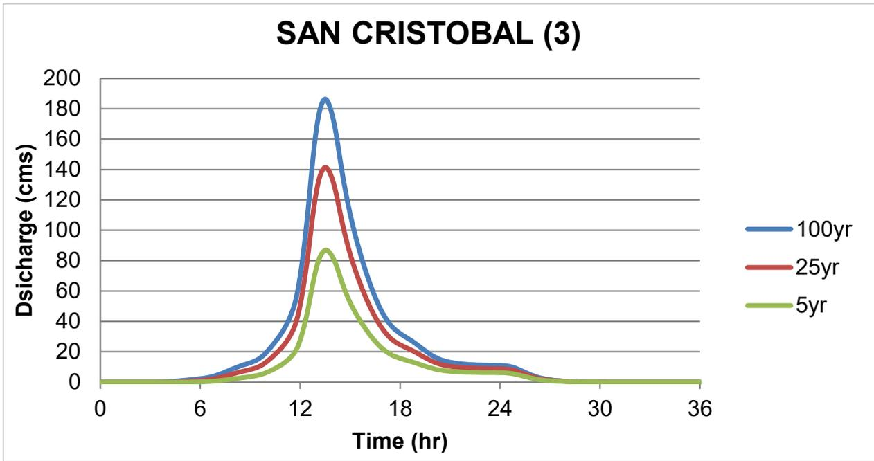
Figure 62. San Cristobal river (3) generated discharge using 5-, 25-, and 100-year Ambulong rainfall intensity-duration-frequency (RIDF) in HEC-HMS.
