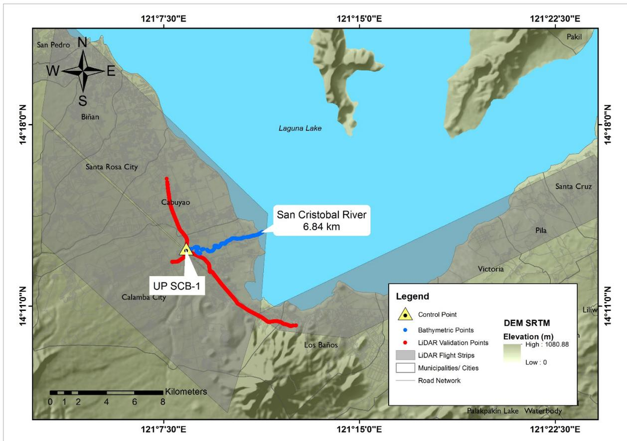
Figure 40. Validation Points Acquisition Survey along the Municipality of Cabuyao to Municipality of Los Baños
