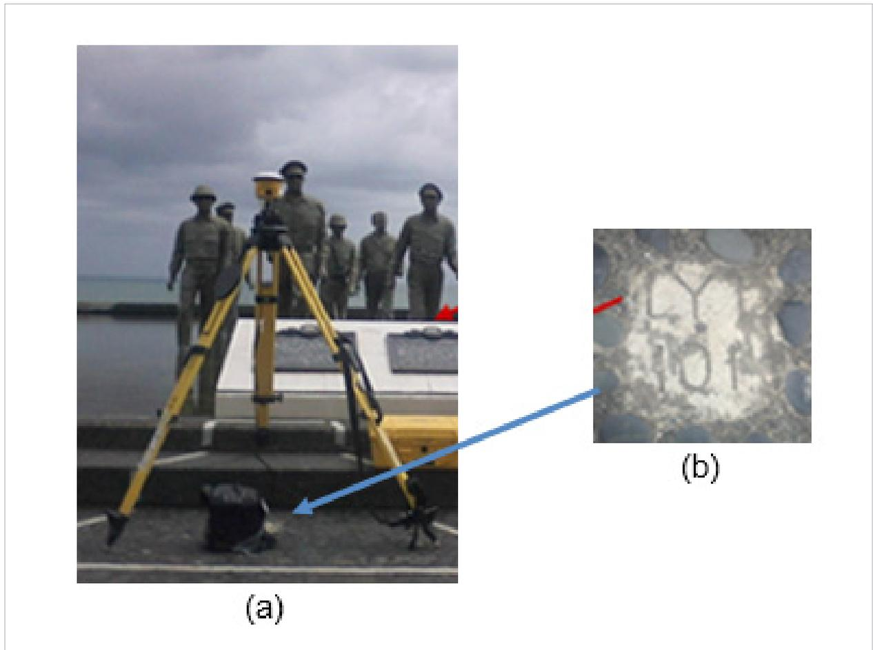
Figure 7. GPS set-up over LYT-101 located within the premises of MacArthur’s Landing Memorial Park, Palo, Leyte (a) and NAMRIA reference point LYT-101 (a) as recovered by the field team.
