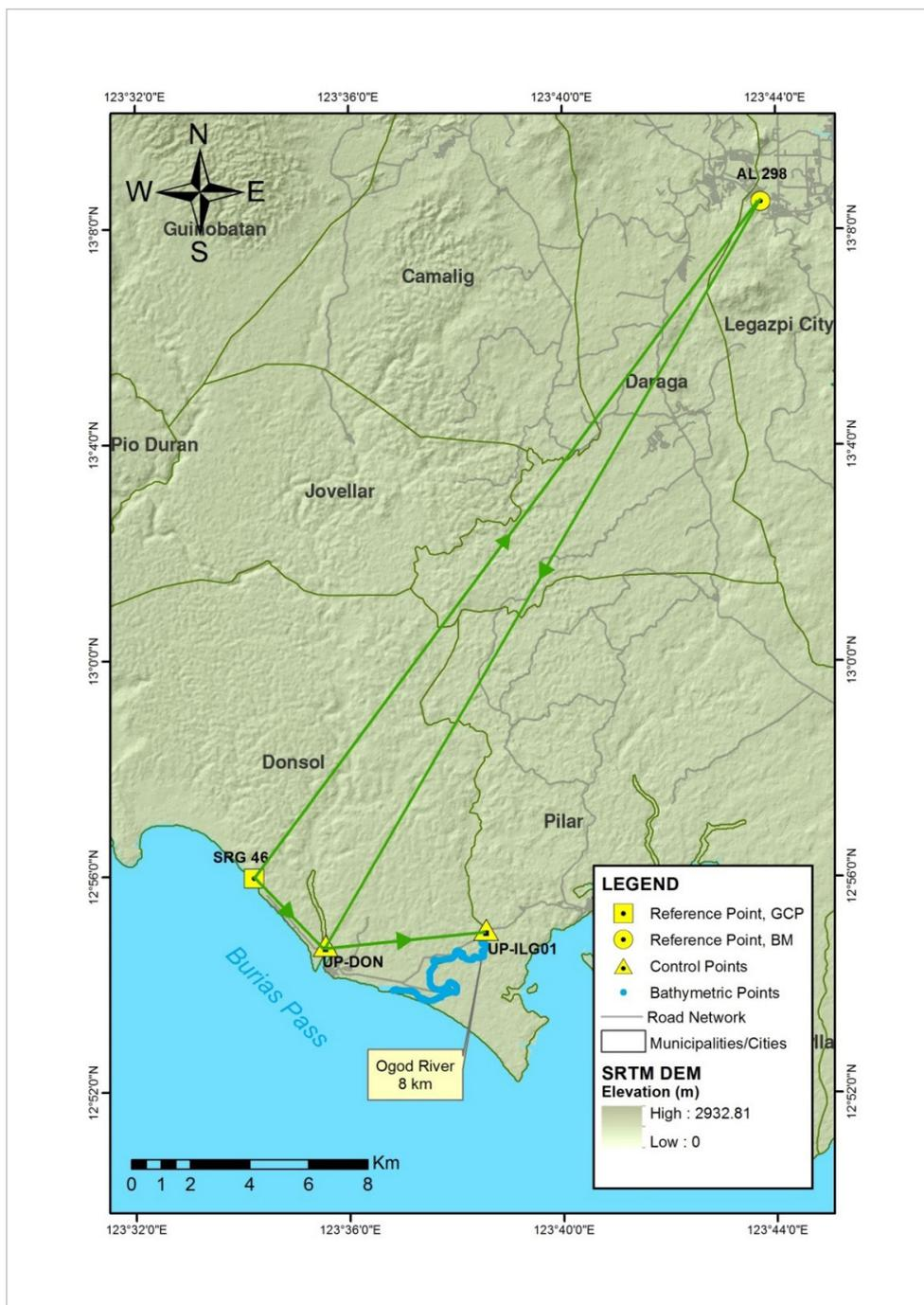
Figure 31. GNSS Network of San Cristobal River Field Survey.
