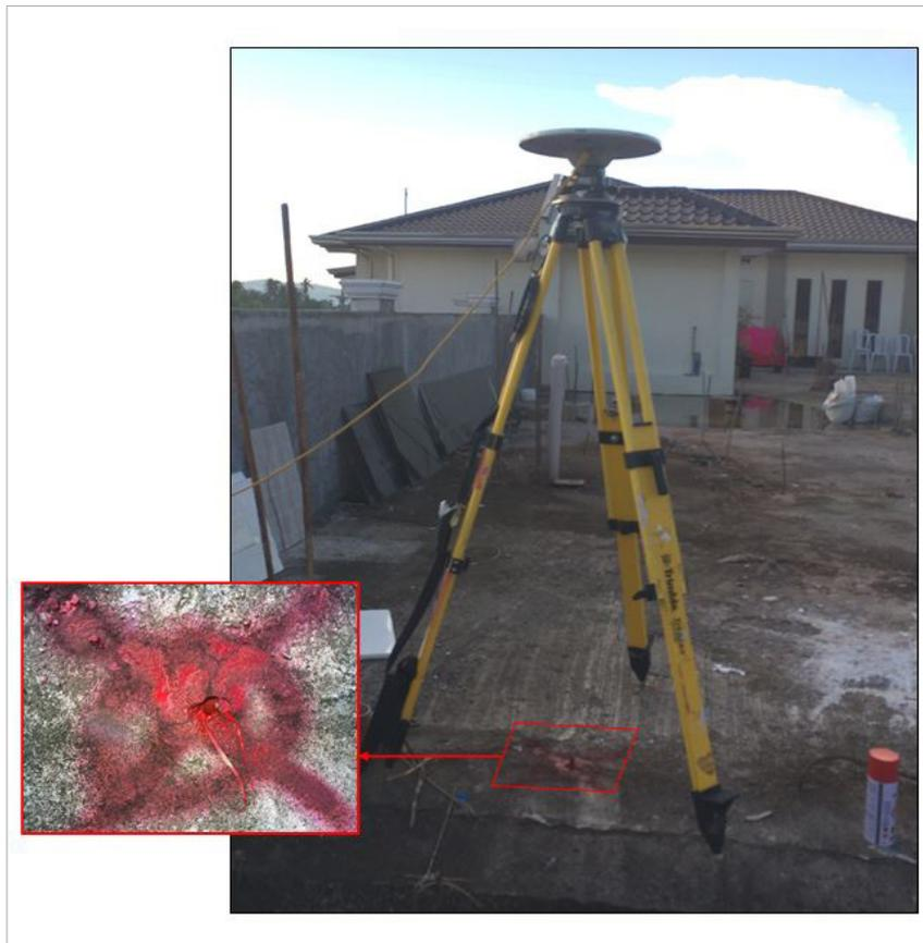
Figure 34. GNSS base receiver setup, Trimble® SPS 852 at RB-1, located at the roof top of Asia Blooms Hotel, Brgy. Patimbao, Sta. Cruz, Laguna
