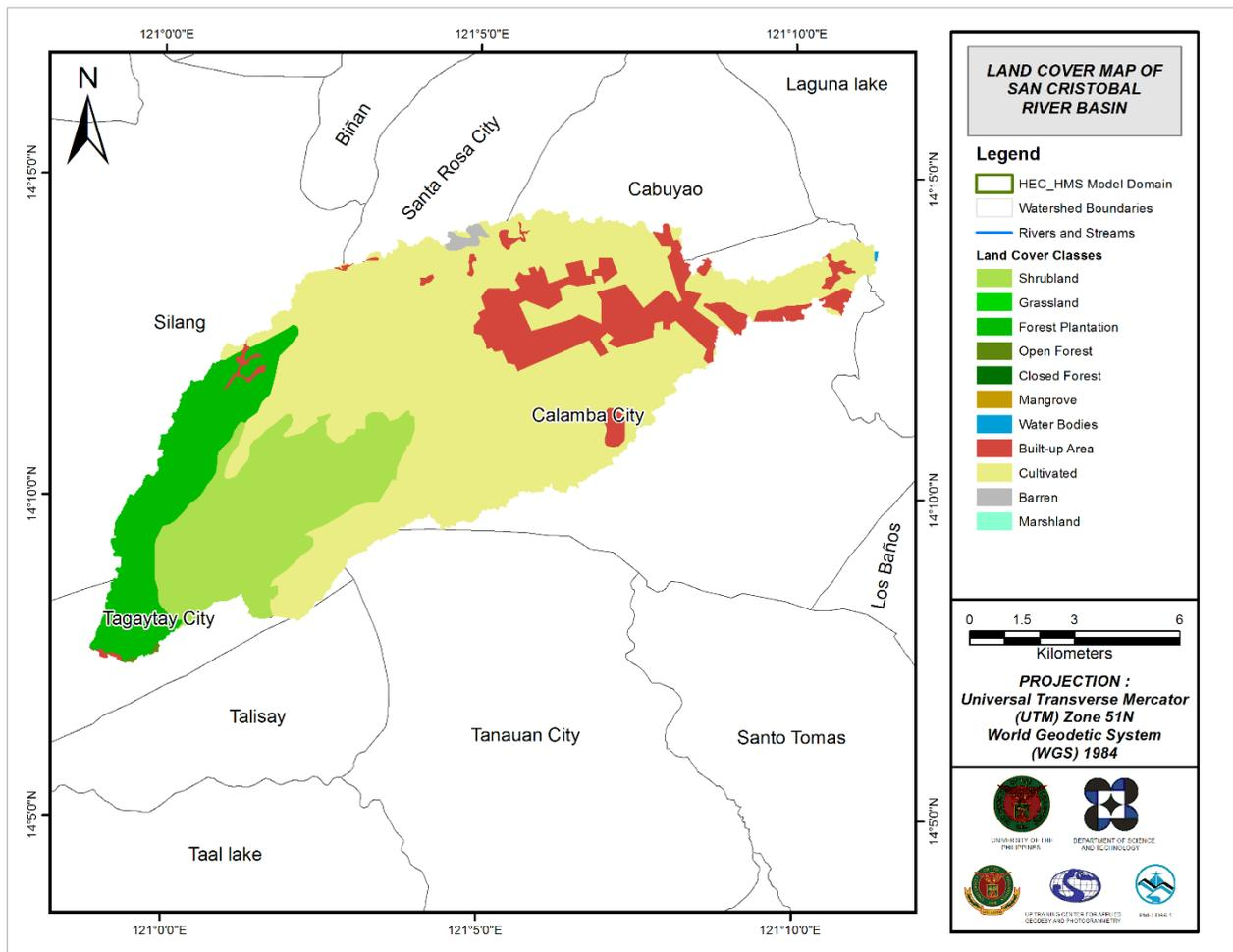
Figure 51. The land cover map of the San Cristobal River Basin used for the estimation of the CN and watershed lag parameters of the rainfall-runoff model. (Source of data: Digital soil map of the Philippines published by the Bureau of Soil and Water Management – Department of Agriculture)
