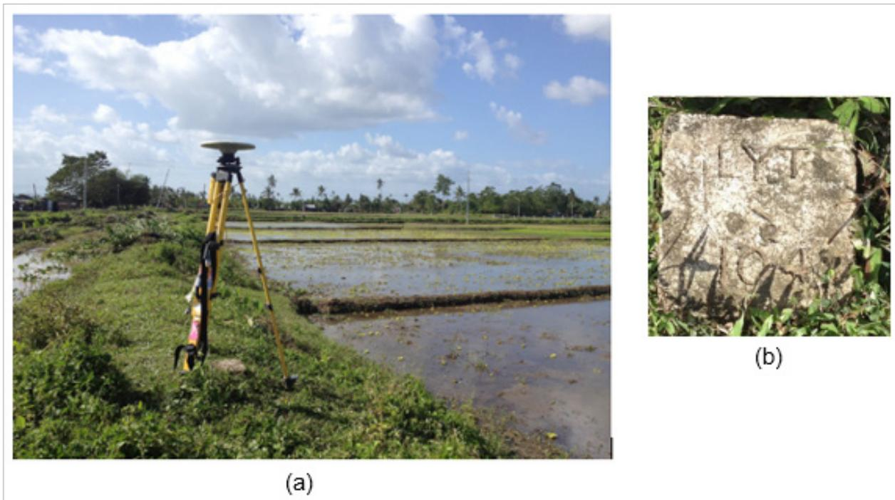
Figure 8. GPS set-up over LYT-104 located and re-established along rice paddy trail, approximately 90 meters from the centerline, east side of Pastrana-Santa Fe Road, District IV, Pastrana, Leyte (a) and NAMRIA reference point LYT-104 (b) as recovered by the field team.
