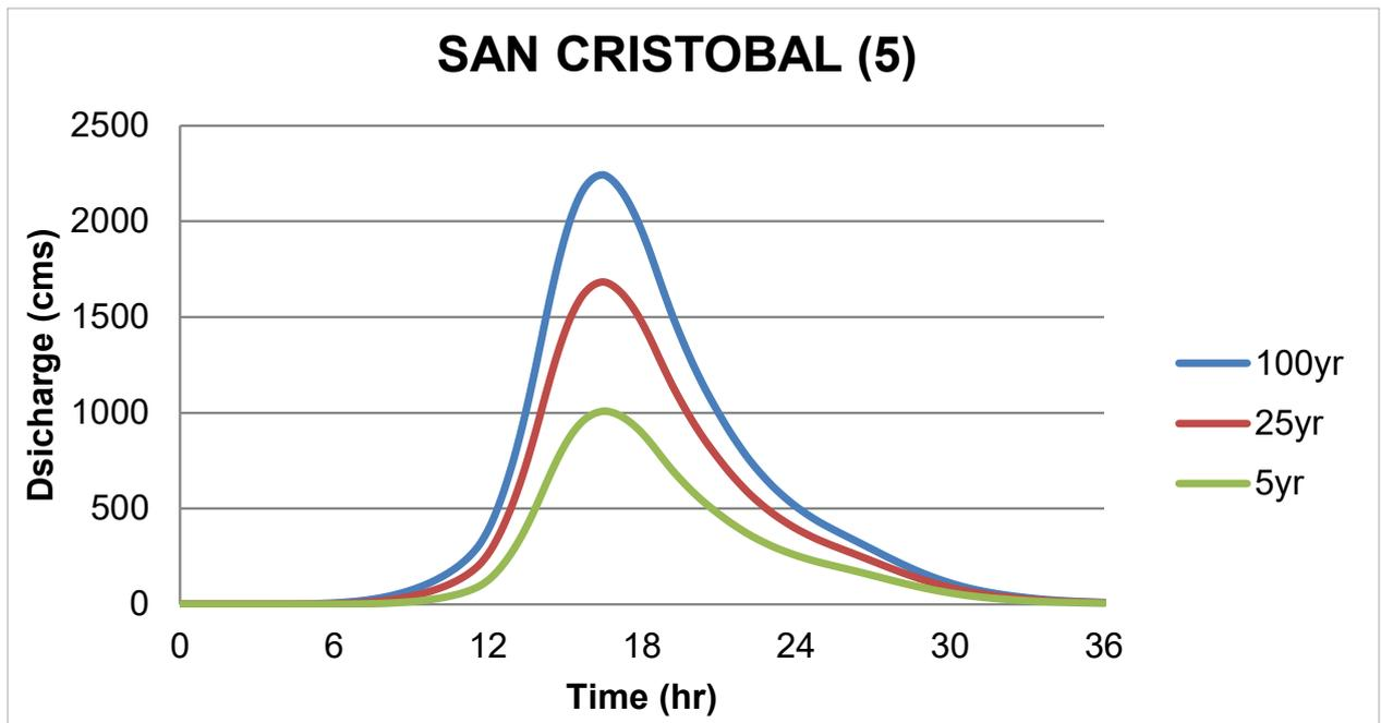
Figure 64. San Cristobal river (5) generated discharge using 5-, 25-, and 100-year Ambulong rainfall intensity-duration-frequency (RIDF) in HEC-HMS.
