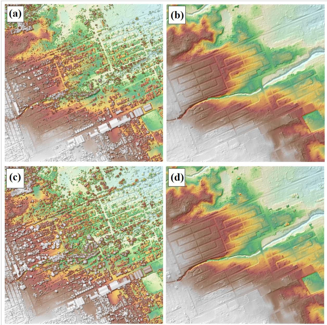
Figure 21. The production of last return DSM (a) and DTM (b), first return DSM (c) and secondary DTM (d) in some portion of San Cristobal floodplain.
