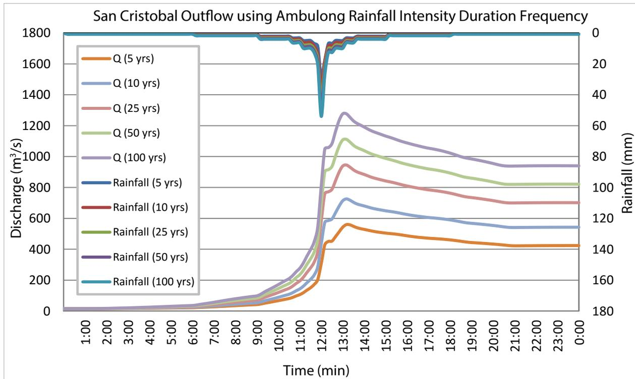
Figure 59. Outflow hydrograph at San Cristobal Station generated using Ambulong RIDF simulated in HEC-HMS.
