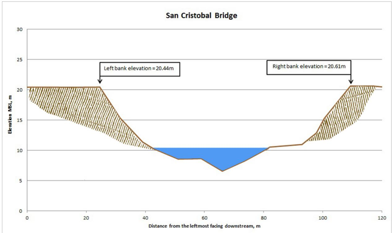
Figure 45. Cross-Section Plot of San Cristobal Bridge.
