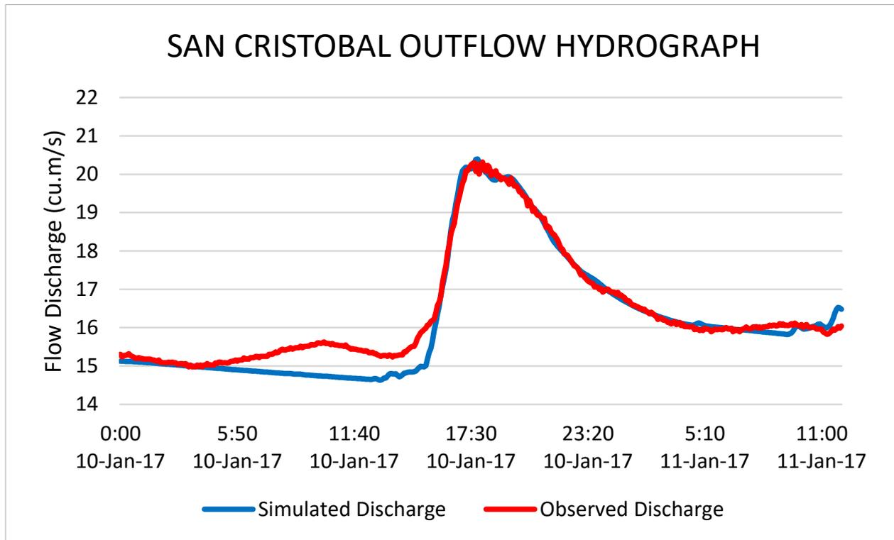
Figure 58. Outflow Hydrograph of San Cristobal produced by the HEC-HMS model compared with observed outflow.
