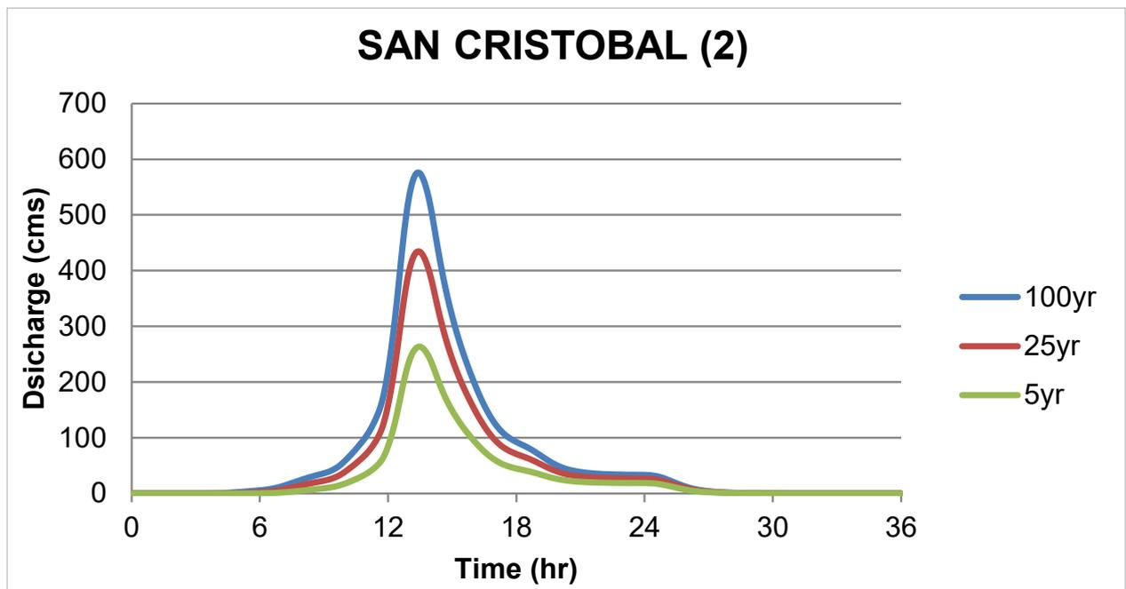
Figure 61. San Cristobal river (2) generated discharge using 5-, 25-, and 100-year Ambulong rainfall intensity-duration-frequency (RIDF) in HEC-HMS.
