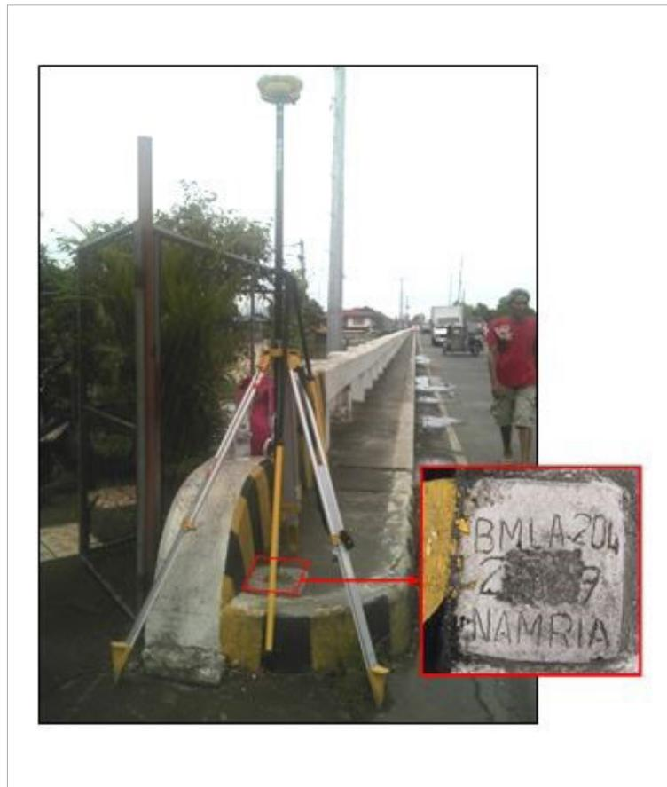
Figure 33. GNSS receiver setup, Trimble® SPS 882 at LA-204 in the Municipality of Lumban, Laguna
