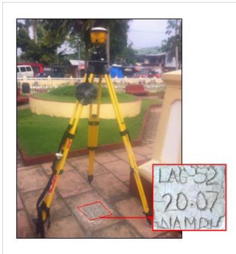
Figure 32. GNSS receiver setup, Trimble® SPS 985 at LAG-52 in the Municipality of Magdalena, Laguna
