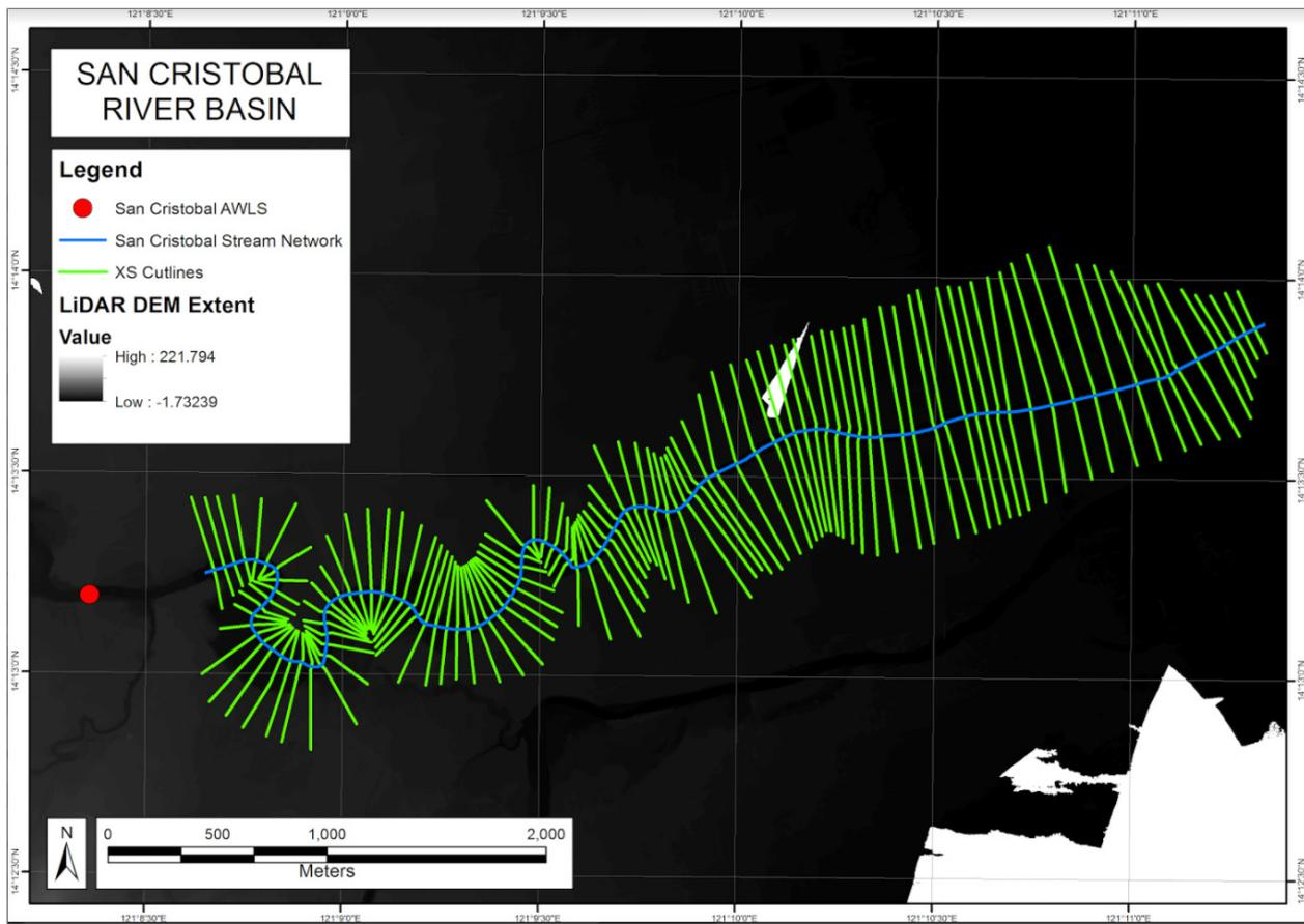
Figure 55. River cross-section of San Cristobal River generated through Arcmap HEC GeoRAS tool.
