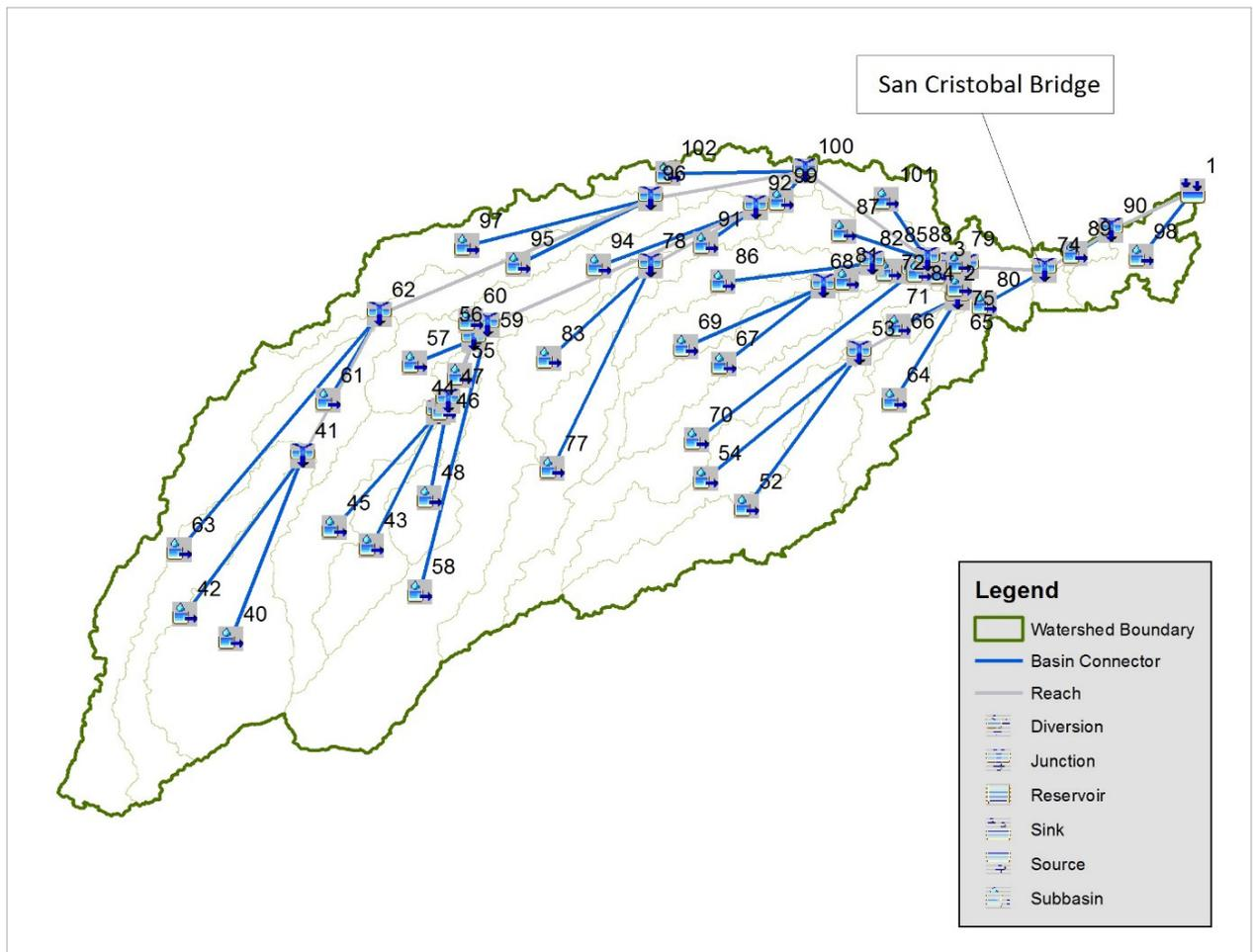
Figure 54. The San Cristobal river basin model generated using HEC-HMS.
