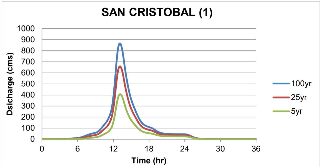
Figure 60. San Cristobal river (1) generated discharge using 5-, 25-, and 100-year Ambulong rainfall intensity-duration-frequency (RIDF) in HEC-HMS
