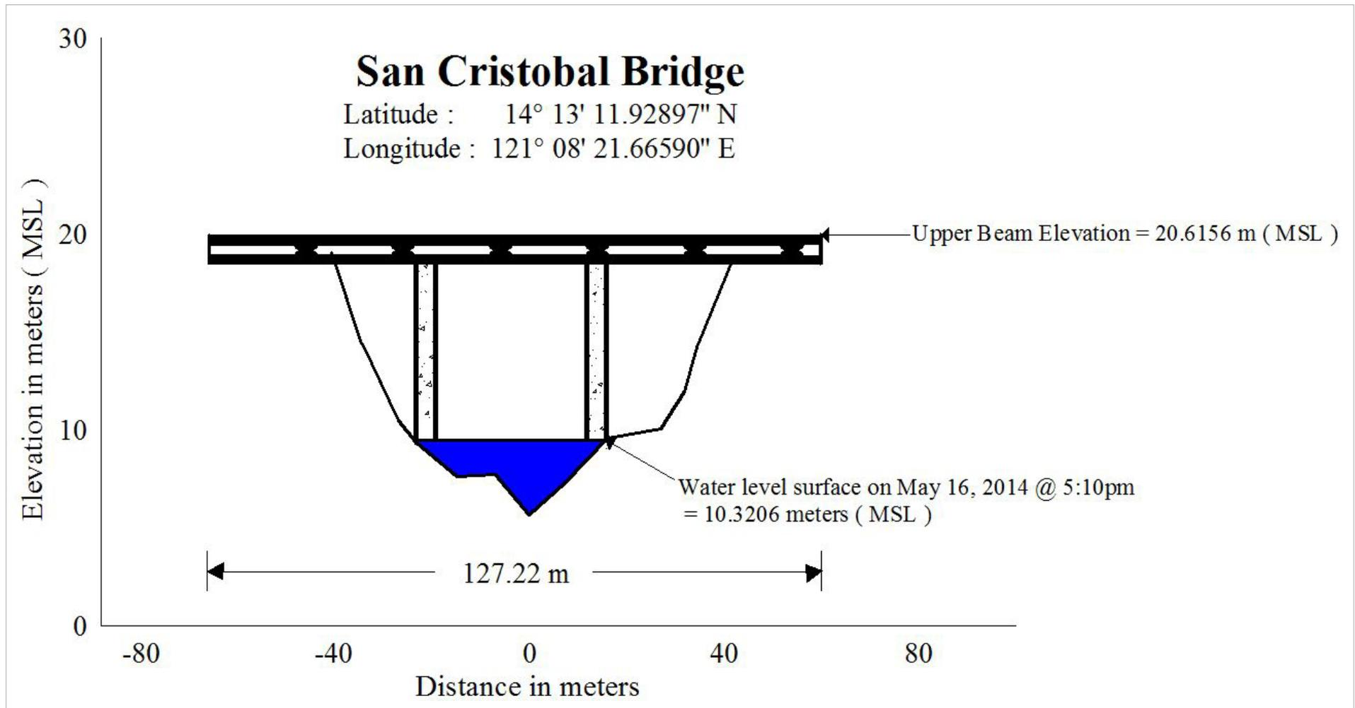
Figure 36. San Cristobal Bridge cross section diagram.
