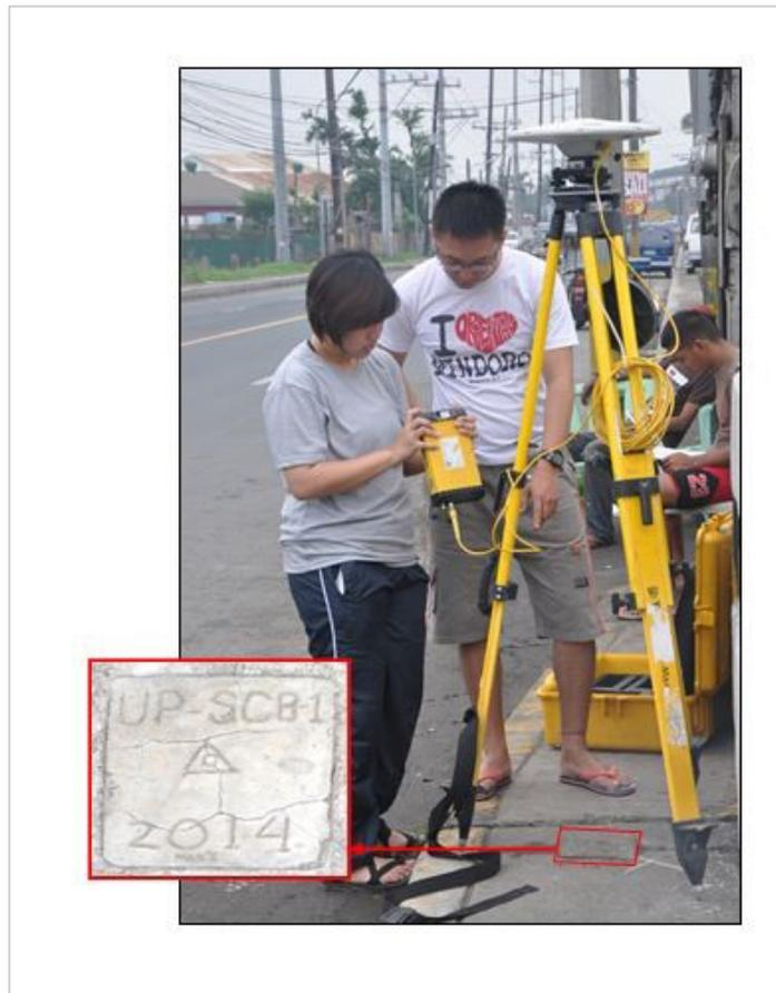
Figure 35. GNSS base receiver setup, Trimble® SPS 852 at UP-SCB-1, San Cristobal Bridge in Calamba City, Laguna
