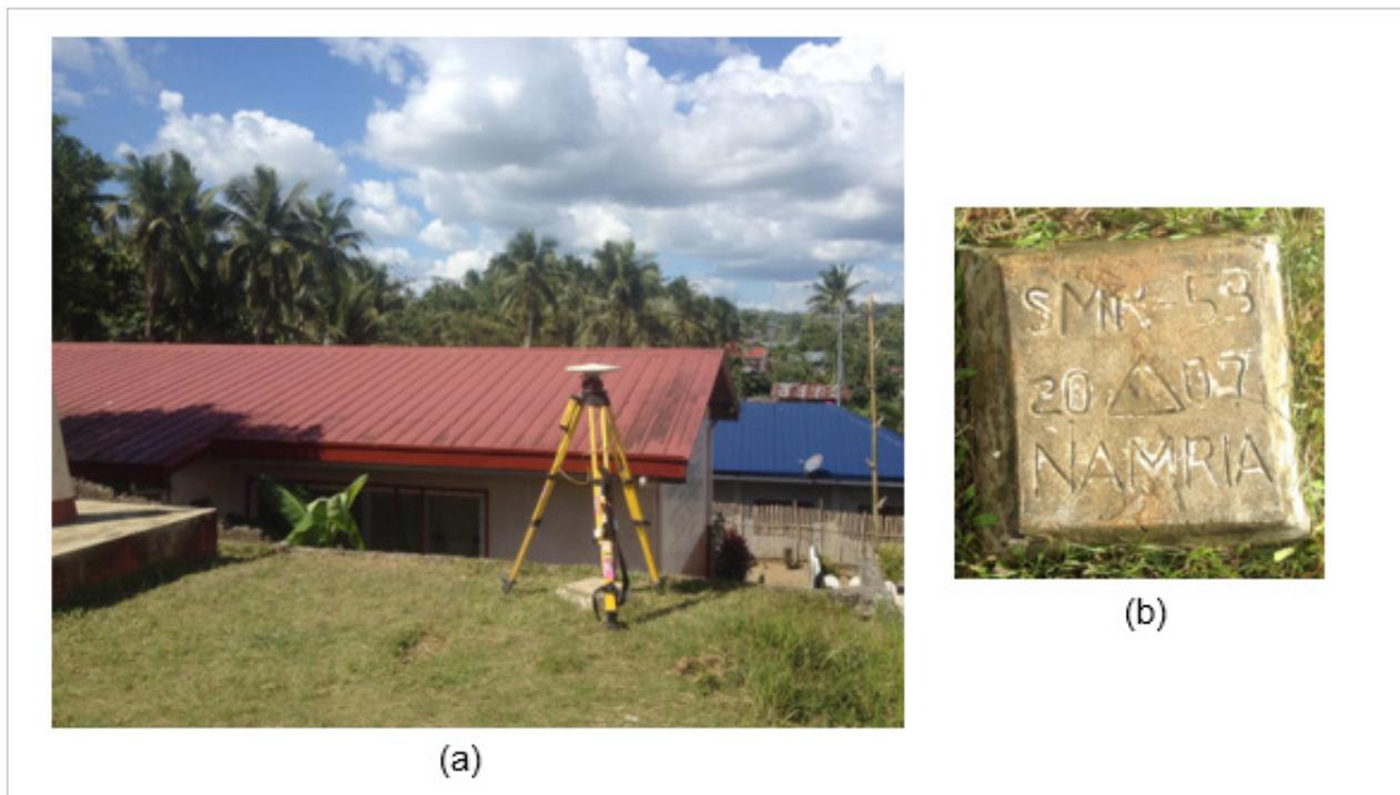
Figure 2. GPS set-up over SMR-53 located near the school building flag pole of San Isidro Elementary, Brgy. San Isidro, Santa Rita (a) and NAMRIA reference point SMR-53 (b) as recovered by the field team.
