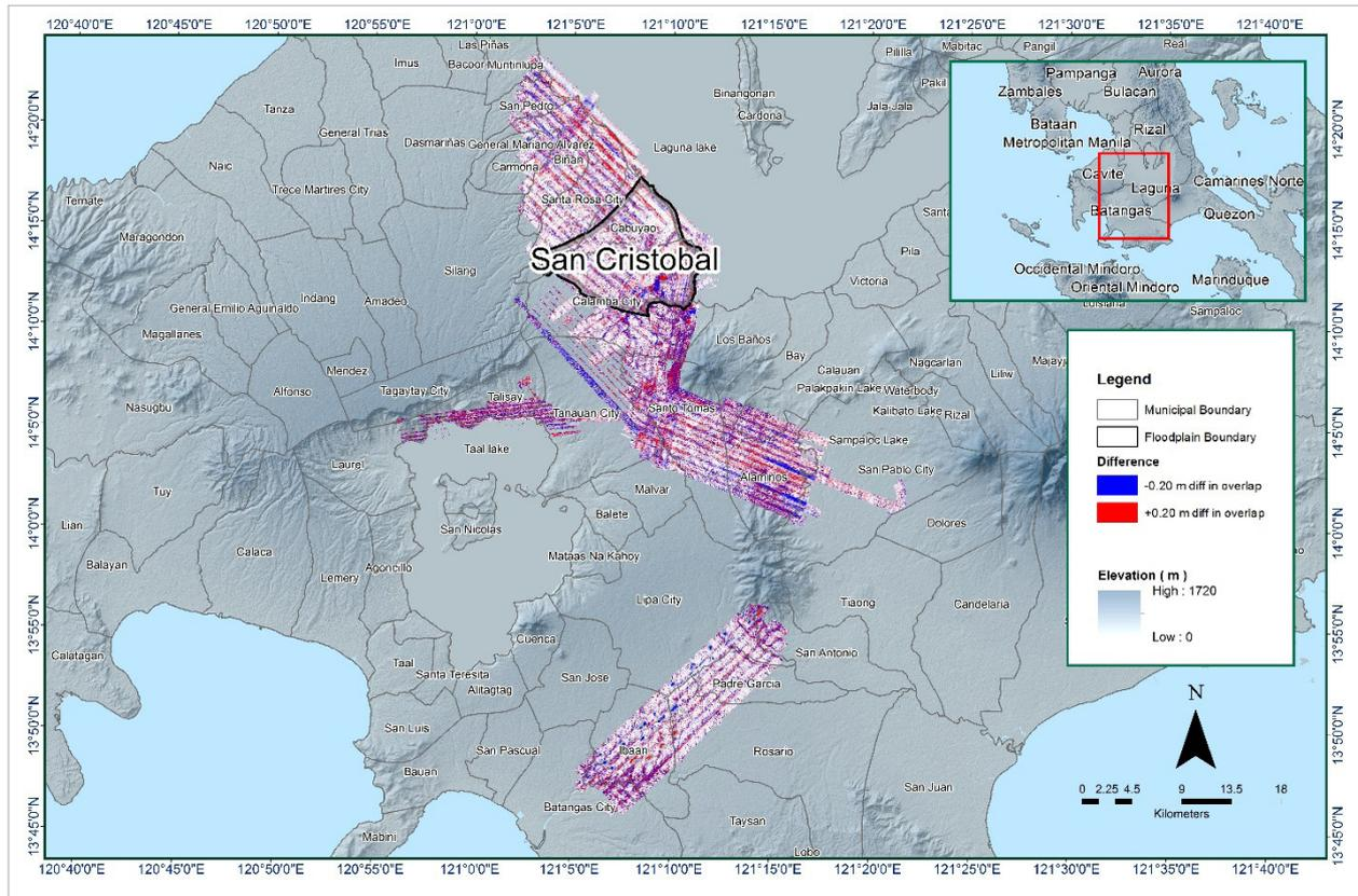
Figure 17. Elevation difference map between flight lines for San Cristobal floodplain.
