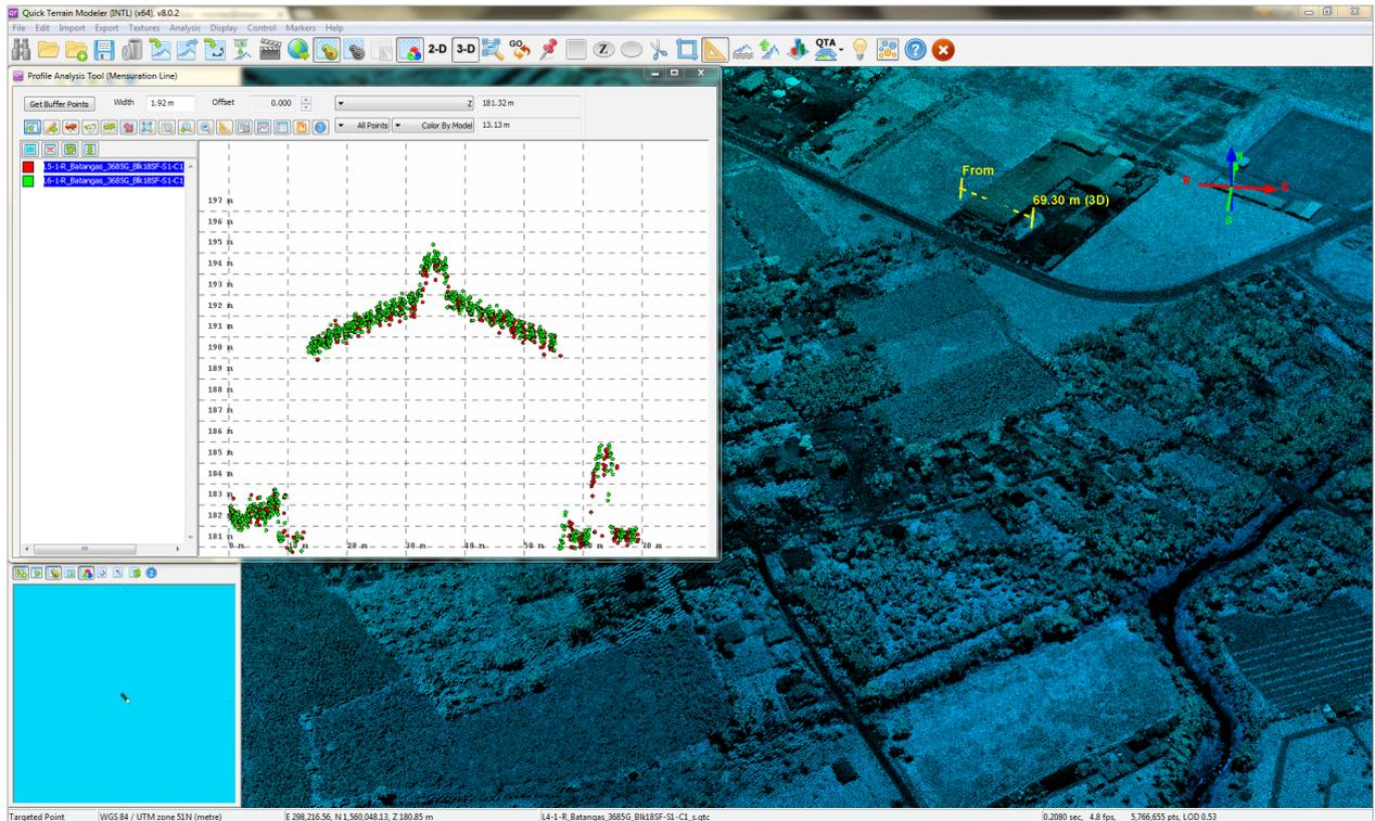
Figure 18. Quality checking for a San Cristobal flight 3685G using the Profile Tool of QT Modeler.
