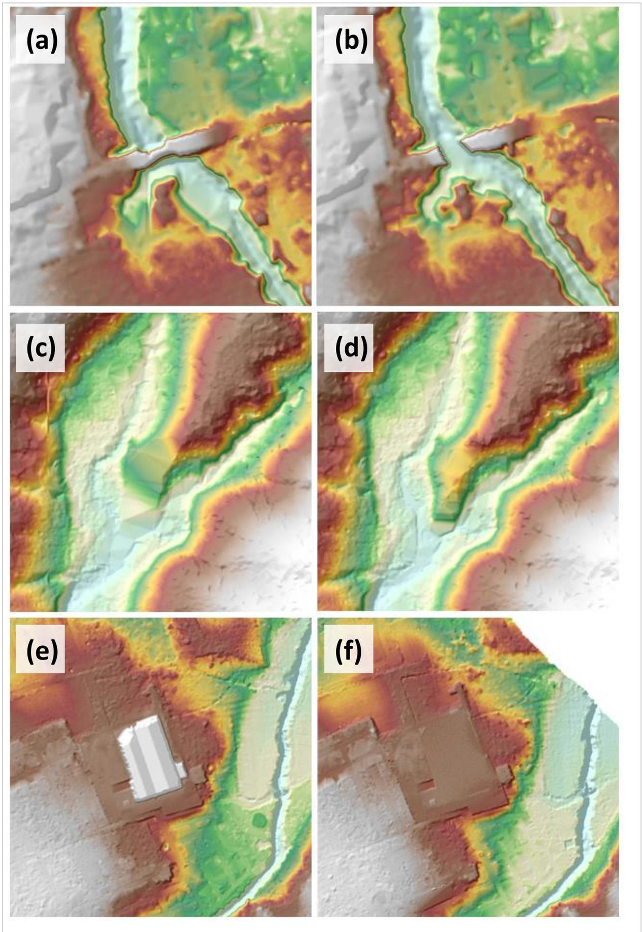
Figure 24. Portions in the DTM of San Cristobal floodplain – a bridge before (a) and after (b) manual editing; a mountain before (c) and after (d) data retrieval; and a building before (e) and after (f) manual editing.
