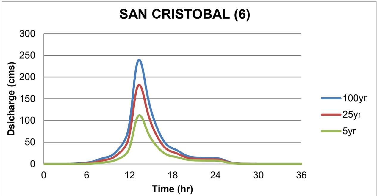
Figure 65. San Cristobal river (6) generated discharge using 5-, 25-, and 100-year Ambulong rainfall intensity-duration-frequency (RIDF) in HEC-HMS
