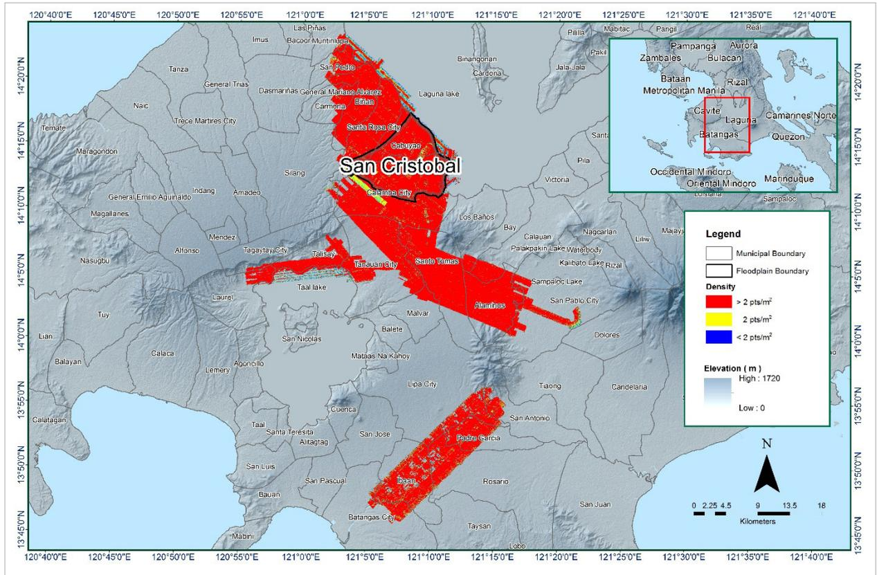
Figure 16. Density map of merged LiDAR data for San Cristobal floodplain.
