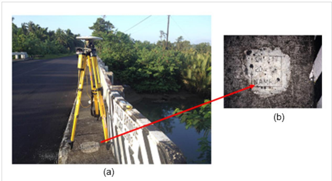
Figure 5. GPS set-up over SM-286 located at Dalid bridge along national highway in Brgy. San Pascual, Sta. Rita, Samar (a) and NAMRIA reference point SM-286 (a) as recovered by the field team.
