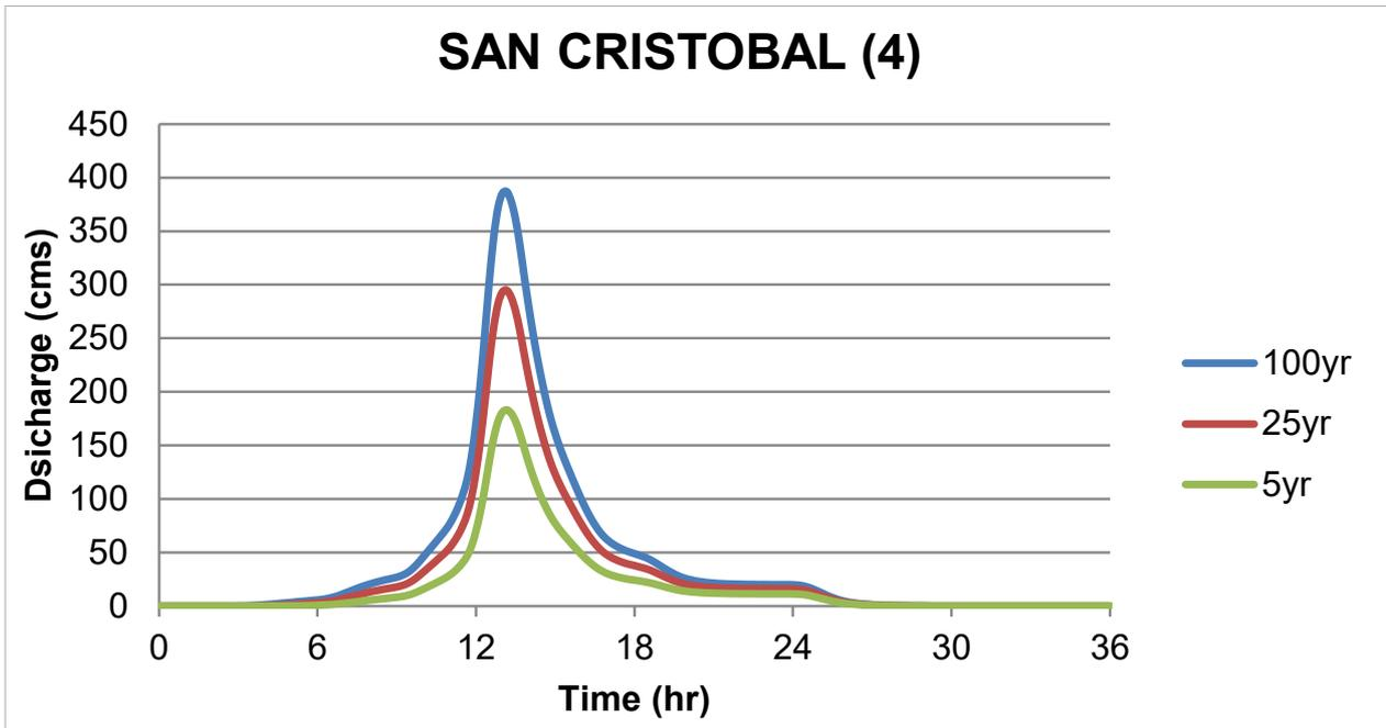
Figure 63. San Cristobal river (4) generated discharge using 5-, 25-, and 100-year Ambulong rainfall intensity-duration-frequency (RIDF) in HEC-HMS.
