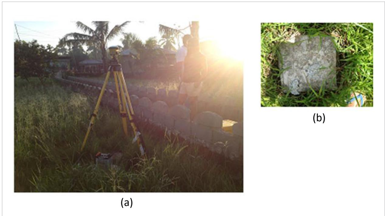
Figure 3. GPS set-up over SMR-56 located inside Cabacungan Elementary School in Brgy. Cabacungan, Sta. Rita, Samar (a) and NAMRIA reference point SMR-56 (b) as recovered by the field team.
