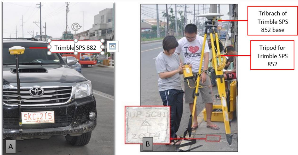
Figure 39. (A) Setup of Trimble® SPS 882 attached to a vehicle and (B) Setting up of GNSS base station at UP-SCB-1
