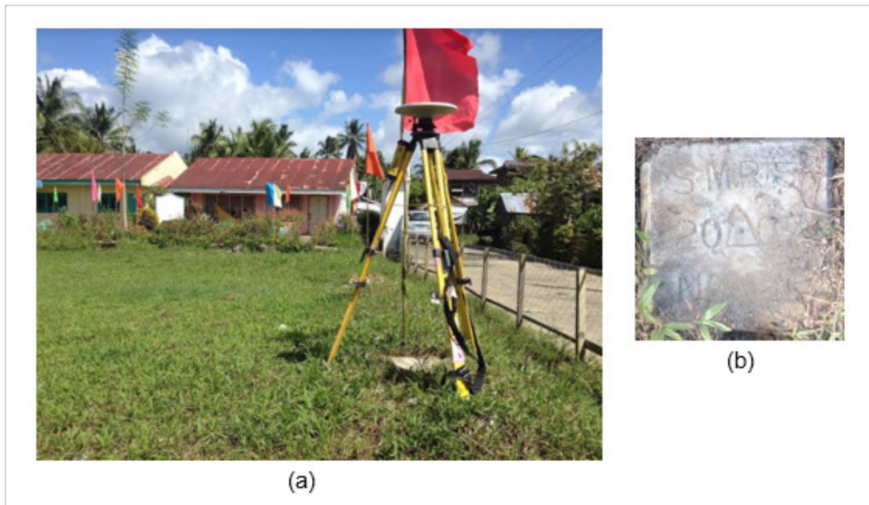
Figure 4. GPS set-up over SMR-58 located inside Serum Elementary School, Brgy. Serum, Basey (a) and NAMRIA reference point SMR-58 (b) as recovered by the field team.
