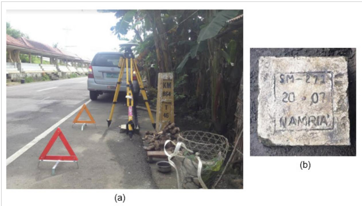
Figure 6. GPS set-up over SM-271 located beside kilometer post 864 along right side of the national highway, Bgry. Laygayon, Pinabacdao (a) and NAMRIA reference point SM-271 (b) as recovered by the field team.
