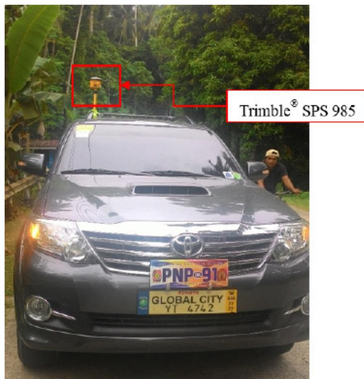
Figure 36. Validation points acquisition survey set-up along Tawiran-Tagum River Basin
