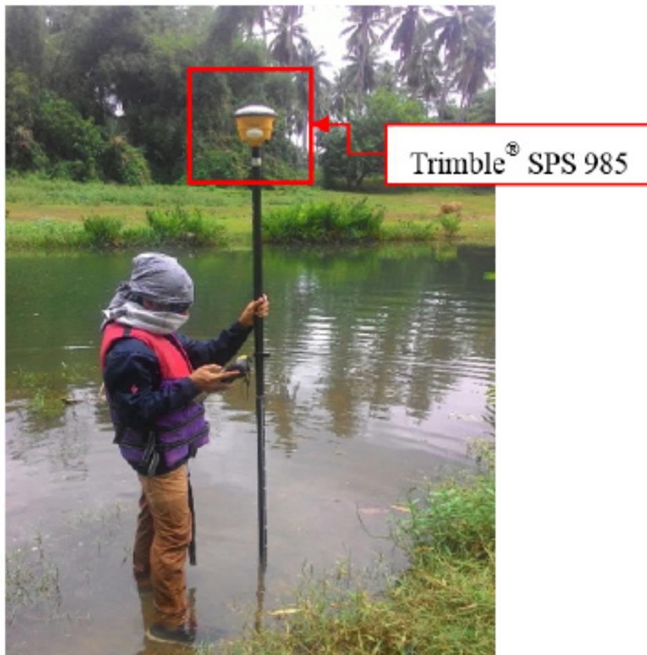
Figure 39. Bathymetric survey using Trimble® SPS 882 in GNSS PPK survey technique in Tawiran-Tagum River
