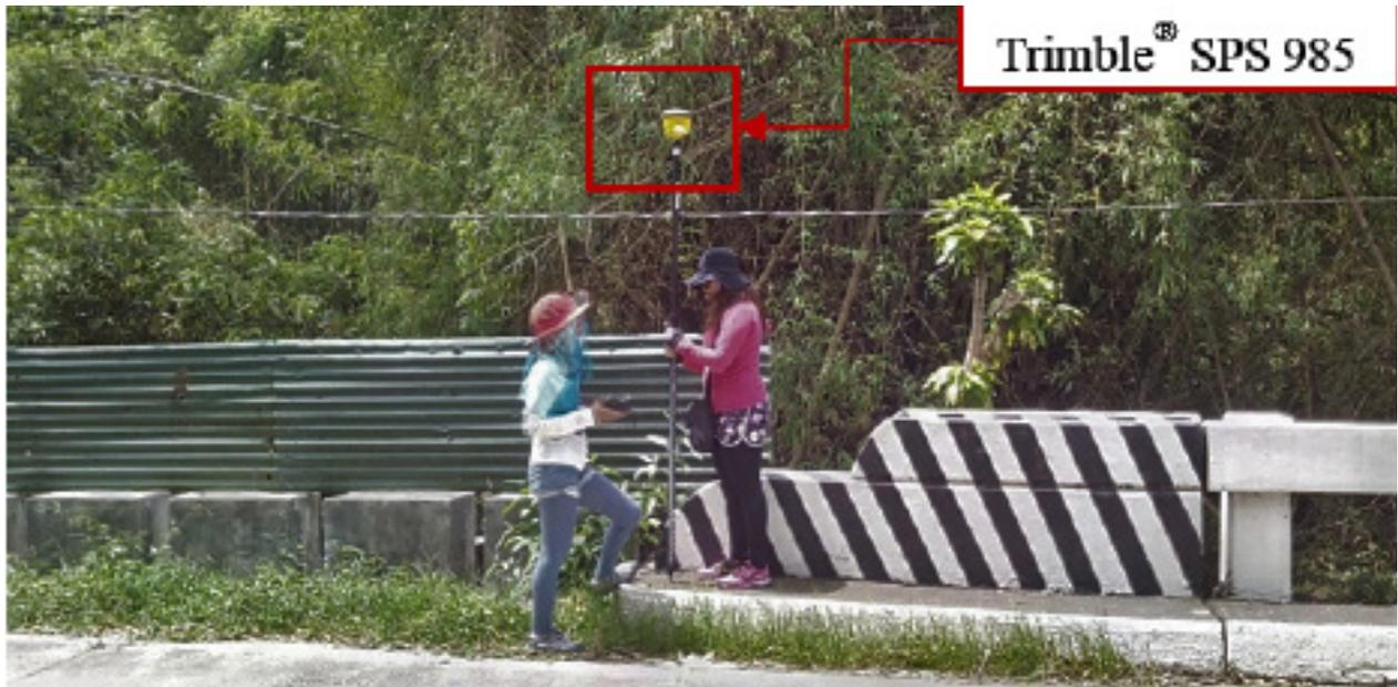
Figure 31. Bridge As-Built Survey using PPK Technique.
