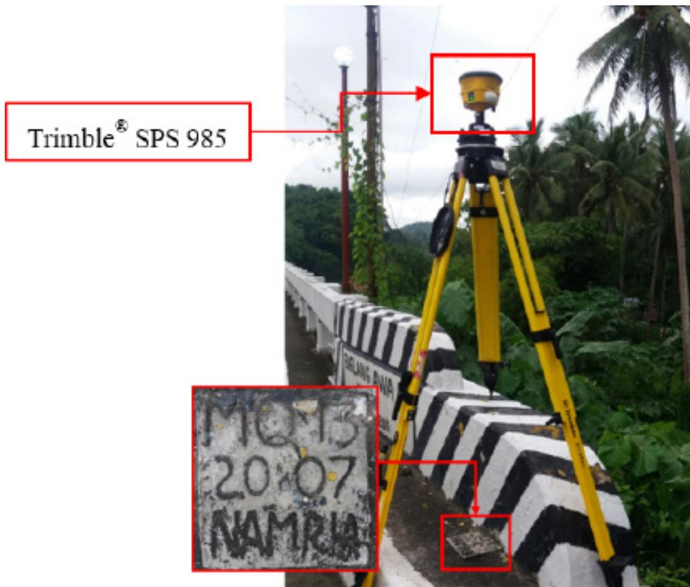
Figure 28. GNSS receiver setup, Trimble® SPS 985, at MQ-13 located at the approach of Biglang-Awa Bridge, Brgy. Mataas na Bayan, Boac, Marinduque
