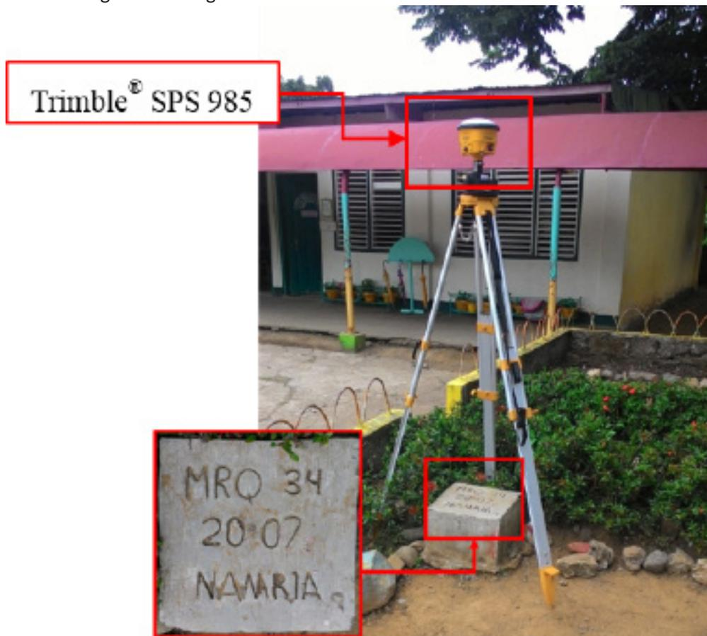
Figure 27. GNSS base set up, Trimble® SPS 985, at MRQ-34 located near the Rizal statue inside Makapuyat Elementary School in Brgy. Napo, Sta. Cruz, Marinduque
