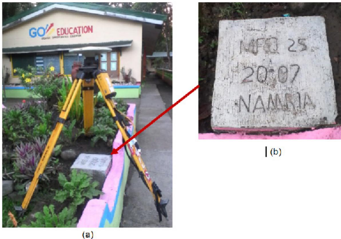
Figure 3. GPS set-up over MRQ-25 at the top of the plant box near the gate of Tugos Elementary School, Barangay Tugos, Boac, Marinduque (a) and NAMRIA reference point MRQ-25 (b) as recovered by the field team.
