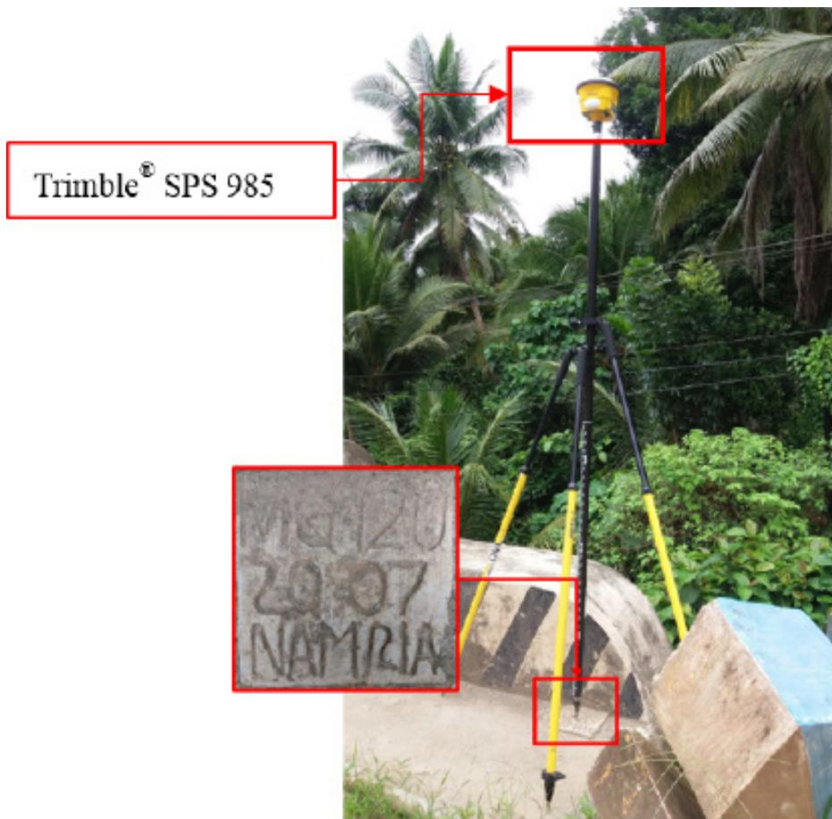
Figure 29. GNSS receiver setup, Trimble® SPS 985, at MQ-120 located at the approach Mangamnan Bridge, Brgy. Butansapa, Mogpong, Marinduque
