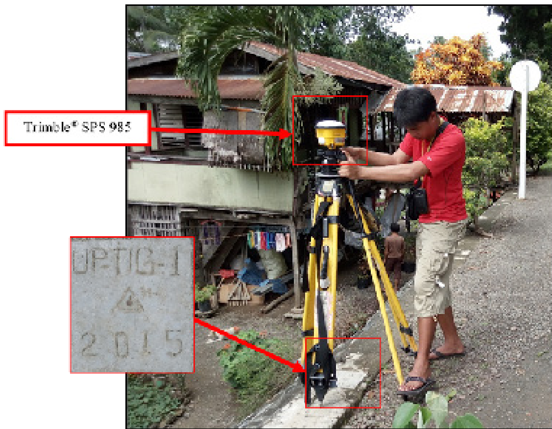
Figure 32. GNSS receiver set up, Trimble® SPS 985, at UP_TIG-1, located at the approach of Tigaplan Bridge in Brgy. Tigaplan, Brookes Point, Province of Palawan
