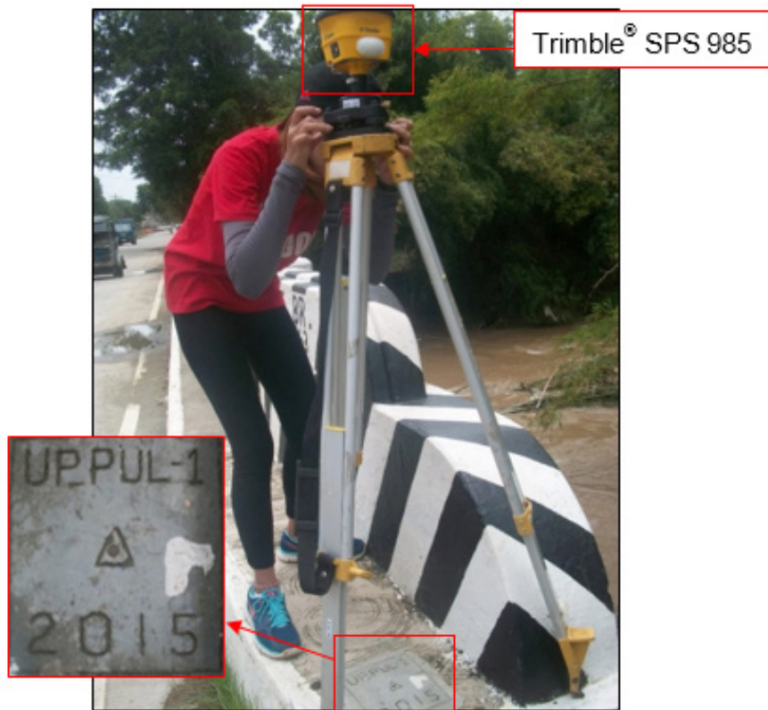
Figure 31. GNSS receiver set up, Trimble® SPS 985, at UP_PUL-1, located at the approach of Pulot Bridge, In Brgy. Pulot Shore, Sofronio Española, Province of Palawan
