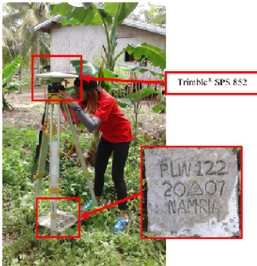
Figure 28. GNSS base set up, Trimble® SPS 852, at PLW-122, located in an open lot beside the house of Ms. Liza Jamili in Brgy. Calasaguen, Brookes Point, Province of Palawan
