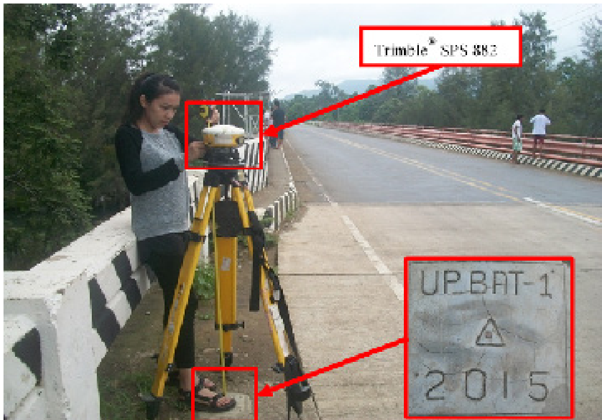
Figure 30. GNSS receiver set up, Trimble® SPS 882, at UP_BAT-1, located near the approach of Batangbatang Bridge in Brgy. Princesa Urduja, Narra, Province of Palawan
