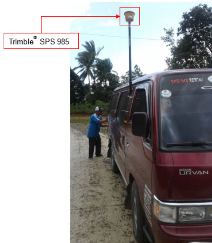
Figure 39. Validation points acquisition survey set-up for Tigaplan River
