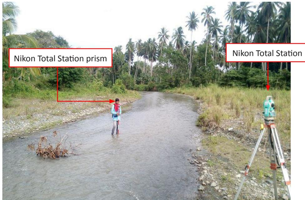
Figure 44. Manual bathymetric survey of ABSD at Bitanayan River using Nikon Total Station
