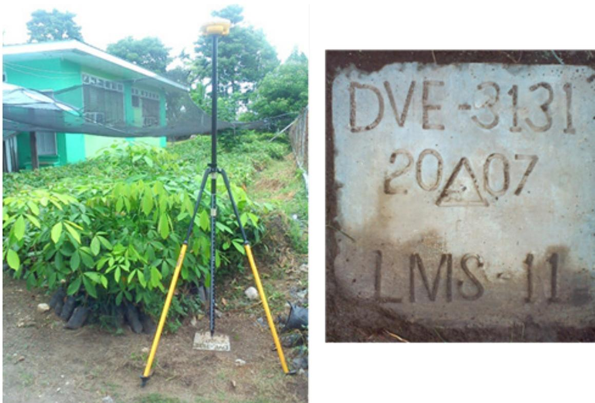
Figure 4. GPS set-up over DVE-3131 located inside the premises of DENR CENRO Office (a) and NAMRIA reference point DVE-3131 (b) as recovered by the field team.
