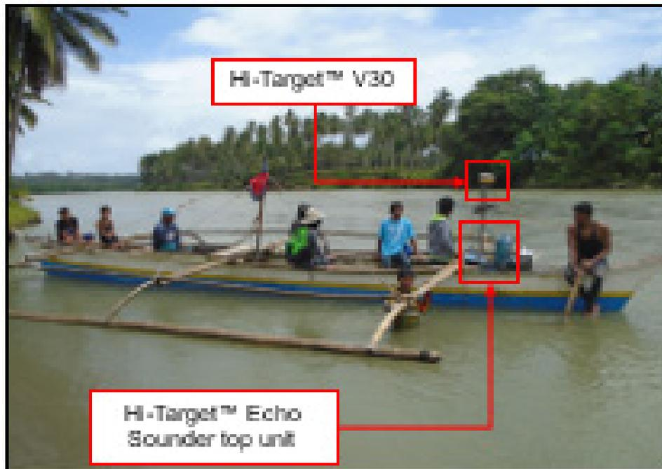
Figure 43 Bathymetric survey of ABSD at Caraga River using Hi-Target™ Echo Sounder
