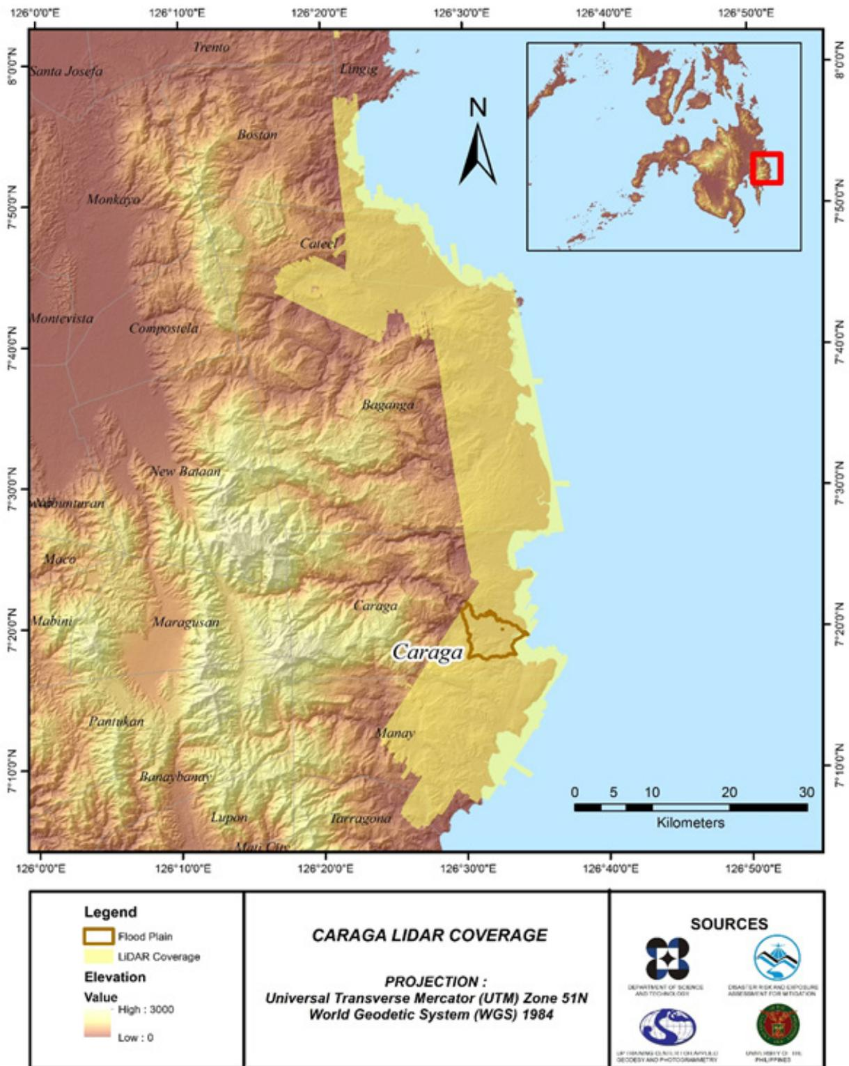
Figure 9. Actual LiDAR survey coverage for Caraga floodplain.
