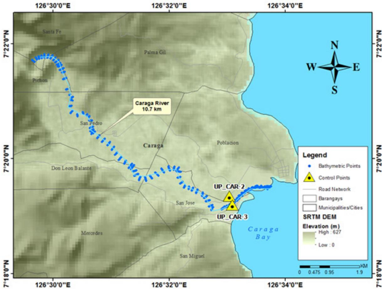
Figure 46. Bathymetric survey of Caraga River
