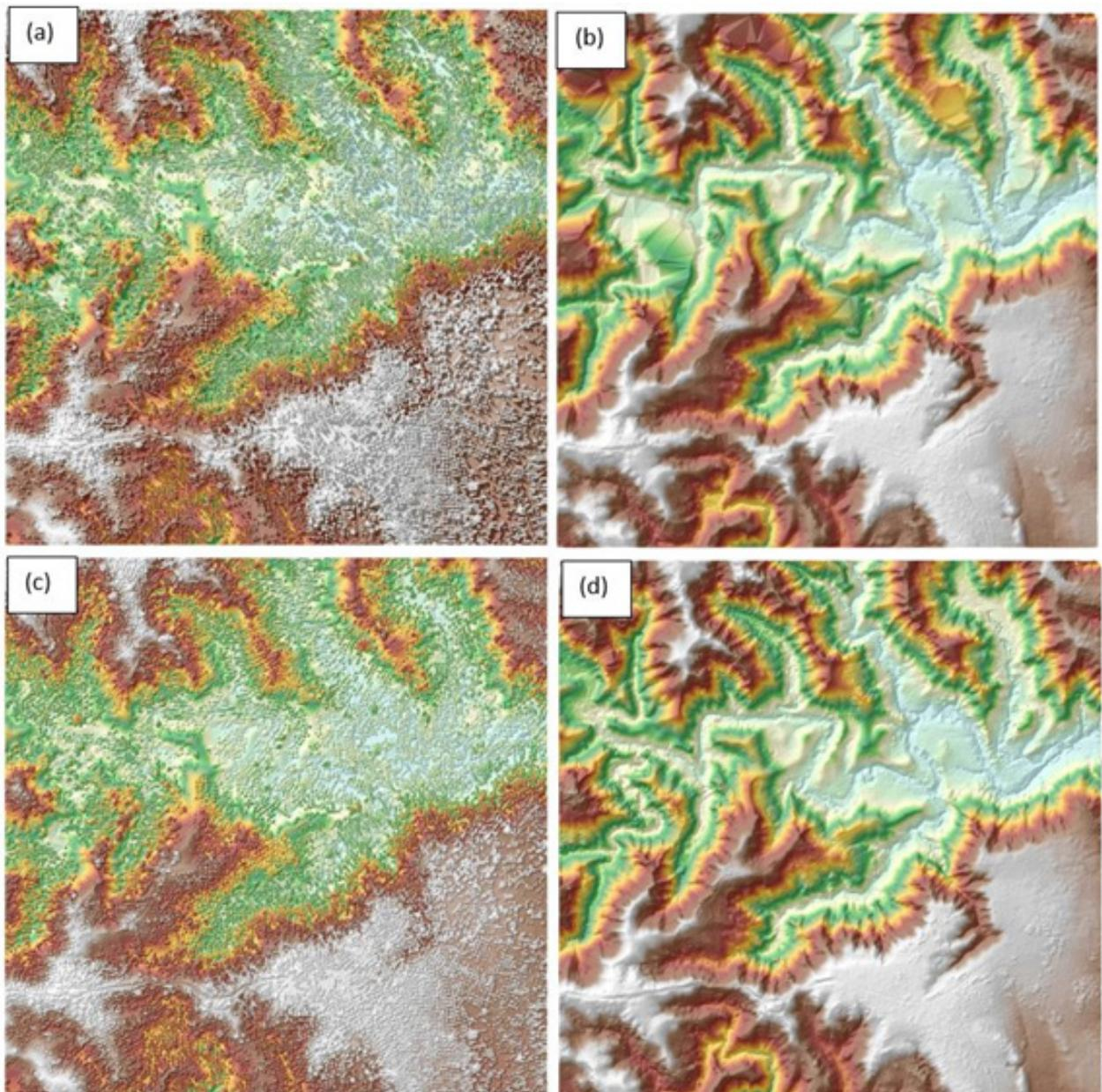
Figure 21. The production of last return DSM (a) and DTM (b), first return DSM (c) and secondary DTM (d) in some portion of Caraga floodplain.
