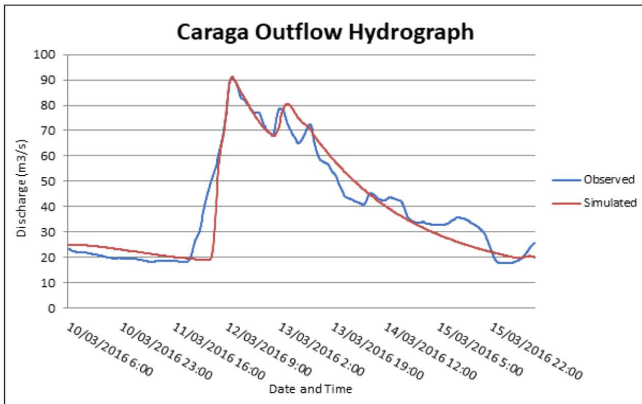
Figure 62. Outflow Hydrograph of Caraga produced by the HEC-HMS model compared with observed outflow
