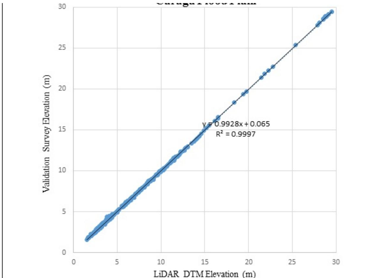
Figure 24. Correlation plot between validation survey points and LiDAR data.
