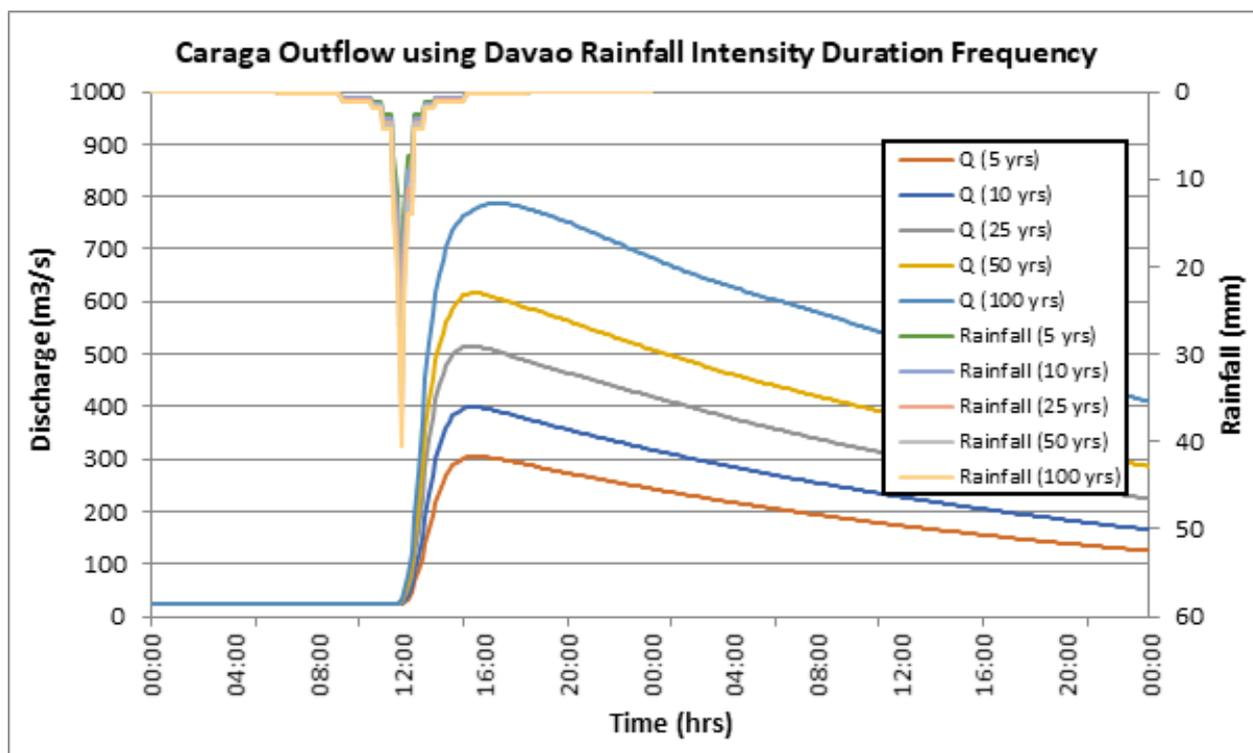
Figure 63. Outflow hydrograph at Caraga Station generated using the Davao RIDF simulated in HEC-HMS.
