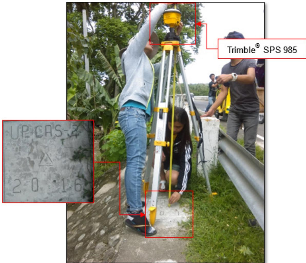
Figure 33 GNSS receiver set up, Trimble® SPS 985, at UP\_CAS-2, located beside the railings near Casaunan Bridge in Brgy. Zaragosa, Manay, Davao Oriental
