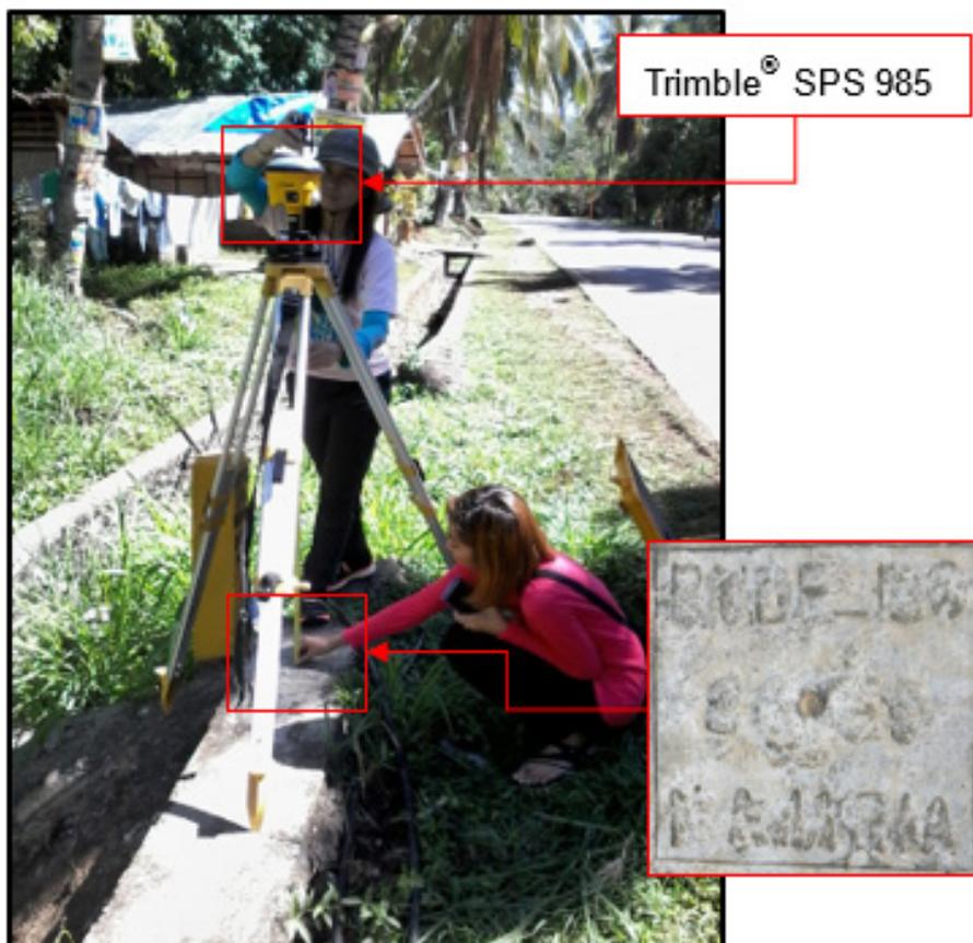
Figure 31 GNSS receiver set up, Trimble® SPS 985, at DE-130, located on top of a culvert at the side of the road in Brgy. San Ignacio, Municipality of Manay, Province of Davao Oriental
