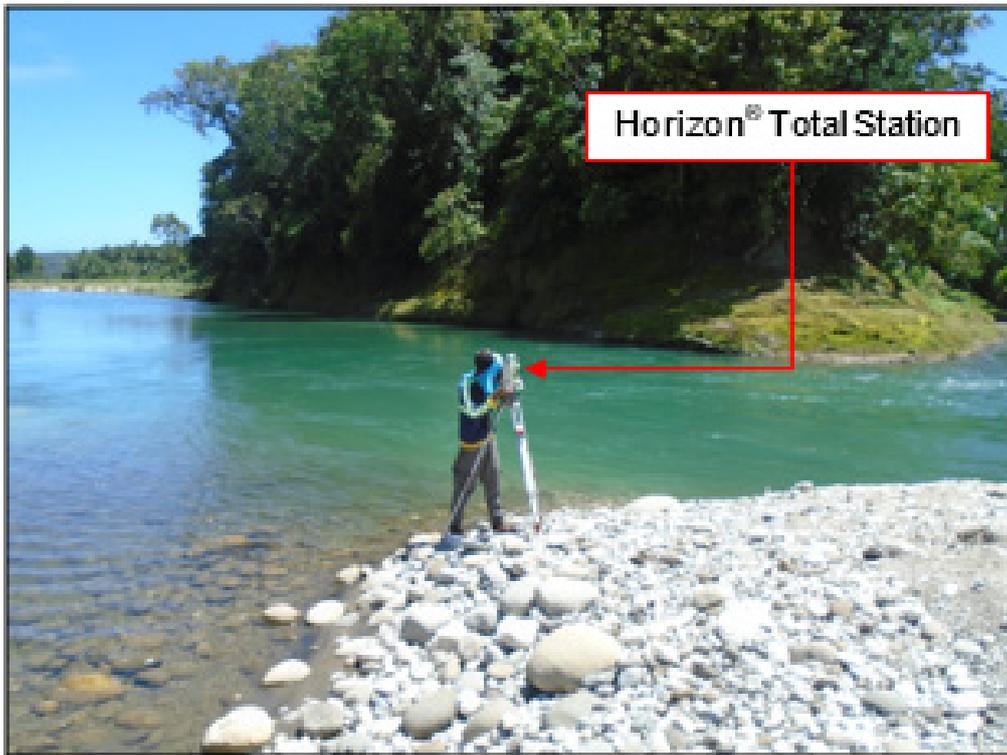
Figure 44 Manual bathymetric survey of ABSD at Caraga River using Horizon® Total Station
