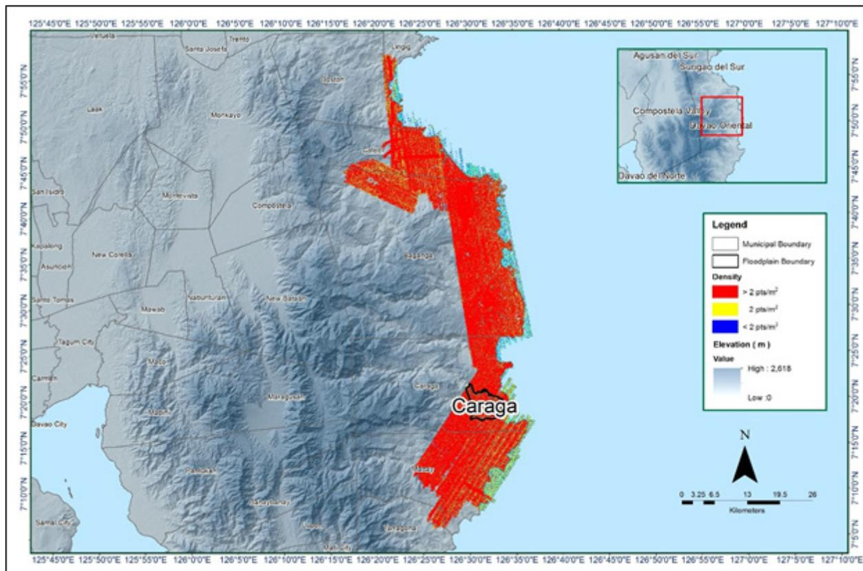
Figure 16. Density map of merged LiDAR data for Caraga floodplain.
