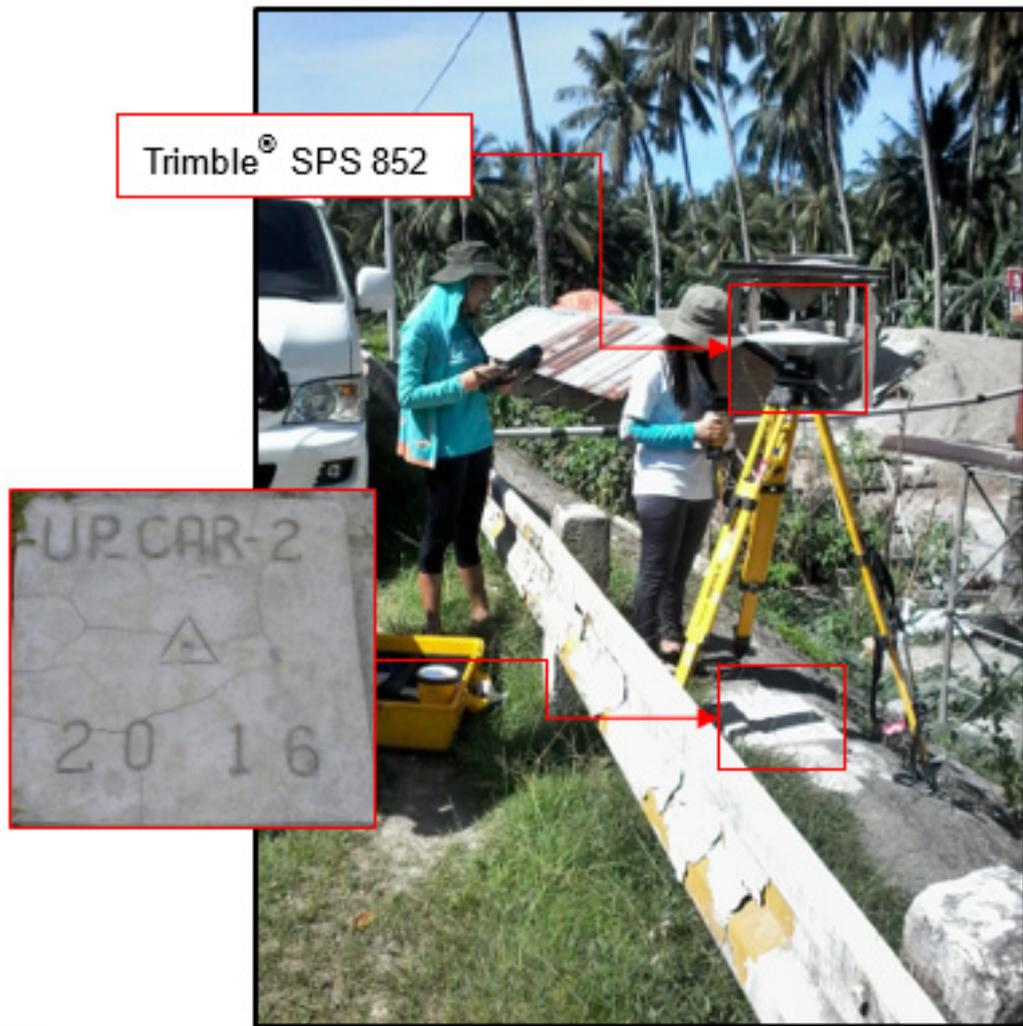
Figure 32 GNSS receiver set up, Trimble® SPS 852, at UP\_CAR-2, located at the side of the railing near Caraga Bridge in Brgy. Poblacion, Caraga, Davao Oriental
