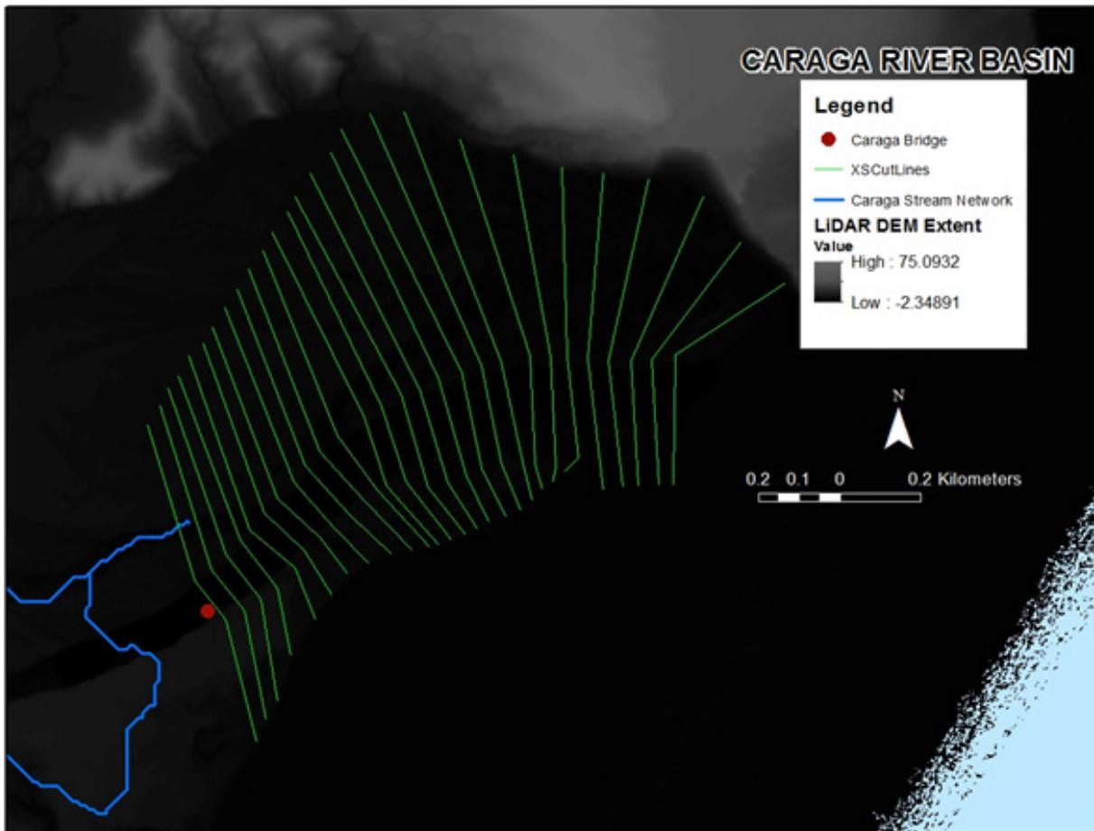
Figure 60. River cross-section of Caraga River generated through Arcmap HEC GeoRAS tool
