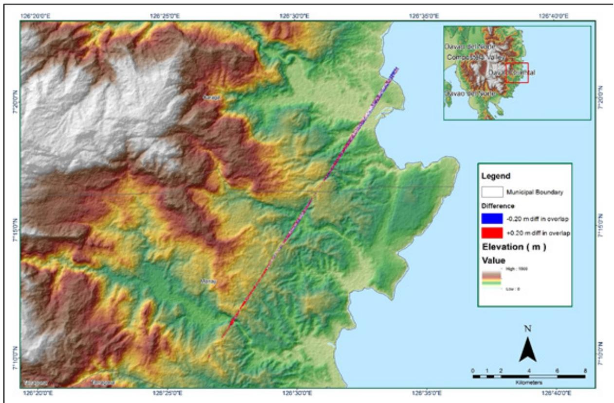
Elevation difference between flight lines
