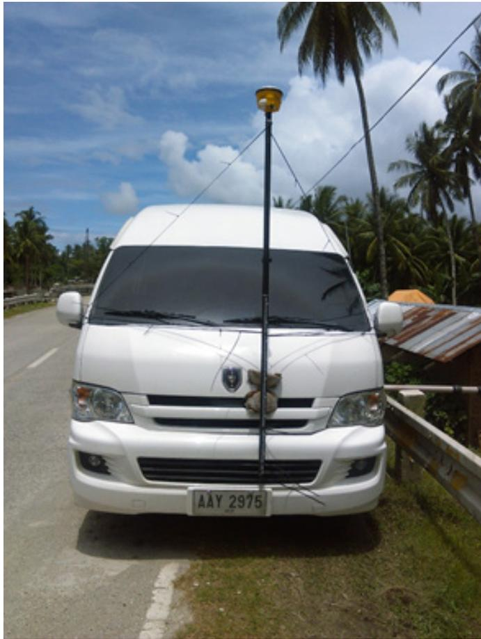
Figure 41. Validation points acquisition survey set-up for Caraga River
