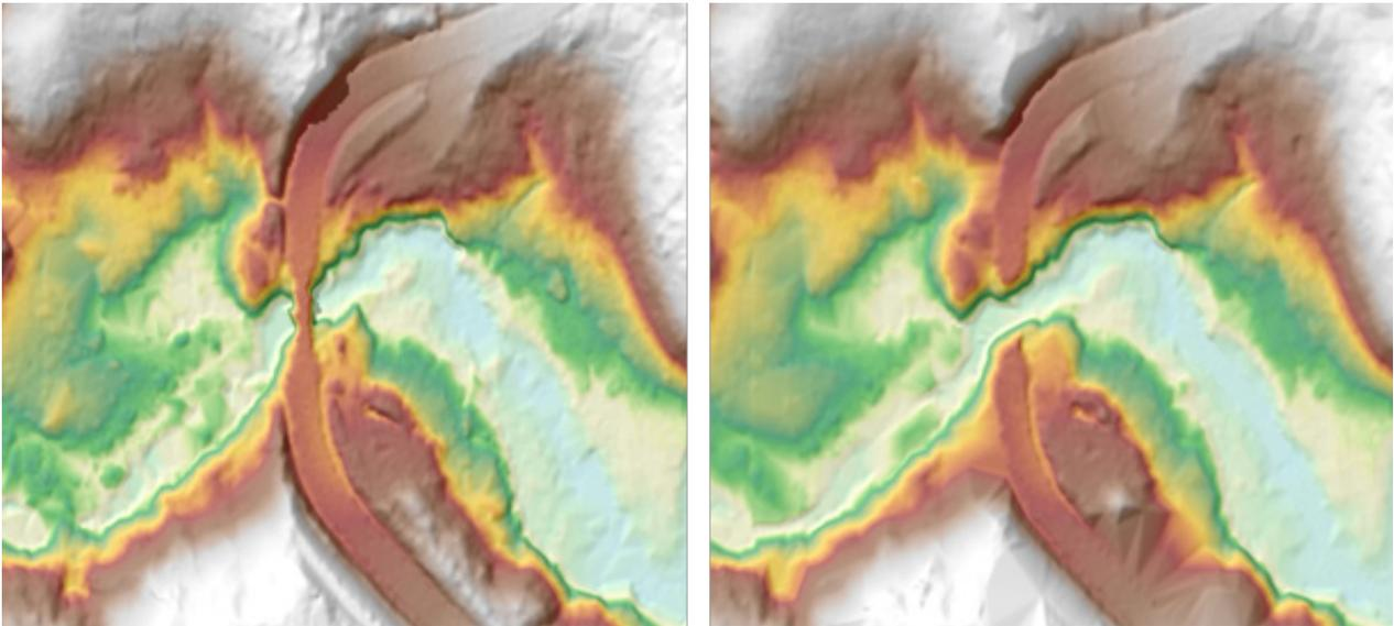
Figure 22. Portions in the DTM of Caraga Floodplain – a bridge before (a) and after (b) manual editing
