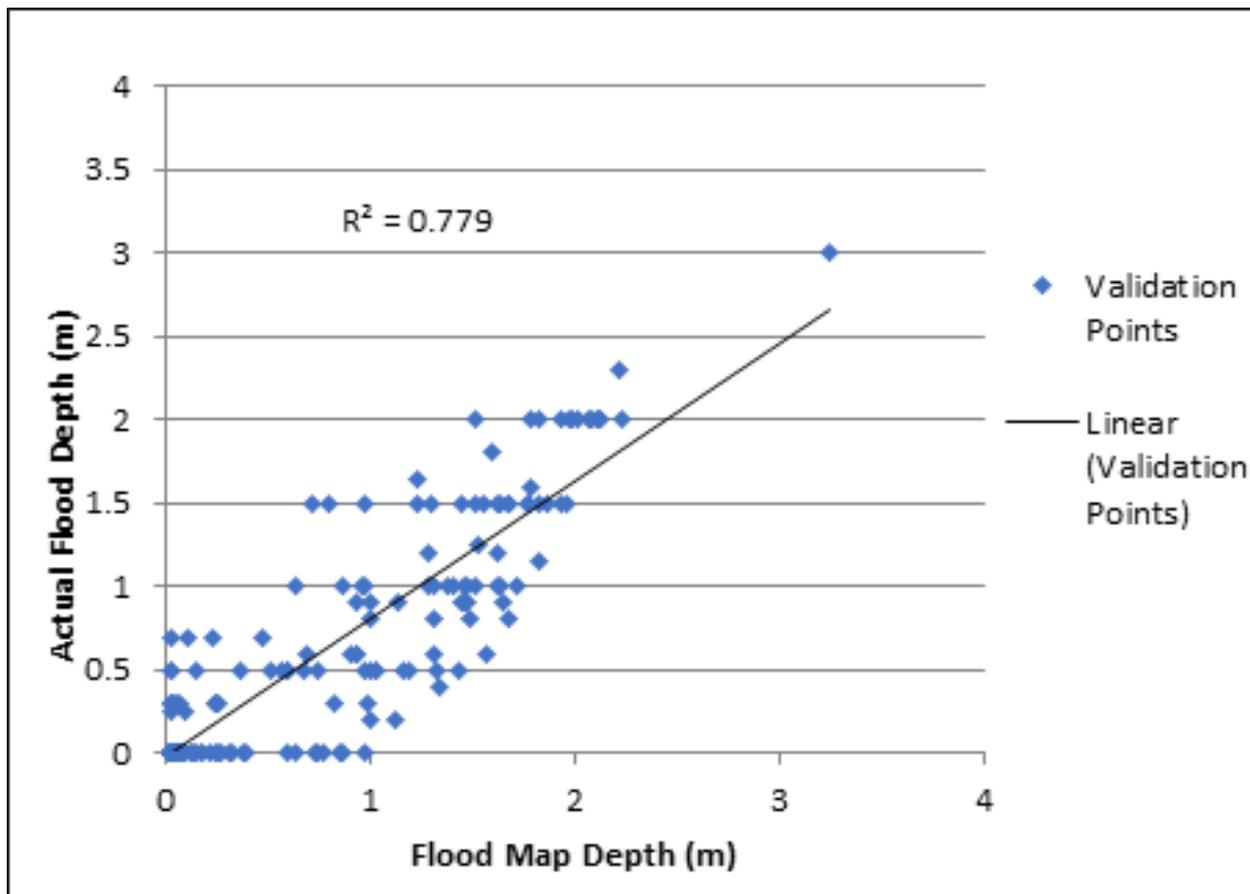
Figure 76. Flood Map Depth vs Actual Flood Depth for Caraga
