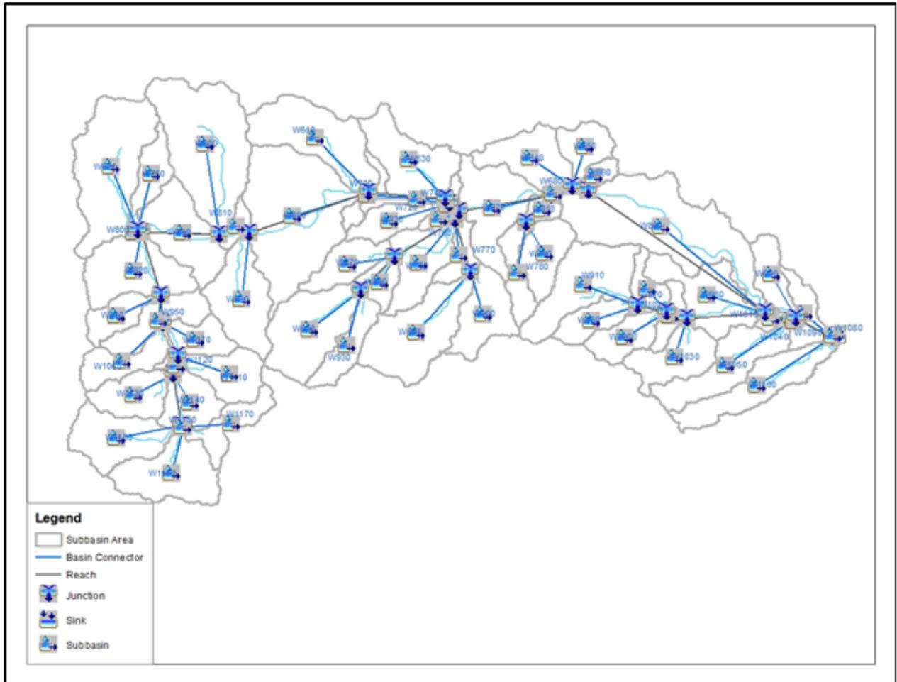
Figure 59. The Caraga river basin model generated using HEC-HMS.
