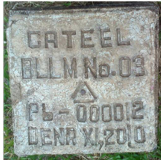
Figure 8. GPS set-up over CATEEL BLLM-03 located inside the compound of San Rafael Elementary School (a) and NAMRIA reference point CATEEL BLLM-03 (b) as recovered by the field team.
