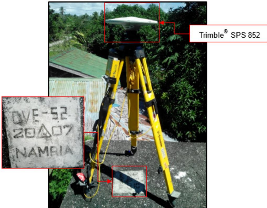
Figure 30 GNSS base set up, Trimble® SPS 852, at DVE-52, located on top of a water reservoir inside the grounds of the barangay of Brgy. Holy Cross in Manay, Davao Oriental
