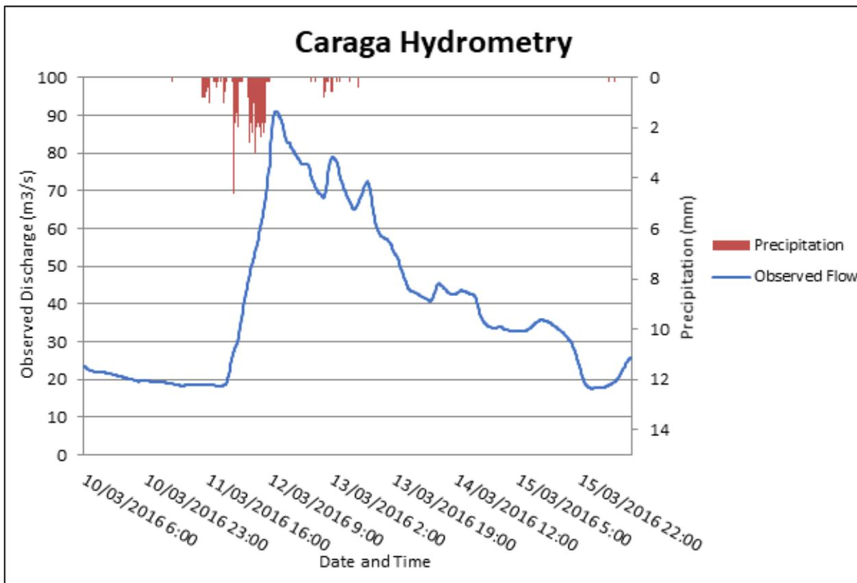
Figure 52. Rainfall and outflow data at Caraga Bridge used for modeling
