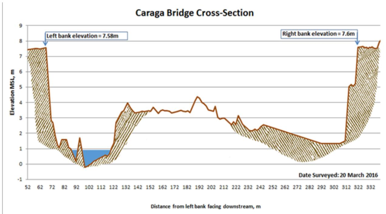
Figure 50. Cross-Section Plot of Caraga Bridge
