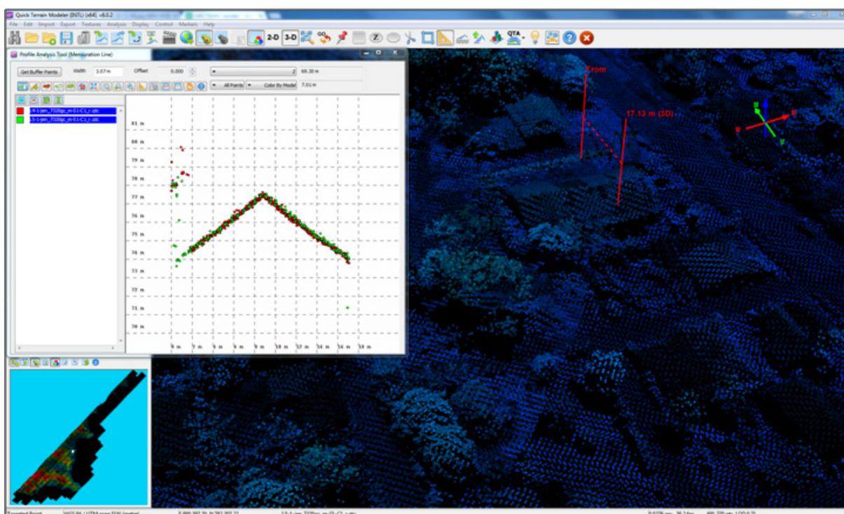
Figure 16. Quality checking for Casauman flight 7320G using the Profile Tool of QT Modeler.
