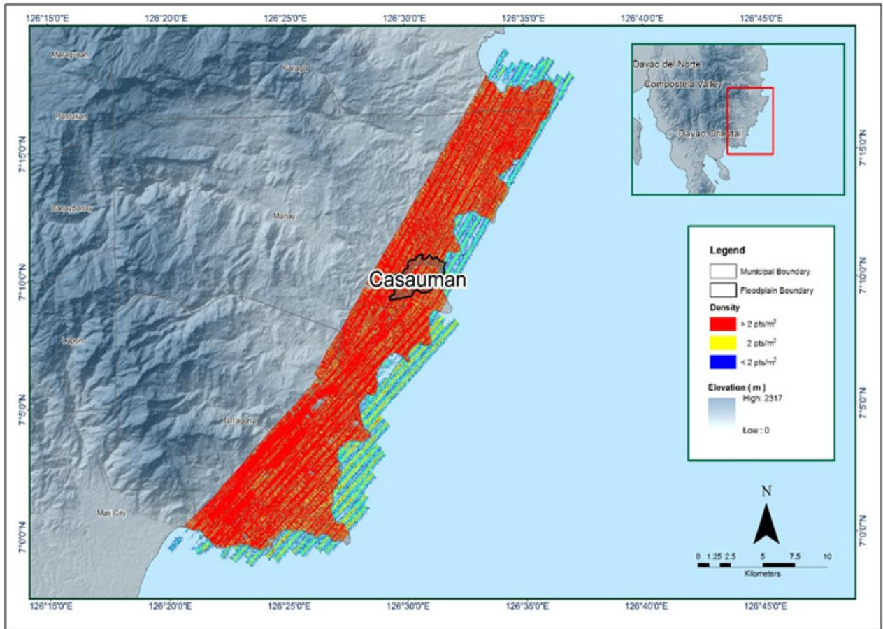
Figure 14. Pulse density map of the merged LiDAR data for Casauman floodplain.
