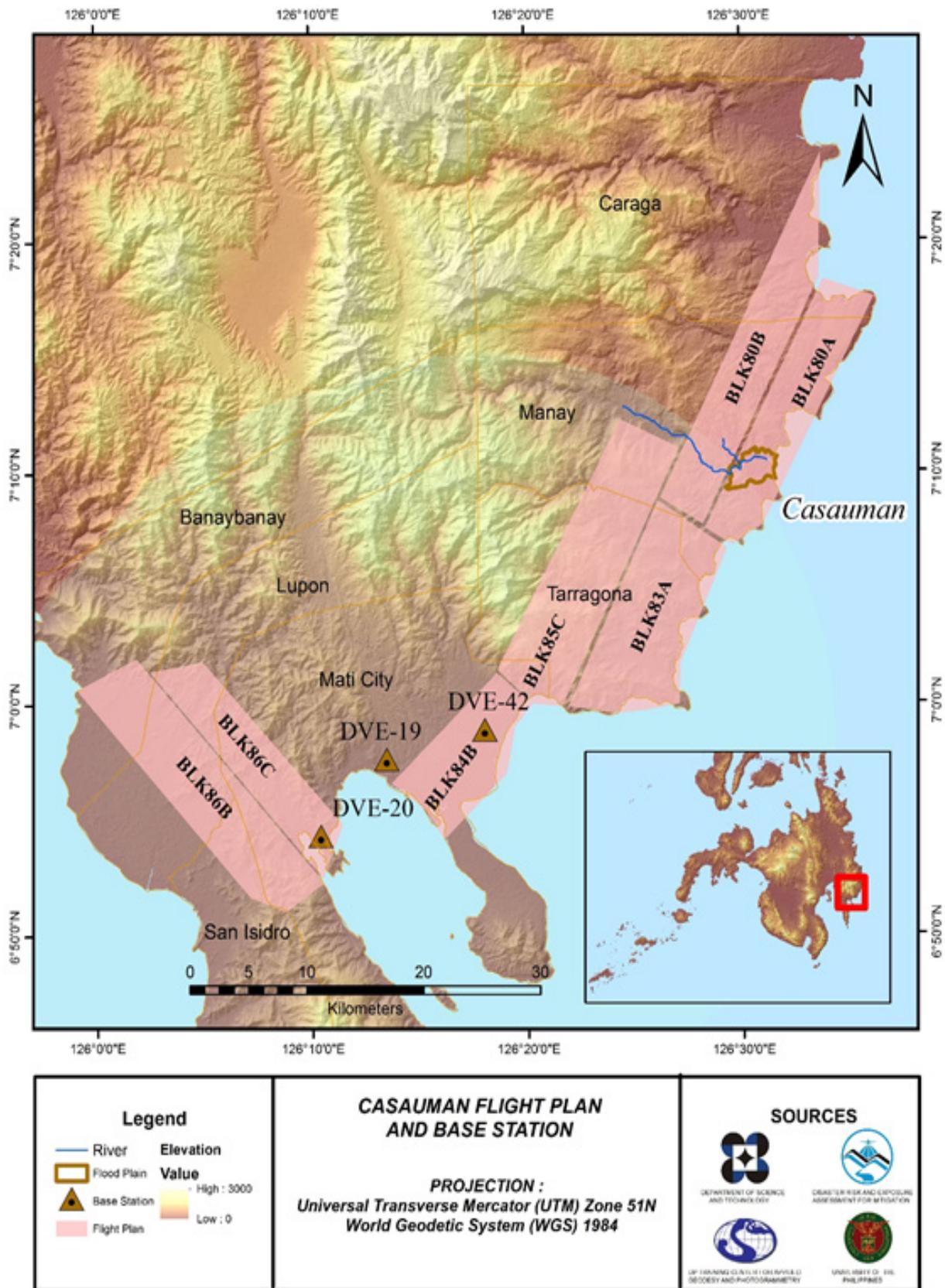
Figure 2. Flight plans and base stations used for Casauman floodplain using Gemini LiDAR system.
