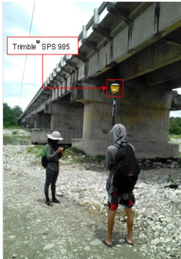
Figure 39. Gathering of random cross-section points along the downstream side of Casauman River.
