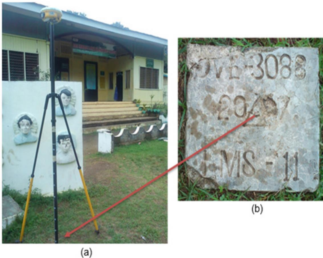
Figure 5. GPS set-up over DVE-3088 located inside Don Enrique Lopez Elementary School (a) and NAMRIA reference point DVE-3088 (b) as recovered by the field team.
