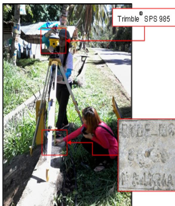
Figure 31. GNSS receiver set up, Trimble® SPS 985, at DE-130, located on top of a culvert at the side of the road in Brgy. San Ignacio, Municipality of Manay, Province of Davao Oriental
