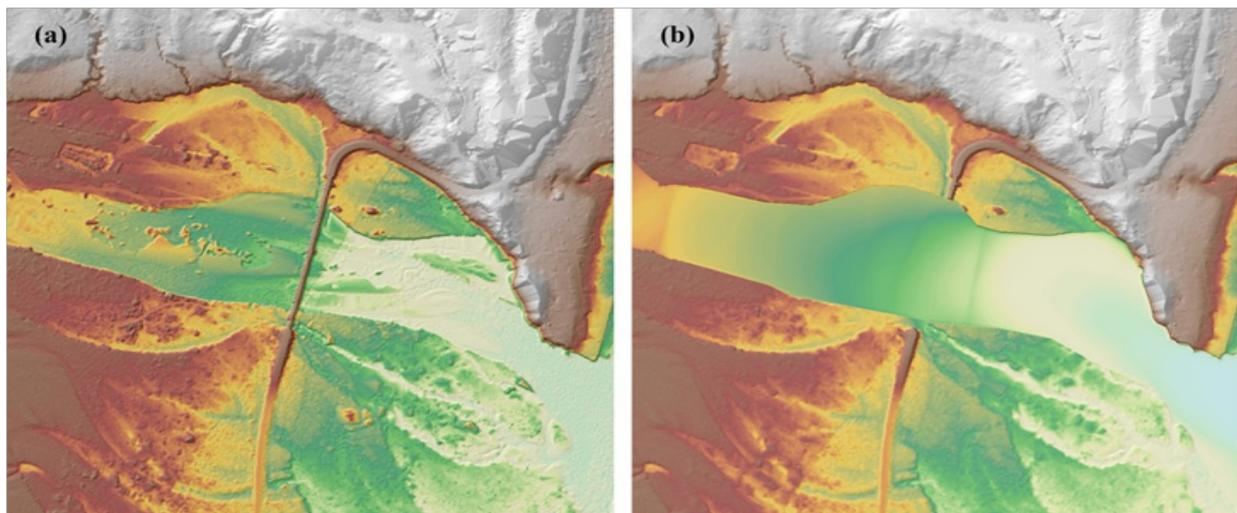
Figure 20. Portions in the DTM of the Casauman Floodplain – a bridge before (a) and after (b) manual editing.
