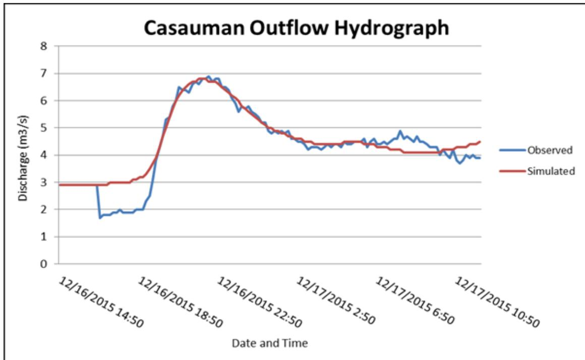
Figure 61. Outflow Hydrograph of Casauman produced by the HEC-HMS model compared with observed outflow.
