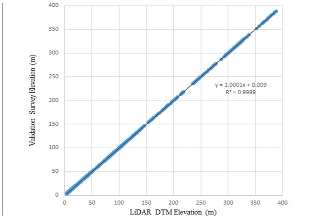
Figure 24. Correlation plot between the validation survey points and the LiDAR data.
