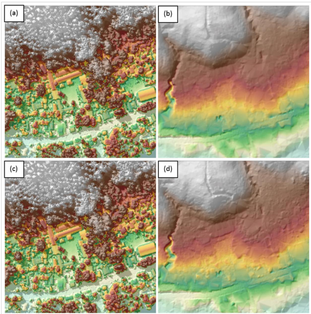
Figure 19. The production of last return DSM (a) and DTM (b), first return DSM (c) and secondary DTM (d) in some portion of Casauman floodplain.
