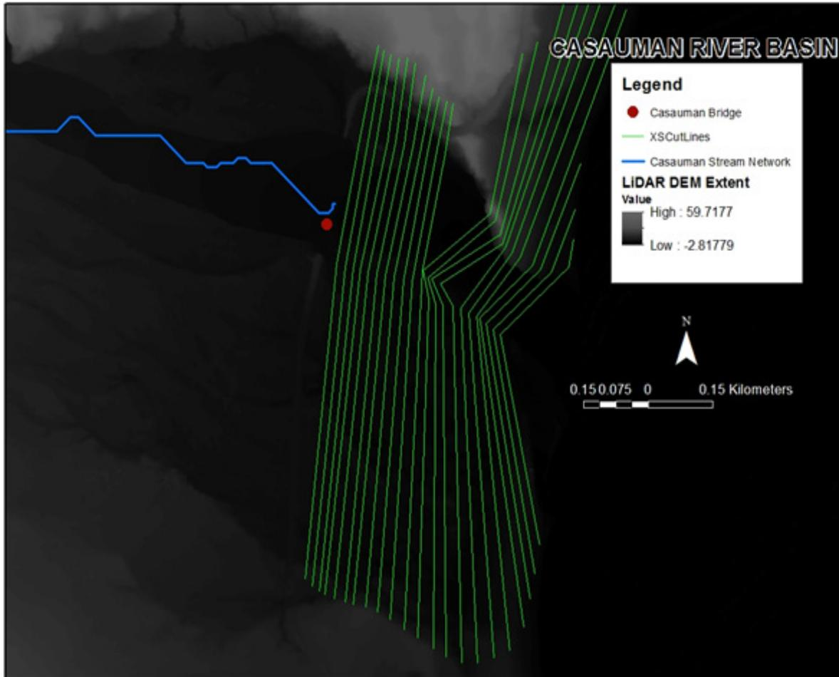
Figure 59. River cross-section of the Casauman River through the ArcMap HEC GeoRas tool.
