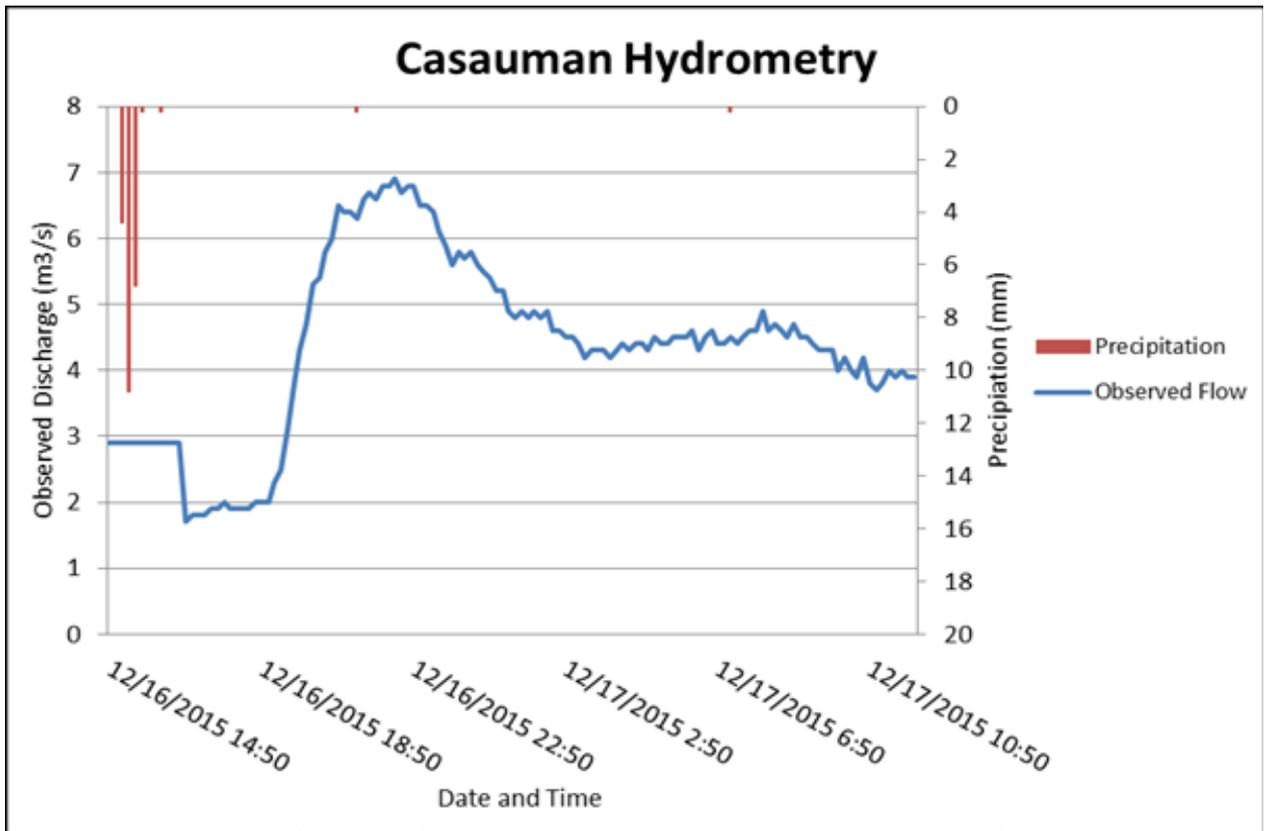
Figure 51. Rainfall and outflow data at Governor Lopez Bridge, which was used for modeling.
