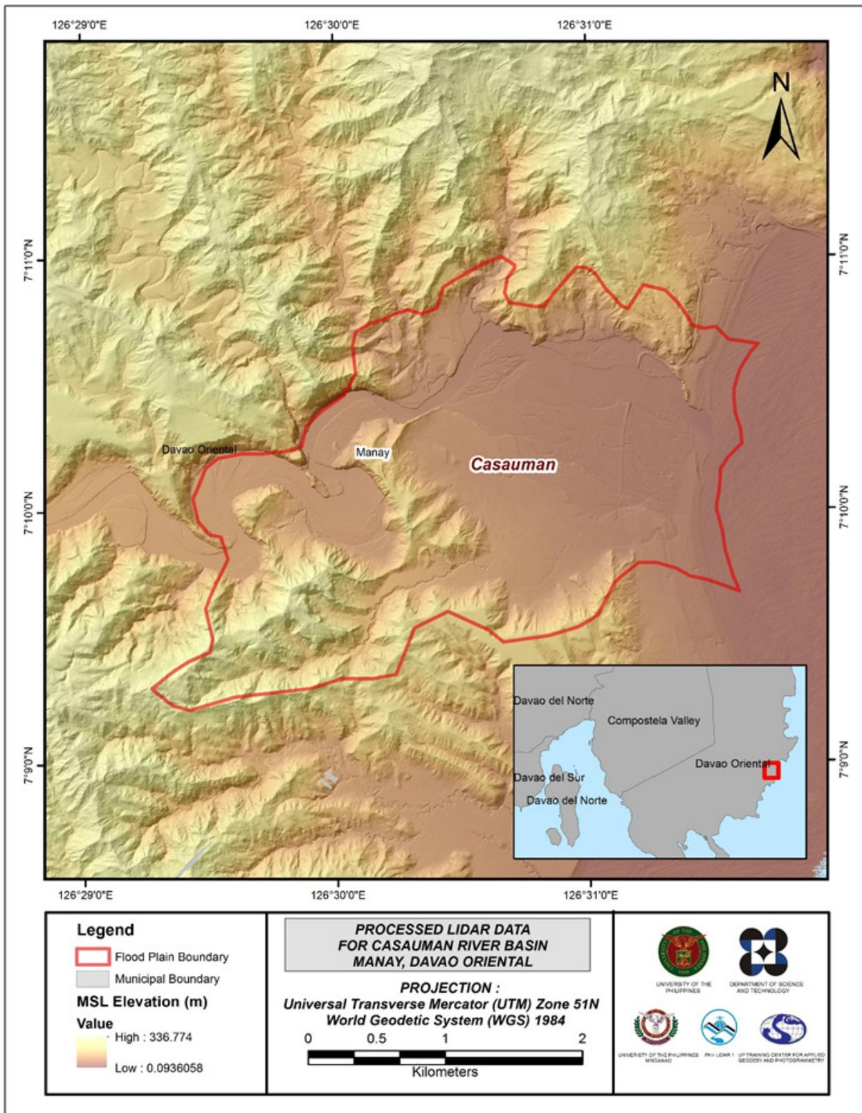
Figure 21. Map of processed LiDAR data for the Casauman Floodplain.
