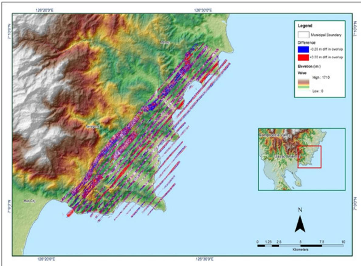
Figure A-8.7 Elevation difference between flight lines
