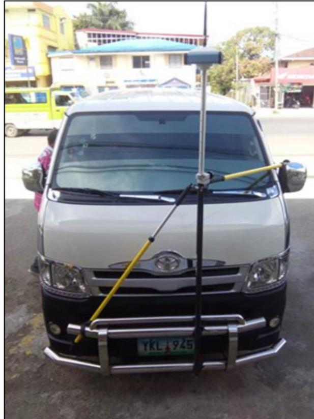
Figure 41. GNSS Receiver South® S86T installed on a vehicle for Ground Validation Survey.
