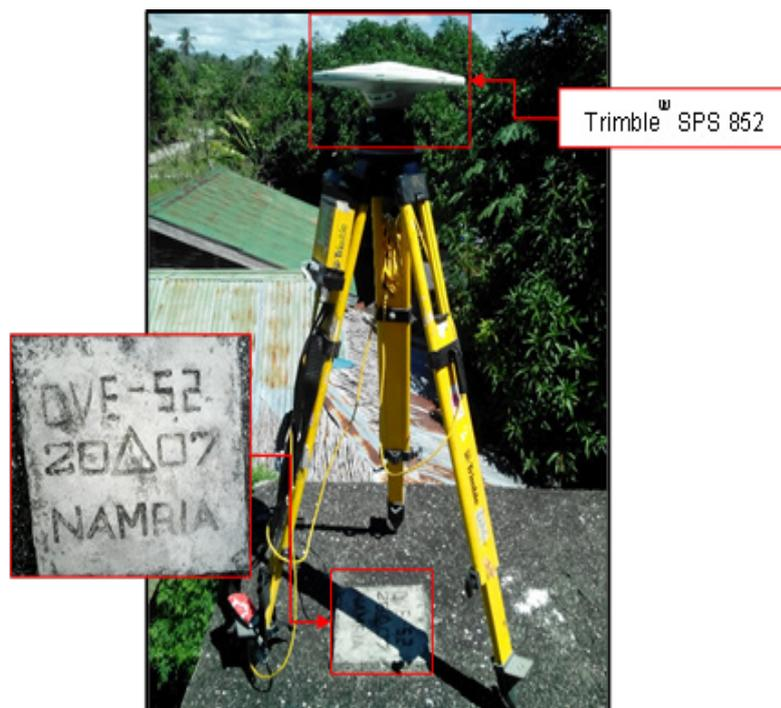
Figure 30. GNSS base set up, Trimble® SPS 852, at DVE-52, located on top of a water reservoir inside the grounds of the barangay of Brgy. Holy Cross in Manay, Davao Oriental
