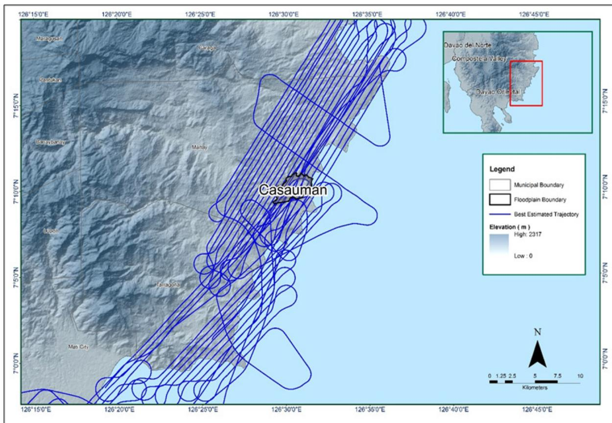
Figure 11. Best Estimated Trajectory of the LiDAR missions conducted over the Casauman Floodplain.
