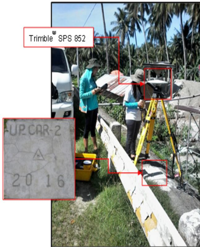
Figure 32. GNSS receiver set up, Trimble® SPS 852, at UP\_CAR-2, located at the side of the railing near Caraga Bridge in Brgy. Poblacion, Caraga, Davao Oriental
