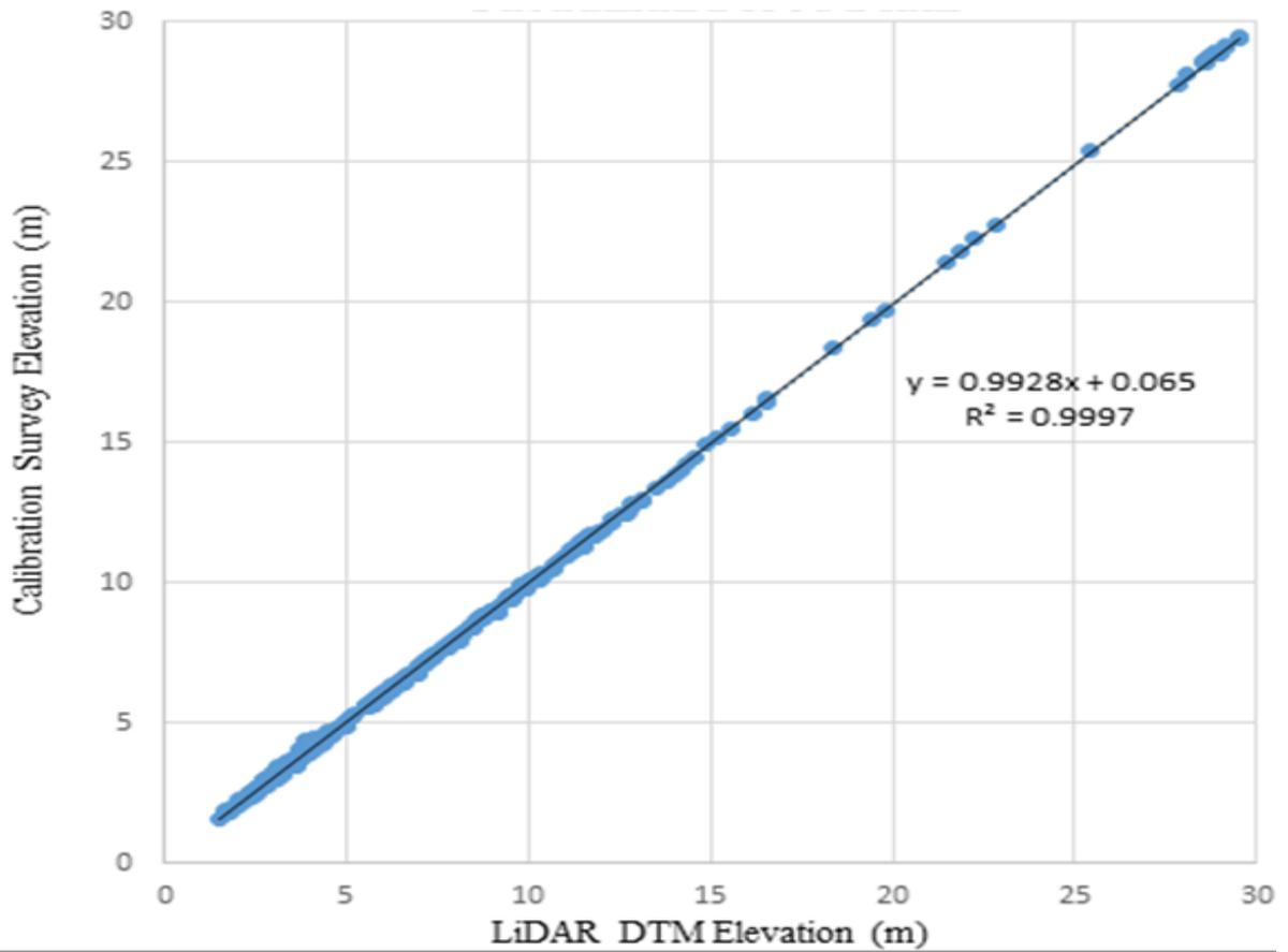
Figure 23. Correlation plot between calibration survey points and LiDAR data.
