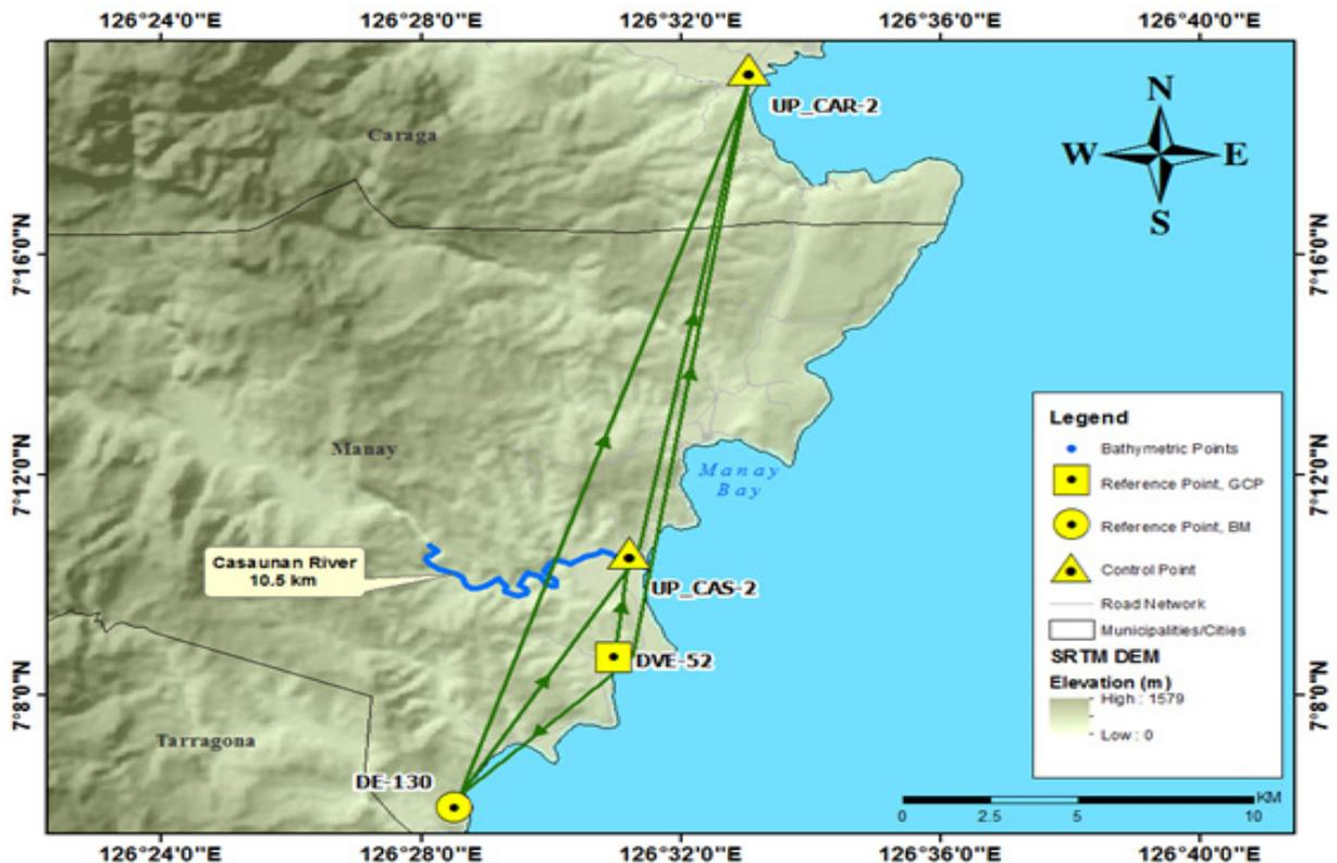
Figure 29. GNSS Network of CASAUMAN Field Survey
