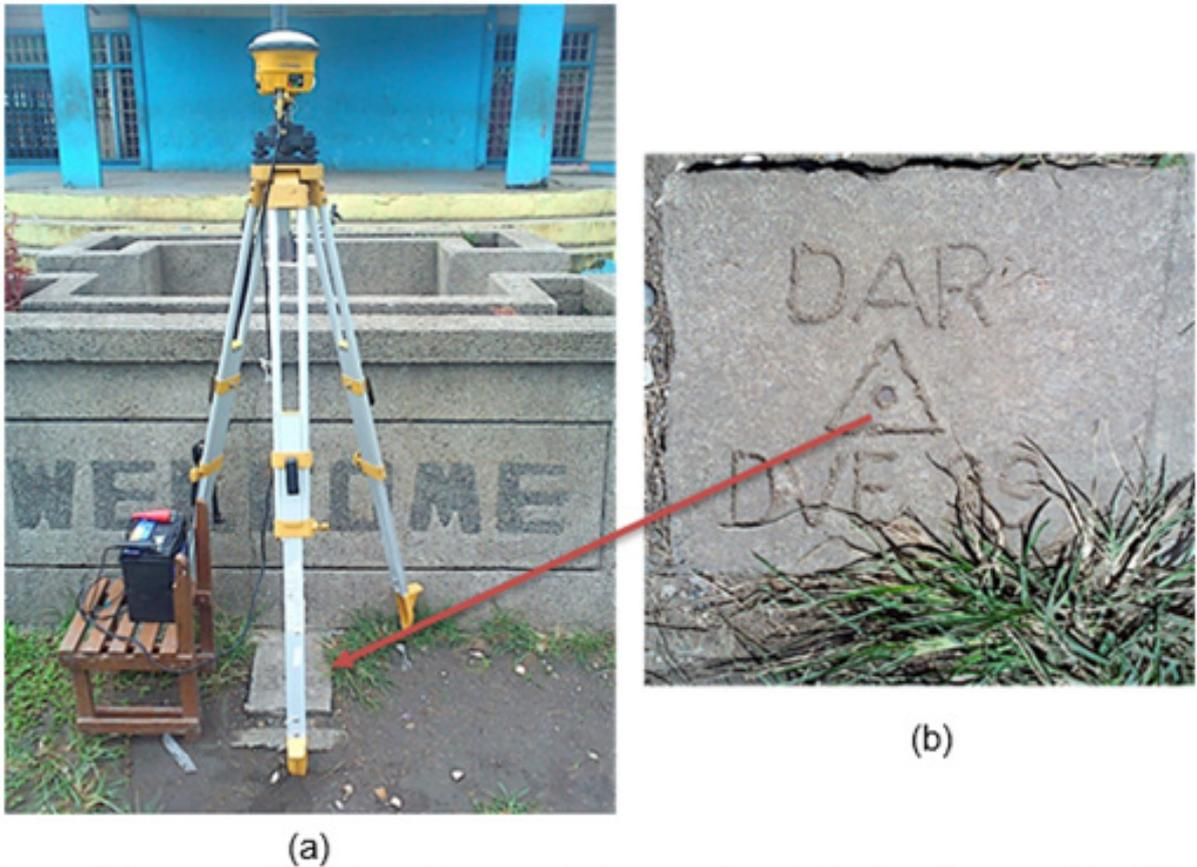
Figure 4. GPS set-up over DVE-19 located in front of the flagpole of Gregorio Moralizon Elementary School II (a) and NAMRIA reference point DVE-19 (b) as recovered by the field team.
