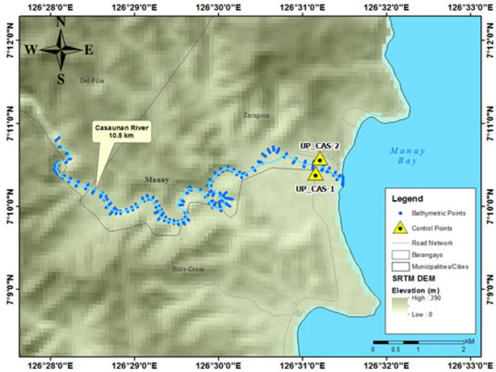
Figure 45. The extent of the Casaunan River Bathymetry Survey.
