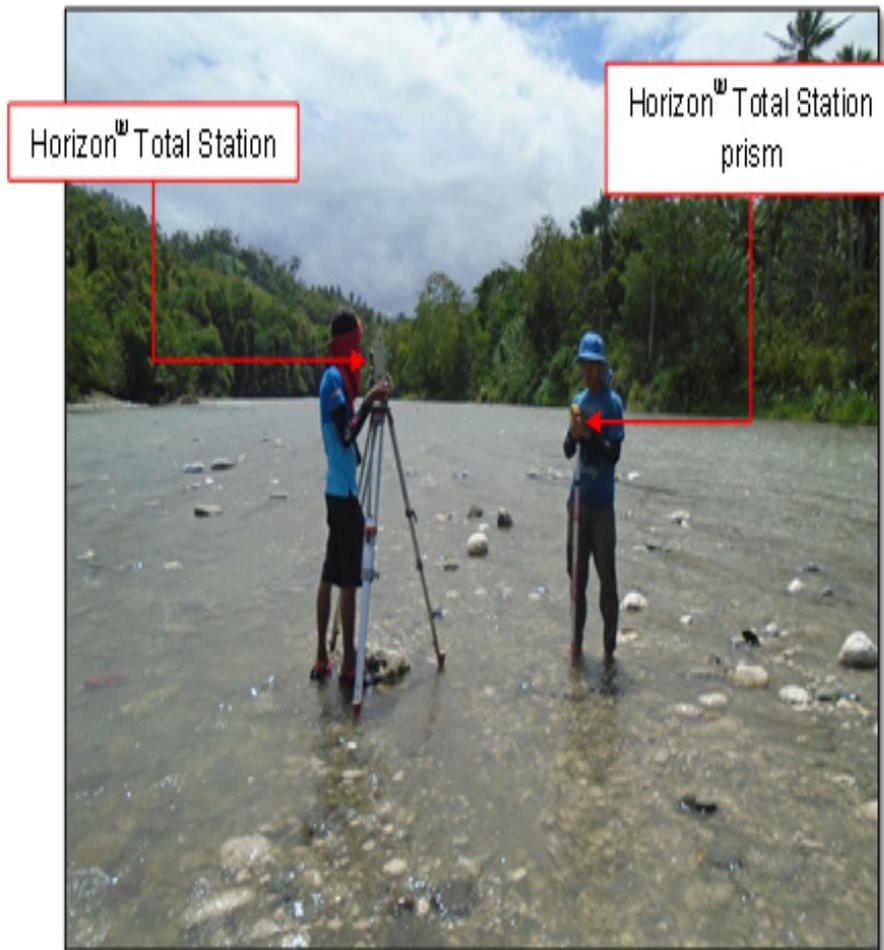
Figure 43. Set up of the bathymetric survey of ABSD at Casauman River using Horizon® Total Stationsurvey
