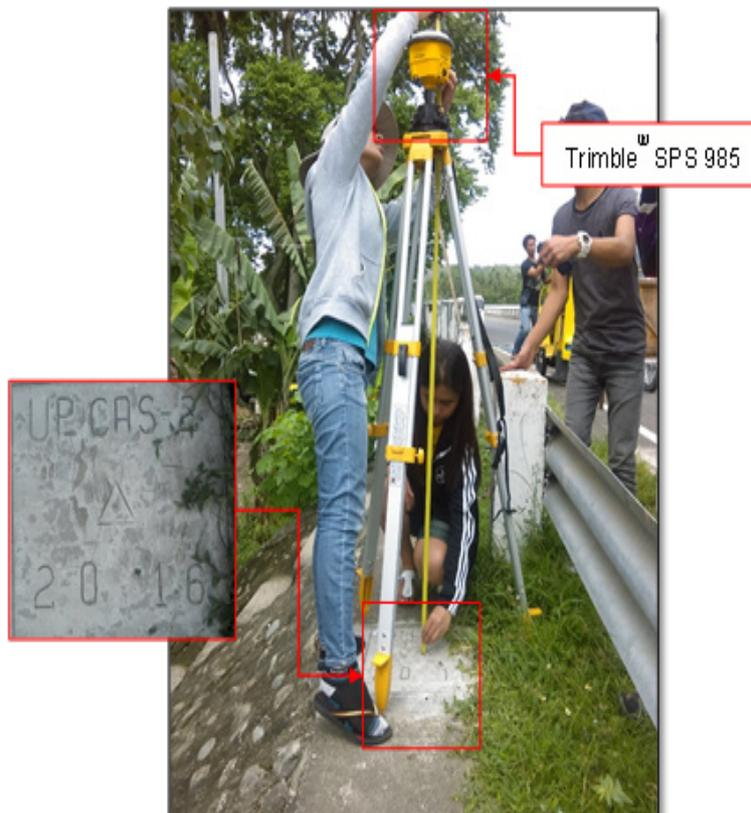
Figure 33. GNSS receiver set up, Trimble® SPS 985, at UP\_CAS-2, located beside the railings near Casauman Bridge in Brgy. Zaragosa, Manay, Davao Oriental
