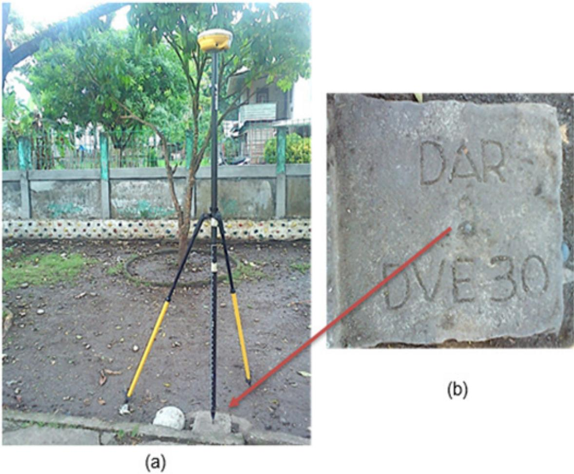
Figure 6. GPS set-up over DVE-20 located inside the premises of Gregorio Moralizon Elementary School I, at the corner side of the basketball court 3 meters from the gate of the school (a) and NAMRIA reference point DVE-20 (b) as recovered by the field team.
