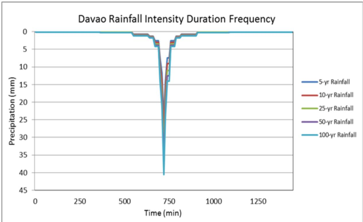
Figure 53. The synthetic storm generated for a 24-hour period rainfall for various return periods
