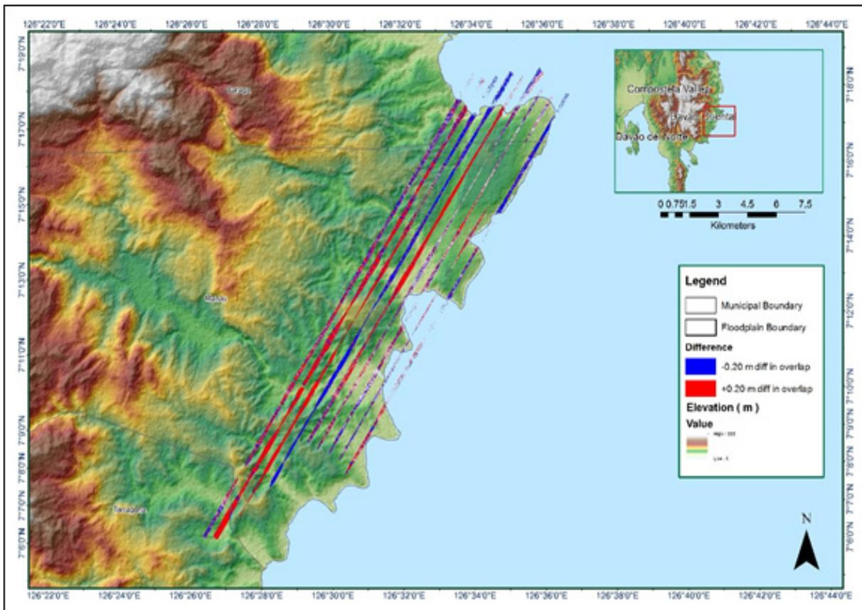
Figure A-8.14 Elevation difference between flight lines
