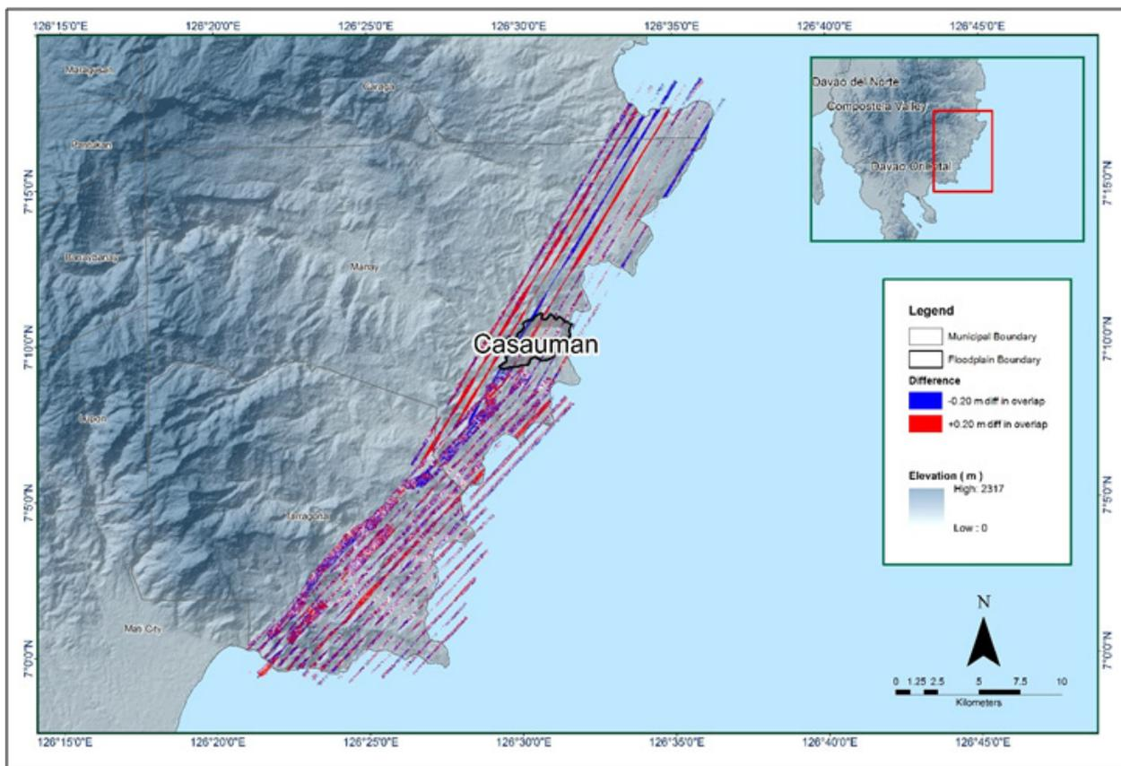
Figure 15. Elevation difference Map between flight lines for the Casauman Floodplain Survey.
