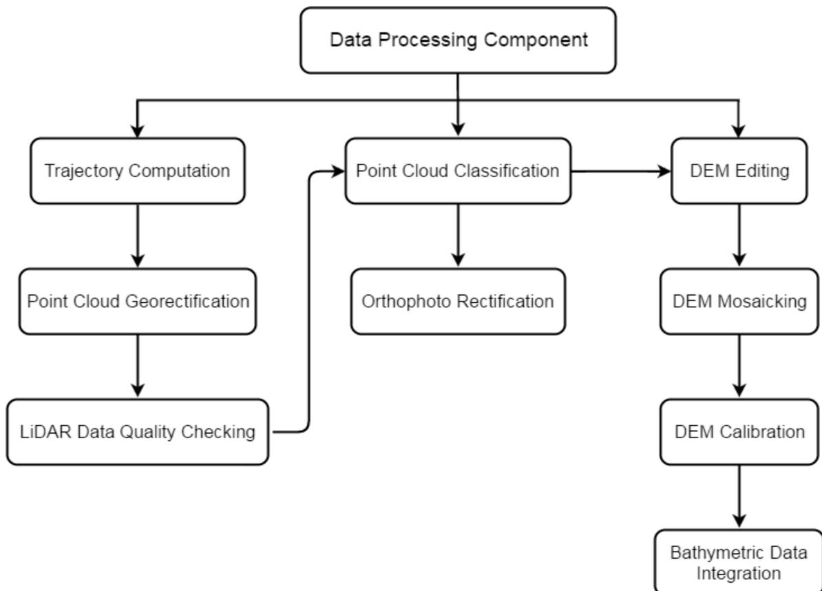
Figure 8. Schematic diagram for the data pre-processing.
