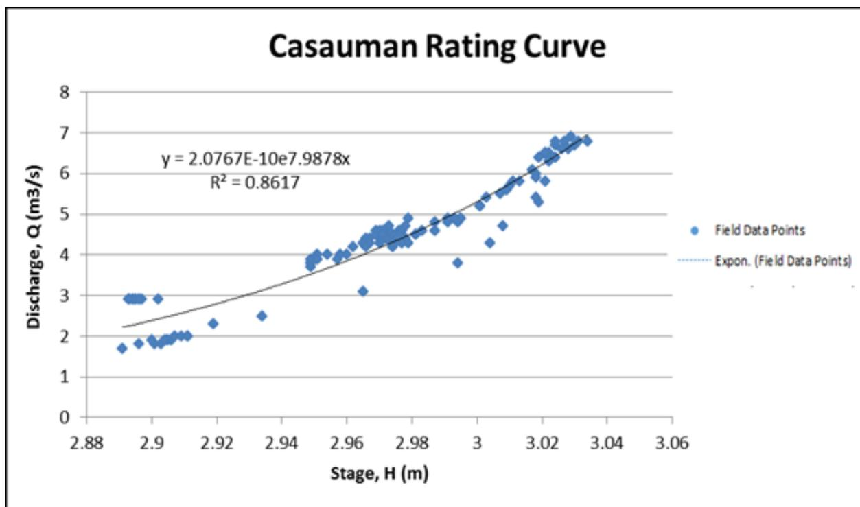
Figure 50. Rating Curve at Polanco Bridge
