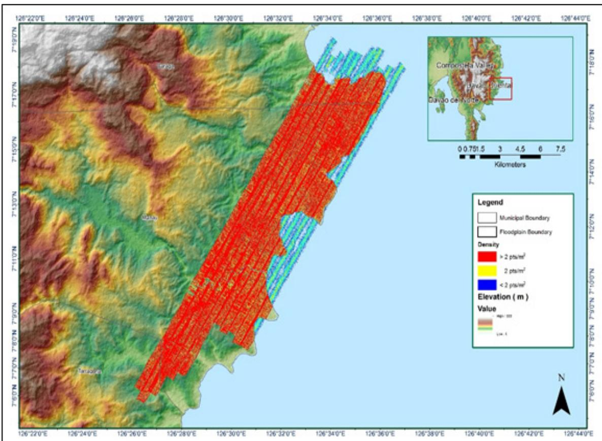
Figure A-8.13 Density map of merged LiDAR data
