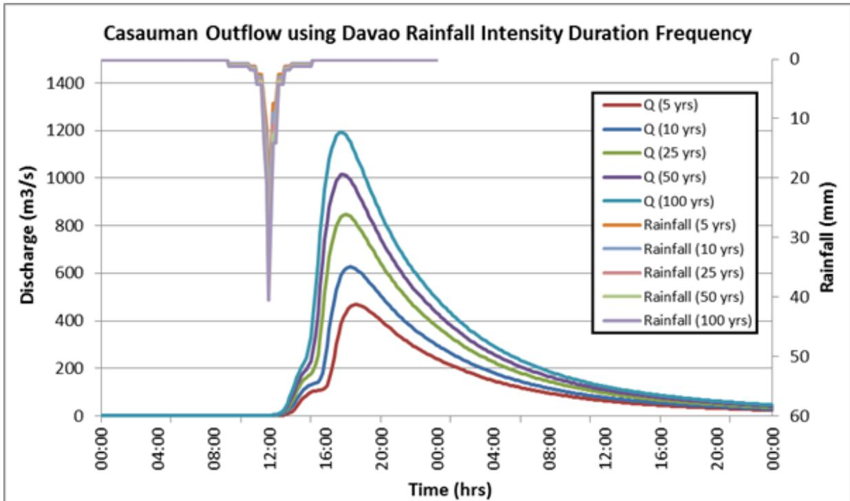
Figure 62. The Outflow hydrograph at the Casauman Station, generated using the Davao RIDF simulated in HEC-HMS.
