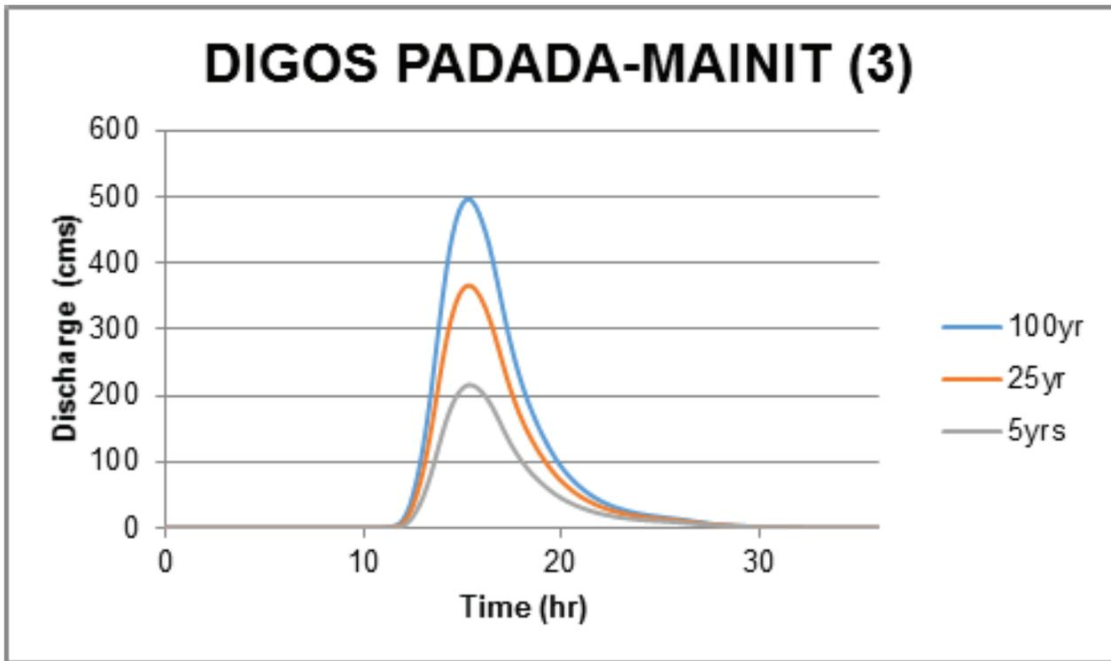
Figure 64. Digos Padada-Mainit river (3) generated discharge using 5-, 25-, and 100-year GenSan rainfall intensity-duration-frequency (RIDF) in HEC-HMS
