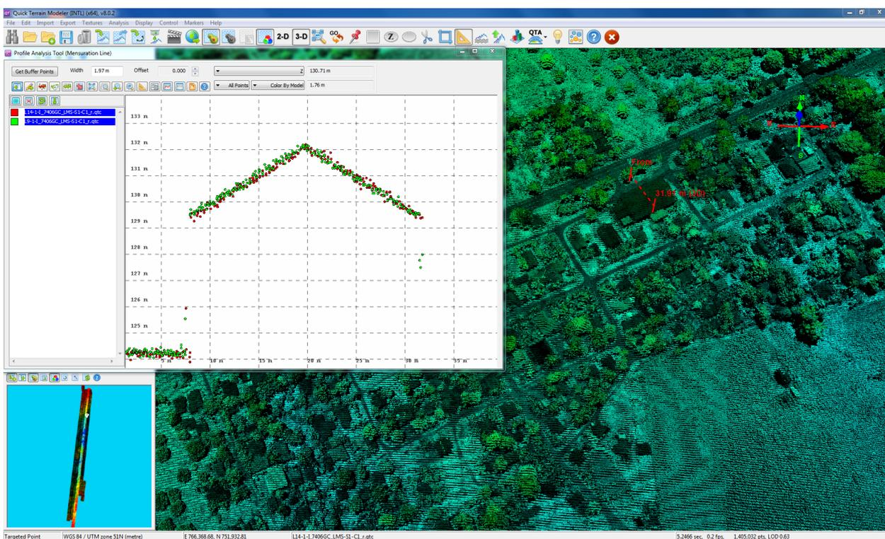
Figure 14. Quality checking for a Digos flight 7406GC using the Profile Tool of QT Modeler
