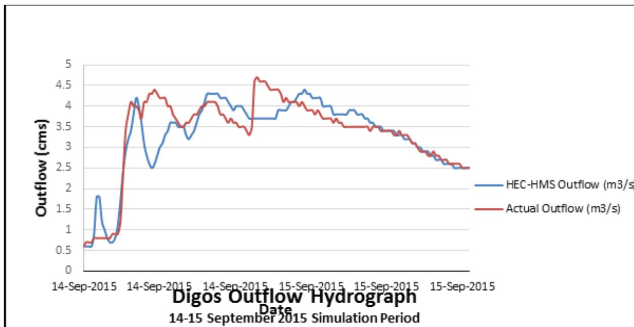
Figure 60. Outflow Hydrograph of Digos produced by the HEC-HMS model compared with observed outflow
