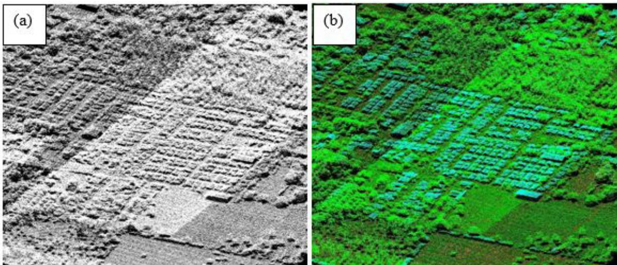
Figure 16. Point cloud before (a) and after (b) classification
