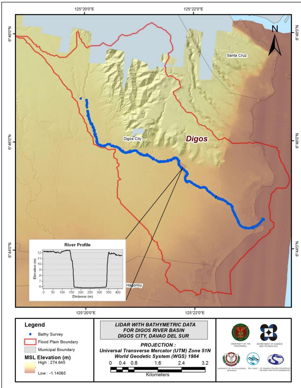
Figure 23. Map of Digos Flood Plain with bathymetric survey points shown in blue
