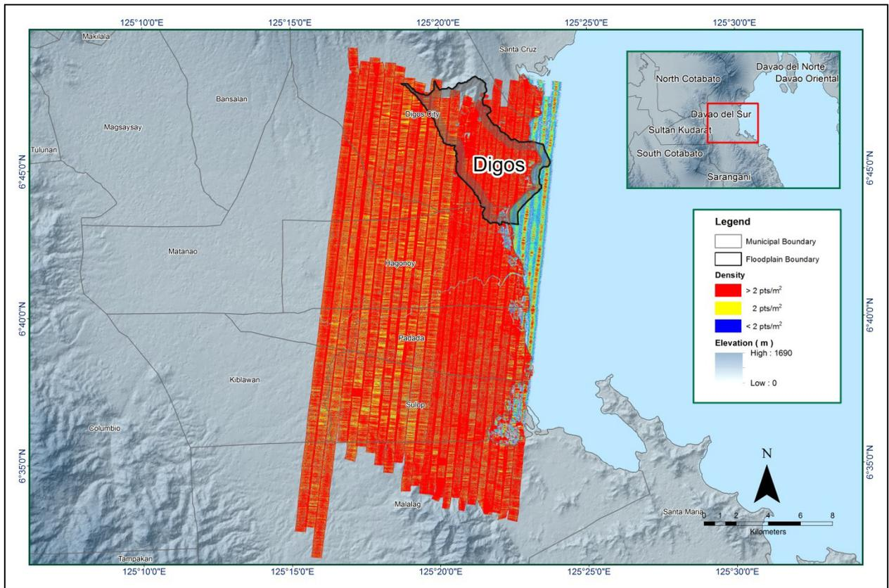
Figure 12. Pulse density map of merged LiDAR data for Digos Floodplain
