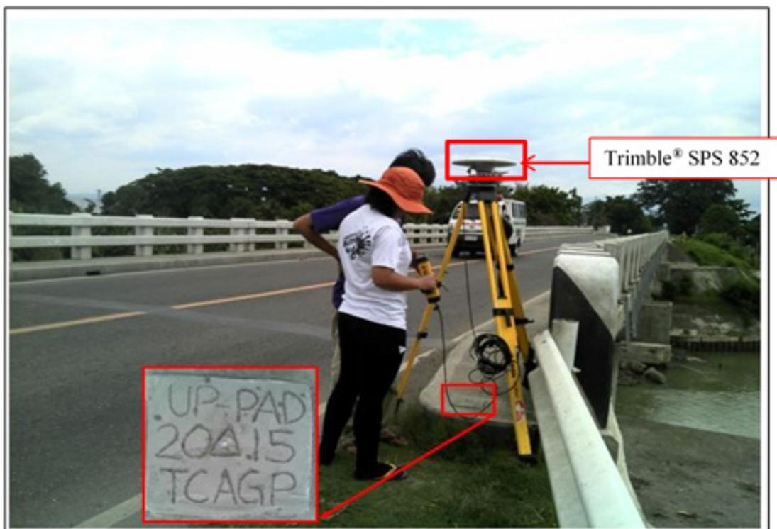
Figure 34. GNSS base receiver setup, Trimble® SPS 882 at UP-PAD, Padada Bridge, Brgy. Guihing, Municipality of Hagonoy, Davao del Sur
