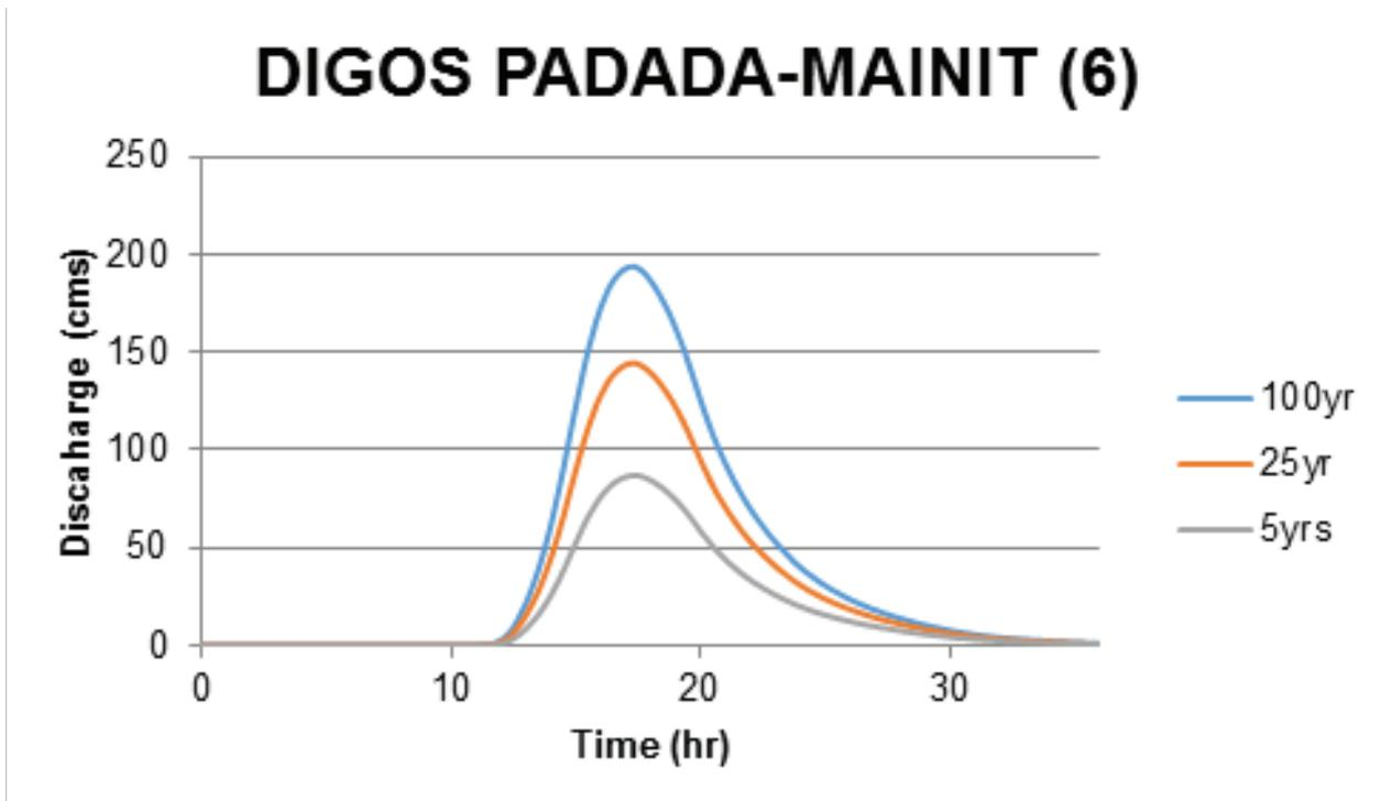
Figure 67. Digos Padada-Mainit river (6) generated discharge using 5-, 25-, and 100-year GenSan rainfall intensity-duration-frequency (RIDF) in HEC-HMS
