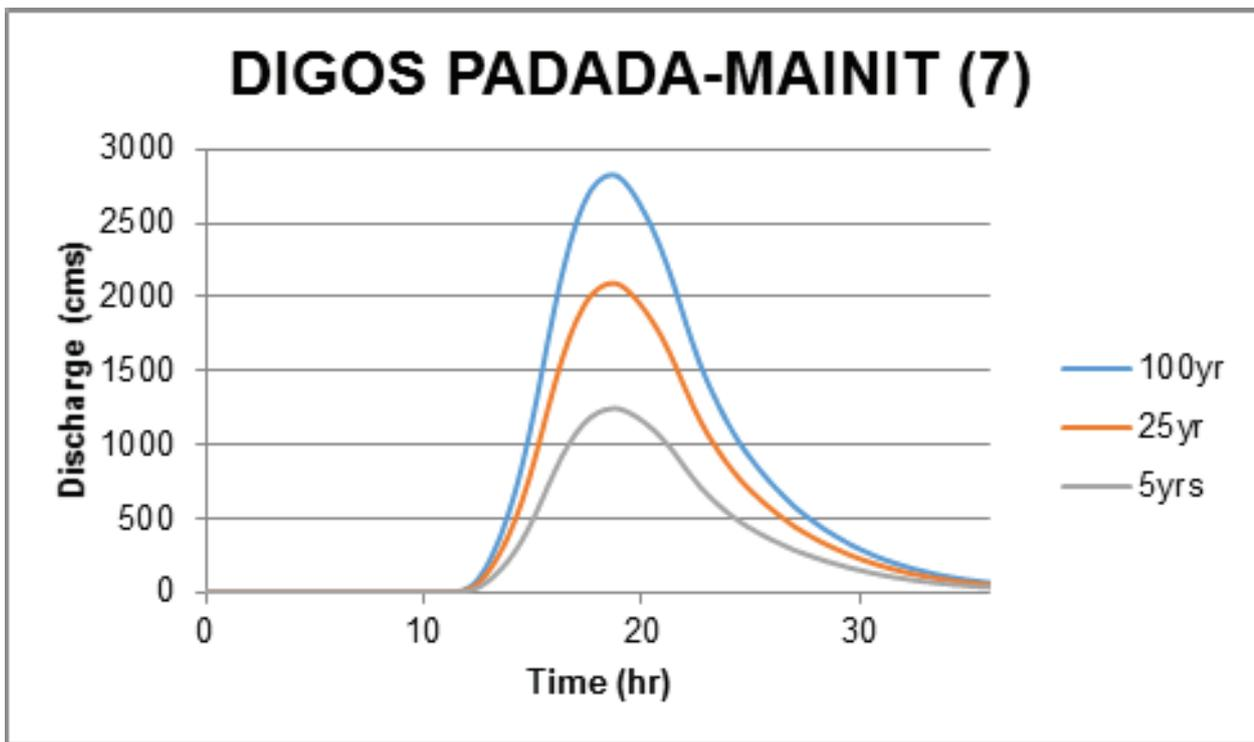
Figure 68. Digos Padada-Mainit river (7) generated discharge using 5-, 25-, and 100-year GenSan rainfall intensity-duration-frequency (RIDF) in HEC-HMS
