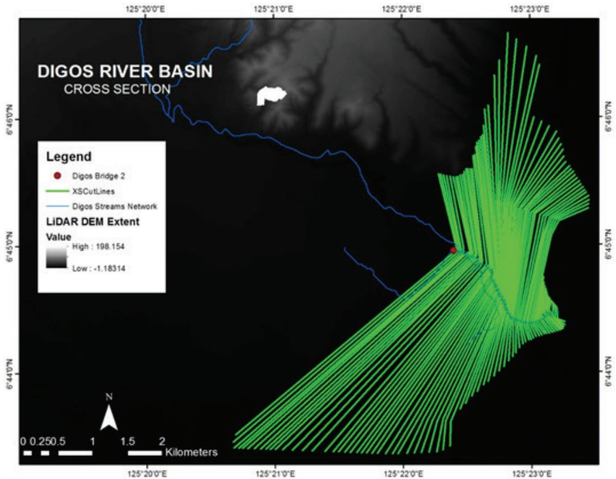
Figure 56. River cross-section of Digos River generated through Arcmap HEC GeoRAS tool
