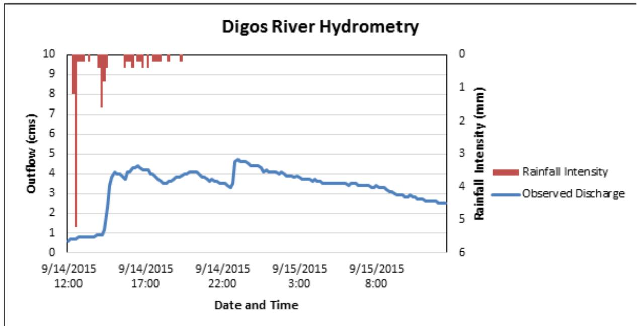
Figure 48. Rainfall and outflow data at Digos used for modeling
