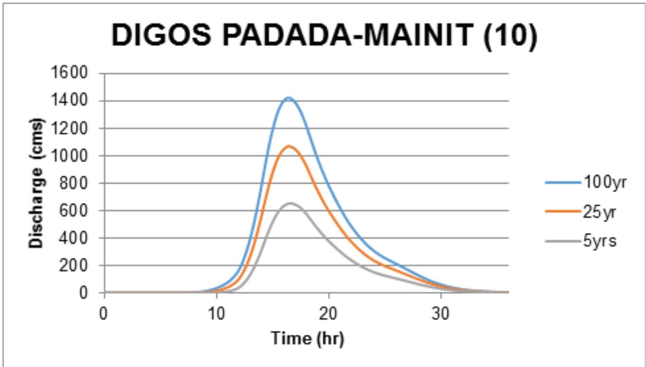
Figure 71. Digos Padada-Mainit river (10) generated discharge using 5-, 25-, and 100-year GenSan rainfall intensity-duration-frequency (RIDF) in HEC-HMS
