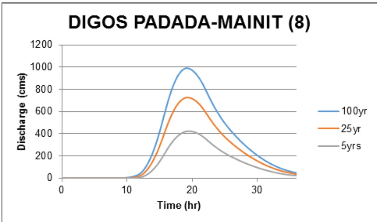
Figure 69. Digos Padada-Mainit river (8) generated discharge using 5-, 25-, and 100-year GenSan rainfall intensity-duration-frequency (RIDF) in HEC-HMS
