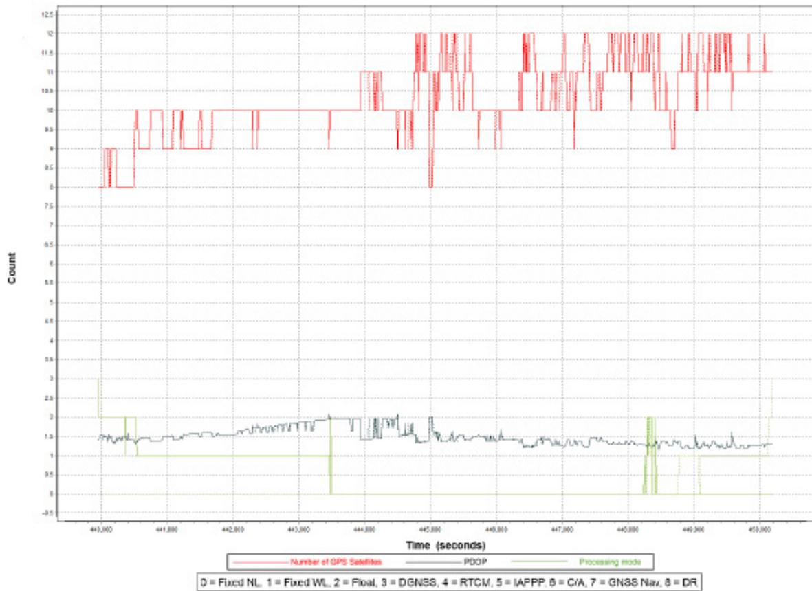
Figure 8. Solution Status Parameters of Digos Flight 7406GC.
