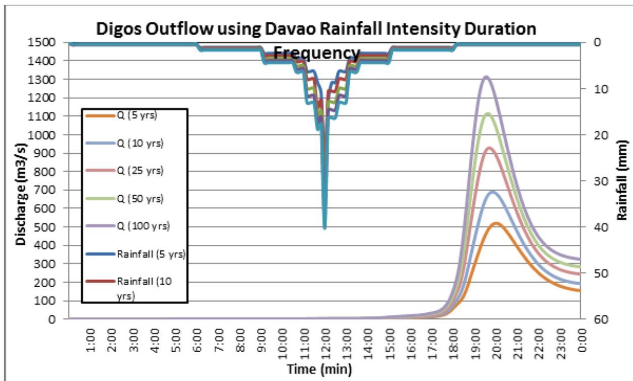
Figure 61. Outflow hydrograph at Digos Station generated using Davao RIDF simulated in HEC-HMS
