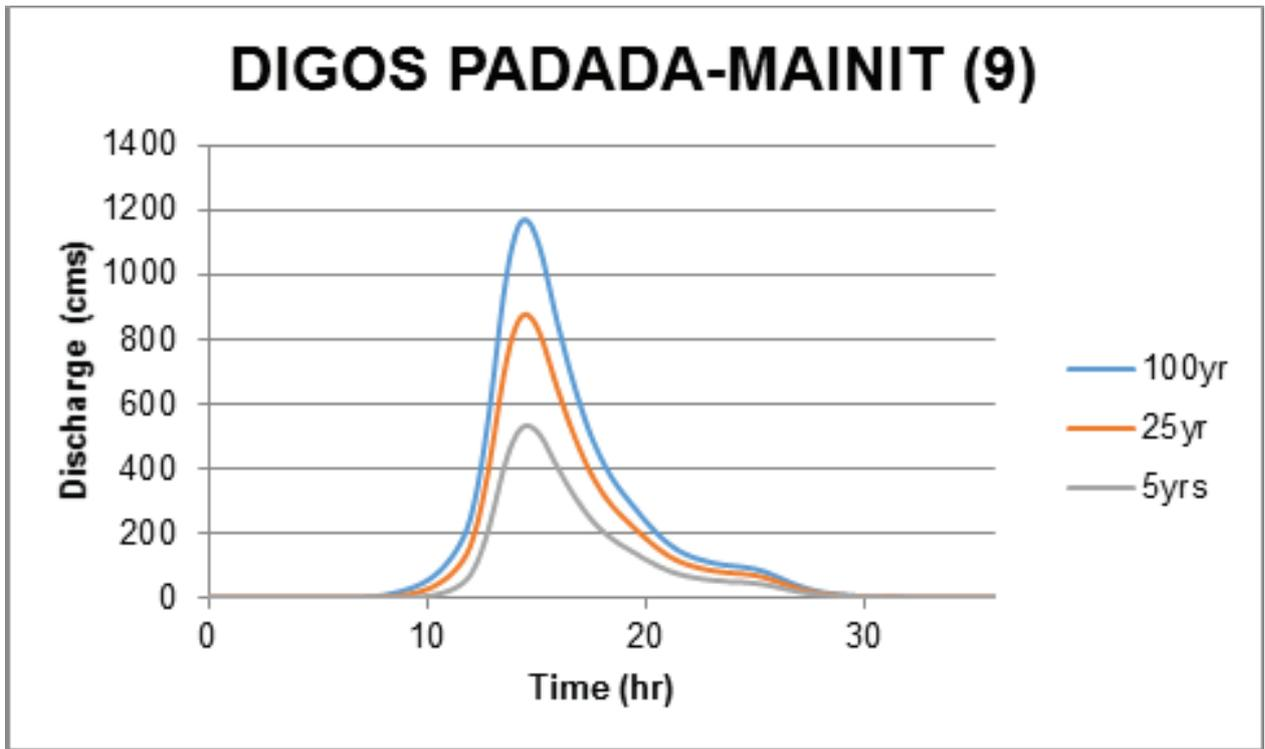
Figure 70. Digos Padada-Mainit river (9) generated discharge using 5-, 25-, and 100-year GenSan rainfall intensity-duration-frequency (RIDF) in HEC-HMS
