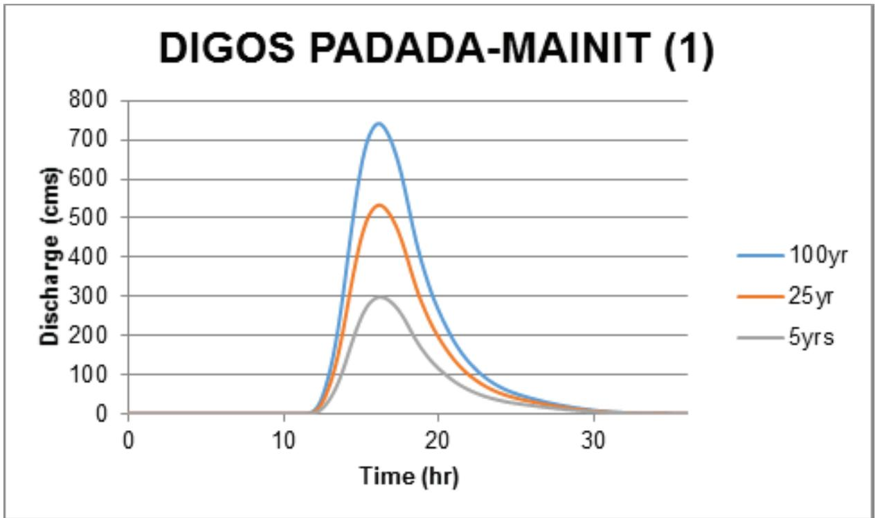
Figure 62. Digos Padada-Mainit river (1) generated discharge using 5-, 25-, and 100-year GenSan rainfall intensity-duration-frequency (RIDF) in HEC-HMS
