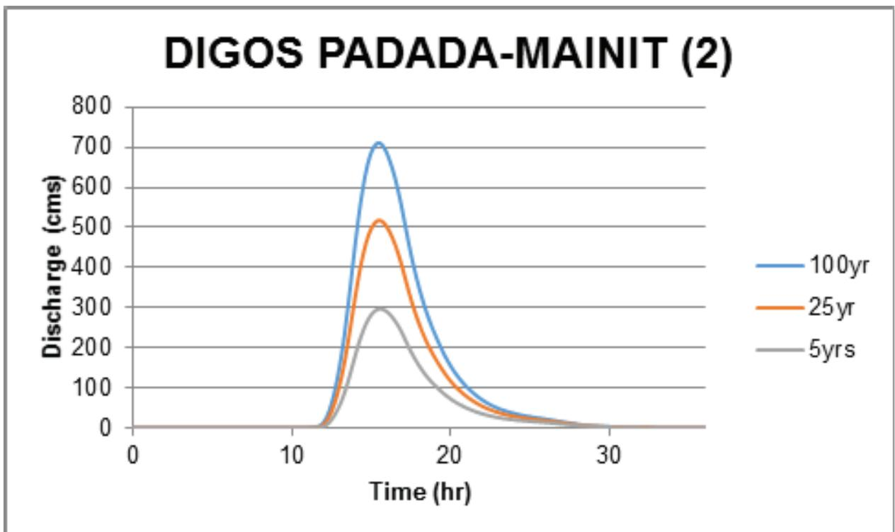
Figure 63. Digos Padada-Mainit river (2) generated discharge using 5-, 25-, and 100-year GenSan rainfall intensity-duration-frequency (RIDF) in HEC-HMS
