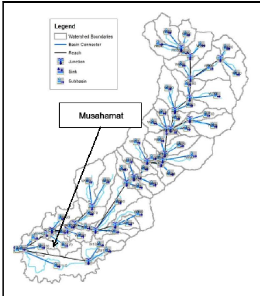
Figure 54. The Kingking river basin model generated using HEC-HMS.
