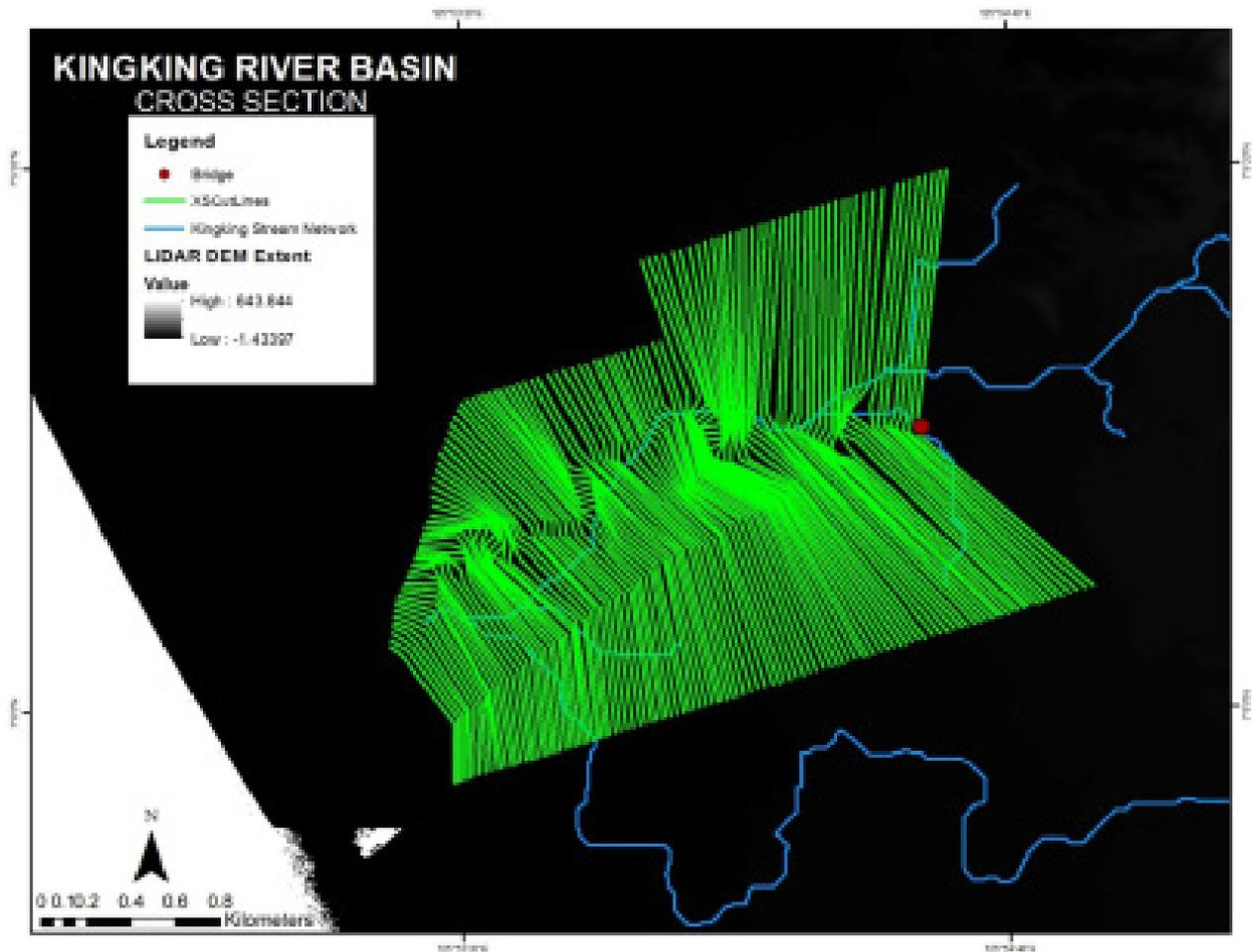
Figure 55. River cross-section of Kingking River generated through Arcmap HEC GeoRAS tool
