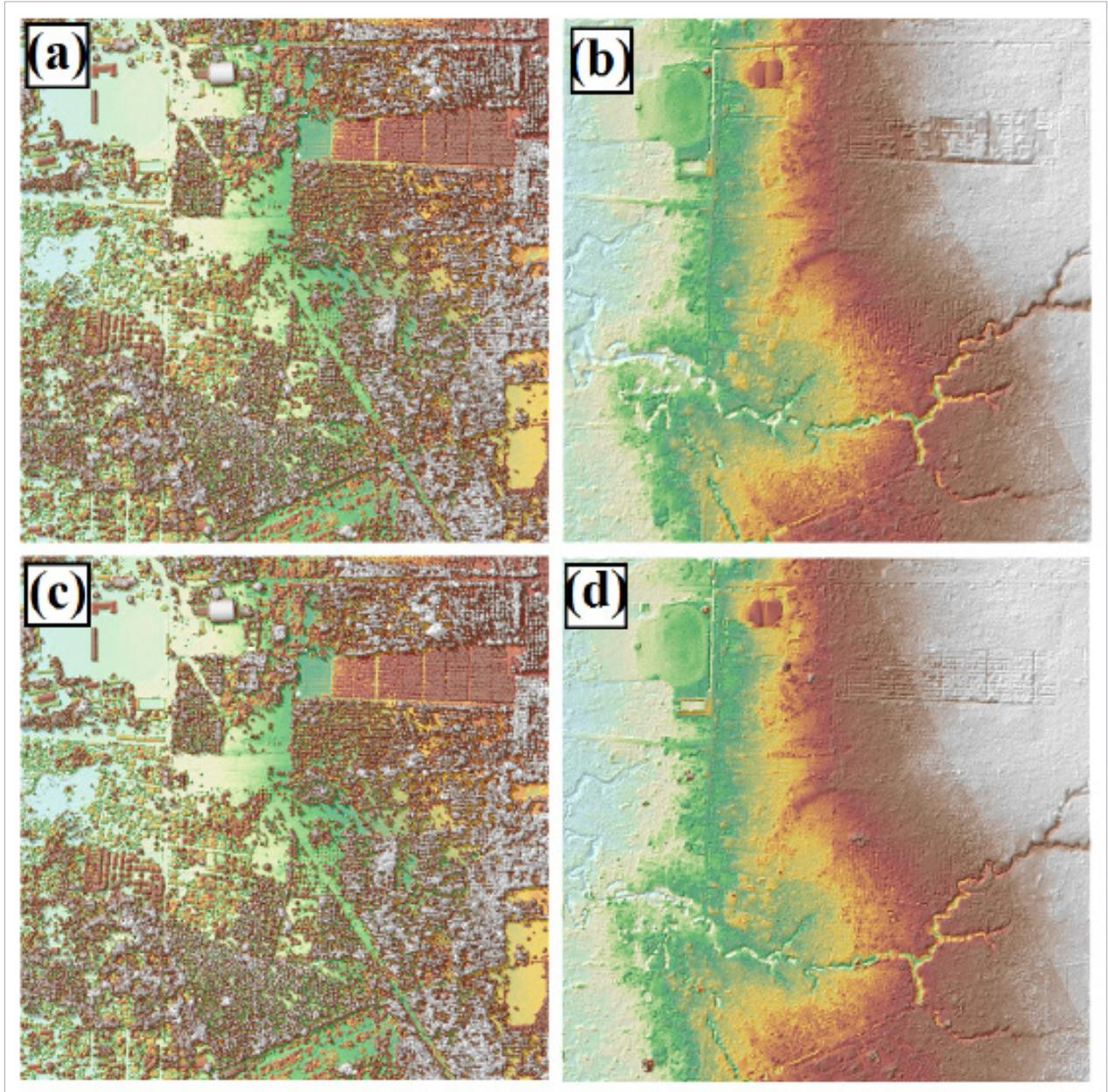
Figure 18. The production of last return DSM (a) and DTM (b), first return DSM (c) and secondary DTM (d) in some portion of Kingking floodplain.
