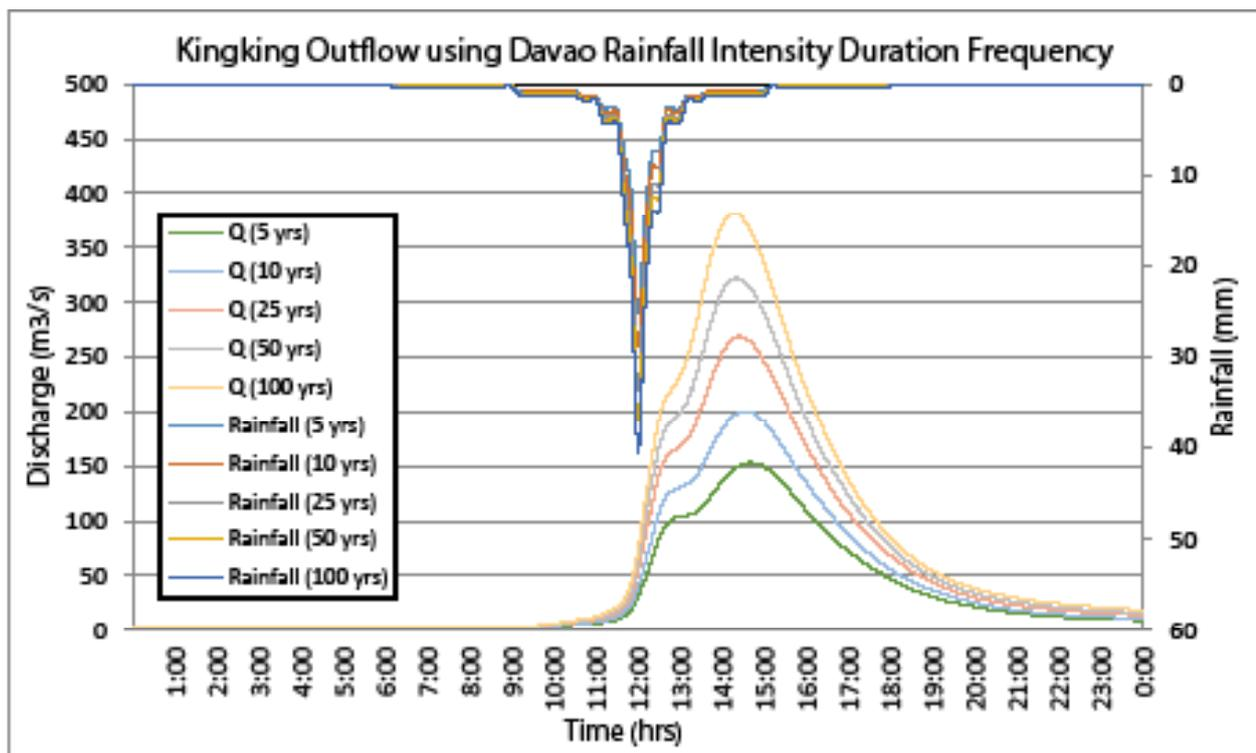
Figure 58. Outflow hydrograph at Kingking Station generated using the Davao RIDF simulated in HEC-HMS.
