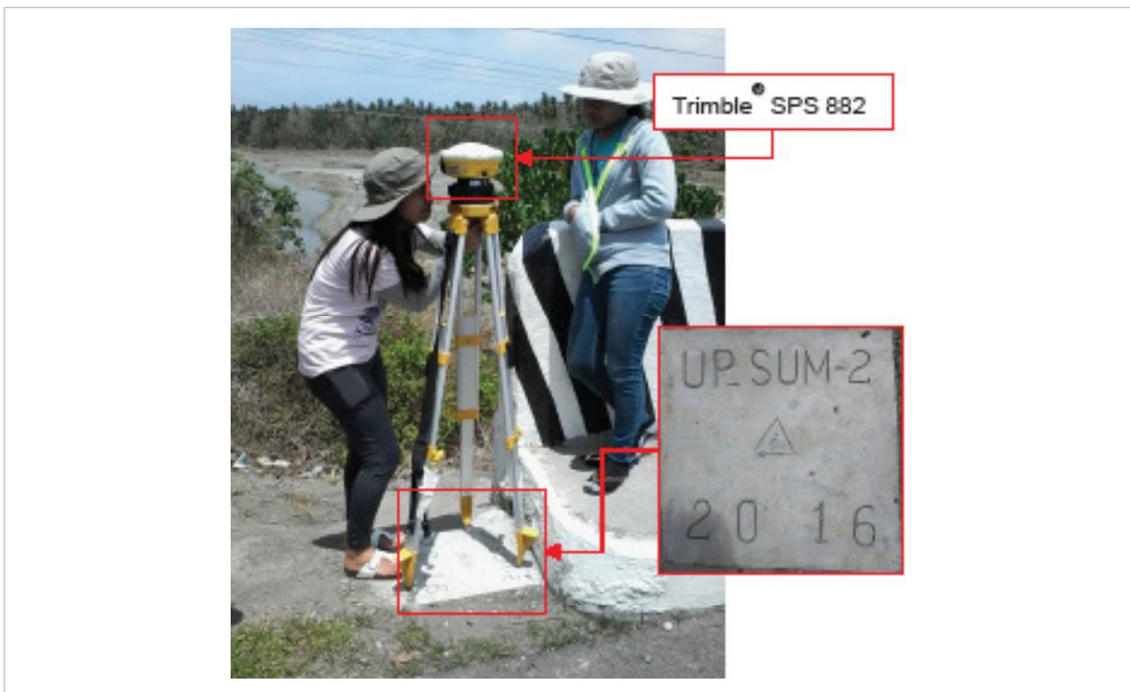
Figure 31. GNSS receiver set up, Trimble® SPS 882, at UP\_SUM-2, located beside the approach of Sumlog Bridge in Brgy. Ilangay, Municipality of Lupon, Province of Davao Oriental.
