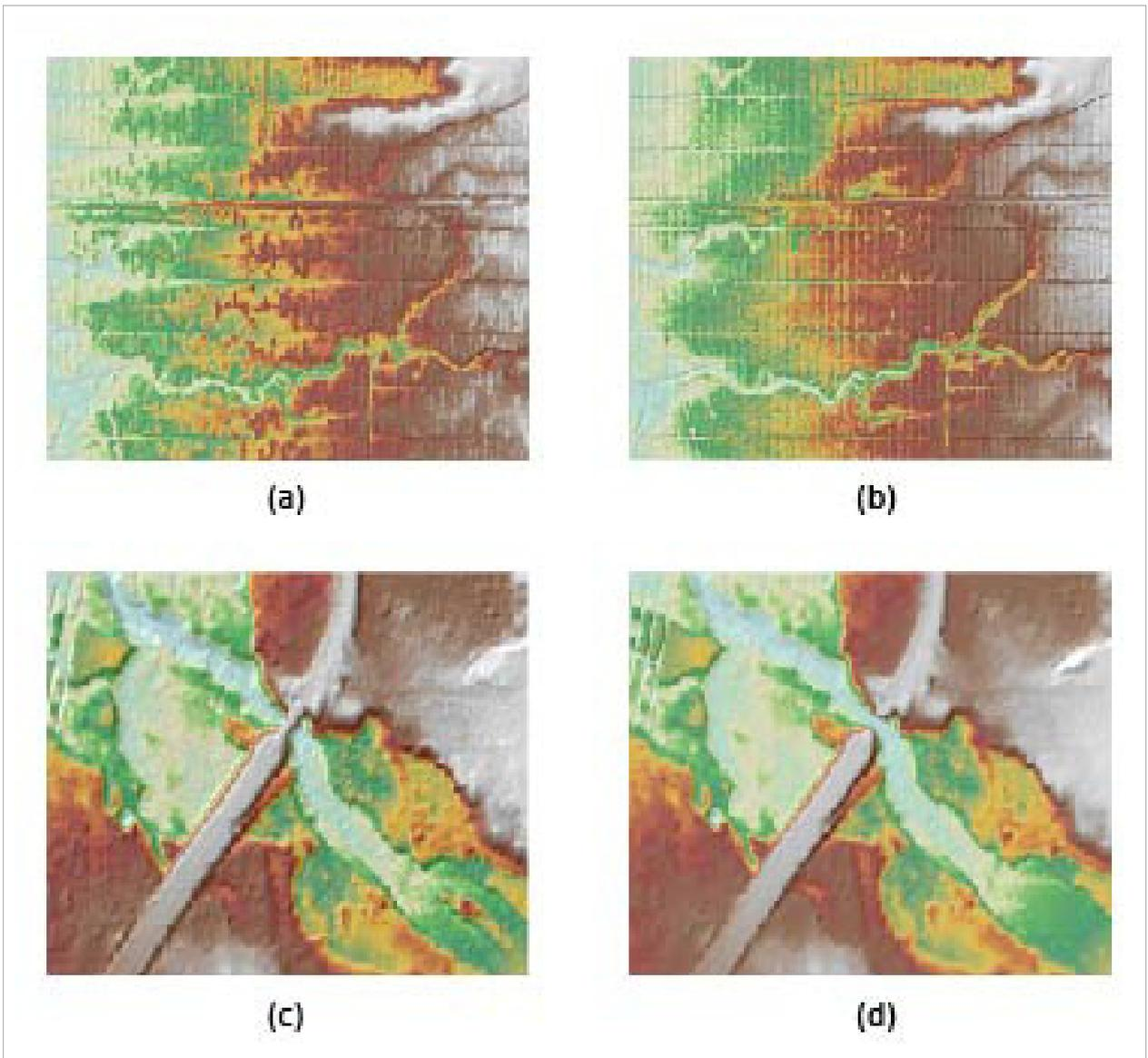
Figure 19. Portions in the DTM of Kingking floodplain – a paddy field before (a) and after (b) data retrieval; and a bridge before (c) and after (d) manual editing.
