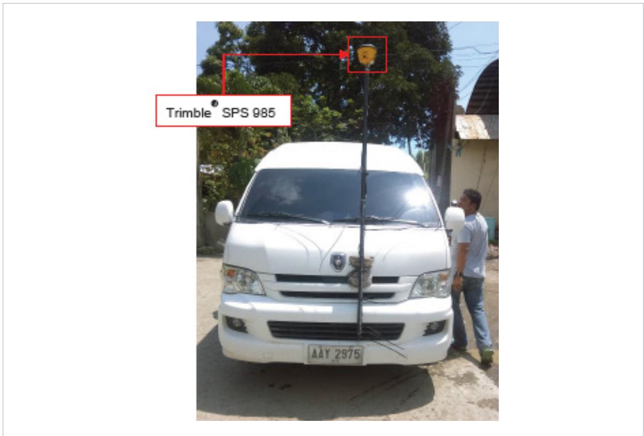
Figure 38. Validation points acquisition survey set-up for Kingking River.
