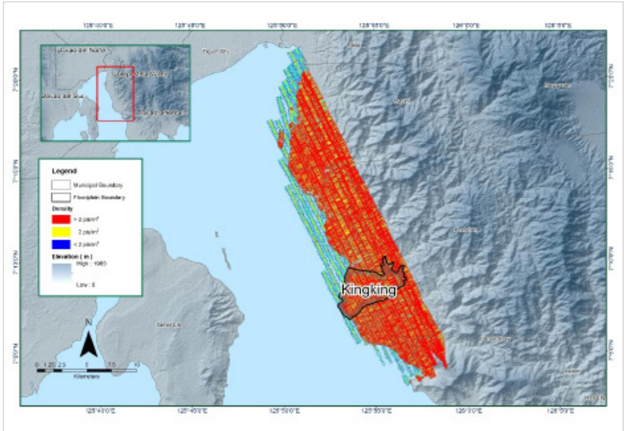
Figure 13. Pulse density map of merged LiDAR data for Kingking floodplain.
