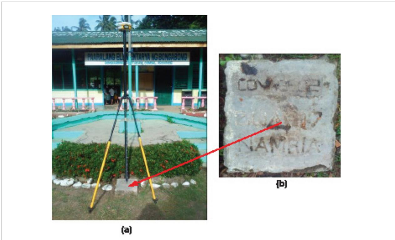
Figure 5. GPS set-up over COV-3062 located in front of the flagpole of Bongabong Elementary School (a) and NAMRIA reference point COV-3062 (b) as recovered by the field team.
