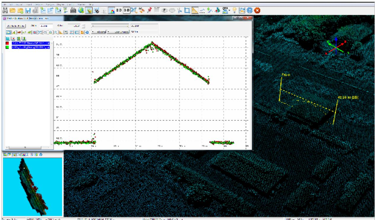
Figure 15. Quality checking for a Kingking flight 7350GC using the Profile Tool of QT Modeler.
