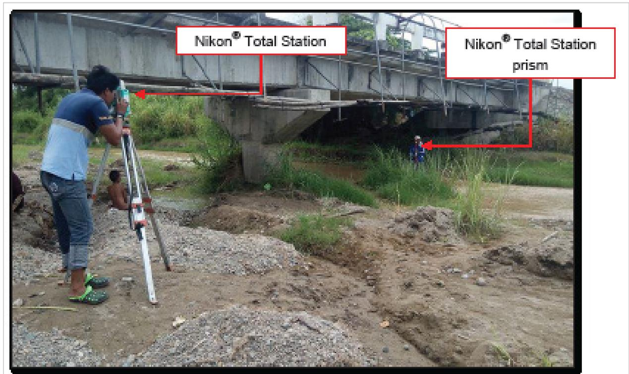
Figure 40. Manual bathymetric survey of ABSD at Kingking River using Nikon® Total Station.
