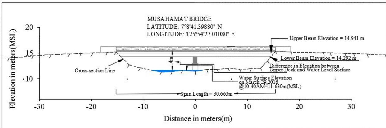
Figure 35. Musahamat Bridge Cross-section Diagram.
