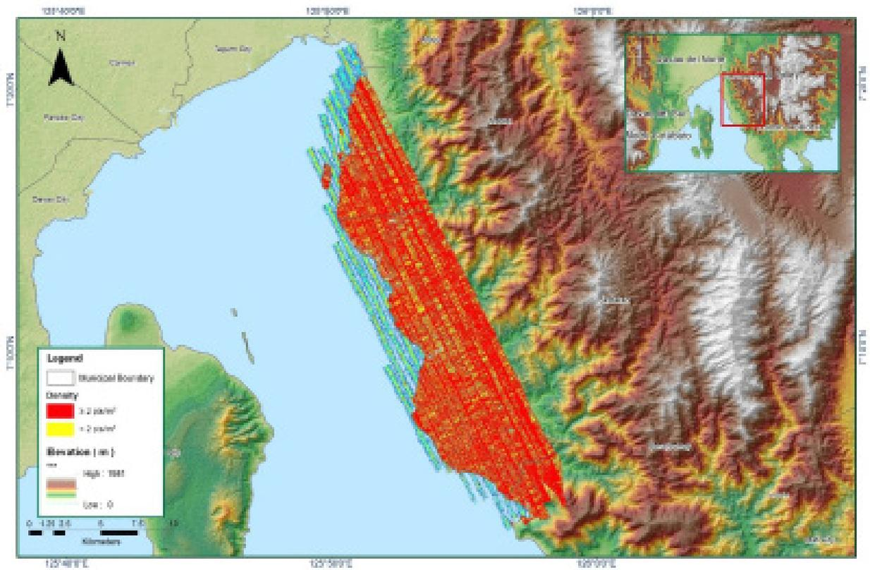
Figure 76. Density map of merged LiDAR data
