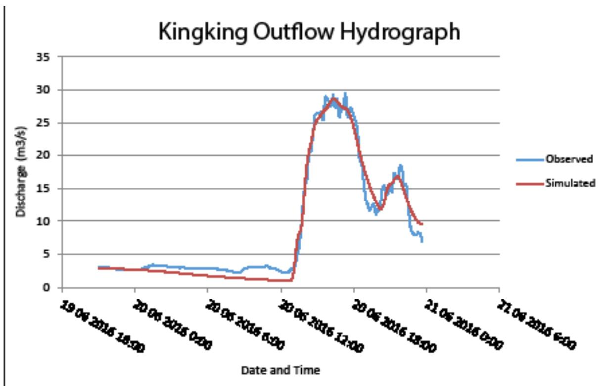
Figure 57. Outflow Hydrograph of Kingking produced by the HEC-HMS model compared with observed outflow
