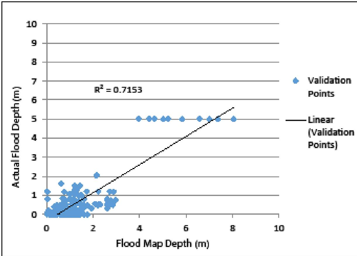
Figure 70. Flood Map Depth vs Actual Flood Depth for Kingking
