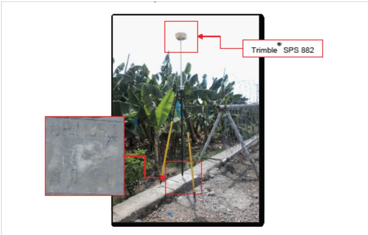
Figure 30. GNSS receiver set up, Trimble® SPS 882, at UP\_MUS-1, located at the approach
