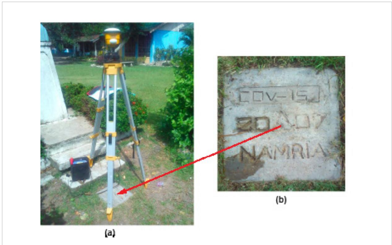
Figure 4. GPS set-up over COV-15 inside the premises of Tibagon Elementary School (a) and NAMRIA reference point COV-15 (b) as recovered by the field team.
