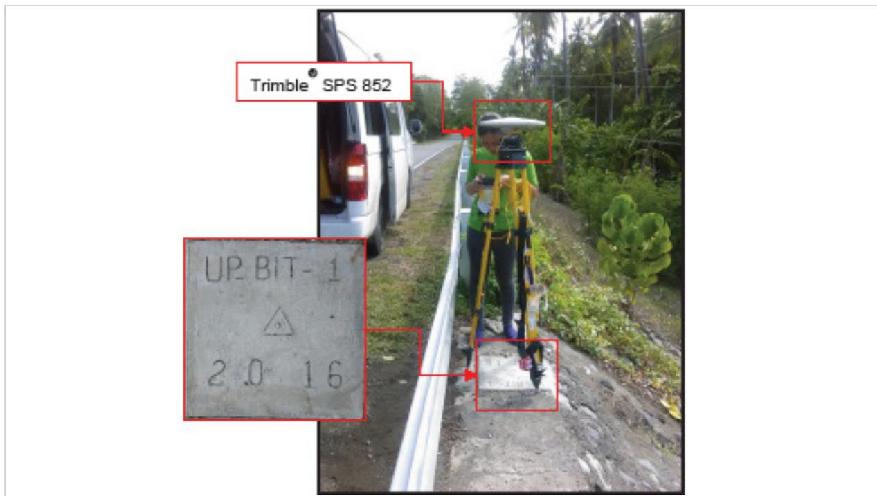
Figure 29. GNSS receiver set up, Trimble® SPS 852, at UP\_BIT-1, located at the side of the railing near the approach of Bitanagan Bridge in Brgy. Don Enrique Lopez, City of Mati, Davao Oriental.
