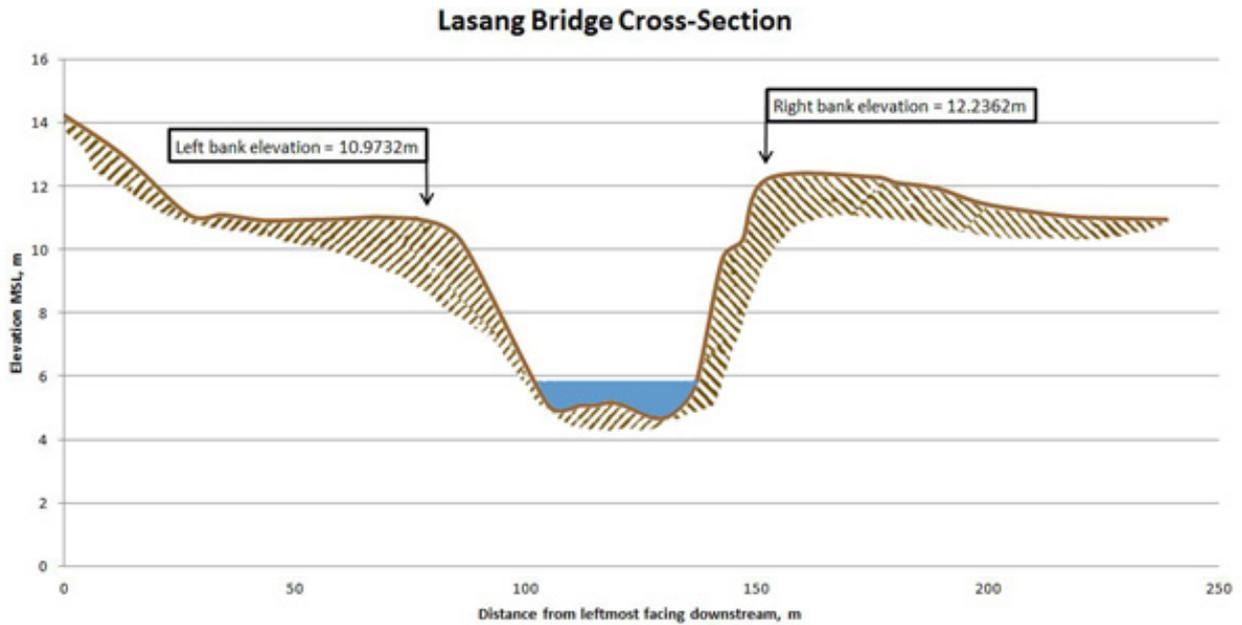
Figure 50. Cross-Section Plot of Lasang Footbridge
