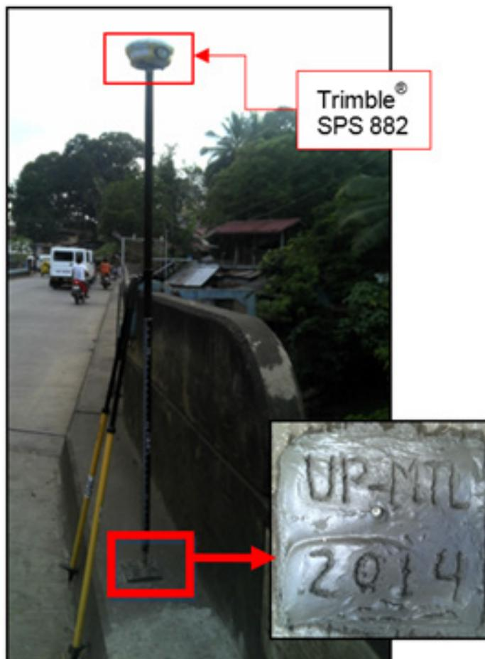
Figure 37. GNSS receiver occupation set up, Trimble® SPS 882 at control point UP-MTL, Mintal Bridge in Brgy. Mintal, Davao City
