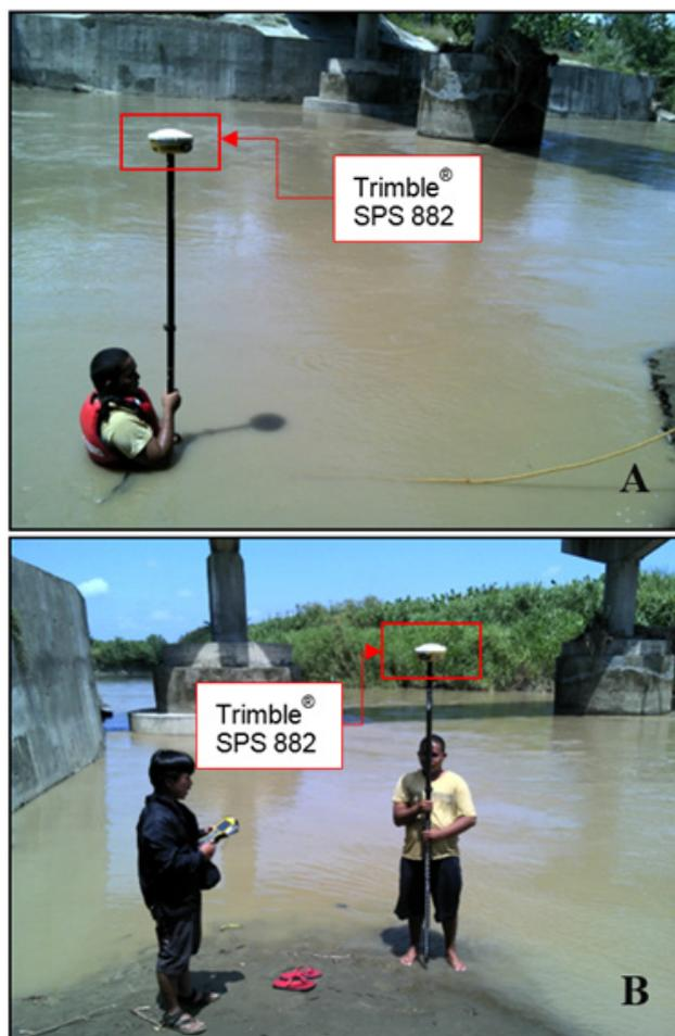
Figure 38. Cross-section survey at the Lasang Bridge in Panabo City
