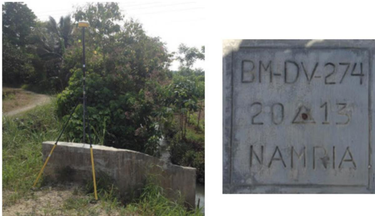
Figure 10. GPS set-up over BMDV-274 as recovered along the Tagum-Laak National Highway (a) and NAMRIA reference point BMDV-274 (b) as recovered by the field team.
