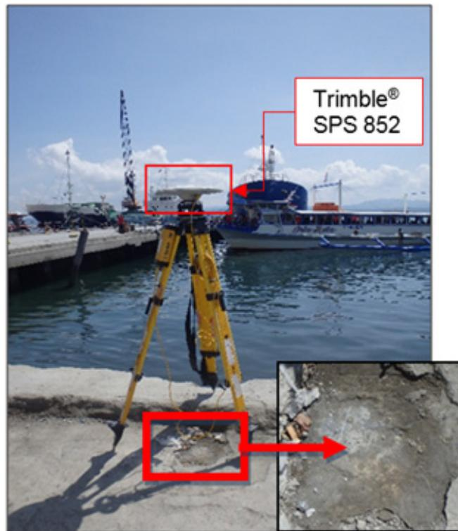
Figure 34. GNSS base receiver set up, Trimble® SPS 852 at DVS-1 in Sta. Ana Wharf, Davao City
