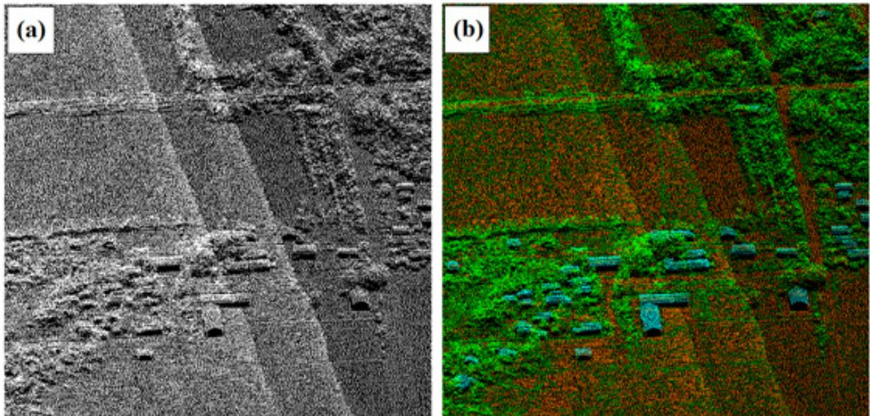
Figure 22. Point cloud before (a) and after (b) classification.
