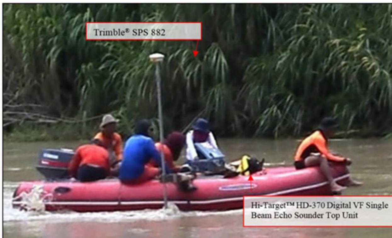
Figure 45. Setup of bathymetric survey using Hi-Target™ Single Beam Echo Sounder
