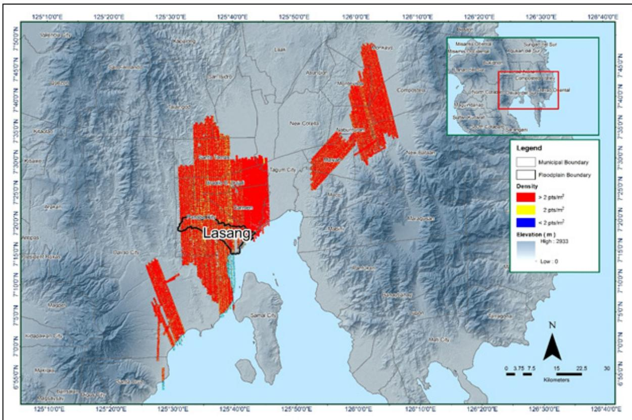
Figure 18. Pulse density map of merged LiDAR data for Lasang floodplain.
