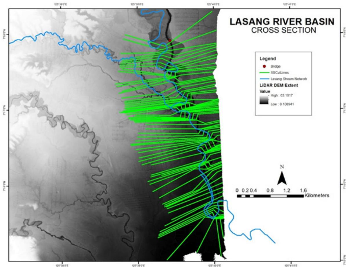
Figure 60. River cross-section of the Lasang River generated through Arcmap HEC GeoRAS tool
