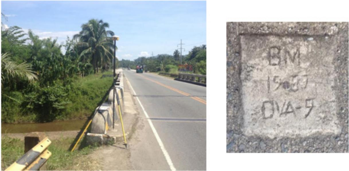
Figure 9. GPS set-up over BMDVA-9 as recovered in Barangay Magsaysay, Nabunturan, Compostela Valley (a) and NAMRIA reference point BMDVA-9 (b) as recovered by the field team.
