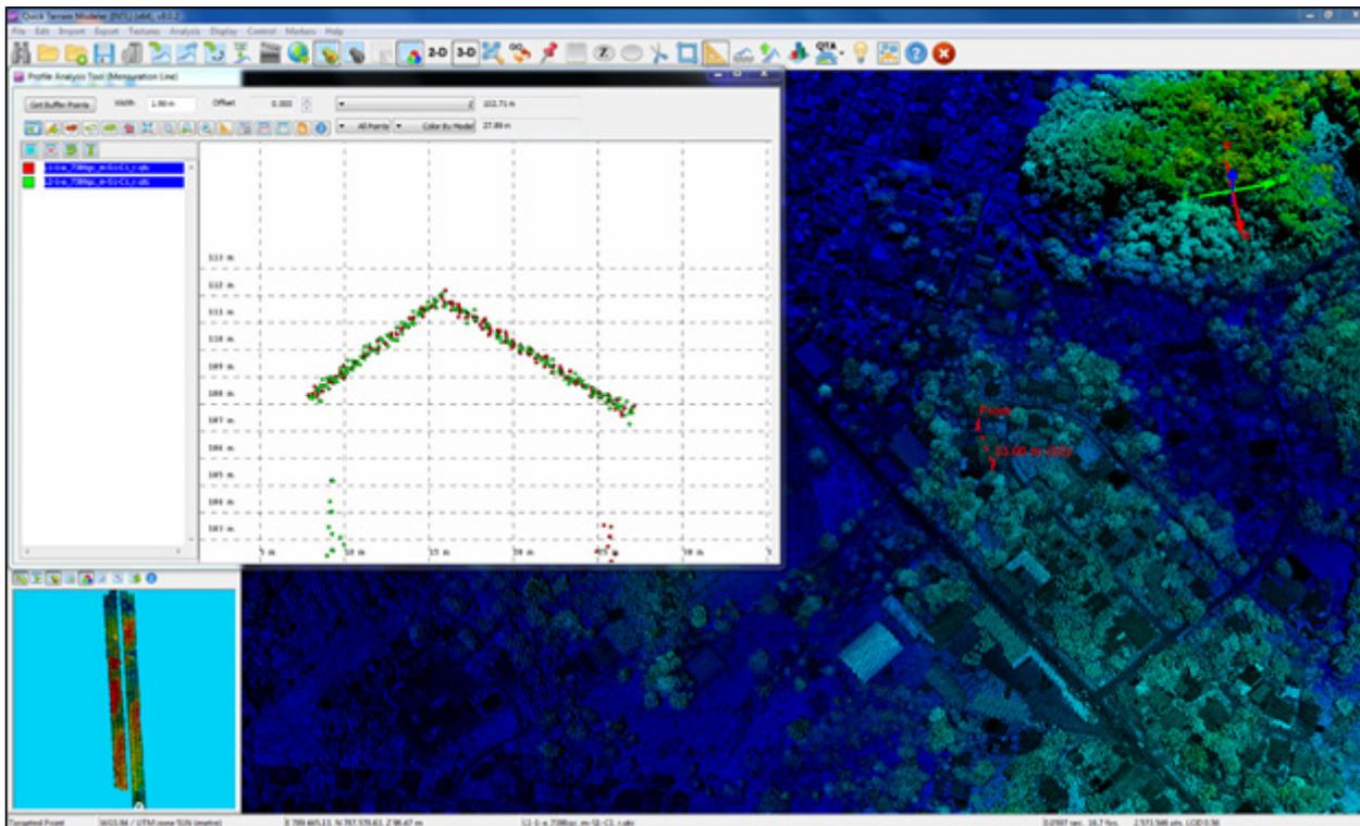
Figure 20. Quality checking for a Lasang flight 7386GC using the Profile Tool of QT Modeler.
