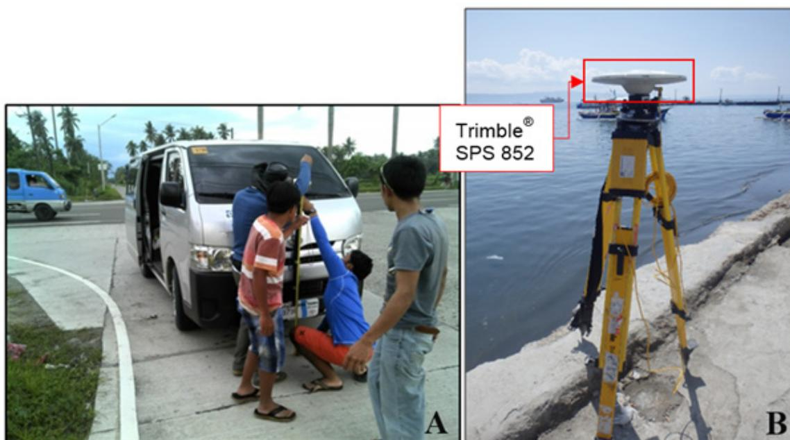
Figure 43. Validation points acquisition survey set-up (A) and the occupied base station, DVS-1, (B) at Sta. Ana Port
