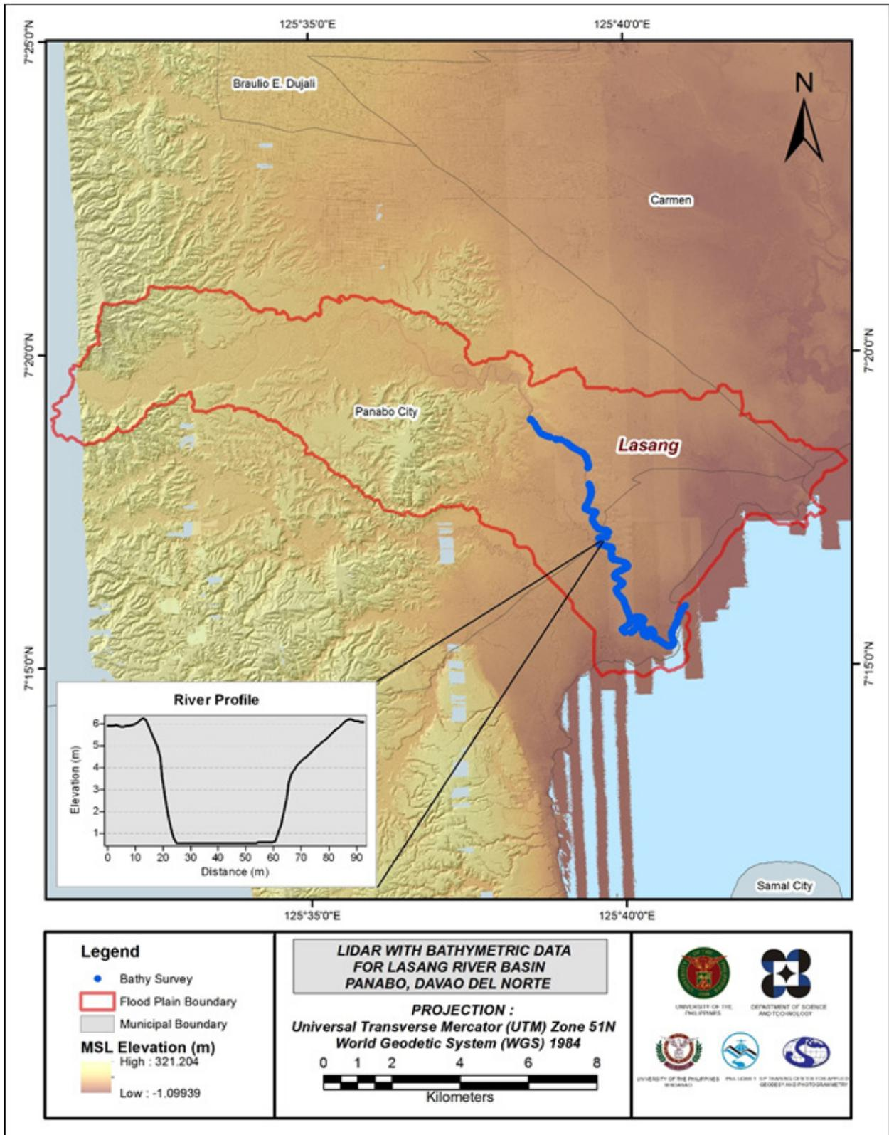
Figure 29. Map of Lasang Floodplain with bathymetric survey points shown in blue.
