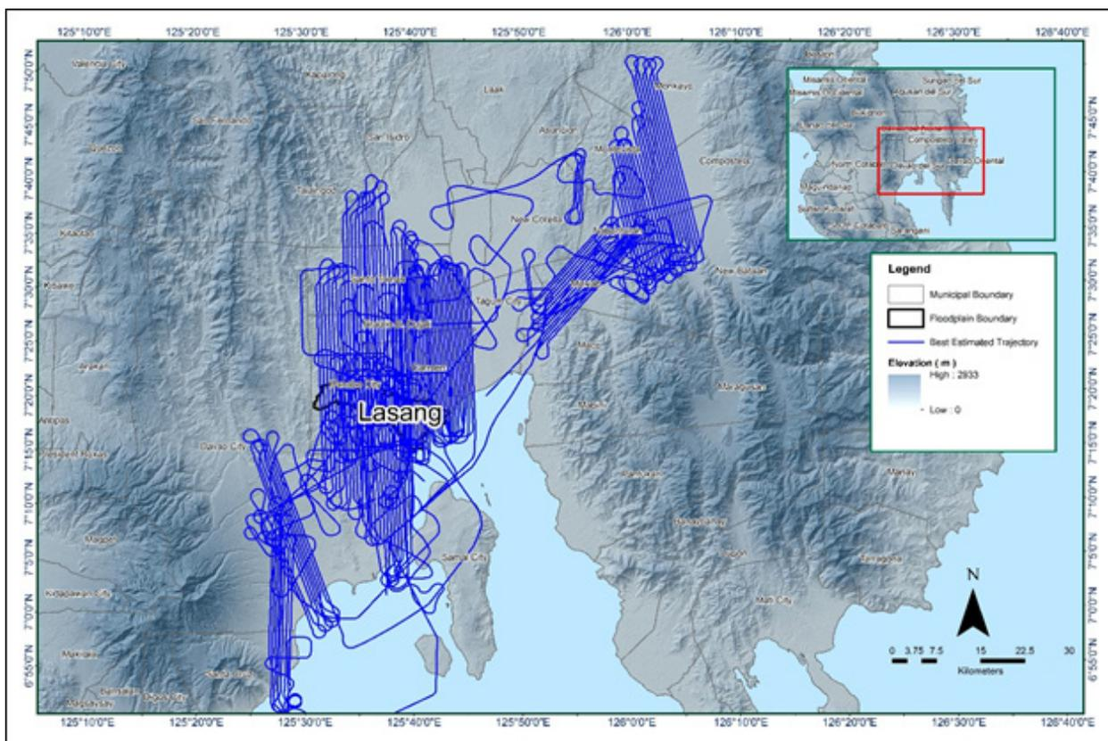
Figure 15. Best estimated trajectory conducted over the Lasang Floodplain
