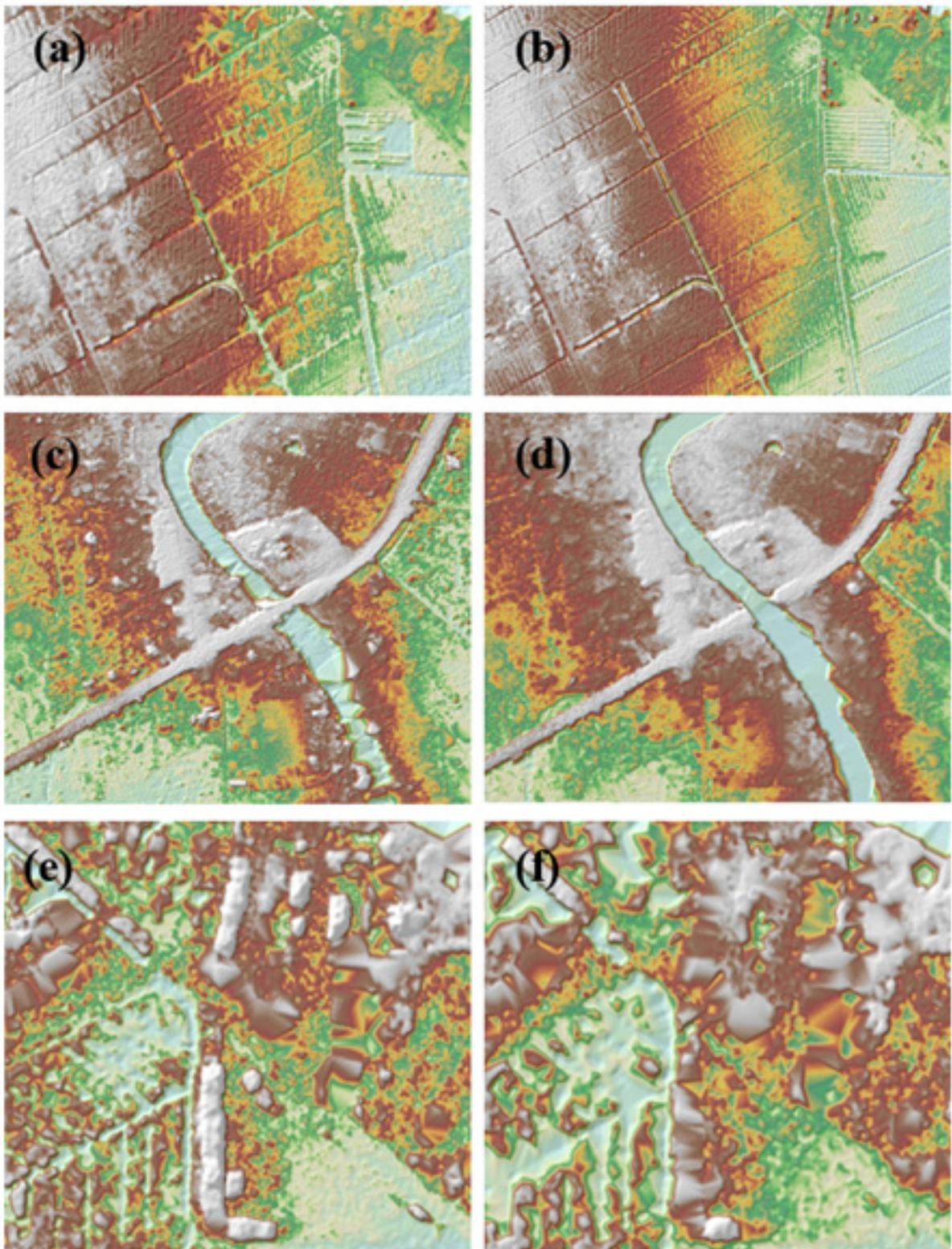
Figure 24. Portions in the DTM of Lasang floodplain – a paddy field before (a) and after (b) data retrieval; a bridge before (c) and after (d) manual editing; and a building before and after (f) manual editing
