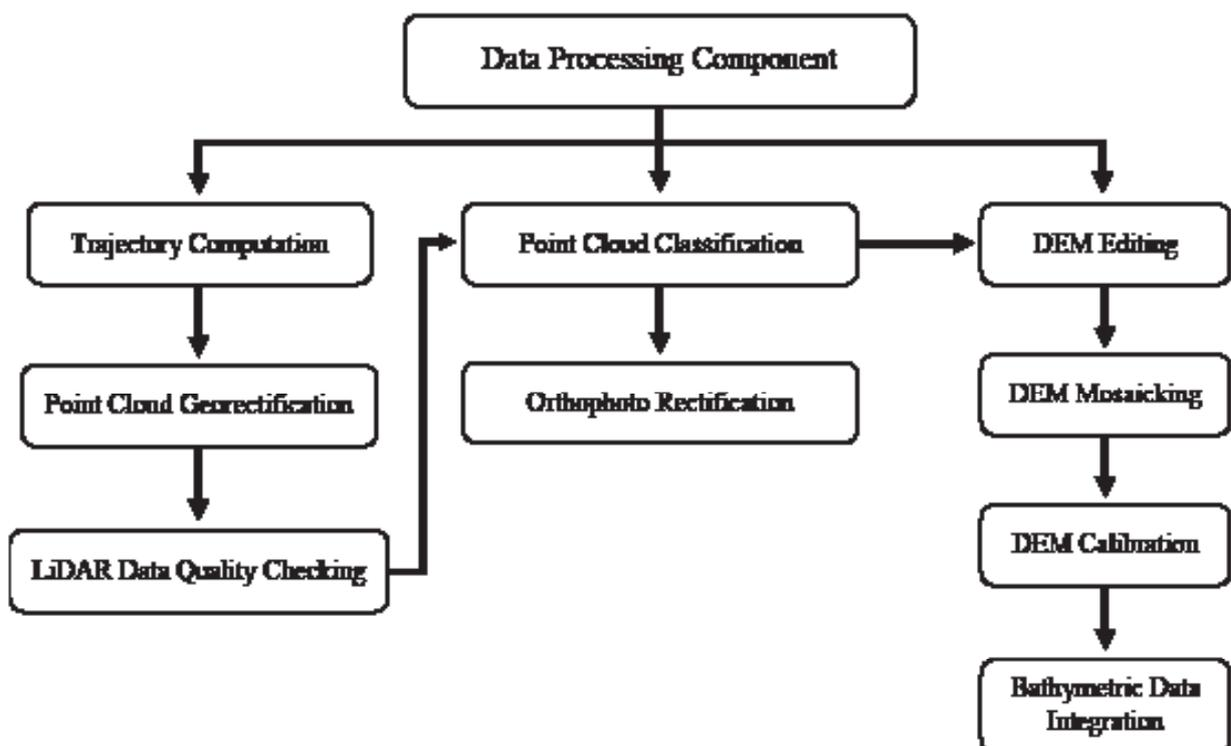
Figure 12. Schematic Diagram for Data Pre-Processing Component
