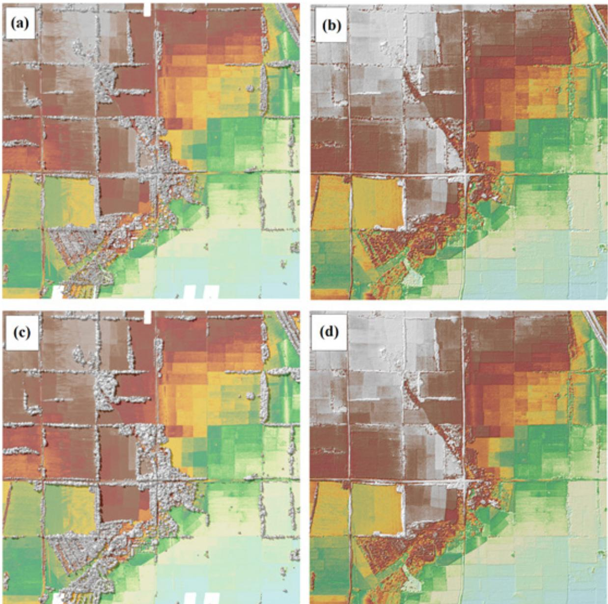
Figure 23. The production of last return DSM (a) and DTM (b), first return DSM (c) and secondary DTM (d) in some portion of Lasang Floodplain.
