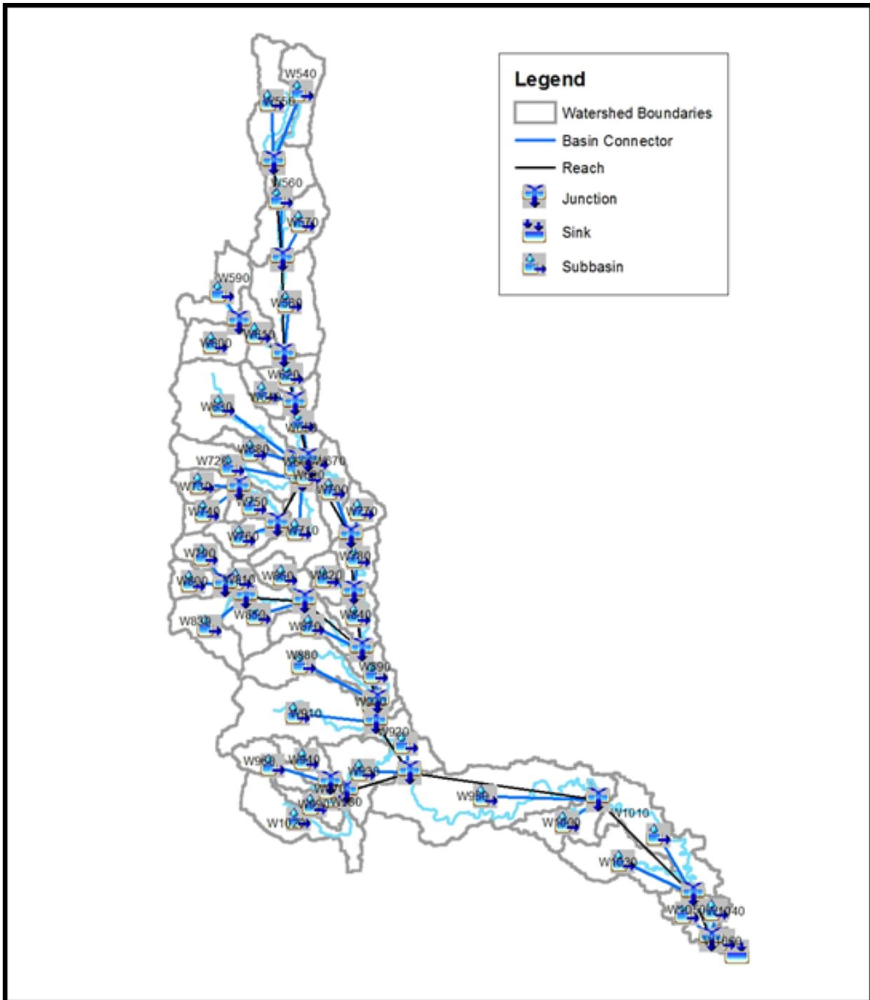
Figure 59. The Lasang river basin model generated using HEC-HMS.
