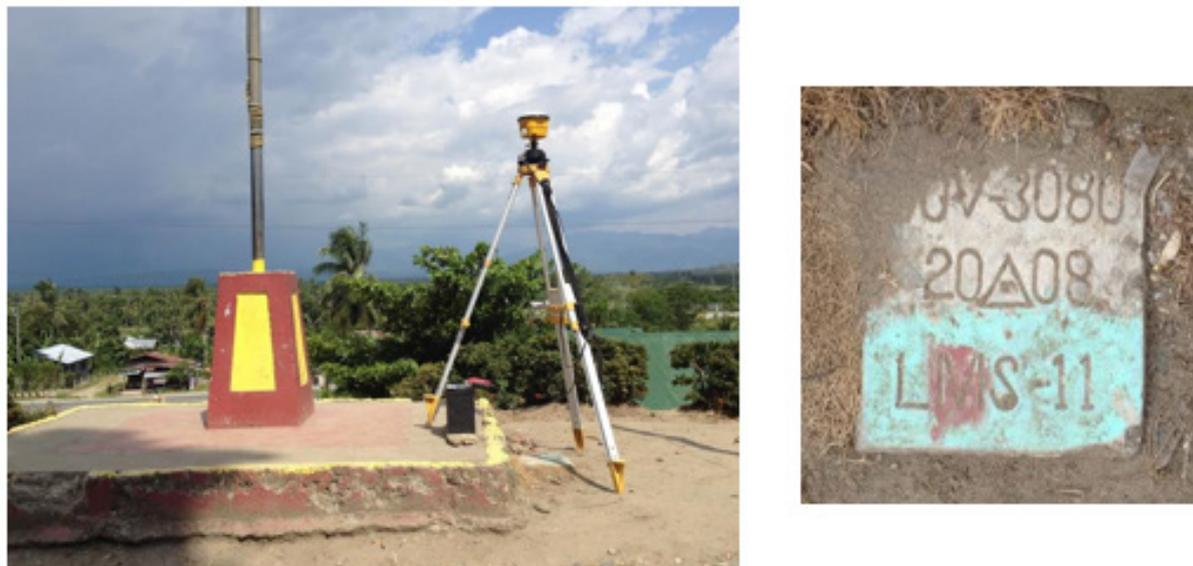
Figure 8. GPS set-up over COV-3080 as recovered in Barangay Magsaysay, Nabunturan, Compostela Valley (a) and NAMRIA reference point COV-3080 (b) as recovered by the field team
