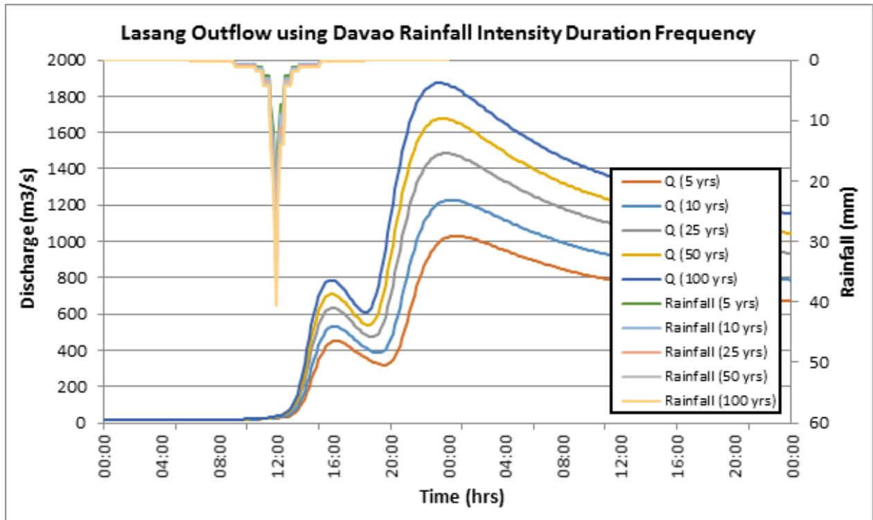
Figure 63. Outflow hydrograph at the Lasang Station generated using the Davao RIDF simulated in HEC-HMS.
