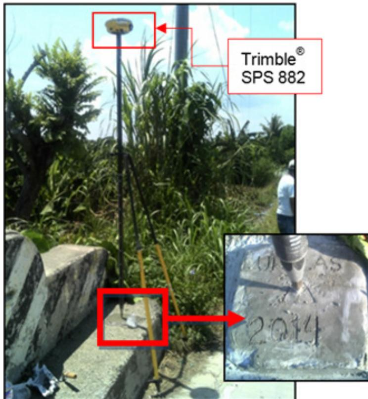
Figure 36. GNSS receiver occupation set up, Trimble® SPS 882 at control point UP-LAS in Brgy. Little Panay, Panabo City
