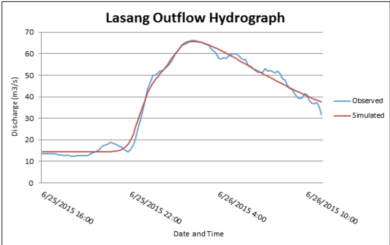
Figure 62. Outflow Hydrograph of Lasang produced by the HEC-HMS model compared with observed outflow
