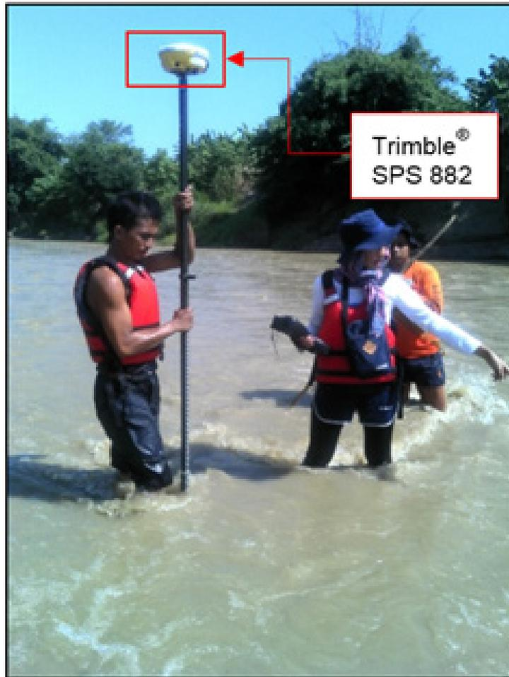
Figure 46. Actual execution of manual bathymetric survey along Lasang River
