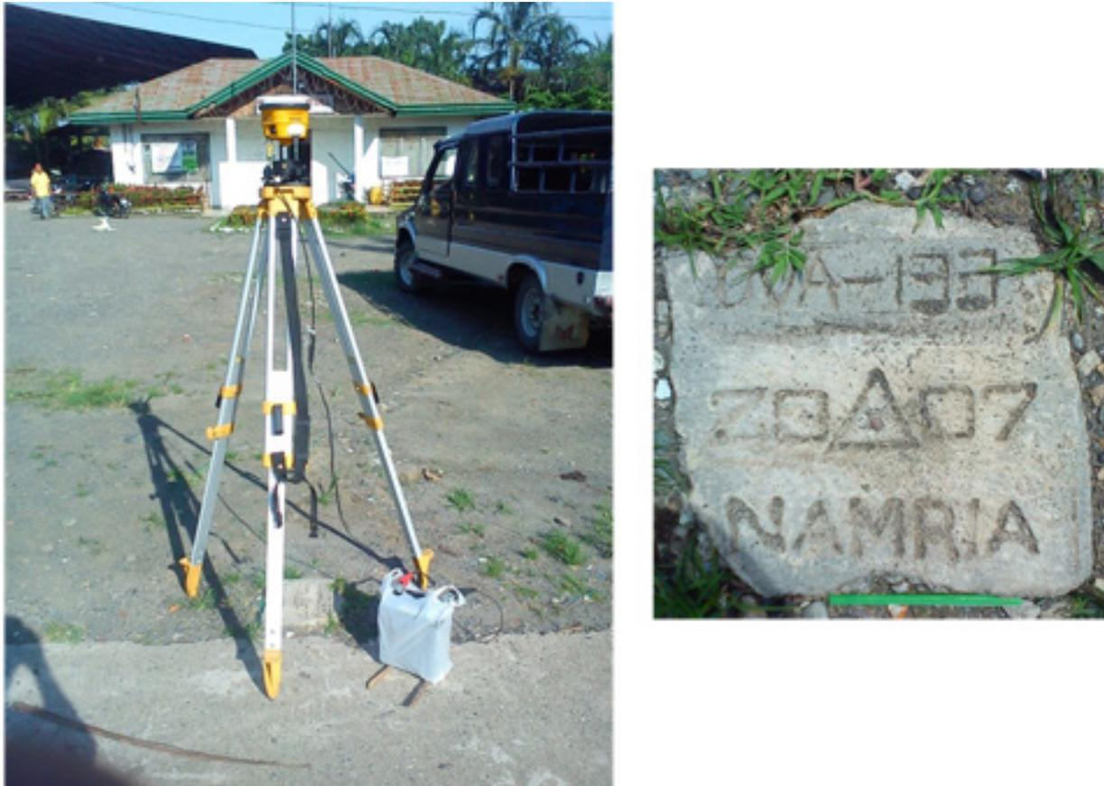
Figure 4. GPS set-up over DVA-133 as located in front of the barangay hall of Manay (a) and NAMRIA reference point DVA-133 (b) as recovered by the field team.
