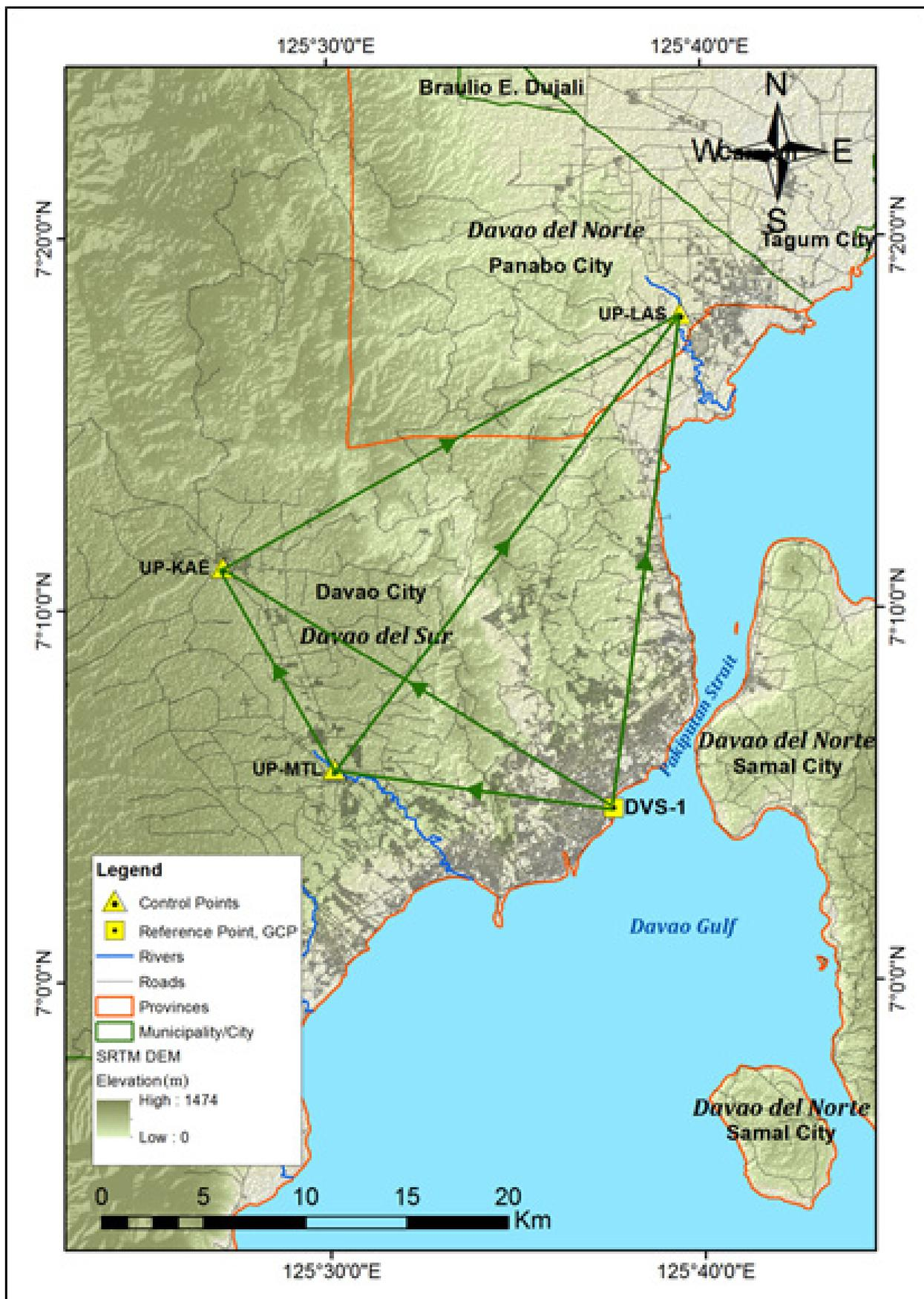
Figure 33. GNSS Network of Talomo and Lasang Rivers Field Survey
