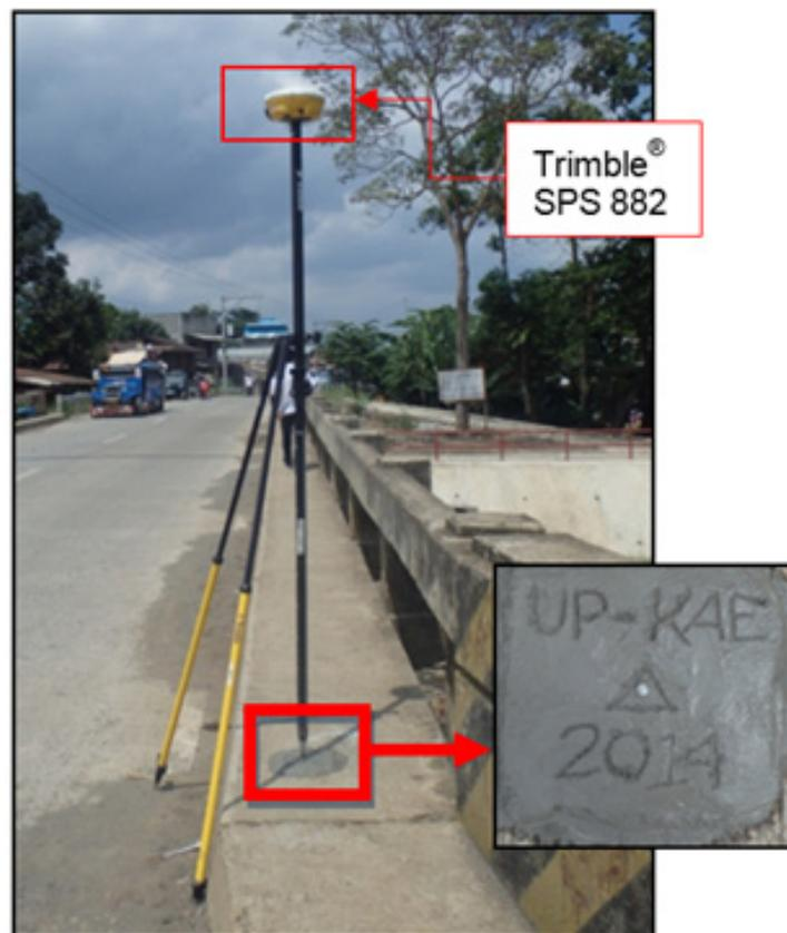
Figure 35. GNSS receiver occupation set up, Trimble® SPS 882 at control point UP-KAE, Kalye Apike Bridge in Brgy. Calinan, Davao City
