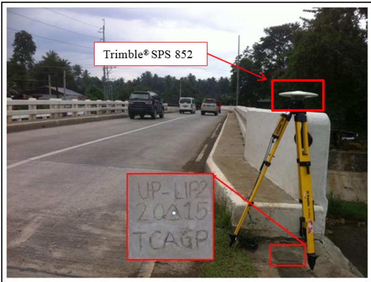
Figure 35. GNSS base receiver setup, Trimble® SPS 852 at UP-LIP2, on the right approach of Lipadas Bridge along National Highway in Brgy. Lizada, Toril District, Davao Del Sur
