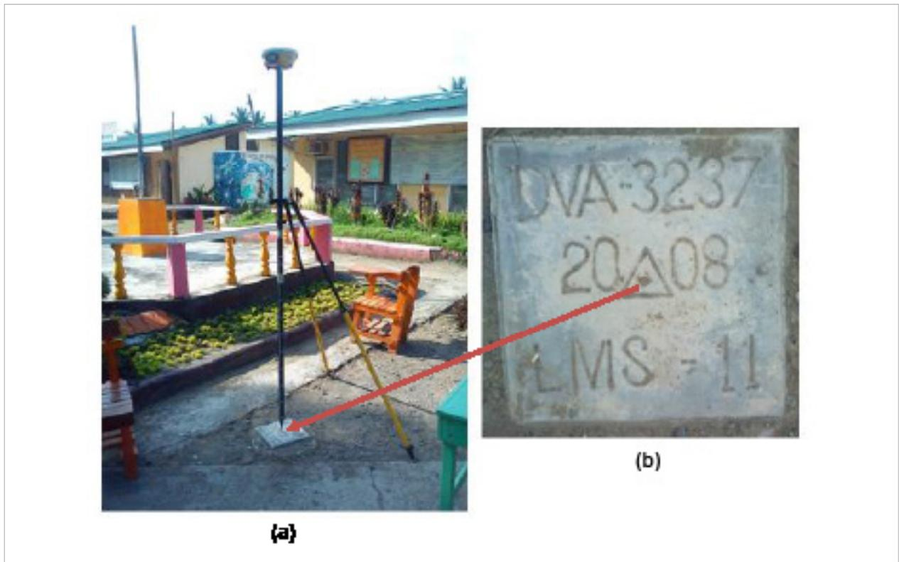
Figure 4. GPS set-up over DVA-3237 located beside the flagpole inside the compound of Nanyo Elementary School (a) and NAMRIA reference point DVA-3237 (b) as recovered by the field team.
