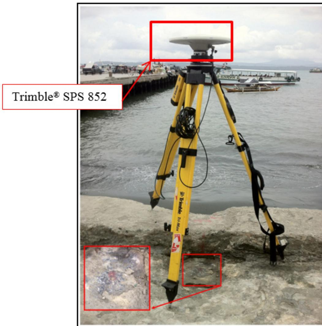
Figure 30. GNSS base receiver setup, Trimble® SPS 852 at DVS-1 at the east side of Pier, in Brgy. Leon Garcia Sr., Davao City, Davao Del Sur
