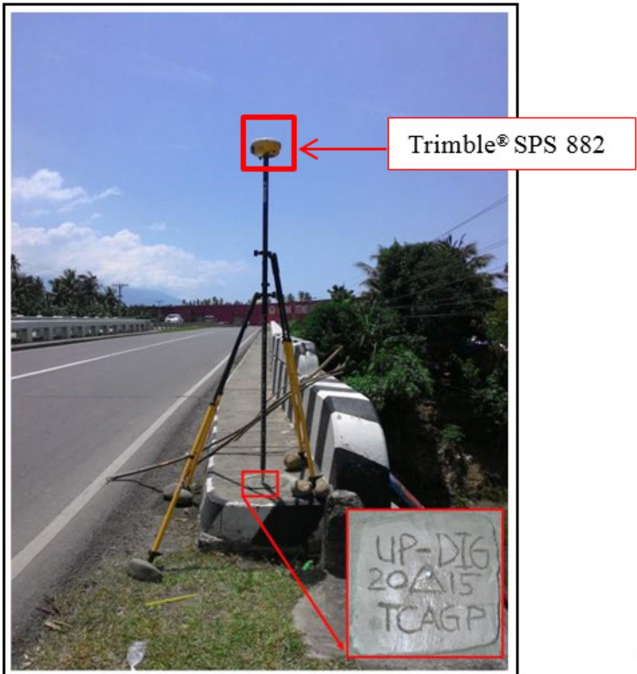
Figure 34. GNSS base receiver setup, Trimble® SPS 882 at UP-DIG, right approach of Digos Bridge in Brgy. Aplaya, Digos City, Davao Del Sur
