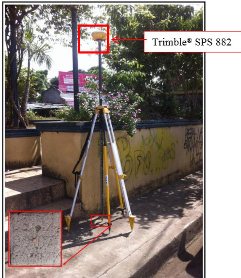
Figure 32. GNSS base receiver setup, Trimble® SPS 882 at DS-09 located at stair of Nograles Park along Mac Arthur Highway, in Brgy. Talomo, Davao City, Davao Del Sur
