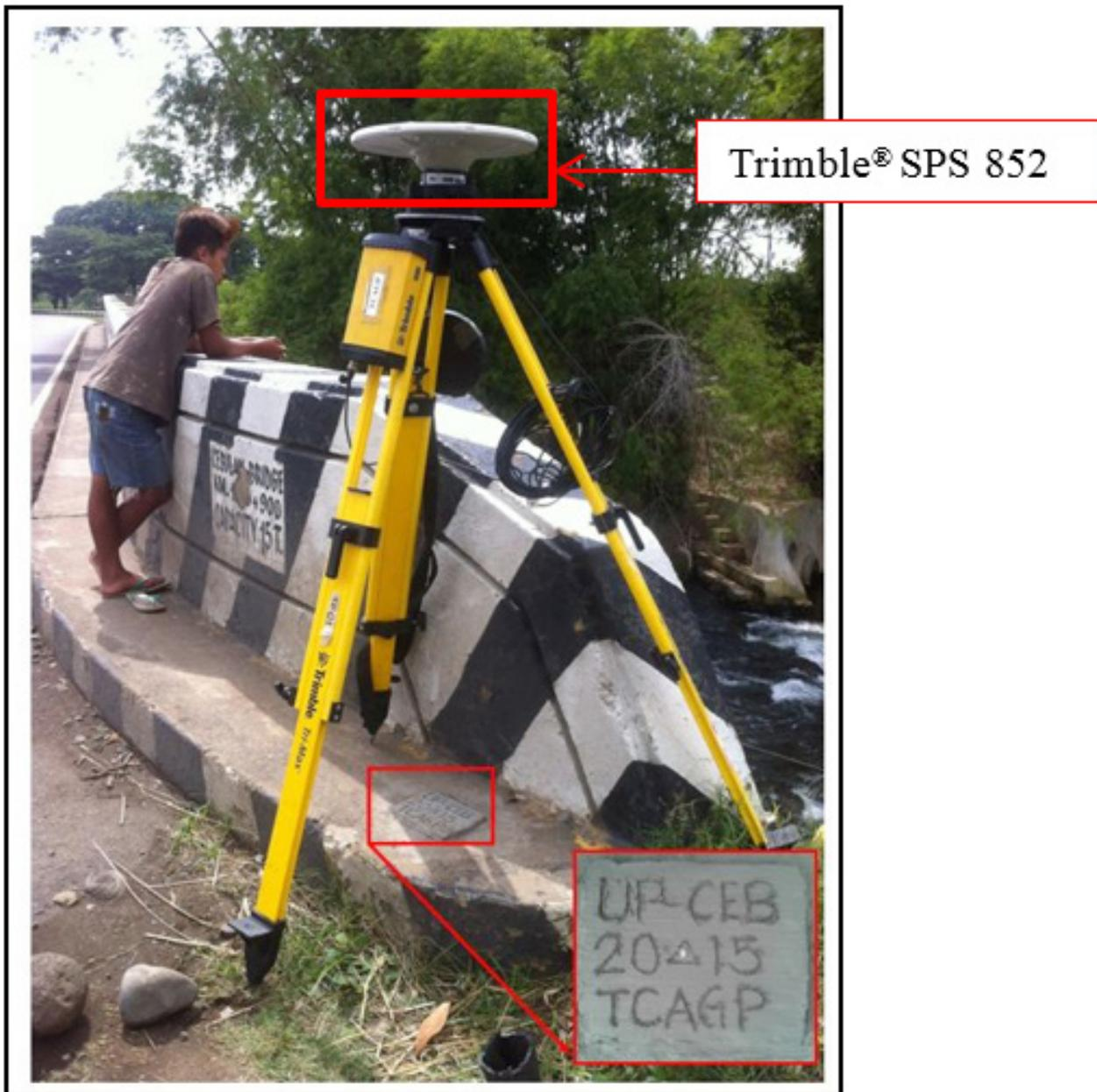
Figure 33. GNSS base receiver setup, Trimble® SPS 852 at UP-CEB on the right approach of Cebulan Bridge in Brgy Darong, Municipality of Santa Cruz, Davao Del Sur
