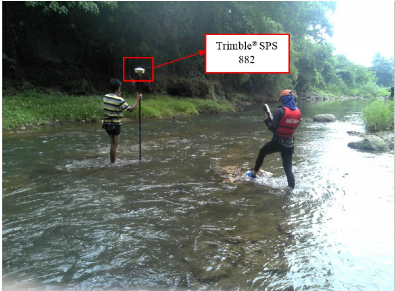
Figure 46. Bathymetric survey in Lipadas River.
