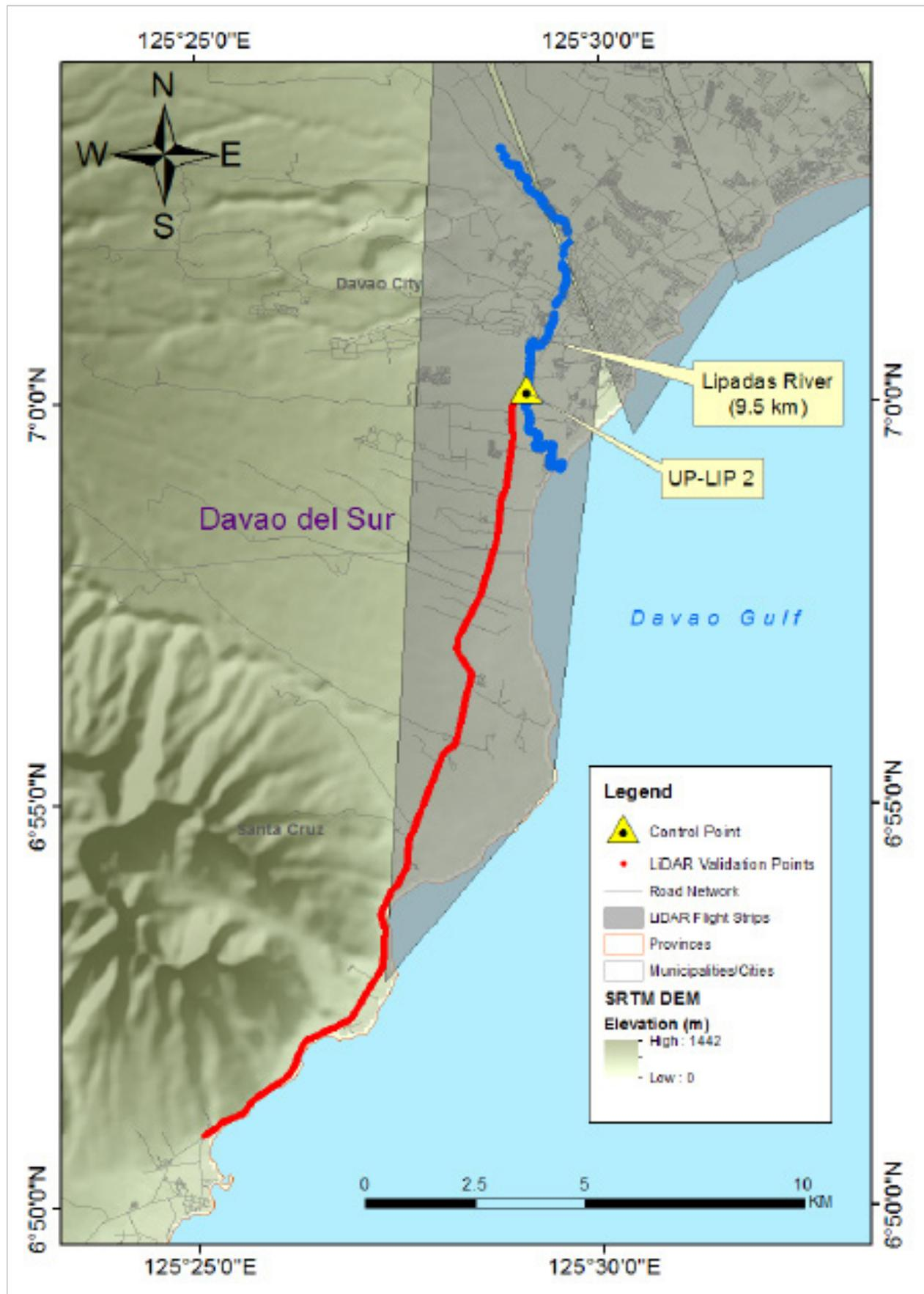
Figure 45 Validation points acquisition survey coverage for Lipadas River
