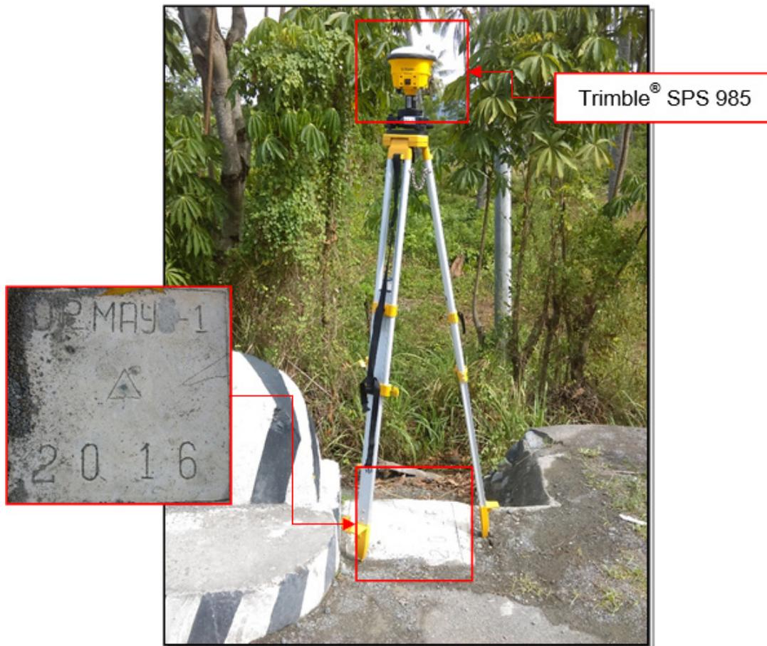
Figure 34. GNSS receiver set up, Trimble® SPS 985, at UP\_MAY-1, located beside the approach of Mayo Bridge in Brgy. Mayo, City of Mati, Province of Davao Oriental
