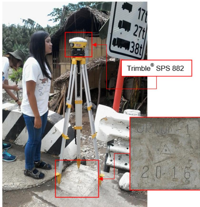
Figure 35. GNSS receiver set up, Trimble® SPS 882, at UP QUI-1, located beside the approach of Quinonoan Bridge in Brgy. San Ignacio, Municipality of Manay, Province of Davao Oriental
