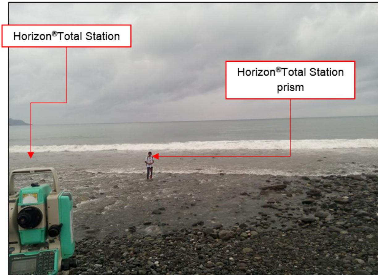
Figure 43. Manual bathymetric survey of ABSD at Bugnan Mayo River using Horizon<sup>®</sup> Total Station
