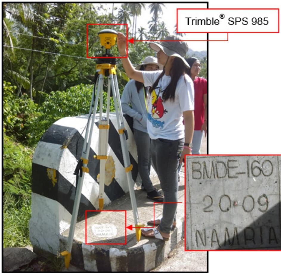
Figure 32. GNSS receiver set up, Trimble® SPS 985, at DE-160, located at approach of Calinan Bridge in Brgy. Mayo, City of Mati, Davao Oriental
