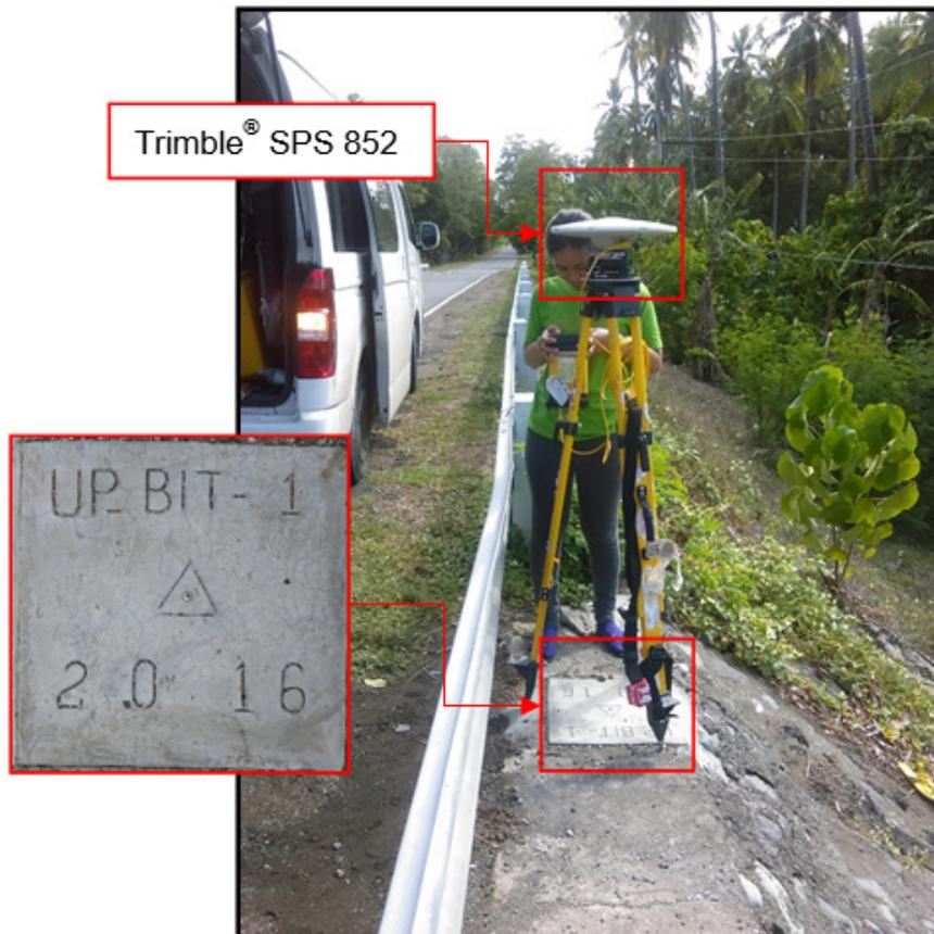
Figure 33. GNSS receiver set up, Trimble® SPS 852, at UP\_BIT-1, located at the side of the railing near the approach of Bitanagan Bridge in Brgy. Don Enrique Lopez, City of Mati, Davao Oriental
