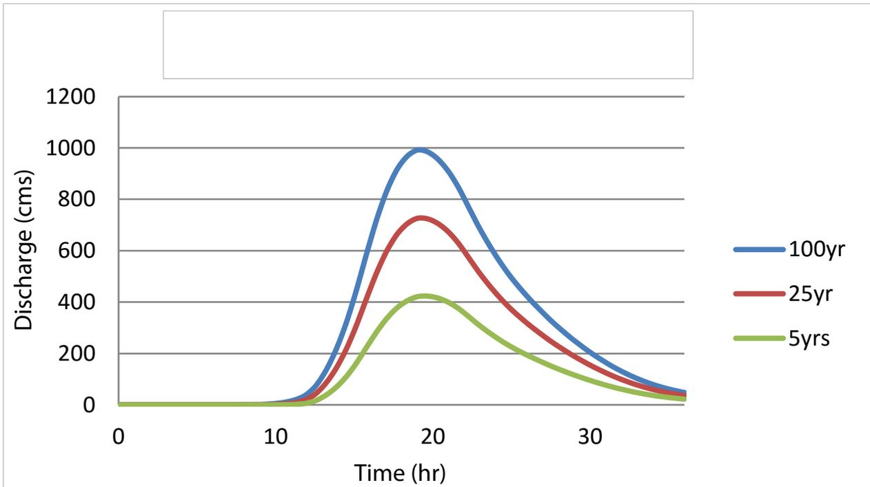
Figure 68. Digos Padada-Mainit river (8) generated discharge using 5-, 25-, and 100-year GenSan rainfall intensity-duration-frequency (RIDF) in HEC-HMS
