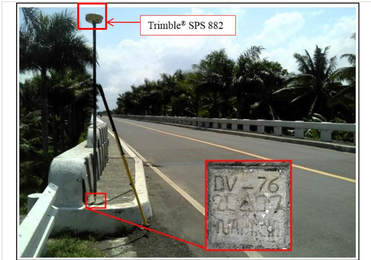
Figure 30. GNSS base receiver setup, Trimble® SPS 882 at DV-76 at the Gov. Miranda Bridge Approach, Brgy. Guadalupe, Municipality of Carmen, Davao Del Norte
