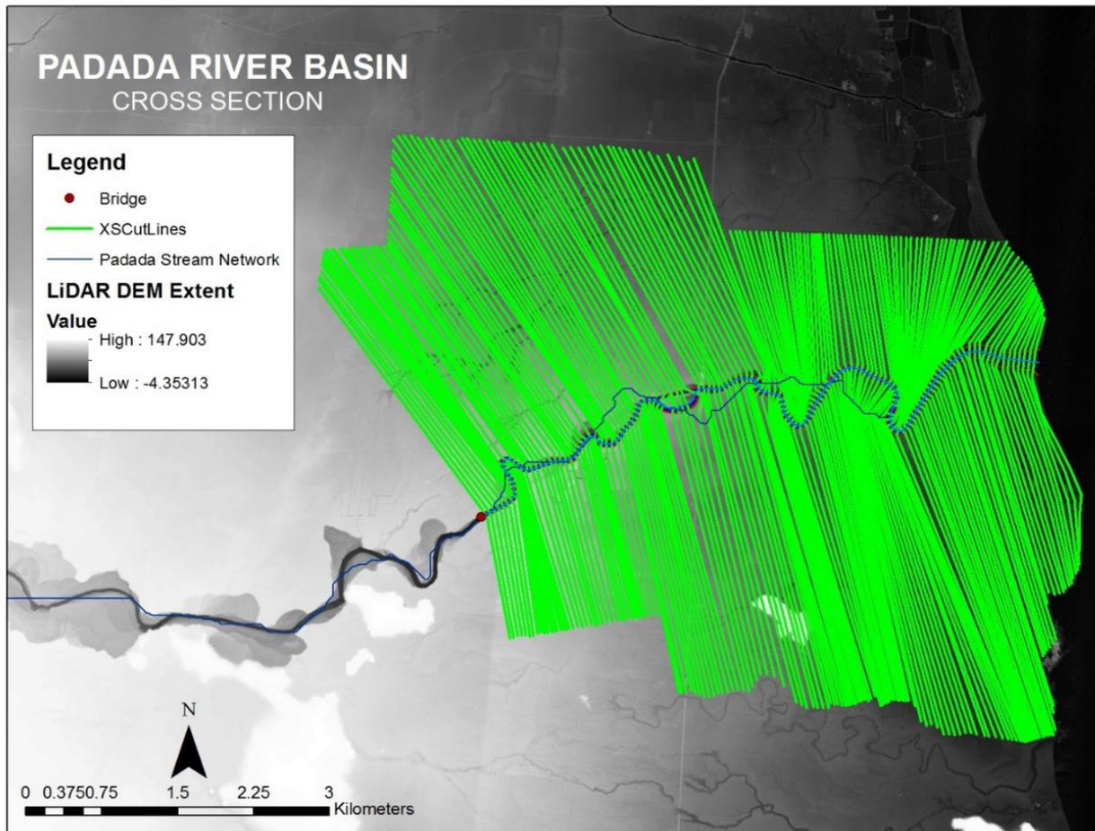
Figure 57. River cross-section of Padada River generated through Arcmap HEC GeoRAS tool
