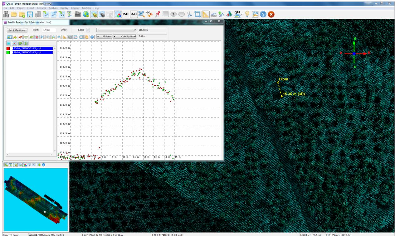
Figure 15. Quality checking for a Padada flight 7418GC using the Profile Tool of QT Modeler.
