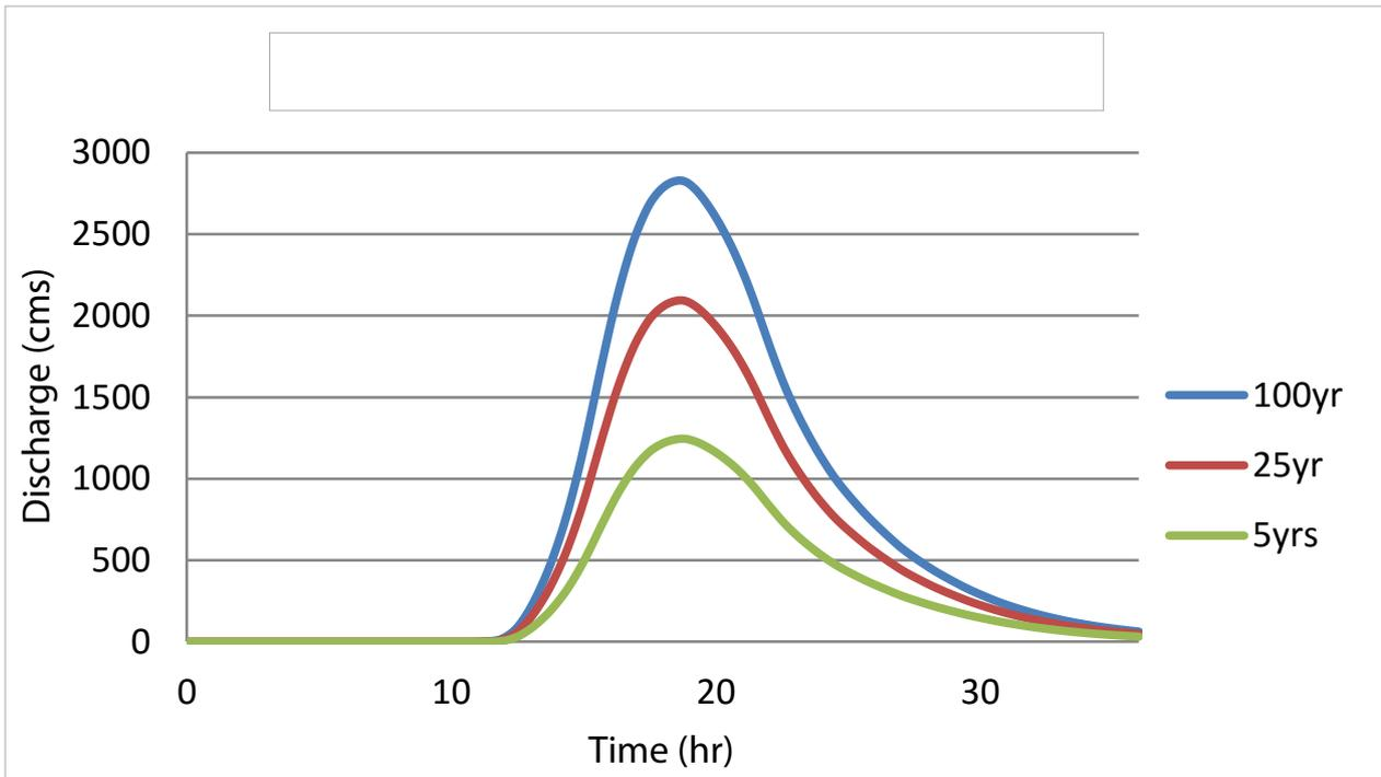
Figure 67. Digos Padada-Mainit river (7) generated discharge using 5-, 25-, and 100-year GenSan rainfall intensity-duration-frequency (RIDF) in HEC-HMS
