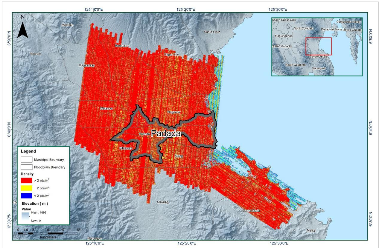
Figure 13. Density map of merged LiDAR data for Padada floodplain.
