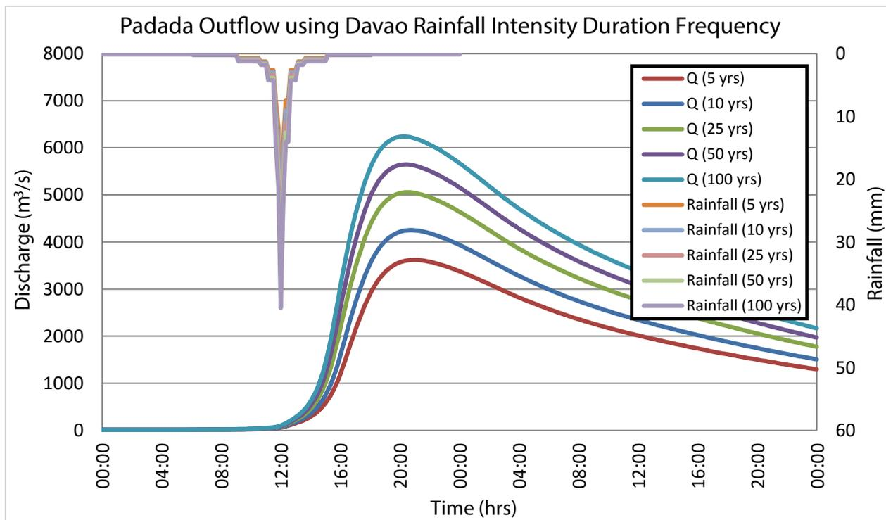
Figure 60. Outflow hydrograph at Padada Station generated using the Davao RIDF simulated in HEC-HMS.
