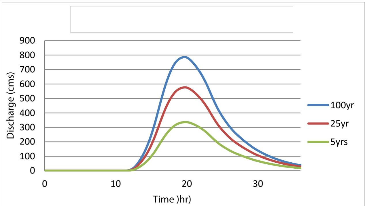
Figure 65. Digos Padada-Mainit river (5) generated discharge using 5-, 25-, and 100-year GenSan rainfall intensity-duration-frequency (RIDF) in HEC-HMS
