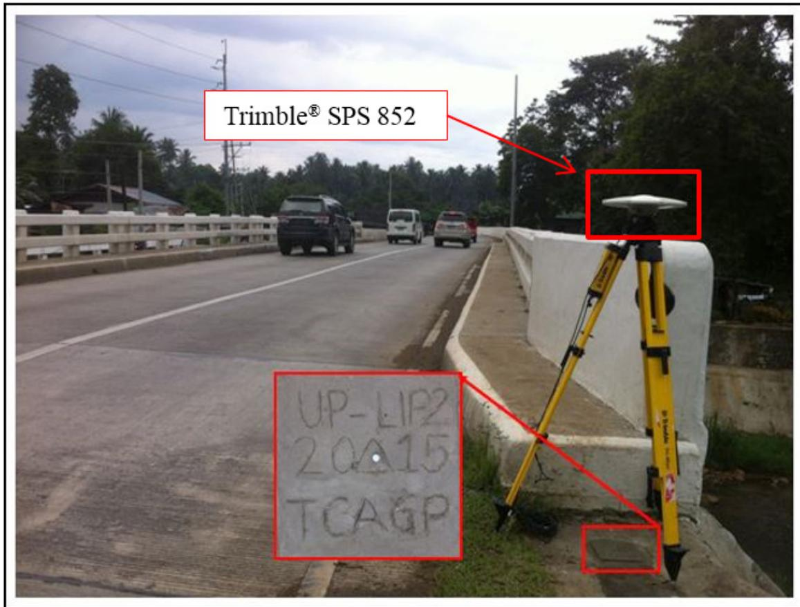
Figure 34. GNSS base receiver setup, Trimble® SPS 852 at UP-LIP2, on the right approach of Lipadas Bridge along National Highway in Brgy. Lizada, Toril District, Davao Del Sur
