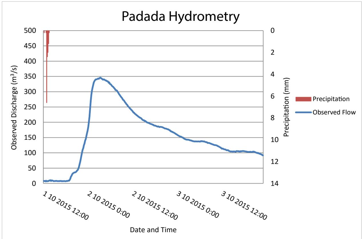
Figure 49. Rainfall and outflow data at Tologan Bridge used for modeling
