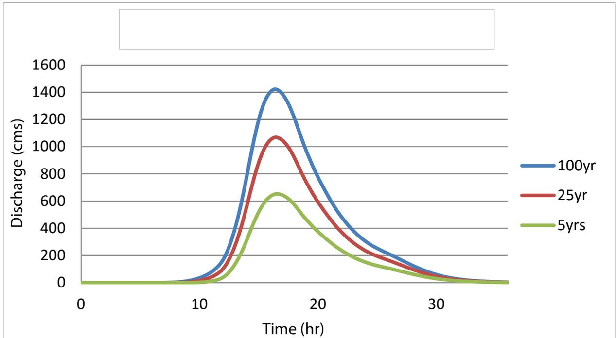
Figure 70. Digos Padada-Mainit river (10) generated discharge using 5-, 25-, and 100-year GenSan rainfall intensity-duration-frequency (RIDF) in HEC-HMS
