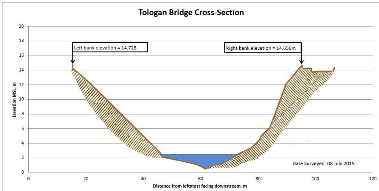
Figure 47. Cross-Section Plot of Tologan Bridge
