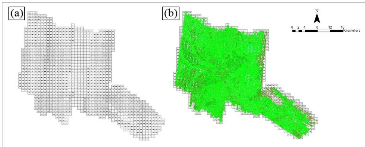
Figure 16. Tiles for Padada floodplain (a) and classification results (b) in TerraScan.
