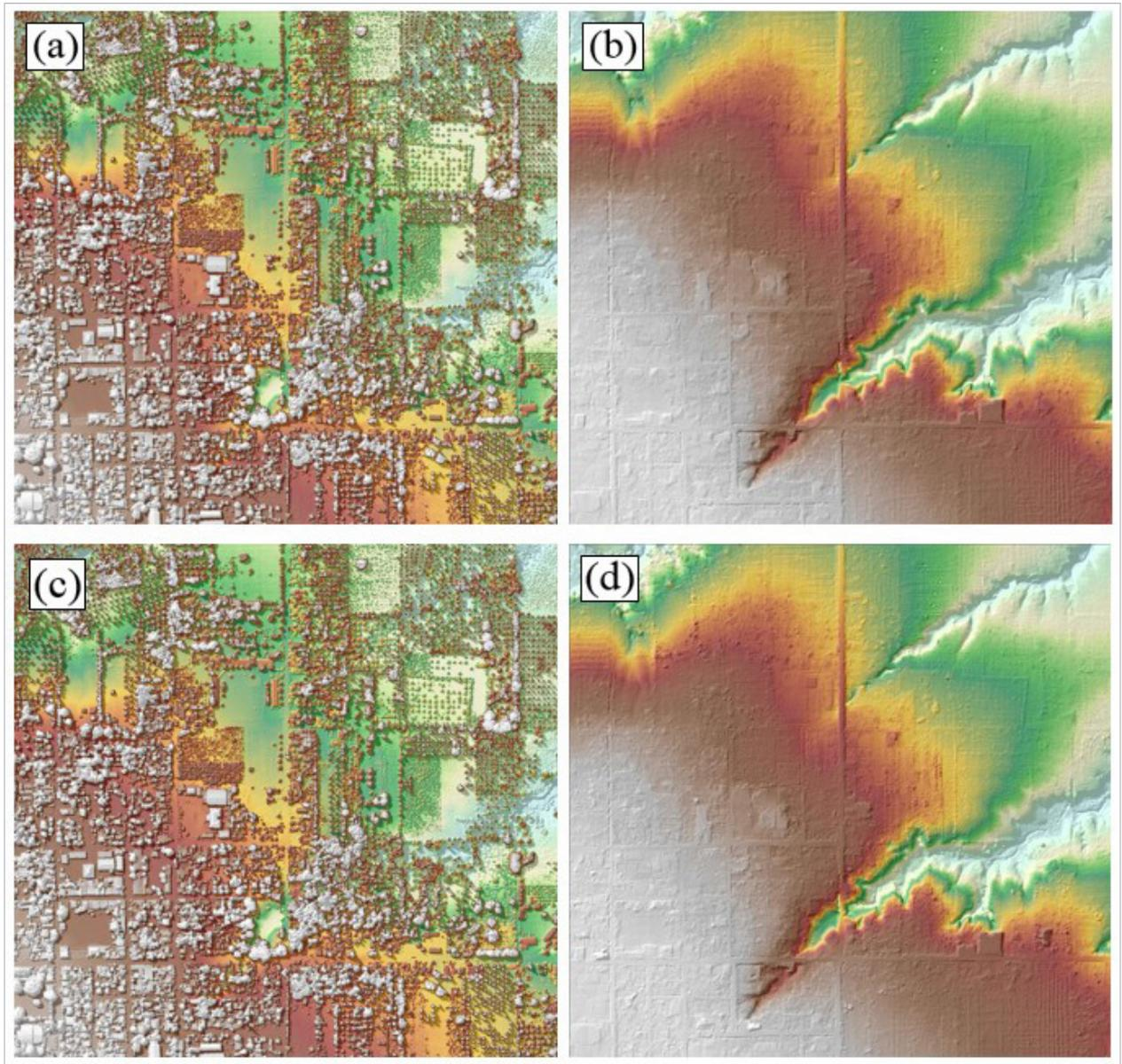
Figure 18. The production of last return DSM (a) and DTM (b), first return DSM (c) and secondary DTM (d) in some portion of Padada floodplain.
