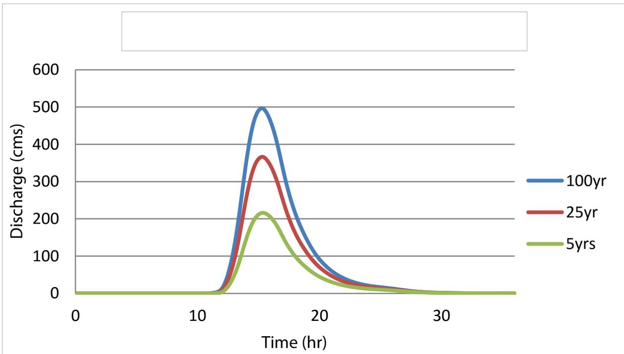
Figure 63. Digos Padada-Mainit river (3) generated discharge using 5-, 25-, and 100-year GenSan rainfall intensity-duration-frequency (RIDF) in HEC-HMS
