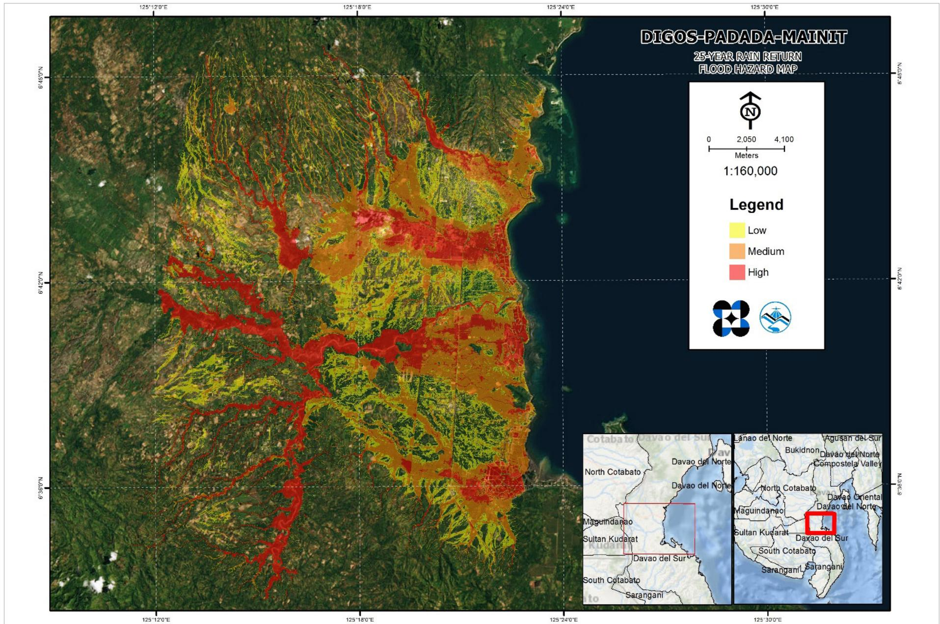
Figure 74. 25-year Flood Hazard Map for Padada Floodplain overlaid on Google Earth imagery
