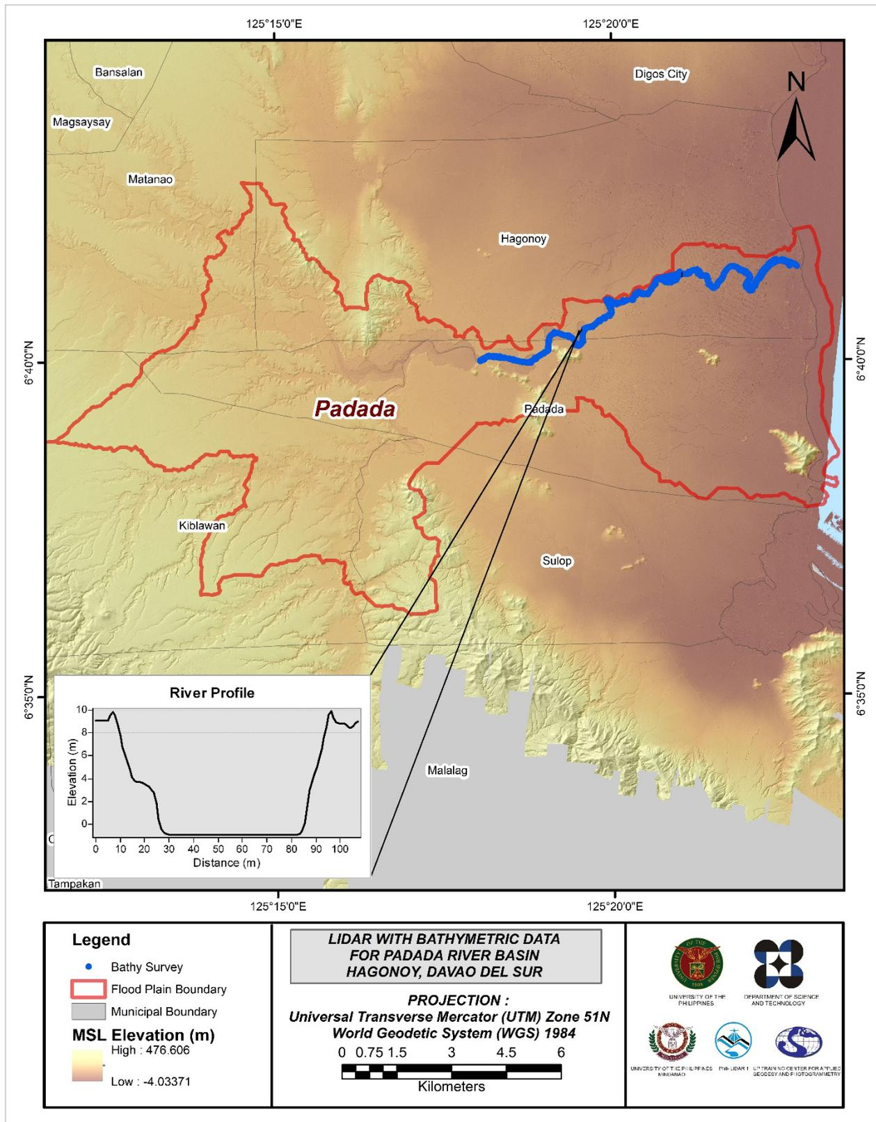
Figure 24. Map of Padada Flood Plain with bathymetric survey points shown in blue.
