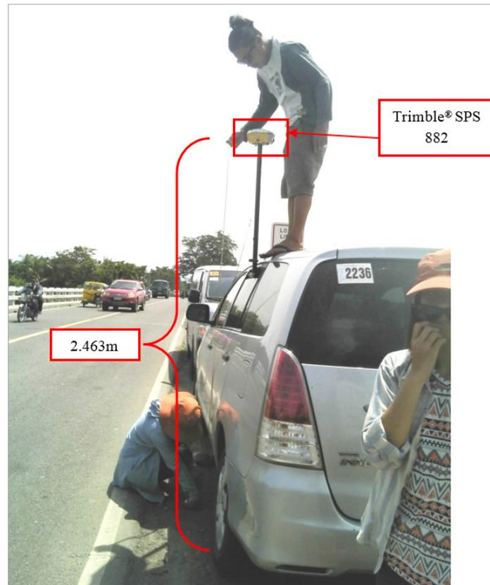
Figure 41. Validation points acquisition survey set-up for Davao del Sur.
