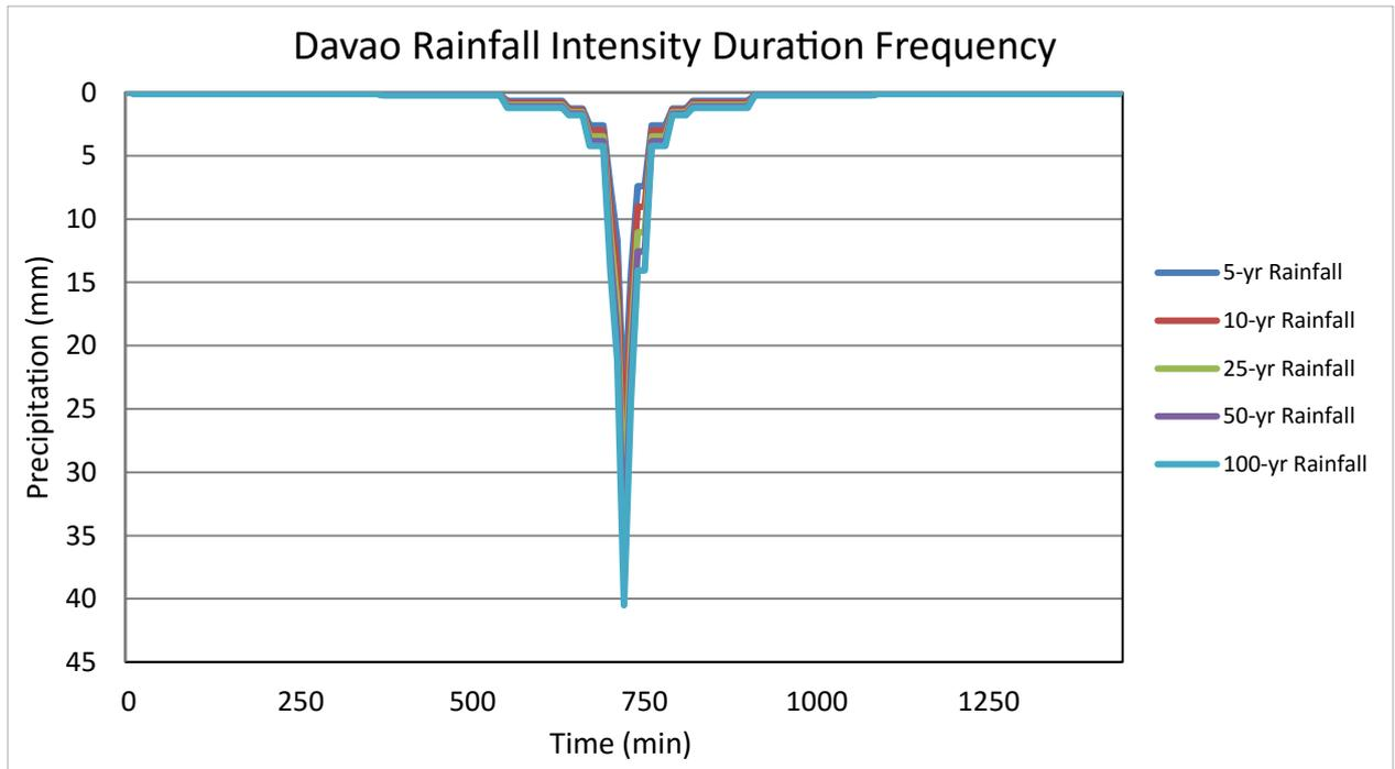
Figure 51. Synthetic storm generated for a 24-hr period rainfall for various return periods
