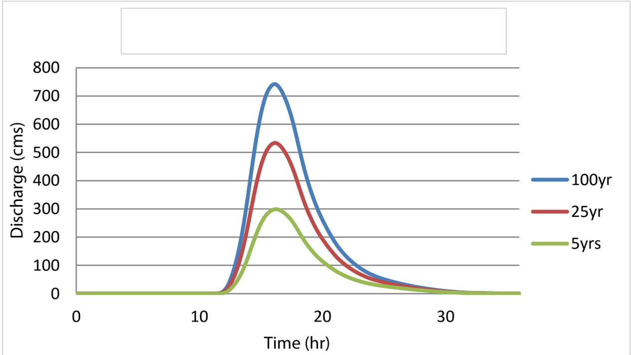
Figure 61. Digos Padada-Mainit river (1) generated discharge using 5-, 25-, and 100-year GenSan rainfall intensity-duration-frequency (RIDF) in HEC-HMS
