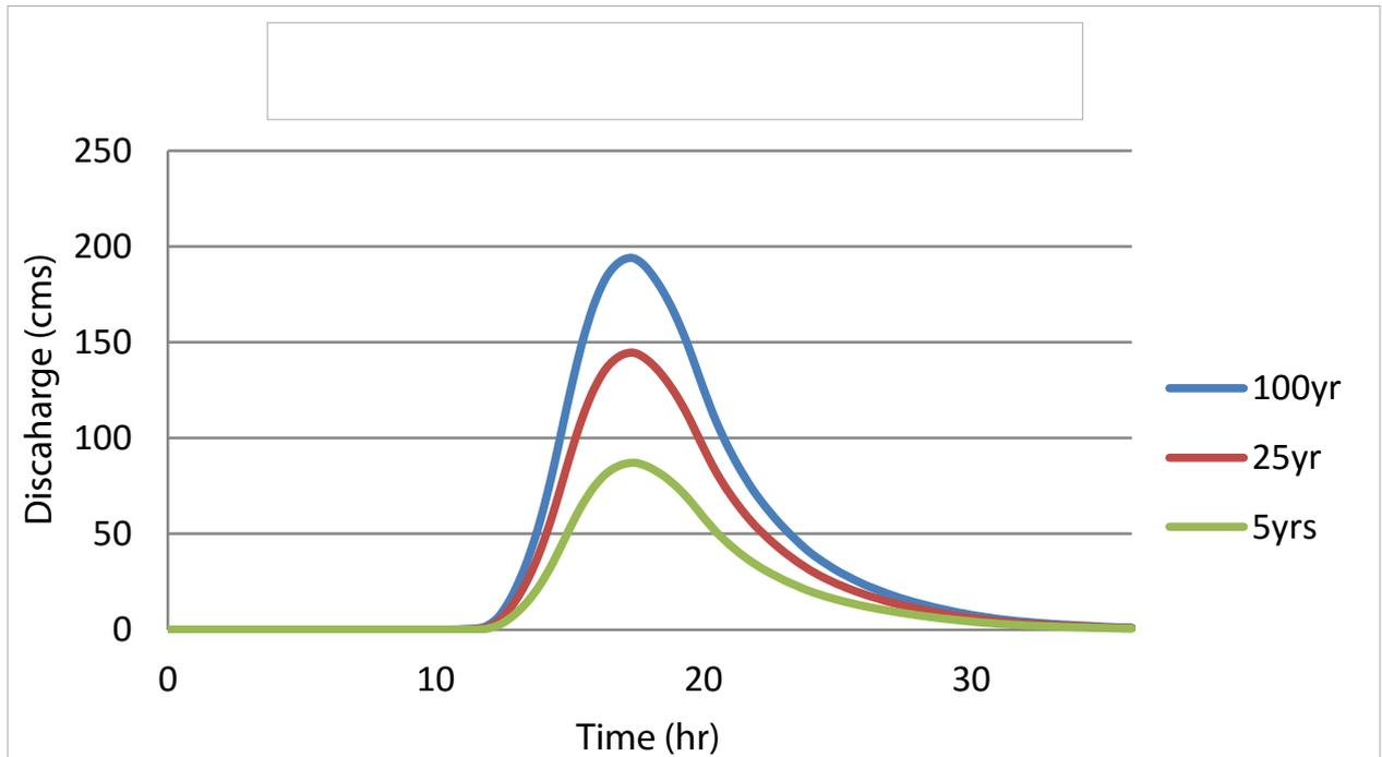
Figure 66. Digos Padada-Mainit river (6) generated discharge using 5-, 25-, and 100-year GenSan rainfall intensity-duration-frequency (RIDF) in HEC-HMS
