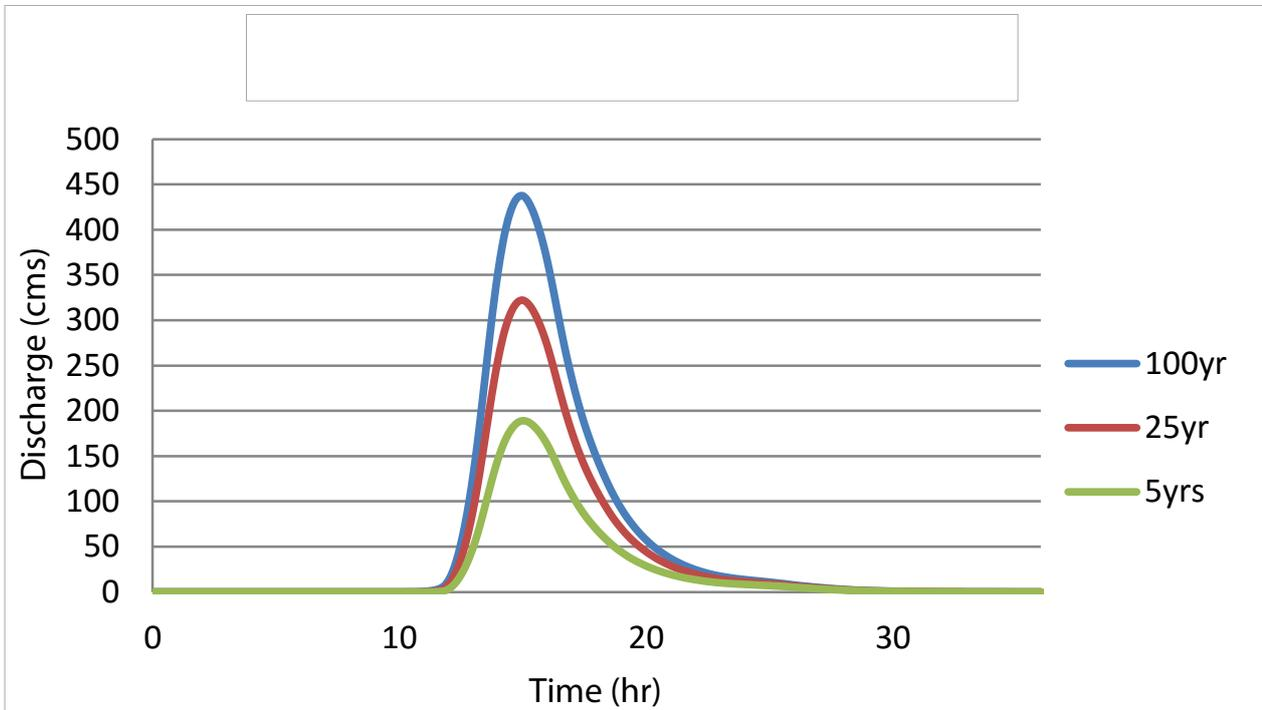
Figure 64. Digos Padada-Mainit river (4) generated discharge using 5-, 25-, and 100-year GenSan rainfall intensity-duration-frequency (RIDF) in HEC-HMS
