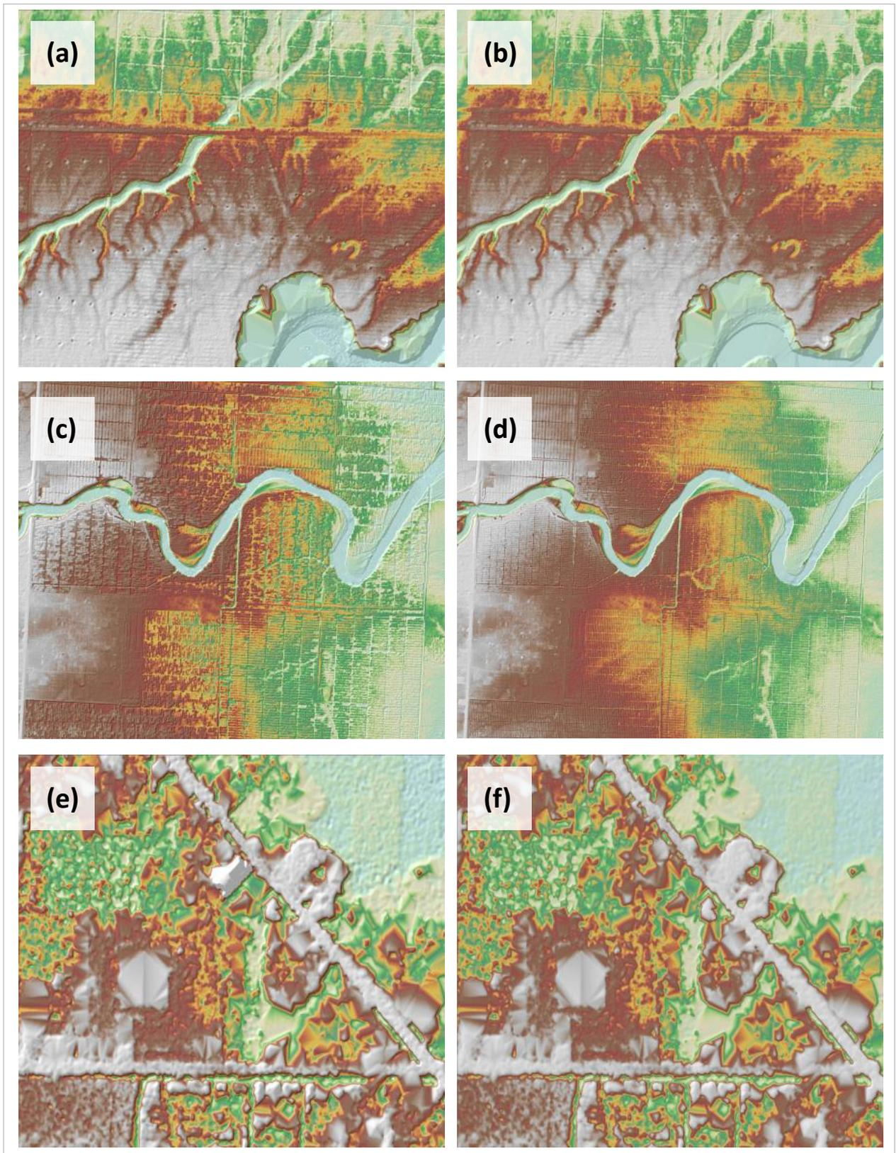
Figure 19. Portions in the DTM of Padada floodplain – a bridge before (a) and after (b) manual editing; a paddy field before (c) and after (d) data retrieval; and a building before (e) and after (f) manual editing.
