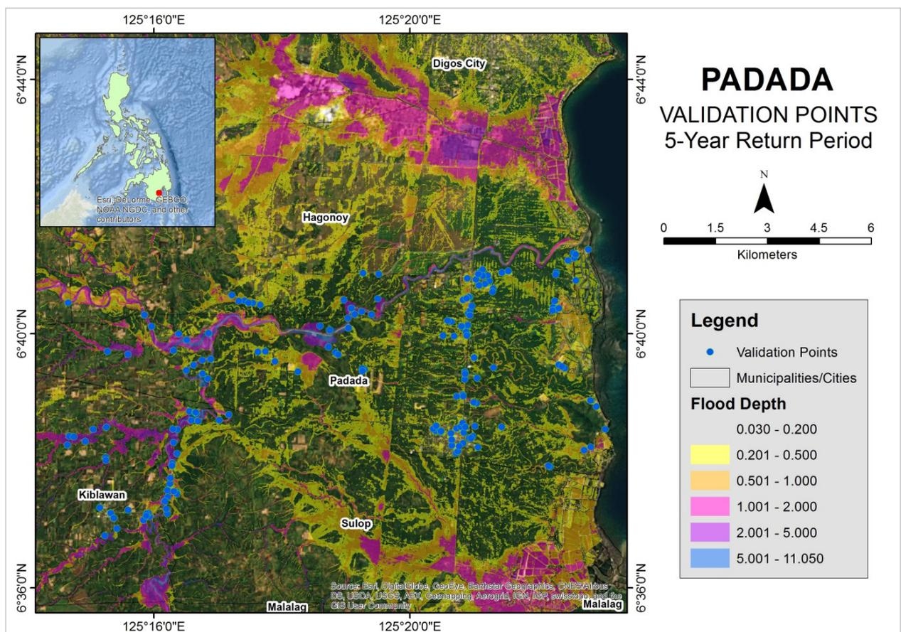
Figure 138. Flood Validation Points of Padada River Basin
