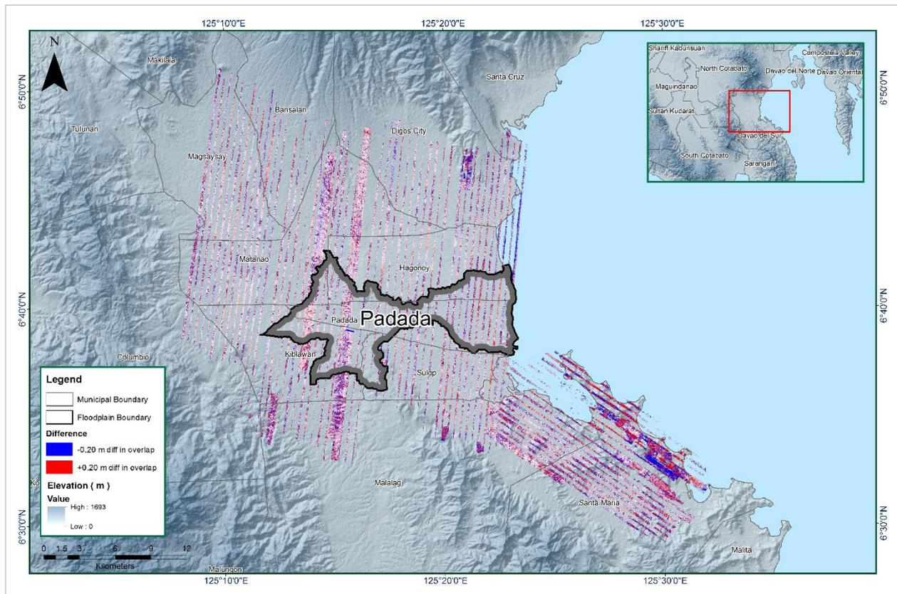
Figure 14. Elevation difference map between flight lines for Padada floodplain.
