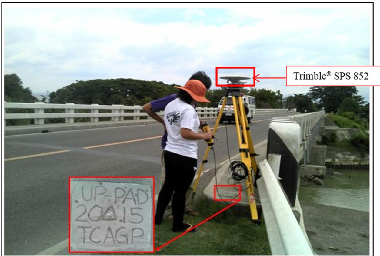
Figure 35. GNSS base receiver setup, Trimble® SPS 882 at UP-PAD, Padada Bridge, Brgy. Guihing, Municipality of Hagonoy, Davao del Sur
