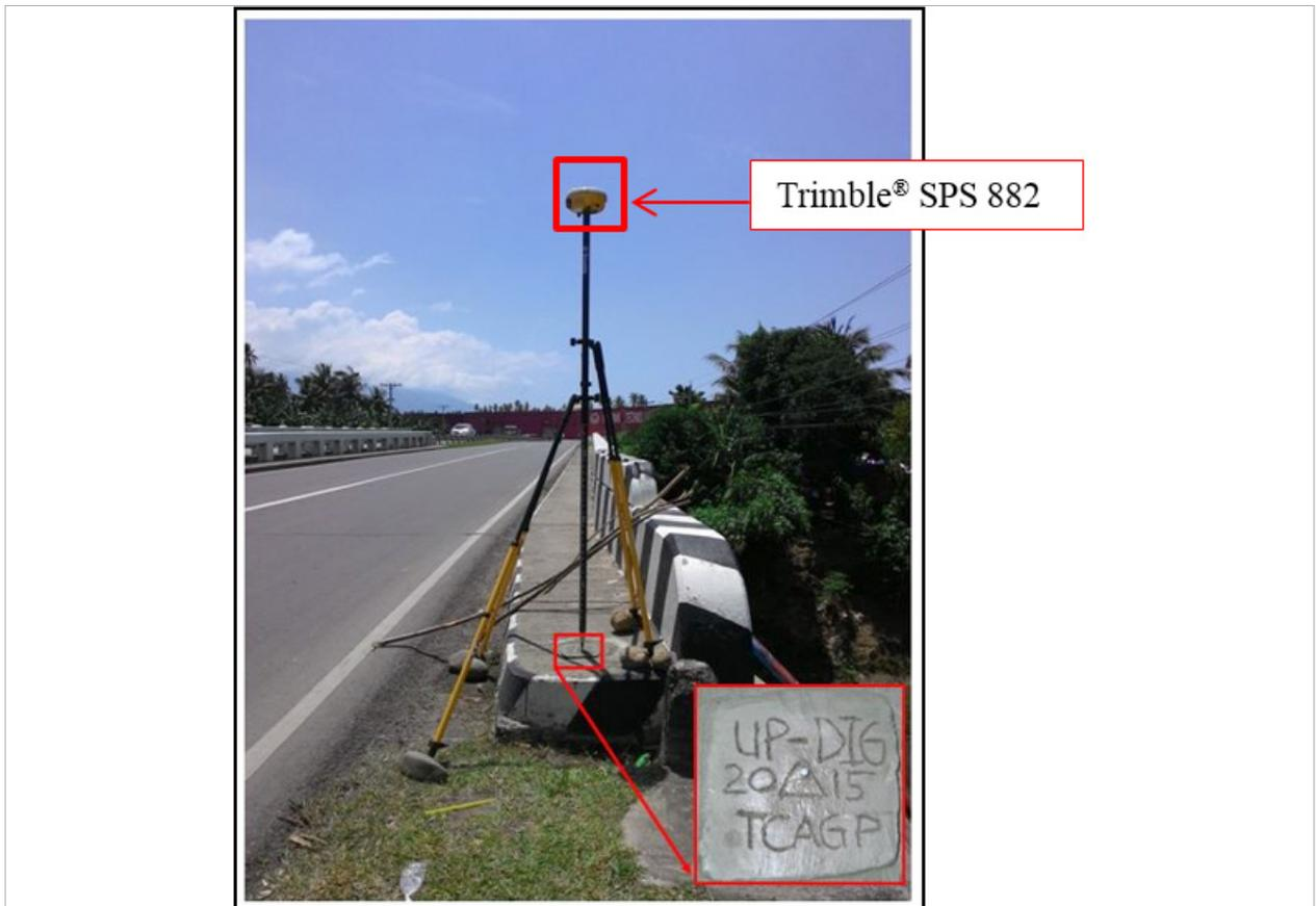
Figure 33. GNSS base receiver setup, Trimble® SPS 882 at UP-DIG, right approach of Digos Bridge in Brgy. Aplaya, Digos City, Davao Del Sur
