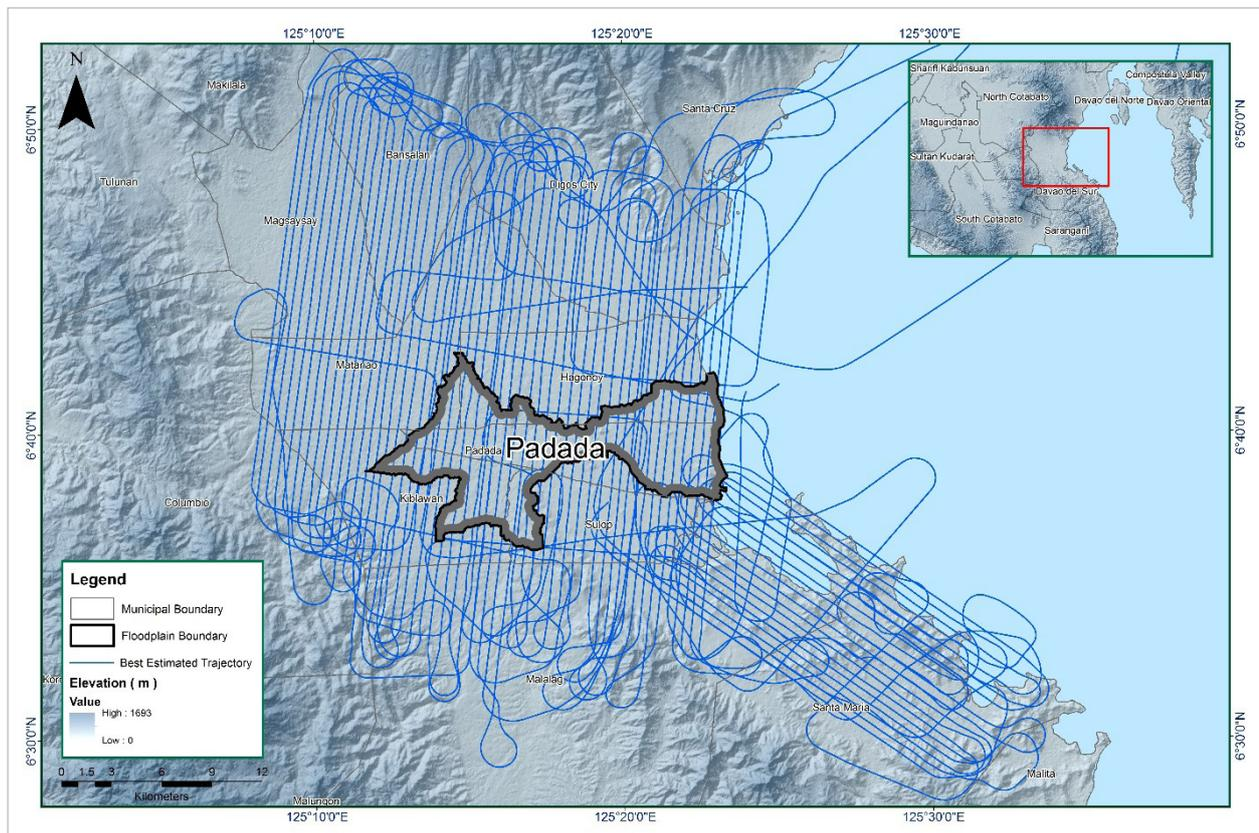
Figure 10. Best estimated trajectory for the Padada floodplain.
