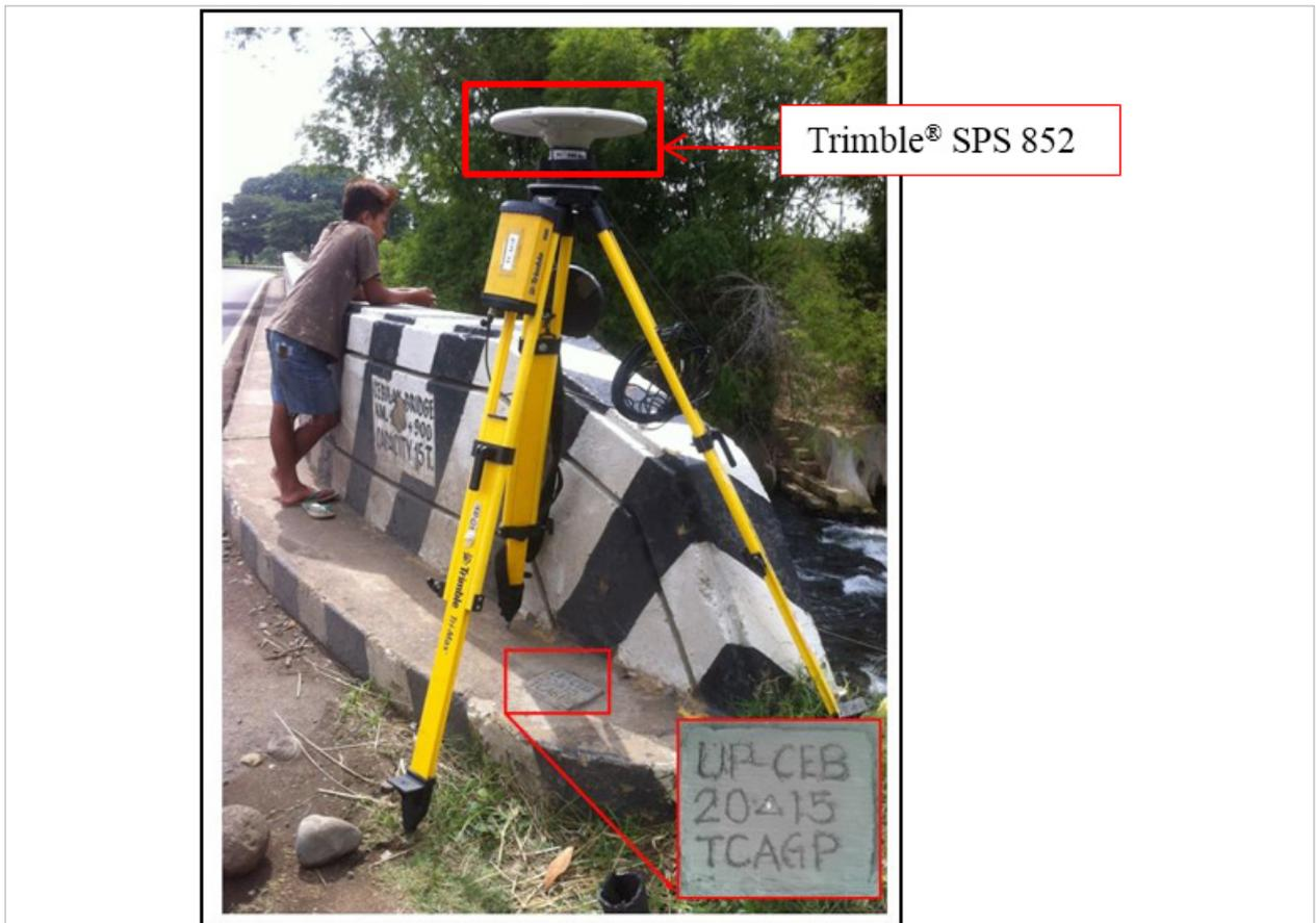
Figure 32. GNSS base receiver setup, Trimble® SPS 852 at UP-CEB on the right approach of Cebulan Bridge in Brgy Darong, Municipality of Santa Cruz, Davao Del Sur
