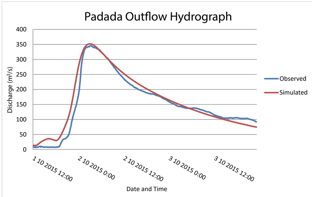
Figure 59. Outflow Hydrograph of Padada produced by the HEC-HMS model compared with observed outflow
