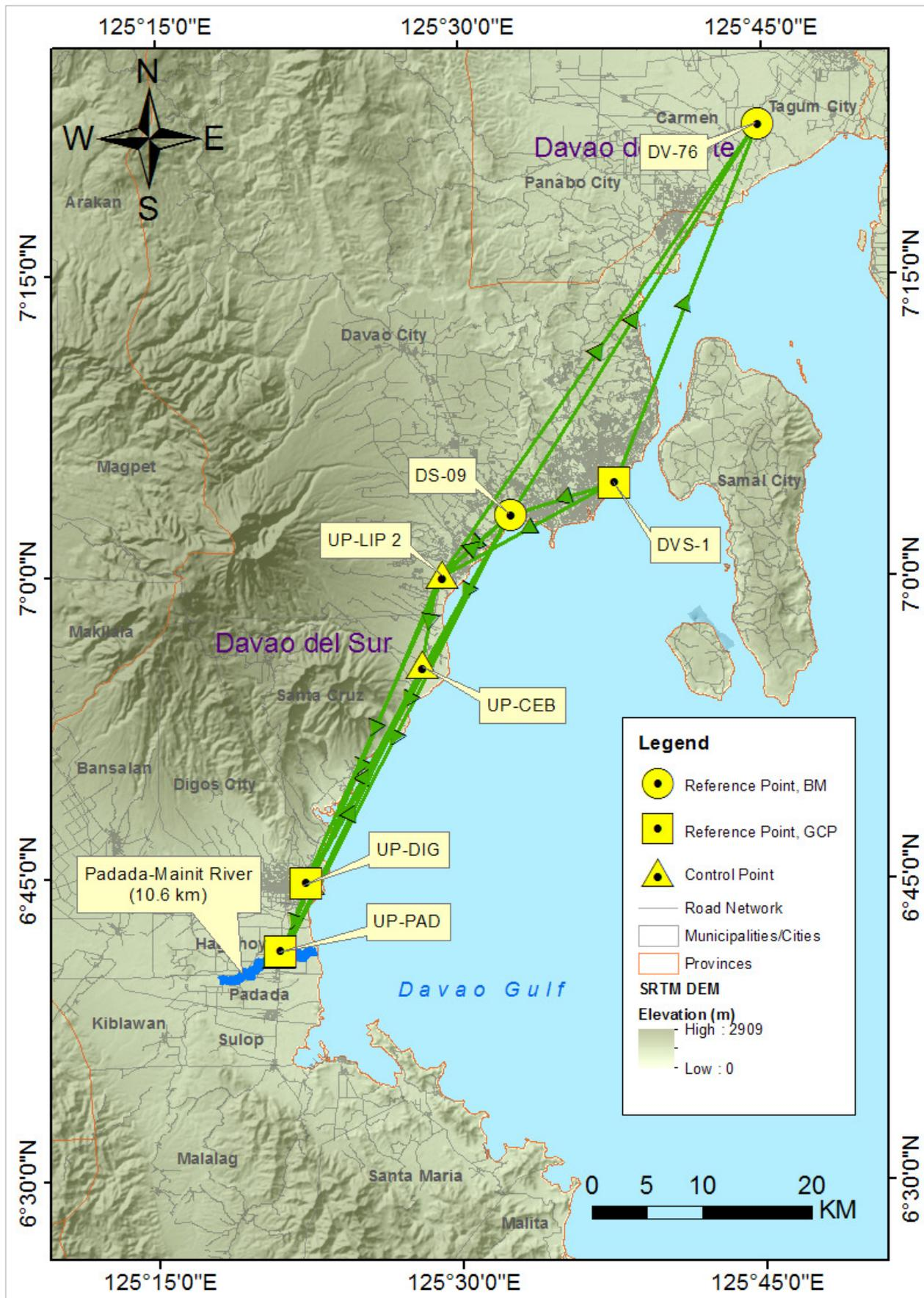
Figure 28. Overall GNSS Survey loop of Padada Mainit River Basin
