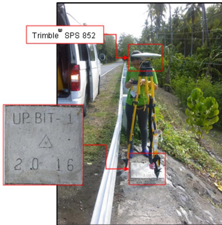
Figure 32. GNSS receiver set up, Trimble® SPS 852, at UP\_BIT-1, located at the side of the railing near the approach of Bitanagan Bridge in Brgy. Don Enrique Lopez, City of Mati, Davao Oriental.
