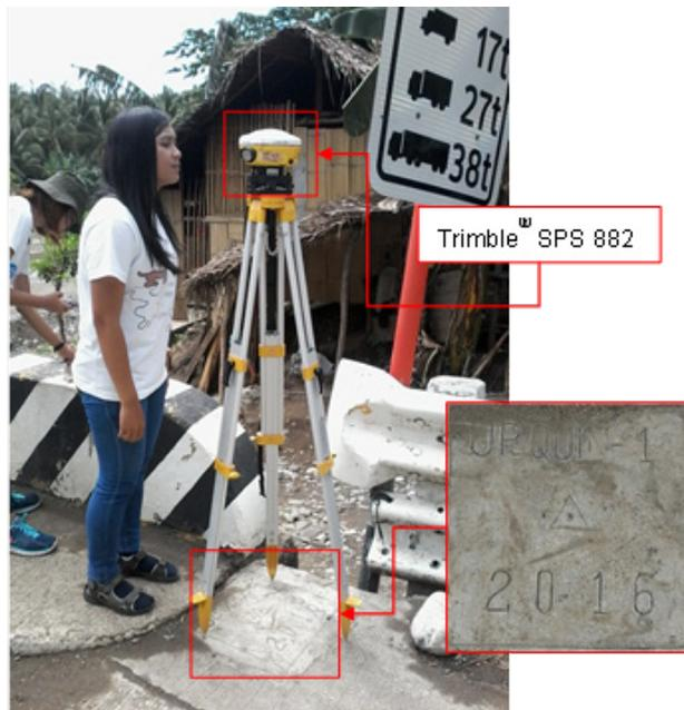
Figure 34. GNSS receiver set up, Trimble® SPS 882, at UP QUI-1, located beside the approach of Quinonoan Bridge in Brgy. San Ignacio, Municipality of Manay, Province of Davao Oriental.
