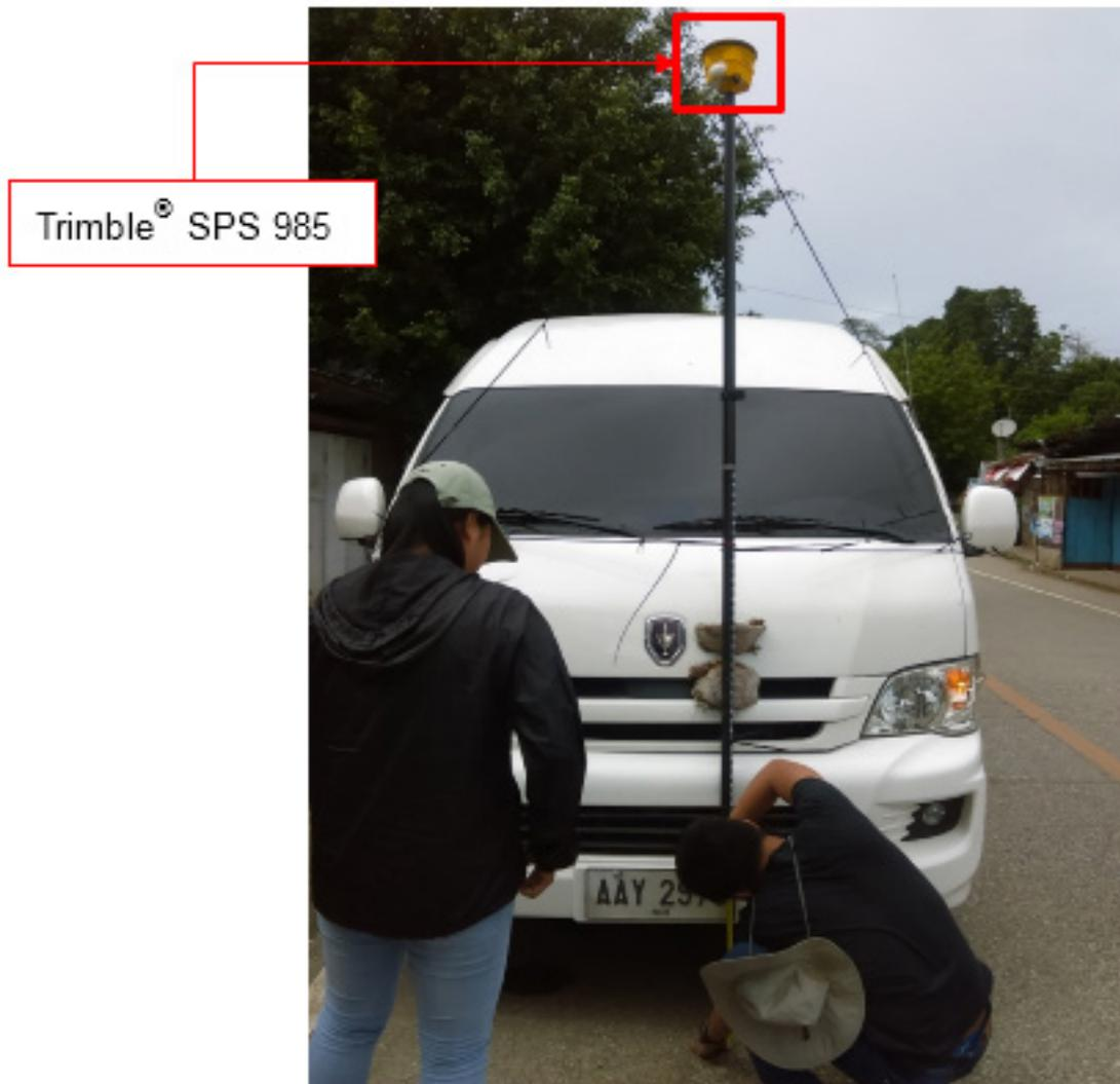
Figure 41. GNSS Rover receiver, Trimble® SPS 985 installed on a vehicle for Ground Validation Survey.
