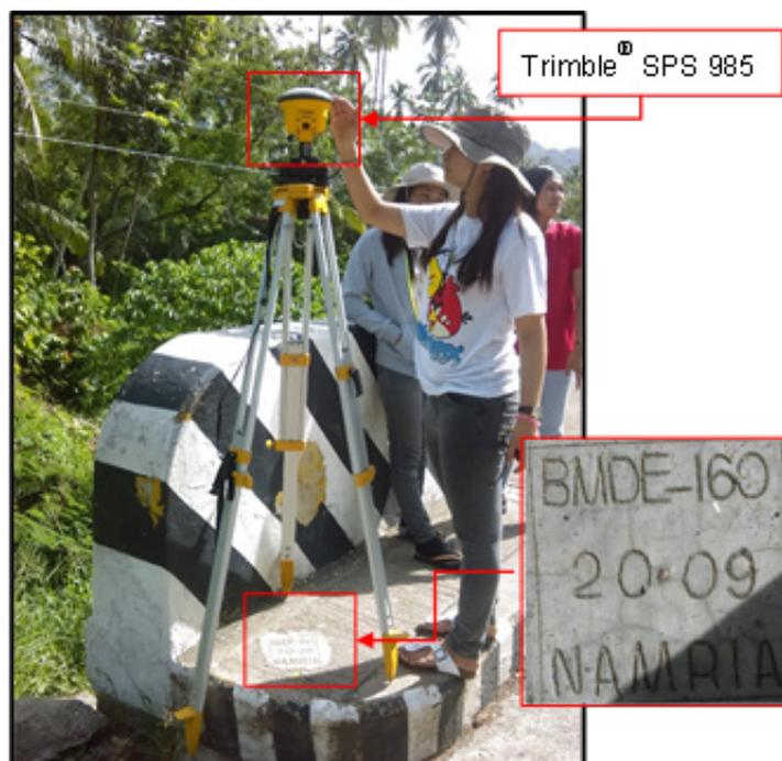
Figure 31. GNSS receiver set up, Trimble® SPS 985, at DE-160, located at approach of Calinan Bridge in Brgy. Mayo, City of Mati, Davao Oriental.
