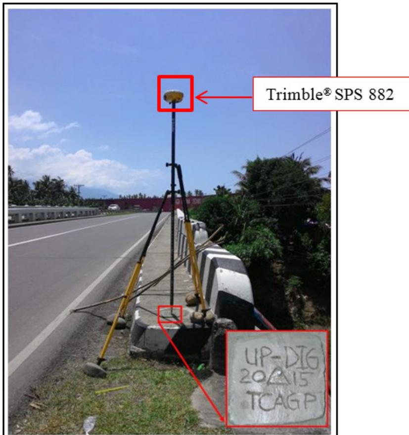
Figure 35. GNSS base receiver setup, Trimble® SPS 882 at UP-DIG, right approach of Digos Bridge in Brgy. Aplaya, Digos City, Davao Del Sur
