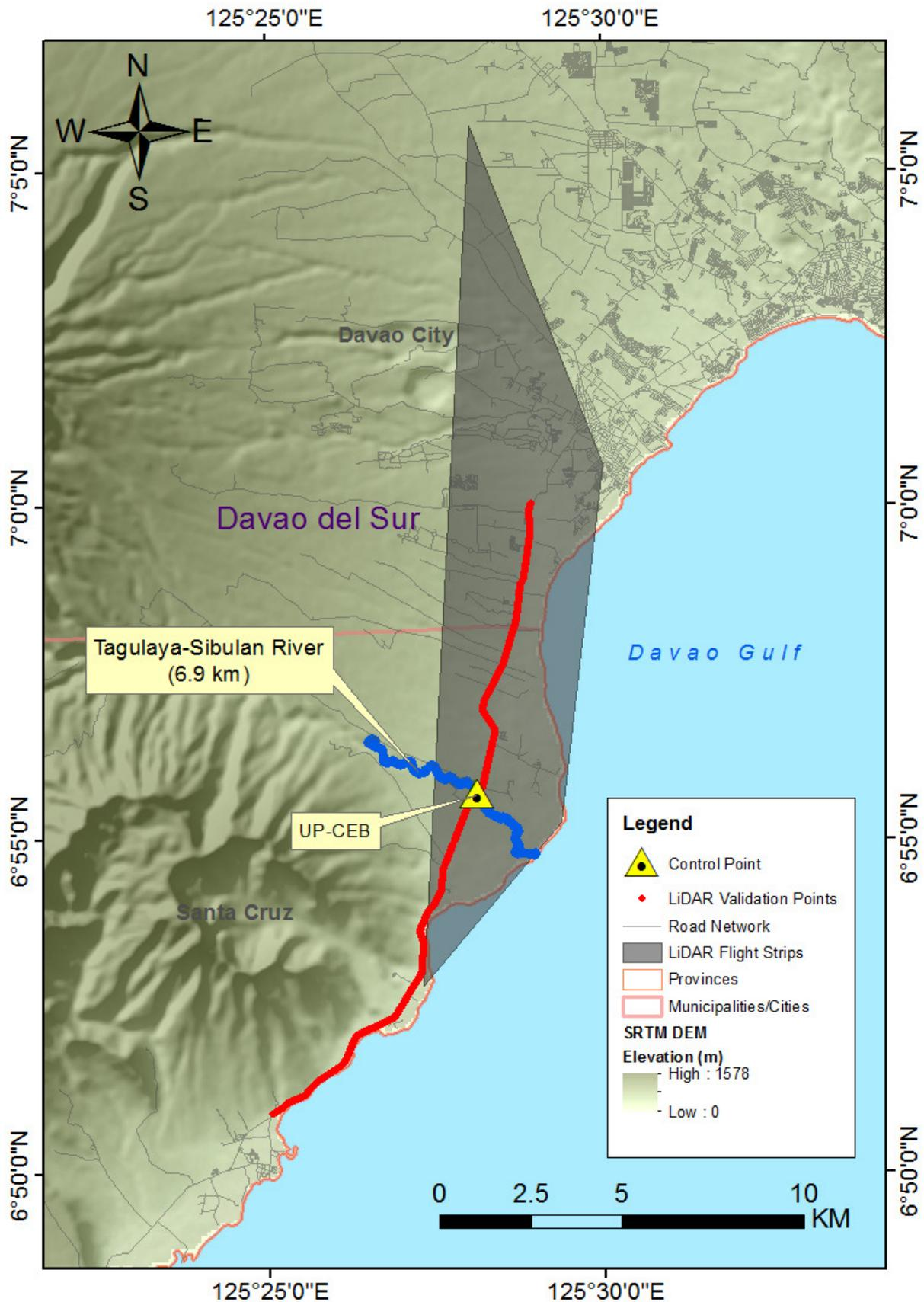
Figure 44. Validation point acquisition survey of Sibulan River Basin
