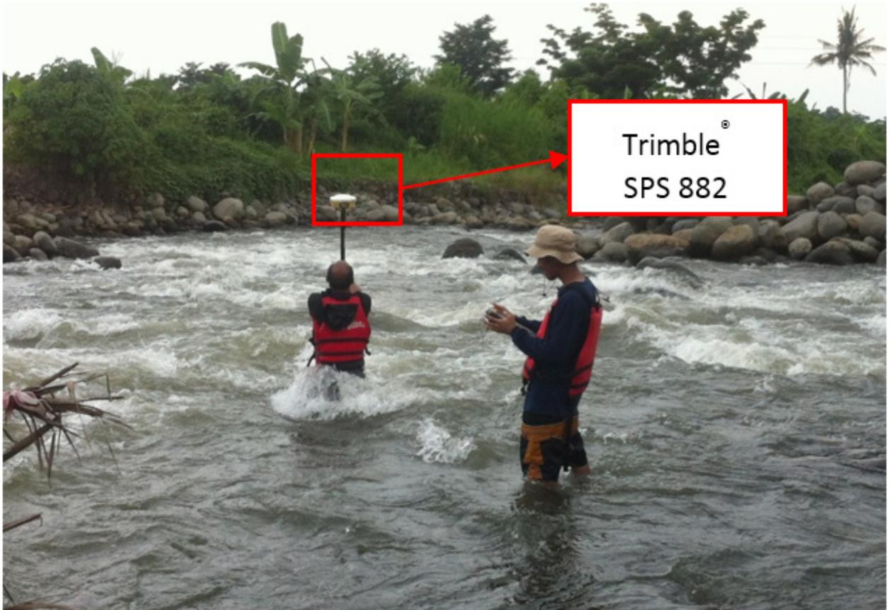
Figure 45. Bathymetric survey in Sibulan River
