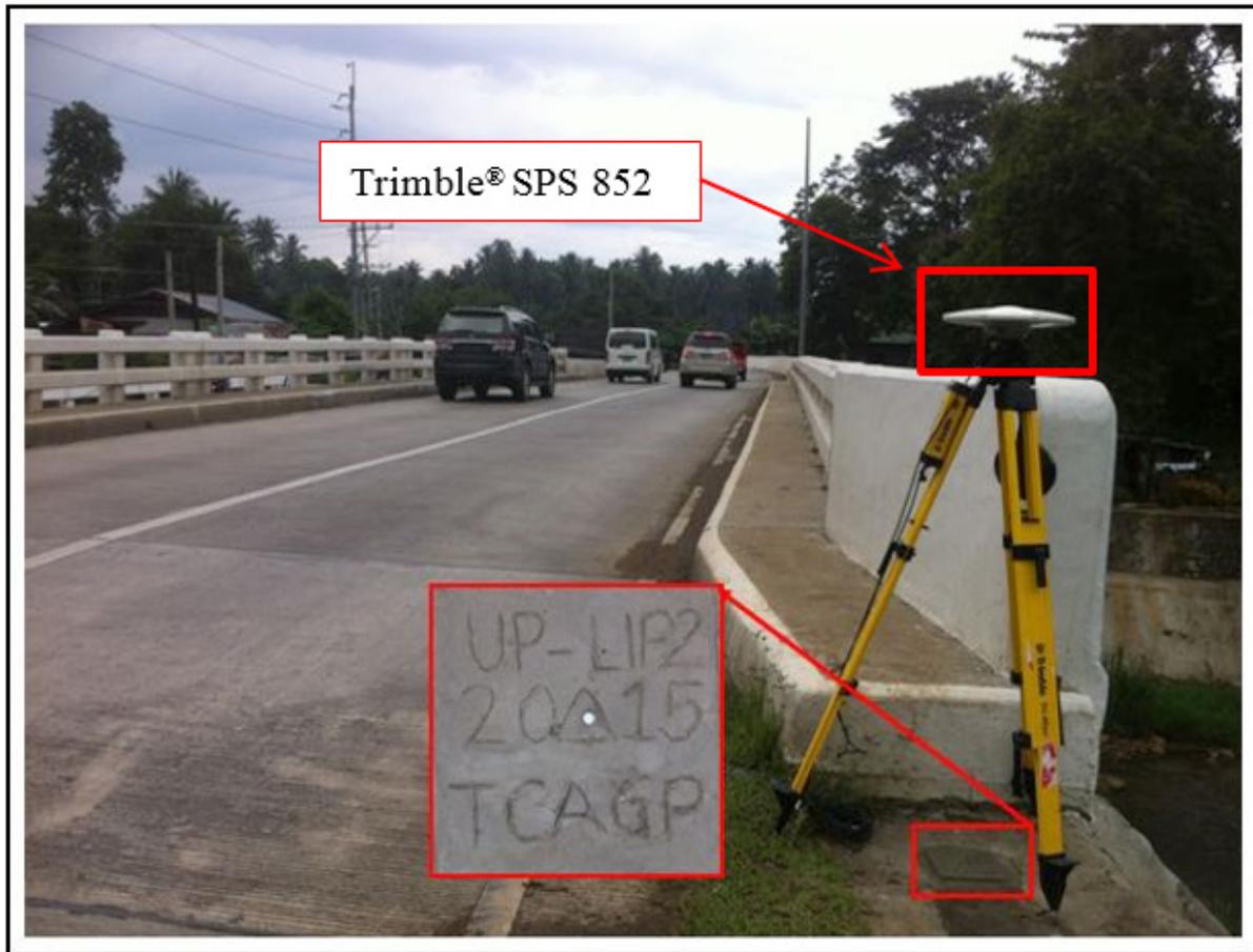
Figure 36. GNSS base receiver setup, Trimble® SPS 852 at UP-LIP2, on the right approach of Lipadas Bridge along National Highway in Brgy. Lizada, Toril District, Davao Del Sur
