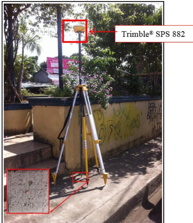
Figure 33. GNSS base receiver setup, Trimble® SPS 882 at DS-09 located at stair of Nograles Park along Mac Arthur Highway, in Brgy. Talomo, Davao City, Davao Del Sur
