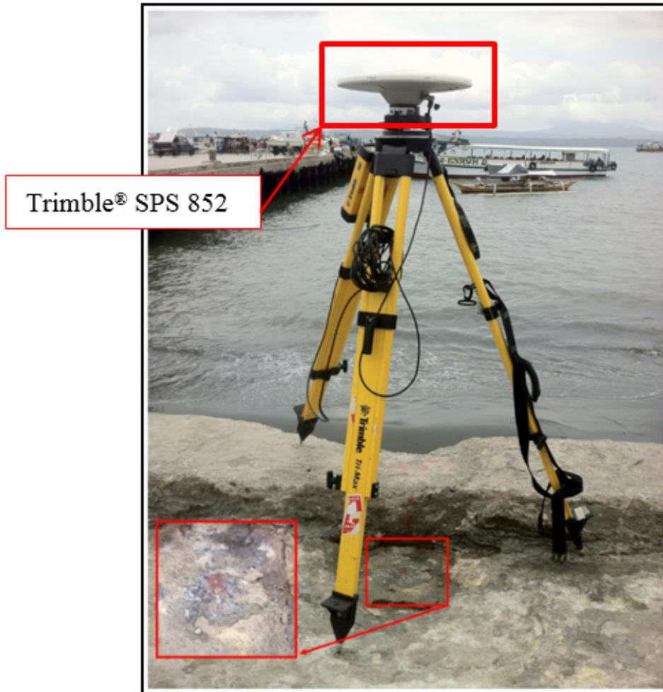
Figure 31. GNSS base receiver setup, Trimble® SPS 852 at DVS-1 at the east side of Pier, in Brgy. Leon Garcia Sr., Davao City, Davao Del Sur
