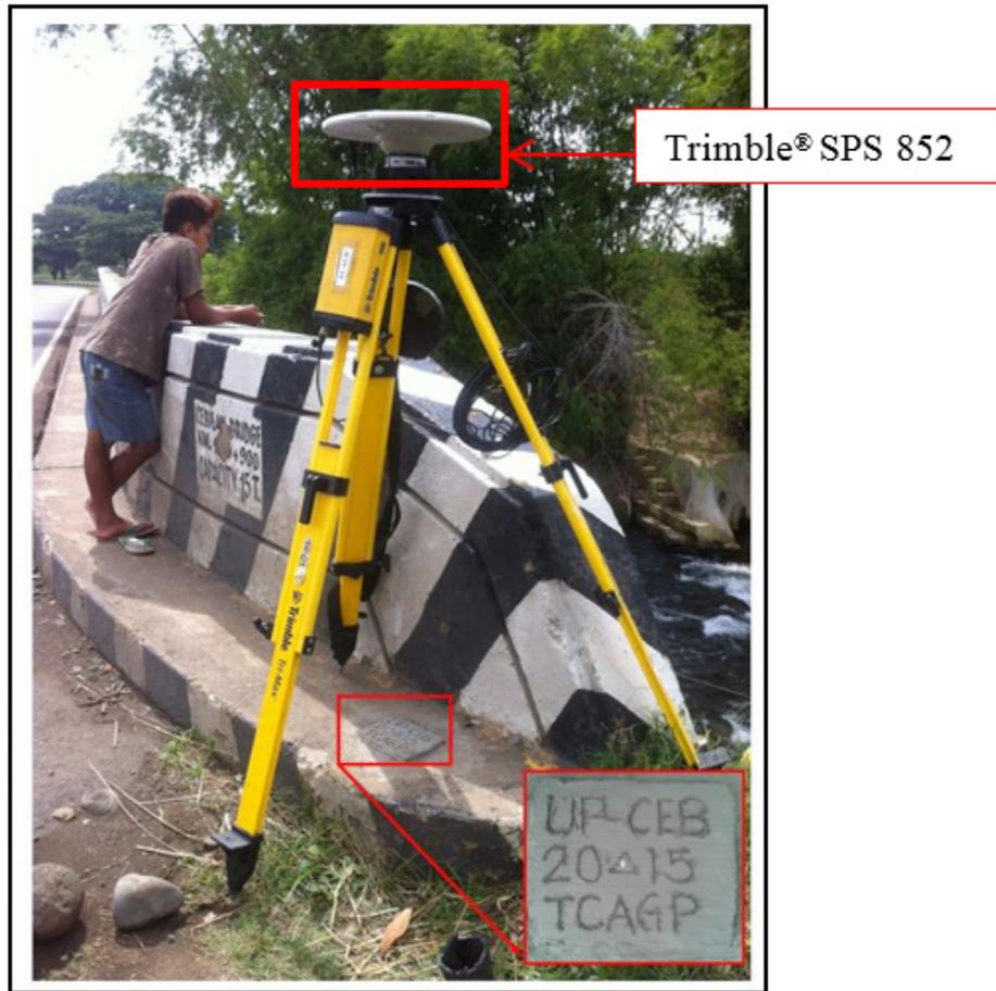
Figure 34. GNSS base receiver setup, Trimble® SPS 852 at UP-CEB on the right approach of Cebulan Bridge in Brgy Darong, Municipality of Santa Cruz, Davao Del Sur
