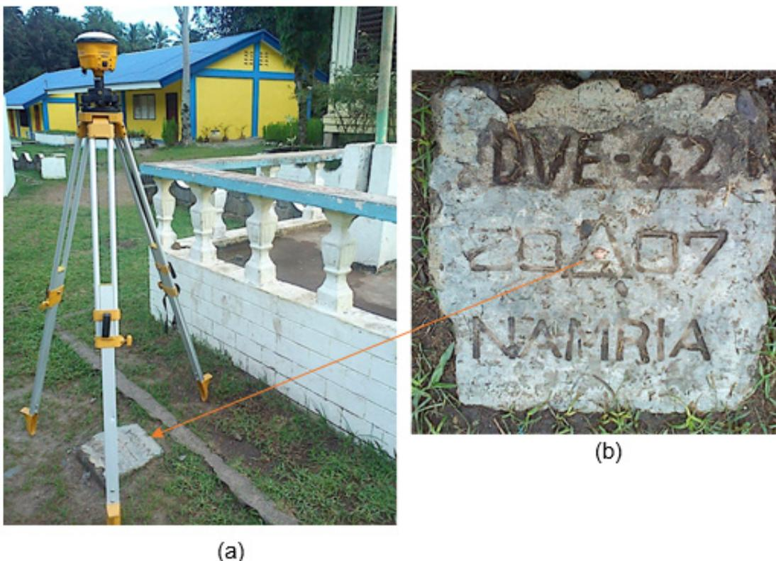
Figure 3. Photo (a) shows the GPS set-up over DVE-42 located in front of the flagpole inside the premises of Don Enrique Elementary School, while Photo (b) depicts a close-up view of NAMRIA reference point DVE-42 as recovered by the field team.
