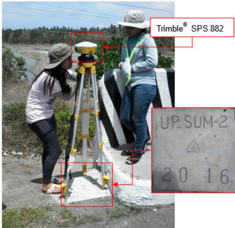
Figure 32. GNSS receiver set up, Trimble® SPS 882, at UP\_SUM-2, located beside the approach of Sumlog Bridge in Brgy. Ilangay, Municipality of Lupon, Province of Davao Oriental.
