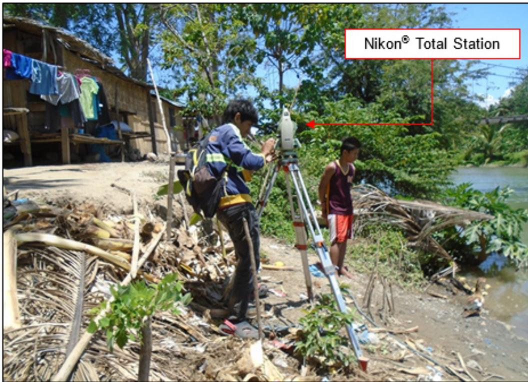
Figure 41. Manual bathymetric survey of ABSD at Sumlog River using Nikon® Total Station.
