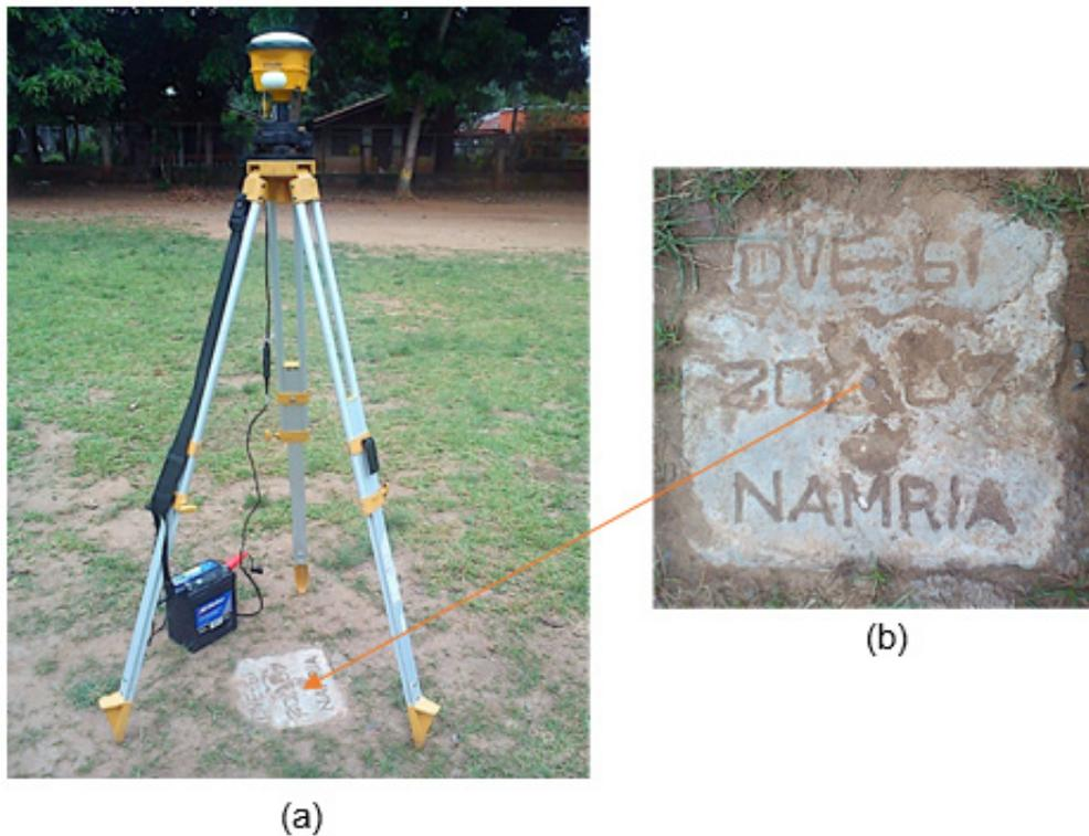
Figure 4. Photo (a) shows the GPS set-up over DVE-61 located at the center of the playground of Zign Elementary School, while Photo (b) depicts a close-up view of NAMRIA reference point DVE-61 as recovered by the field team.
