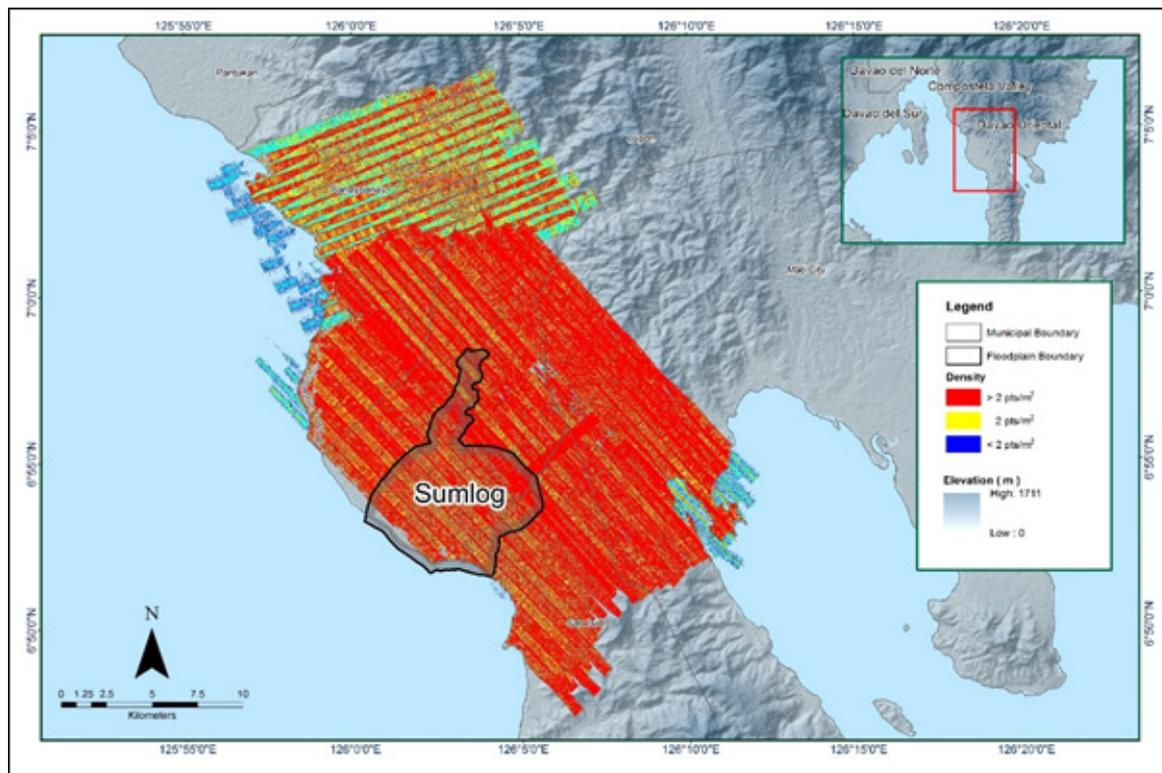
Figure 14. Density map of merged LiDAR data for Sumlog Floodplain.
