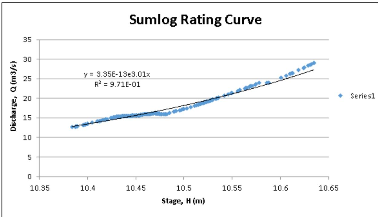
Figure 48. Rating Curve at Sumlog Bridge, Lupon, Davao Oriental.
