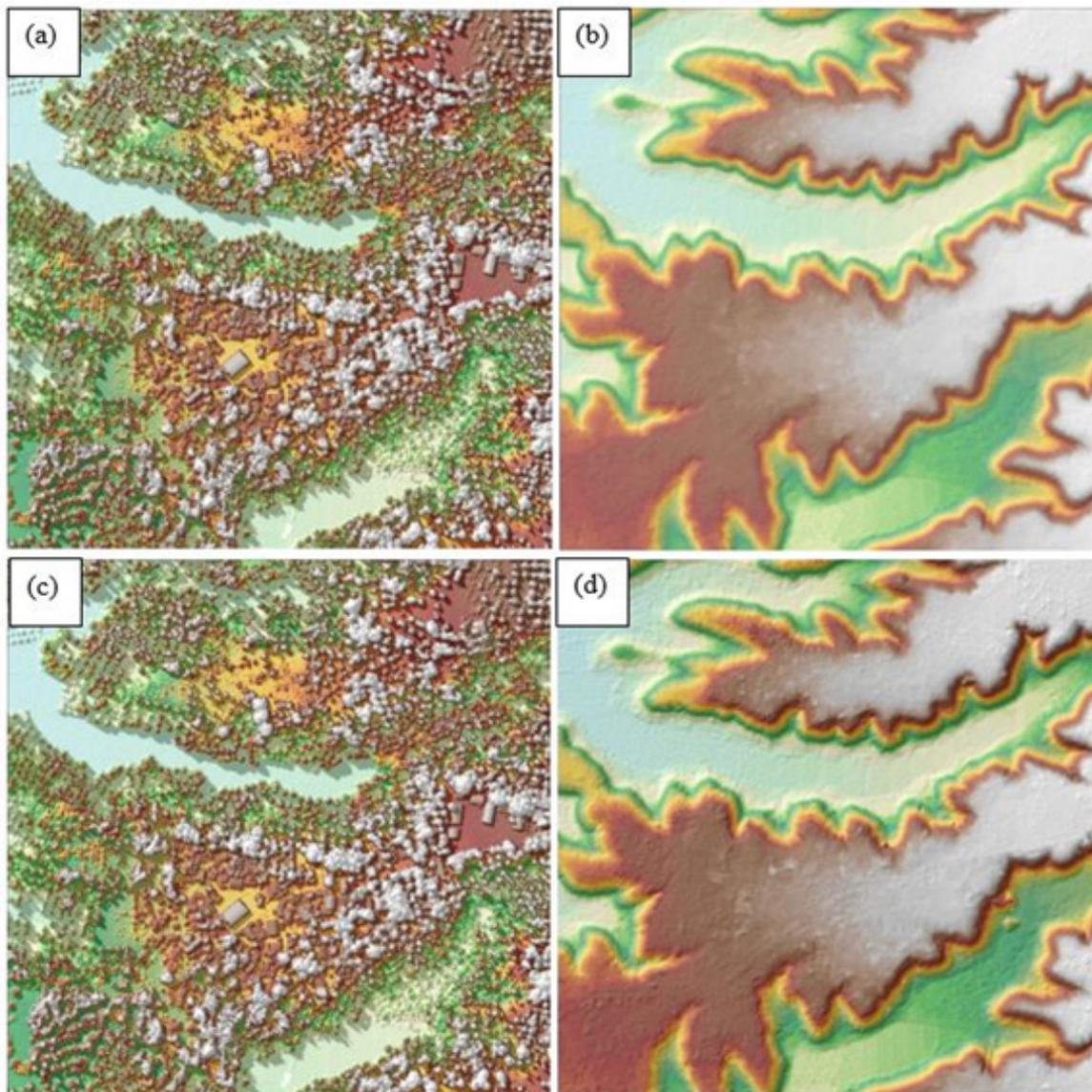
Figure 19. The production of last return DSM (a) and DTM (b), first return DSM (c) and secondary DTM (d) in some portion of Sumlog Floodplain.
