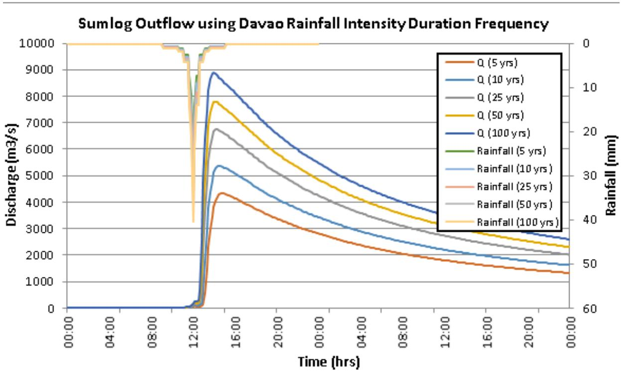
Figure 60. The Outflow hydrograph at Sumlog Station generated using Cagayan de Oro RIDF simulated in HEC-HMS.
