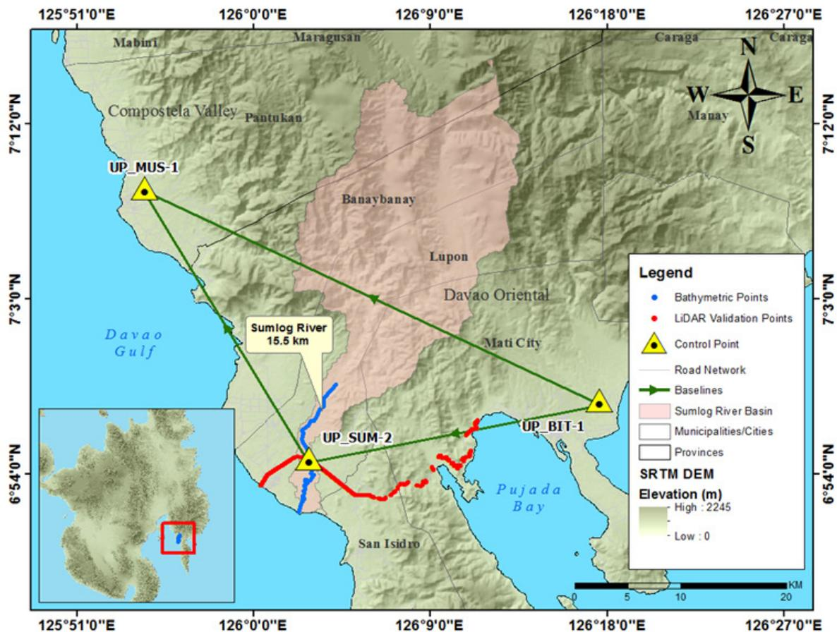
Figure 28. Extent of the bathymetric survey (in blue line) in Sumlog River and the LiDAR Data Validation Survey (in red).
