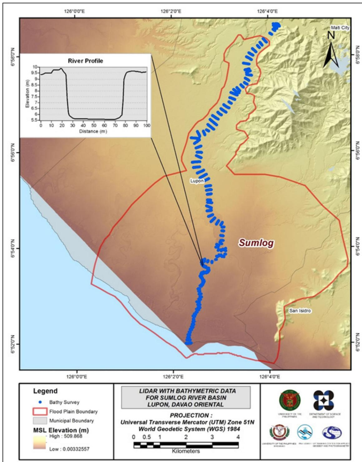
Figure 25. Map of Sumlog Floodplain with bathymetric survey points shown in blue.
