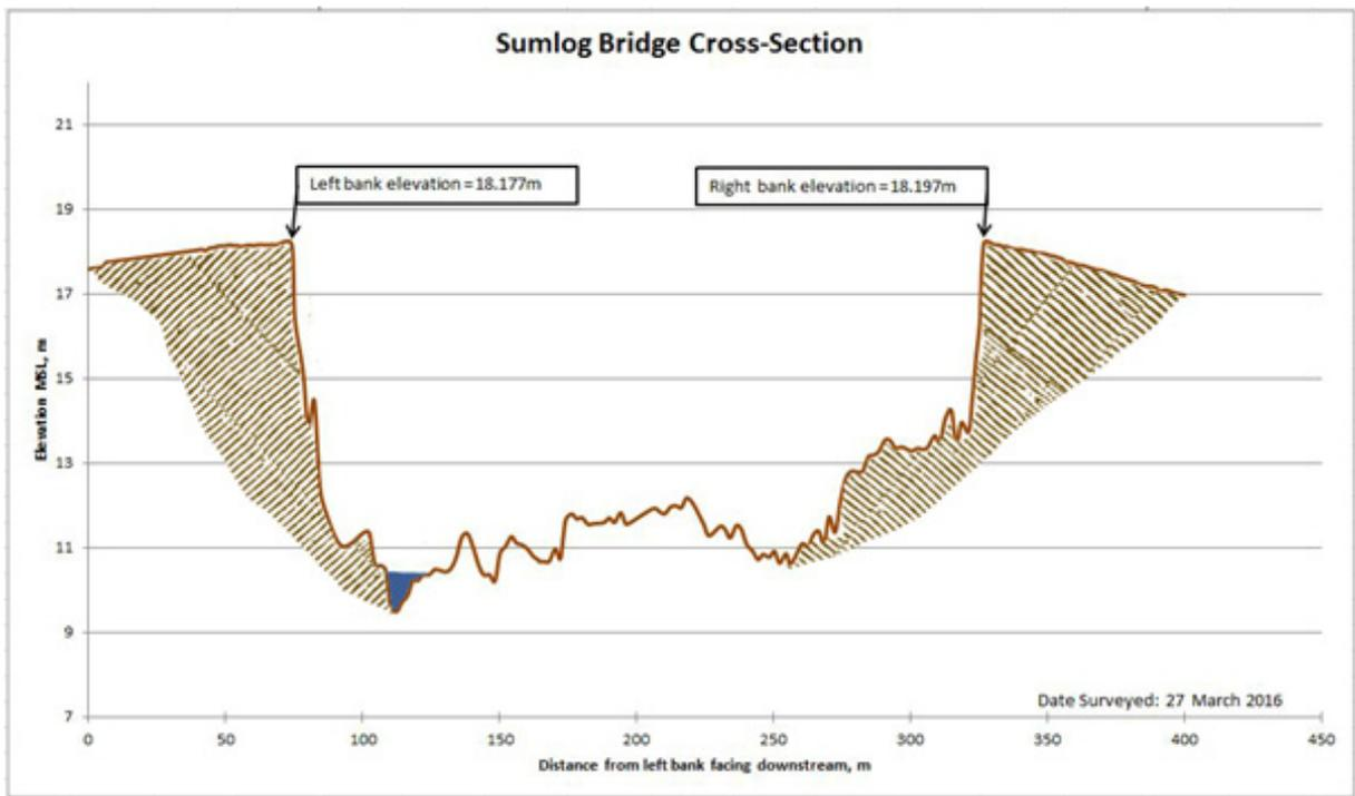
Figure 47. Cross-Section Plot of Sumlog Bridge
