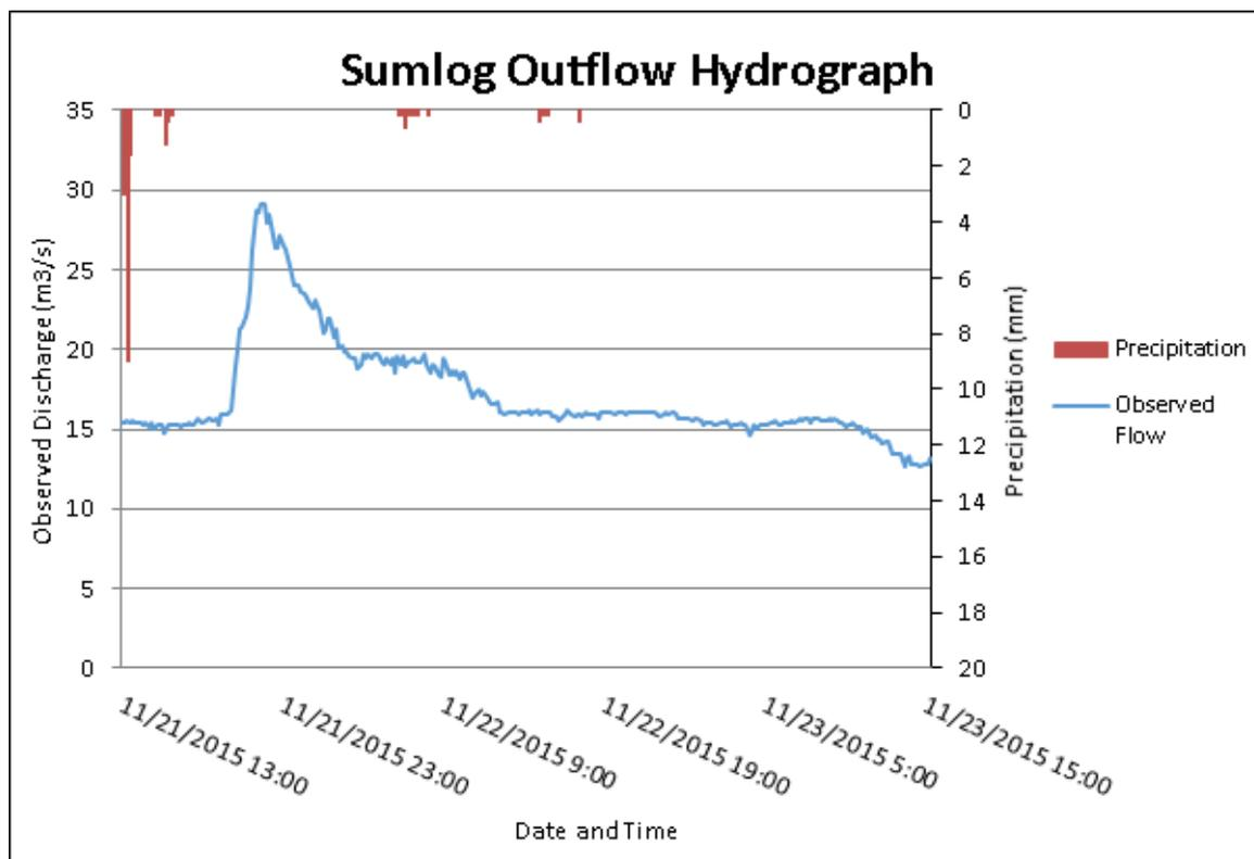
Figure 49. Rainfall and outflow data at Sumlog Bridge used for modeling.
