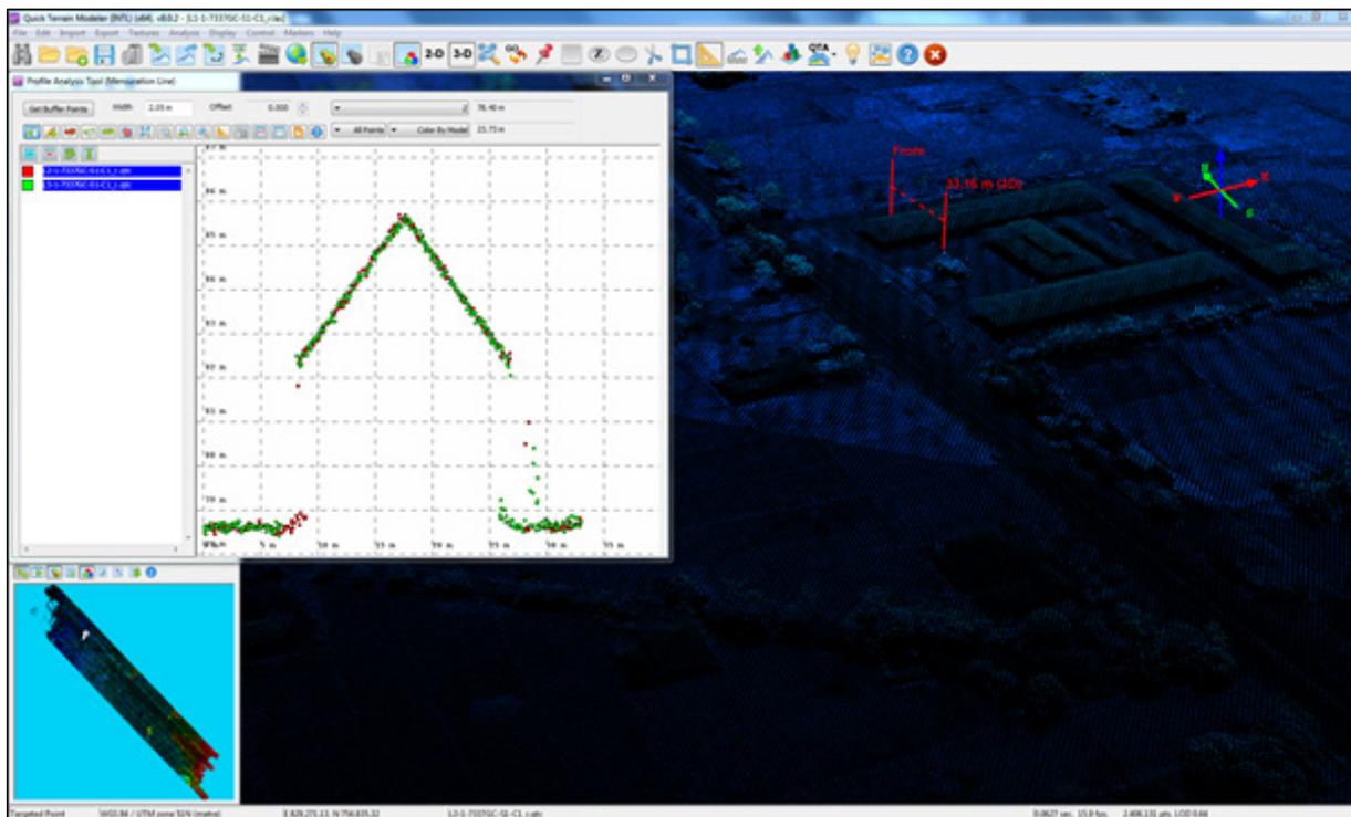
Figure 16. Quality checking for Aunugay flight 3981G using the Profile Tool of QT Modeler.
