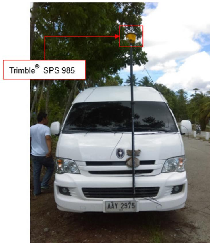
Figure 39. The Validation Points Acquisition survey set-up using a GNSS receiver fixed in a van along the Sumlog River Basin.
