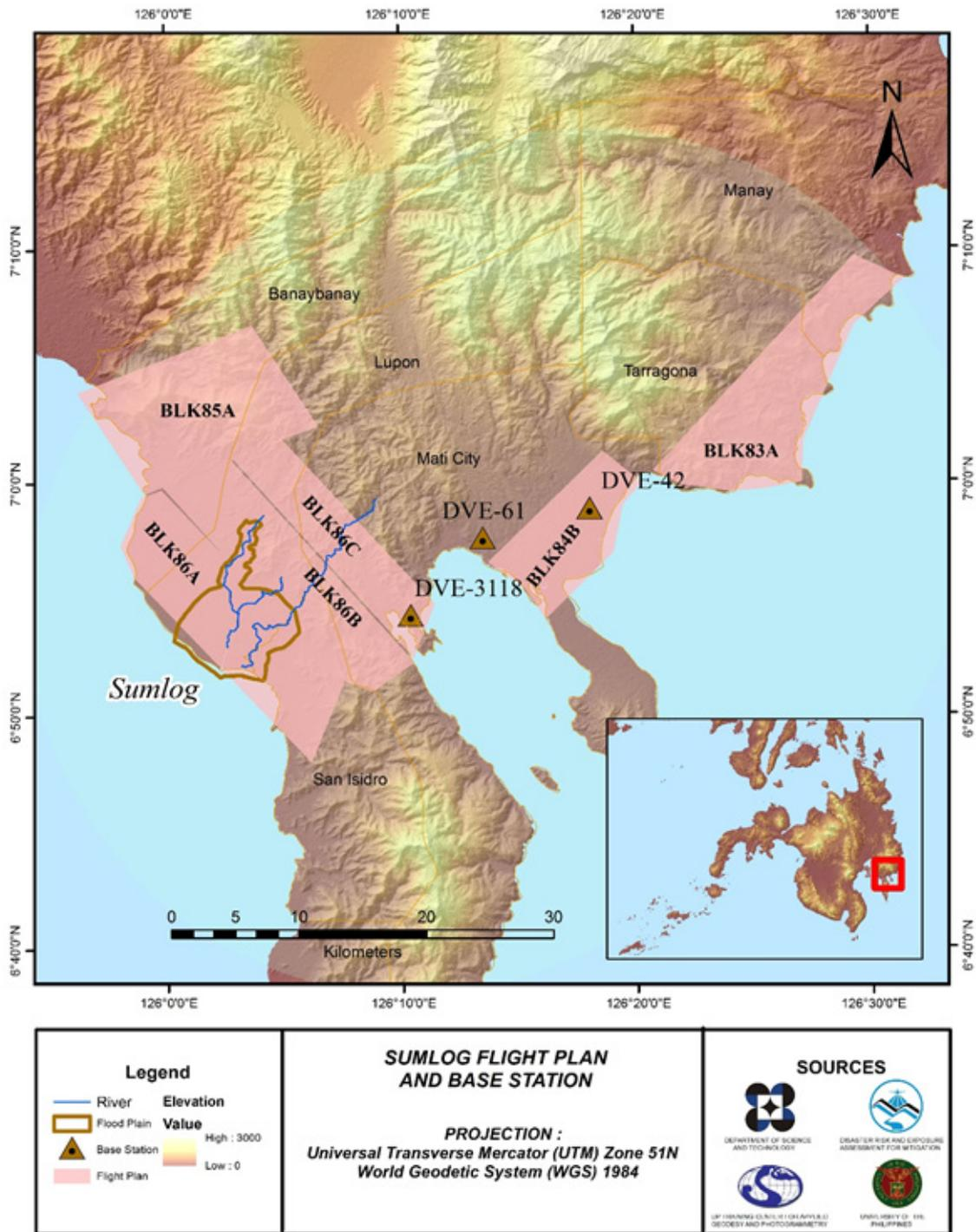
Figure 2. Flight plans and base stations used for Sumlog Floodplain Survey
