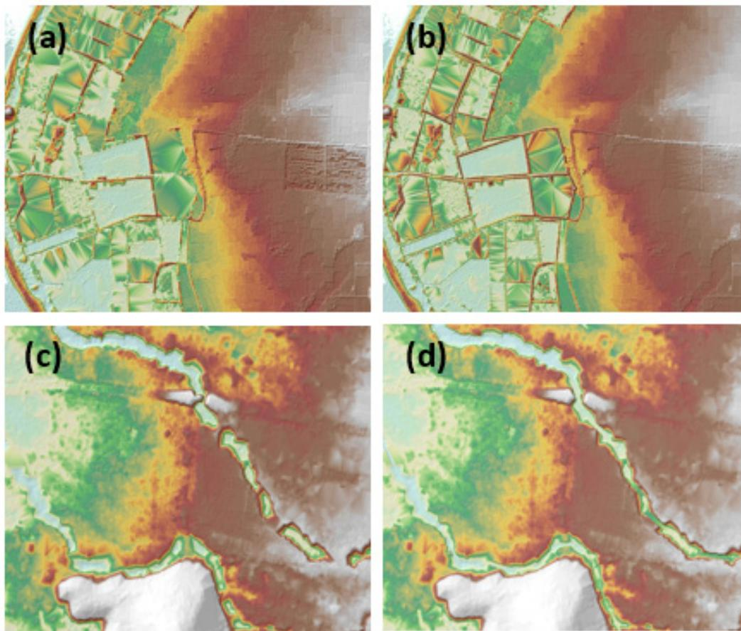
Figure 20. Portions in the DTM of Sumlog Floodplain – a paddy field before (a) and after (b) data retrieval; a bridge before (c) and after (d) manual editing.
