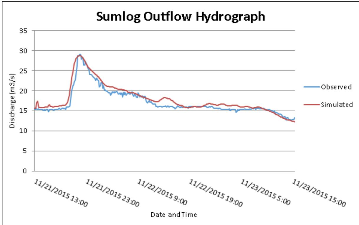
Figure 59. Outflow Hydrograph of Sumlog produced by the HEC-HMS model compared with observed outflow.
