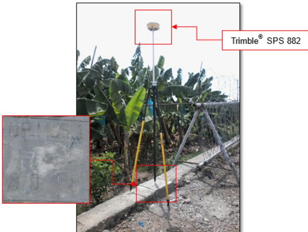
Figure 31. GNSS receiver set up, Trimble® SPS 882, at UP\_MUS-1, located at the approach of Musahamat Bridge in Brgy. Kingking, Pantukan, Province of Compostela Valley.
