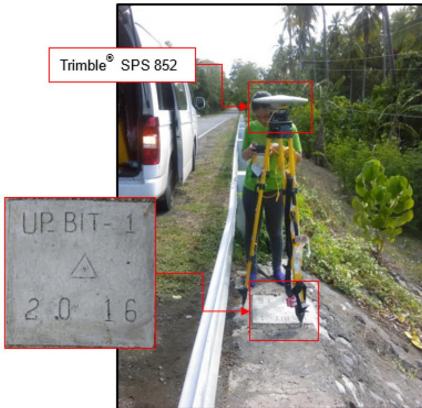
Figure 30. GNSS receiver set up, Trimble® SPS 852, at UP\_BIT-1, located at the side of the railing near the approach of Bitanagan Bridge in Brgy. Don Enrique Lopez, City of Mati, Davao Oriental.
