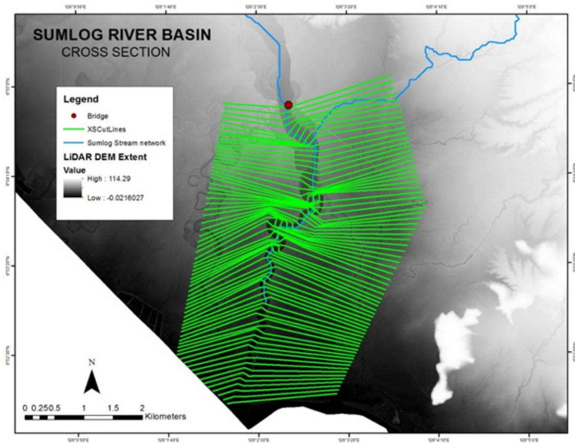
Figure 57. River Cross-section of the Sumlog River generated through Arcmap HEC GeoRAS tool.
