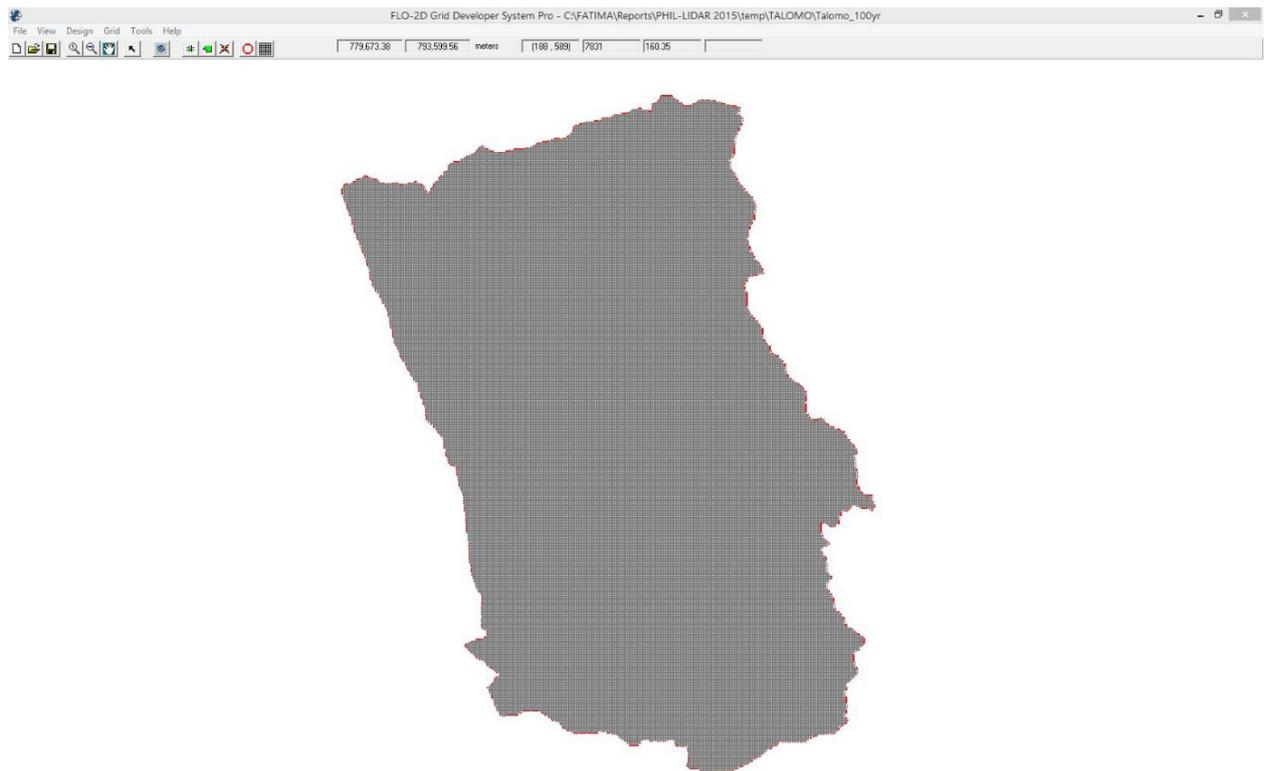
Figure 60. Screenshot of the river sub-catchment with the computational area to be modeled in FLO-2D Grid Developer System Pro (FLO-2D GDS Pro)
