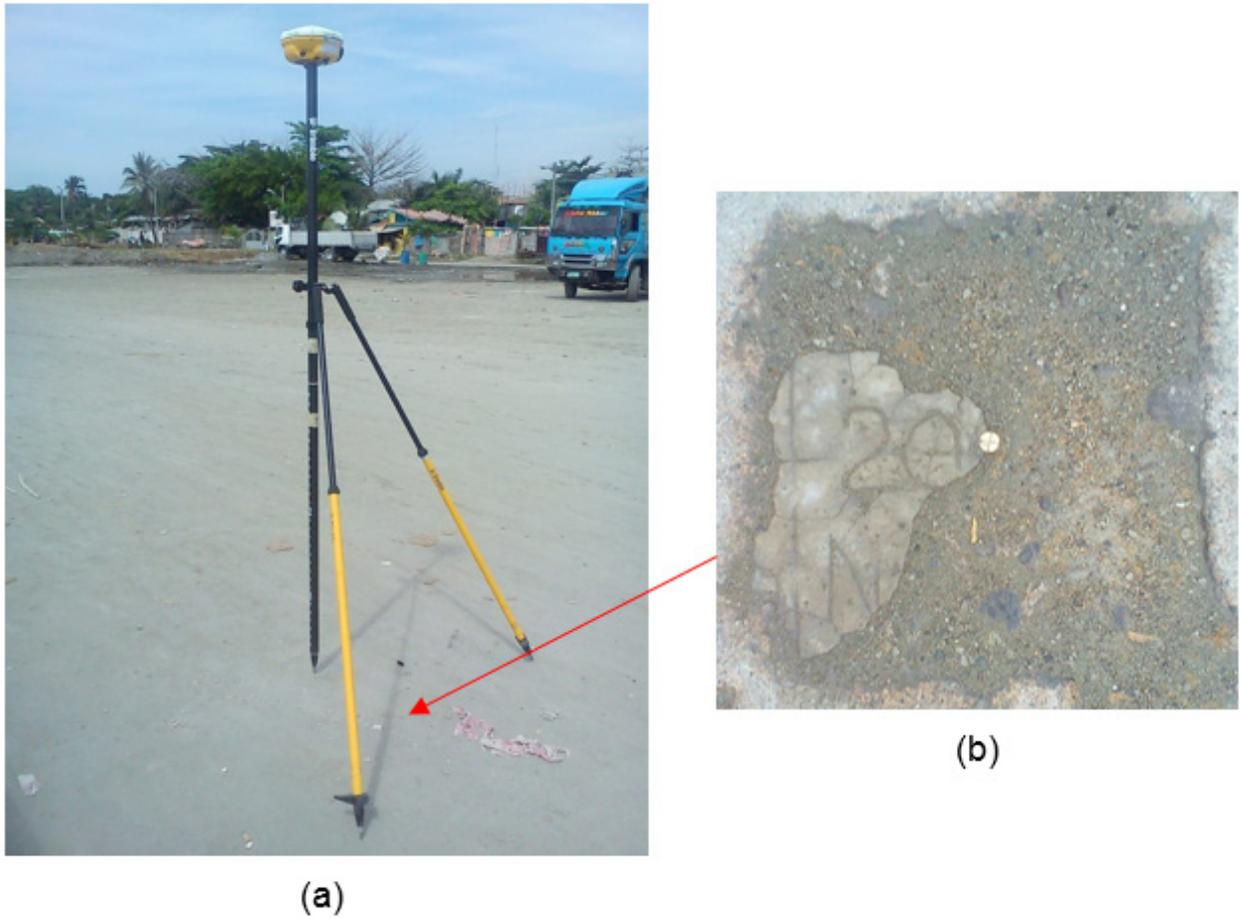
Figure 7. GPS set-up over DVS-1A in the town proper of Davao City, Davao del Sur (a) and NAMRIA reference point DVS-1A (b) as recovered by the field team.
