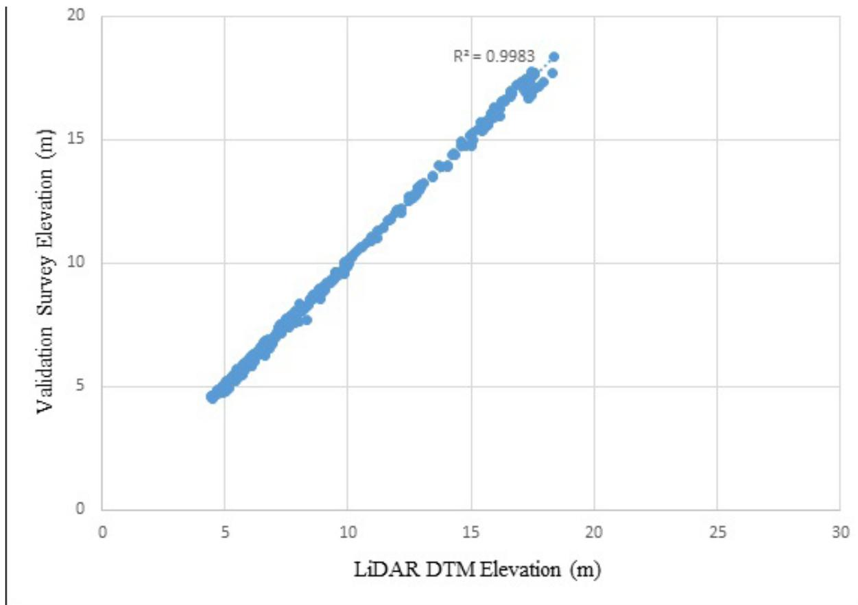
Figure 27. Correlation plot between validation survey points and LiDAR data.
