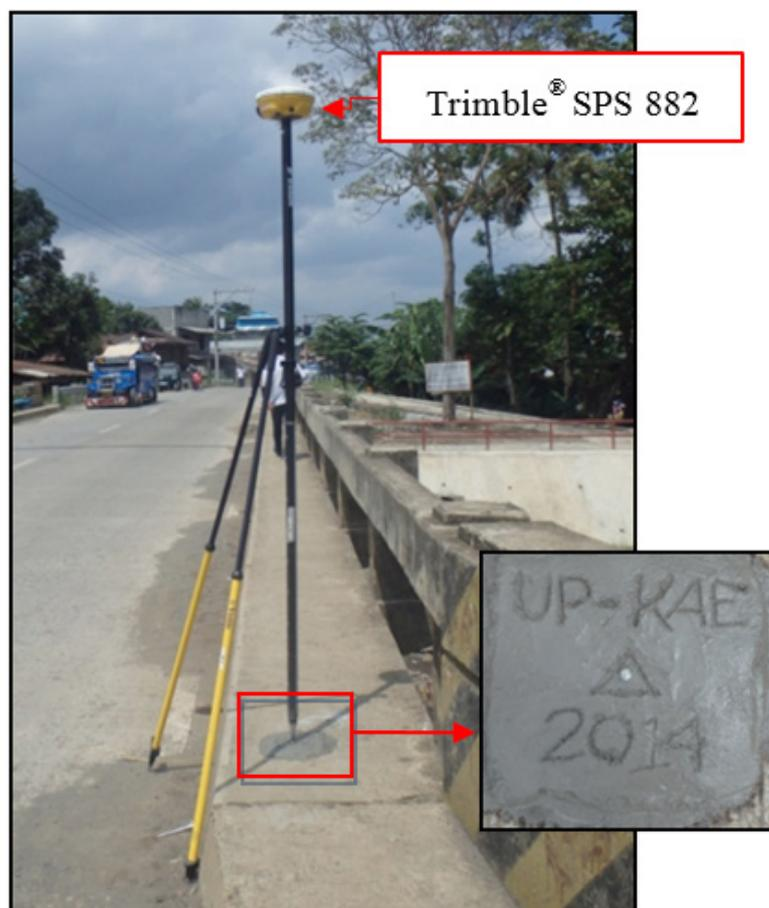
Figure 34. GNSS receiver occupation set up, Trimble® SPS 882 at control point UP-KAE, Kalye Apike Bridge in Brgy. Calinan, Davao City
