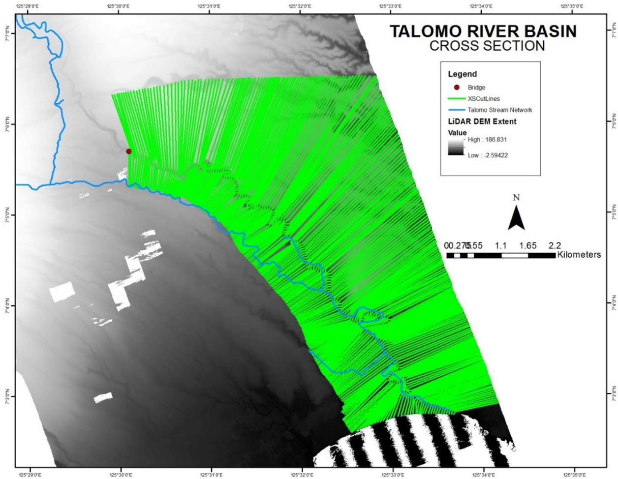
Figure 62. River cross-section of Talomo River generated through Arcmap HEC GeoRAS tool
