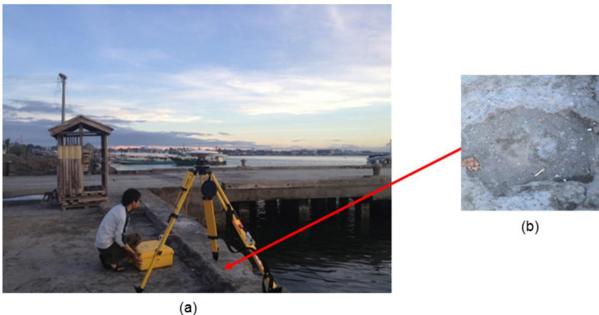
Figure 4. GPS set-up over DVS-1 at Sta. Ana Wharf, Davao City (a) and NAMRIA reference point DVS-1 (b) as recovered by the field team.
