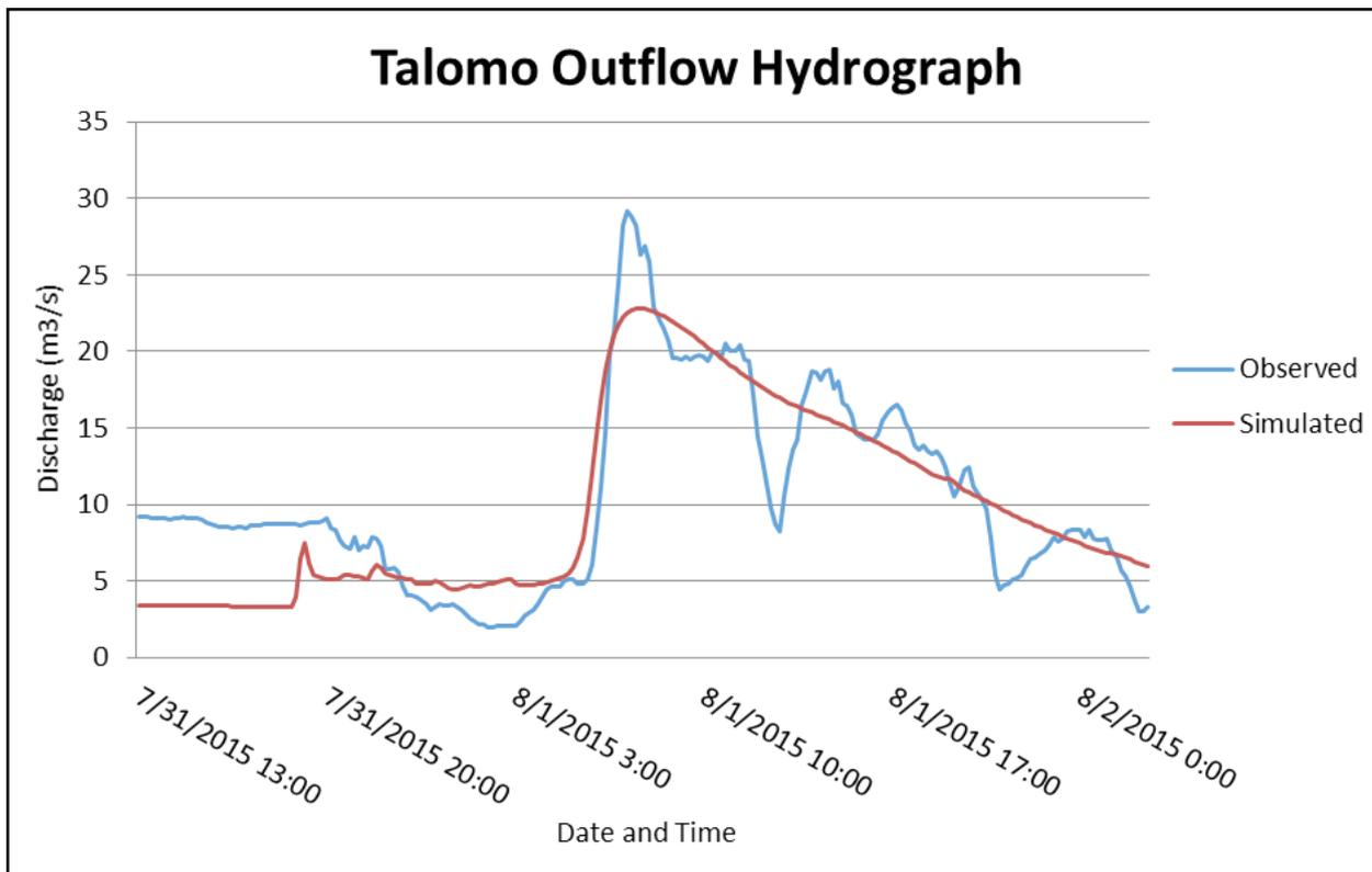
Figure 64. Outflow hydrograph of Talomo produced by the HEC-HMS model compared with observed outflow
