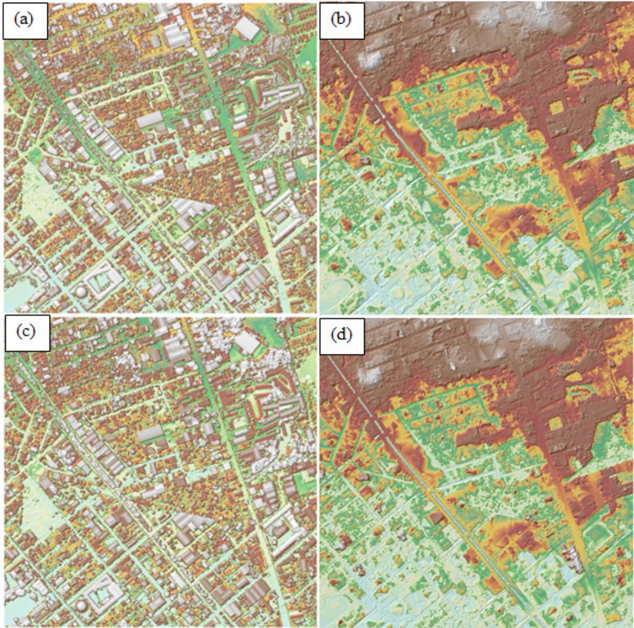
Figure 20. The production of last return DSM (a) and DTM (b), first return DSM (c) and secondary DTM (d) in some portion of Talomo Floodplain.
