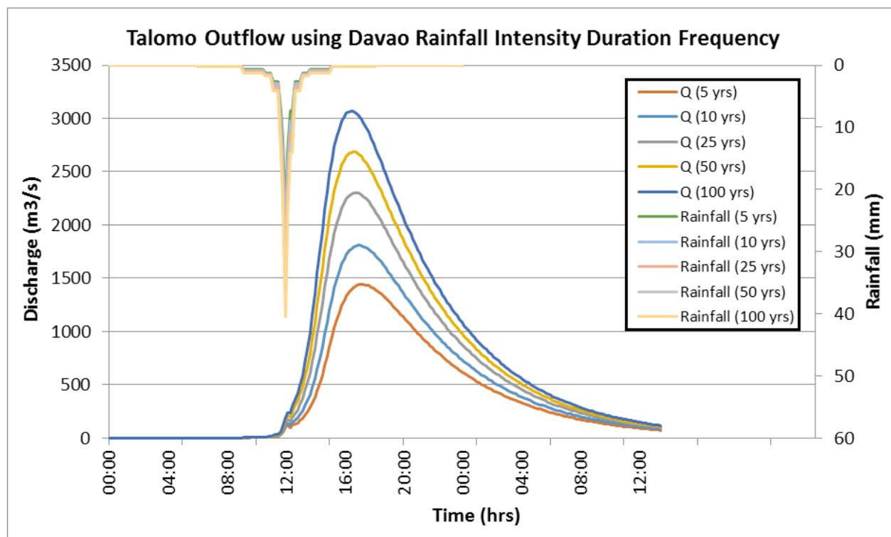
Figure 65. Outflow hydrograph at Talomo Station generated using the Davao RIDF simulated in HEC-HMS.
