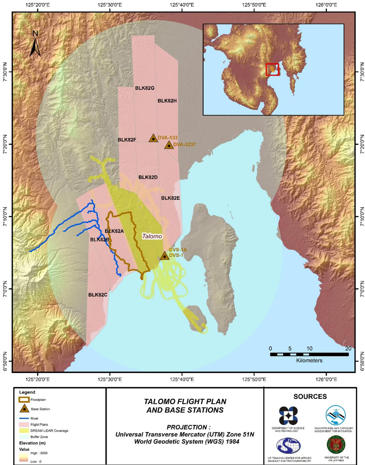
Figure 3. Flight Plan and base station used for the Talomo Floodplain survey.
