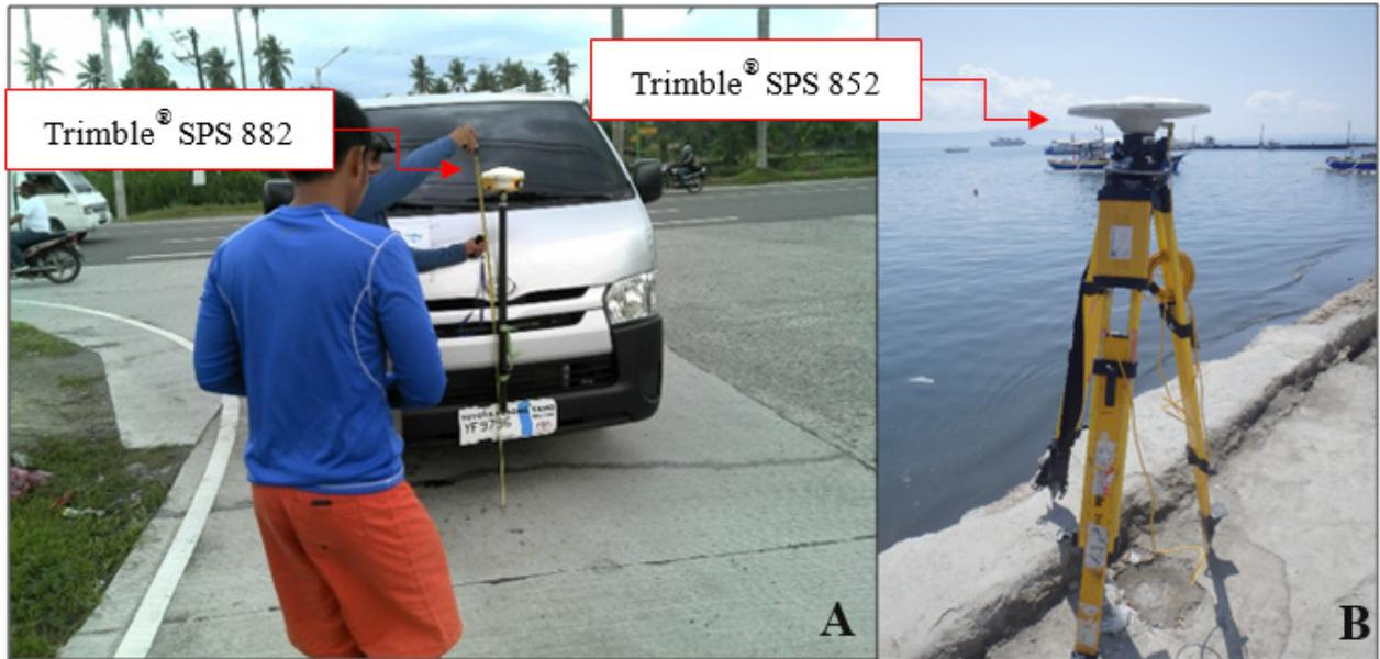
Figure 46. Ground Validation Set-up (A) and (B) GPS base receiver set up, Trimble® SPS 852 at DVS-1, in Sta. Ana Port
