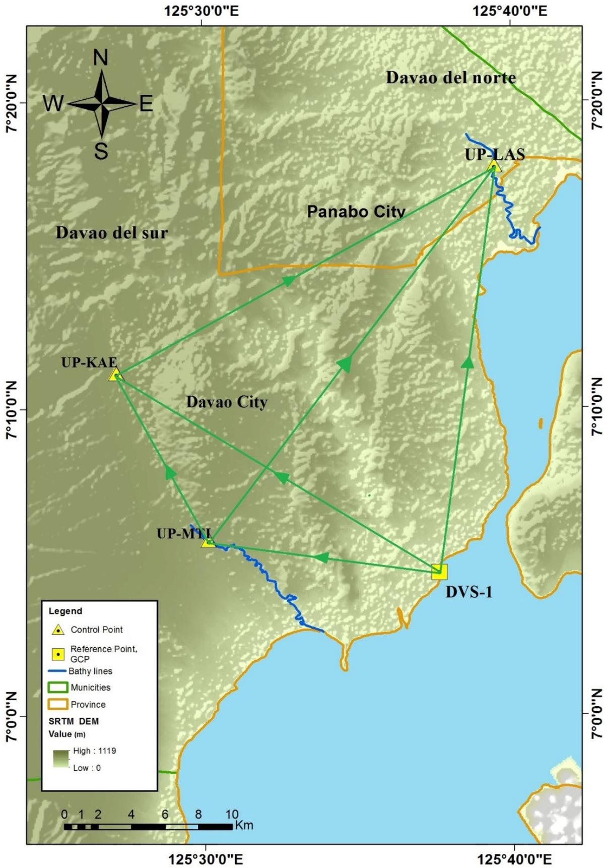
Figure 32. The GNSS Network established in the Talomo River Survey.
