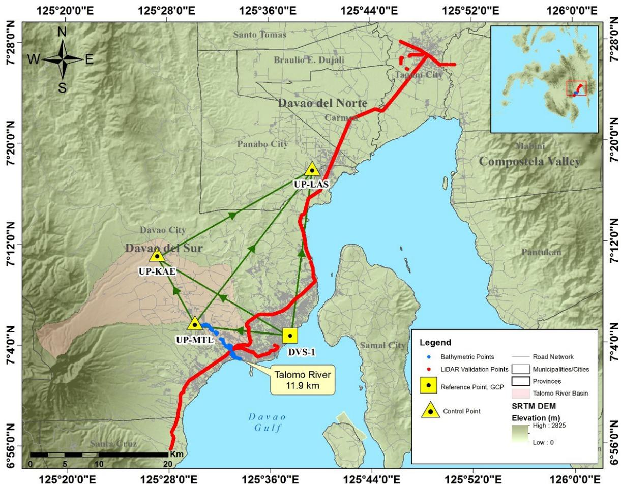
Figure 31. Extent of the bathymetric survey (in blue line) in Talomo River and the LiDAR data validation survey (in red).
