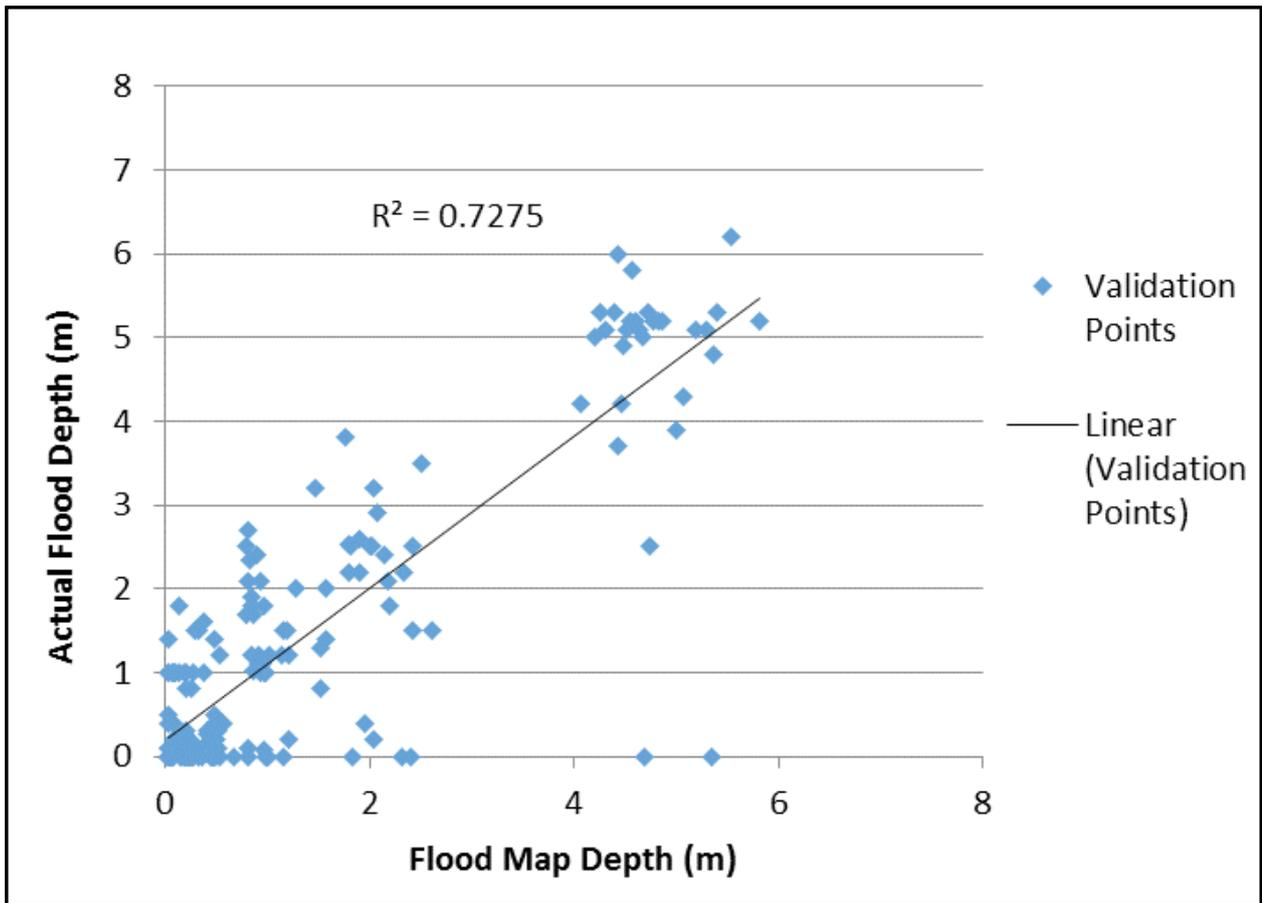
Figure 80. Flood map depth vs. actual flood depth
