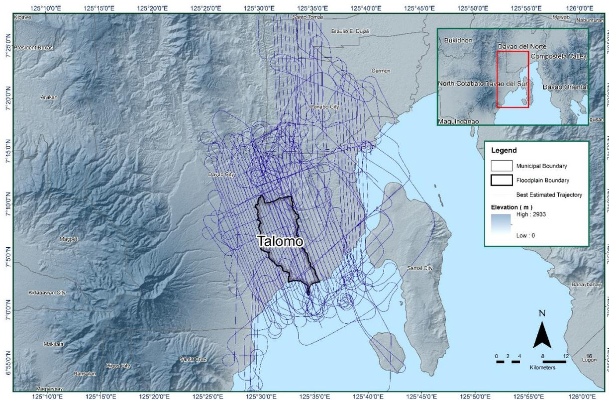
Figure 12. Best Estimated Trajectory of the LiDAR missions conducted over the Talomo Floodplain.
