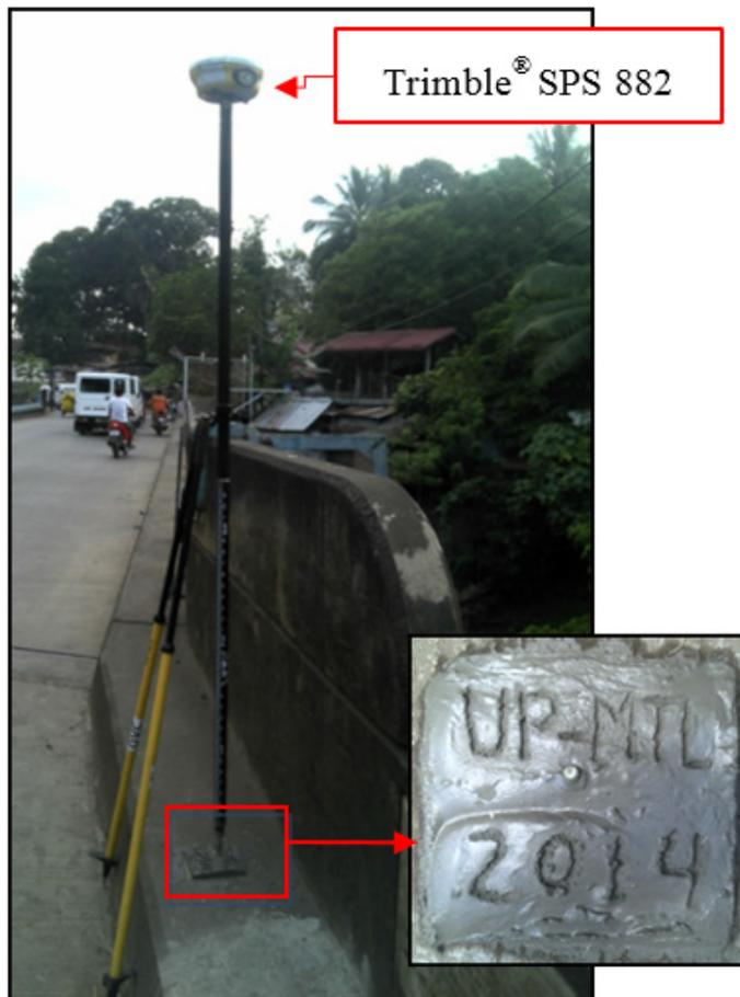
Figure 36. GNSS receiver occupation set up, Trimble® SPS 882 at control point UP-MTL, Mintal Bridge in Brgy. Mintal, Davao City
