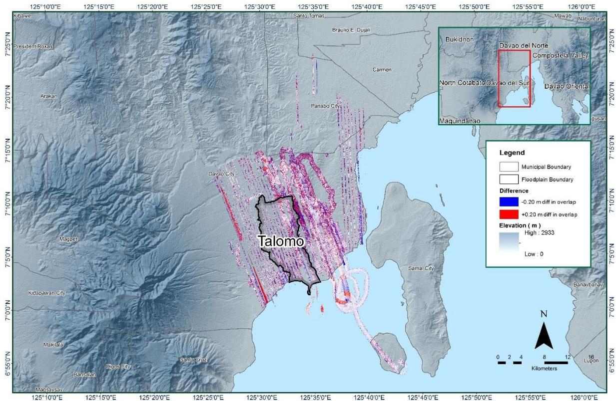
Figure 16. Elevation Difference Map between flight lines for Talomo Floodplain Survey.
