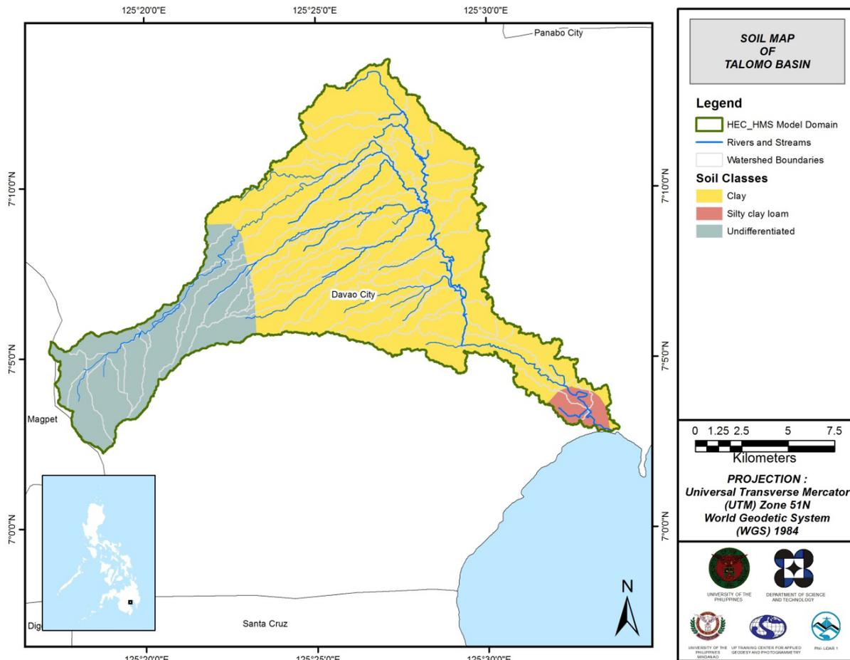
Figure 57. Soil Map of Talomo River Basin used for the estimation of the CN parameter.
