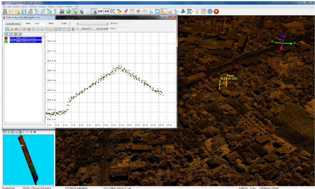
Figure 17. Quality checking for Talomo Flight 7388GC using the Profile Tool of QT Modeler.
