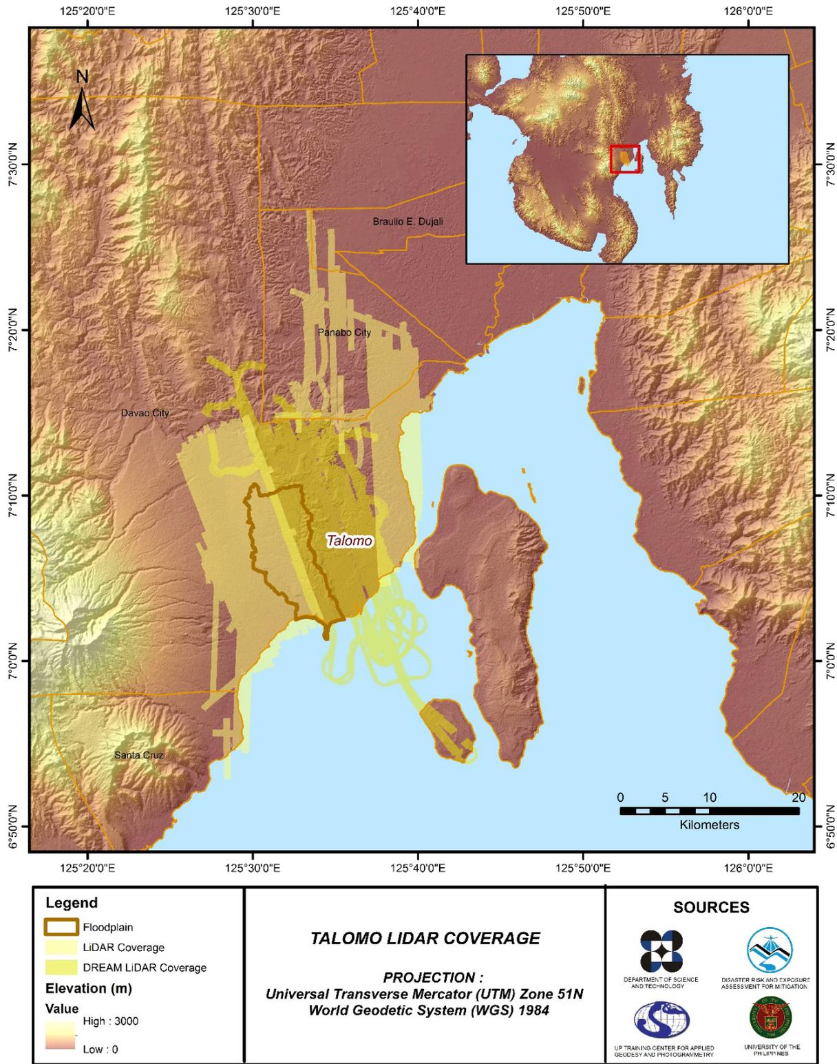
Figure 8. Actual LiDAR survey coverage of the Talomo Floodplain.
