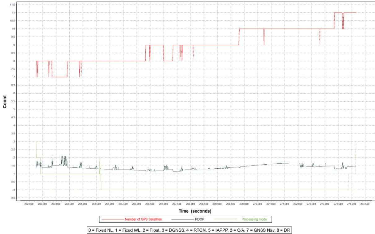
Figure 11. Solution Status Parameters of Talomo Flight 7388GC.
