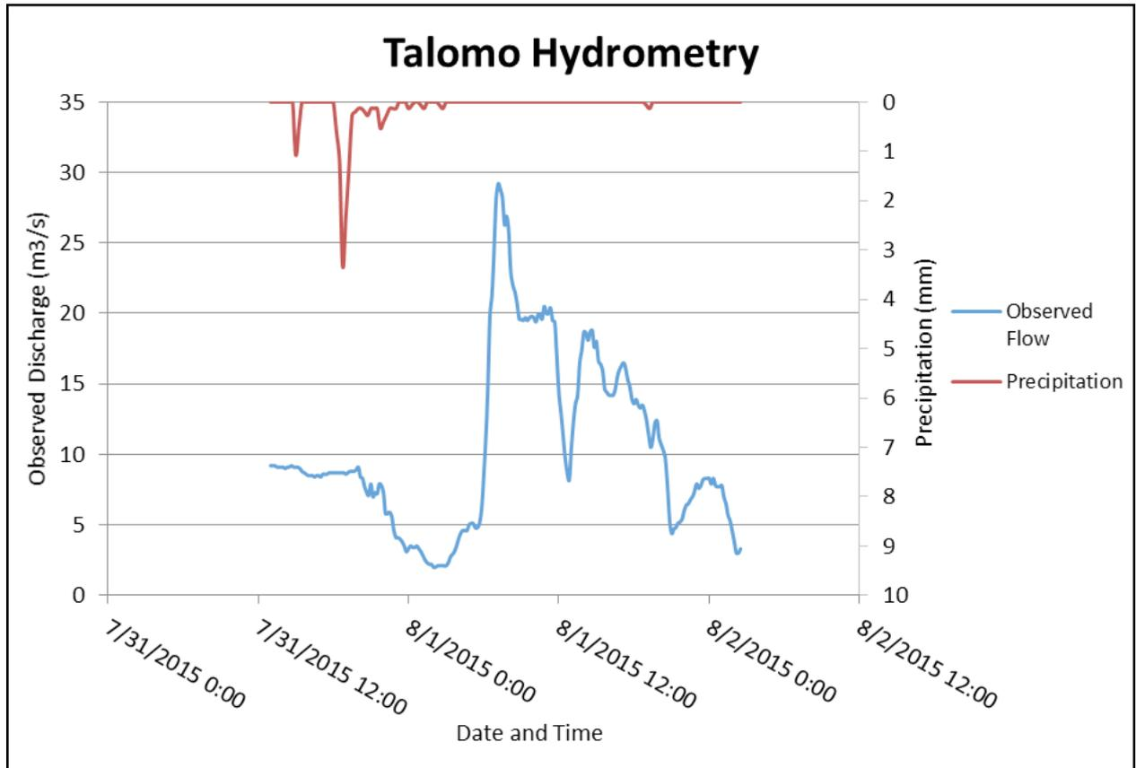
Figure 54. Rainfall and outflow data at Kalye Apike Bridge used for modeling
