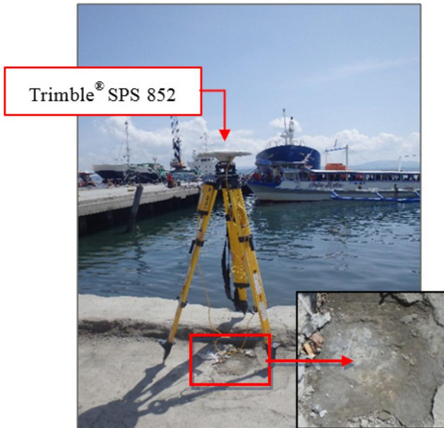
Figure 33. GNSS base receiver set up, Trimble® SPS 852 at DVS-1 in Sta. Ana Wharf, Davao City
