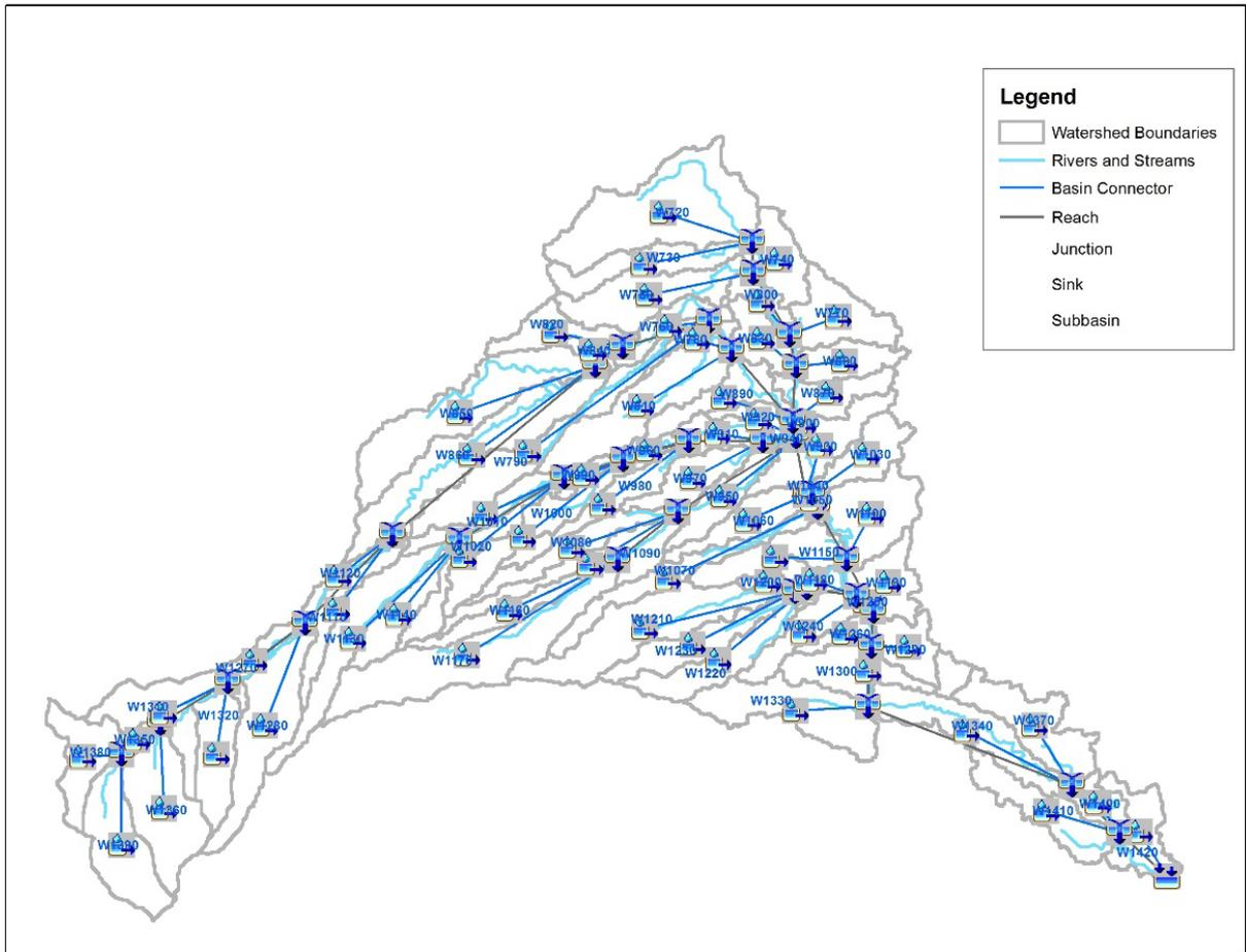
Figure 61. Talomo River Basin model generated in HEC-HMS
