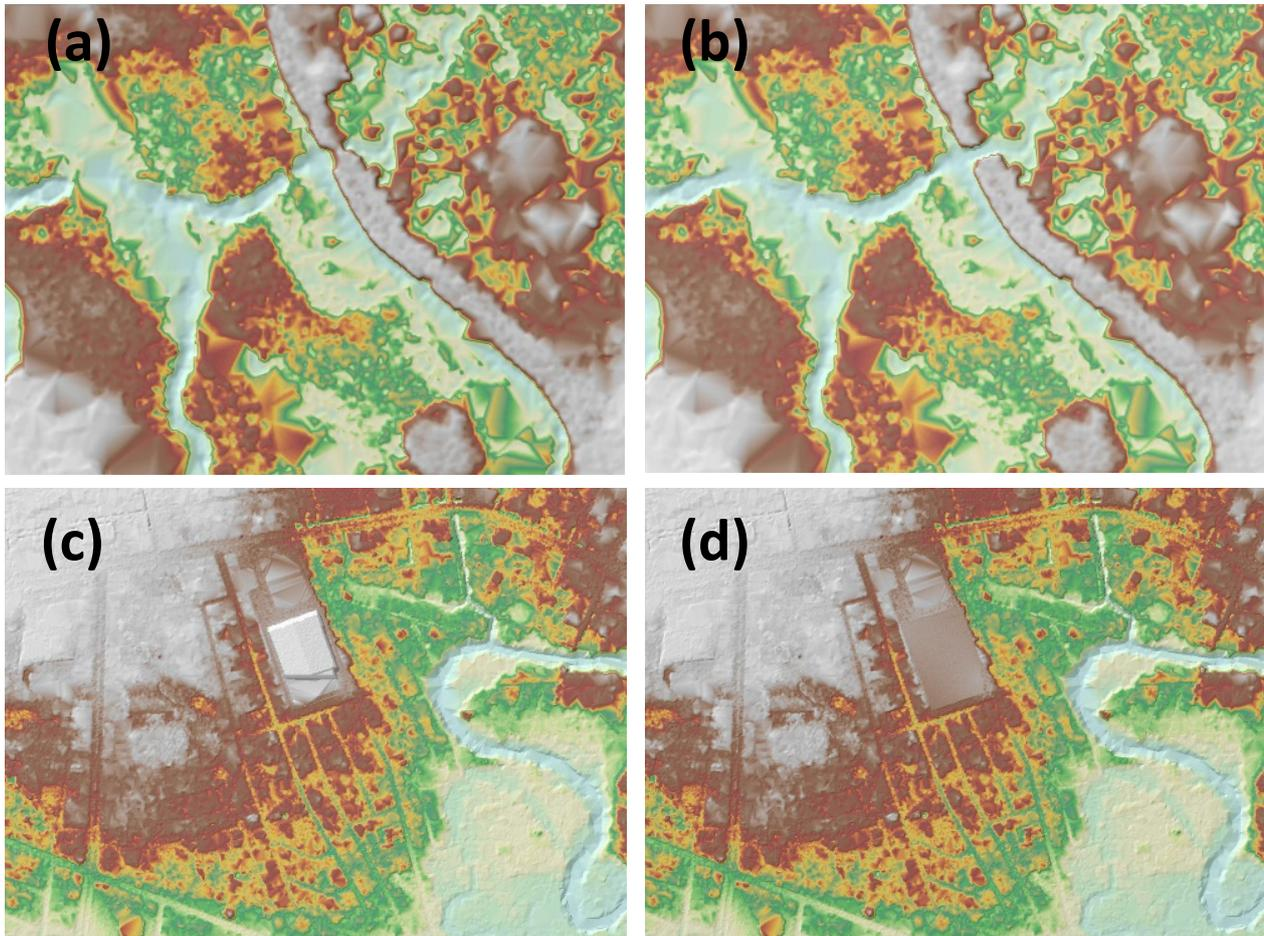
Figure 23. Portions in the DTM of Talomo Floodplain – a bridge before (a) and after (b) manual editing; and a building before (c) and after (d) manual editing
