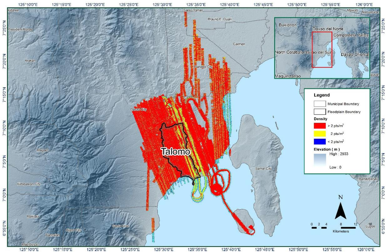
Figure 15. Pulse density map of merged LiDAR data for Talomo Floodplain.
