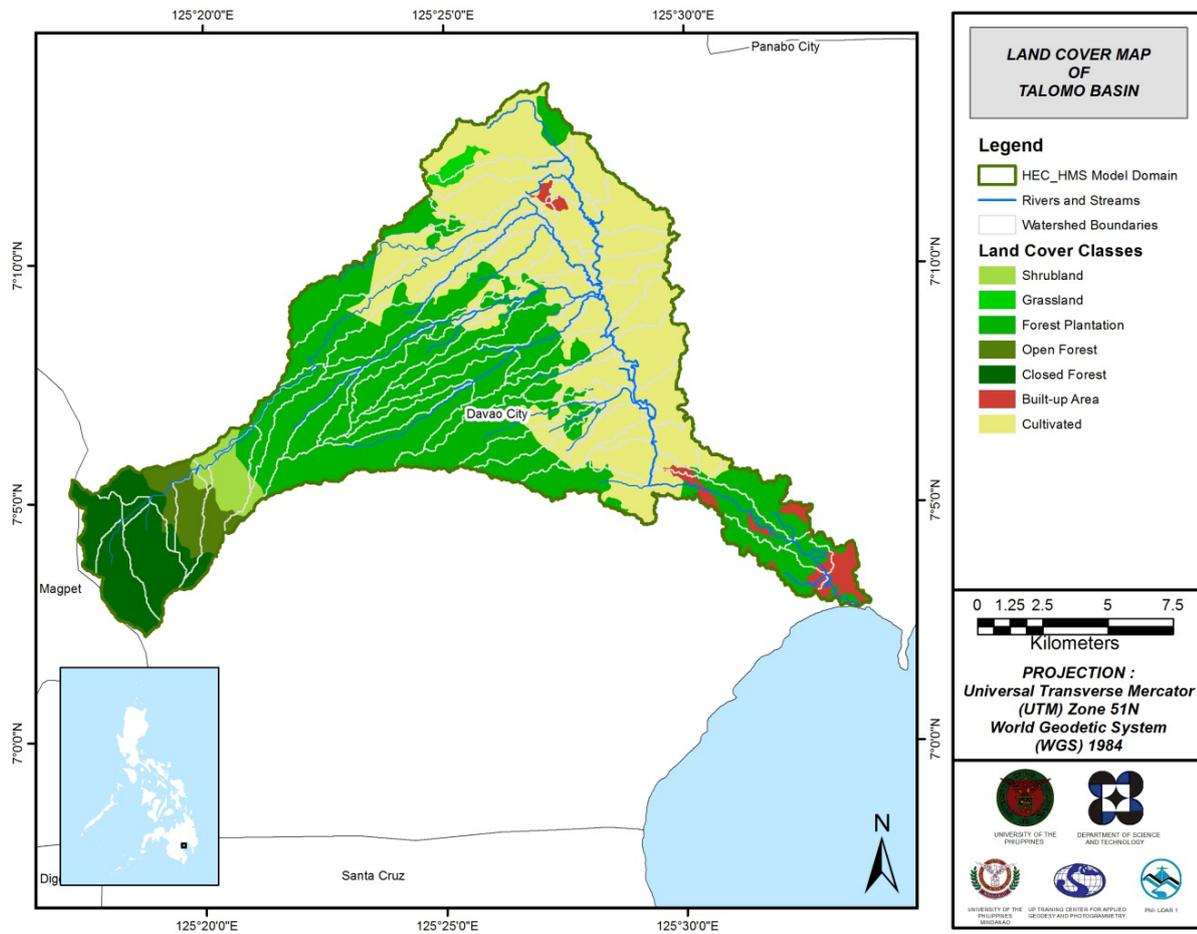
Figure 58. Land Cover Map of Talomo River Basin used for the estimation of the Curve Number (CN) and the watershed lag parameters of the rainfall-runoff model.
