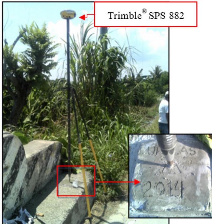
Figure 35. GNSS receiver occupation set up, Trimble® SPS 882 at control point UP-LAS in Brgy. Little Panay, Panabo City
