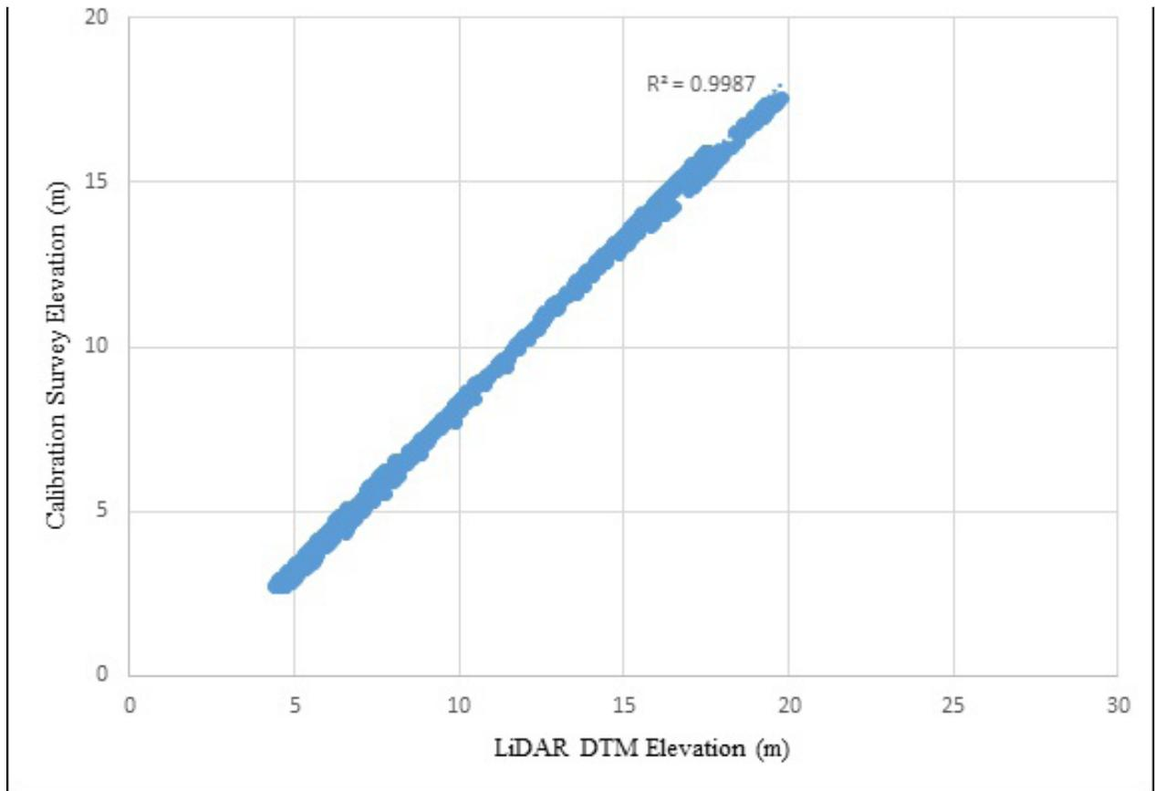
Figure 26. Correlation plot between calibration survey points and LiDAR data.
