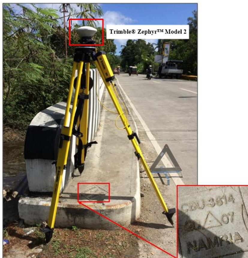
Figure 34. GNSS receiver set-up, Trimble® Zephyr™ Model 2, at CBU-3614, Lapu-lapu Bridge approach in Brgy. Poblacion, Municipality of Asturias, Cebu
