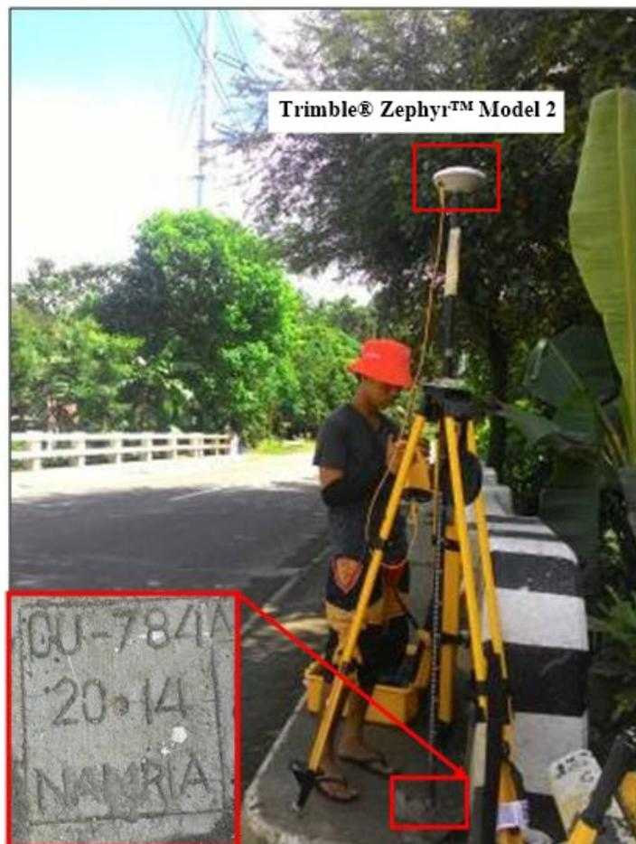
Figure 33. GNSS receiver setup, Trimble® Zephyr™ Model 2, at CU-784 Balud Bridge approach in Brgy. Balud, Toledo City, Cebu
