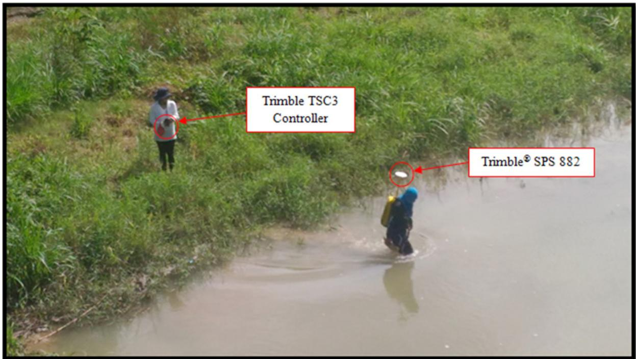
Figure 37. Cross-section survey conducted on Balamban river in Brgy. Biasong, Municipality of Balamban
