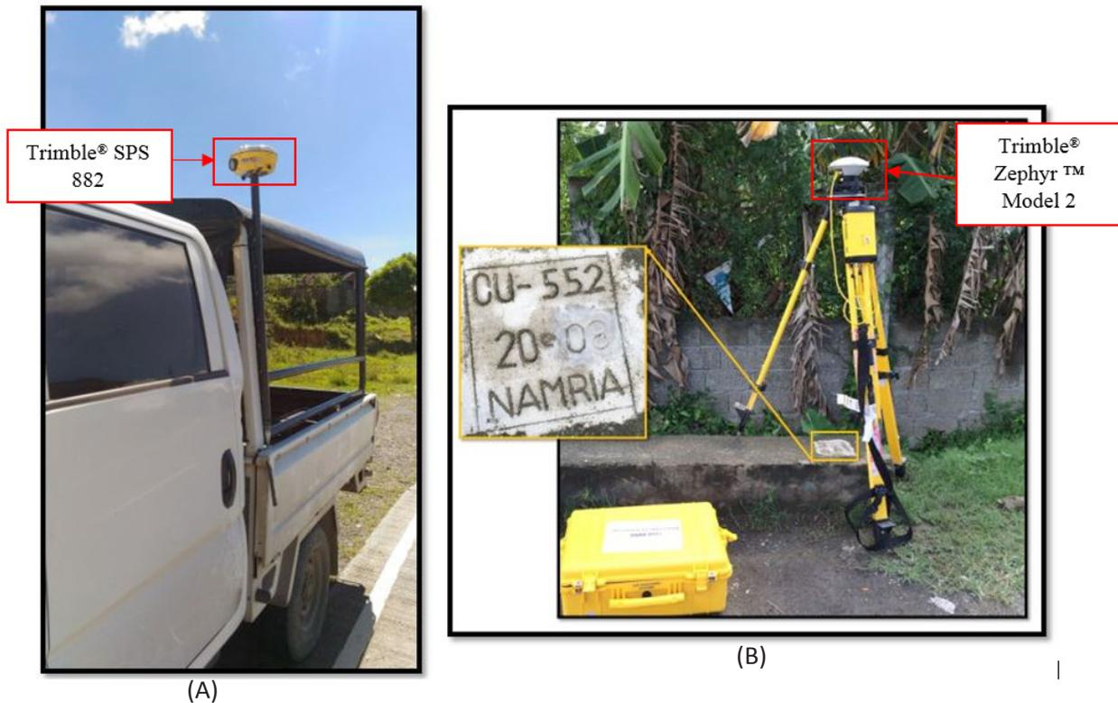
Figure 40. (A) Setup of Trimble® SPS 882 attached to a vehicle and (B) Setting up of GNSS base station at CU-552
