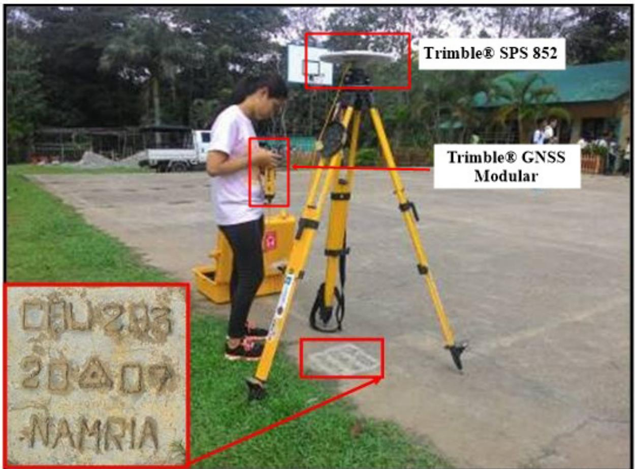
Figure 32. GNSS receiver set-up, Trimble® SPS 852, at CBU-293 in front of Cantabaco National High School in Brgy. Cantabaco, Toledo City, Cebu
