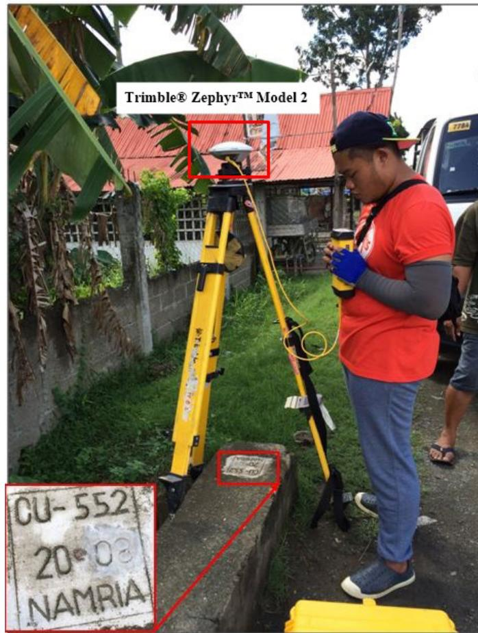
Figure 35. GNSS receiver set-up, Trimble® Zephyr™ Model 2, at CU-552 along the national highway in Brgy. Cantuod, Balamban, Cebu
